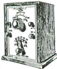
receivers and converts them into double circuit receivers. It consists of a tapped antenna or primary coil and a rotor coil of a few turns of wire inductively coupled to the antenna coil. The rotor coil connects to the antenna and ground binding posts of the single circuit receiver. With its use the single circuit receiver is made very selective. Manufactured by the A-C Electrical Mfg. Co., Dayton, Ohio.
