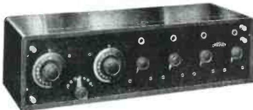
Is a combination tuning element, radio frequency tuned amplifier, audion detector and two-stage audio frequency amplifier, all mounted neatly in one cabinet, simple and easy to tune, has wonderful range and volume of sound. Price.....\$55.00
