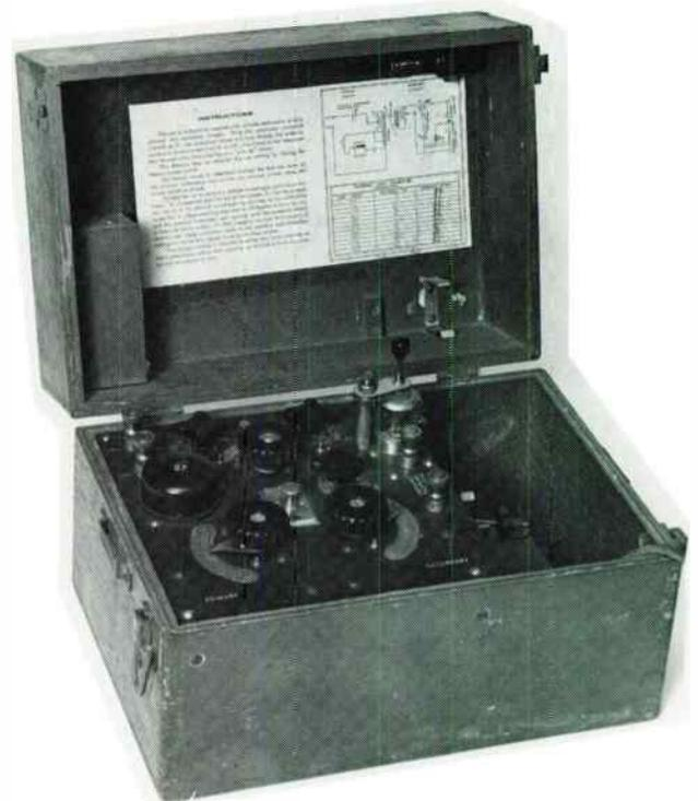
BC14A made by Liberty, identical to the De Forest model. The General Radio version was quite different, with internal buzzer and engraved dial scales.
