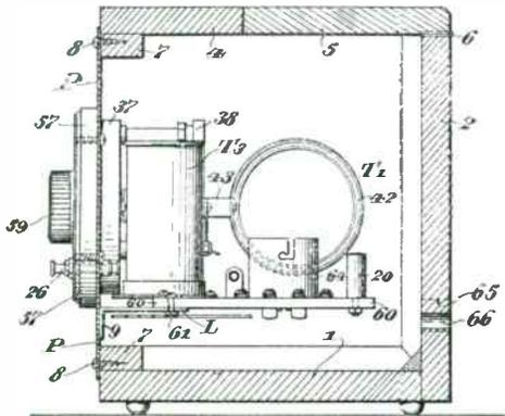
1. The combination with a housing, of a panel structure forming a detachable wall of said housing and comprising a sheet metal panel and a member secured thereto and having substantial extent normal thereto for stiffening said panel substantially throughout its entire extent, and radio receiving apparatus carried by said panel structure within said housing and removable as a unit with said panel structure.
