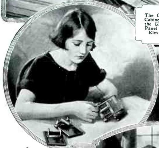
Dext-Fingered Girls Assemble the Book-Type Condensers (Above); the Inventor, at Right, Checks the Blueprints for a New Set, Soon to Be Placed in Quantity Production
