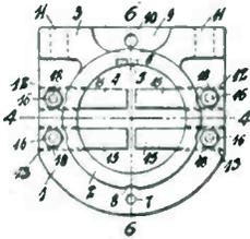
8. A receptacle for audions comprising a tubular socket member having an integral rib projecting from its outer surface and extending longitudinally thereof, said rib having a support engaging surface extending substantially parallel to the axis of the socket, and means providing additional support engaging surface disposed to one side of said rib.
