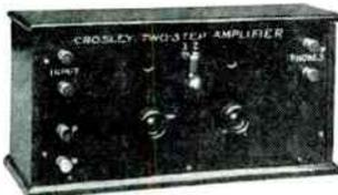
Complete with amplifying transformers, sockets, rheostats, switch, binding posts, etc., mounted on formica panel in mahogany finished cabinet. Price complete as shown in illustration ..... \$25.00
