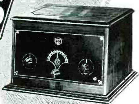
A 2-tube coupled antenna circuit receiver utilizing regenerative detection and one stage A.F. Amplification. "Slow motion" low loss variable condenser. Etched metal panel. Mahogany cabinet. Price includes 2 Radiotron tubes, "Musicone" Headset and Grid Leak.
