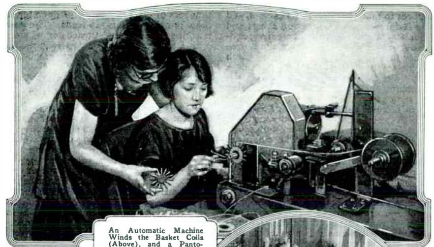
An Automatic Machine Winds the Basket Coils (Above), and a Pantograph Engraver (Below at Left) Marks Panels from a Master Plate
