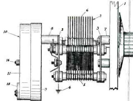
1. In combination with a radio transformer, a shield comprising two parts for supporting, prelocating and protecting said transformer, a condenser, and means for mounting the shield on the condenser.
