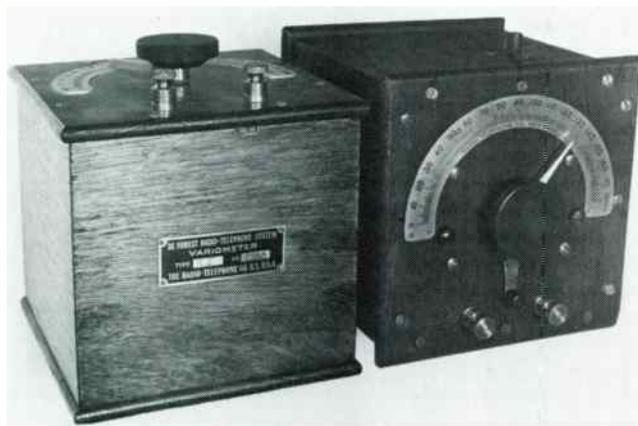
These RJ variometers are quite different internally from the advertised model, using wood rather than hard rubber.
