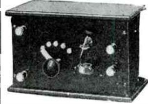
No batteries, tubes, etc., required. Hook it to your aerial and phone. It will tune from two hundred to six hundred meters, bringing in spark, voice, and music, with an average amateur aerial. Complete with battery and interrupter for crystal testing, crystal, etc. Price \$7.00. Phones extra.
