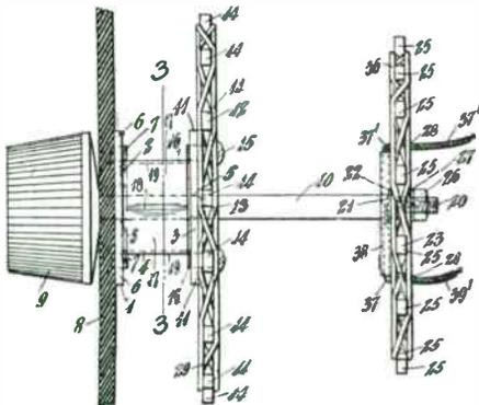
1. In a device of the character described, the combination with relatively movable coils, of a shaft of angular cross-section supporting one of the coils, means fixed to the other coil and having a bearing holding said shaft for non-rotative longitudinal sliding in said bearing, and having edges substantially parallel with said shaft, and a spring formed of a flat sheet bent with members meeting in a ridge bearing along said shaft and with flanges lying along said edges of said bearing means.
