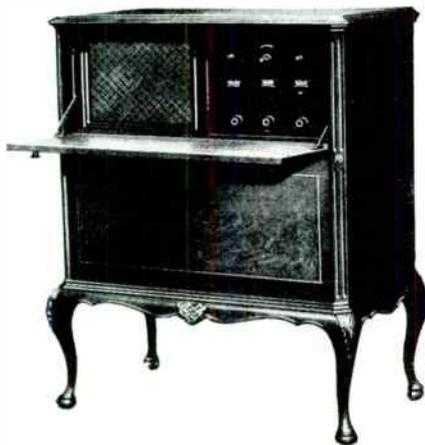
**B-36** Five tubes—199's or 201-A's. Balanced tuned radio frequency. Floor cabinet of choice mahogany woods with rich, two-tone brown finish. Enclosed Federal Speaker. Space for batteries. Without accessories . . . . . **\$250**
