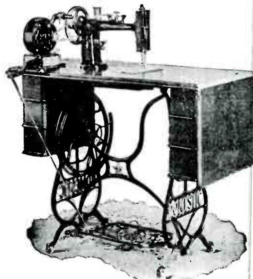
THE KENT ALTERNATING SEWING MACHINE MOTOR.
