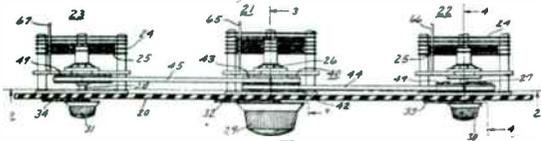
5. An apparatus of the character described comprising a pair of control devices each having a movable element, primary means for moving said elements in unison, a secondary means for moving one or said elements independently of the other, and stop means for a rotatable element adapted upon movement of the primary means to a predetermined position to coordinate said movable elements to a definite normal relationship with respect to one another.
