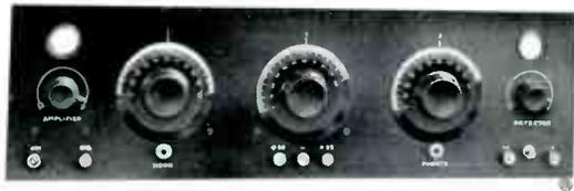
Photograph of panel front of home-made four tube "Neutrodyne" receiver giving full stages of tuned radio frequency amplification, vacuum tube detector, and two stages of audio frequency amplification.
