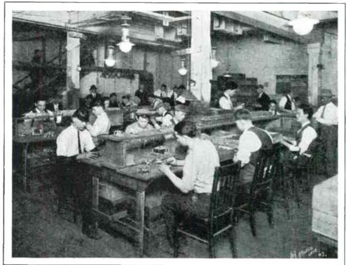
A section of the plant where condensers are assembled
