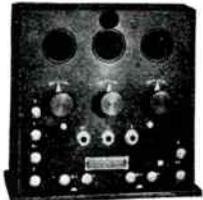
**Detector and Two-Stage Audio Frequency Amplifier.**
