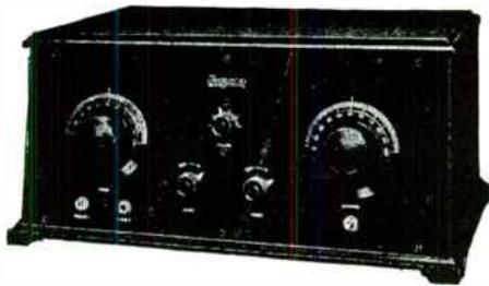
**FERGUSON MODEL FOUR.** Manufactured by J. B. Ferguson, Inc., 41 East 42nd street, New York City. Four tube receiving set employing one stage of balanced tuned radio frequency, non-radiating detector, and two stages of audio frequency. Sloping Bakelite panel. Mahogany finished cabinet with space provided for "B" batteries. List price \$95.00.
