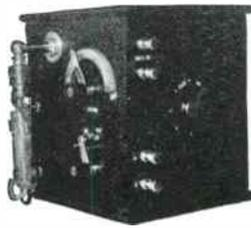
**NEW AUDION AMPLIFIER FOR INCREASING STRENGTH OF RECEIVED SIGNALS 25 TIMES.**
