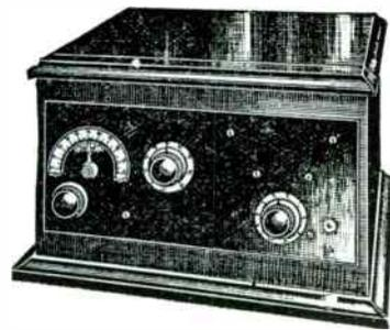
The Crosley 52 Special DeLuxe is a three tube receiver consisting of a genuine Armstrong regenerative detector and two stages of audio frequency amplification. Stations from coast to coast heard on loud speaker by many owners. Tunes through powerful local stations. Cabinet has sloping panel and is large enough to house dry cell batteries. Similar to the Crosley 52 Regular, which sells for \$25.00, except cabinet is larger. Price of the 52 Special DeLuxe, without accessories
