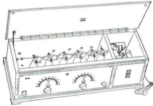
Model 62 B open, showing compact arrangement of AC Tubes, "B" eliminator, etc.
