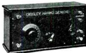
Complete tuner and audion detector assembled on a formica or other high grade dielectric panel, mounted complete in mahogany finish cabinet. Range, 150 to 600 meters, non-regenerative hook-up. Price without battery, tube or phones .....\$16.00
