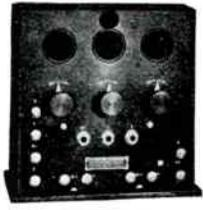
**Detector and Two-Stage Audio Frequency Amplifier.**
