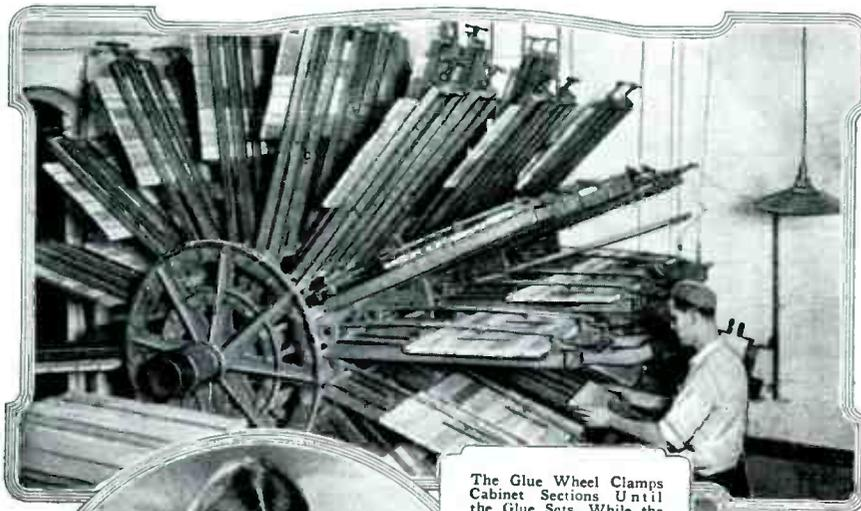
The Glue Wheel Clamps Cabinet Sections Until the Glue Sets. While the Panel Drill, Below, Drills Eleven Holes at Once
