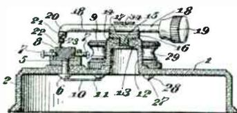
1. In a detector, a member rotatable in but one plane and having a groove in a face thereof, a rod disposed in said groove for longitudinal and rotative movement therein, and a detector element carried by said rod.
