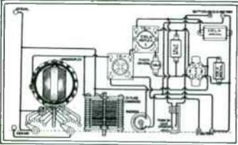
At the top of this page is the usual symbol diagram for the three-tube Erla hookup dealt with in this article. To the left is a pictorial diagram showing the hookup of the single-tube Erla reflex circuit.
