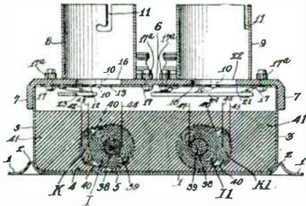
14. An audion coupling unit comprising an enclosing casing, insulating material in said casing, a plurality of audion coupling means embedded in said material and held thereby in predetermined position with respect to each other and to said casing, whereby substantial coupling between said means is prevented.
