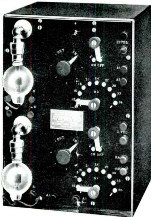
Combination Audion Detector and Single Step Audion Amplifier.
