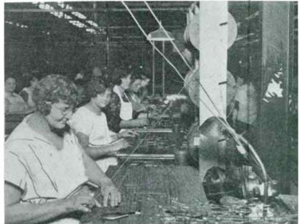
Assembling the wiring bridge in the plant of the Day-Fan Electric Company, Dayton. O. Every wire except grid leaks is placed within this cable
