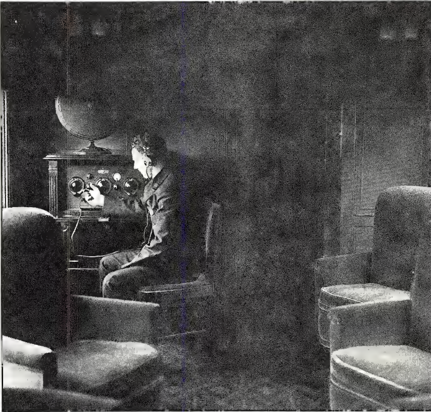
◀ Operator tuning receiver on radio car. Passengers were supplied with earphones if anyone objected to the sound of the loudspeaker.
