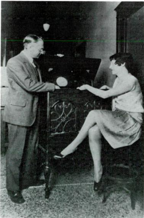
The Rise of Electronic Television: 1930s / An experimental model television receiver (with a mirror to reflect the picture tube, which faces straight up) is tried out by RCA's Vladimir Zworykin—inventor of the iconoscope tube and one of the key figures in the development of electronic television. Courtesy of Group W and Broadcast Pioneers Library.
