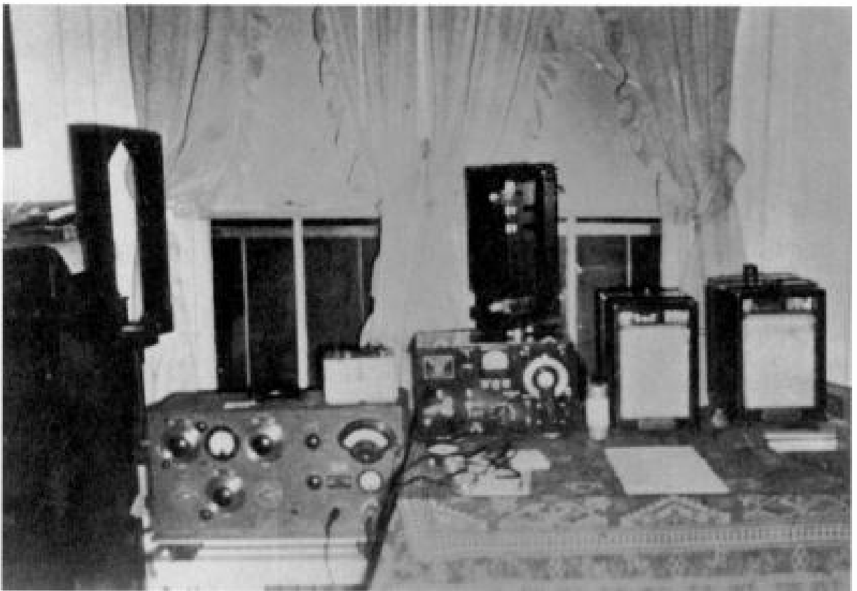
The original "bread-board" 50-watt transmitter of KRLD, Dallas, built and operated by Robert Z. Glass in 1926 and located on the top floor of the Adolphus Hotel. Courtesy Texas/Dallas History and Archives Division, Dallas Public Library, Dallas, Texas
