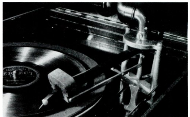
The Vitaphone tone-arm/reproducer of 1920 can play both lateral and vertical-cut records through a simple change in the diaphragm link. (Walter Bellm collection)
