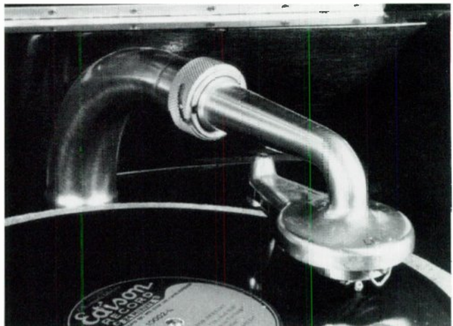
The Edison Diamond Disc reproducer is a refinement of the late-style cylinder reproducers.
