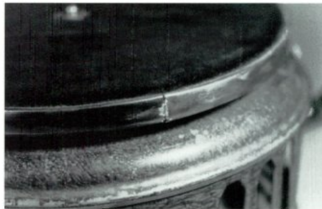
This turntable rim can be removed by melting the solder at the joint.
