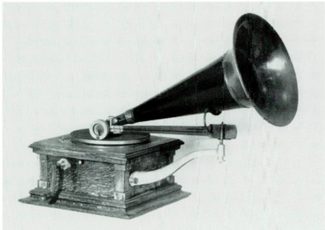
Victor model E "Monarch Junior," 1902-05. This simple double-spring machine was capable of playing five 7" records on one winding. The metal traveling arm on the machine shown here is pictured in catalog illustrations on the model R rather than the E, but surviving examples indicate that the configuration shown here was much more common. Conversely, Victor R's are rarely seen with the metal arm. The Victor E sold for $25.00. (Ernie Bennett collection)
