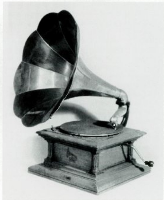
Model BII "Improved Sterling," 1909-11. The BII is an oak double-spring machine with a 10" turntable. Aside from the redesigned cabinet and speed regulator, the BII is very similar to the BI. Note the restyled crank. This crank style is also used on the BY and represents the last of the "typical" Columbia cranks. The BII cost $50.00. (Walter Bellm collection)
