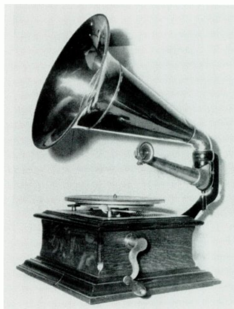
“Concert,” 1904-05. Here is a factory produced rear-mount based on the front-mount design. The case has been simplified and has the late style decal. The price was increased to $35.00. (Robert Adams collection. Photograph courtesy of Charles Mandrake)
