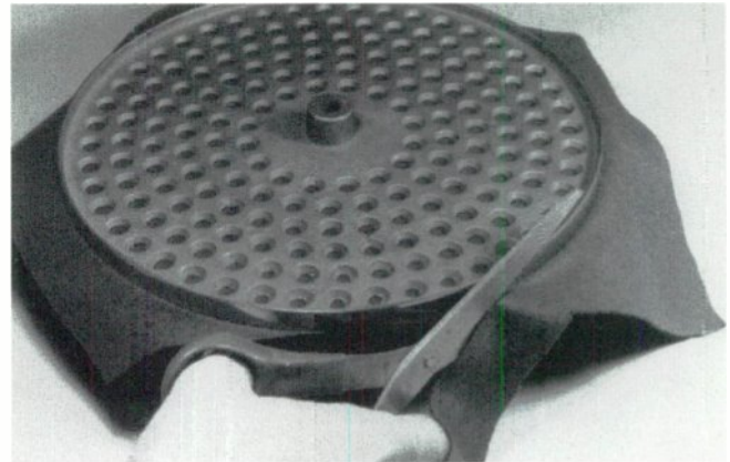
Trimming the new cloth with scissors is easiest to do if you turn the turntable upside down.
