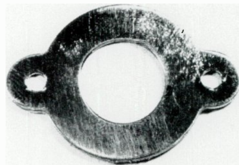
After careful grinding, most of the minor damage is gone.
