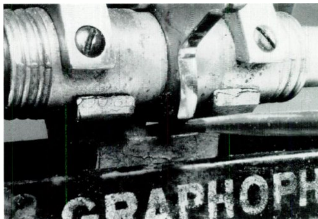
The screwdriver is inserted between the lift lever and the half-nut in order to push the half-nut down and out of the way.
