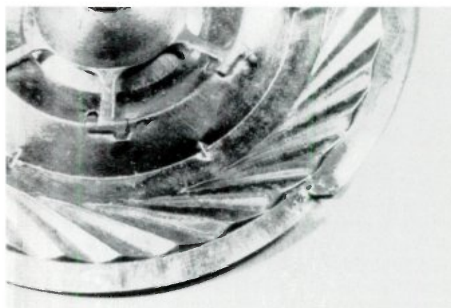
Creases on the edge of an aluminum diaphragm must be repaired for good results.
