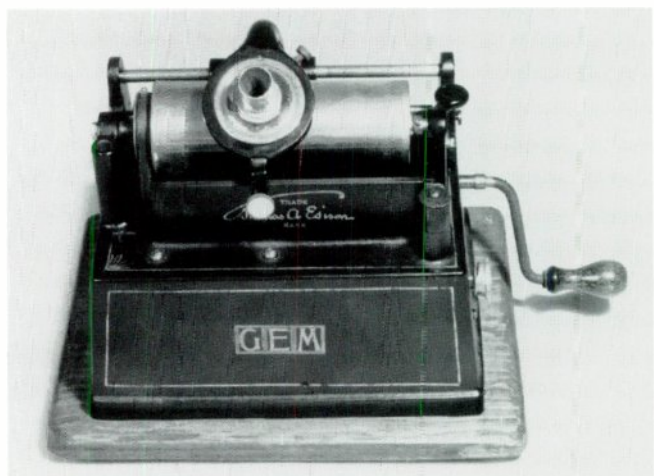
"Gem" model B, 1905-08. The model B has a restyled motor and a permanently attached crank. The machine shown here has a socket on the left-hand end of the casting which accepts the one-piece crane introduced in 1907. Earlier Bs do not have this socket. The Gem was still priced at $10.00. (Author's collection)
