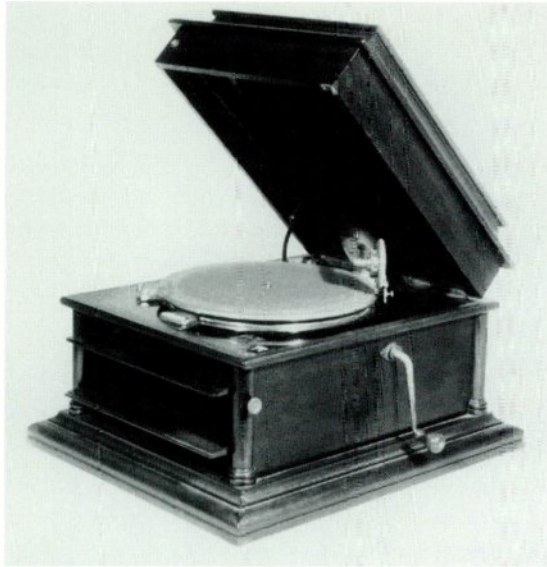
Grafonola "Favorite," 1911-25. Early internal horn models had double doors similar to those used on the Victor Victrola, but already in 1912, this was changed to the characteristic louver design seen on all subsequent Grafonolas. The Favorite cost $50.00 when first introduced in 1911. It has a 12" turntable, triple-spring motor, and a mahogany cabinet. (Walter Bellm collection)
