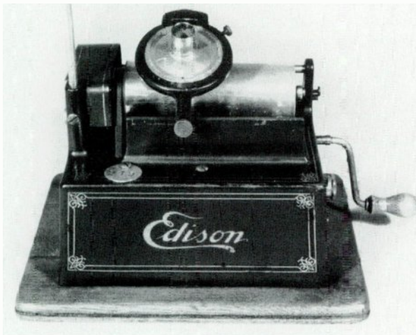
"Idelia," 1907-12. The mahogany Idelia, a glorified Triumph, appeared in four variations between 1907 and 1912. Usually, these have oxidized hardware, but the machine shown here is gold-plated. This very early model, equipped with an endgate, originally had a slanted reproducer carriage, but 2/4-minute gearing and a large carriage have been added. The Idelia sold for $125.00 with an oxidized crane and 11-panel flower horn. The model D1 from 1908 is very similar, but does not have the endgate. The model D2 from 1909 features a metal Cygnet horn, and the late-style model E from 1910 has a horizontal carriage and was equipped with a mahogany Music Master Cygnet horn.
