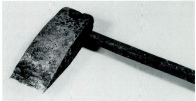
A soldering iron like this is heated in a gas flame until it is red hot. The large head quickly heats up the parts to be joined. Small soldering guns, etc., cannot really do the job properly.
