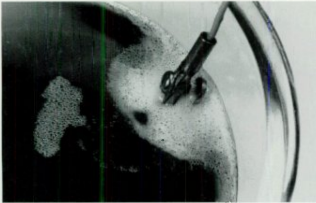
Bubbles at the cathode indicate too much current.
