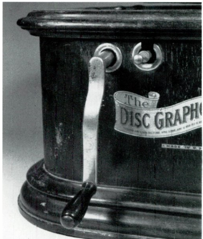
Cranks and speed regulators must usually be removed before the case can be opened. However, this Columbia BD disc machine has a slot so that the speed regulator can remain in place while the machine is being serviced.
