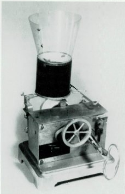
Lioretgraph No. 2, c. 1898. This machine exhibits Lioret's expertise as a clockmaker, although the primitive reproducer and short celluloid horn leave much to be desired acoustically. This is a two-minute machine, although Lioret also produced a four-minute version—the first four-minute machine ever marketed. The special celluloid cylinders that the machine uses were also a Lioret first. (Claes O. Friberg collection)
