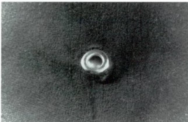
A new eyelet. Small folds in the cloth around the edge of the metal ring are easily smoothed out.
