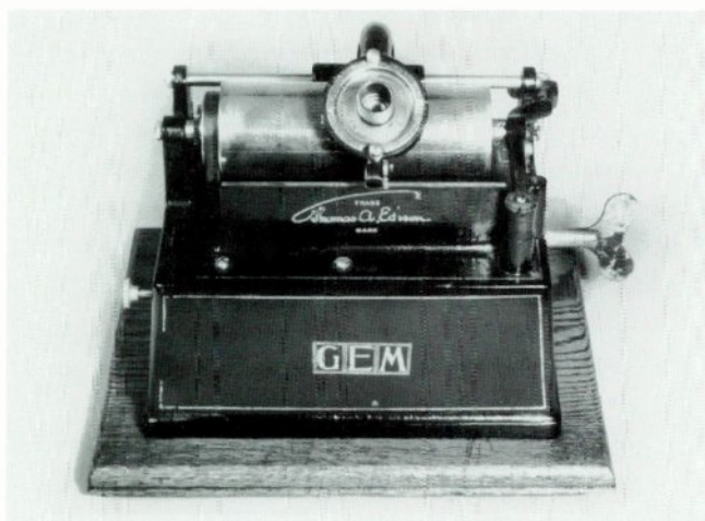
"Gem" model A, 1900-02. The second model A has a different motor configuration, an endgate, and a special "Gem" reproducer. A simple case was provided in place of the drip pan. The improved model A cost $10.00, complete with a simple 10" cone horn. (Bob and Susan Lloyd collection)
