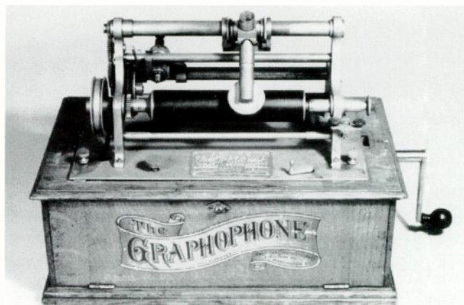
Model K "Standard," 1895. The top casting of this machine was also designed to play the early 6" x 1 5/8" Bell-Tainter cylinders, but comes with a separate Edison mandrel adapter like the model I. However, in contrast to the I, the large pulley wheel has been reduced in size and the machine is equipped with a spring motor. The cabinet front is hinged. An electric version also exists. The model F, introduced the year before, is very similar, but lacks the shaving knife. The machine in the picture is shown playing an early Bell-Tainter cylinder. (Allen Koenigsberg collection)
