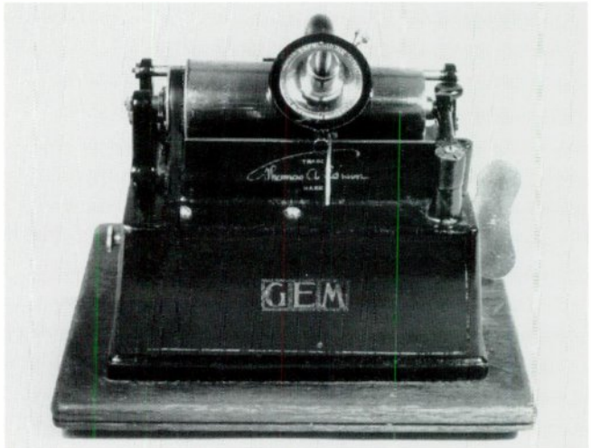
"Gem" model A, 1902-1905. The third and final model A variation features a standard reproducer carriage and a slotted winding shaft which accepts a flat key. (Bob and Susan Lloyd collection)
