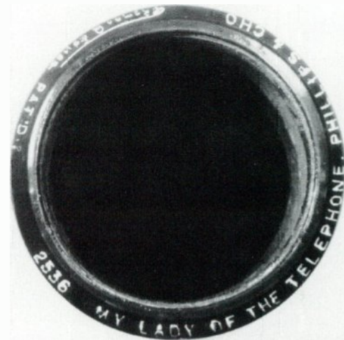
The embossed lettering on Edison Blue Amberol cylinders can be enhanced with a white crayon.
