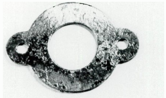
After wire brushing, loose plating and most of the rust has been removed.
