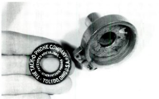
Decorative paper discs inside the reproducer should be preserved at all costs. Replacements can be made on a graphic computer or with pressure-sensitive letters if needed.
