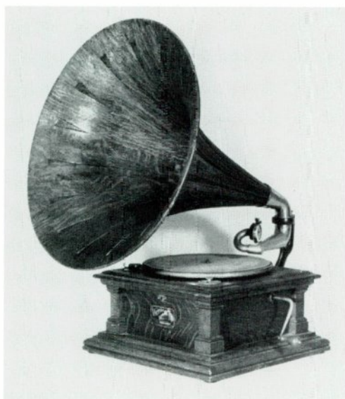
Victor V, 1906-20. The triple-spring Victor V has a 12" turntable, like its predecessor, the model D. The standard issue black flower horn is 26" long, but this model is usually found with the optional oak horn, which added $15.00 to the initial price of $60.00. (Ernie Bennett collection)
