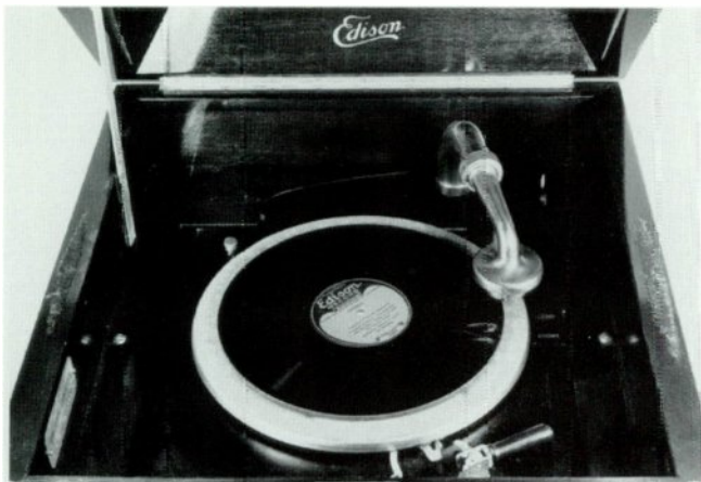
The Edison Diamond Disc phonograph also has a feedscrew. (Ernie Bennett collection)
