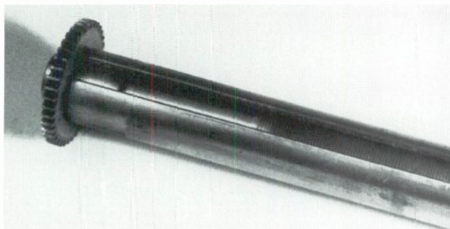
The feedscrew threads are much finer on Edison Homes, Triumphs, etc.
