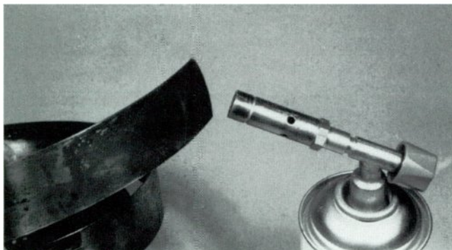
Two or three inches of spring are annealed by heating the end with a propane torch.
