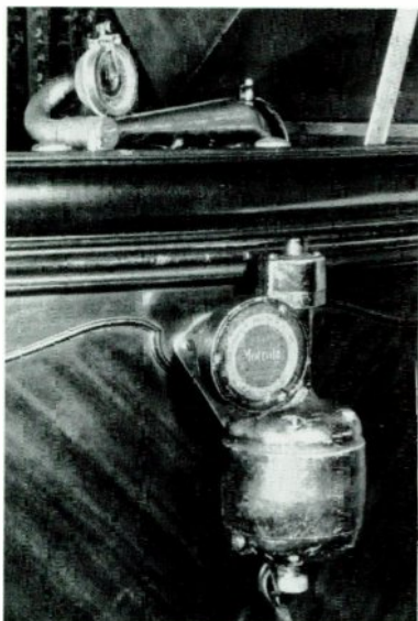
Bristolphon model L, c. 1925. The Bristolphon, made by the Bristol Co. of Waterbury, Conn., is an attachment for converting an acoustic machine into an electric one. The leads are meant to be plugged into a radio. The device simply sits on the motor board and does not require more permanent installation. (Peter Dilg collection)
