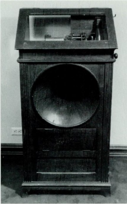
Regina Hexaphone, 1908-21. The Regina Music Box Co. made about 8000 of these machines in four very similar models: style 101, style 102, style 103, and style 104. The one shown here is a style 102, built between 1911-15. The Hexaphone can play any one of six four-minute cylinders, hence the name. Normally, the Hexaphone has a top gallery, but this is missing from the machine in the photo. (Ernie Bennett collection)
