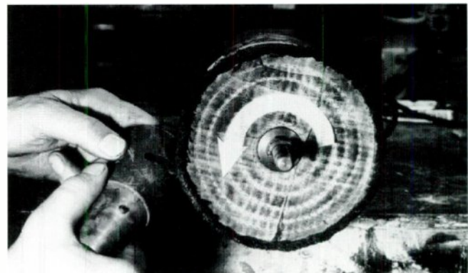
Make sure that the buffing (or grinding) wheel pushes parts in the direction of the floor and doesn't fling them in your face!
