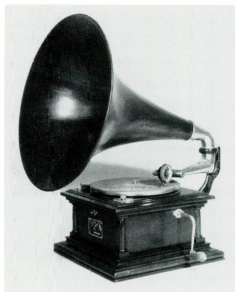
Victor IV, 1906-20. The Victor IV is a restyled Monarch Special with a mahogany cabinet and powerful double-spring motor capable of playing six 10" records per winding. The basic machine cost $50.00. The optional mahogany horn (shown) cost an additional $10.00. The standard-issue black flower horn is 24" long. (Author's collection)
