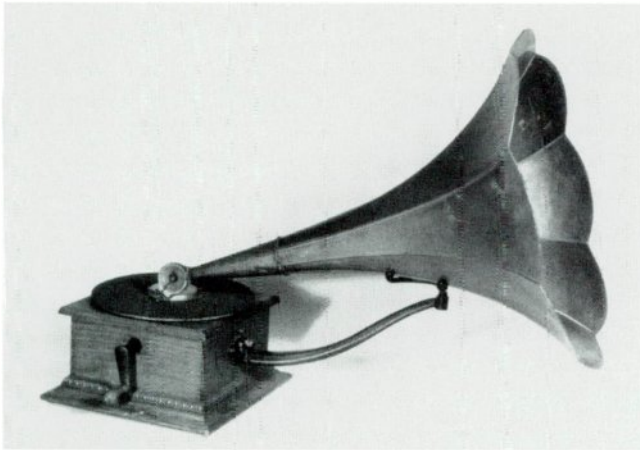
Aretino, 1906-09. The Aretino has a huge 3" hub in the center, a bit too large to be considered a spindle. The Aretino front-mount, as well as its cousin, the Busy Bee Grand, has no traveling arm. Instead, the horn is stuck into a socket on the special cast pot-metal reproducer. The motor is of very simple single-spring construction—so simple in fact, the crank turns as the record plays. The horn is a light, transparent green. (Ernie Bennett collection)
