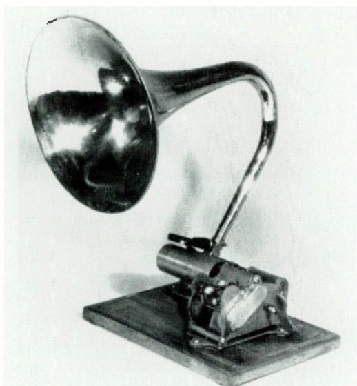
Pathé "Coq" No. 25, 1898-1906. One of the first of a long line of Pathé cylinder machines. The horn is known as a "cor de chasse." (Ernie Bennett collection)
