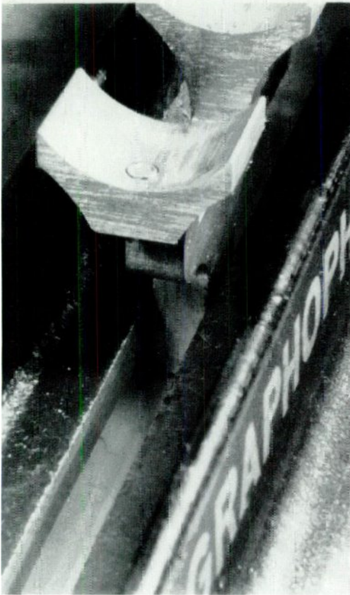
The half-nut bracket must slide freely in the guide groove.
