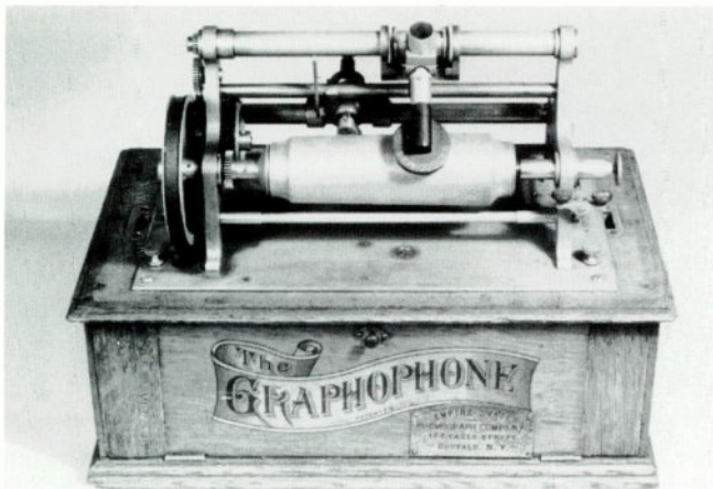
Model K "Standard," 1895. The top casting of this machine was also designed to play the early 6" x 1 5/8" Bell-Tainter cylinders, but comes with a separate Edison mandrel adapter like the model I. However, in contrast to the I, the large pulley wheel has been reduced in size and the machine is equipped with a spring motor. The cabinet front is hinged. An electric version also exists. The model F, introduced the year before, is very similar, but lacks the shaving knife. The machine in the picture is shown playing an early Bell-Tainter cylinder. (Allen Koenigsberg collection)
