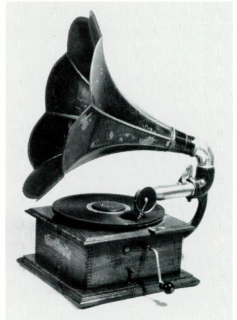
Aretino, 1909-14. After Columbia started to manufacture the Aretino, the machine received a characteristic Columbia motor with a combination on/off/speed control projecting through the front of the case, and a typical Columbia tone-arm. (Ernie Bennett collection)
