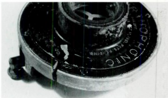
The pot metal back of this Orthophonic reproducer has cracked due to intergranular corrosion. There is no satisfactory way of repairing damage of this kind.
