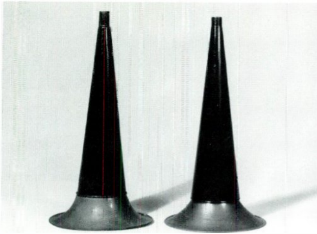
Recognizing reproduction parts will help you determine a machine's value. The "witch's hat" on the left is original, while the one on the right is a recent reproduction. Note the different bell shapes.
