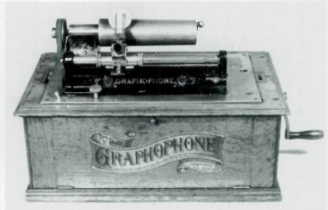
The Commercial Graphophone, 1906-14. This large electric machine replaced the Universal as the standard dictation unit marketed by Columbia. A number of variations exist. The version shown here dates from about 1910 and has a 110V electric motor and special dual-purpose reproducer, which is equipped with both recording and reproducing styli. (Ernie Bennett collection)
