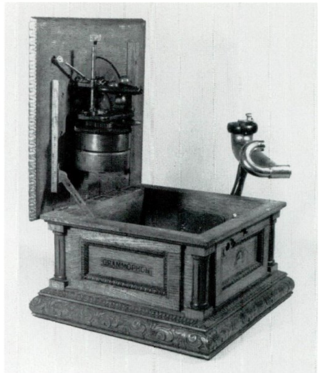
Many disc machines have a hinged lid which provides easy access to the motor.
