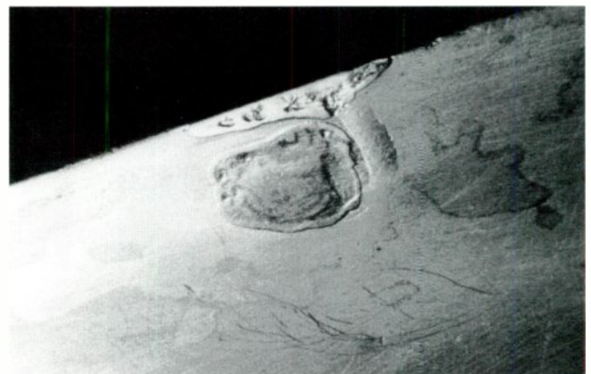
A small nick in a bedplate has been filled with shellac, tinted with nigrosine. Polishing with rottenstone will remove most of the surface imperfections.
