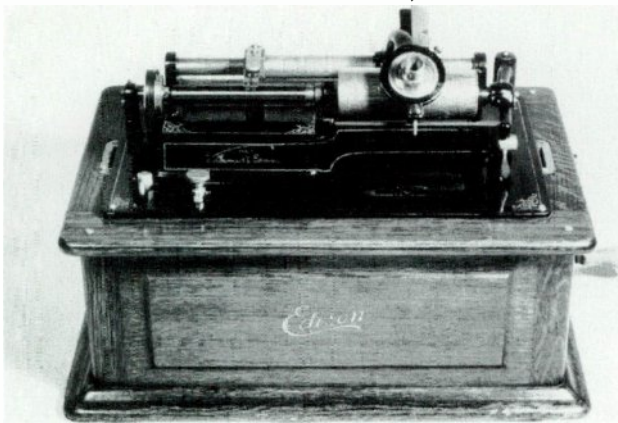
"Triumph" model B, 1906-08. The model B is essentially the same as the model A, but features a restyled case and endgate lock. After 1907, the machine came with a 12-panel 33" black flower horn, as did the model C and D. The model B cost $50.00. The model C (1908, not shown) is essentially a model B without the endgate. (Peter Dilg collection)
