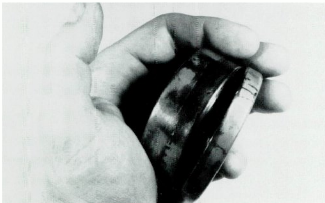
Opening a spring barrel of the "cookie tin" variety.
