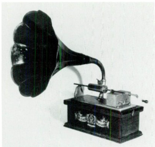
The Wizard Phonograph, c. 1911. Made by the International Phonograph Company of Newark, N.J., the name of both the machine and the mother company are obvious take-offs on Edison, the wizard of Menlo Park and his National Phonograph Co. The machine also turns up occasionally bearing the name "Champion" or "Ellisdon." The case is a simple pine box. The lower portion forms the lid when the machine is not in use. The Wizard was produced for about a year. (Peter Dilg collection)
