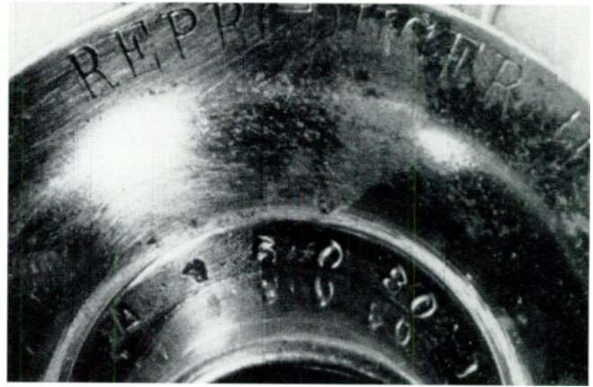
Original Edison reproducers have a serial number at the base of the neck.
