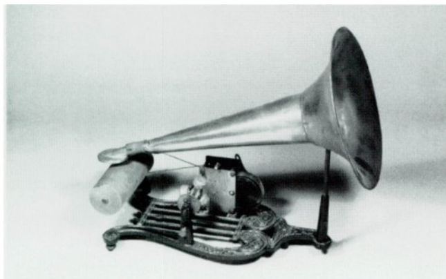
The German-made "Puck" has no feedscrew.
