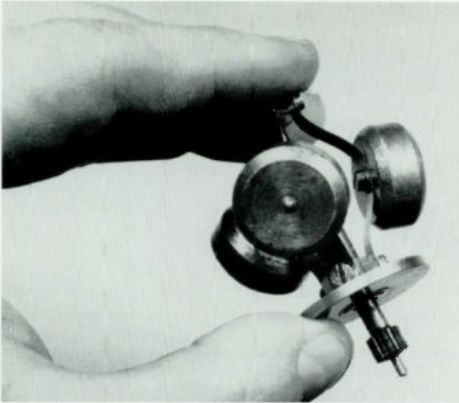
Flex the governor after assembly to make sure the large flange is not binding on the center axle.
