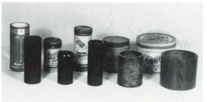
Some common cylinder types: (from left to right) Edison dictation cylinder; standard cylinder; Columbia "20th Century" cylinder; Pathé "Salon" cylinder; "Concert" or "Grand" cylinder
