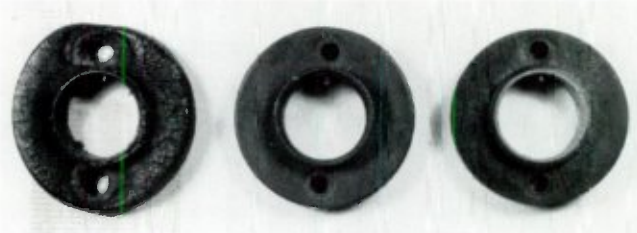
Left: a badly misshapen Exhibition flange. Middle: a usable original flange Right: a modern replacement
