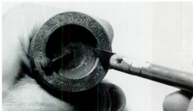
Cutting through the old diaphragm, the first step in disassembly.
