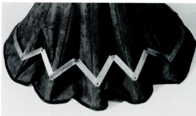
A detail of the folding horn. A nice party trick, but an acoustically poor invention.
