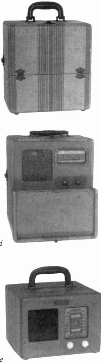
9.3 A sampling of 1939 portables. a , RCA 94BP1 (12-3/8" wide); b , Packard Bell 41 (11-7/8" wide); c , Pilot T1451 (13" wide); d , Sentinel 151BL (12" high), closed and open views; e , Emerson CT275 (8-7/8" wide)
