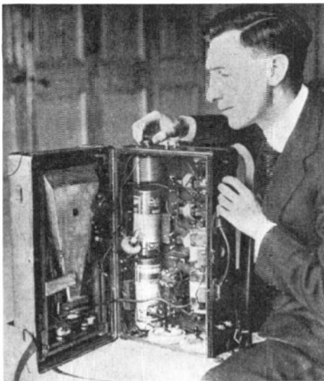
6.5 NBS demonstration portable sets. Above , early NBS portable with horn speaker, 1920; below , Francis Dunmore posing with the NBS "Radio Valise," a completely self-contained portable, ca. 1921
