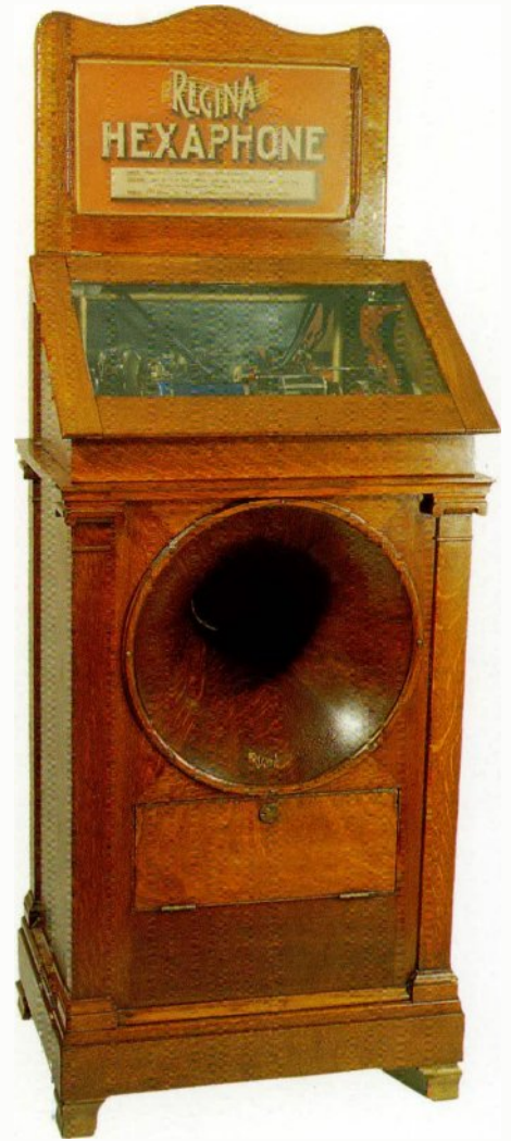
5-53 The Regina Company of Rahway, New Jersey, had been a well-known maker of disc music boxes for many years when they produced this coin-operated "Hexaphone" in 1914. Intended to play (six selective) Edison "Blue Amberol" cylinders, it was reliable and enjoyed considerable popularity. Regina had made coin-op cylinder machines since about 1907, beginning with two-minute models. The firm had cooperated with Columbia to produce a line of "Reginaphones" (music box/disc talking machine combinations). The "Hexaphone" was also something of a joint effort, with reproducers made by the Indestructible Record Company and Music Master wooden horns. Courtesy of Norm and Janyne Smith.
