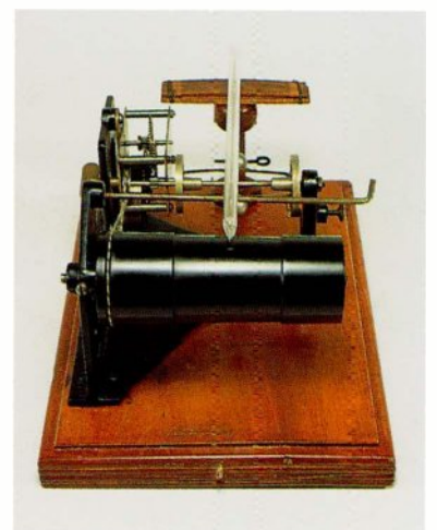
2-45 The final version of the "Echophone" used a mandrel made of gutta-percha. Courtesy of the Howard Hazelcorn Collection.
