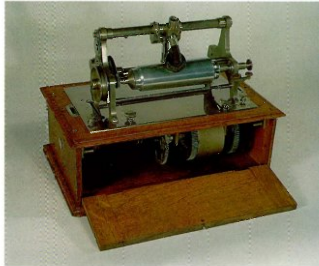
2-29 A very early example of the McDonald-motored Type "K", in which the motor is made of steel rather than brass. Courtesy of the Charles Hummel Collections.
