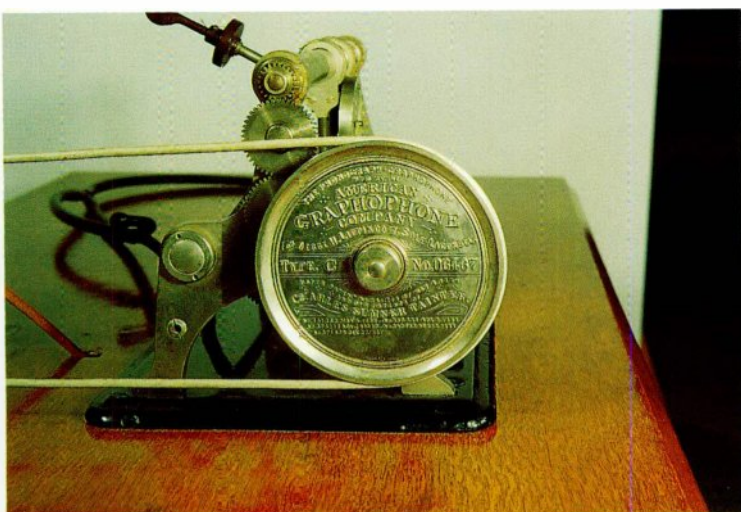
1-22 The pulley plate of the Type "C" treadle Graphophone. Courtesy of the Howard Hazelcorn Collection.
