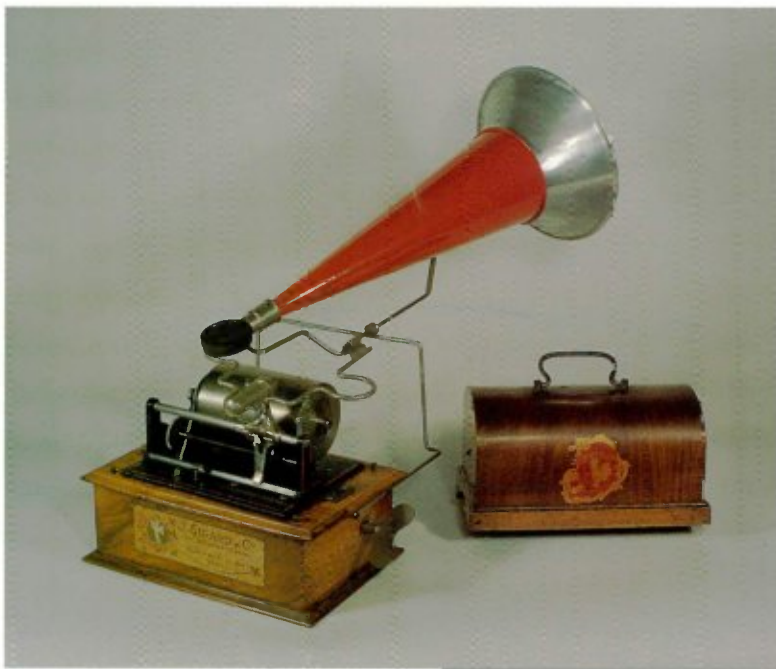
4-9 A Pathé "Coquet" adapted and sold by the French mail-order firm of Girard. As equipped with "Système Vérité", the horn and fixed reproducer "float" above the record, giving ample lateral movement for proper tracking.
