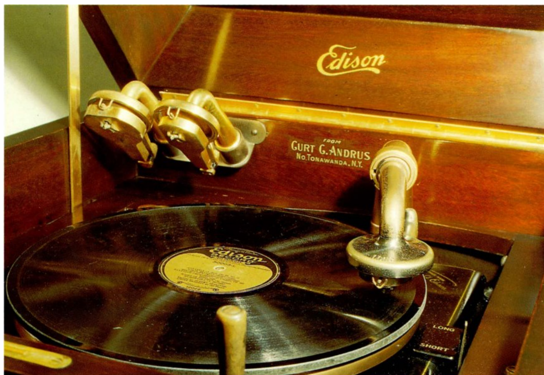
7-6 The "Edison Long Playing Records" were conceptually ahead of their time, but fell short technically. The 12" record shown played for twenty minutes on each side. An "Edisonic" (with larger floating weight to increase volume) and conventional "Diamond Disc" reproducer are shown to the left. Courtesy of George F. Paul.
