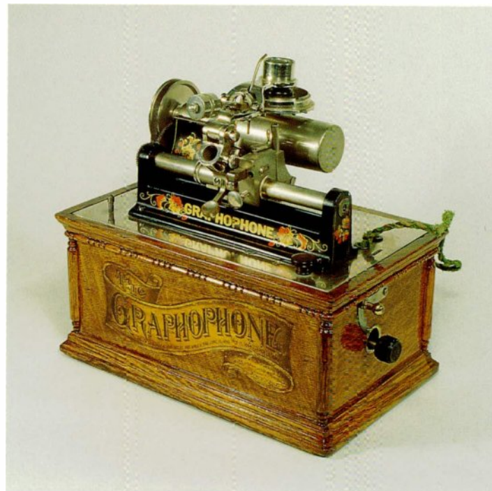
2-92 Lt. Gianni Bettini offered a high-quality line of reproducing/recording attachments for Phonographs and Graphophones. This incandescent-motor Type "AI" Graphophone from 1898 is equipped with a "Bettini Attachment". Courtesy of the Howard Hazelcorn Collection.
