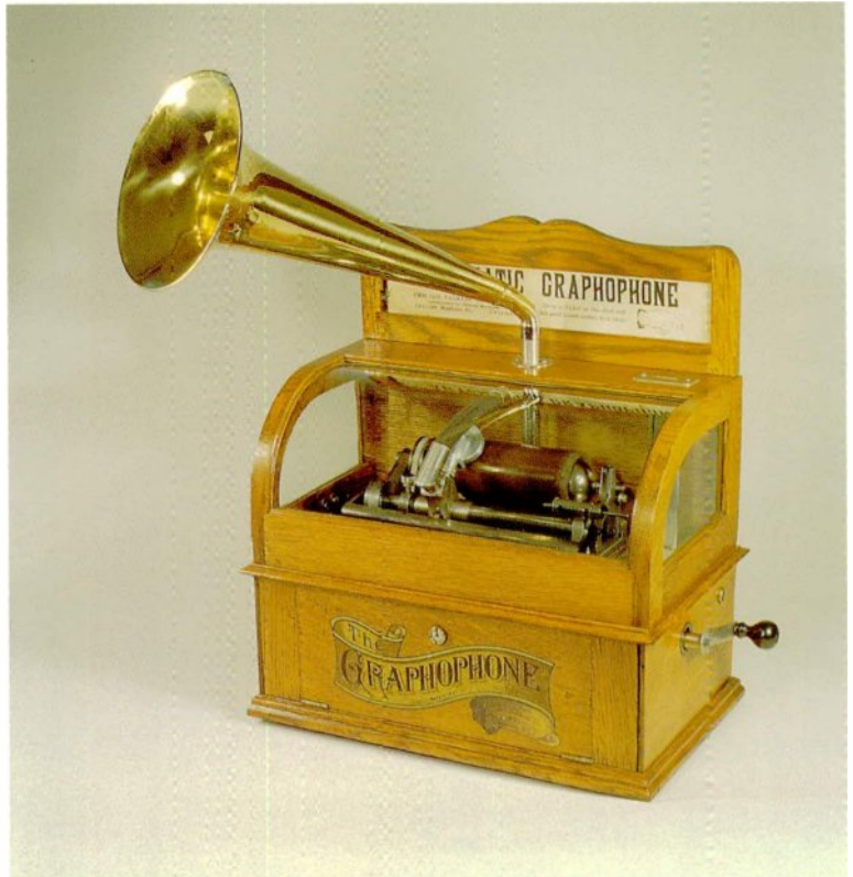
2-50 The industry's first spring-driven coin-slot talking machine: the 1896 coin-operated Type "N" which sold for $50.00. Courtesy of George F. Paul.
