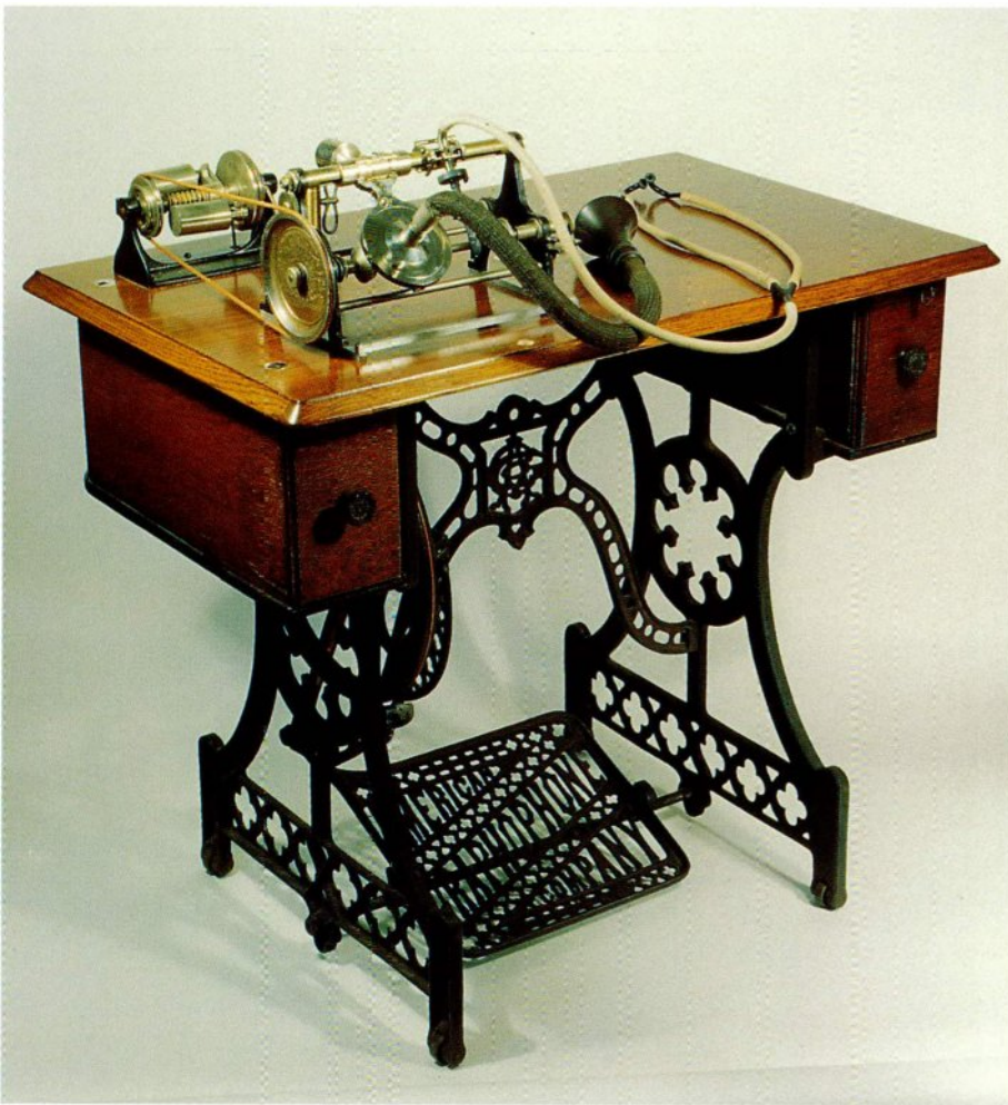
1-18 A Type "B" treadle Graphophone as manufactured from May 1889 to September 1889. Courtesy of Sam Sheena.
