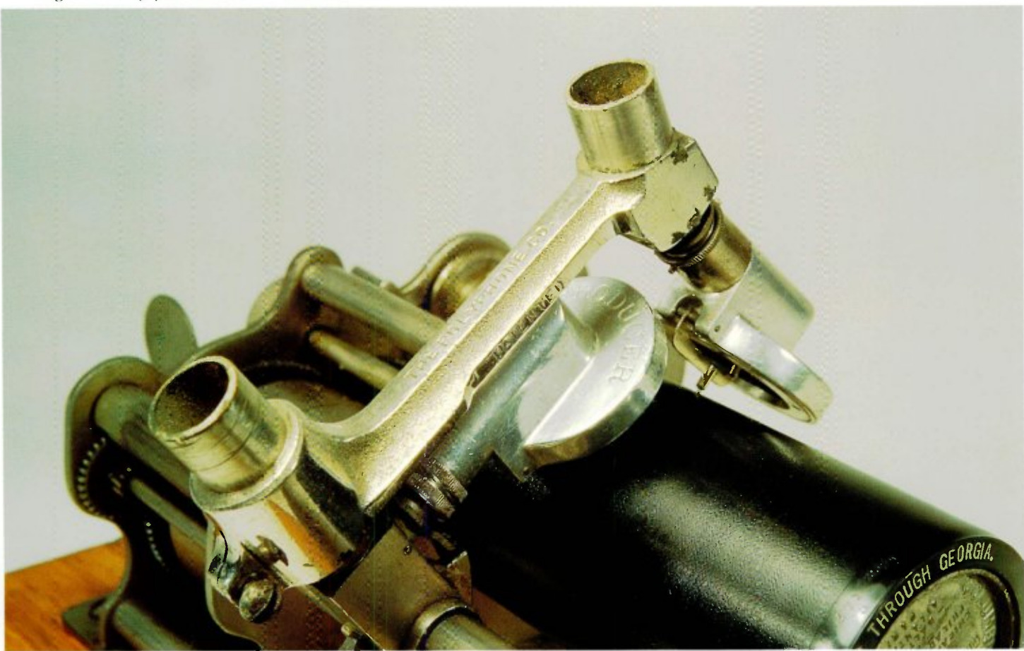
2-91 A close-up of a "Polyphone" attachment mounted to a Columbia "Eagle". Courtesy of the Howard Hazelcorn Collection.
