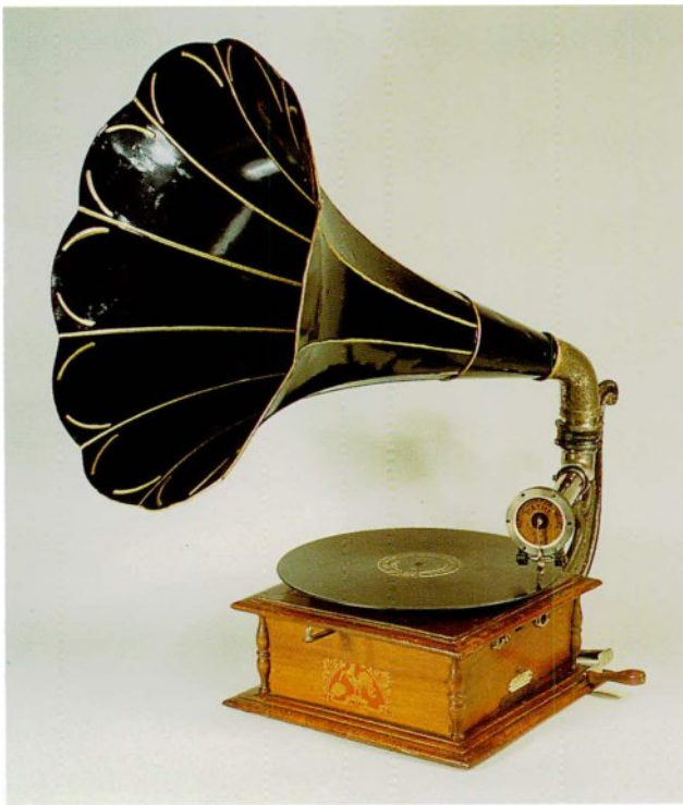
4-110 This Pathé Model "P" disc machine, circa 1907, suggests the earliest design features. The cabinets were often rather low and plain (this one has been dressed-up with pillars), and made of a light-colored walnut. The motor was activated by a "push-pull" lever at the top of the front panel. The decal was the same used on Pathé's cylinder models: depicting a rooster before a cylinder talking machine.
