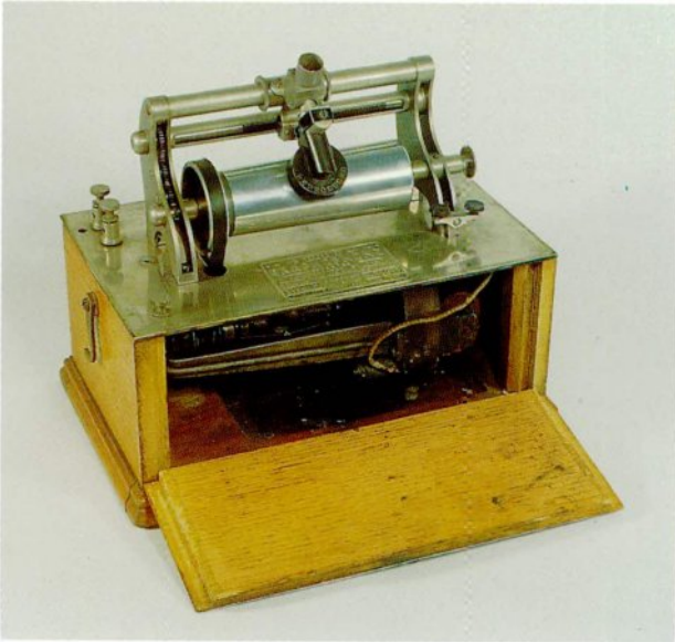
2-23 A Type "H" Graphophone, which is an electric-motored version of the Type "G". Courtesy of the Howard Hazelcorn Collection.
