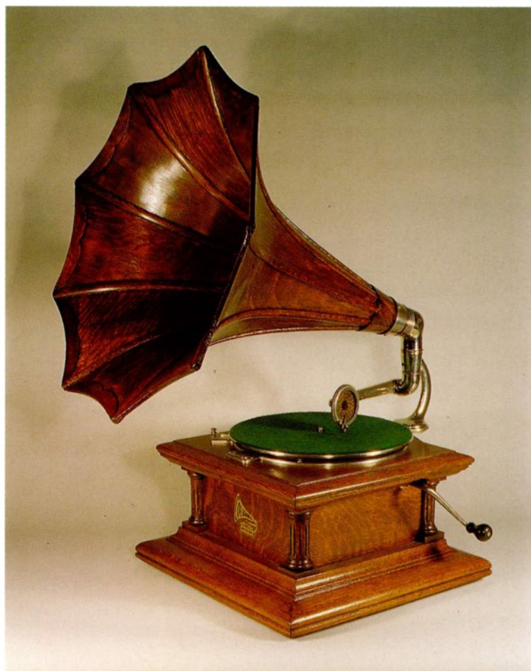
6-37 One of the last of Columbia's external-horn disc talking machines was the "60H", introduced in 1915 (with the model number denoting its price). Columbia placed an unaltered Grafonola motor into a cabinet based on the former "BII", and added an inverted Grafonola tone-arm and wooden horn to create this machine. It is shown here with a panelled rather than smooth wooden horn.
