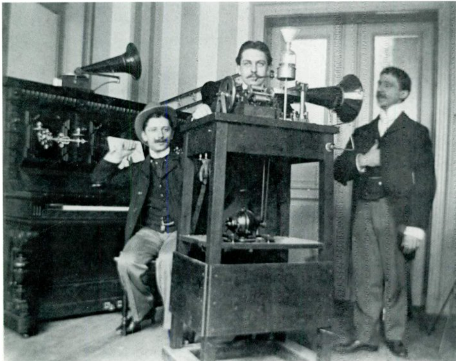
2-102 An 1899 Gramophone recording session in Europe, with engineer William Sinkler Darby at the center. The accompanist and rakishly-posed vocalist are unknown. The zinc master of this performance could be rapidly processed by acid-etching and auditioned on the "Improved Gramophone" atop the piano. Thanks to Raymond Wile, Courtesy of the late Robert Sanders.
