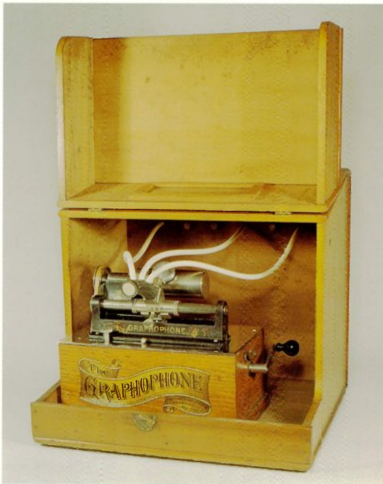
2-75 The interior view shows a Type "A" Graphophone to which the listening-tubes are connected. Courtesy of George F. Paul.
