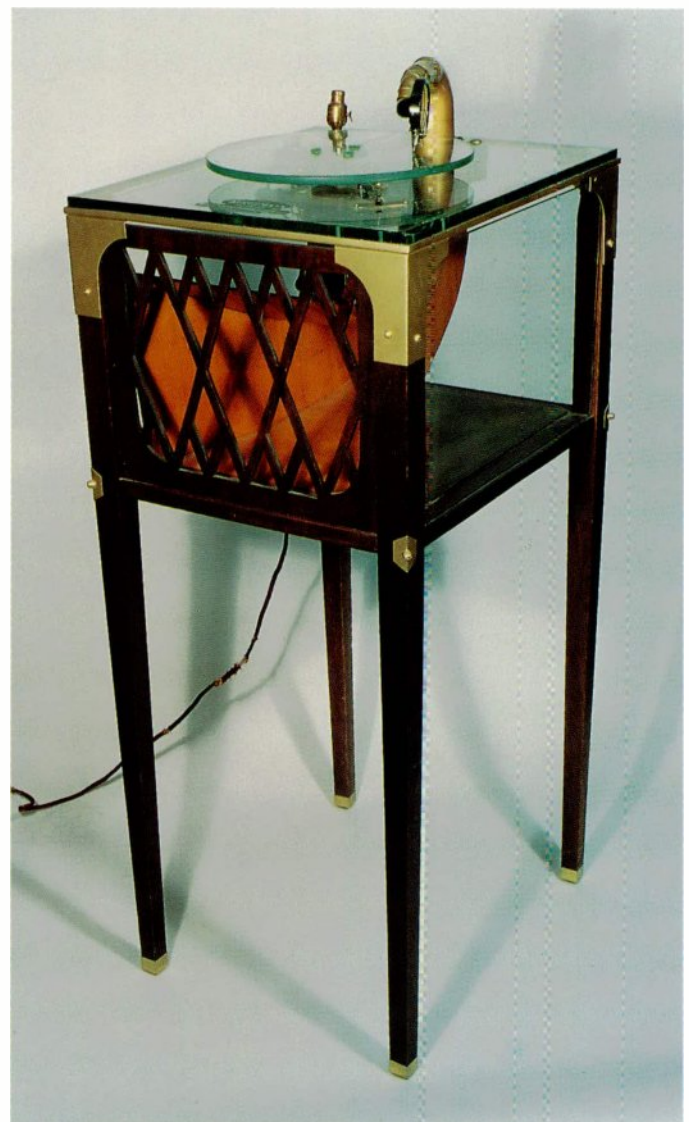
6-6 The "Kurtzmann", produced in Buffalo, New York, was constructed largely of plate glass—even the turntable! Courtesy of Robert and Marilyn Laboda.
