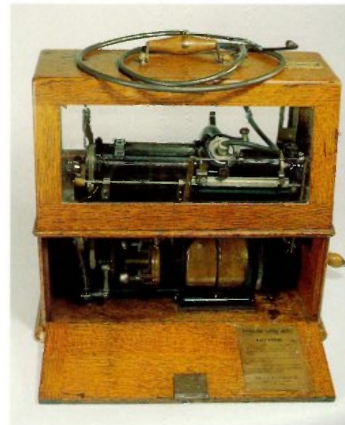
2-37 An Edison Class "M" converted in 1895 to coin- slot operation by the Western Phonograph Company of Chicago. The motor is an Amet. Courtesy of the Charles Hummel Collections.
