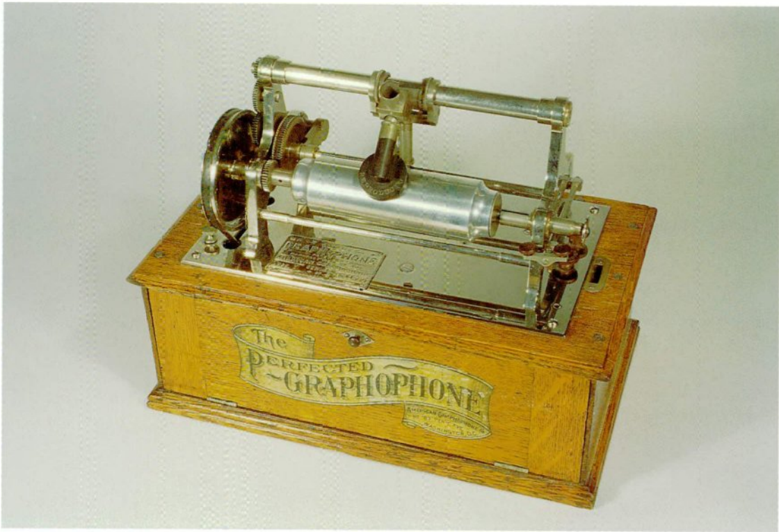
2-24 A Type "I" Graphophone using a 110 volt motor. The upper works is recycled from a Type "C." treadle Graphophone. Courtesy of Sam Sheena.
