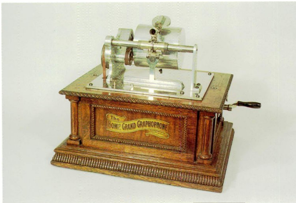
3-90 The Type "AD" Graphophone used a nickeled upper works and a six-spring motor in a Home Grand cabinet. It too was capable of playing both standard and 5" cylinders. The "AD" used two separate belts in the mechanism, and was originally offered for $75.00. Courtesy of the William Kocher Collection.
