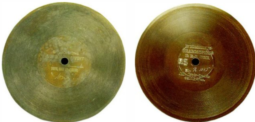
1-40 On the left, a directly-recorded acid-etched zinc 5" Berliner disc. Although some of these were sold (with ink-stamped title information, as in this example), the primary purpose of the zinc disc was to provide a "master" from which multiple copies of the same performance could be created. The "master" was given a thick electroplated skin of metal which, when separated and processed, became the stamper from which celluloid or hard rubber Berliner discs were pressed. On the right, a 5" stamped celluloid Berliner disc of "The Lord's Prayer." Courtesy of George F. Paul.
