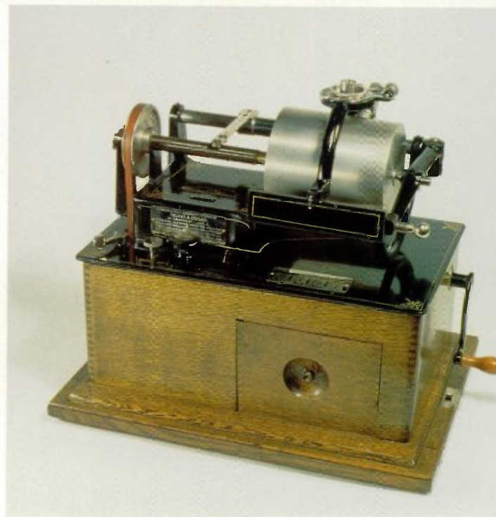
3-26 The Edison "Concert" Phonograph as introduced in February 1899, for $125.00. A 24" brass horn and stand were included.
