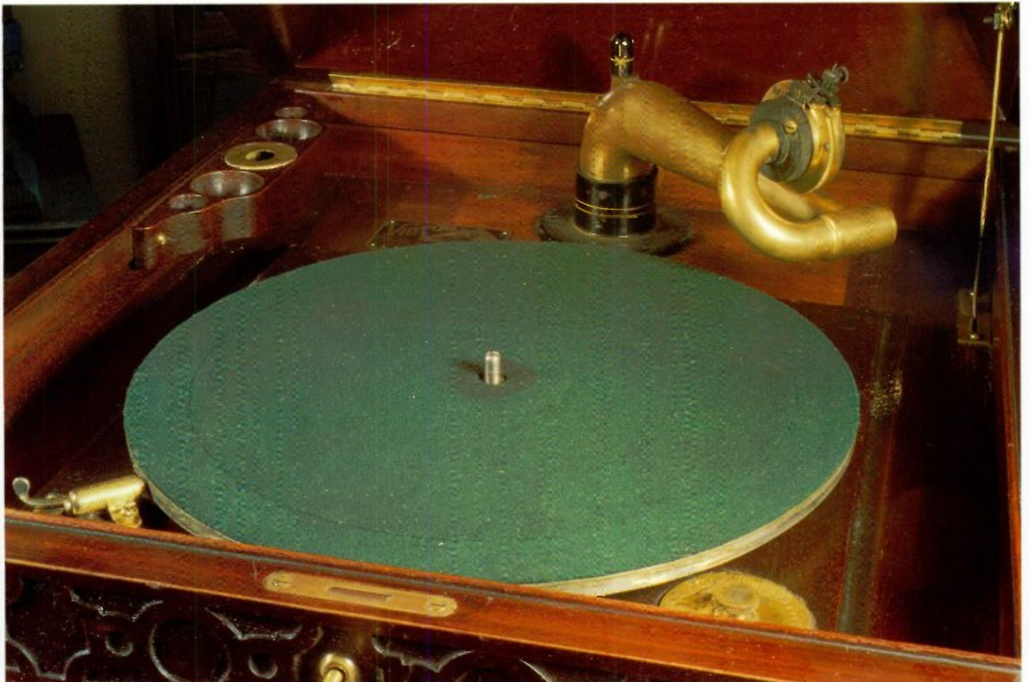
4-91 The interior of the "VTLA/XVI" shows that the mounting board, controls, and motor of a Victor "VF" were dropped in with no modification. Courtesy of Norm and Janyne Smith.
