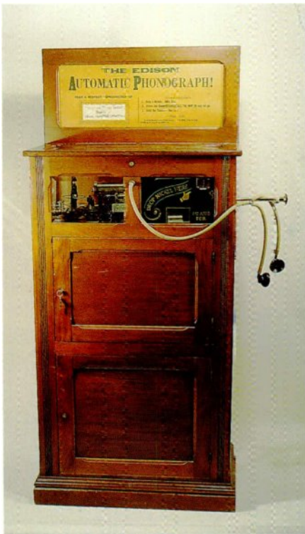
1-31 A Keller-designed coin-slot Phonograph of 1890. The plunger on the right controls the operation with a single action. Courtesy of the Charles Hummel Collections.
