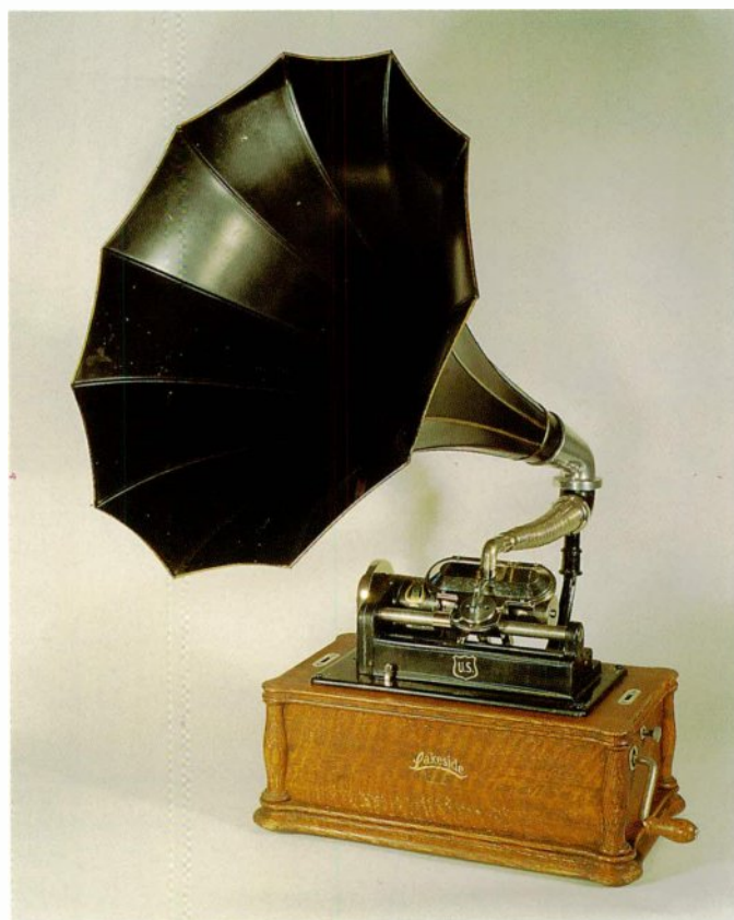
5-26 This "Lakeside" machine, sold by the Montgomery-Ward catalogue house of Chicago was really a U.S. Phonograph Company "Banner" model! ($45.00, circa 1911). Clearly featured are the articulated sound arm and wide, oval reproducer housing. Two separate diaphragms were used to achieve reproduction in either the two- or four-minute format.
