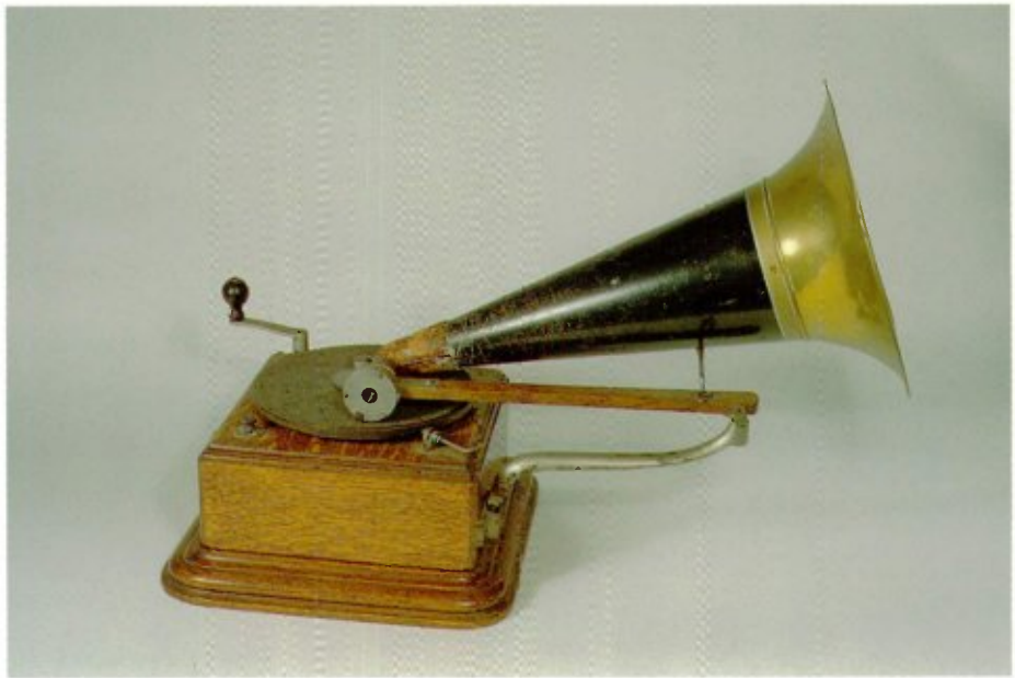
3-40 An unknown-make disc gramophone found in Philadelphia. The support arm bears strong resemblance to a "Vitaphone", but cabinet and motor are unique. Courtesy of the Charles Hummel Collections.
