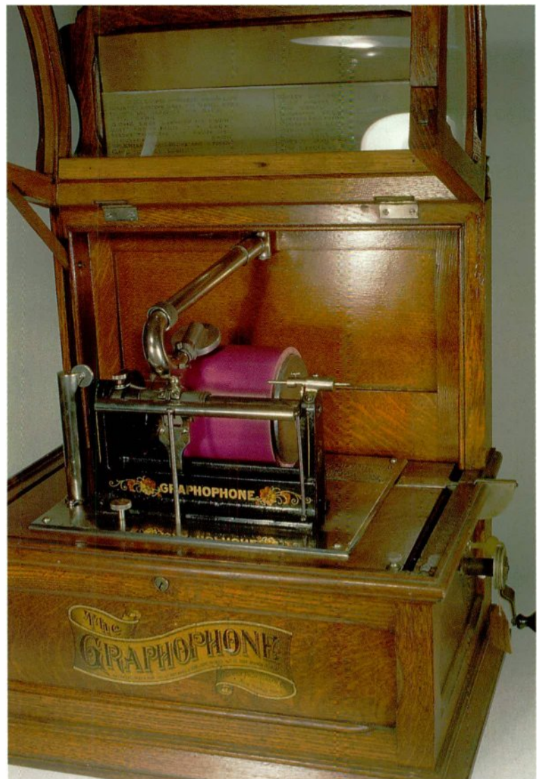
3-17 The Type "SG" ("Slot Grand") was offered in 1899 for $100.00 with a spring-driven motor in a floor-standing cabinet. This close-up shows the coin-slot to the lower right, as well as the upper works based on the "HG". This Type "SG" has a Lambert 5" cylinder in place. Courtesy of Peter N. Dilg, Baldwin Antique Center.
