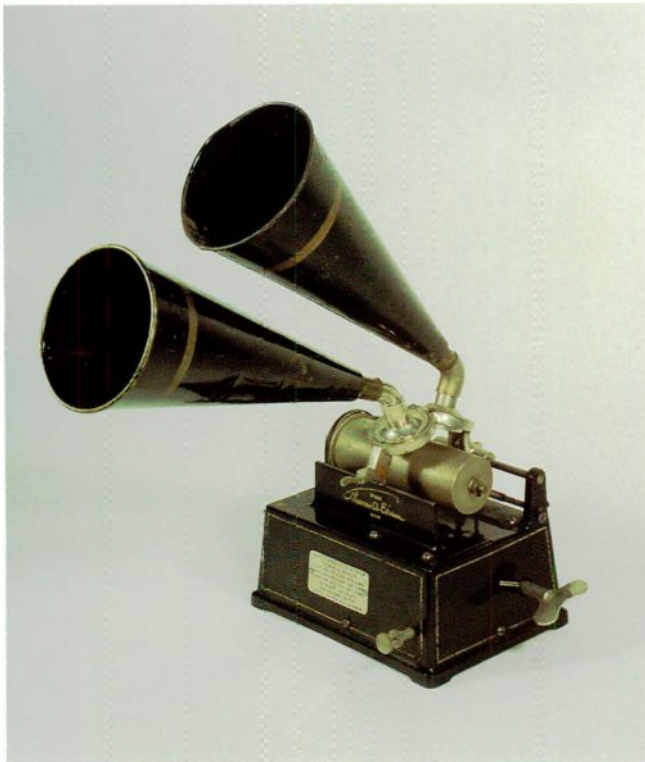
3-33 An early Edison "Gem" with a Polyphone attachment. Courtesy of the Howard Hazelcorn Collection.
