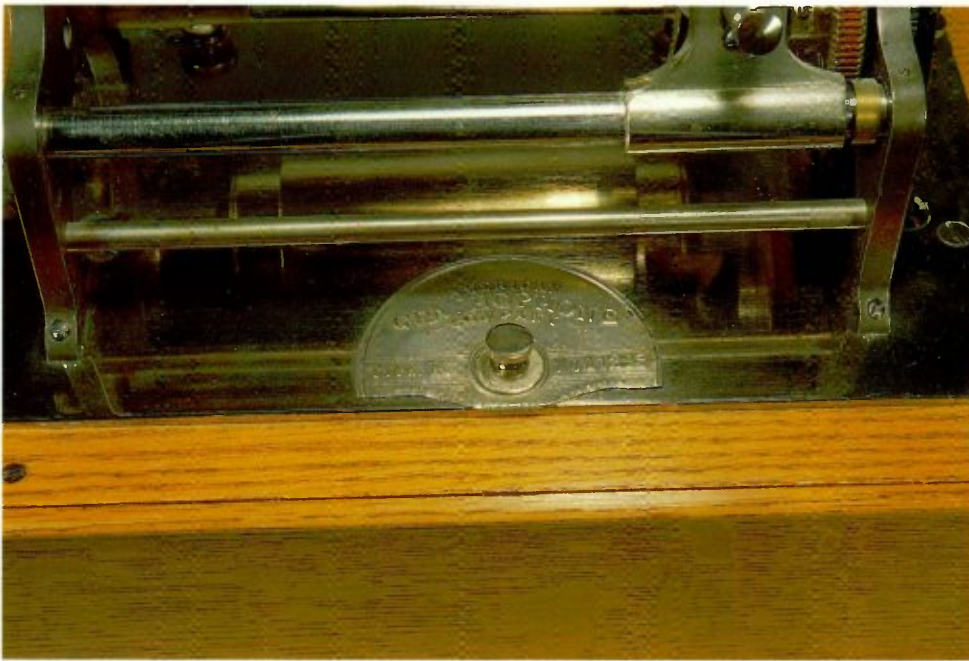
2-28 On spring-motored versions of the Type "K", the upper pulley was smaller, and the large pulley plates were nailed inside the lids or fastened, as in this example, to the rear of the bedplate. Courtesy of Sam Sheena.
