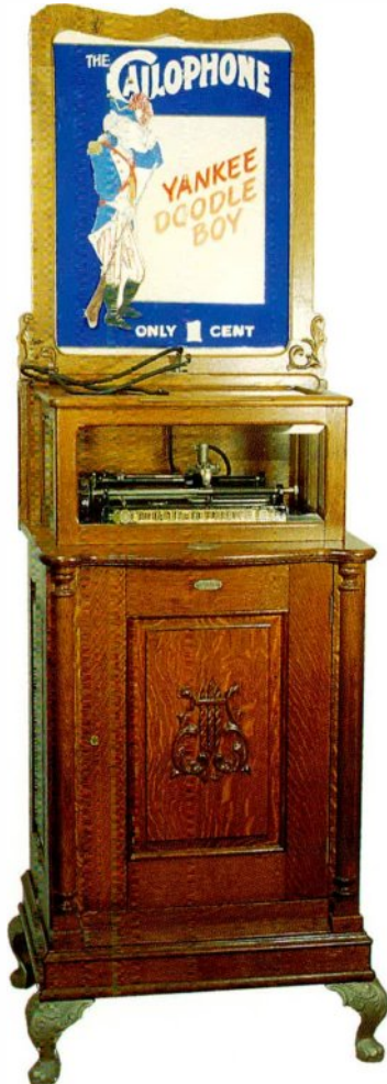
4-116 The "Cailophone" of 1906 employed the works of an Edison Phonograph activated by a coin. The cabinet style reflected a design frequently seen in other coin-op talking machines of the period, including Edison's own line. Courtesy of the Howard Hazelcorn Collection.
