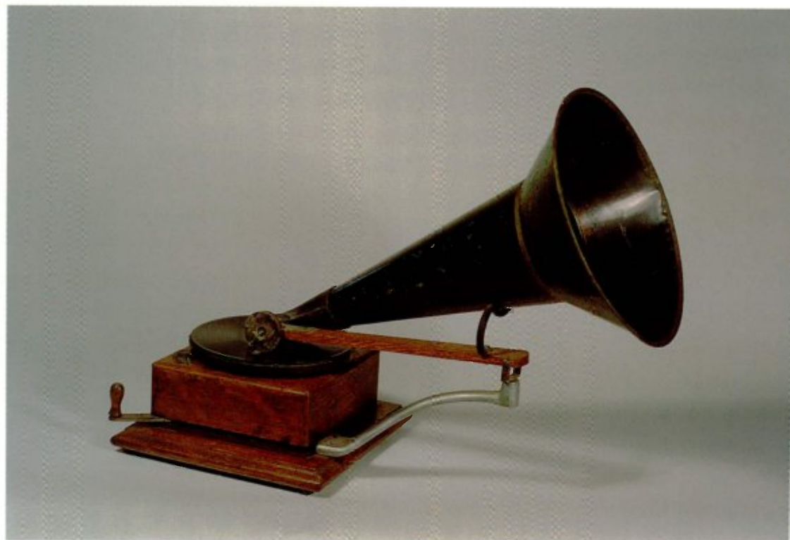
2-65 In early 1897, the lever-wind Berliner mechanism was housed in a square oak cabinet and provided with the new Clark-Johnson soundbox. The price remained $25.00. Courtesy of Robert Adams.
