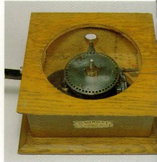
4-21 A close-up of the "Harmony" with the turntable removed shows how the manufacturers, Hawthorne and Sheble, designed it to allow the most economical access to the motor.
