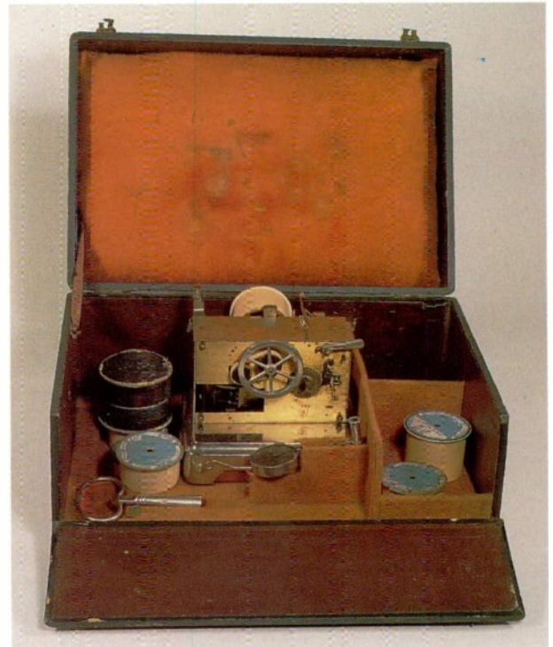
2-41 An 1896 Lioret "No. 2" equipped with a special reproducer for listening-tubes, in its carrying case.
