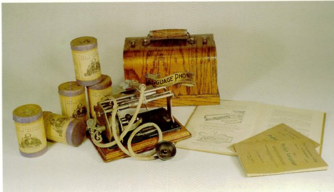
3-122 The versatile Type "Q" was sold as a "Languagephone" to play Rosenthal cylinders developed to teach a variety of languages. This example retains its original instruction books and cylinders. Courtesy of Norm and Janyne Smith.
