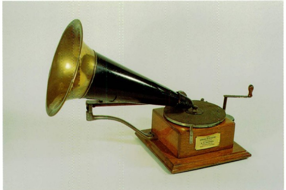
3-53 The "Gramophone" as sold by Eldridge Johnson in the early fall of 1900. The celluloid plate replaces the Berliner decal on the cabinet. The horn on this example (No. 34983) is from a slightly later machine. Courtesy of Dr. Jay Tartell.
