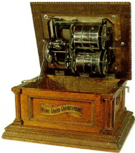
3-52 The nicked six spring motor of the Type "HG" Gramophone.
