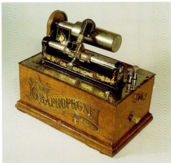
2-60 The Columbia Type "AE", introduced in 1897 for $40.00, was driven by the same type of 2 1/2 volt electric motor used by the Graphophone Company since 1893. Courtesy of Sam Sheena.
