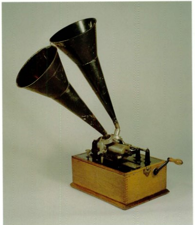
3-23 Polyphone attachments were available for Edison Phonographs in early 1899. This is an Edison "Standard" so equipped. The Polyphone attachments for Edison Phonographs were available separately for $15.00, including two horns. Courtesy of Peter N. Dilg, Baldwin Antique Center.
