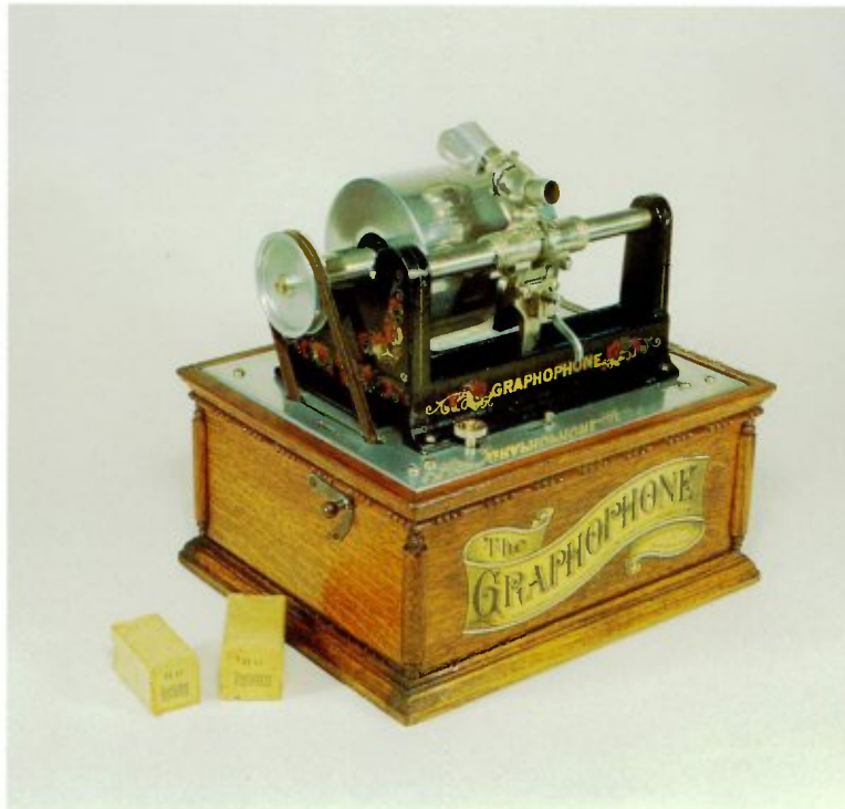
3-37 The 1899 "HG" (Home Grand") Graphophone allowed Columbia to offer a machine to play 5" cylinders for $100.00, underpricing Edison's "Concert" by $25.00. The motor was the same as used in the Type "AT". Courtesy of George F. Paul.
