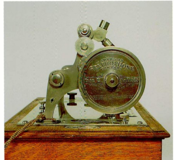
2-26 Close-up of the Type "U" pulley plate. Note that the "North American Phonograph Company", Charles Sumner Tainter's and Jesse Lippincott's names have been effaced. Courtesy of the Charles Hummel Collections.
