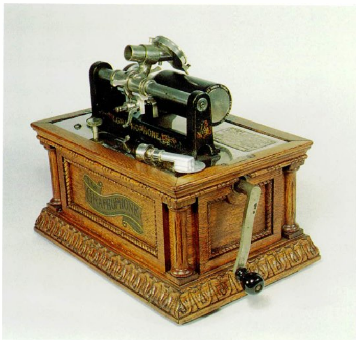
3-97 The "AO" was first offered with a conventional aluminum floating reproducer. Subsequently, an option was available for $5.00 to equip the machine with "...an entirely new form of reproducer, giving greater volume and perfection of tone." This reproducer was inspired by the soundbox used on Disc Graphophones. When sold with this reproducer, this machine was known as the "AW". Courtesy of the Howard Hazelcorn Collection.
