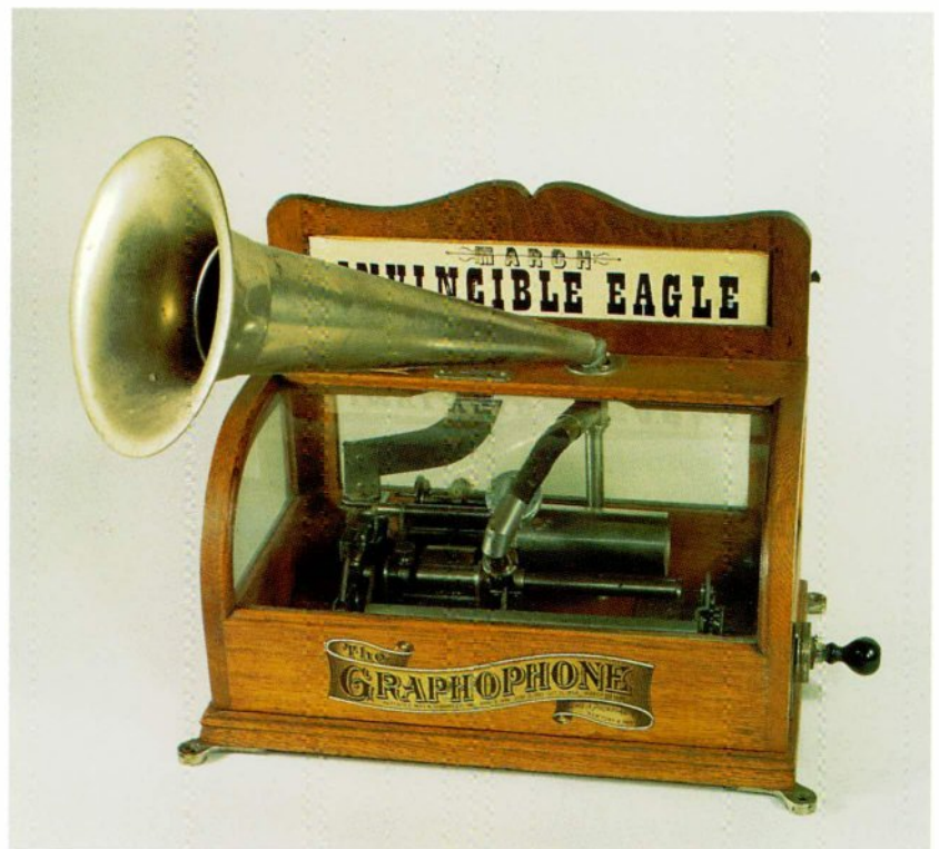
3-14 The Type "BS" Graphophone sold for $20.00 from its introduction in late 1898. Based on the popular Type "B" mechanism, it was carried in Columbia catalogues until 1905. This was the most popular coin-slot in Columbia's history as well as the least-expensive. Courtesy of Allen Koenigsberg.
