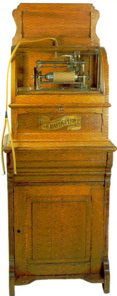
2-39 An 1895 Type "S" coin-slot Graphophone still using the old treadle machine upper works powered by an electric motor. This cabinet design would serve Columbia coin-ops well into the next century. Courtesy of Sam Sheena.
