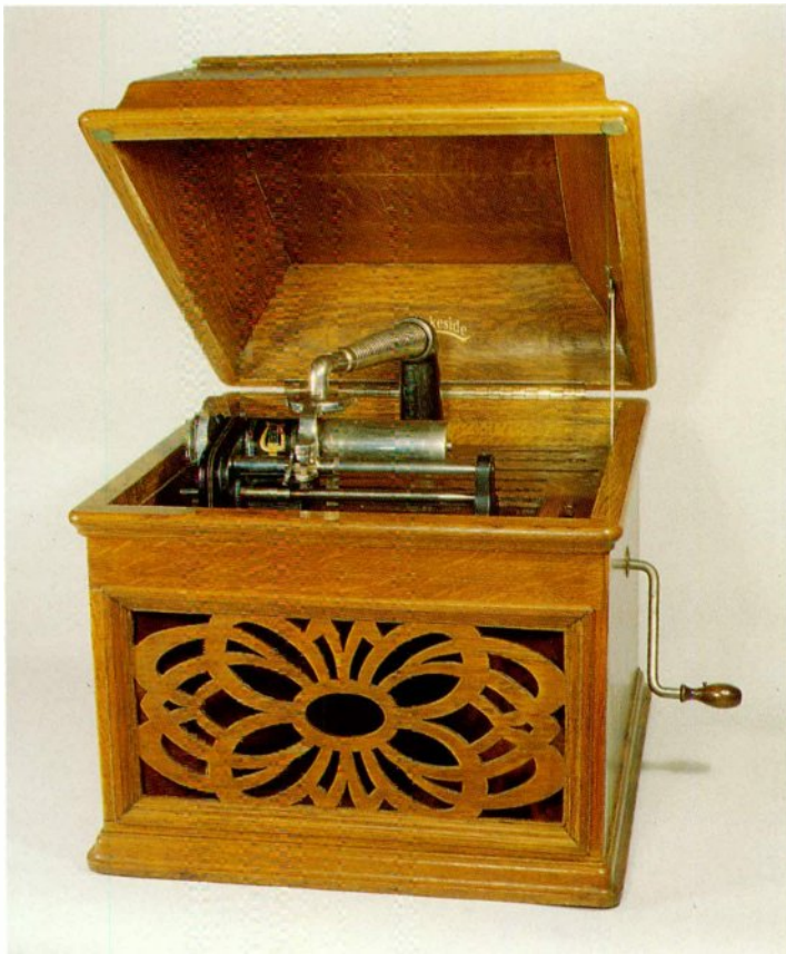
5-29 Another "Lakeside" manufactured by the U.S. Phonograph Company of Cleveland, Ohio. Sold as a U.S. "Royal" ($50.00) it can be found with either a double-diaphragm reproducer or conventional one (shown).
