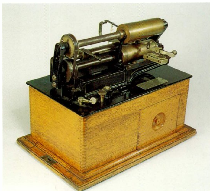
2-3 A cylinder copying machine or “pantograph”. Such machines were used by large manufacturers to create enough copies of popular selections to fill demand. Unscrupulous entrepreneurs often used pantographs to duplicate professional recordings, thus avoiding overhead costs. Pantographs were routinely confiscated when found engaged in illegal duplication, but the period was rife with such activity. This example is composed of a modified Edison Class “M” upper works mounted to a “Spring Motor” mechanism. Courtesy of the Charles Hummel Collections.
