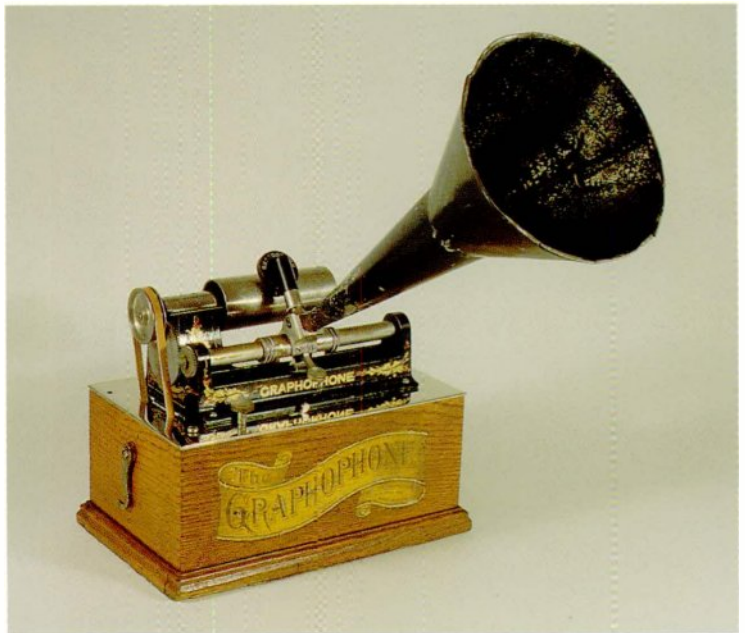
2-49 The Type "A" ("Columbia") of 1896 used a simplified motor and cast-iron upper works to lower the price of a Graphophone to $25.00. Courtesy of George F. Paul.
