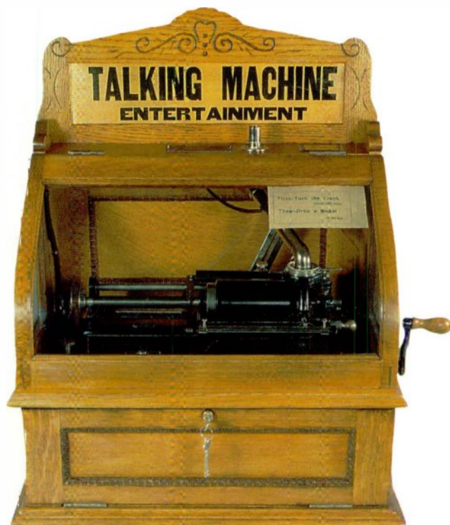
3-16 The 1899 Edison "H" coin-slot Phonograph was based on the "Home" upper works. This was Edison's first spring-driven coin-slot, selling for $50.00. Courtesy of Sam Sheena.
