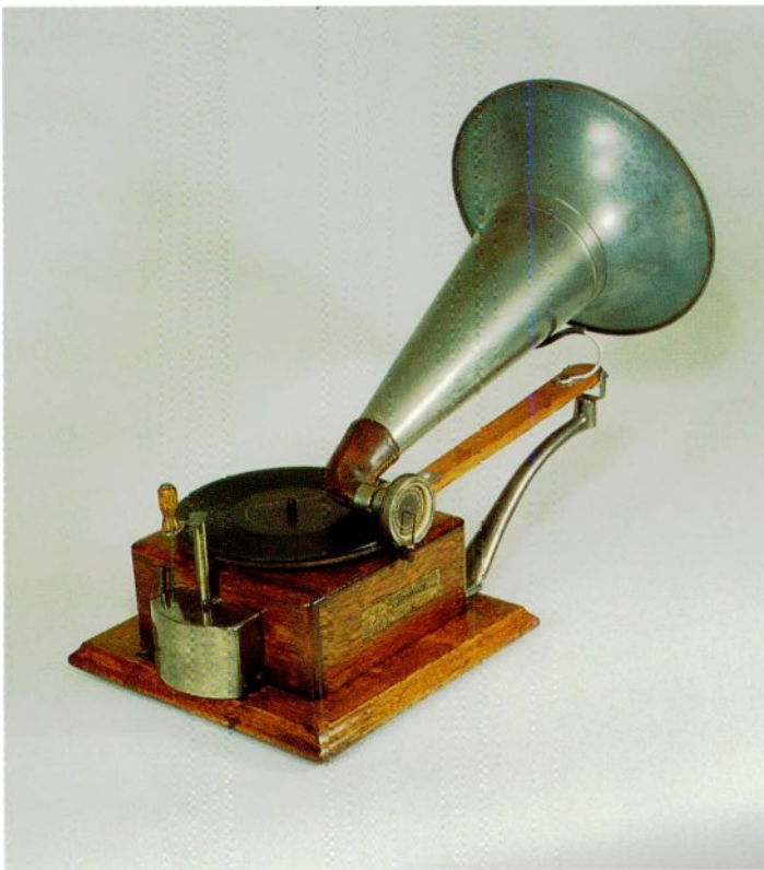
3-132 Gramophones based on Berliner's "Improved Gramophone" of 1897-1900 persisted in Europe until about 1904. Various slight modifications were made to cabinet and mechanism, but these low-priced machines retained unmistakable clues (most noticeably the vertical crank) to their origins. This Gramophone and Typewriter model is typical. Courtesy of Alan H. Mueller.
