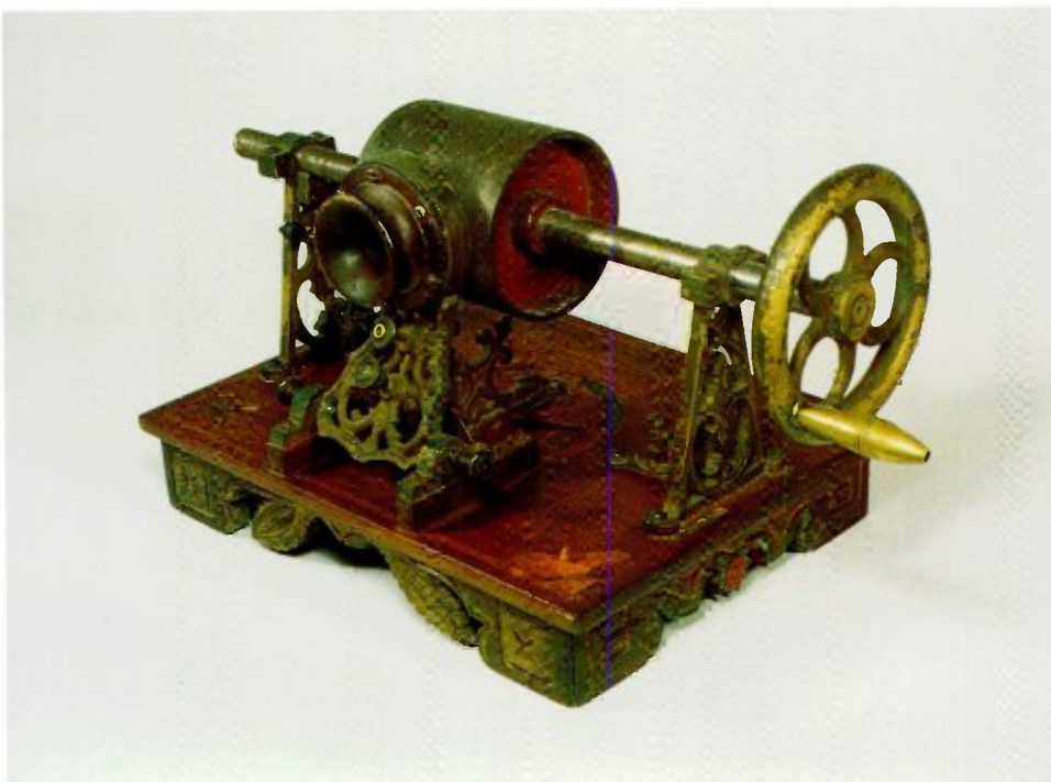
1-9 An American Tinfoil Phonograph typical of those made by local precision instrument manufacturers. Courtesy of Charles Hummel Collections.
