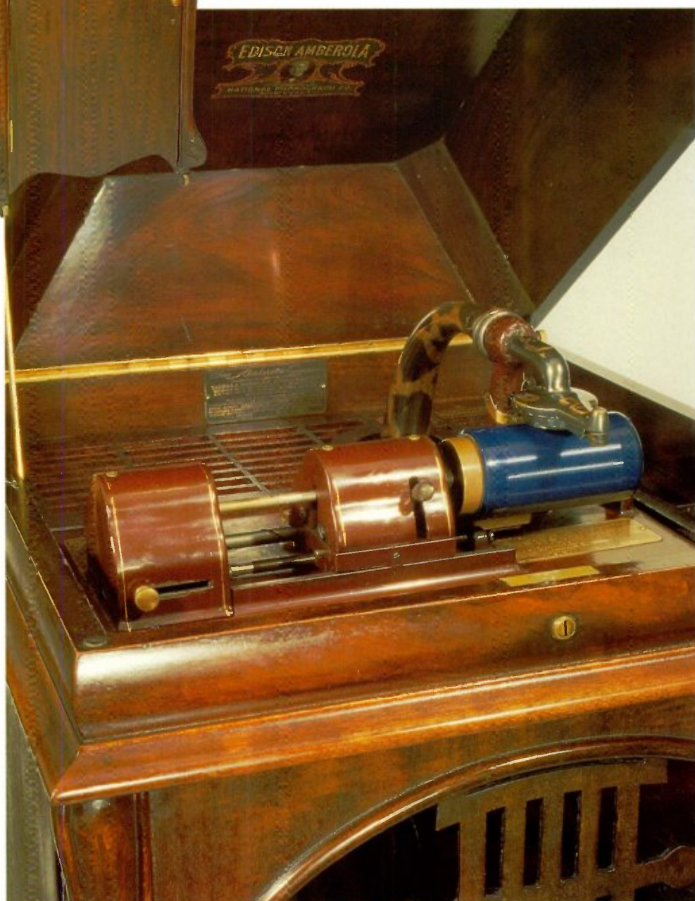
5-17 The interior of the earliest Amberola, showing the maroon-painted works, with gold-plated and oxidized bronze features. The mandrel tracked under a stationary reproducer, in a redefinition of Edison's original concept of the Phonograph. This Amberola was geared for both two- and four-minute cylinders. Courtesy of Norm and Janyne Smith.
