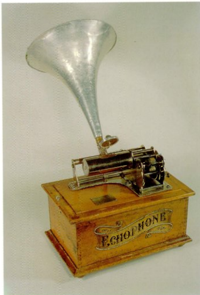
3-124 The "Echophone" was a Swiss-manufactured cylinder machine based heavily on the Columbia "Eagle". This one, which carries a brass plate indicating it was sold in an Arabic country, used a Columbia-made floating reproducer.
