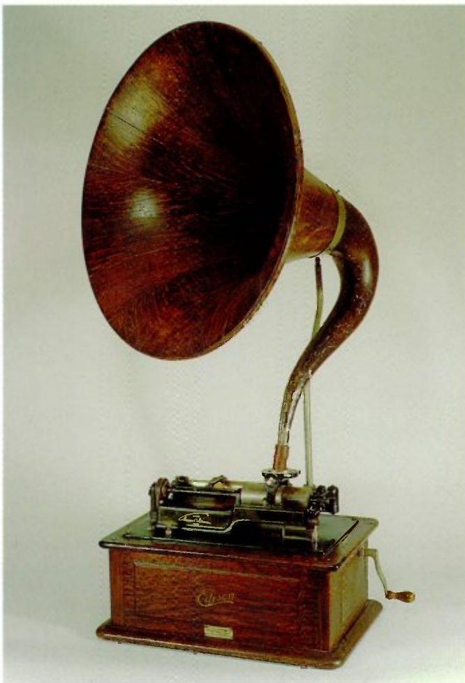
5-8 This Edison "Triumph" Model "B" was refitted with a two- and four- minute attachment, Model "O" reproducer, and oak cygnet horn after August 1910. Courtesy of Dan and Sandy Krygier.
