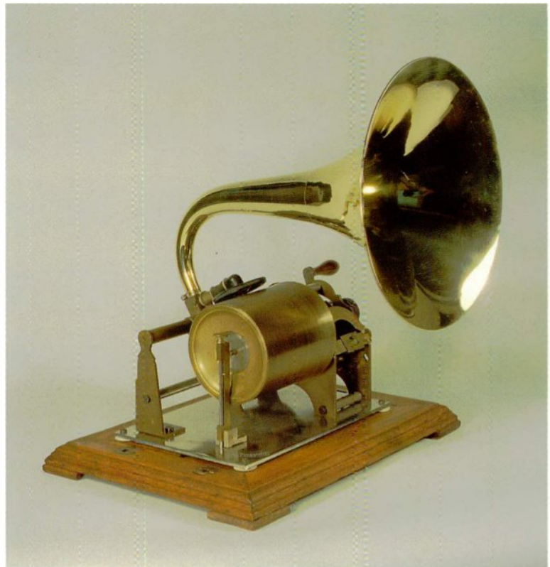
3-73 The "Idéal" talking machine was sold by the French religious publishing firm of Maison de la Bonne Presse. This company found it profitable to add talking machines and records to its printed offerings. The machine was available nickel-plated or in lacquered brass (shown). It featured a removable mandrel for the 5" cylinders, and an ebonite reproducer known as "Le Cahit".
