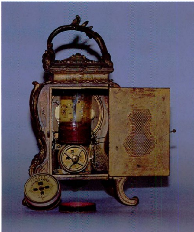
3-72 Hidden in the "Lioret Clock" was a "Le Merveilleux" mechanism which played a special cylinder. "Talking machine clocks" had been envisioned from the earliest days of Edison's Tinfoil machine. Many versions would be tried, including clocks that spoke the hours or merely used a record as an alarm (like this one). Courtesy of the Julien Anton Collection.
