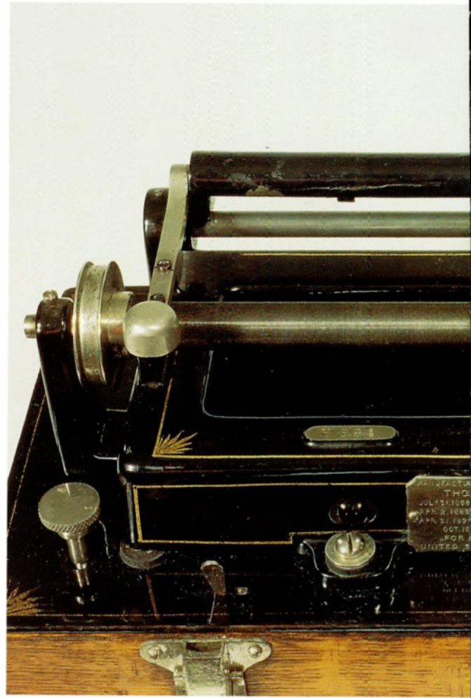
2-59 A close-up of Edison "Home" Phonograph No. 394 shows the upper casting with open frame beneath the feedscrew. Cast "fingers" to the right of the nicked parent plate hold the lift-lever in the resting position. Both of these features were soon abandoned. Courtesy of the William Kocher Collection.
