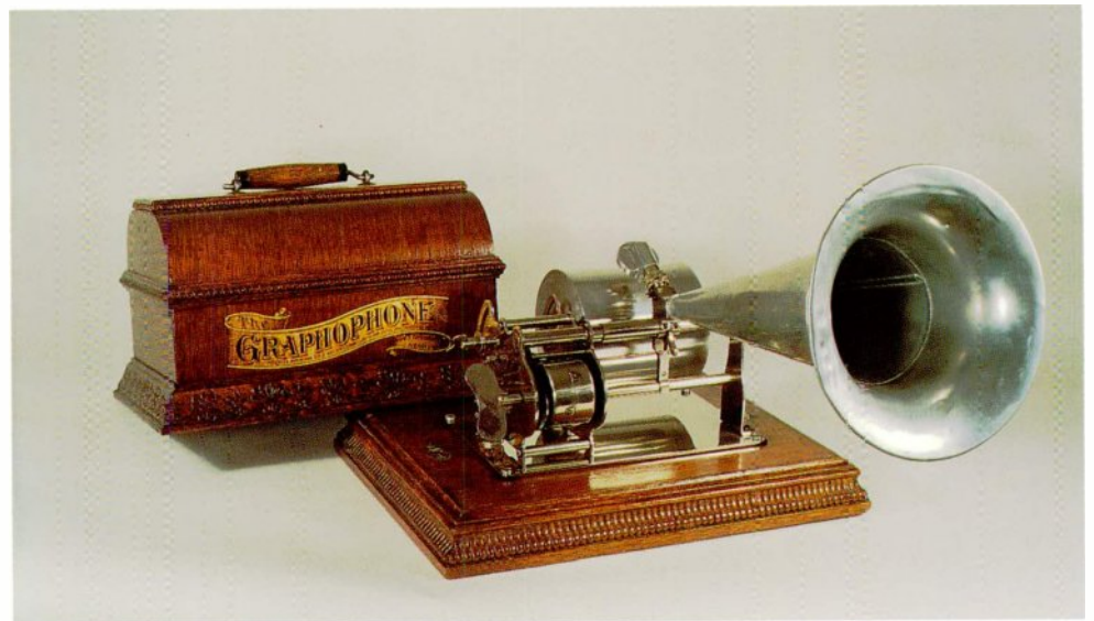
3-89 The Type "AB" Graphophone was closely based on the Type "B". At $25.00, the "AB" was the least expensive American talking machine capable of playing 5" cylinders. A telescoping mandrel allowed standard-sized cylinders to be played as well. Courtesy of George F. Paul.
