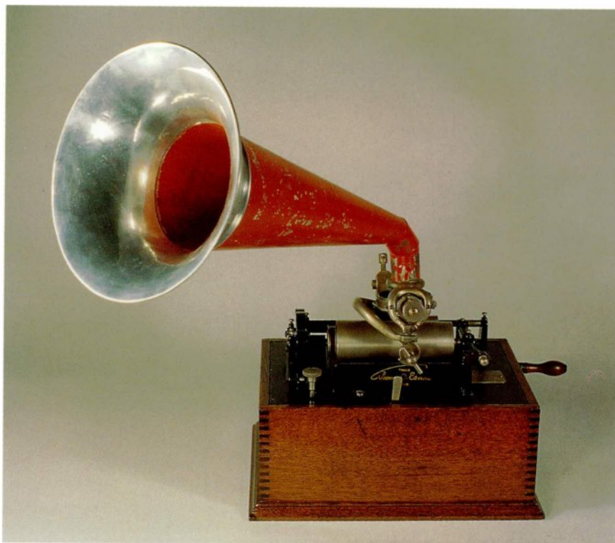
2-93 A "Bettini Micro-Attachment" on an 1898 Edison "Standard". Bettini horns commonly had lightweight aluminum bells and red painted steel bodies, with a soldered metal elbow.
