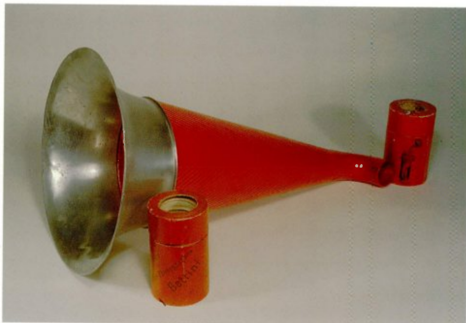
3-91 Another Type "AD" Graphophone, but with Bettini attachment and horn. A Lambert 5" cylinder is in position on the mandrel. Courtesy of the Howard Hazelcorn Collection.
