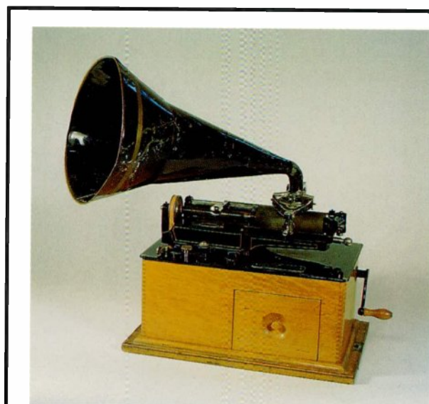
2-94 An Edison "Spring Motor" equipped with a Bettini recorder and rather unusual black Bettini horn. Courtesy of Sam Sheena.
