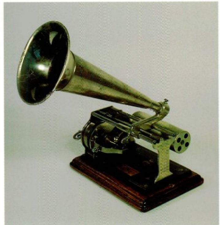
4-45 This machine appears to be a prototype for a final version of the Type "Q" Graphophone, considered by Columbia about 1906. It differs from the last production model most notably in the extended reproducer carriage (reproducer not in place). Courtesy of the Howard Hazelcorn Collection.
