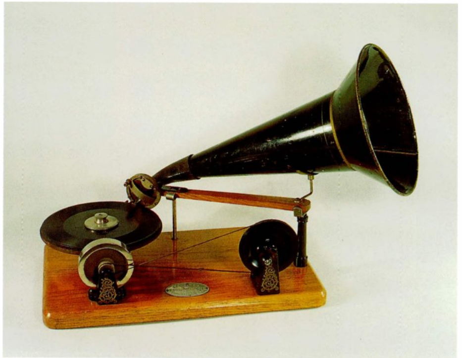
2-7 A hand-driven Berliner Gramophone originally sold for $15.00. This reasonably-priced machine inaugurated Berliner's activities in the United States. Courtesy of the Howard Hazelcorn Collection.
