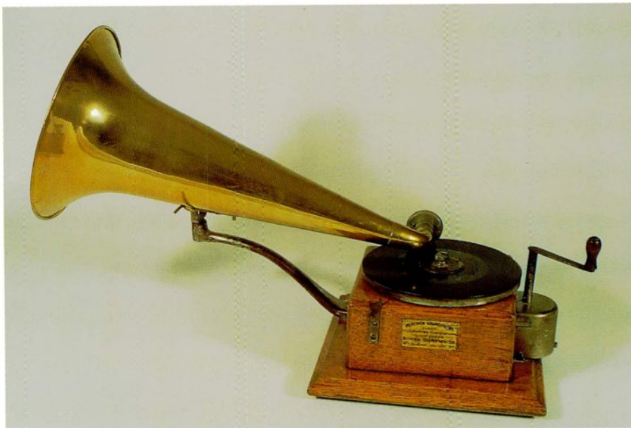
2-84 During the latter part of 1898, the "Improved Gramophone" was the only spring-driven disc talking machine available. It was occasionally sold with this all-brass "seamless" horn. Courtesy of Norm and Janyne Smith.
