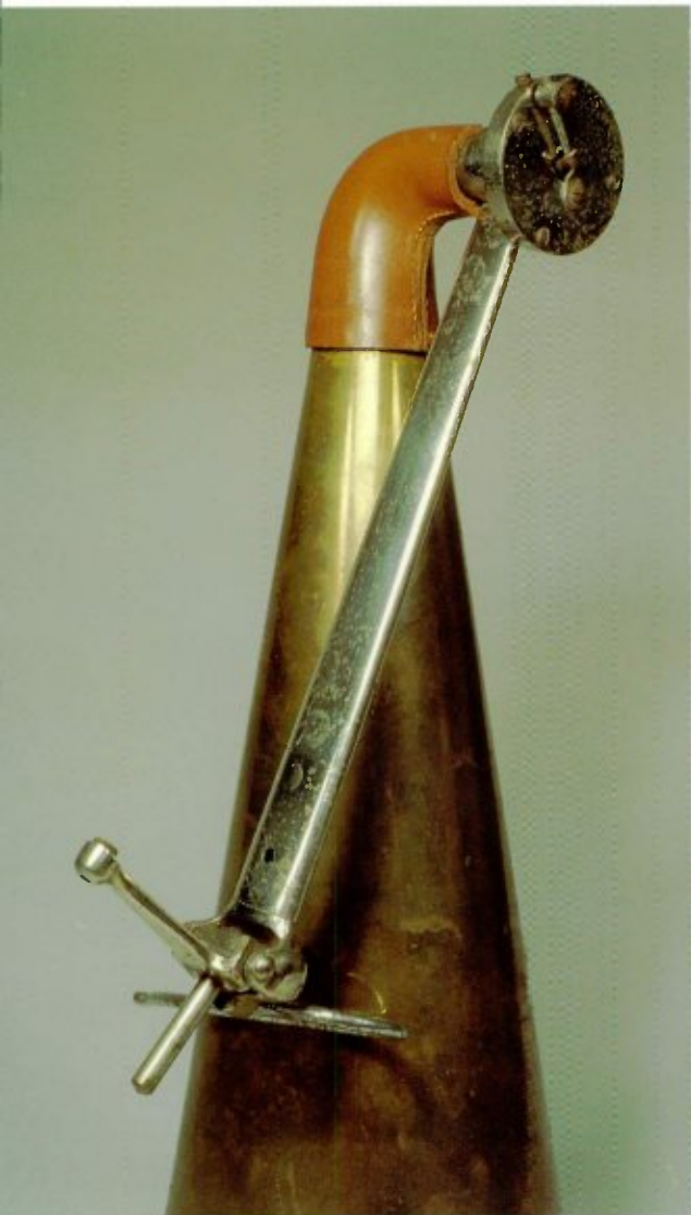
3-46 Close-up of the earliest style Zonophone traveling arm: note its ovular cross-section. Courtesy of the William Kocher Collection.
