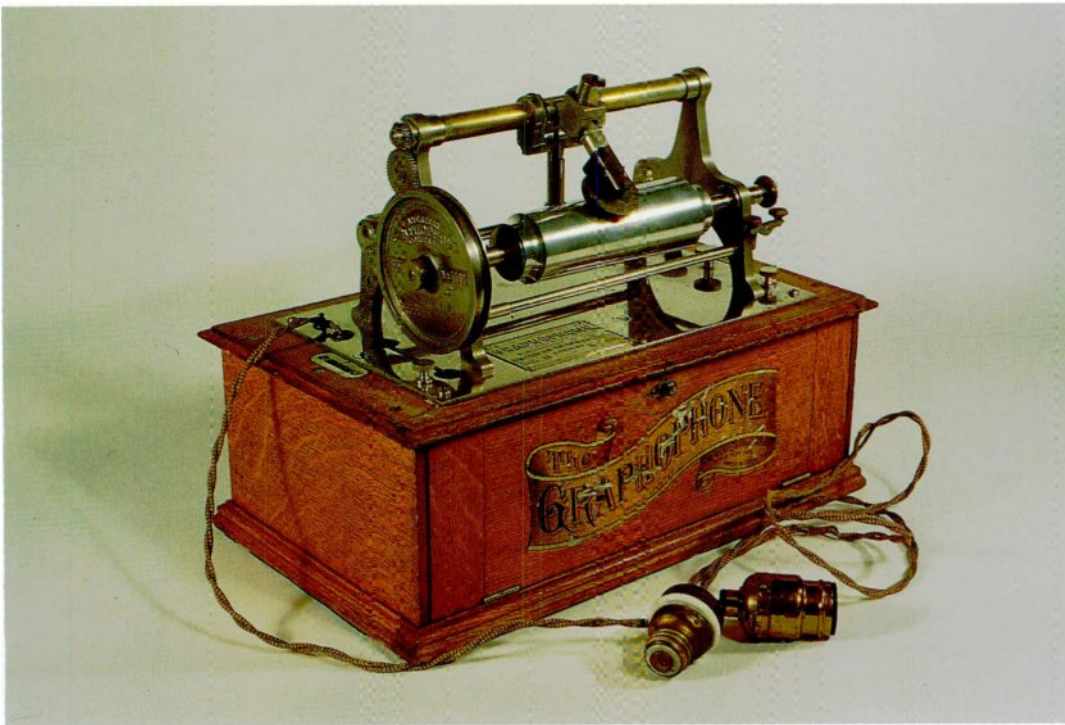
2-25 A Type "U" Graphophone of 1895 with a 110 volt electric motor. Courtesy of the Charles Hummel Collections.
