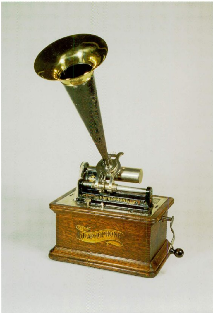
4-37 The Graphophone "AZ" (1905, $25.00) was the first of the "Lyric" reproducer machines. The initial version of the new reproducer (used here) employed a counter-weight design similar to Edison's. Later examples of the "Lyric" reproducer (from the "B" series Graphophones) would be known by the system substituted for the counter-weight: "Spring Tension". Courtesy of Lou Caruso.
