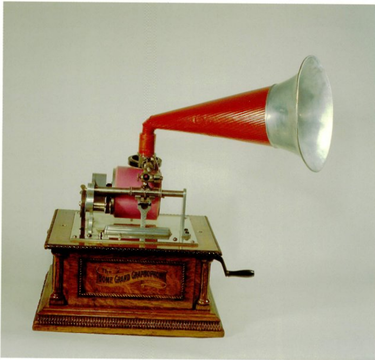
3-91 Another Type "AD" Graphophone, but with Bettini attachment and horn. A Lambert 5" cylinder is in position on the mandrel. Courtesy of the Howard Hazelcorn Collection.
