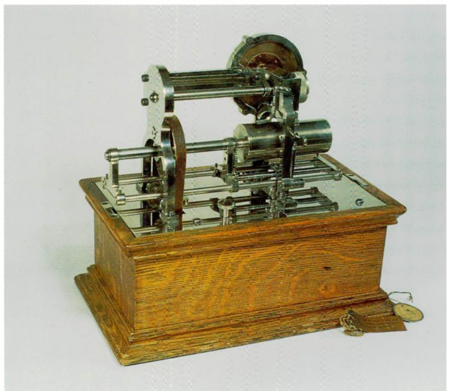
4-37 The Graphophone "AZ" (1905, $25.00) was the first of the "Lyric" reproducer machines. The initial version of the new reproducer (used here) employed a counter-weight design similar to Edison's. Later examples of the "Lyric" reproducer (from the "B" series Graphophones) would be known by the system substituted for the counter-weight: "Spring Tension". Courtesy of Lou Caruso.
