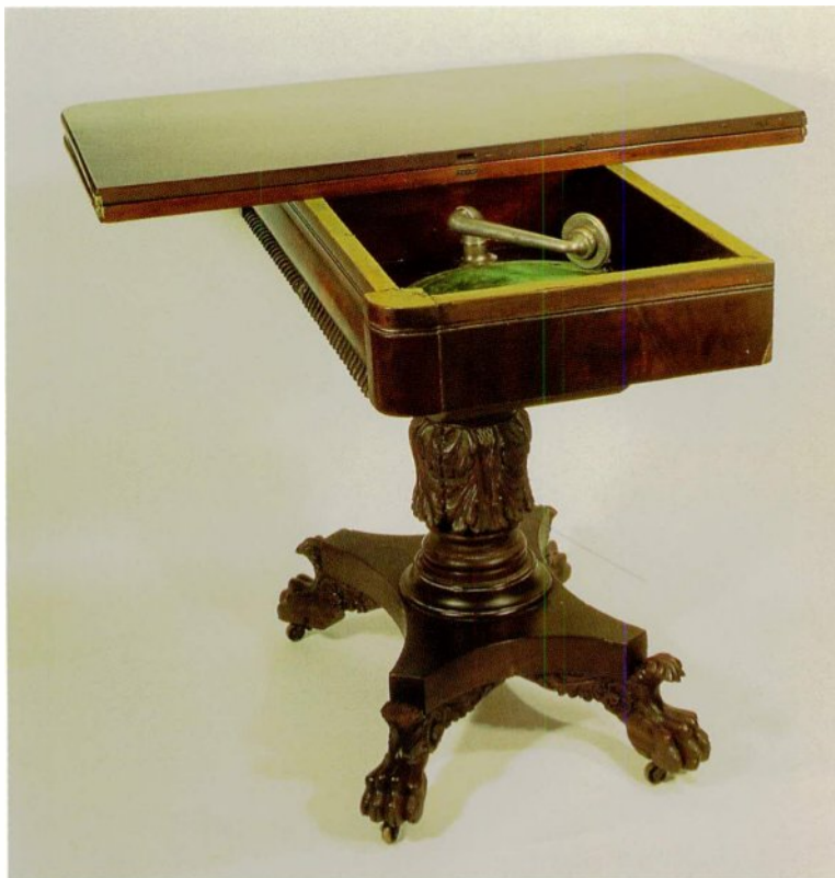
6-40 A view of the gaming table in the open position reveals a conventional Grafonola mechanism. Courtesy of Norm and Janyne Smith.
