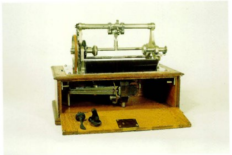
1-28 An 1893 Type "E" Graphophone consisting of a Type "C" treadle upper works with a 2 1/2 volt electric motor in a drop-front cabinet. Serial No. 10,431. Courtesy of the Aaron and Thea Cramer Collection.
