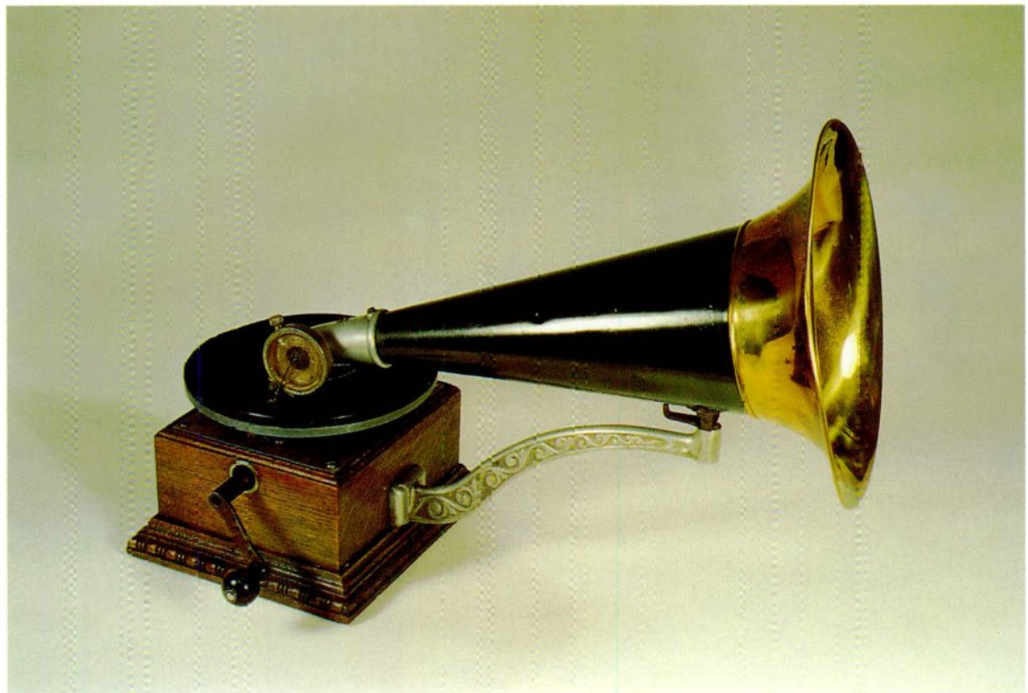
3-112 A 1902 Type "AK" Disc Graphophone. This machine featured a soundbox attached directly to the 16" horn, a single-spring motor, 7" turntable, and an original price of $15.00. Courtesy of Norm and Janyne Smith.
