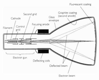
Figure 10. The Kinescope
