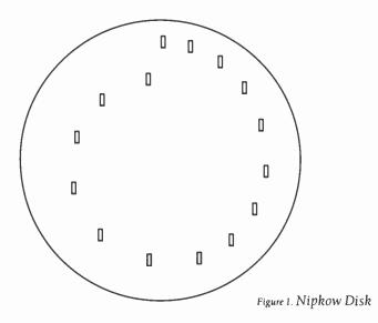
Pictures through wires were far-flung enough—too far-flung, in fact, for his time. His patent pictured a disk perforated with a sequence of holes that spiraled inward (Figure 1). The disk would be placed so that it cut off the light from the viewed object to the photocell. When it
