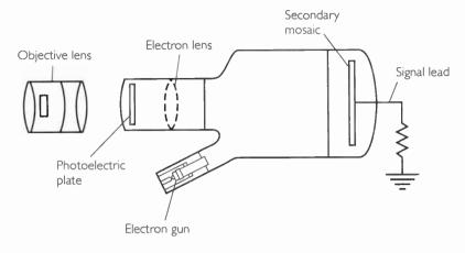
Figure 14. The Image Iconoscope
