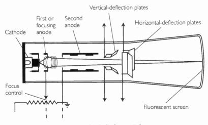
Figure 7. The Cathode-Ray Tube
