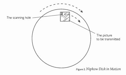
mitted by making the holes smaller and more numerous, each hole would allow even less light to come through, necessitating even greater illumination. Taken altogether, these problems called for a significant number of improvements to be made before any real results could be achieved.
