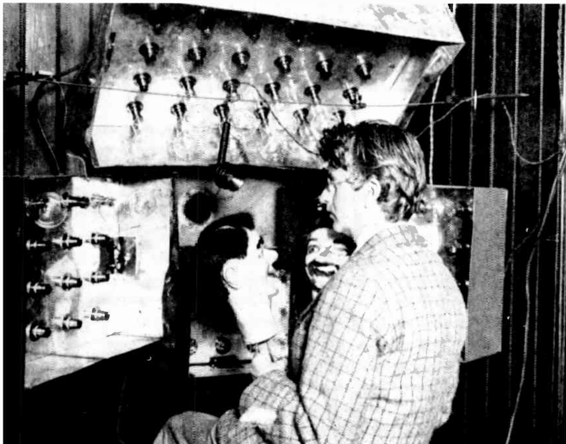
With the Nipkow disk, a bank of powerful light bulbs was needed to illuminate the subject to be scanned—in this case, Baird and his dummies in his laboratory (Henley Publishing Company 1929)
