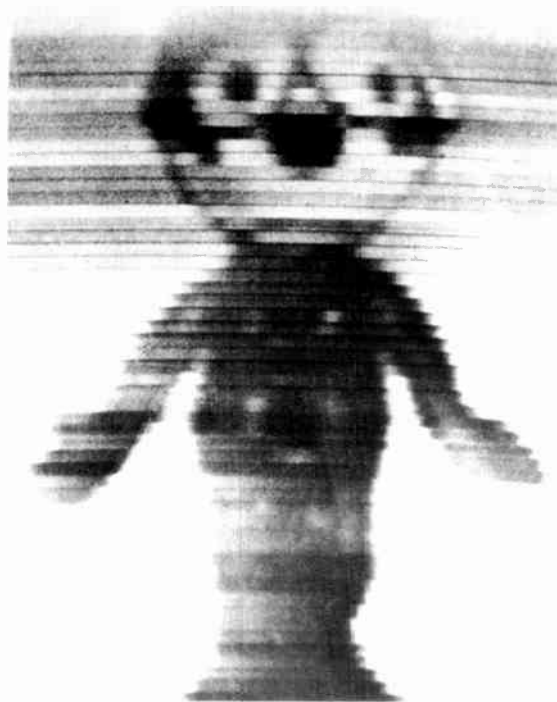
A plastic model of Felix the Cat provided a willing test model for RCA's experimental transmissions in 1929 and 1930. Felix stood atop a phonograph turntable in front of a Nipkow-disk camera (above). The result was a 60-line picture on Zworykin's Kinescope receiver (left). (David Sarnoff Research Center)
