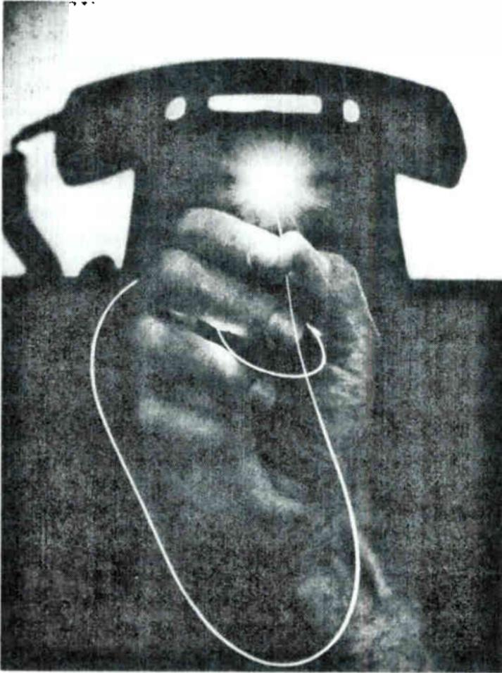
Communication superhighway—glass fiber through which a laser beam can carry numerous streams of communication, far exceeding capacity of coaxial cable.
