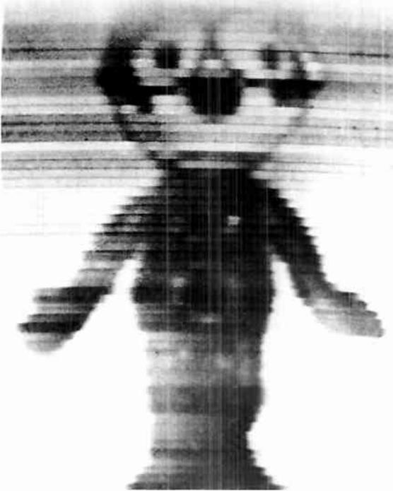
A plastic model of Felix the Cat provided a willing test model for RCA's experimental transmissions in 1929 and 1930. Felix stood atop a phonograph turntable in front of a Nipkow-disk camera (above). The result was a 60-line picture on Zworykin's Kinescope receiver (left). (David Sarnoff Research Center)
