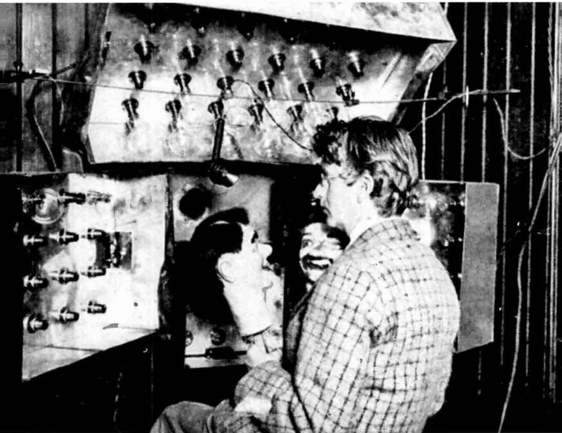
With the Nipkow disk, a bank of powerful light bulbs was needed to illuminate the subject to be scanned—in this case, Baird and his dummies in his laboratory.
