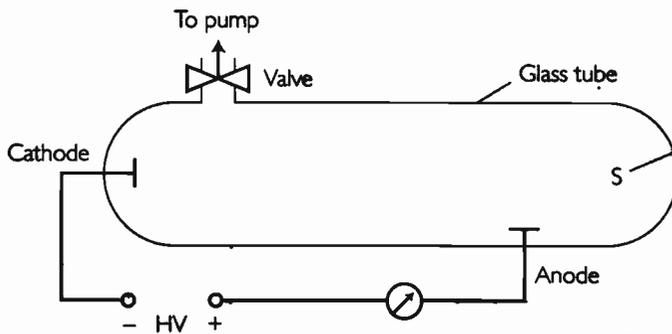
Figure 6. Geissler Vacuum Tube
