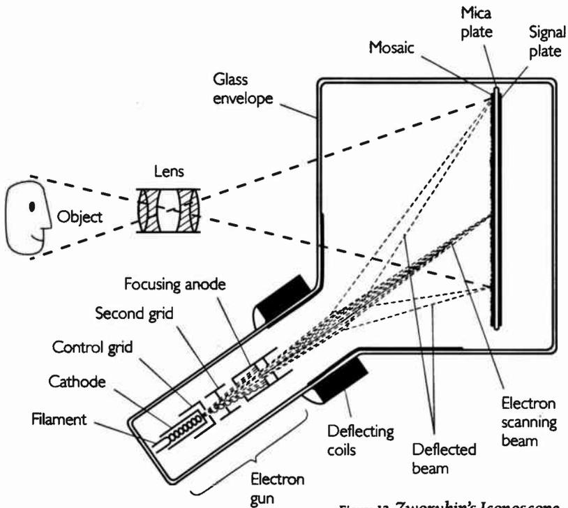
Figure 13. Zworykin's Iconoscope
