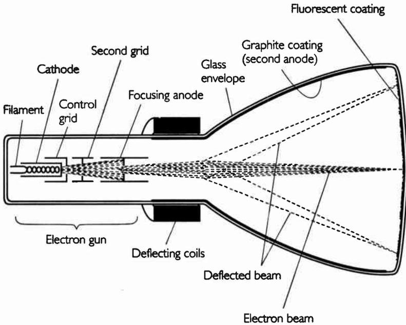
Figure 10. The Kinescope
