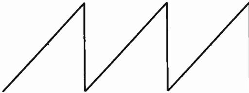
Figure 12. Sawtooth-Wave Scanning Current
