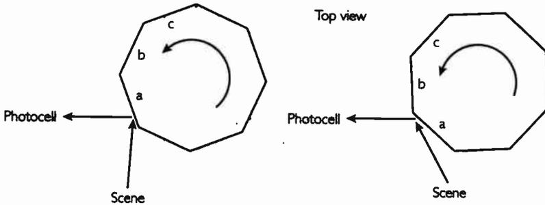
*Figure 5. Angle of Reflected Light Shifts as Drum Rotates*
