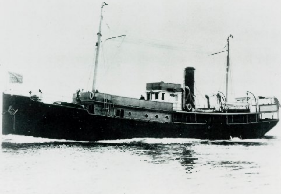
The S.S. Rowena prior to conversion to become the Peary. During conversion, the after deck house was removed to provide space for the Loening aircraft. Courtesy of Zenith.
