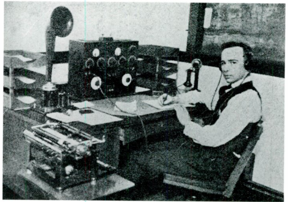
The Chicago Tribune receiving station installed by Mathews and Hassel in 1919 to receive news of the Versailles Peace Conference. The antenna for the installation was on the roof of the Tribune building and was 70 feet long and 30 feet high and was aimed at Bordeaux, France. The receiver was an early prototype for the 1921 CRL Allceiver. Courtesy of Zenith.
