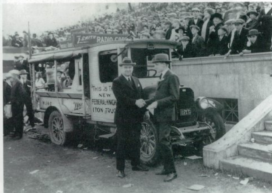
Below: R.H.G. Mathews (r) being welcomed to Soldier's Field with the new WJAZ mobile unit. The mobile unit was built on a 1924 Federal-Knight 1-ton truck chassis.
