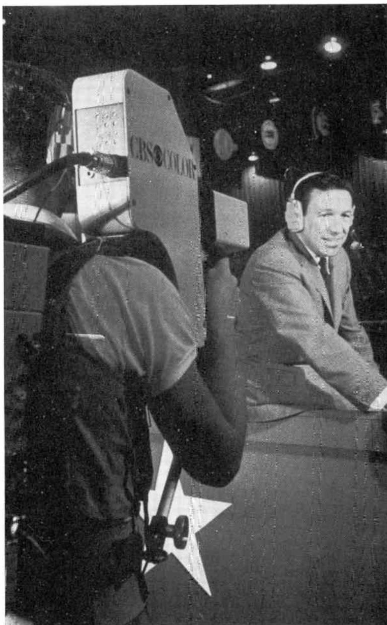
A portable, wireless color TV camera in use at a remote pickup with CBS News Correspondent Mike Wallace. (Courtesy CBS News)
