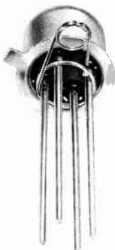
Fig. 367—Illustration shows shorting spring for RCA MOS field-effect transistors that do not contain the integral gate protection. (Spring should not be removed until after the device is soldered into circuit.)
