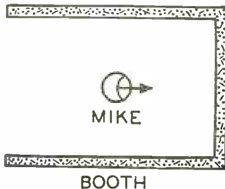
Fig. 4-14. When a microphone is placed in a booth with walls lined with sound-absorbent material, the resulting speech seems to be coming from a telephone booth.
