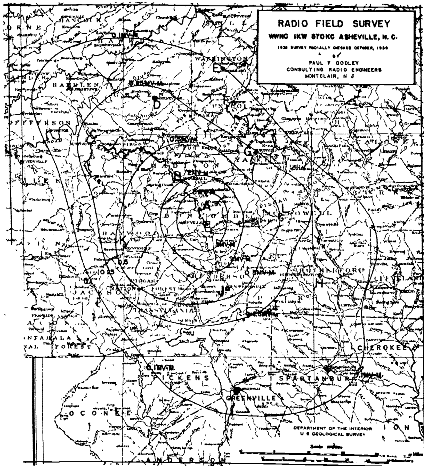
Fig. 3.—Listening areas plotted by the field-strength method. Station WWNC, 1,000 watts, Asheville, N. C.
