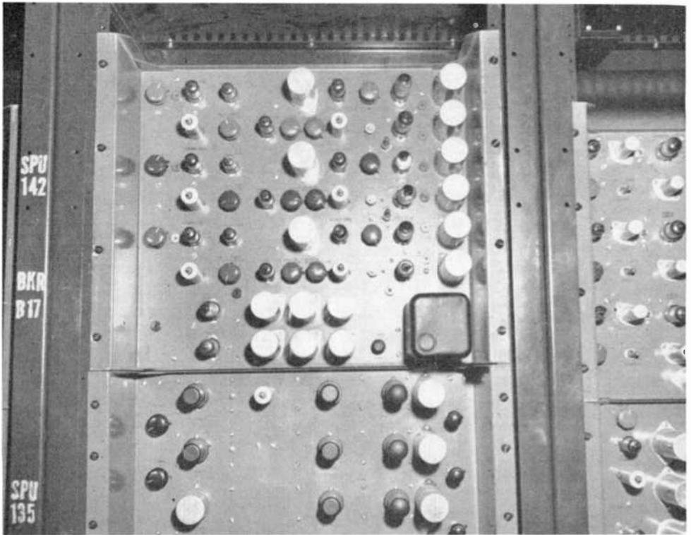
*Fig. 22 — Three-channel gamma corrector (upper chassis).*
