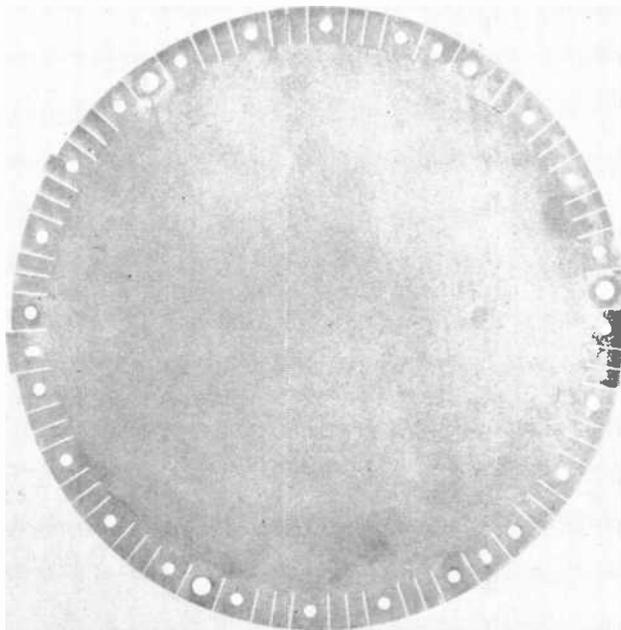
*Fig. 18 – Plan view of shadow mask.*
