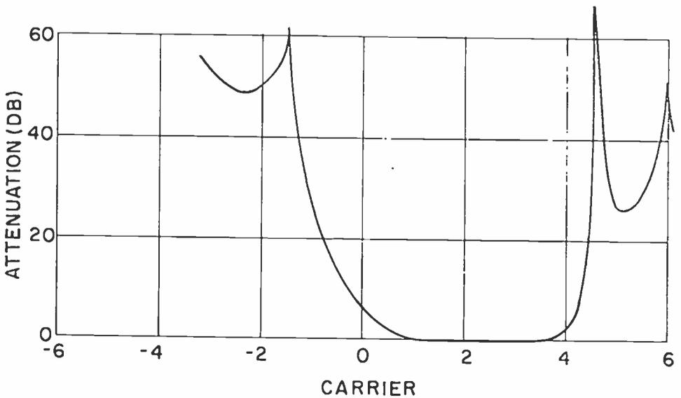
Fig. 7 – Selectivity characteristic of color receiver.
