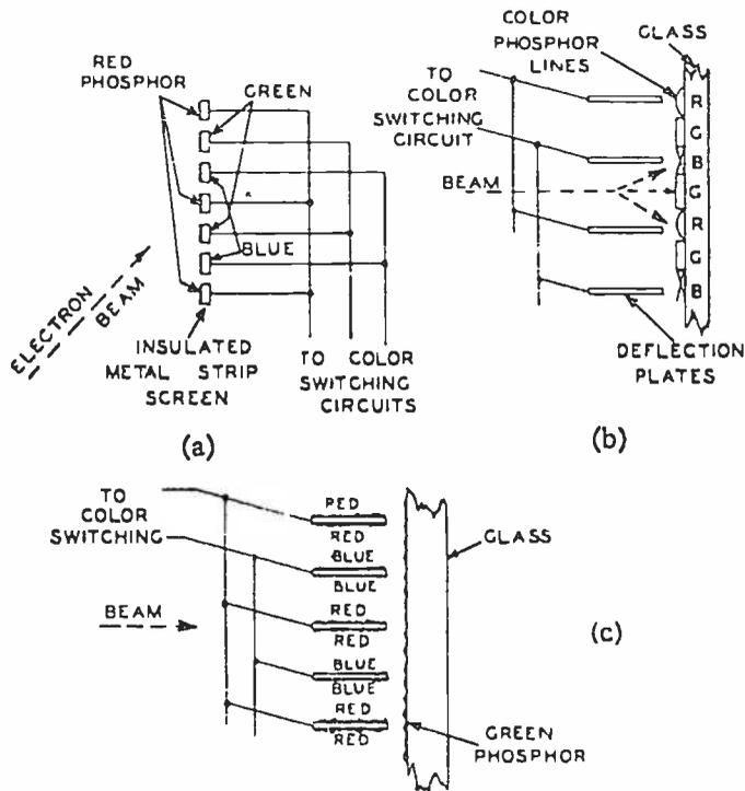
Fig. 5 — Beam control at phosphor screen for changing color. (a) Simple line-screen color switching. (b) Deflection switching of colors with line screen. (c) Deflection switching without requiring registry.
