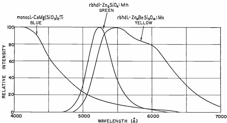
Fig. 4.—Spectral characteristics of red, green, and blue silicate phosphors. At the present time (1953),  $\text{ZnS:Ag}$  is being used as the blue phosphor, and  $\text{Zn}_2(\text{PO}_4)_2:\text{Mn}$  as the red phosphor in tricolor kinescopes.
