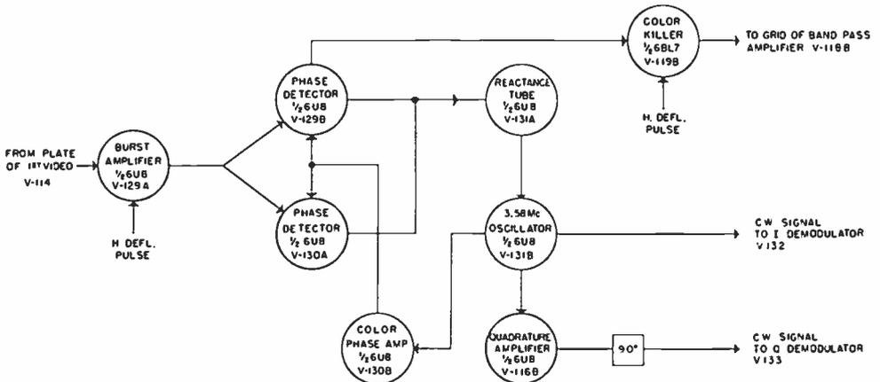
Fig. 10—Color synchronization channel block diagram.
