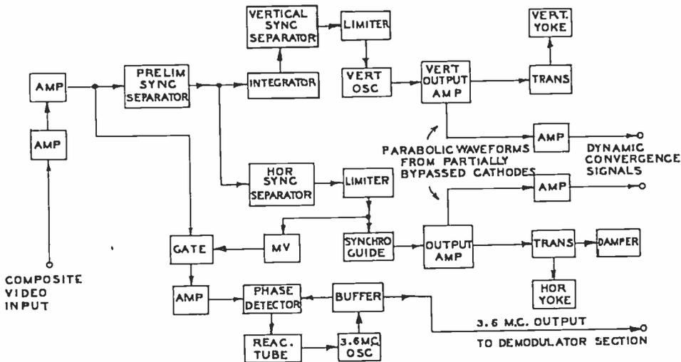
Fig. 38 — Block diagram showing sync separator, deflection, and burst-controlled oscillator circuits for a single-input color monitor.
