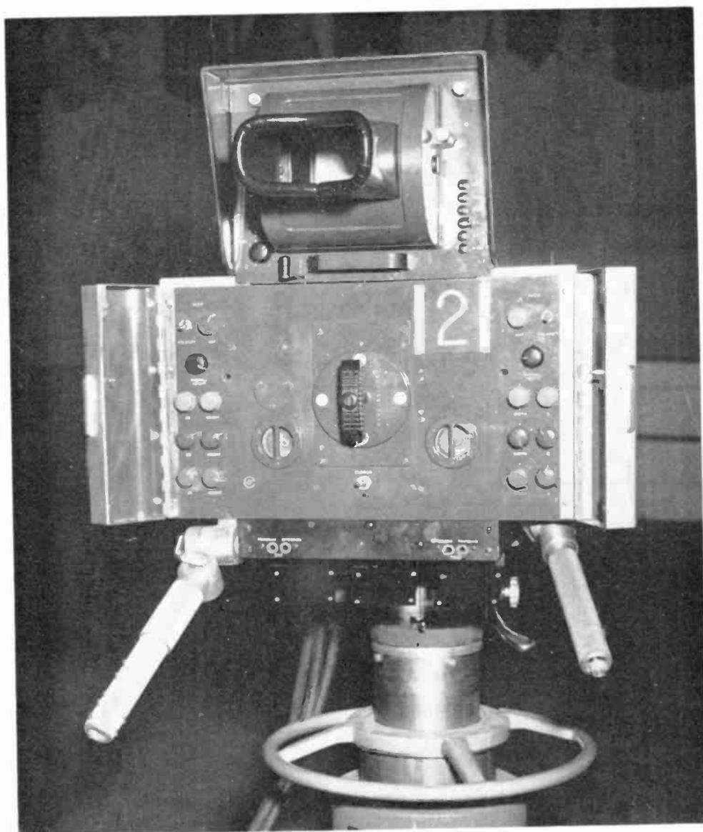
*Fig. 15 — Rear view of an RCA color television camera, showing electrical controls.*
