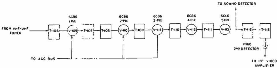
Fig. 4a—Picture IF channel block diagram.
