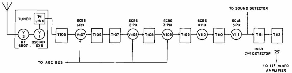
Fig. 3a—RF tuner and IF channel.
