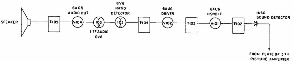
*Fig. 5—Sound IF and audio channel block diagram.*
