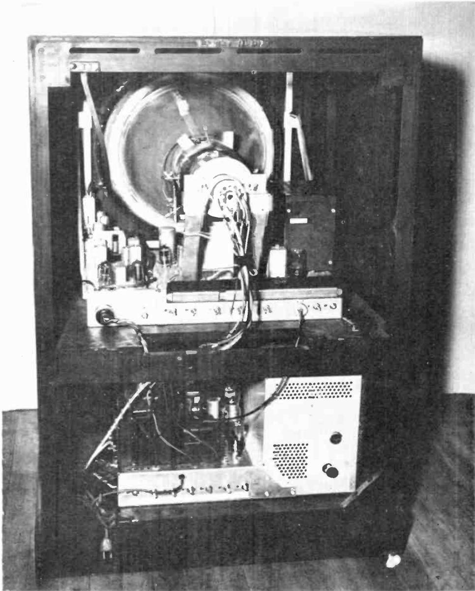
*Fig. 6 — 16-inch Tricolor Kinescope Receiver Model No. 1*
