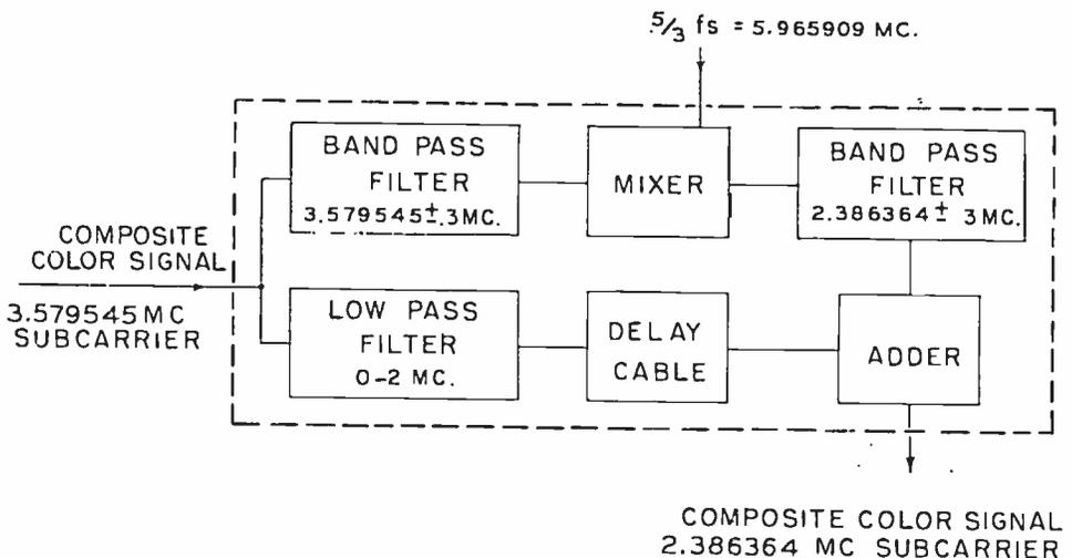
Fig. 10 — Cable transmitting heterodyne system.
