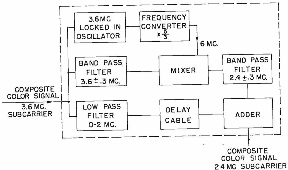
Fig. 3 — Cable transmitting heterodyne system.
