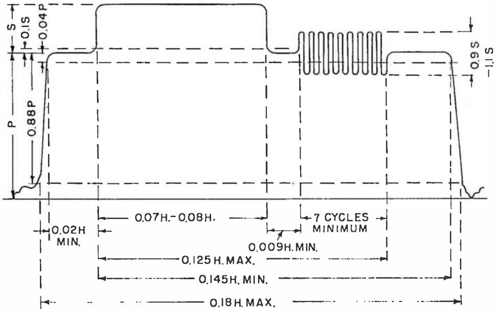
Fig. 1—Proposed field test synchronizing wave form.
