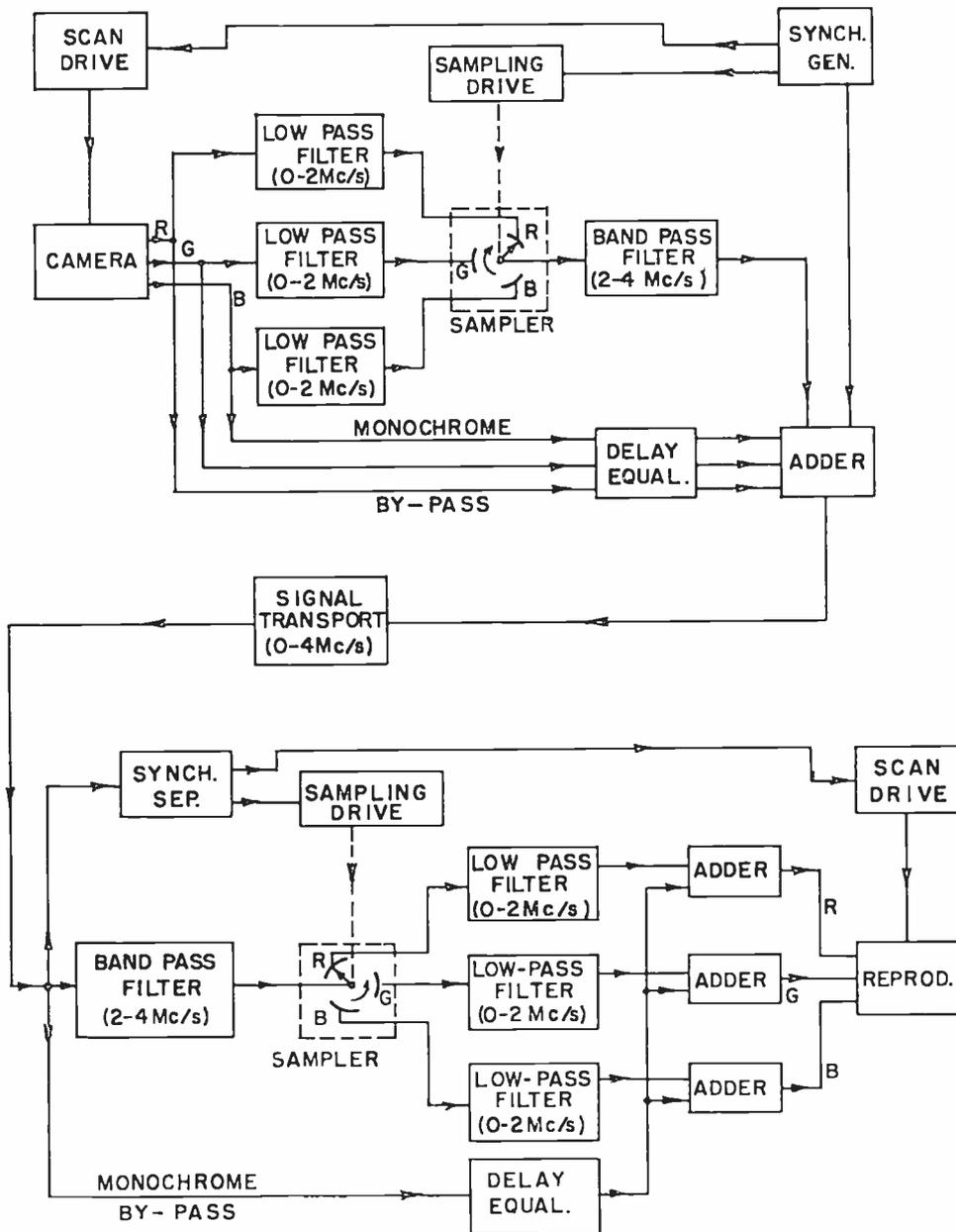
Fig. 10 — A simultaneous-transmission system using complete monochrome by-pass.
