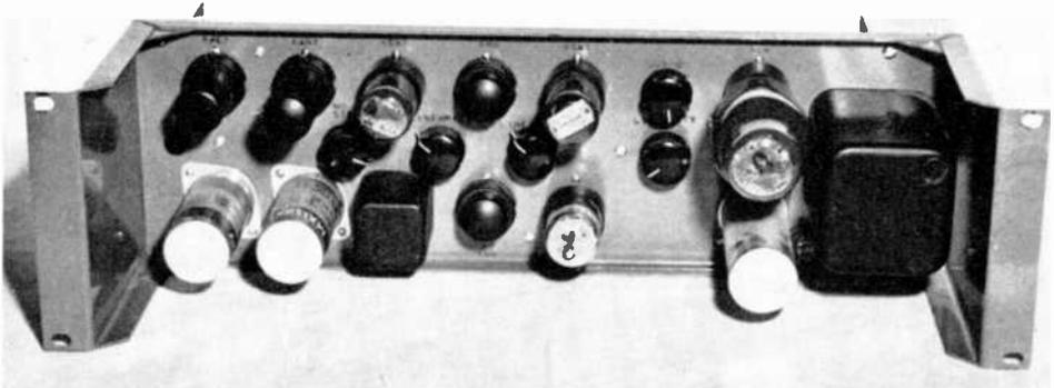
*Fig. 42 — Step-wedge generator.*
