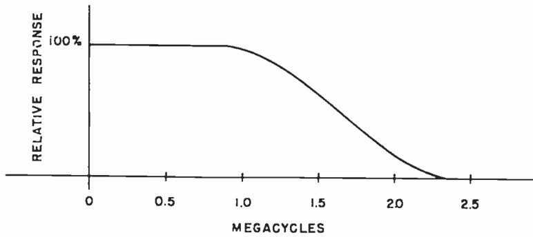
*Fig. 9—I channel frequency response.*
