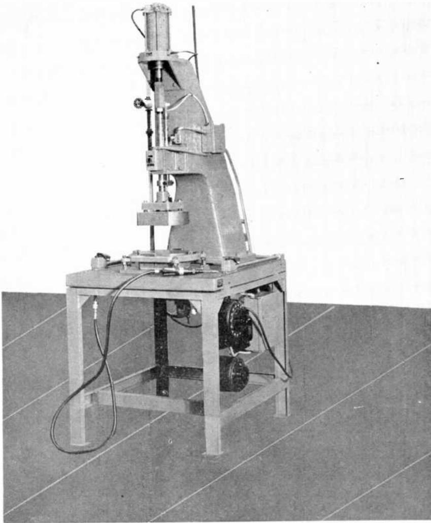
*Fig. 21 – Factory “hot-blocking” equipment.*
