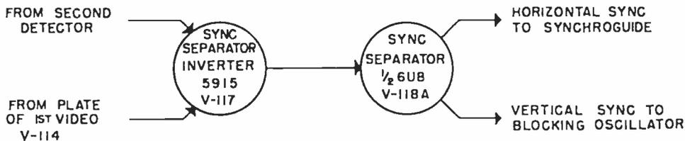
Fig. 11—Deflection synchronization channel block diagram.
