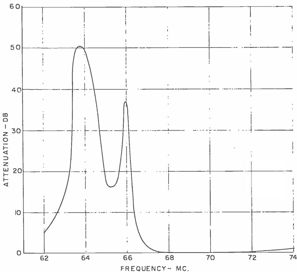
Fig. 2a - Transmission characteristic channel 4 (undesired).
