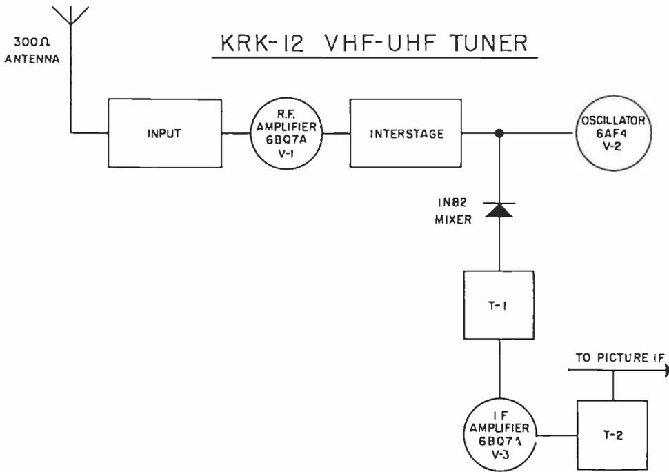
*Fig. 3a—RF tuner — VHF operation block diagram.*
