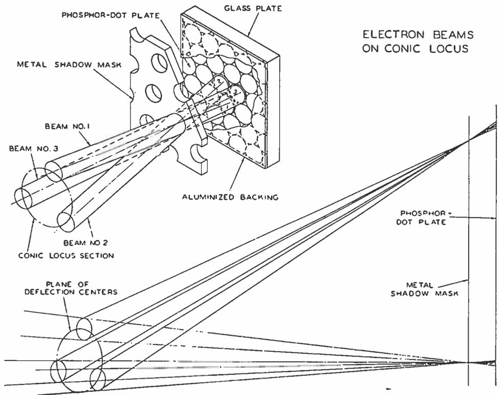
Fig. 22 – Diagram illustrating beam convergence.
