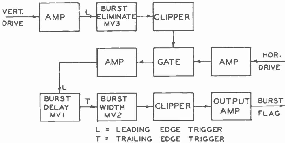
Fig. 6 – Block diagram of a burst flag generator.
