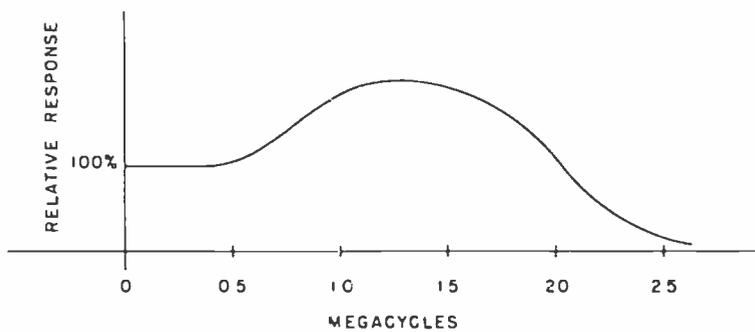
*Fig. 8—I channel frequency response.*
