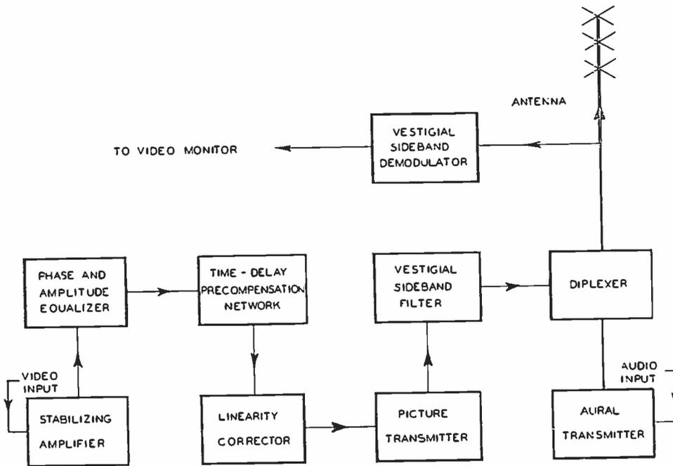
Fig. 52—Block diagram for a color television transmitter with auxiliary equipment.\*
