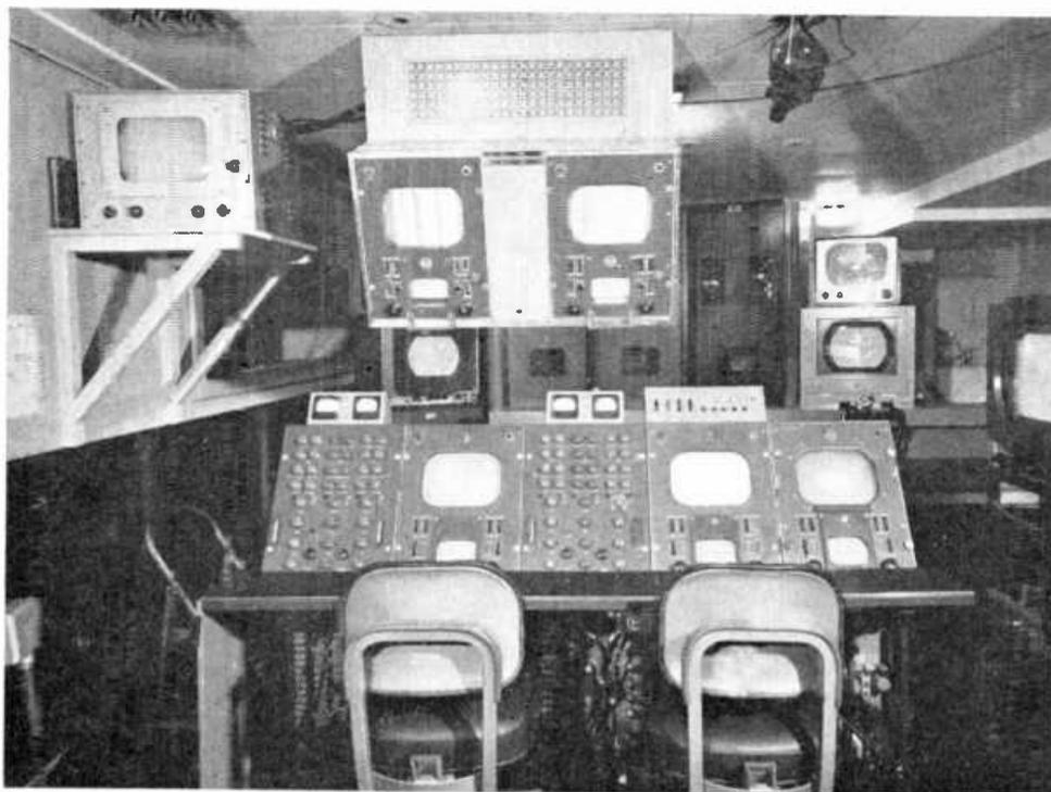
*Fig. 6—Photograph of video control console.*
