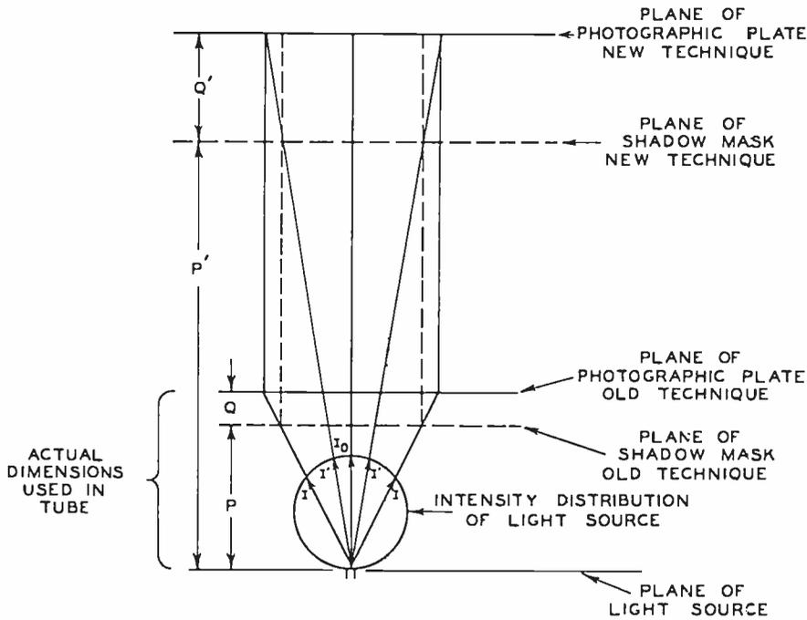
THE PROJECTED ARRAYS ARE IDENTICAL IF  $\frac{P}{Q} = \frac{P'}{Q'}$ ; HOWEVER, THE INTENSITY VARIATION CENTER TO EDGE  $\frac{I_0 - I'}{I_0} \ll \frac{I_0 - I}{I_0}$
