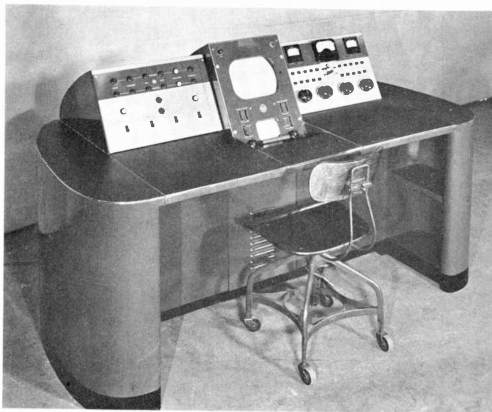
*Fig. 51 — Control console for a TT5A television transmitter.*
