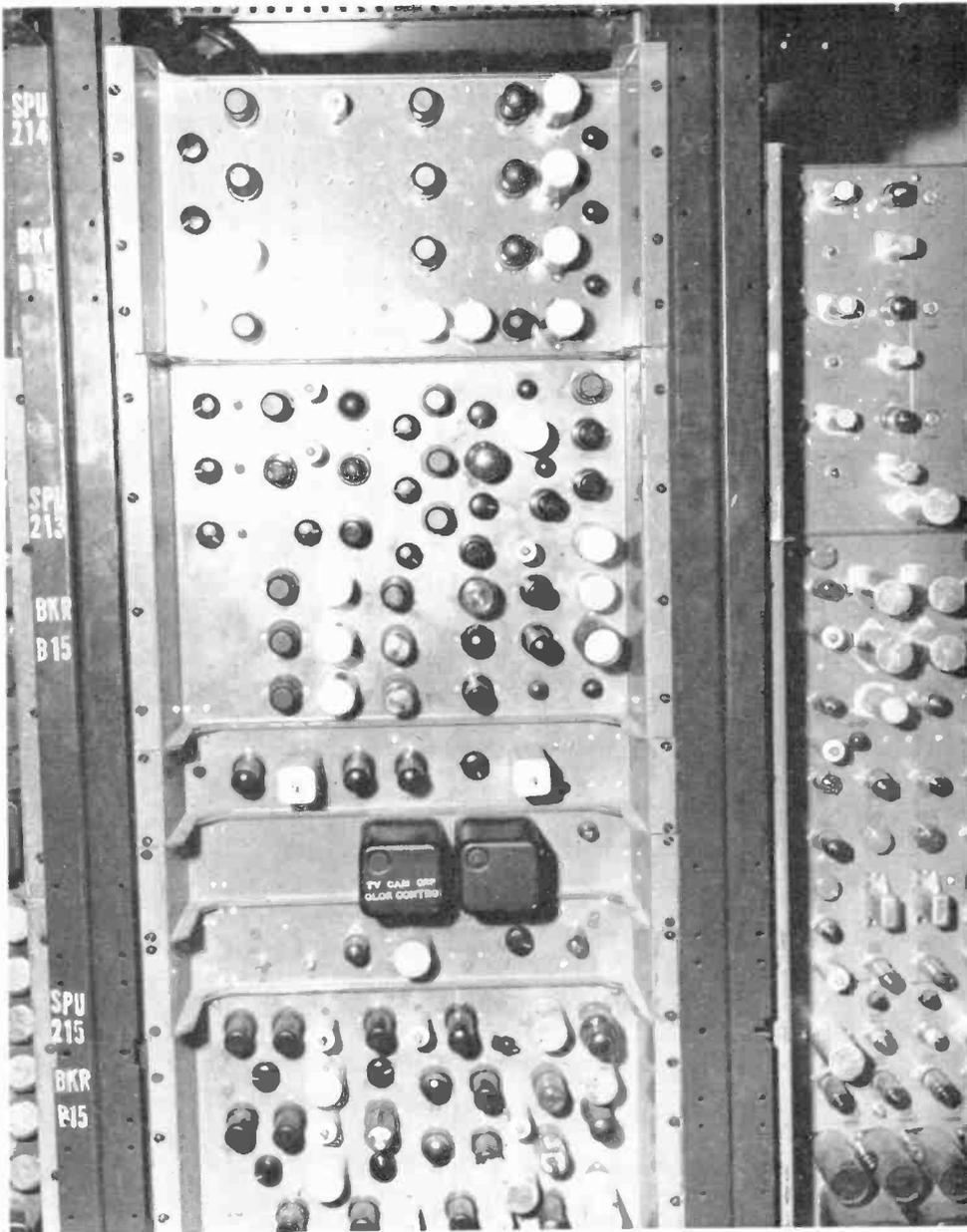
*Fig. 36 — Typical colorplexer (upper two chassis).*
