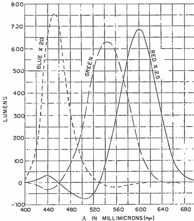
Fig. 1—Color mixture curves giving the number of lumens of three monochromatic primaries (Red—650 m $\mu$ , Green—530m $\mu$ , Blue—460m $\mu$ ) required to match one watt of radiant power having indicated wavelength. Based on data obtained by W. D. Wright.<sup>1</sup>
