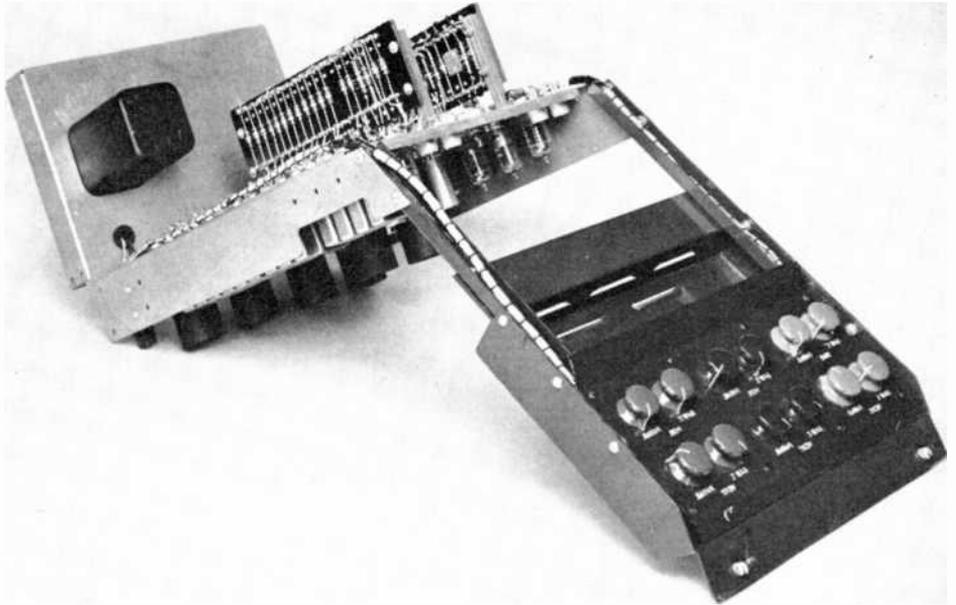
*Fig. 20 — Shading generator.*
