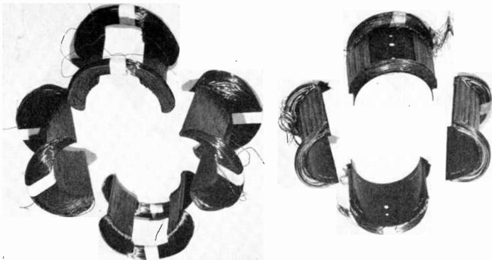
*Fig. 23 — Deflecting coils designed for tricolor kinescope. Left: Early design using section-wound coils. Right: Later design using continuously wound coils.*
