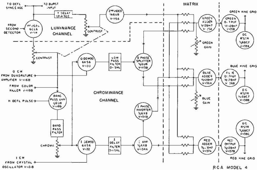
Fig. 6—Video section block diagram.
