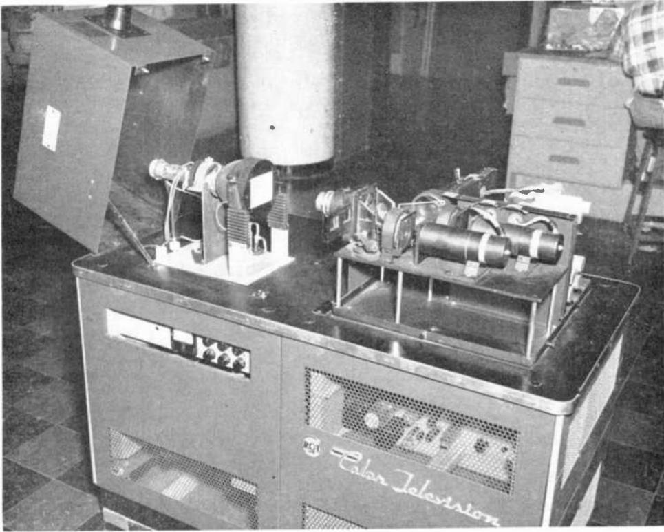
*Fig. 29 — Flying-spot scanner with protective covers removed.*
