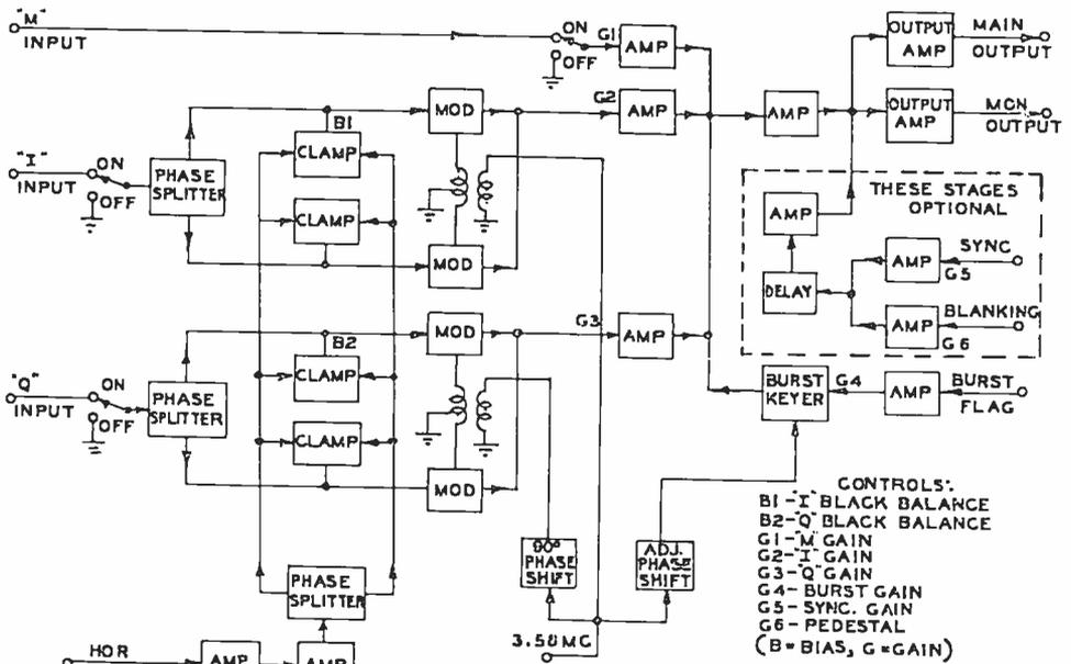
Fig. 35 - Block diagram for a colorplexer modulator and mixer section.
