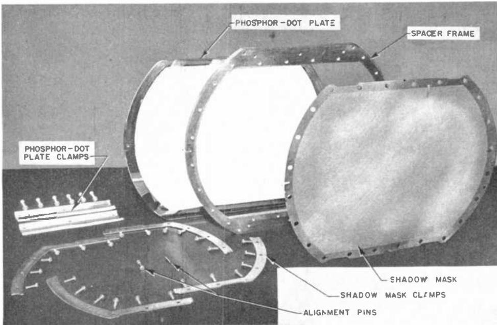
Fig. 16 — Exploded view of viewing-screen assembly — early design.
