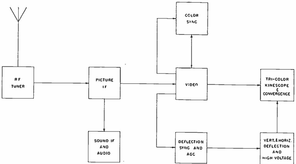
*Fig. 2—Color TV receiver master block diagram.*
