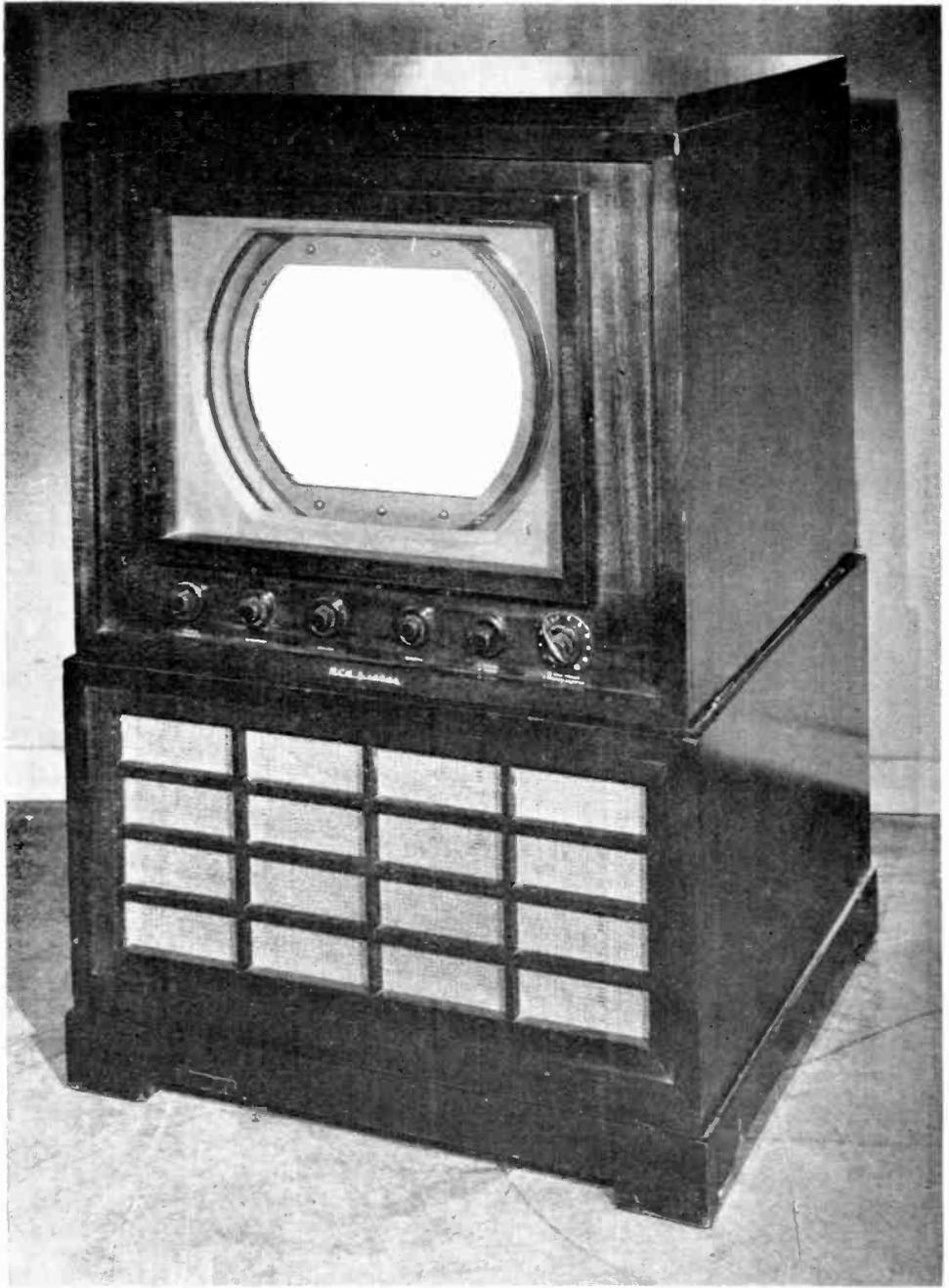
*Fig. 7 — 16-inch Tricolor Kinescope Receiver Model No. 2*
