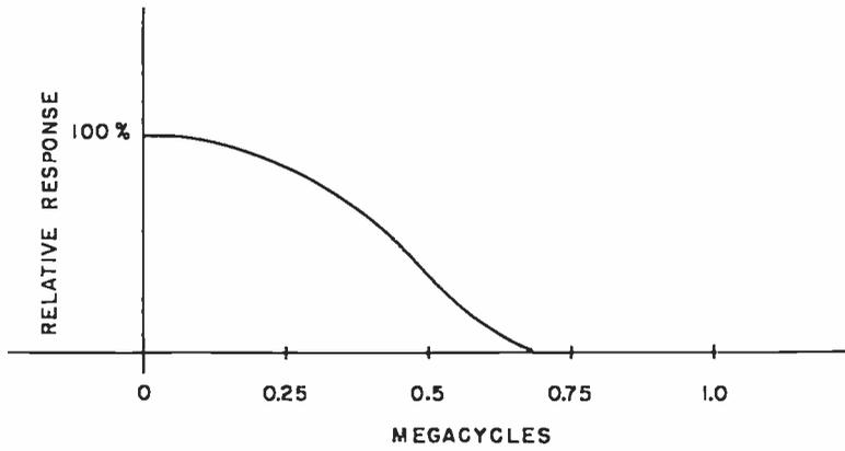
*Fig. 8—Q channel frequency response.*
