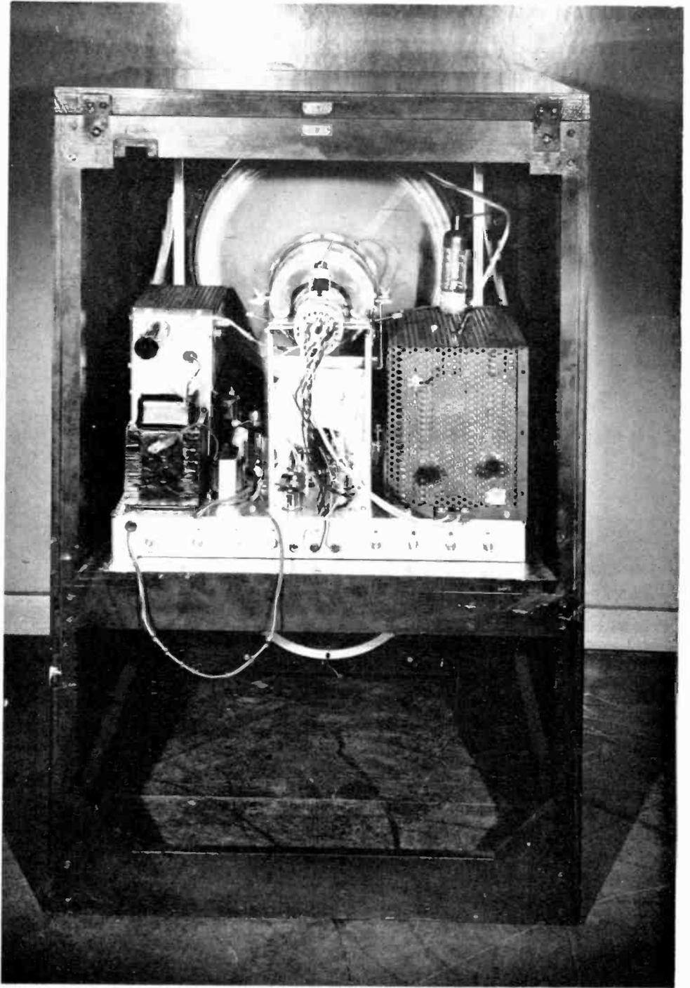
*Fig. 1b—Back view of 16-inch Tricolor Kinescope Receiver Model No. 3A.*
