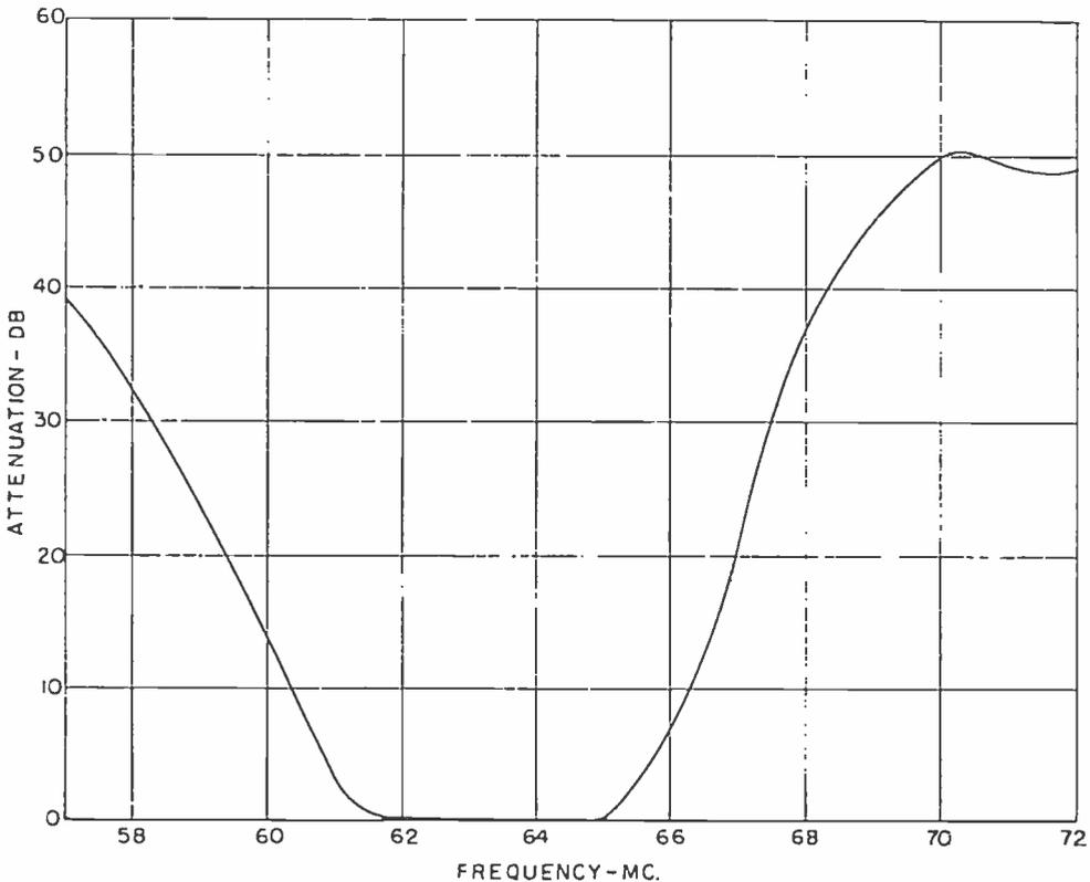
Fig. 2b - Transmission characteristic channel 3.
