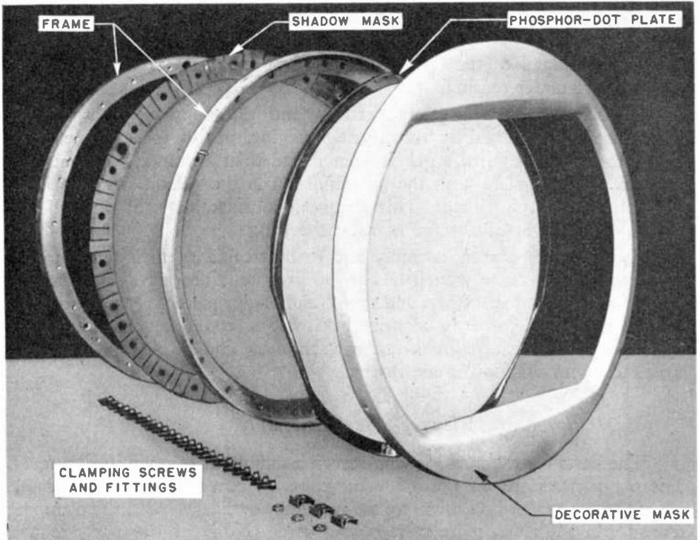
*Fig. 17 — Exploded view of new viewing-screen assembly.*
