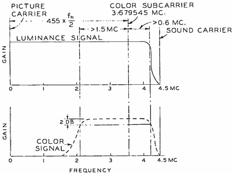
Fig. 9 - Video spectrum of the color television signal.
