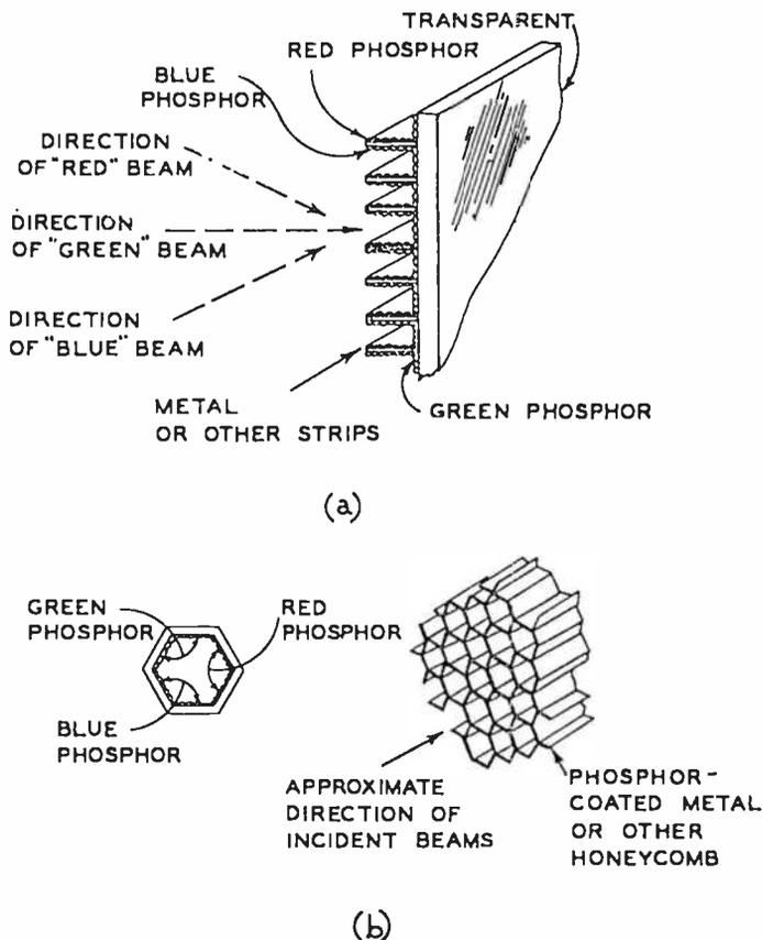
Fig. 9 — Two forms of nonplanar direction-sensitive color screen.
