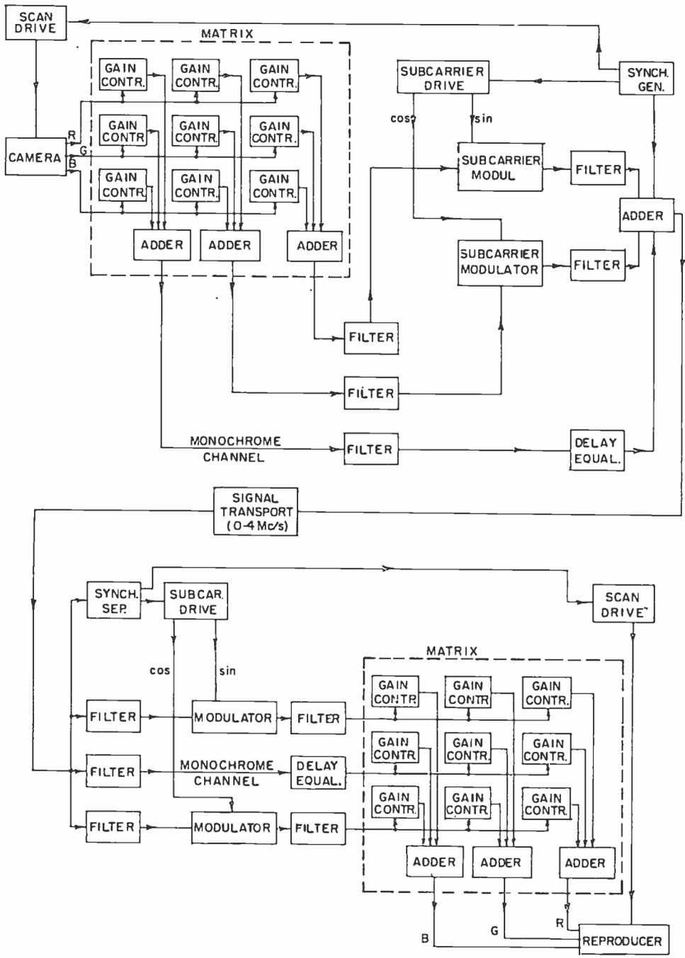
Fig. 11 - A basic modulated-subcarrier color television system.
