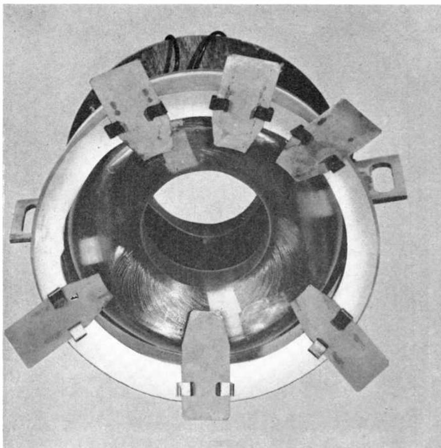
*Fig. 24 — Developmental deflecting yoke showing field-compensating tabs.*
