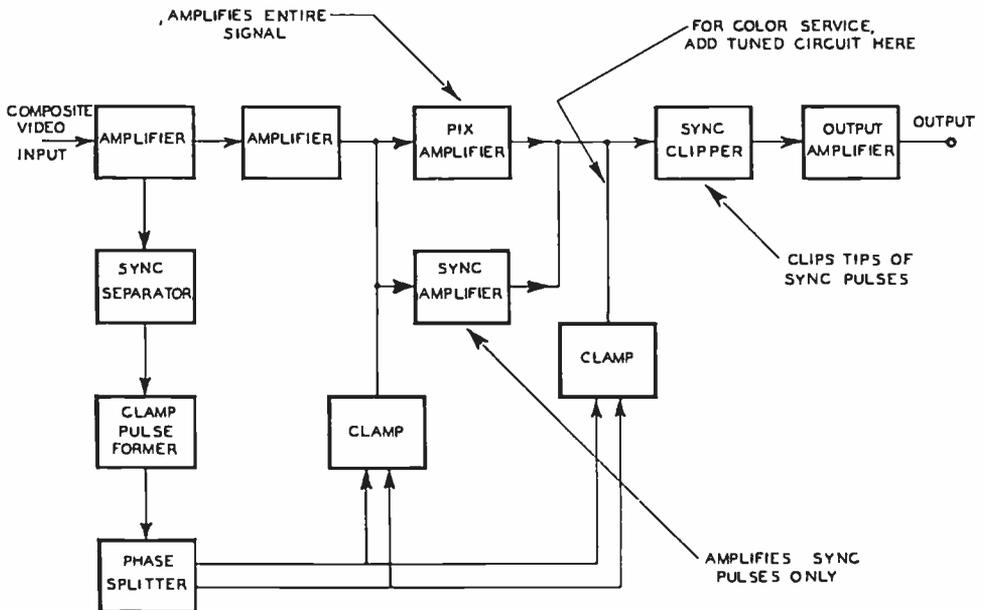
Fig. 46 — Simplified block diagram for a TA5B stabilizing amplifier.
