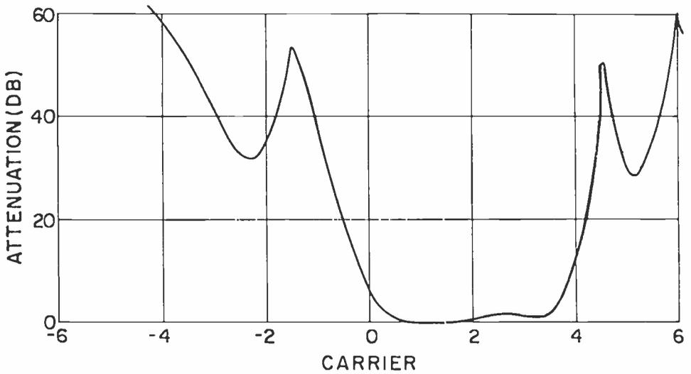
Fig. 6 – Selectivity characteristic of monochrome receiver.
