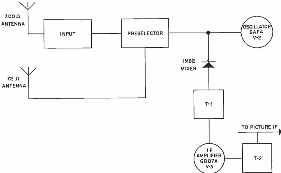
*Fig. 3b—RF tuner — UHF operation block diagram.*
