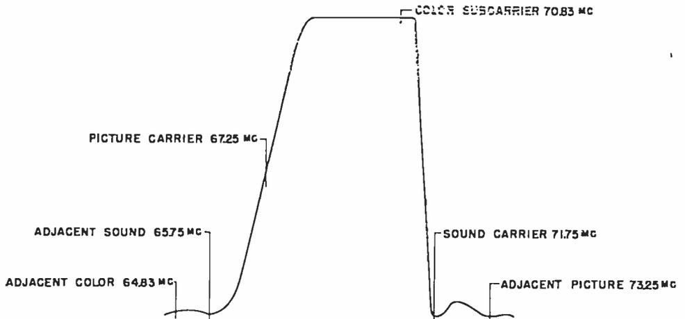
Fig. 3b—Overall RF-IF response channel 4.
