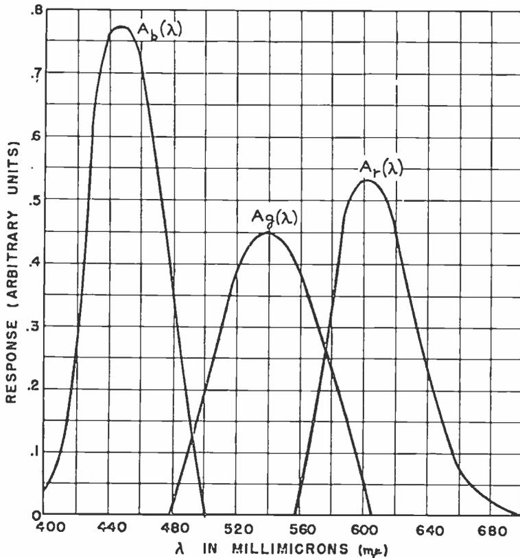
Fig. 9—Camera spectral sensitivities having only regions of positive response adjusted so that the areas under the curves are equal to those of Figure 7.
