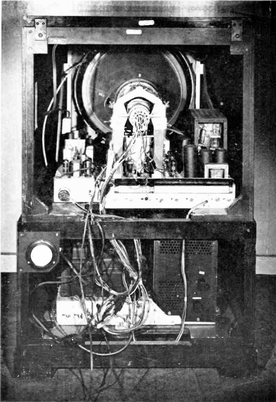
*Fig. 8 — 16-inch Tricolor Kinescope Receiver Model No. 2*
