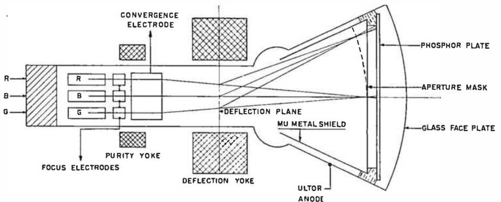
Fig. 14--Tricolor kinescope diagram.
