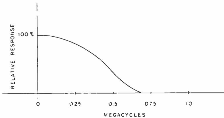
*Fig. 7—Q channel frequency response.*
