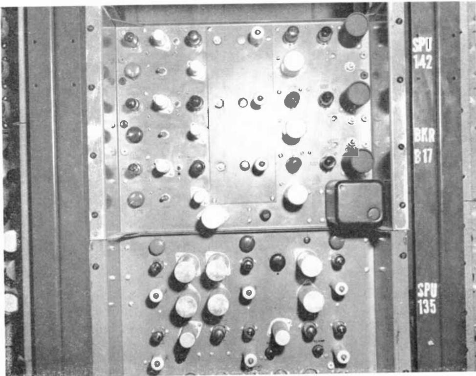
*Fig. 17 — Three-channel aperture compensator (upper chassis).*
