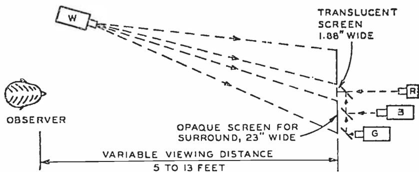
Fig. 3—Plan of eye-test apparatus.
