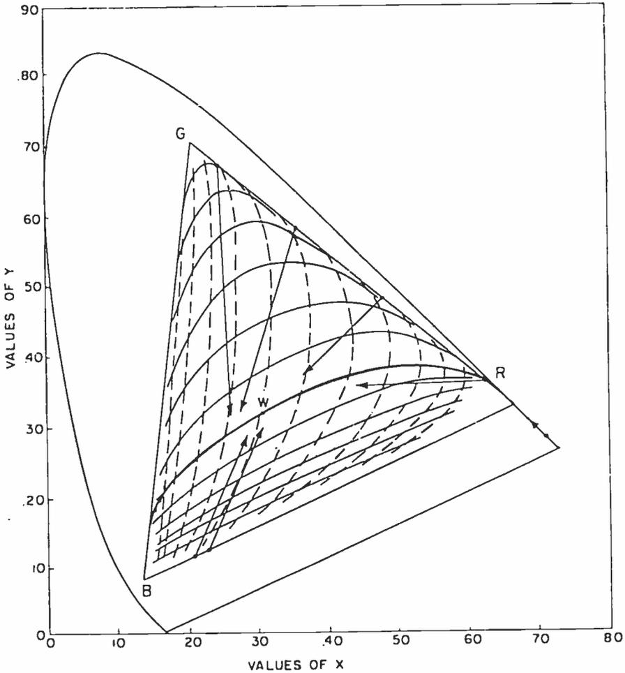
Fig. 6—Comparison of NTSC field test signal specifications with data of Hartridge.
