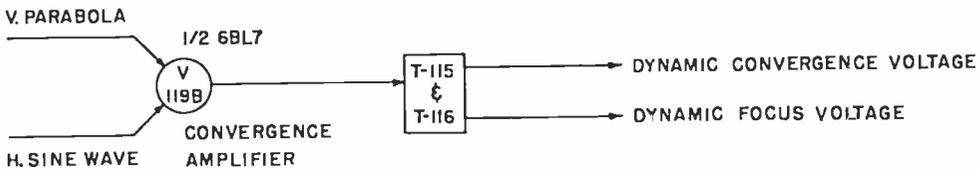
*Fig. 15—Dynamic convergence block diagram.*
