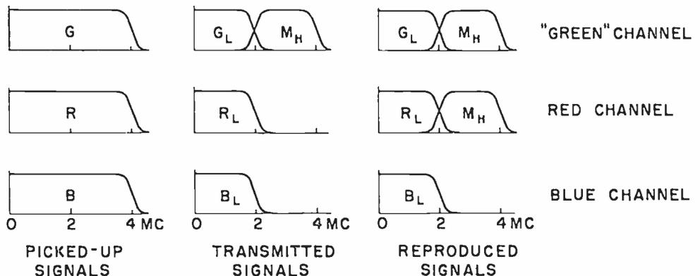
Fig. 8 - Spectra of the signals in the simultaneous-transmission system.
