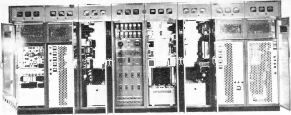
*Fig. 50—Front view of a TT5A television transmitter with doors open.*
