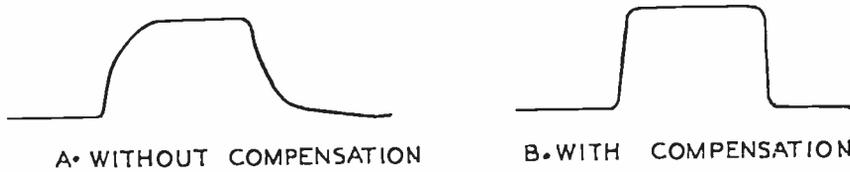
Fig. 27 — Waveforms resulting from the scanning of a white bar on a black background in a flying-spot scanner, showing the effect of phosphor decay time.
