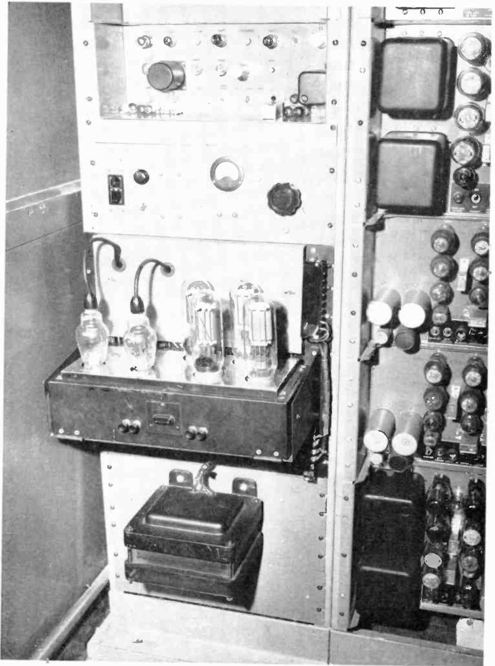
*Fig. 32 — Motor drive equipment for motion picture scanner.*
