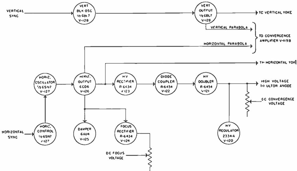
Fig. 13—Deflection and high voltage block diagram.
