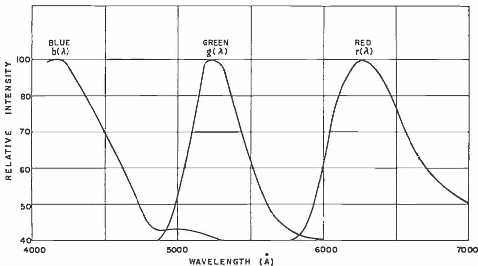
Fig. 5—Spectral characteristics of Red, Green, and Blue kinescopes (receiver primaries) plus dichroics and red filter.
