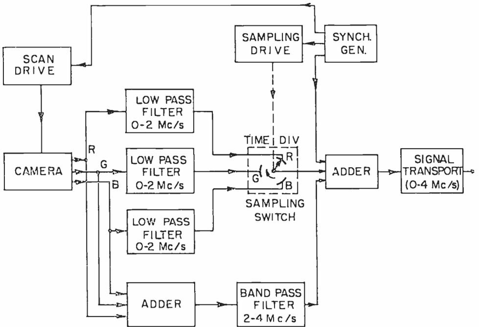
Fig. 9 — Early element-sequential transmission system.
