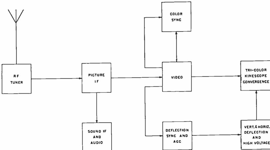
Fig. 2—Color television receiver master block diagram.
