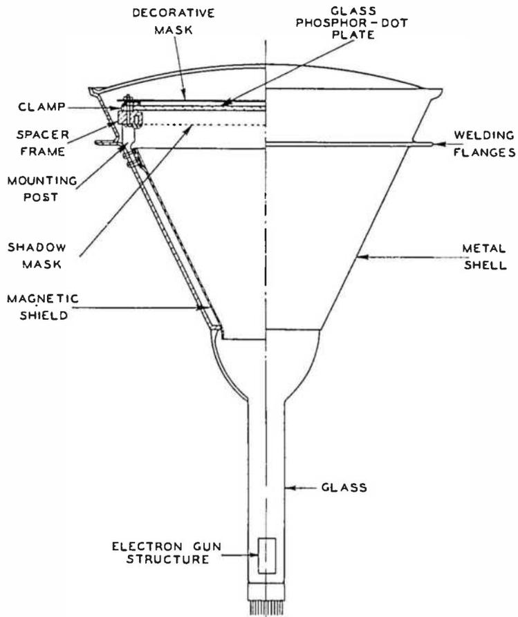
*Fig. 12 — Cross section of envelope — old design.*
