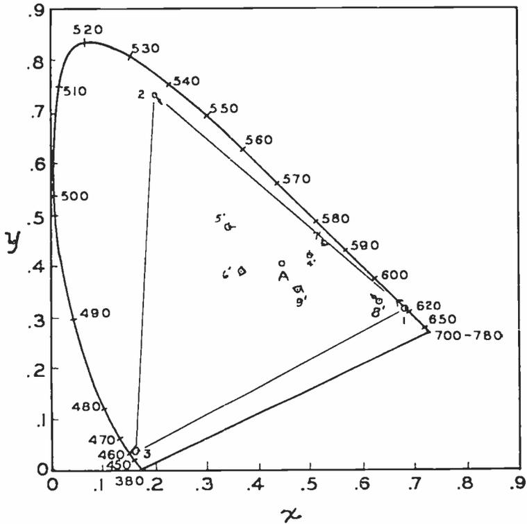
Fig. 18—Calculated chromaticity reproductions with receiver primaries of Figure 6, camera spectral sensitivities of Figure 10, and studio illuminant A (2848° K incandescent):
