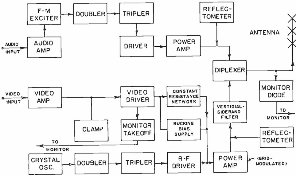
Fig. 49 — Simplified block diagram for a TT5A television transmitter.
