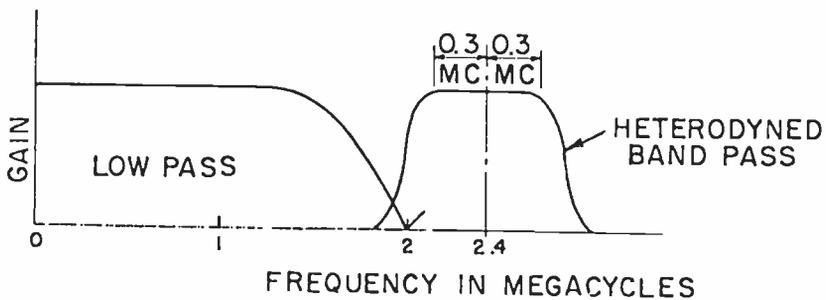
Fig. 4c - Heterodyned signal.
