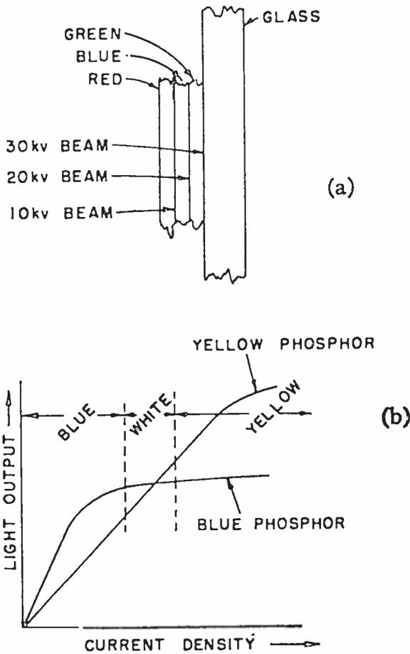
Fig. 4 — Multicolor phosphor screen: (a) shows a multiple-layer screen with color depending on beam velocity, and (b) shows how saturation in a two-component screen makes color dependent on current density.
