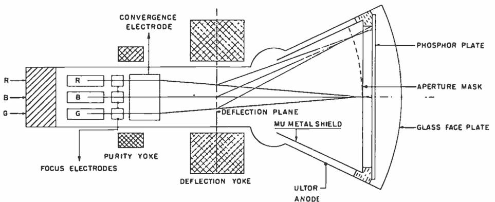
Fig. 13—Tricolor kinescope.
