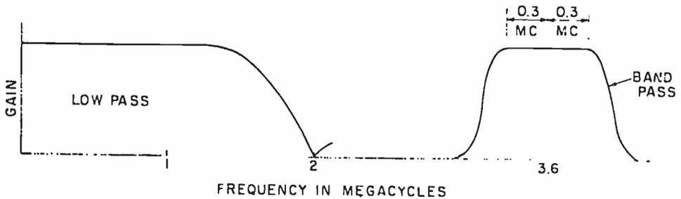
Fig. 6b - Heterodyned signal.
