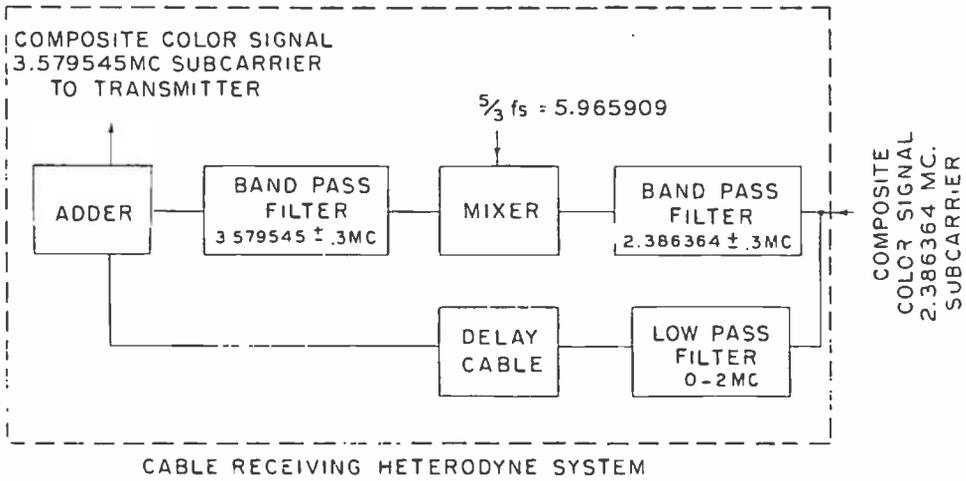
Fig. 12 - Cable receiving heterodyne system.
