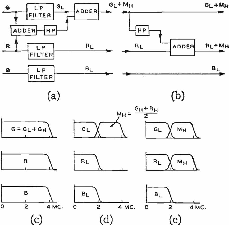
Fig. 1—Color television system with mixed highs. (a) Transmitter. (b) Receiver. (c) Pickup signals. (d) Transmitted signals. (e) Reproduced signals.
