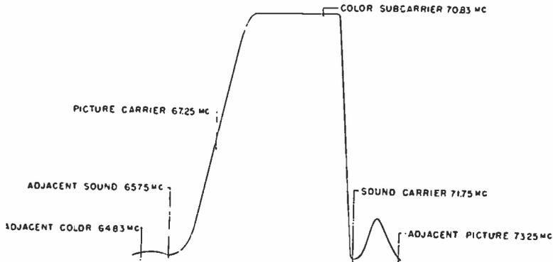
Fig. 4b—Overall RF-IF response channel 4.
