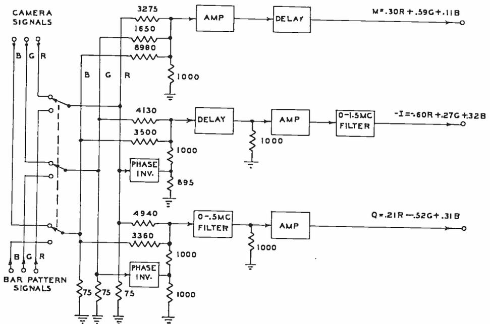
Fig. 34 — Block diagram for a colorplexer matrix section.
