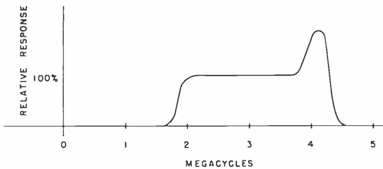
*Fig. 6—Band-pass filter response.*
