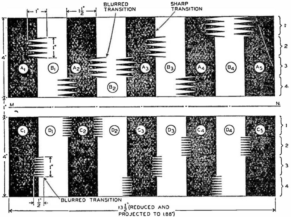
Fig. 2—Test pattern without surround, before reduction.
