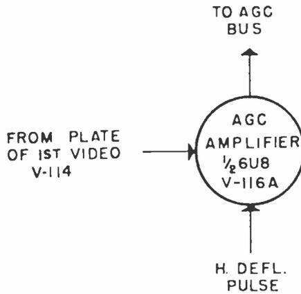
Fig. 12--AGC block diagram.
