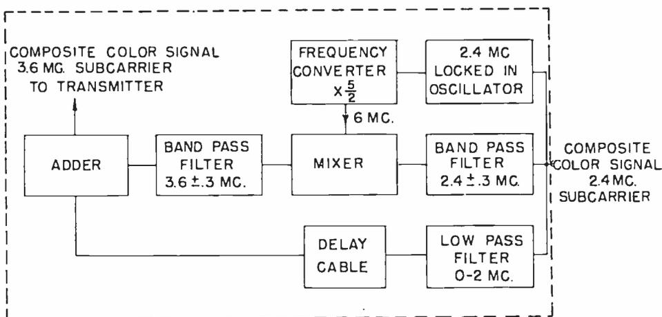
Fig. 5 — Cable receiving heterodyne system.
