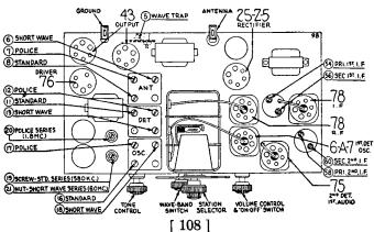
\*Use a 200-mmf. condenser in series as a dummy antenna on broadcast band and a 400-ohm carbon resistor on the shortwave band.
