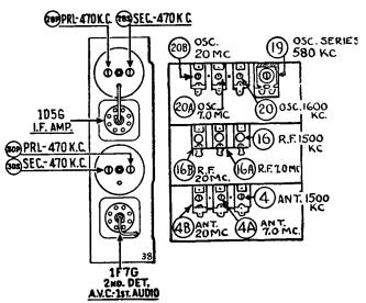
Note 1.—Dial adjustment—Turn variable condenser to maximum-capacity pobeam indicator is centered between first and second index lines at low-frequency end of broadcast scale. Then retighten set screw.
