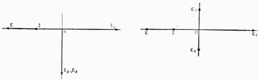
Fig. 7-27 (A), left, (B) right. Vector diagrams of the current and voltage relationships existing in the phase discriminator. Note that in (B) vector  $OE_3$  is shifted in phase by  $180^\circ$  from its position in (A).
