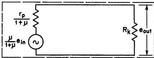
all of the output is fed back to the input. It is also out of phase with the input and may therefore be designated as  $b$  having a value of  $-1$ . The gain with feedback modifies Formula 116 and it should read:
