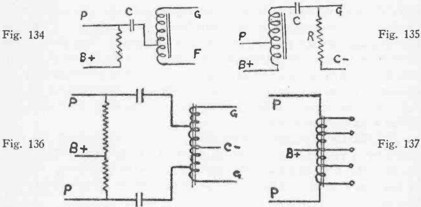
provided to adapt speakers of different electrical impedance or any number of speakers. Such output impedance units are more frequently used in public address and power amplifiers than in radio receivers.
