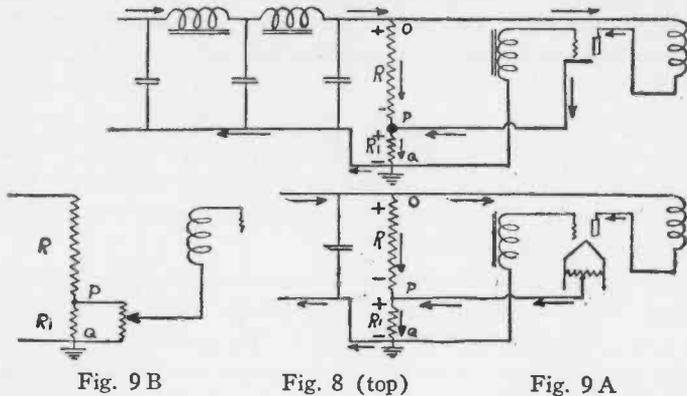
nected to the point Q and the cathode to the point P. The voltage across these two points is the voltage across the grid and the cathode, hence the negative grid bias.
