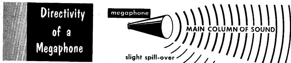
The directivity of a horn is dependent on its precise shaping. For example, a shape called the *tractrix*, which is nearly identical with the exponential shape, except at the mouth, is designed to produce hemispherical waves; in other words, to cover the entire  $180^\circ$  in front of its mouth. This ideal distribution from the tractrix only exists at the lower frequencies it radiates. At higher frequencies, the bell has progressively less effect.
