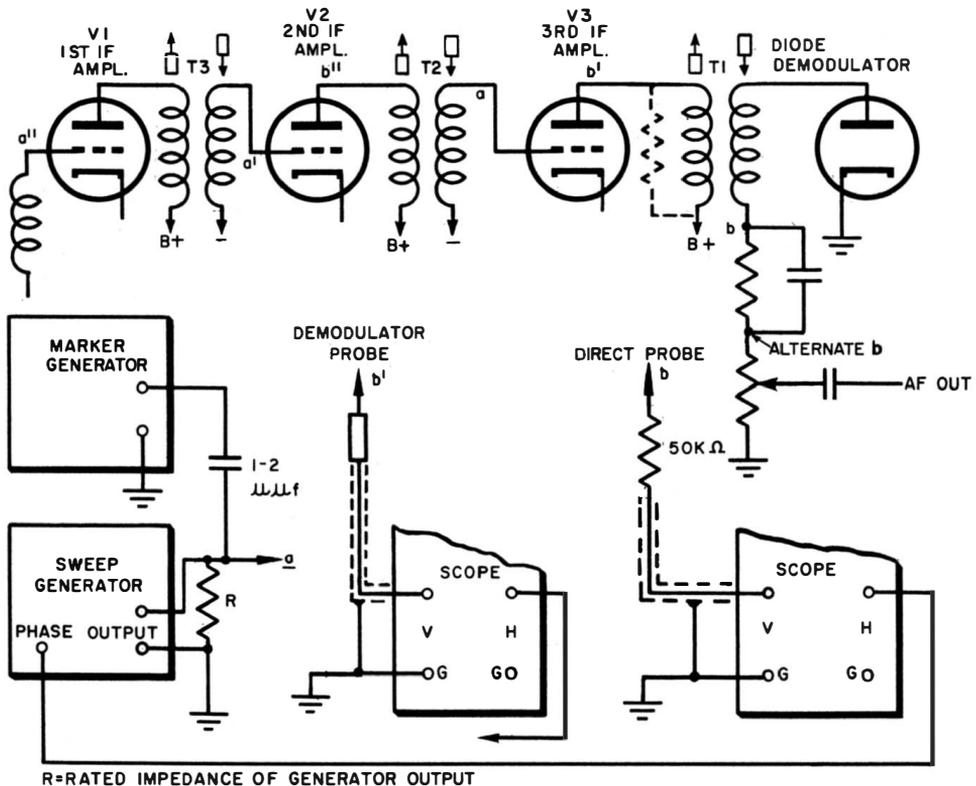
Fig. 11-10. I-F alignment setup combinations
