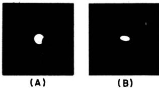
Fig. 8-4. Poorly focused beam spots.
