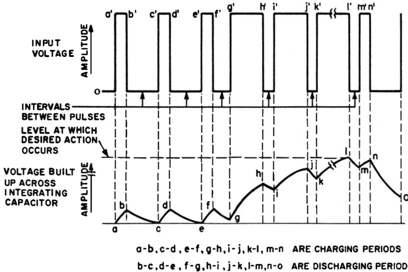
Fig. 5-6. How integration becomes cumulative to build up a single wide pulse from many narrower closely-spaced ones.
