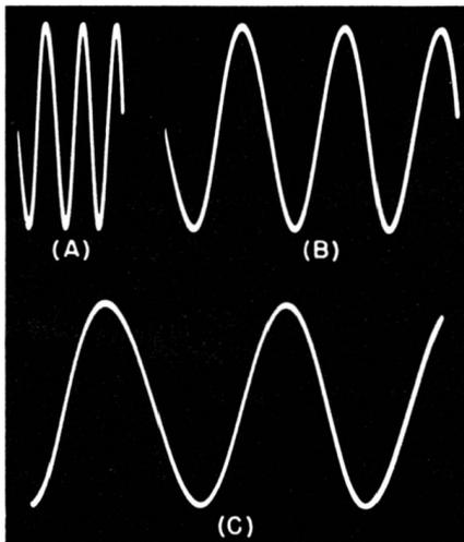
Fig. 8-11. Examples of effect on sine-waveform trace of adjustment of the horizontal gain control.
