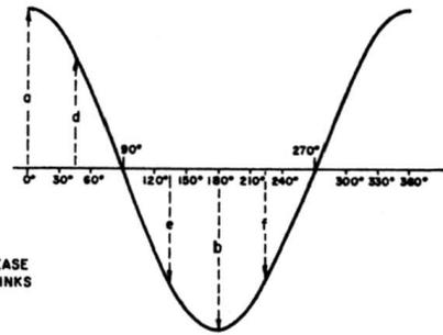
Fig. 1-2. The cosine waveform.
