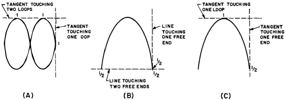
Fig. 10-10. Drawing tangents to check frequency ratio.
