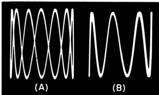
Fig. 8-20. Typical Lissajous patterns obtained when vertical voltage has a higher frequency than horizontal voltage, both being of sine waveform.
