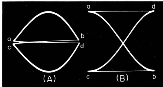
Traces (B), (C) and (D) in Fig. 8-16 and trace (B) in Fig. 8-17 represent exactly the same frequency ratio between the signal and the sweep voltages as in (A) in each case. The difference in appearance is attributable to a change in the phase relationship between the signal and sweep voltages.
