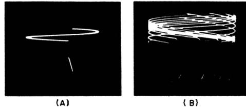
Fig. 8-22. Sawtooth waveform with peaking, as viewed with a sine wave horizontal sweep. (A) 1:1 frequency ratio; (B) non-integral frequency ratio.
