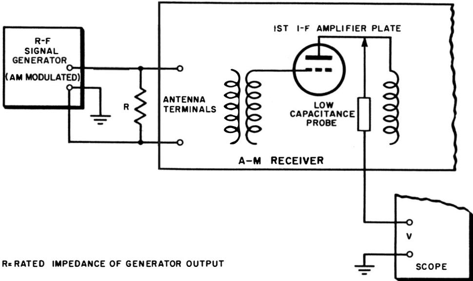
$R$  = RATED IMPEDANCE OF GENERATOR OUTPUT
