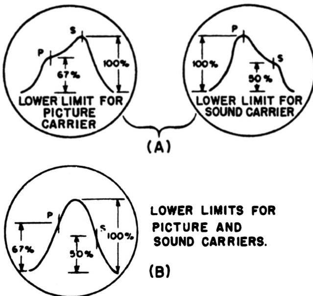
Fig. 7-10. Allowable deviations in the response curves of (A) low-frequency and (B) high-frequency channels.
