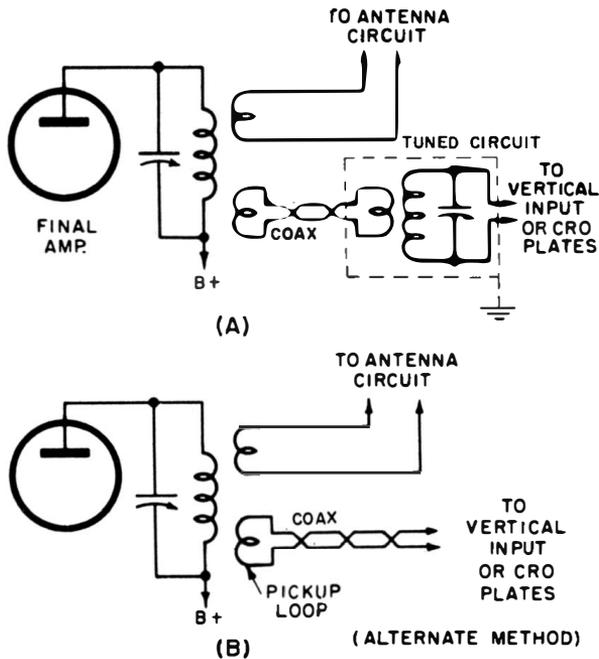
Fig. 11-13. Two methods of displaying modulated output from the transmitter.
