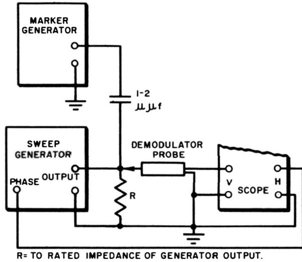
Fig. 11-7. Linearity-output test of sweep generator.
