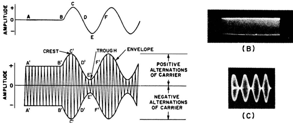
Fig. 6-1. Basic features of the amplitude-modulated waveform.
