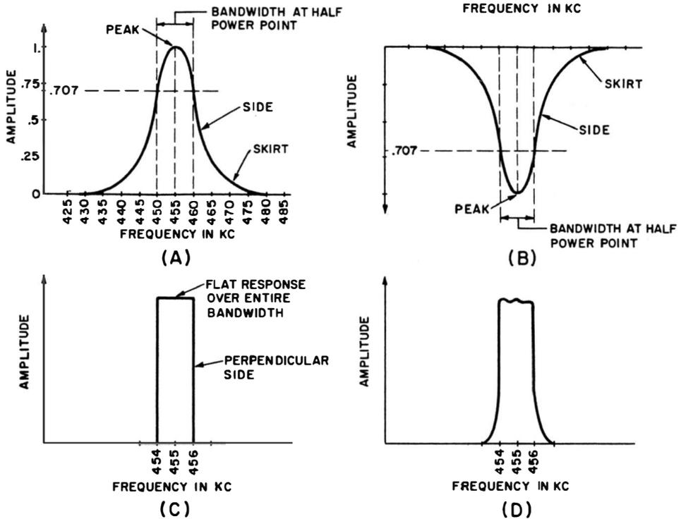
Fig. 7-1. (A) Basic features of response curve, (B) ideal response.
