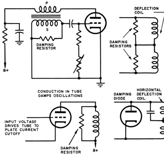
Fig. 9-4. Typical circuits in which damping action influences waveform.
