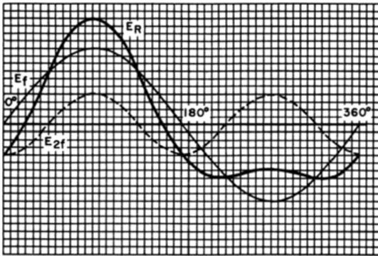
Fig. 1-4. Wave resulting from combination of fundamental and second harmonic 90° out of phase.
