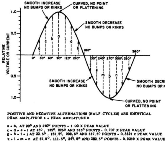
Fig. 1-1. Development and important ideal features of a sine waveform.
