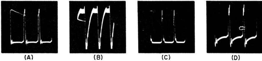
Fig. 9-38. Traces (A), (B), (C) and (D) illustrate waveforms at the input to the filter system in a tripler type of high voltage power supply. Trace (A) is the normal waveform and (B) illustrates the effect of an open in the doubling capacitor. Trace (D) illustrates the waveform when the tripling capacitor is open. Trace (C) shows the effect of an open in one of the filament path capacitors.
