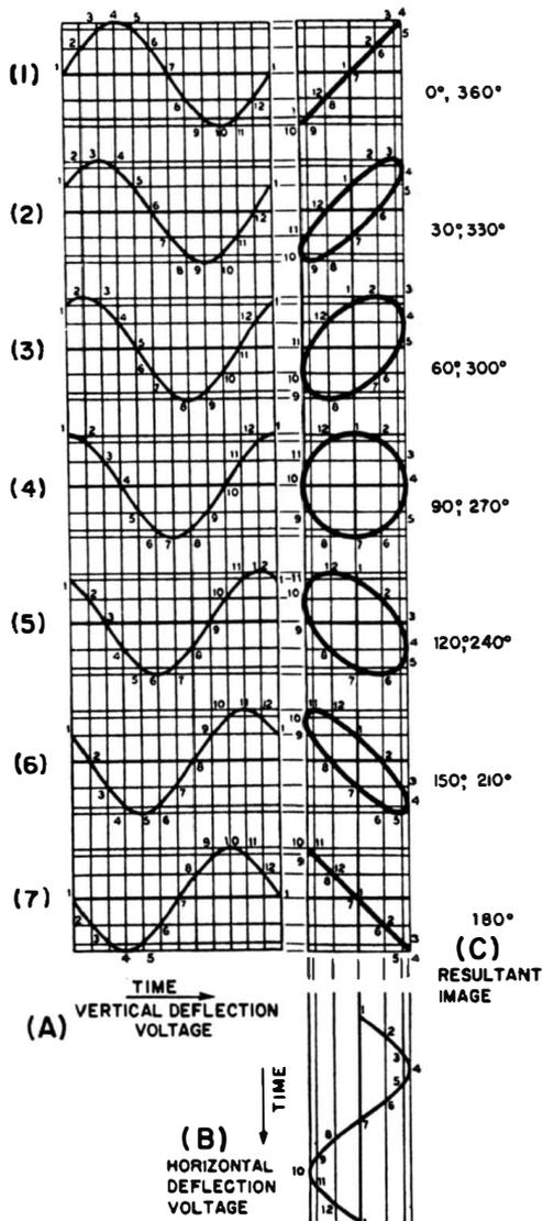
Fig. 8-18. Types of patterns when both horizontal sweep and signal (vertical) voltages have sine waveforms.
