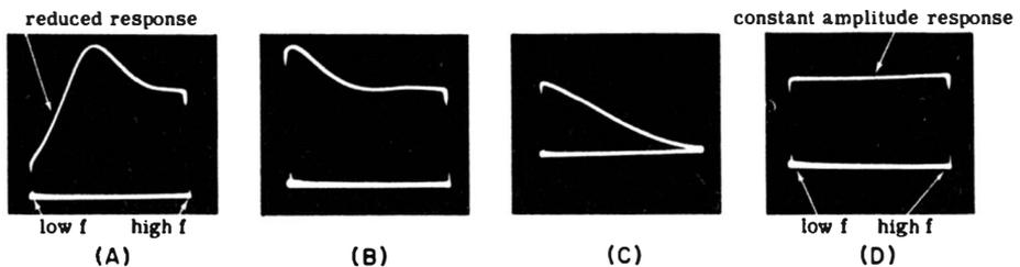
Fig. 9-53. Trace (A) shows severe attenuation over the lower third of the frequency passband, with a peak towards the center of the band. Trace (B) shows a peak at the low frequency end and gradual reduction to about the middle of the channel, then linear response. Trace (C) shows a marked reduction in signal transfer and a reduction to substantially zero response at the high end of the passband of the channel.
