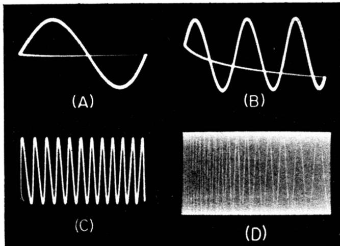
Fig. 8-13. Effect of signal-to-sweep frequency ratio.
