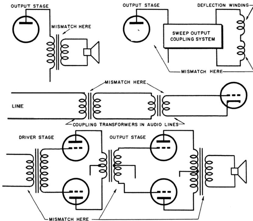
Fig. 9-3. Some systems in which mismatching of impedances can cause distorted waveform.
