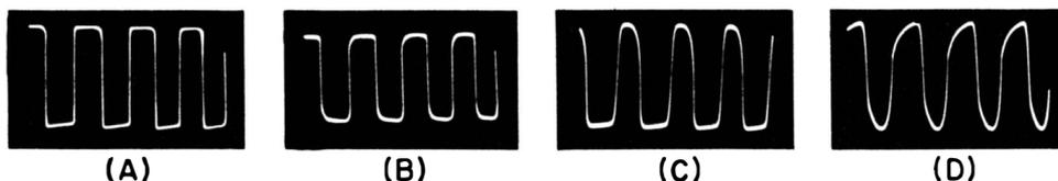
Fig. 9-30. Traces (A) and (B) are the square waveforms obtained from the two plate circuits in a cathode-coupled symmetrical multivibrator. In traces (C) and (D) are shown the effects of changing the grid return resistor—lowering its value. The changes in waveform are not interpretable in terms of frequency composition, rather in the intervals of tube condition in the system.
