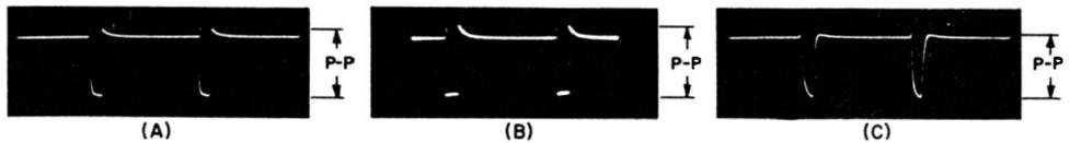
Fig. 9-31. The voltage is a 50-microsecond pulse repeated 4000 times per second. Trace (A) is the output waveform after passage of this signal through a circuit with a 500-kc passband; (B) is the result with a 100-kc passband and (C) is the output for about a 40-kc passband. The overshoot is a consequence of charging the blocking capacitor in the circuit.
