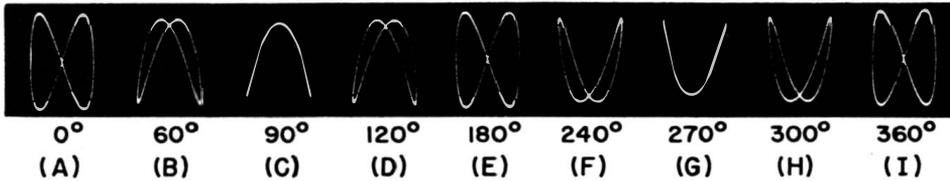
Fig. 10-8. Traces resulting when the signal to the vertical plates has twice the frequency of the signal on the horizontal plates.
