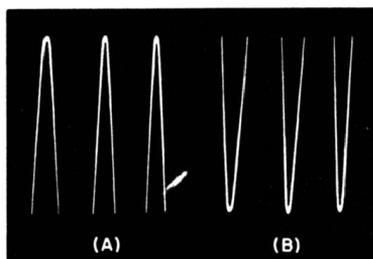
Fig. 8-7. Top (A) and bottom (B) portions of a single expanded sine wave trace. The portions can in this way be examined in greater detail than when one smaller trace including both is used.
