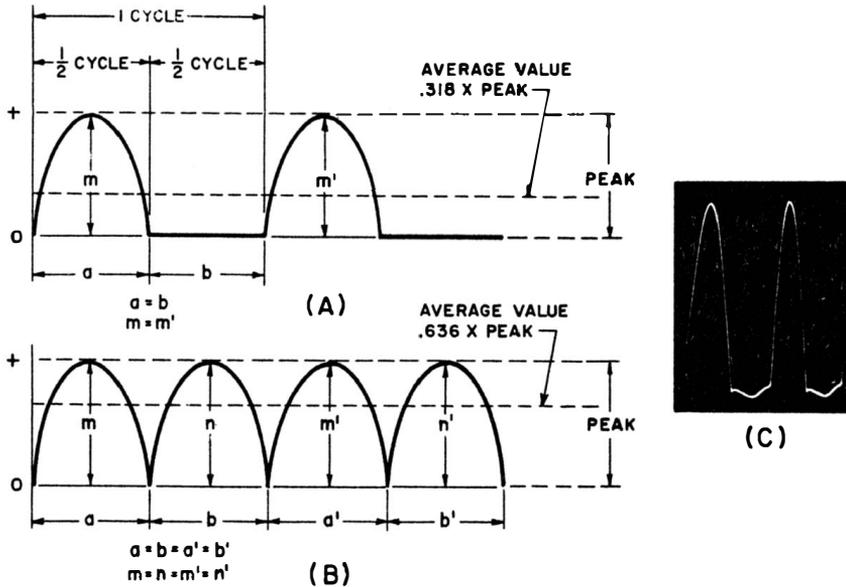
Fig. 1-11. Examples of half-sine waveforms resulting from rectification.
