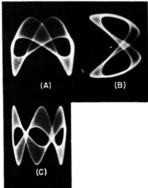
if the trace for 9:8 frequency ratio in Fig. 10-20 is examined, it will be found that it consists of 4 complete loops and 1 free end on top and 4 complete loops on one side and 3 complete loops and 2 free ends on the other. In one case it is  $4\frac{1}{2}:4$  and in the other it is  $4 : (3+\frac{1}{2}+\frac{1}{2})$  or again  $4\frac{1}{2}:4$ , which, if both sides are multiplied by 2, becomes 9:8.
