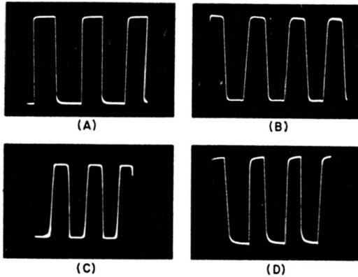
Fig. 2-5. Examples of square waves indicating insufficient high frequency response.
