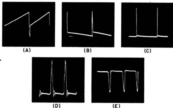
Fig. 4-7. Variations of trapezoidal waveforms.
