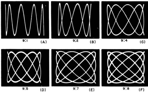
Fig. 10-20. (A) 9:1 frequency ratio, (B) 9:2 frequency ratio, (C) 9:4 frequency ratio, (D) 9:5 frequency ratio, (E) 9:7 frequency ratio, (F) 9:8 frequency ratio.
