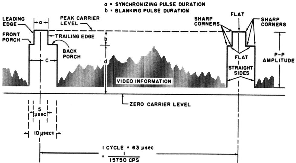
Fig. 3-3. Parts, proportions, and ideal features of rectangular wave used for tv sync.
