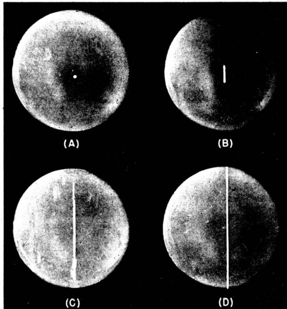
Fig. 8-8. Effect of adjustments of vertical gain control.
