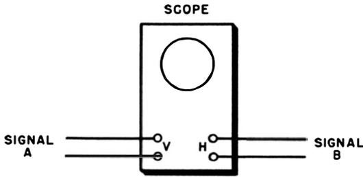
Fig. 10-1. Basic setup for deriving Lissajous figures.
