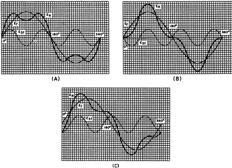
Fig. 1-8. Effect on sine waveform of addition of third harmonic (at amplitude =  $\frac{1}{3}$  of fundamental) at phases of (A)  $0^\circ$ , (B)  $180^\circ$ , and (C)  $270^\circ$ .
