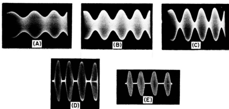
Fig. 6-4. Waveforms representing various percentages of amplitude modulation.
