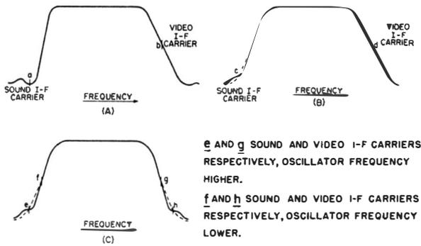
Fig. 7-12. Ideal overall video i-f response curve: (A) for the conventional type of receiver; (B) for the intercarrier type of receiver; and (C) for the intercarrier type which tunes above and below the incoming signal.
