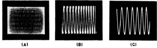
Fig. 8-24. Three stages of patterns as the fine frequency control is adjusted for synchronization.
