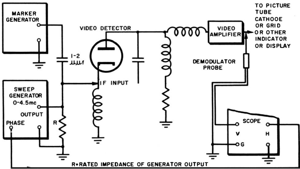
Fig. 11-12. Video response-checking setup.
