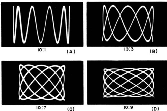
Fig. 10-21. (A) 10:1 frequency ratio, (B) 10:3 frequency ratio, (C) 10:7 frequency ratio, (D) 10:9 frequency ratio.
