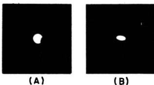
Fig. 8-4. Poorly focused beam spots.
