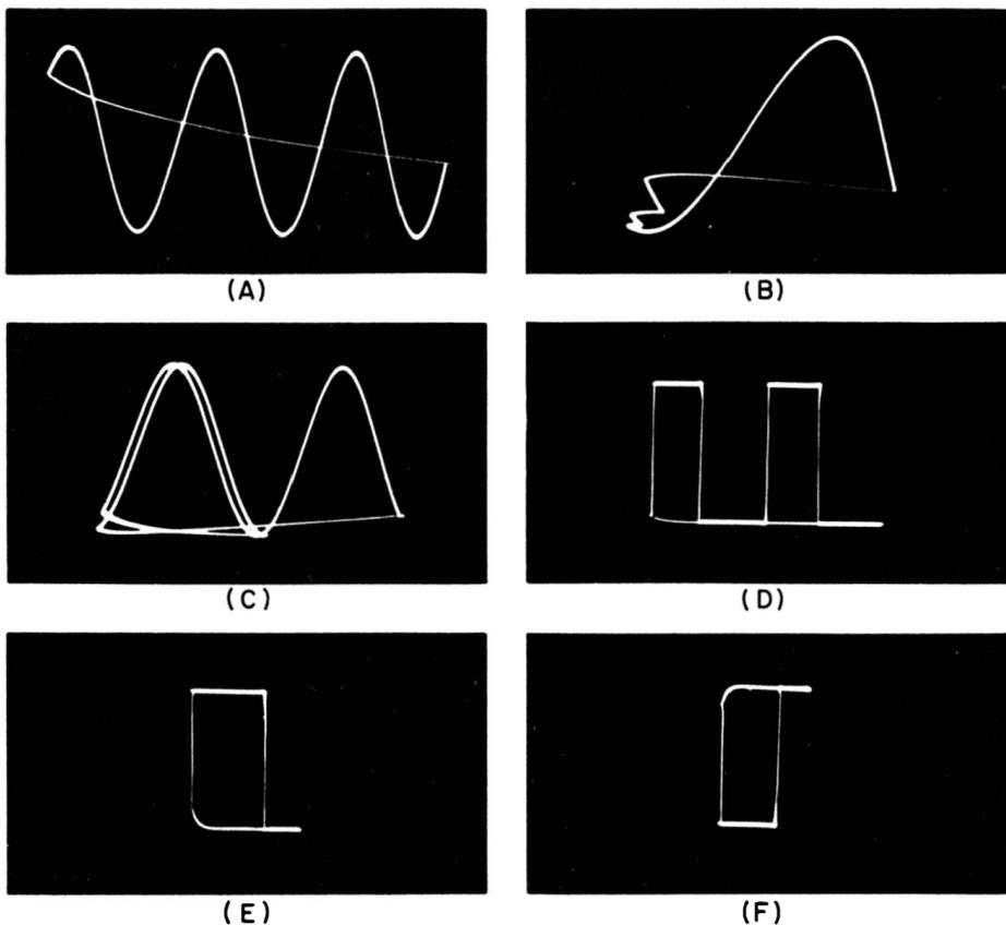
Fig. 8-26. Results of excessive sync voltage.
