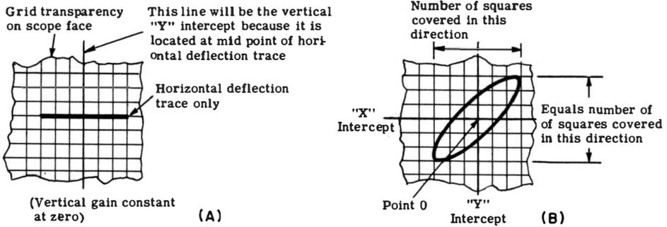
Fig. 10-4. How to set the scope for measurement of phase differences.
