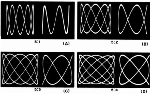
Fig. 10-16. (A) 5:1 frequency ratio, (B) 5:2 frequency ratio, (C) 5:3 frequency ratio, (D) 5:4 frequency ratio.
