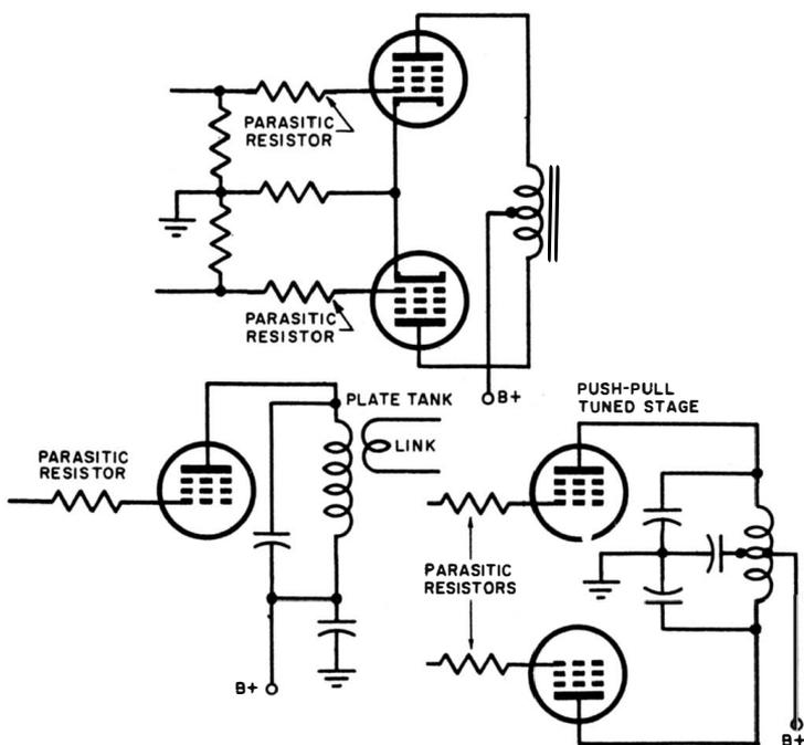
Fig. 9-5. Circuits in which parasitic oscillations may occur to distort waveform, and location of suppressor resistors for eliminating them.
