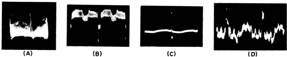
Fig. 9-34. Trace (A) is a buzz voltage waveform as seen in front-end tuned circuits. Trace (B) is a buzz waveform in i-f coils. Trace (C) is a buzz voltage seen in video amplifiers, and trace (D) is an example of a buzz waveform in audio amplifiers.
