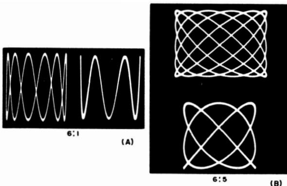
Fig. 10-17. (A) 6:1 frequency ratio, (B) 6:5 frequency ratio.
