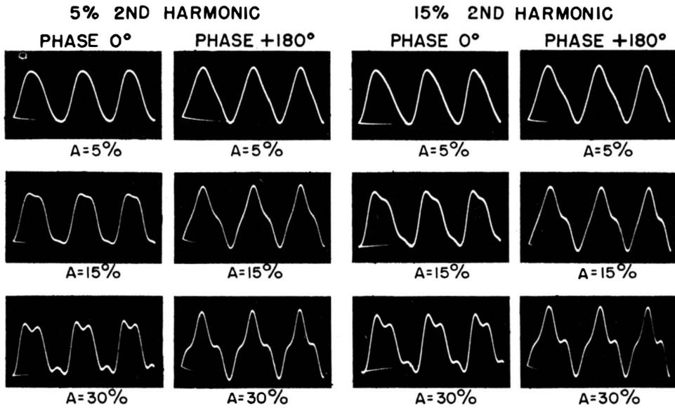
**Fig. 1-10. Effect on sine waveform of addition of both second and third harmonics. In each case, either 5 or 15 per cent (as indicated) second harmonic at 0° phase is present. Then third harmonic is added in amount indicated as A and in phase indicated above each column.**
