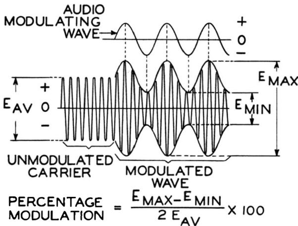
Fig. 6-3. Waveform of r-f wave amplitude-modulated 50 per cent.
