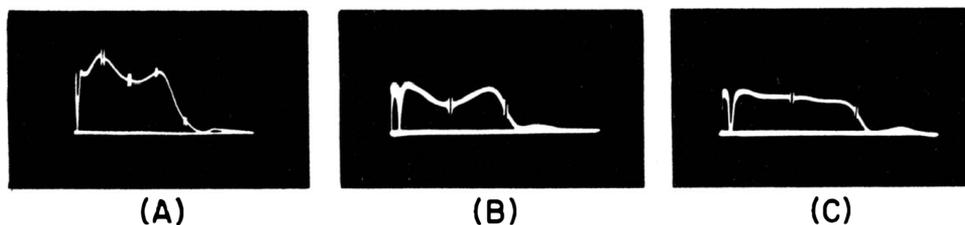
Fig. 7-18. Reference video amplifier response curves.
