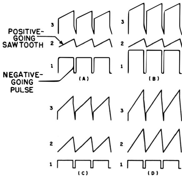
Fig. 4-6. Formation of trapezoidal waveform (3) by combining rectangular (1) and sawtooth (2) waveforms.
