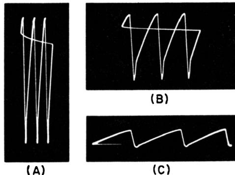
Fig. 8-12. How improper proportioning of the trace may cause loss of important detail.
