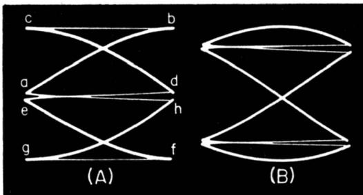
Fig. 8-17. Sine wave trace with sawtooth sweep four times signal frequency, for two phase relations.
