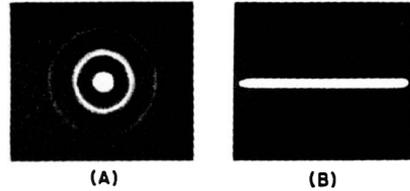
Fig. 8-3. Result of excessively high brightness control adjustment.
