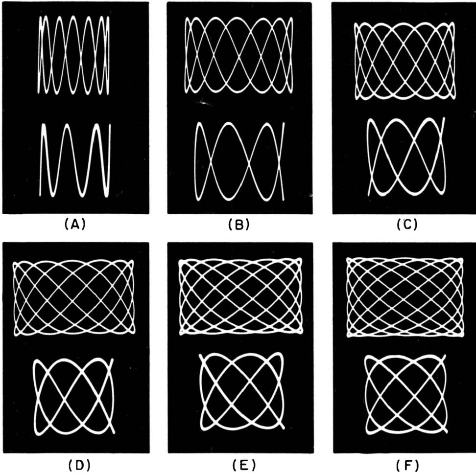
Fig. 10-18. (A) 7:1 frequency ratio, (B) 7:2 frequency ratio, (C) 7:3 frequency ratio, (D) 7:4 frequency ratio, (E) 7:5 frequency ratio, (F) 7:6 frequency ratio.
