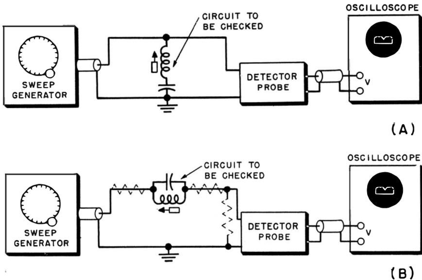
Fig. 11-3. Resonant frequency determination.
