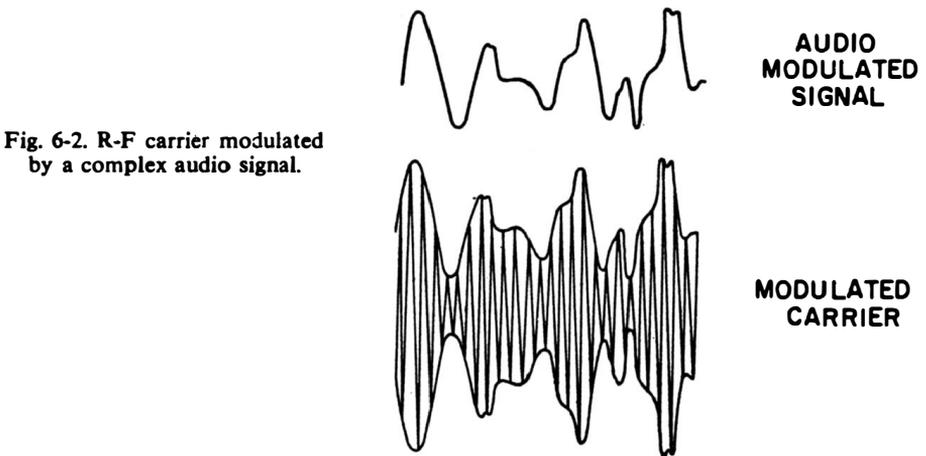
Fig. 6-2. R-F carrier modulated by a complex audio signal.
