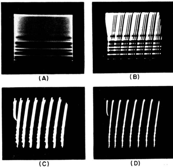
Fig. 8-25. Stages approaching synchronization of a sawtooth waveform.
