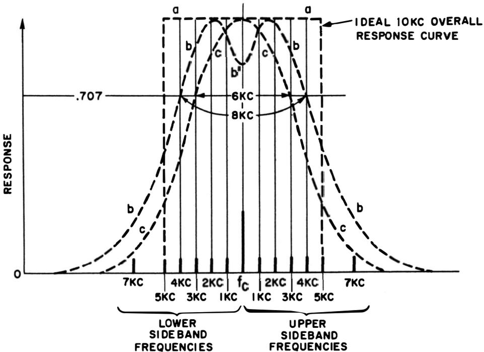
Fig. 7-6. Frequency distribution in an a-m signal with modulating tones of 1, 2, 3, 5 and 7 kc, and ideal and practical response curves.
