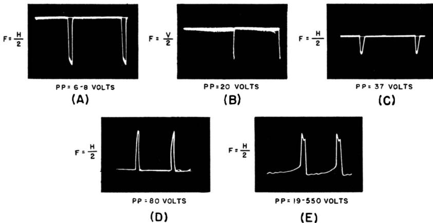
Fig. 3-2. Practical rectangular waveforms.
