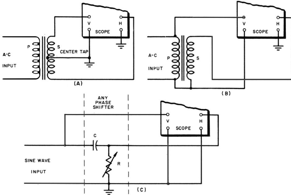
Fig. 11-4. Checking phase shift in transformers and phase-shifting network.
