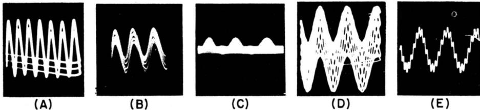
Fig. 9-9. Examples of scope trace when spurious or hum signal is present on vertical plates. Note amplitude modulation of signal cycles in (A). The trace in (C) appears to rotate around its horizontal axis. In (D) the spurious signal has a lower frequency than the vertical input signal. In (E) the spurious signal has a higher frequency than the vertical input signal.
