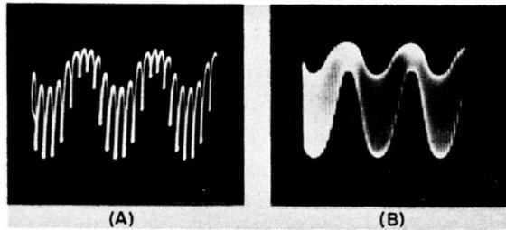
Fig. 6-8. Intermodulation waveforms.
