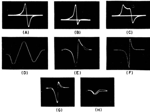
Fig. 9-54. Trace (A) is the normal shape of an “S” curve. Traces (B) and (C) are examples of incorrect alignment of the discriminator transformer. Misalignment of the primary usually results in a change in shape of the “S” curve, whereas misalignment of the secondary results in zero voltage being produced at some frequency other than the intermediate frequency.
