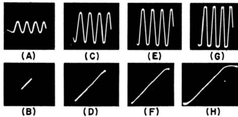
$A$  and  $B$  in Fig. 10-5 is simply the numerical ratio of the lineal dimensions  $A$  and  $B$  as measured on the grid transparency. The value of  $\sin \theta$  for the ratio  $A/B$  is determinable from any table of sines and cosines. Thus if  $A/B$  equals 0.7, the phase difference is 45 degrees or 315 degrees. Other typical values are indicated in Fig. 10-5.
