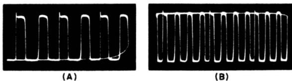
Fig. 8-14. Effect of signal-to-sweep frequency ratio on typical square waveforms.
