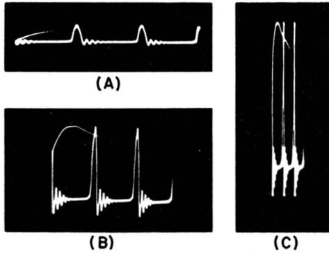
Fig. 8-9. Variations of waveform trace with adjustment of vertical gain control.
