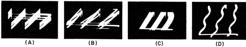
Fig. 9-41. Traces (A) and (B) illustrate the effect on a sawtooth waveform when 60-cps hum voltage is present on the vertical deflection plates. Trace (C) shows 60-cps or 120-cps hum on the horizontal plates of the scope.
