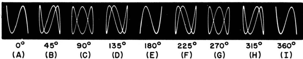
Fig. 10-11. Vertical signal frequency three times horizontal frequency.
