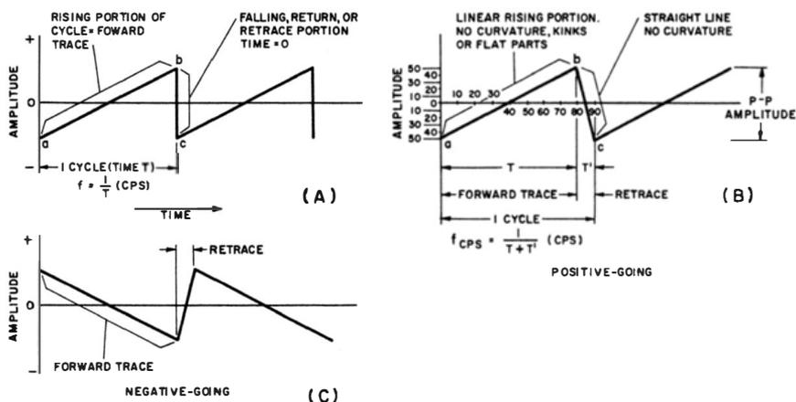
Fig. 4-1. Features of ideal sawtooth waveforms.
