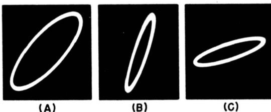
Fig. 10-2. Effect of relative amplitudes of component signals. (A), (B) and (C) represent 45 degrees.
