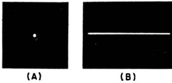
Fig. 8-2. Properly-focused dot (A) and horizontal line trace (B).
