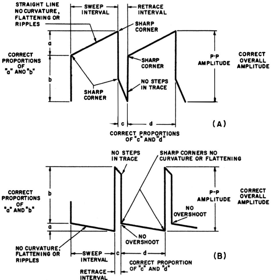
Fig. 4-8. Differences between trapezoidal waveforms in (A) sweep oscillator and shaping circuits and (B) sweep output circuits.
