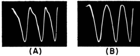
Fig. 9-14. Distortion of sine waveform when frequency is too low for transformer.
