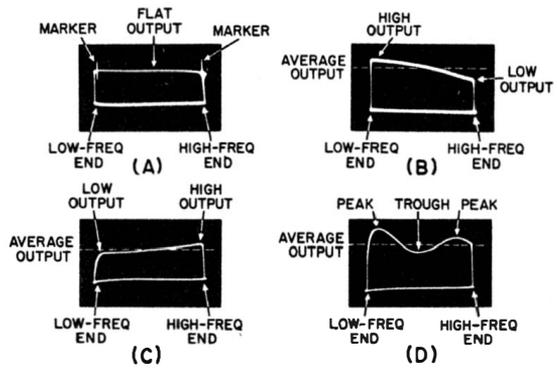
Fig. 7-19. Sweep generator voltage output curves.
