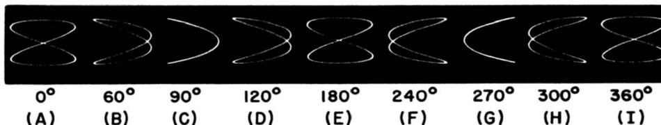
Fig. 10-9. Traces resulting when the signal to the horizontal plates has twice the frequency of the signal on the vertical plates.
