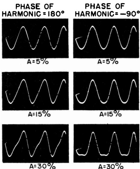
Fig. 1-6. Effect on fundamental sine waveform of addition of second harmonic in different amounts and  $180^\circ$  and  $-90^\circ$  phases. A = per cent second harmonic.
