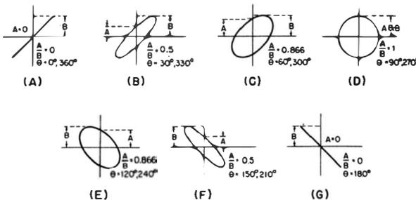
Fig. 10-5. Calculating phase angle from scope pattern.
