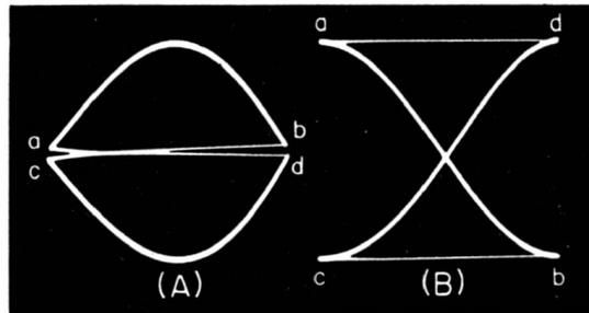
Traces (B), (C) and (D) in Fig. 8-16 and trace (B) in Fig. 8-17 represent exactly the same frequency ratio between the signal and the sweep voltages as in (A) in each case. The difference in appearance is attributable to a change in the phase relationship between the signal and sweep voltages.
