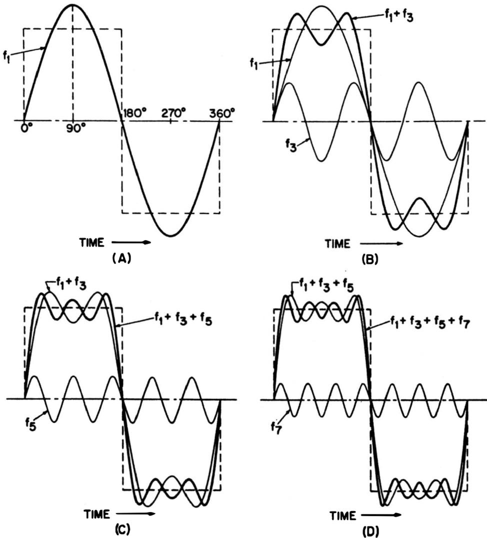
Fig. 2-2. Oscillograms showing the gradual change in waveform to a square wave as 3rd, 5th, and 7th harmonics are added to a sine waveform fundamental.
