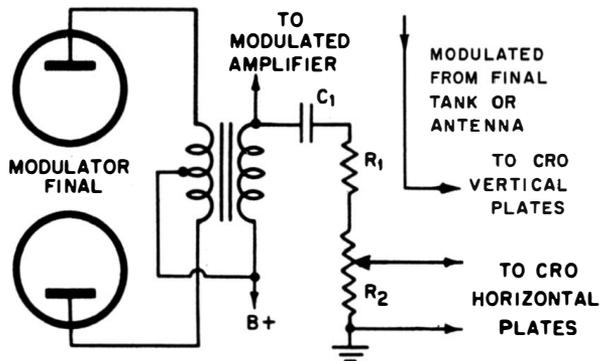
Fig. 11-14. Trapezoid-method for checking modulation percentage.
