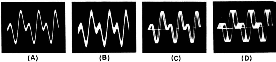
Fig. 9-22. Traces (A) and (B) show the distortion of a complex voltage waveform when hum is present on the vertical deflection plates. The hum affects the trace in the vertical direction. Traces (C) and (D) show the same complex waveform when hum is present on the horizontal deflection plates.
