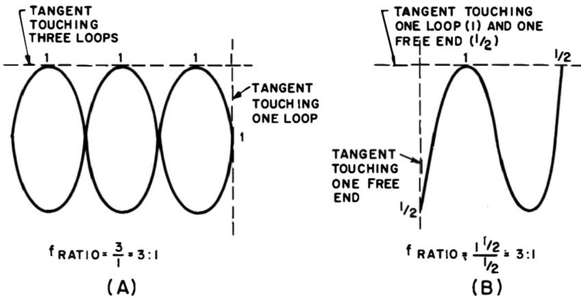
Fig. 10-13. How tangents are used to check 3:1 frequency difference.
