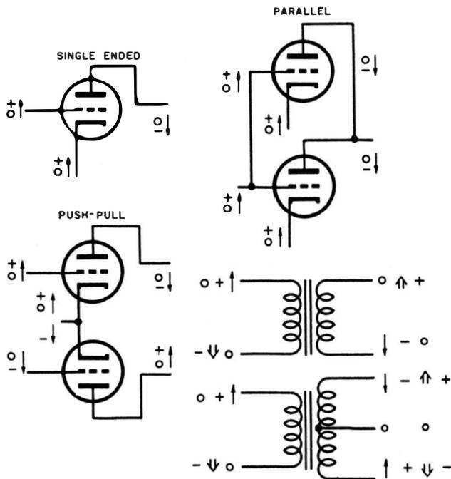
Fig. 9-8. Inversion of signal voltage in single-ended, push-pull and parallel tube systems.
