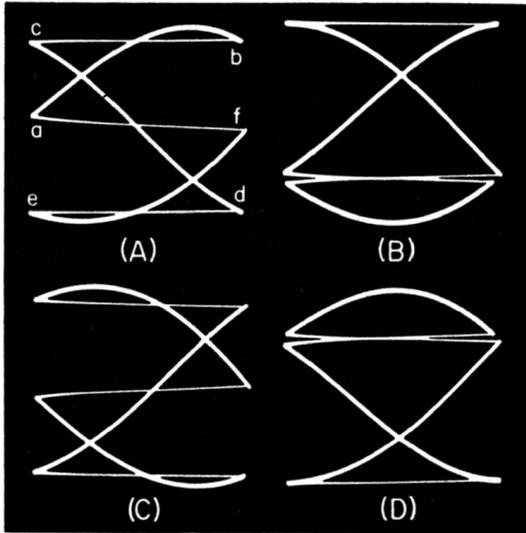
Fig. 8-16. Sine wave trace viewed with sawtooth sweep frequency three times sine-wave frequency, for four different sweep-to-signal phase relations.
