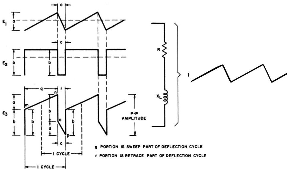
Fig. 4-5. How resistive voltage component  $E_1$  and inductive voltage component  $E_2$  combine in a practical inductor to form the trapezoidal resultant  $E_3$ .
