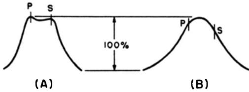
Fig. 7-9. Reference r-f response waveforms for (A) low-frequency, (B) high-frequency tv channels.
