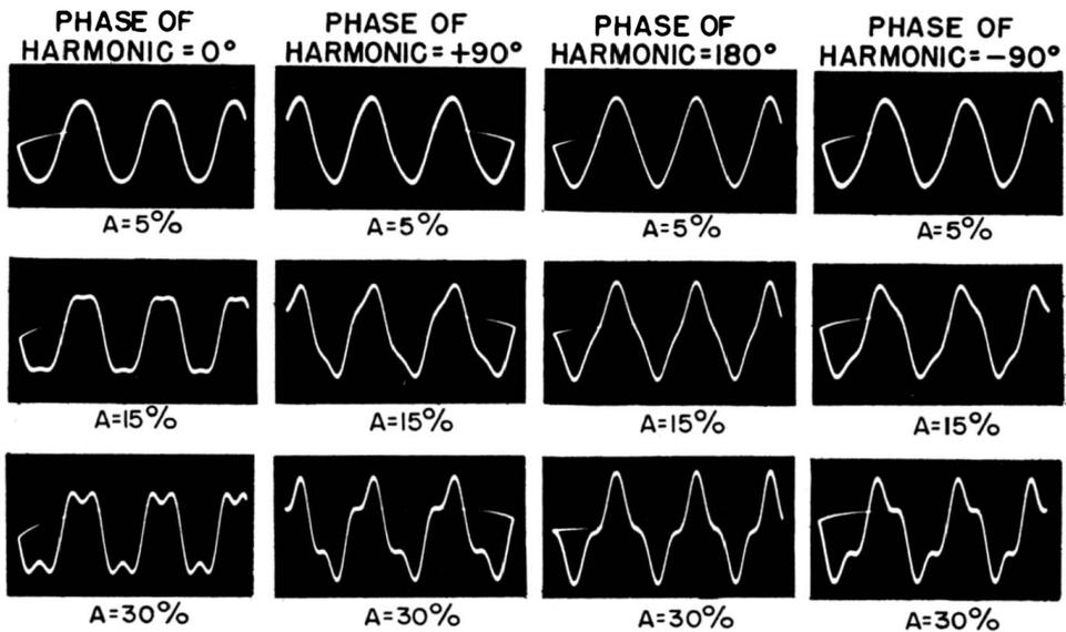
Fig. 1-9. Effect on sine waveform of third harmonic in different amounts and in four different phase relations. As before  $A =$  per cent harmonic.
