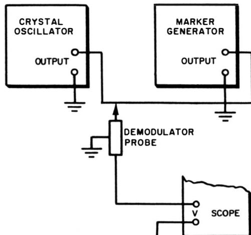
Fig. 11-8. Check of marker generator accuracy by beating against crystal oscillator harmonics.
