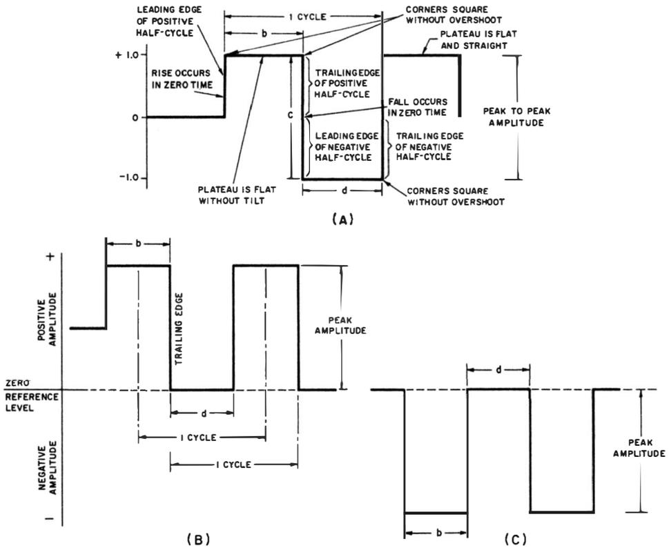
Fig. 2-1. A-c and unidirectional forms of the square wave.
