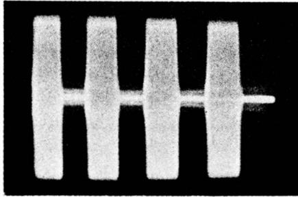
Fig. 6-5. Waveform of r-f wave modulated by a square wave.
