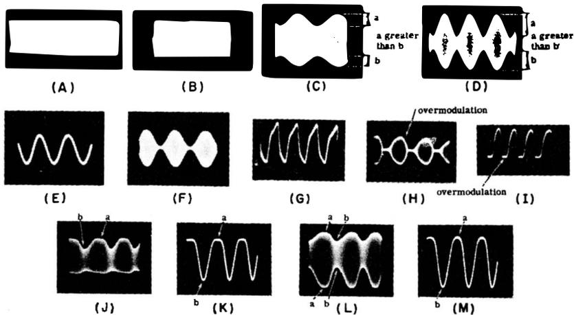
Fig. 9-46. Traces (A) and (B) show the unmodulated carrier (A) and the modulated carrier (B) as rectangular traces.
