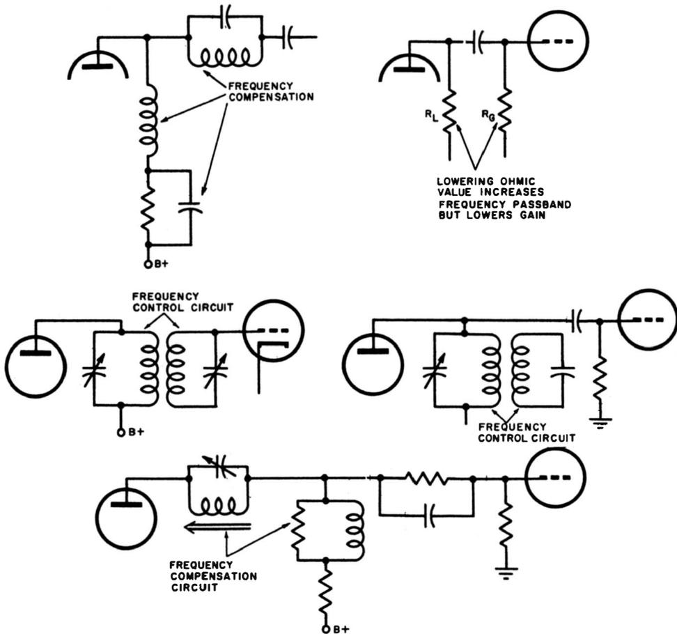
Fig. 9-1. Typical circuits in which signal can be distorted by improper action of resonant circuits.
