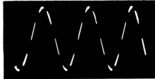
Fig. 9-20. This shows the appearance of a sine waveform when a higher frequency signal is applied to the intensity-modulating grid of the scope's cathode-ray tube. The intensity modulation separates the trace into segments. The higher the frequency of the intensity-modulating signal the greater the number of segments.
