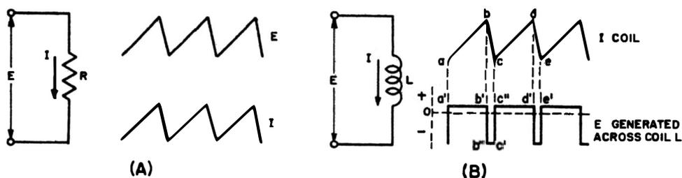
Fig. 4-4. Difference between current through a resistor (A) and an inductor (B) for applied sawtooth waveform.
