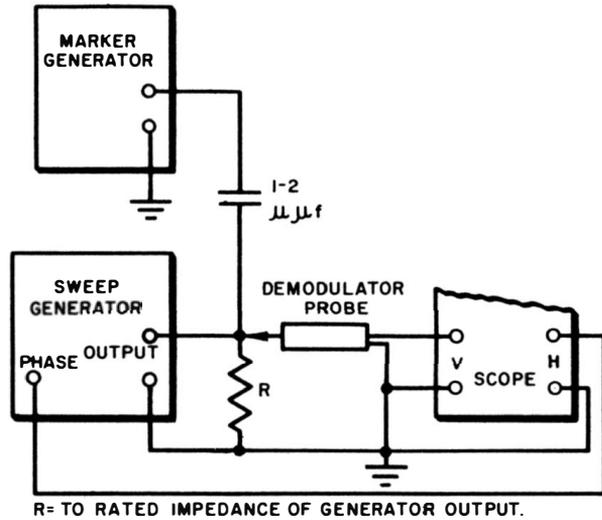
Fig. 11-7. Linearity-output test of sweep generator.
