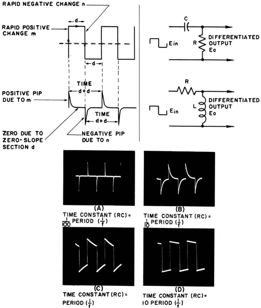
Fig. 5-1. Basic differentiating process and results of differentiation of a square wave when RC network has different time constants.
