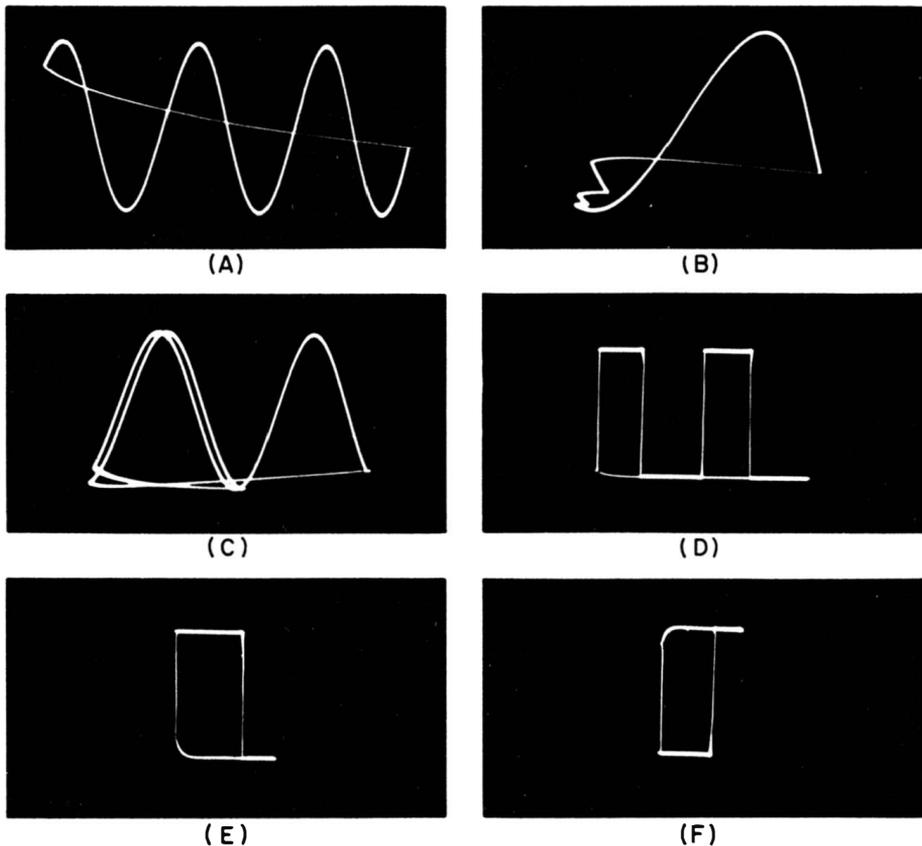
Fig. 8-26. Results of excessive sync voltage.
