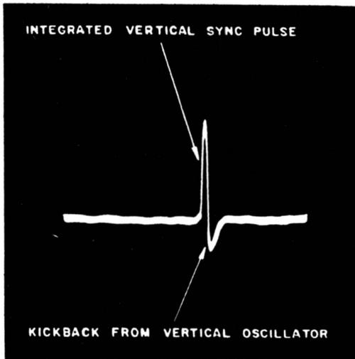
Fig. 5-7. Scope display of a typical integrator output pulse.
