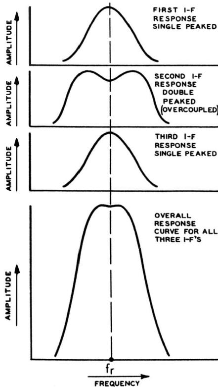
Fig. 7-3. Combination of separate responses to produce desired overall response.
