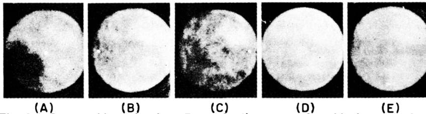
Fig. 8-6. Spot positions showing effects of adjustments of positioning controls.
