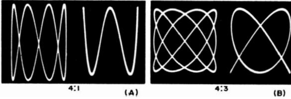
Fig. 10-15. (A) 4:1 frequency ratio, (B) 4:3 frequency ratio.
