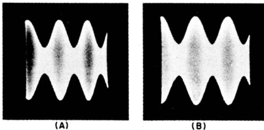
Fig. 6-6. Similarity between waveform of r-f input signal to a receiver (A) and the i-f signal resulting from it (B).
