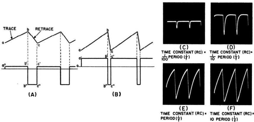
**Fig. 5-4.** (A) and (B) show basic ideal sawtooth waves and effect of differentiation. (C), (D) and (E) show actual waveforms as differentiated in circuits of progressively smaller time constant.
