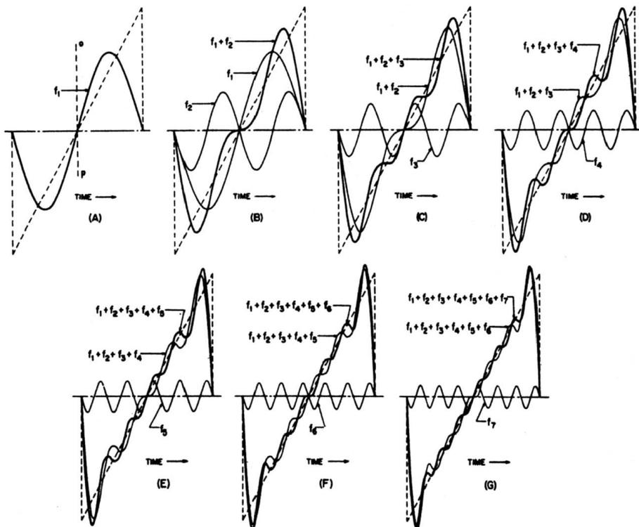
Fig. 4-2. Addition of frequency components to form sawtooth resultant.
