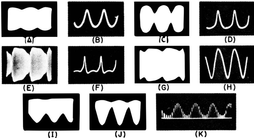
Fig. 9-47. Traces (A) (B), (C) (D), and (E) (F) form a family illustrating the effects of progressively increasing amounts of overloading of an i-f amplifier in a radio receiver by a sine waveform a-m signal voltage, and the waveform of the demodulated signal, as seen across the demodulator load. In each instance, the modulated wave envelope was observed at the plate of the third i-f amplifier.
