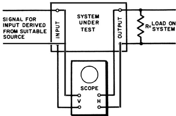
Fig. 11-2. Setup for checking phase shift.
