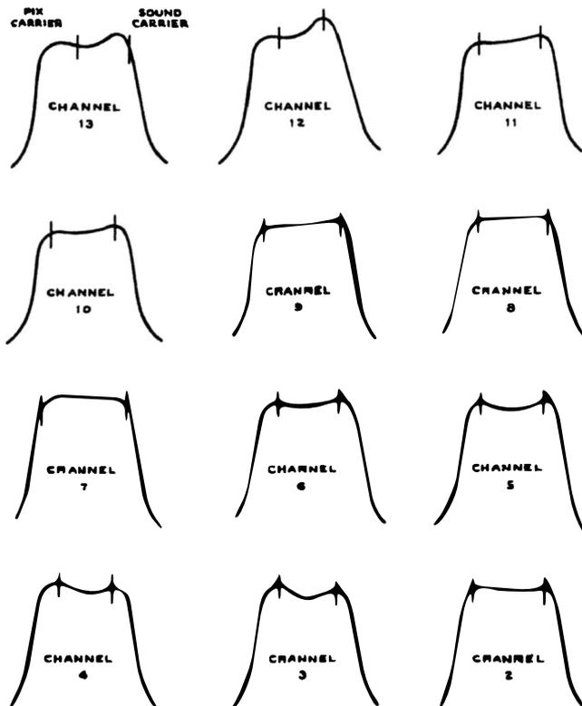
Fig. 7-8. Typical antenna-to-grid response curves for tv receivers. Courtesy RCA.
