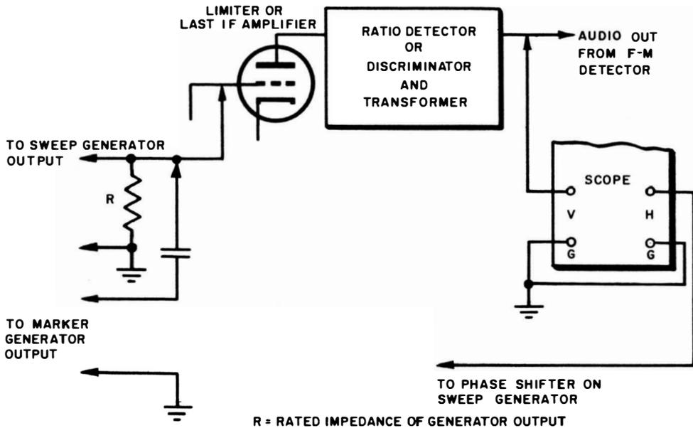
Fig. 11-11. Alignment of f-m detector transformer.
