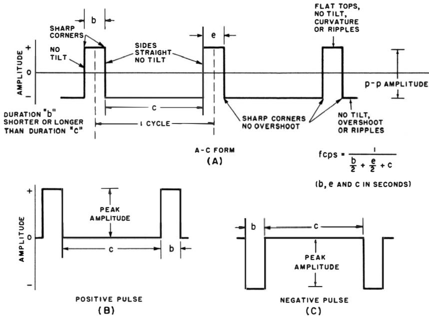
Fig. 3-1. Basic forms of the rectangular wave.
