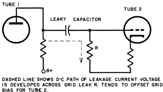
Fig. 9-7. Effect of leaky coupling capacitor.
