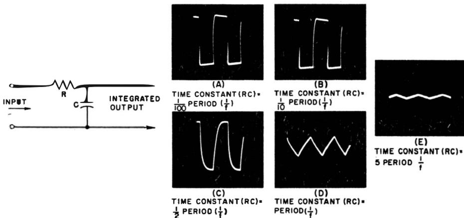
Fig. 5-5. Basic integrator circuit, and examples of integration of a square wave for RC networks of different time constants.
