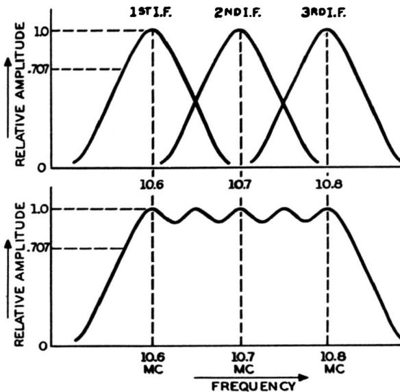
Fig. 7-4. Individual stage response curves for an f-m receiver and final overall i-f curve.
