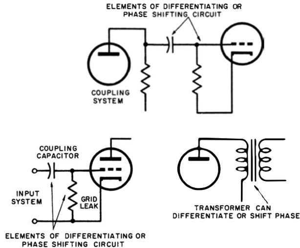
Fig. 9-6. Typical circuits in which RC and RL combinations can affect waveform.
