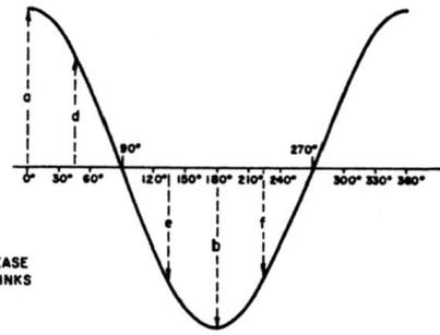
**Fig. 1-2.** The cosine waveform.
