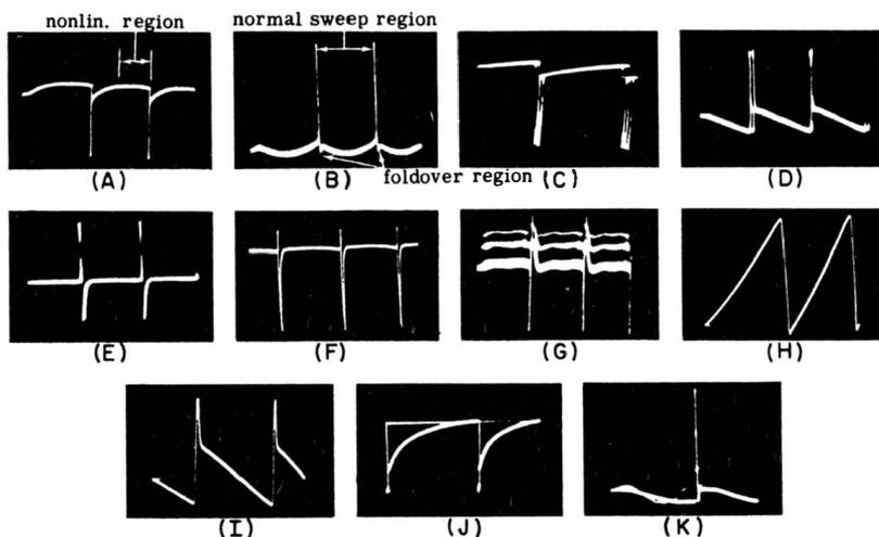
Fig. 9-44. Trace (A) shows improperly shaped trapezoidal voltage waveform at the control grid of the vertical output tube in a self-excited vertical sweep output system. A positive-going a-c pulse is fed from the output tube plate to the oscillator grid circuit. Trace (A) corresponds to reduced vertical height and severe nonlinearity over the lower half of the picture. This region of the voltage waveform is indicated by the arrow.
