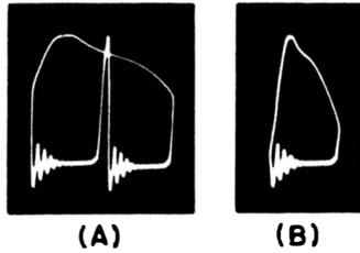
Fig. 8-27. Horizontal output voltage waveform (A), and distortion due to excessive scope sync voltage (B).
