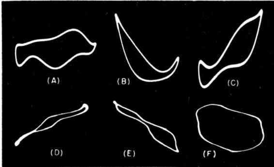
Fig. 8-19. Typical patterns resulting when signal and sweep voltages both have sine waveform, and one (or both) is distorted.
