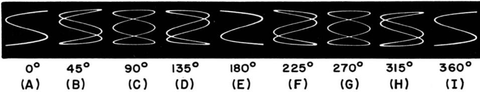
Fig. 10-12. Horizontal signal frequency three times vertical frequency.
