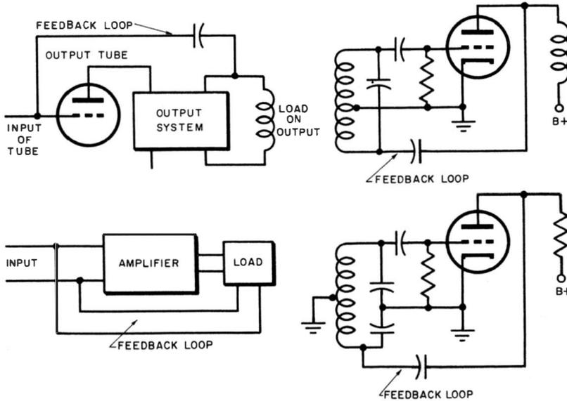
Fig. 9-2. Systems in which waveform may be distorted by improper feedback.
