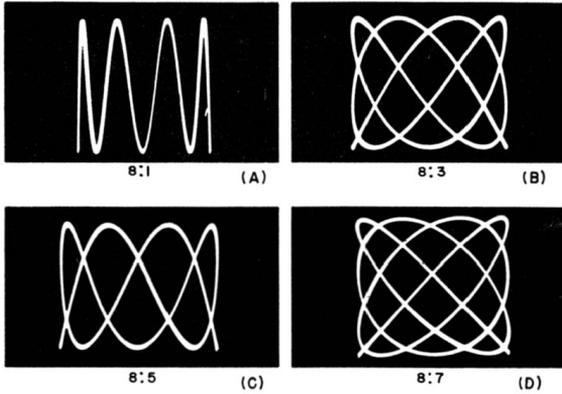
Fig. 10-19. (A) 8:1 frequency ratio, (B) 8:3 frequency ratio, (C) 8:5 frequency ratio, (D) 8:7 frequency ratio.
