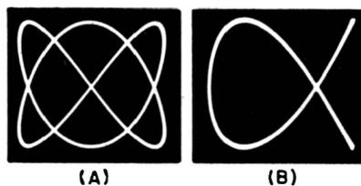
Fig. 10-14. Lissajous pattern depicting a 3:2 frequency ratio.
