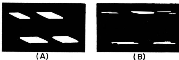
Fig. 9-25. Traces (A) and (B) illustrate the distortion of a good square waveform by the presence of a 60-cps hum field originating external of the scope in a current-carrying transformer, choke, or soldering iron, which is close to the scope.
