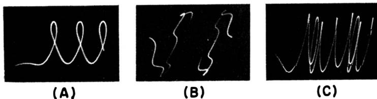
Fig. 9-12. Examples of traces when hum voltages (60 or 120 cps) are present in the scope's d-c operating voltages. The vertical amplifier is processing a sine waveform.
