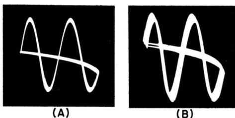
Fig. 9-11. Non-uniform spreading and tilt of trace due to the presence of external field in the vicinity of scope.
