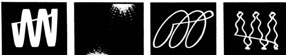
Fig. 9-10. In (A) and (D) the spurious signal has a high frequency relative to that of the signal.
