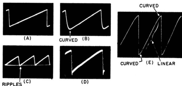
Fig. 4-3. Typical practical sawtooth waveforms.
