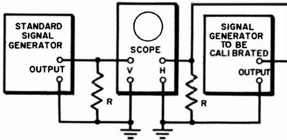
Fig. 11-1. Setup for comparing frequencies in calibration of a signal generator.
