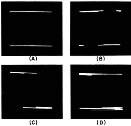
Fig. 8-21. Waveforms resulting from sine wave horizontal sweep and square wave vertical voltage. (A) Vertical and horizontal frequencies the same, (B) vertical frequency three times horizontal frequency, (C) vertical frequency lower than horizontal frequency, and (D) vertical frequency much lower than horizontal frequency.
