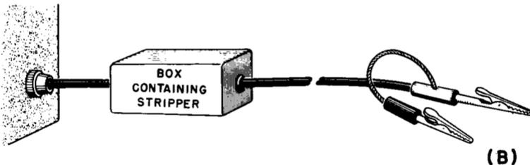
Fig. 2-8. If audio-frequency output is not directly available from the signal generator, it may be obtained from the modulated signal by an "audio stripper". A typical circuit and physical arrangement is shown here.
