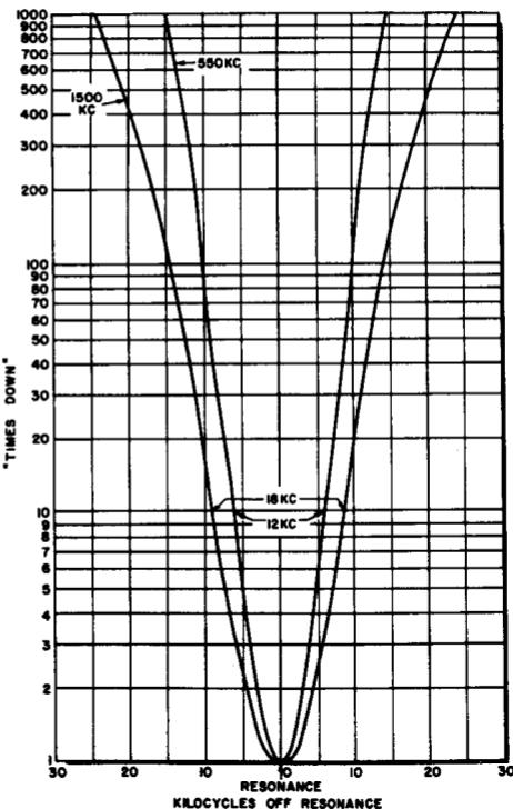
*Fig. 10-1. Typical a-m broadcast receiver selectivity curves.*
