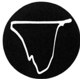
Fig. 9-20. Distortion due to i-f amplifier reflections.
