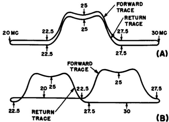
Fig. 4-6. The effect of (A) proper phase adjustment and (B) improper phase adjustment in sweep-response analysis. The forward and return base-line traces are shown separated for clarity, but in practice these would coincide.
