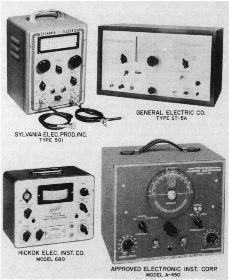
**Fig. 3-9. Photographs of typical, modern marker generators and calibrators.**
