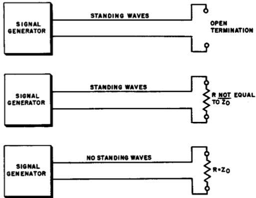
Fig. 7-6. Standing waves can be eliminated by terminating a line in its own characteristic impedance.
