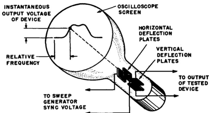
Fig. 8-4. When the two steps of Figs. 8-2 and 8-3 are combined properly, a response curve is traced on the oscilloscope screen, as shown here.
