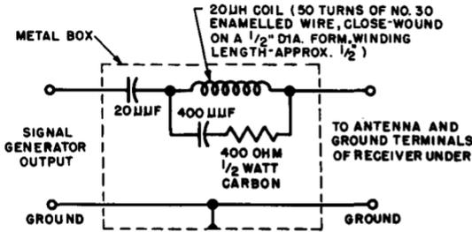
Fig. 7-10. Standard dummy antenna circuit for coupling the signal generator to an a-m receiver to match the receiver input over a wide range of frequencies.
