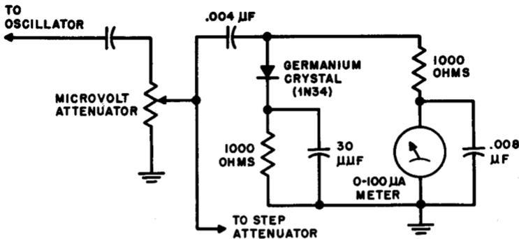
Fig. 6-2. Typical signal generator output voltage meter circuit.
