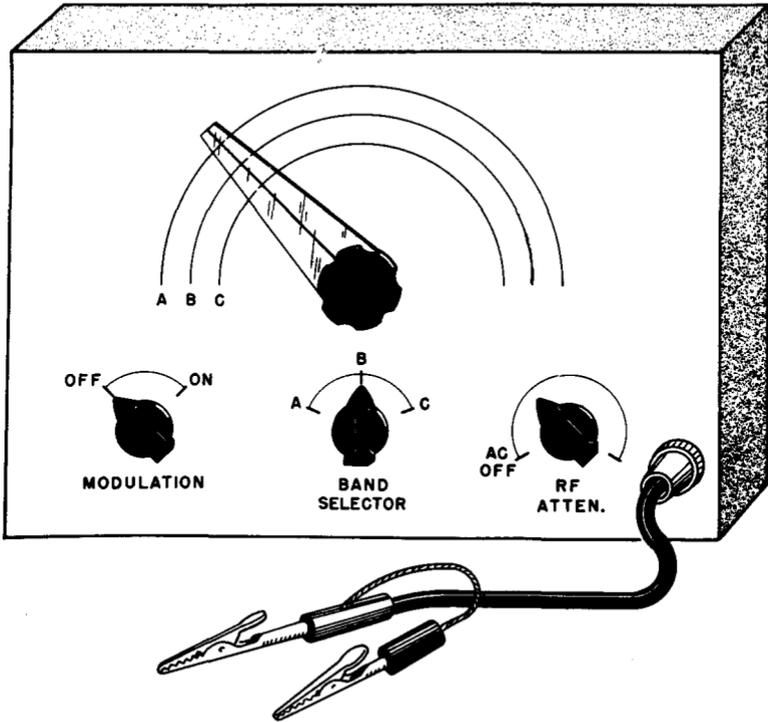
Fig. 2-3. Typical panel layout for simple service-type a-m signal generator.
