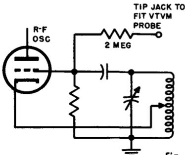
Fig. 10-11. Two methods of providing resonance indication in a signal generator circuit, when the signal generator is to be used as a grid-dip meter.
