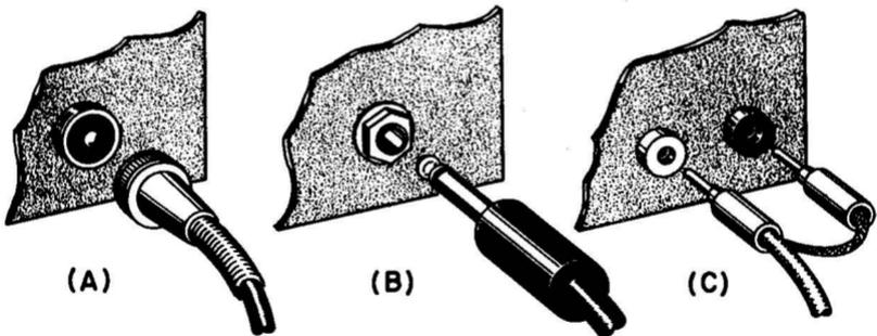
Fig. 9-1. Types of connectors commonly used for signal generator output. (A) Microphone-connector type, (B) phone-plug type, and (C) phone-tip type.
