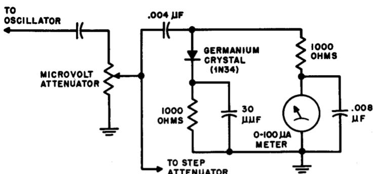
Fig. 6-2. Typical signal generator output voltage meter circuit.
