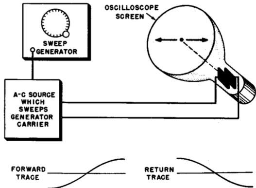
Fig. 8-2. The first step in the development of a response curve on the oscilloscope screen. The oscilloscope beam is deflected horizontally by the same voltage that produces sweep in the generator.
