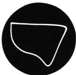
Fig. 9-17. Distortion due to oscillator tube removal.
