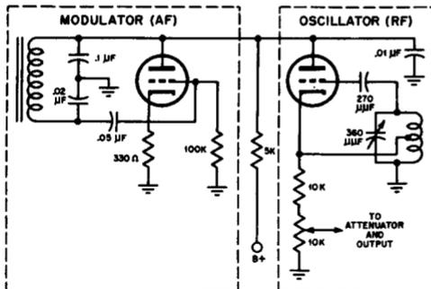
Fig. 2-1. The basic parts of any a-m signal generator are the r-f oscillator and the modulator. Typical circuit arrangements for these two basic parts are shown here.
