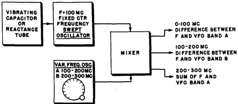
*Fig. 4-9. How a variable-oscillator signal and a signal from a swept oscillator with a fixed center frequency are combined to provide a wide range of output frequencies with a constant sweep width.*
