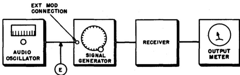
Fig. 10-4. Block diagram of set-up for checking overall receiver frequency response.
