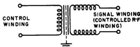
The schematic diagram of a controllable inductor is shown in Fig. 4-4. Note the use of the two windings: the *control winding*, to which the changing current is applied which produces the flux that partially saturates the core, and the *signal winding*, whose inductance is caused to change because of the changing flux in the core. This flux, as it approaches core saturation, reduces the permeability of the core and thus results in a reduction of effective inductance. The two windings
