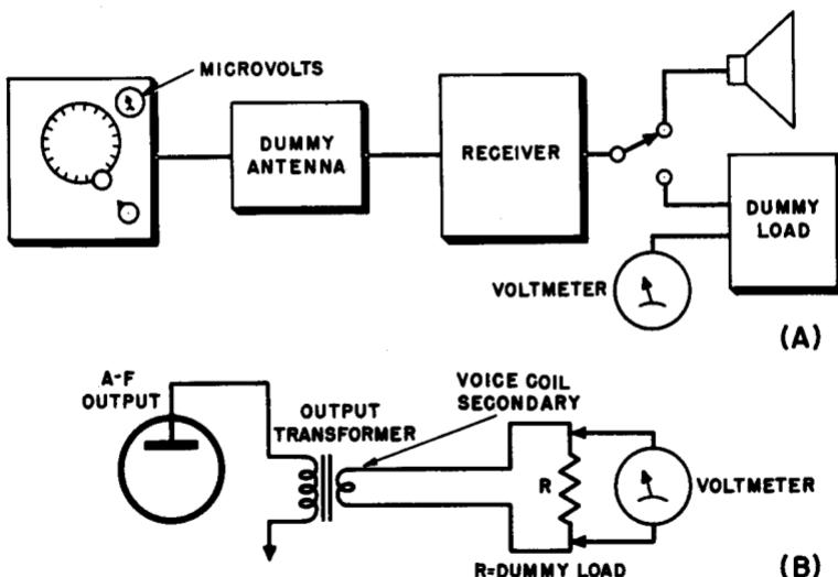
Fig. 10-3. (A) Equipment set-up for sensitivity tests. (B) Method of output voltage indication.
