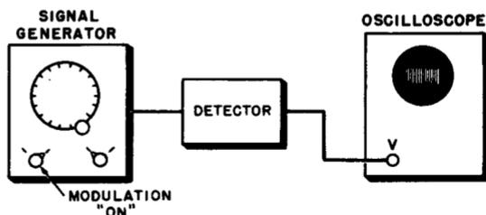
*Fig. 11-4. Set-up described in the text for determining action of the step attenuator.*
