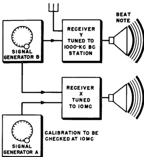
Fig. 11-2. Method for checking calibration of signal generator at frequencies above the a-m broadcast band.
