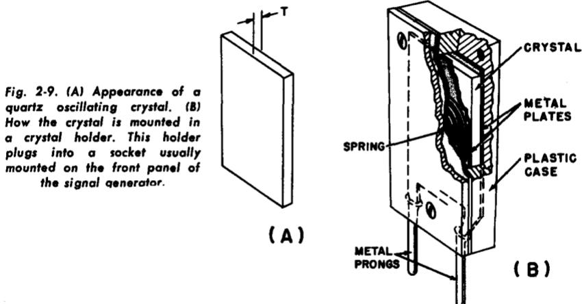
Fig. 2-9. (A) Appearance of a quartz oscillating crystal. (B) How the crystal is mounted in a crystal holder. This holder plugs into a socket usually mounted on the front panel of the signal generator.
