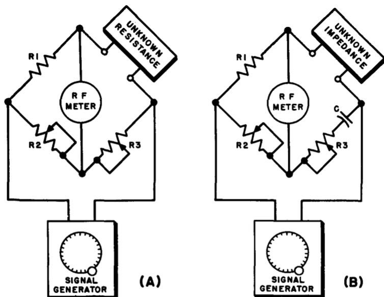
Fig. 10-12. (A) Wheatstone bridge connected to measure the r-f resistance of a component. (B) Adapting the same principle to the impedance bridge, which measures r-f impedance at the frequency of the generator.
