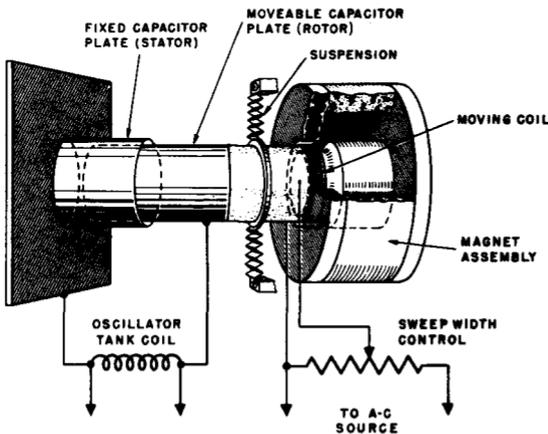
Fig. 4-2. Diagram showing the operation of a vibrating capacitor for sweeping the r-f oscillator in a sweep generator.
