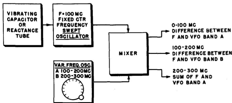
Fig. 4-9. How a variable-oscillator signal and a signal from a swept oscillator with a fixed center frequency are combined to provide a wide range of output frequencies with a constant sweep width.
