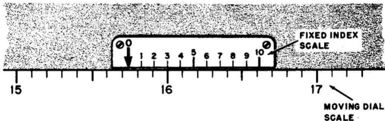
Fig. 5-3. Diagram showing how a vernier is used to indicate small changes in dial reading.
