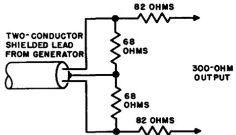
Fig. 7-7. A few typical methods for terminating signal-generator leads. Some are these included in the generator leads; others are recommended by manufacturers as external additions.
