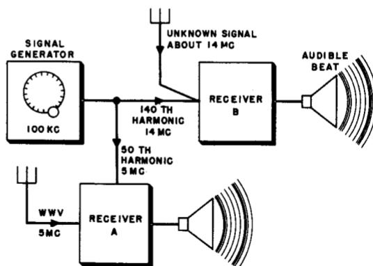
Fig. 10-9. Set-up for using the signal generator as a frequency standard.
