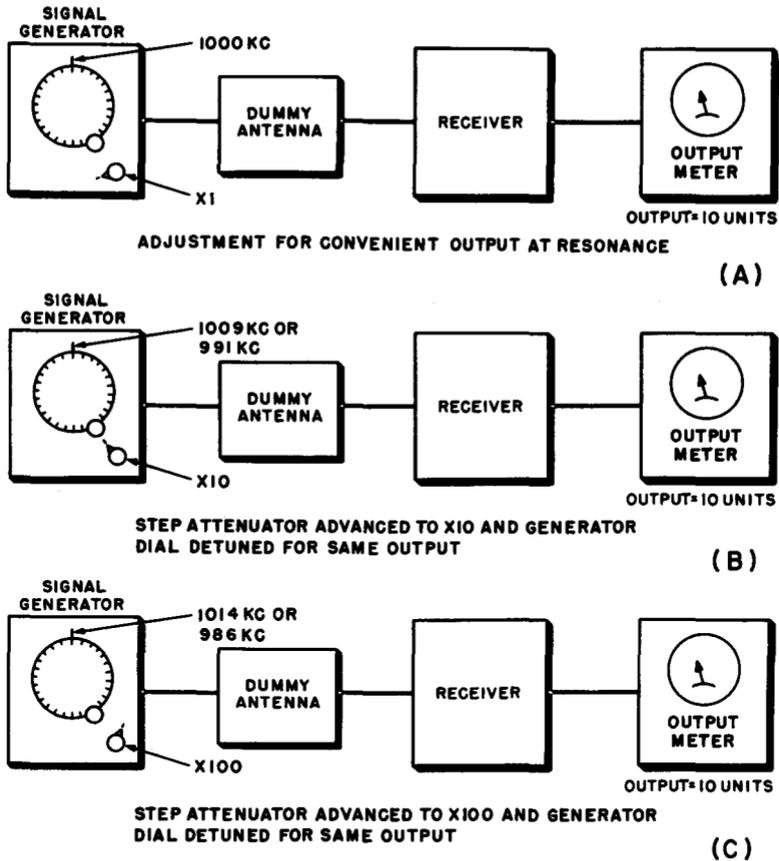
Fig. 10-2. Three steps in determining the selectivity of an a-m receiver.
