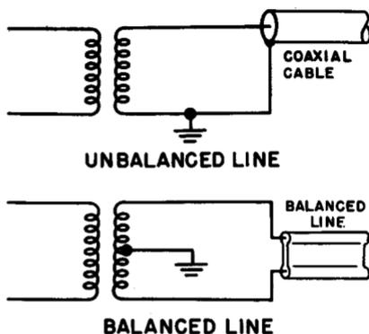
Fig. 7-3. Difference between balanced and unbalanced lines.
