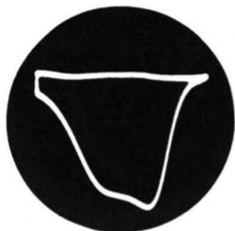
Fig. 9-16. Response curve with 120-cps pick-up distortion on base line.
