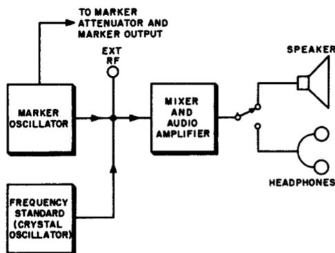
Fig. 3-4. Block diagram expressing the action of a crystal calibrator. The marker signal beats against harmonics of the crystal-oscillator output. The beat signal is detected by the mixer, amplified, and reproduced by speaker or headphones. The marker oscillator is adjusted so that the beat signal is at zero beat. Provision is made on some models for an external marker signal to be checked, as indicated by the terminal "Ext RF."
