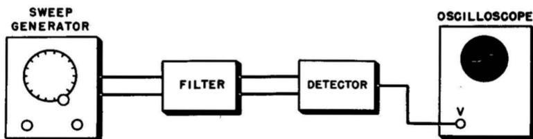
Fig. 10-13. Set-up for checking the response characteristic of a filter with a sweep generator and oscilloscope.
