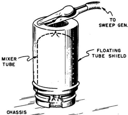
Fig. 9-3. Using a tube shield for coupling to the mixer tube.
