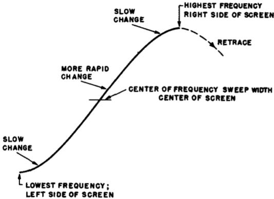
Fig. 8-5. Half cycle of an a-c voltage used to sweep the generator frequency and deflect the oscilloscope beam, showing actions taking place and how the rate of change varies during the deflection period.
