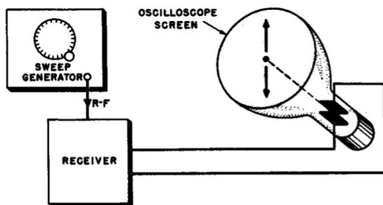
Fig. 8-3. Second step in the formation of a response curve on the oscilloscope screen; the vertical deflection of the beam spot is by the output voltage of the analyzed device, such as a receiver.
