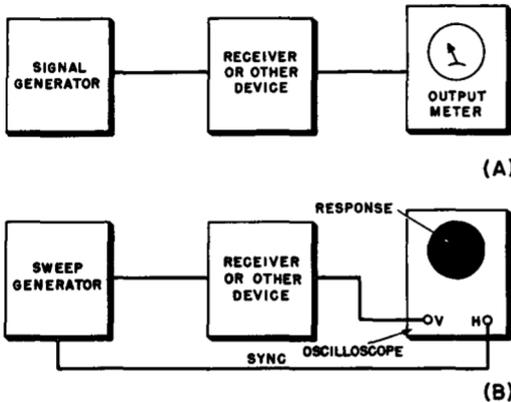
Fig. 8-1. Two ways to obtain a frequency-response characteristic of a device. (A) Step-by-step method, using individual readings at various frequencies in the pass band. (B) Sweep method, in which complete response characteristic is continuously observed on an oscilloscope screen.
