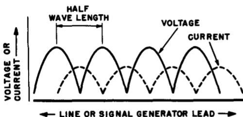
Fig. 7-4. How the voltage and current is distributed along a transmission line when there are standing waves.
