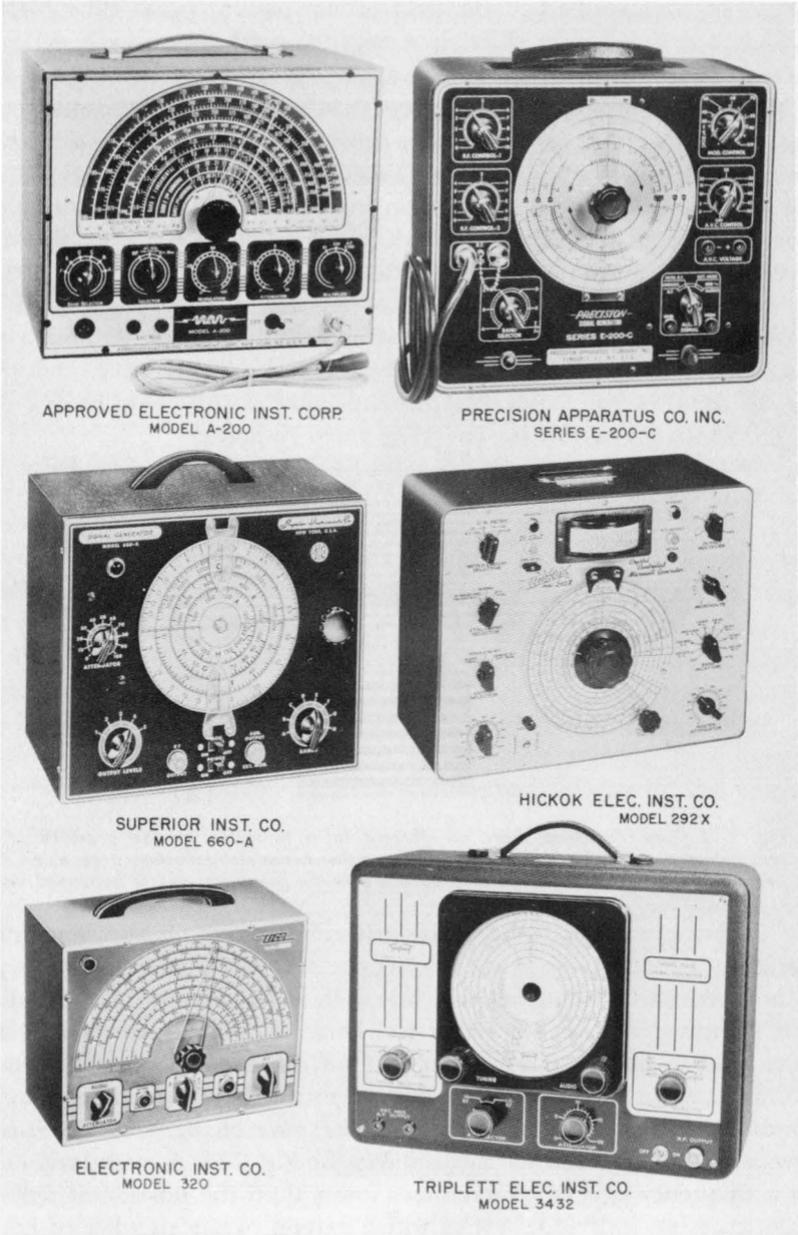
**Fig. 2-13. Photographs of typical, modern a-m signal generators.**
