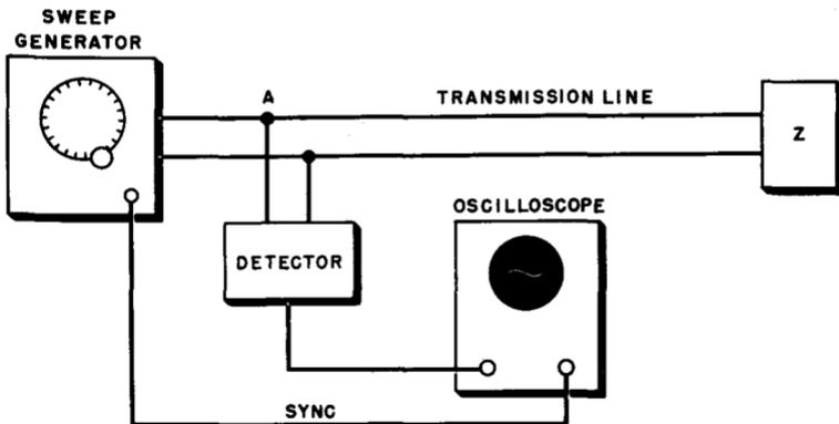
Fig. 10-16. Set-up for checking standing waves on a line with a sweep generator and an oscilloscope.
