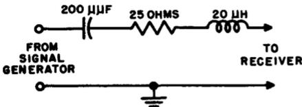
Fig. 7-11. Alternative dummy antenna circuit for a-m broadcast receivers only.
