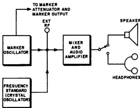
Fig. 3-4. Block diagram expressing the action of a crystal calibrator. The marker signal beats against harmonics of the crystal-oscillator output. The beat signal is detected by the mixer, amplified, and reproduced by speaker or headphones. The marker oscillator is adjusted so that the beat signal is at zero beat. Provision is made on some models for an external marker signal to be checked, as indicated by the terminal "Ext RF."
