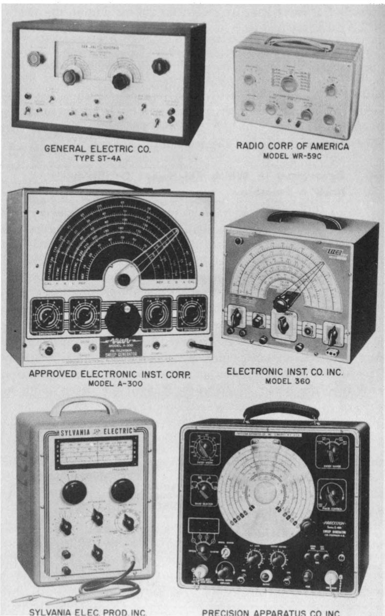
*Fig. 4-11. Photographs of typical, modern sweep generators.*
