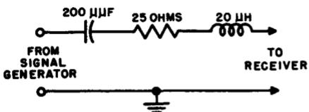
Fig. 7-11. Alternative dummy antenna circuit for a-m broadcast receivers only.
