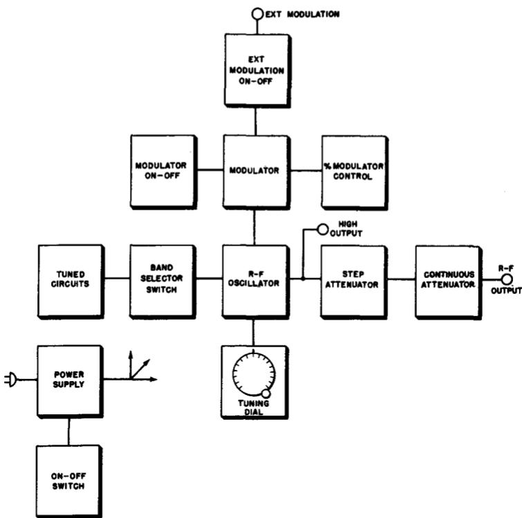
*Fig. 2-4. Typical arrangement for a-m signal generator with most ordinarily used features. This arrangement is typical of many service type and laboratory type a-m generators.*
