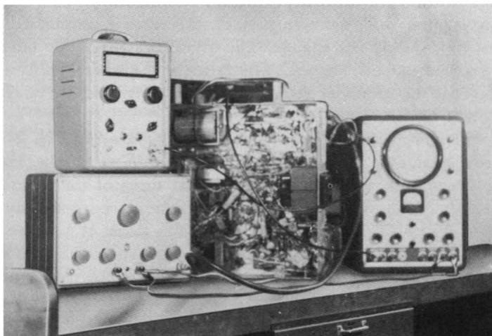
Fig. 9-5. A typical bench set-up ready for sweep alignment or analysis of a tv receiver.
