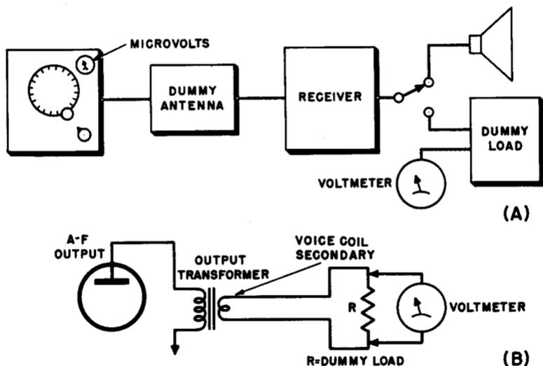
Fig. 10-3. (A) Equipment set-up for sensitivity tests. (B) Method of output voltage indication.
