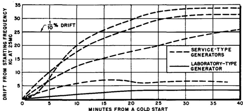
Fig. 5-5. Graph showing the extent of generator drift during warm-up period.
