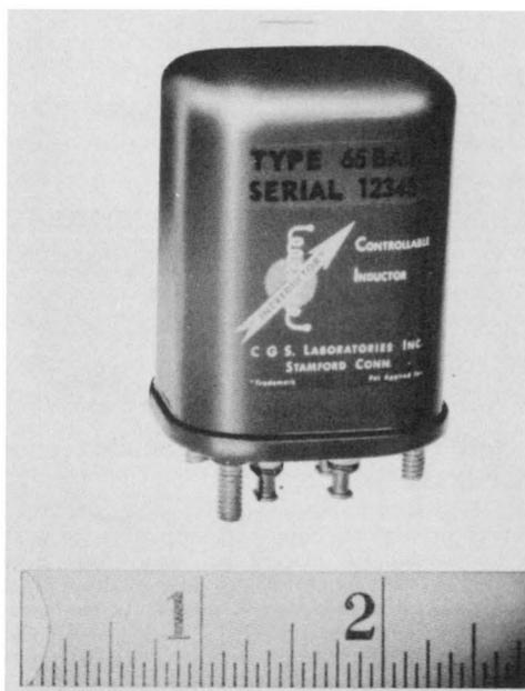
Fig. 4-5. A photograph of a typical controllable inductor.
