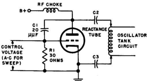
Fig. 4-1. Reactance-tube circuit, such as is used to frequency modulate the r-f oscillator in a sweep generator.
