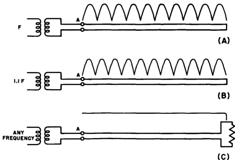
Fig. 10-15. Diagrams showing how the standing-wave distribution along an unmatched line changes as frequency changes. (A) Standing waves along a line 10 half-wavelengths long. (B) Standing waves along the same line when the frequency has been increased to make the line 11 half-wavelengths long. (C) Constant voltage without standing waves on a line which is terminated in its own characteristic impedance.
