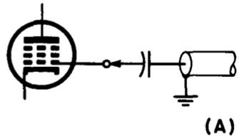
Fig. 7-1. Two ways of applying the low impedance of the signal generator output to a high-impedance circuit, when it is not necessary to know from signal generator indications how much is the input voltage to the circuit.
