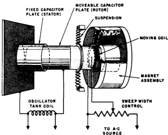
Fig. 4-2. Diagram showing the operation of a vibrating capacitor for sweeping the r-f oscillator in a sweep generator.
