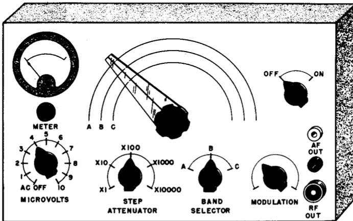
Fig. 2-6. Typical panel layout for signal generator using a meter-type output indicator.
