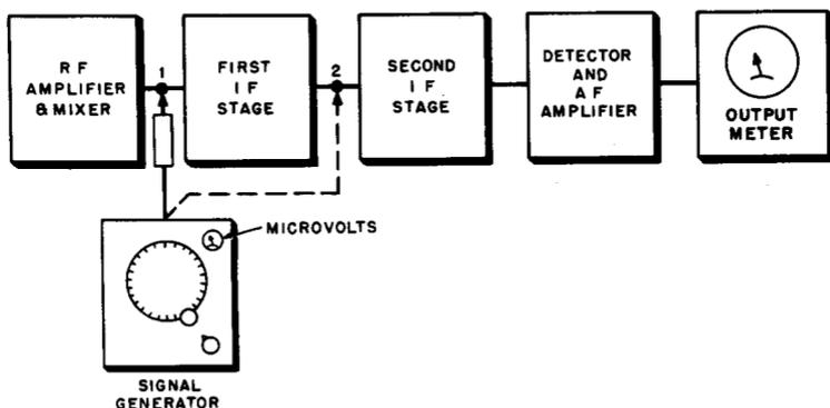
Fig. 10-6. Typical arrangement for measuring stage gain.
