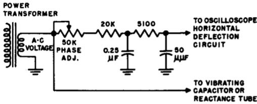
Fig. 4-7. A typical phase-adjusting circuit used in a sweep generator.
