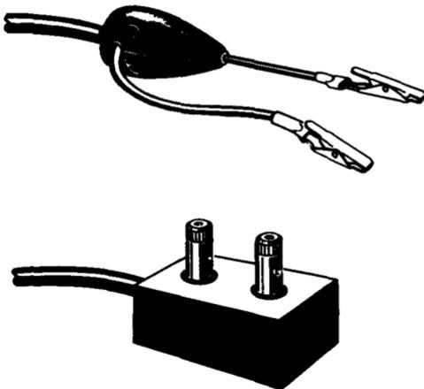
*Fig. 7-8. Two ways of making connection from the end of the signal-generator lead to the device to be tested.*
