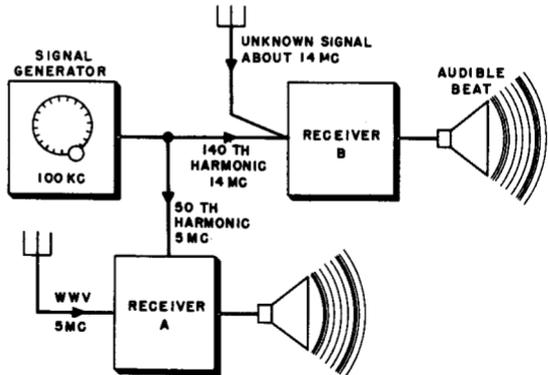
Fig. 10-9. Set-up for using the signal generator as a frequency standard.
