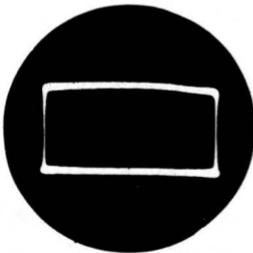
*Fig. 11-6. Typical sweep generator response as observed with the set-up of Fig. 11-5.*
