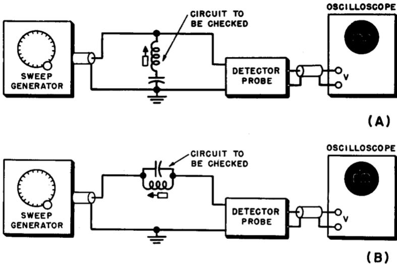
Fig. 10-17. Method used to check resonant frequency on a tuned circuit.
