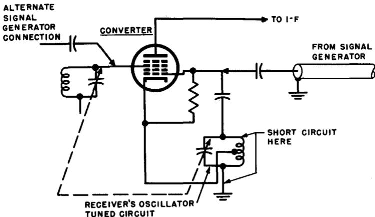
Fig. 10-7. Methods of injecting the signal generator output voltage into a receiver circuit so as to substitute for the receiver's local oscillator.
