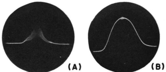
Fig. 9-7. A response curve with excessive marker signal is shown at (A). The proper display appears at (B).
