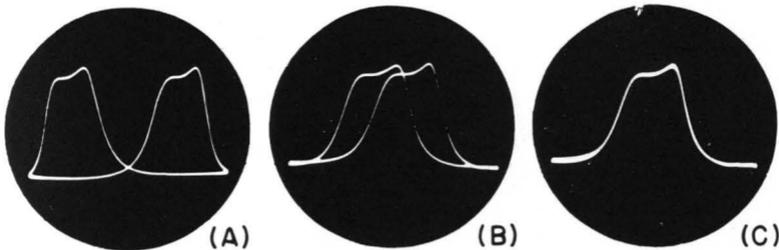
Fig. 9-9. When the phasing is misadjusted, with blanking off, two response curves appear. Adjustment of the phasing brings the curves together to coincide.
