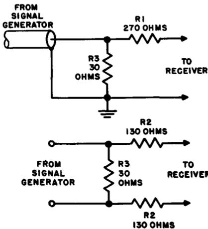
Fig. 7-2. Two ways of terminating signal generator leads to offer the desired impedance to the device tested while maintaining proper impedance load to the generator itself.
