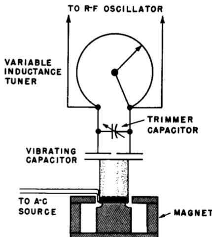
*Fig. 4-10. Tuning and sweeping circuit of the Philco Model 7008 sweep generator, in which the swept oscillator itself is also tunable through a range. The use of inductance tuning allows tuning the center frequency through a range without much change in sweep width.*
