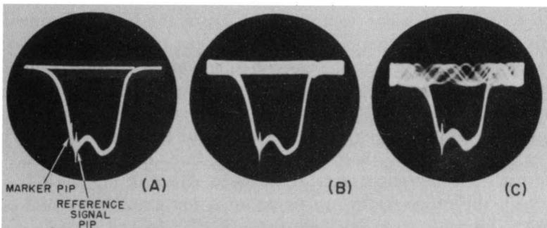
**Fig. 9-10.** The frequency calibration of the marker generator can be checked against a reference signal whose exact frequency is known. The checking can be done by visual means as shown here. Each signal is indicated by a pip on the receiver response curve; the marker pip is then tuned by adjustment of the marker oscillator until the pips coincide and the marker dial checked against the reference frequency.
