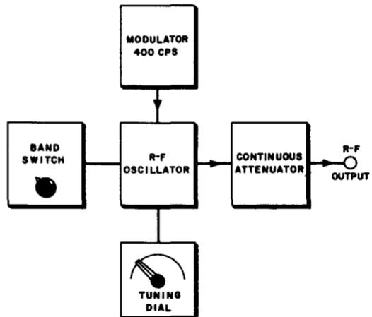
Fig. 2-2. Block diagram of the simplest service-type a-m signal generator.
