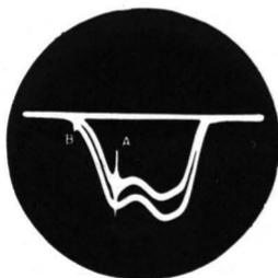
Fig. 3-3. The marker signal must heterodyne with the sweep signal in order to produce a pip. Where the receiver response is low both signals are weak at the second detector, thus their beat signal and the pip are weak. That is why much more marker amplitude is required to produce a pip at *b* than at *a*.
