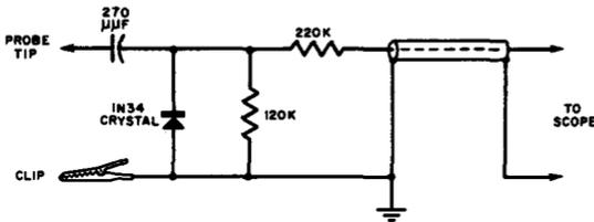
Fig. 9-2. Typical circuit for crystal probe used to rectify r.f. from receiver stages before application to oscilloscope.
