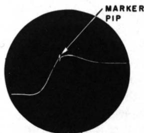
Fig. 10-14. Typical high-pass filter response as swept out on an oscilloscope, with a marker at the cut-off frequency.
