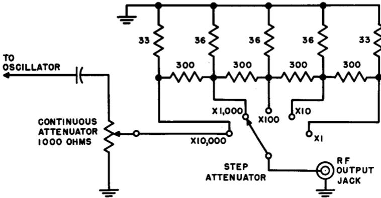
Fig. 6-1. Typical combination continuous and step attenuator circuit for a signal generator.
