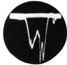
Fig. 9-19. Distortion due to presence of strong local signal.
