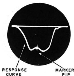
Fig. 3-2. The appearance of a typical marker pip on a response curve.
