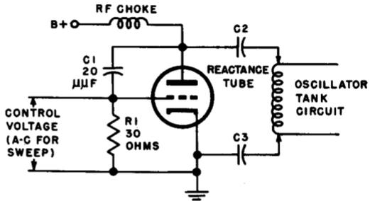
Now if the control voltage is made to vary rapidly back and forth, we produce the same effect as though we were rapidly rotating a variable capacitor across the oscillator tank circuit. This effect causes the oscillator to change frequency rapidly in accordance with the control voltage changes. In other words, the oscillator frequency "sweeps" back and forth.
