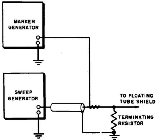
Fig. 9-6. A common method of injecting a marker signal.
