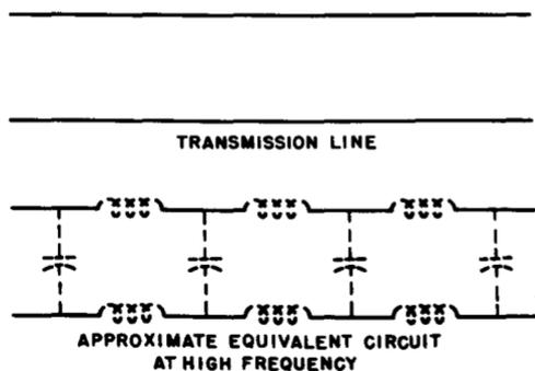
Fig. 7-5. At high frequencies, a transmission line is equivalent to a series of inductances and capacitances blended together into "distributed constants."
