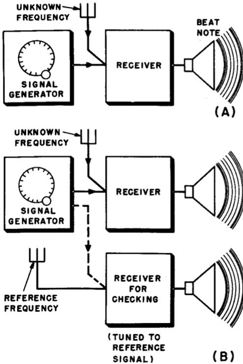
Fig. 10-8. Two ways of using a signal generator for frequency measurement.
