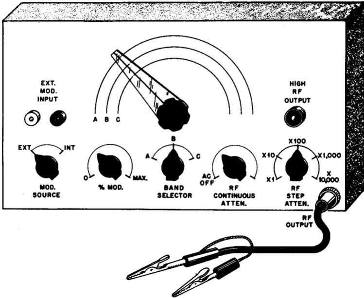
Fig. 2-5. Typical panel layout for signal generator for the type illustrated by the block diagram of Fig. 2-4.
