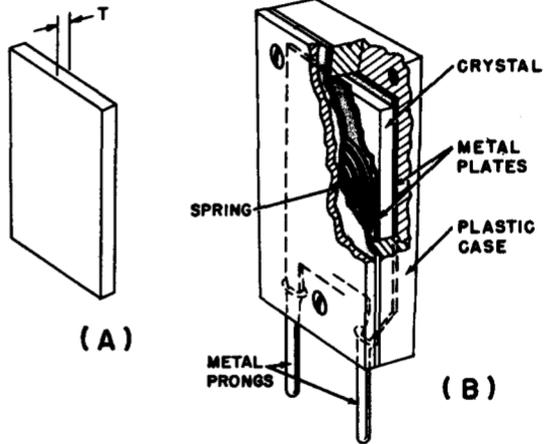
Fig. 2-9. (A) Appearance of a quartz oscillating crystal. (B) How the crystal is mounted in a crystal holder. This holder plugs into a socket usually mounted on the front panel of the signal generator.
