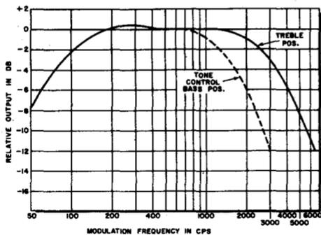
Fig. 10-5. Typical overall frequency response curves for a-m broadcast receiver. The tone control in this case is the simple type most frequently used in moderately priced receivers. As can be seen, it provides "bass" by reducing the high-frequency components of the modulation signal in relation to the lows.
