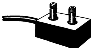
Fig. 7-8. Two ways of making connection from the end of the signal-generator lead to the device to be tested.
