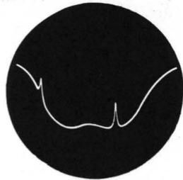
is tuned. Marker frequencies are adjusted by simply tuning the variable element of the tuned circuit, which is usually equipped with a calibrated dial. The appearance of such absorption markers in a response curve is shown in Fig. 3-8.
