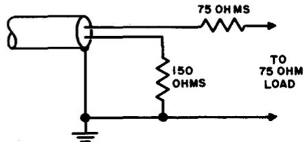
Fig. 7-9. Arrangement for adapting balanced 300-ohm output to match 75-ohm circuit.
