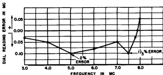
Fig. 11-3. Calibration correction curve and data taken to derive it, for one range of a signal generator.
