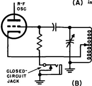
Two things are necessary to convert a signal generator to a grid-dip meter: (1) some means of coupling its output to the circuits to be tested, and (2) some way of measuring grid current or d-c grid voltage.
