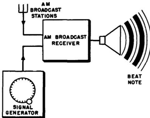
Fig. 11-1. Set-up for checking frequency calibration of signal generator in and below the a-m broadcast band.
