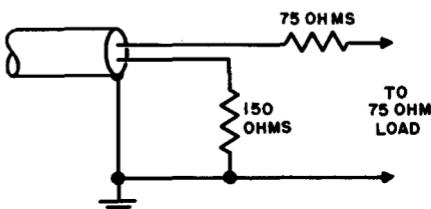
Fig. 7-9. Arrangement for adapting balanced 300-ohm output to match 75-ohm circuit.
