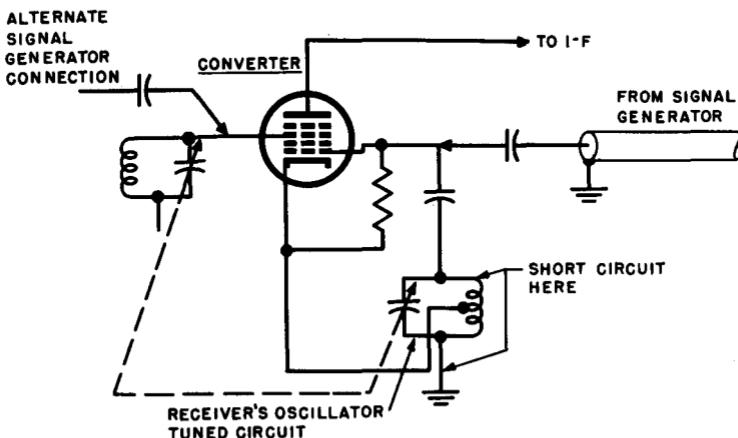
Fig. 10-7. Methods of injecting the signal generator output voltage into a receiver circuit so as to substitute for the receiver's local oscillator.
