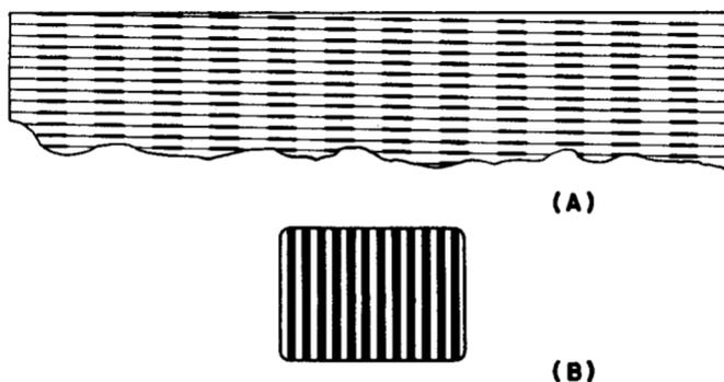
Fig. 2-11. How vertical bars are formed in a tv raster by presence of a modulation signal of a frequency considerably higher than the horizontal-deflection frequency. Several modulation signal cycles take place during one horizontal line period, thus producing a series of black spots along the line. When the frequency ratio is just right, the black spots on the successive lines align themselves, producing the vertical bars.
