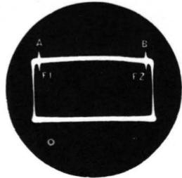
Fig. 11-7. Response of a sweep generator, with marker pips used to determine sweep width.
