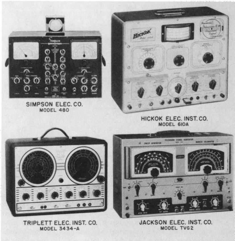
Fig. 4-12. Photographs of typical, modern combination sweep and marker generator units.
