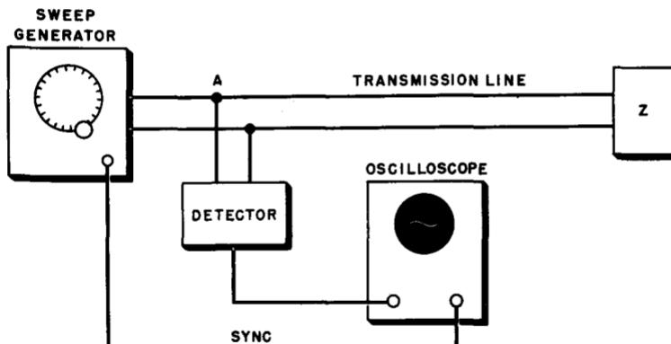
Fig. 10-16. Set-up for checking standing waves on a line with a sweep generator and an oscilloscope.
