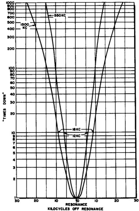
Fig. 10-1. Typical a-m broadcast receiver selectivity curves.
