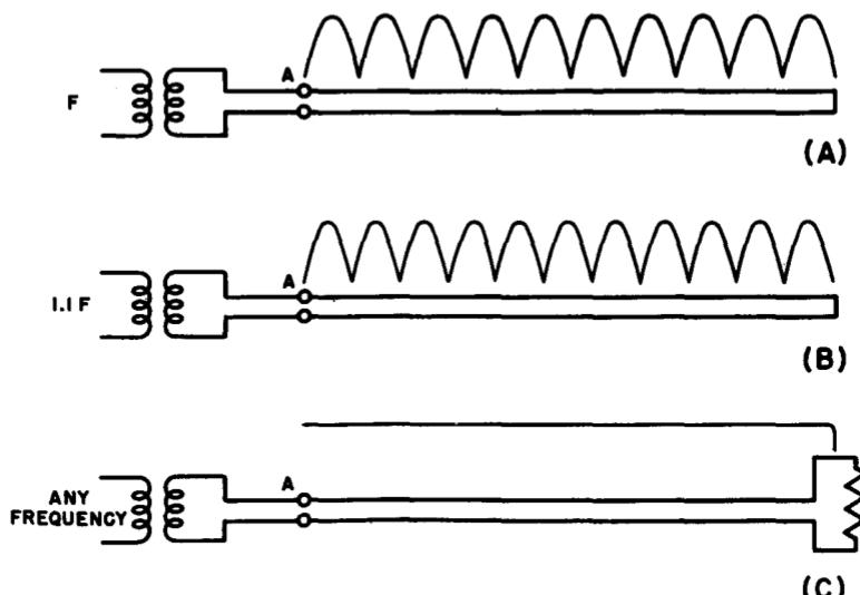
Fig. 10-15. Diagrams showing how the standing-wave distribution along an unmatched line changes as frequency changes. (A) Standing waves along a line 10 half-wavelengths long. (B) Standing waves along the same line when the frequency has been increased to make the line 11 half-wavelengths long. (C) Constant voltage without standing waves on a line which is terminated in its own characteristic impedance.
