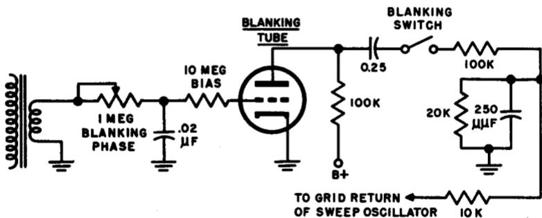
Fig. 4-8. A typical blanking circuit used in a sweep generator.
