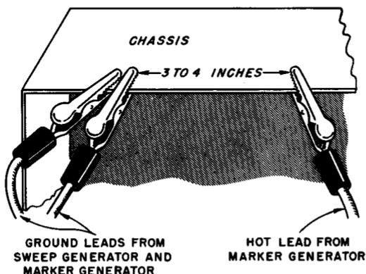
Fig. 9-8. Marker injection by means of a ground loop.
