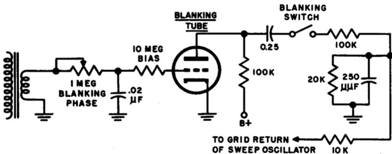
Fig. 4-8. A typical blanking circuit used in a sweep generator.
