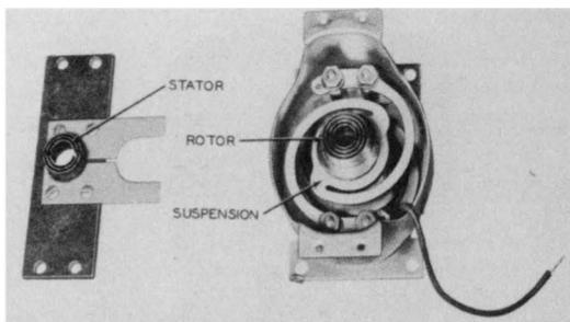
**Fig. 4-3. Typical vibrating capacitor.**
