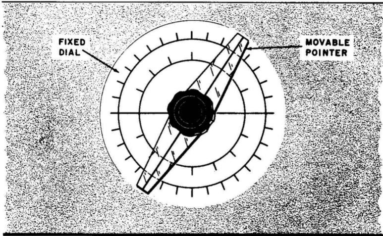
Fig. 5-2. With some generators, the calibration scale is stationary, while the index mark revolves over it, as shown here. The revolving pointer is made of clear plastic.
