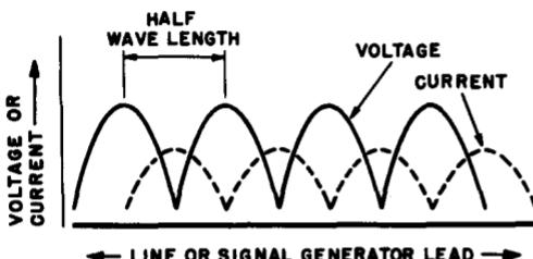
Fig. 7-4. How the voltage and current is distributed along a transmission line when there are standing waves.
