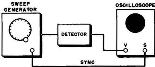
*Fig. 11-5. Arrangement of equipment used to check sweep generator response.*
