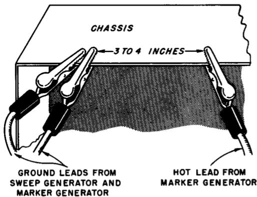
Fig. 9-8. Marker injection by means of a ground loop.
