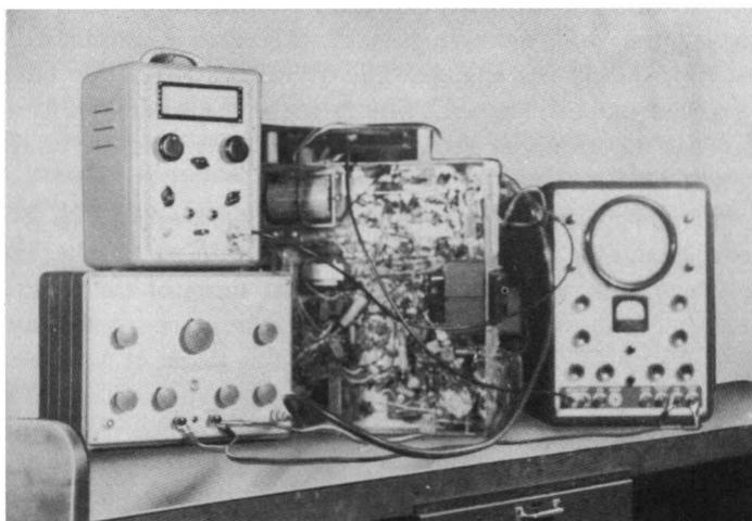
Fig. 9-5. A typical bench set-up ready for sweep alignment or analysis of a tv receiver.
