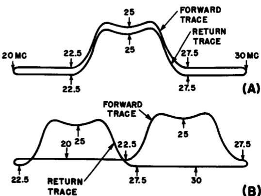
At (B) is shown what happens if the phasing is not correct. The sweep generator is starting from its low-frequency extreme (20 mc) after the oscilloscope beam has started its forward sweep; by the time the sweep generator reaches 30 mc, the oscilloscope beam has completed its forward sweep and started its return sweep. The result is that the forward and return response curves do not occur at the same point along the horizontal axis and are staggered as shown at (B).
