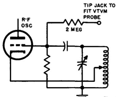
Fig. 10-11. Two methods of providing resonance indication in a signal generator circuit, when the signal generator is to be used as a grid-dip meter.
