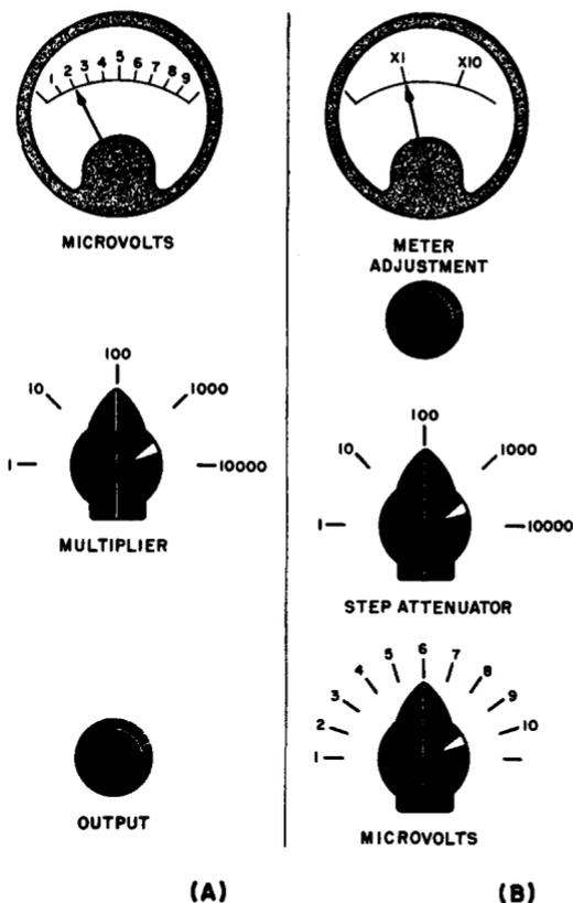
Fig. 2-7. Two methods in which a meter is used to indicate r-f output voltage of a signal generator. At (A) the meter reads microvolts directly, and its indication is multiplied by the multiplier dial indication. At (B) the meter is used to set the reference voltage, after which the output is read from the dials.
