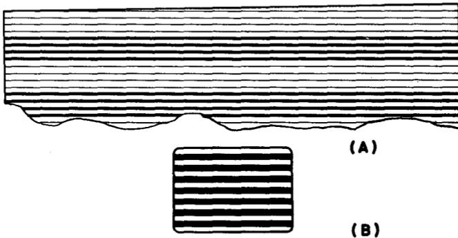
Fig. 2-12. How horizontal bars are formed in a tv raster by the presence of a modulation signal of frequency lower than the horizontal-deflection frequency. The negative portion of each modulation cycle blanks the beam for several horizontal lines.
