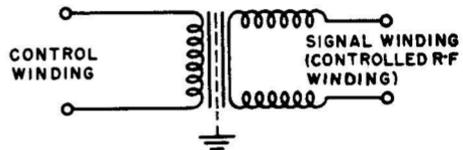
The schematic diagram of a controllable inductor is shown in Fig. 4-4. Note the use of the two windings: the *control winding*, to which the changing current is applied which produces the flux that partially saturates the core, and the *signal winding*, whose inductance is caused to change because of the changing flux in the core. This flux, as it approaches core saturation, reduces the permeability of the core and thus results in a reduction of effective inductance. The two windings
