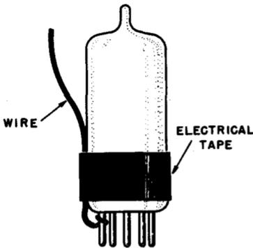
Fig. 9-4. Another method of connecting a sweep generator to the mixer tube.
