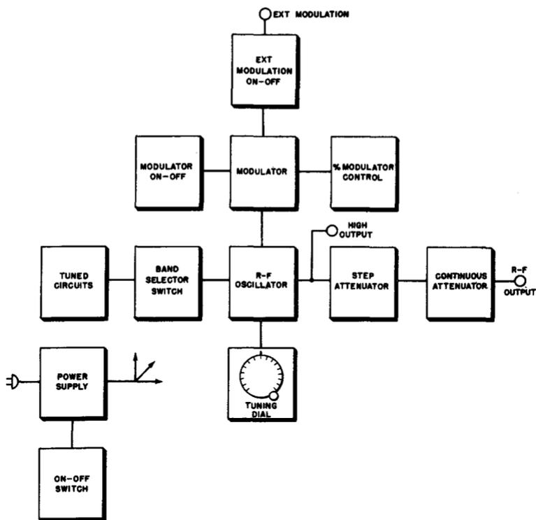
*Fig. 2-4. Typical arrangement for a-m signal generator with most ordinarily used features. This arrangement is typical of many service type and laboratory type a-m generators.*
