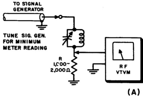
Fig. 10-10. Set-up for determining the resonant frequency of a tuned circuit.
