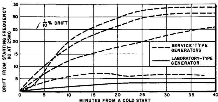
Fig. 5-5. Graph showing the extent of generator drift during warm-up period.
