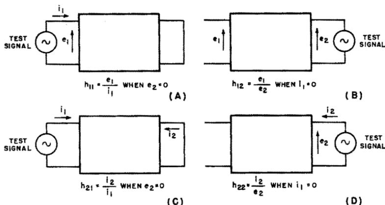
Fig. 7-10. Basic circuits for measuring four-terminal  $h$  parameters.
