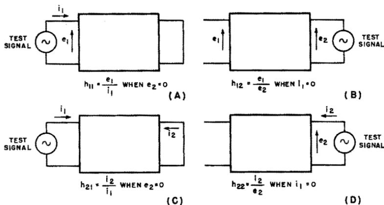
Fig. 7-10. Basic circuits for measuring four-terminal  $h$  parameters.
