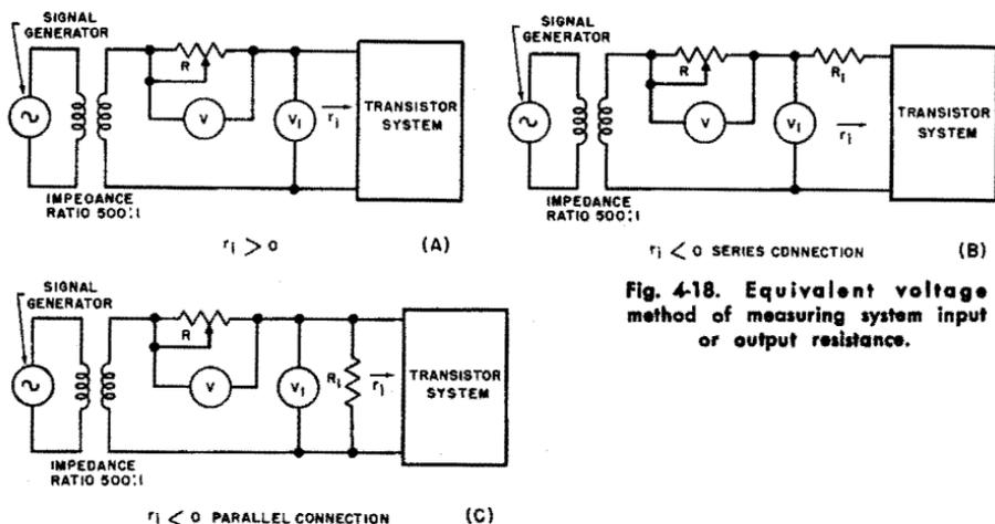
Fig. 4-18. Equivalent voltage method of measuring system input or output resistance.
