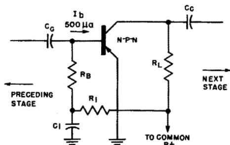
Fig. 5-19 (right). Typical decoupling network.
