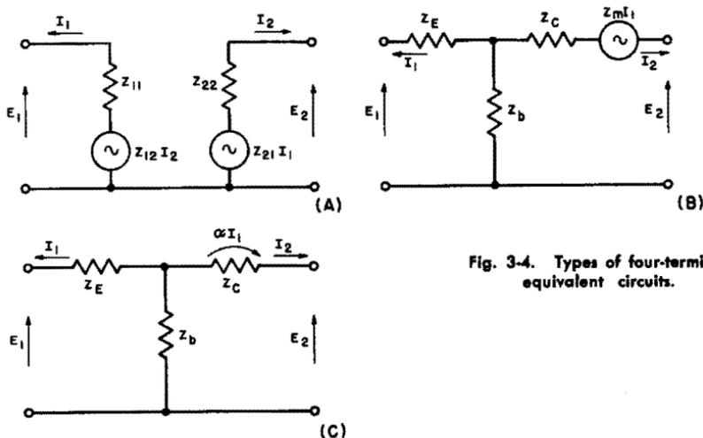
Fig. 3-4. Types of four-terminal equivalent circuits.
