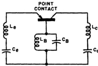
Fig. 6-6. Basic impedance controlled negative resistance oscillator.
