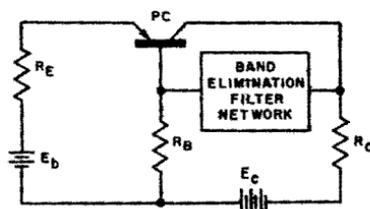
Fig. 6-14. Phase-shift oscillator.
