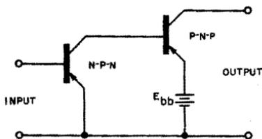
Fig. 5-23 (above). A direct-coupled symmetrical cascade.
