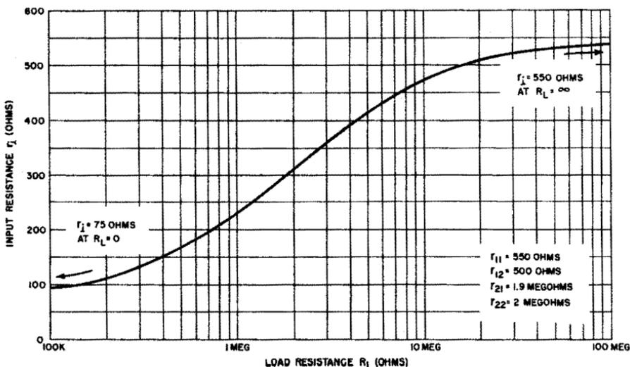
Fig. 3-12. Input resistance vs load resistance for typical junction transistor (grounded base).
