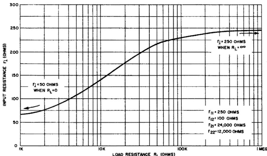
Fig. 3-11. Input resistance vs load resistance for typical point-contact transistor (grounded base).
