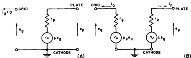
Fig. 3-2. Equivalent circuit of a triode: (A) with negative grid bias, (B) with positive grid bias.
