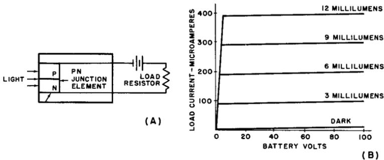
Fig. 2-9. (A) P-N junction photocell construction. (B) Typical junction photocell operating curves.
