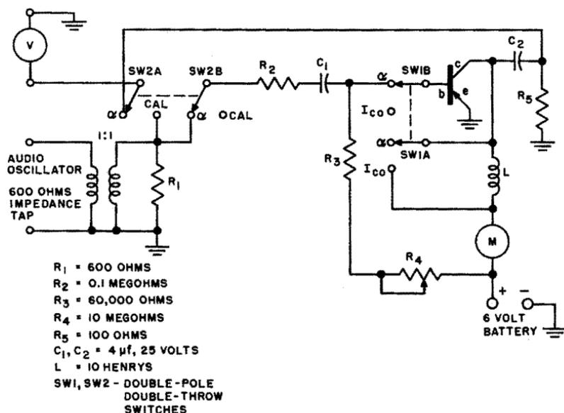
Fig. 4-19. Transistor tester for measuring  $\alpha$  and  $I_{co}$ .
