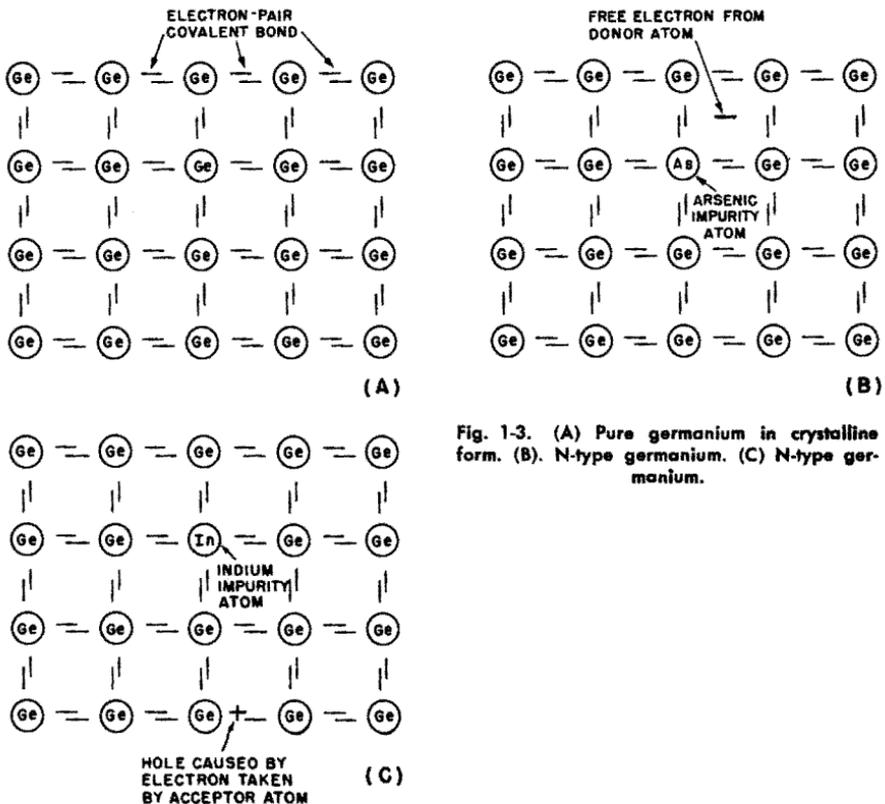
Fig. 1-3. (A) Pure germanium in crystalline form. (B). N-type germanium. (C) N-type germanium.
