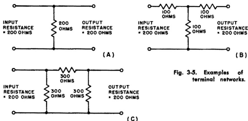
Fig. 3-5. Examples of four-terminal networks.
