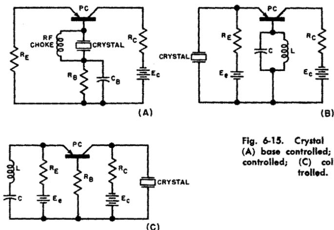
Fig. 6-15. Crystal oscillators: (A) base controlled; (B) emitter controlled; (C) collector controlled.
