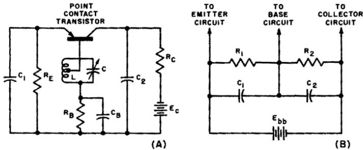
Fig. 6-12. (A) Stabilized base-controlled high-frequency oscillator. (B) Alternate method of providing common bias supply.
