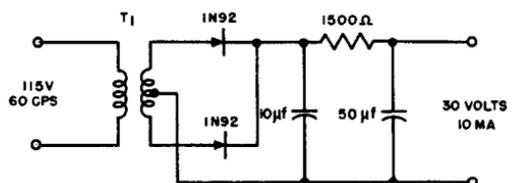
Fig. 7-9. Transistor power supply.
