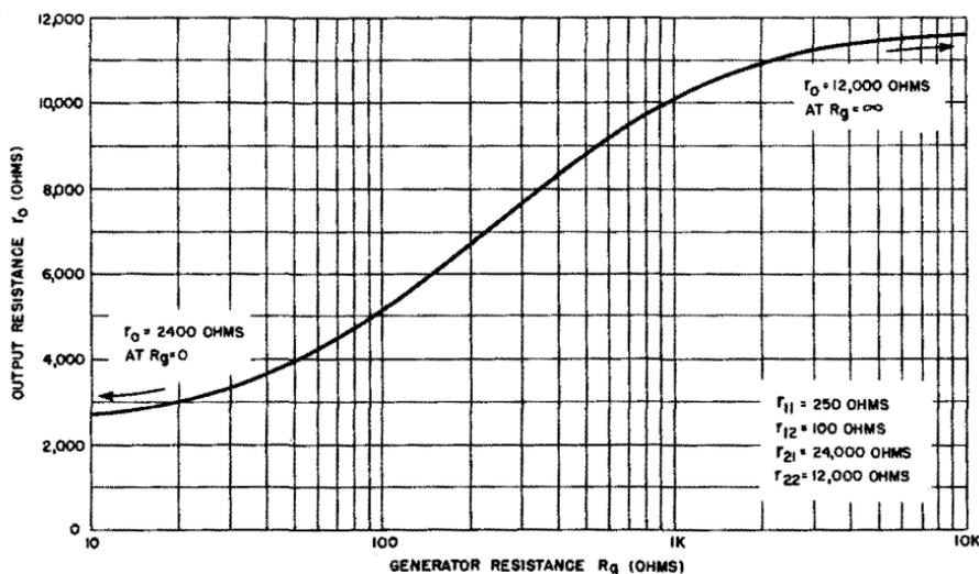
Fig. 3-14. Output resistance vs generator resistance for typical point-contact transistor (grounded base).
