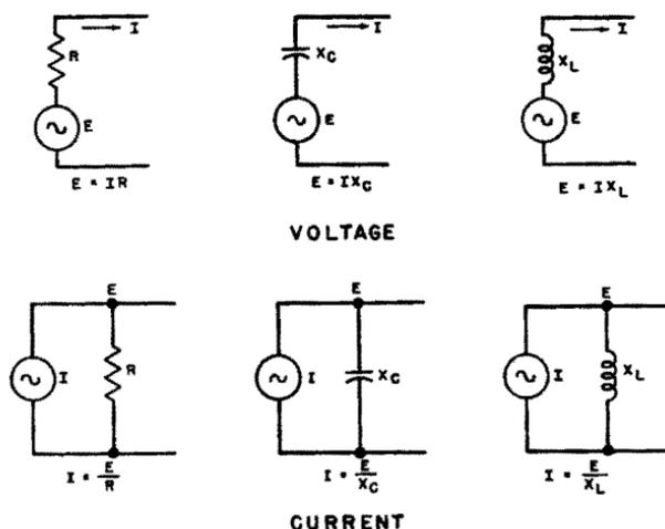
Fig. 5-7. Equivalent voltage-current sources.
