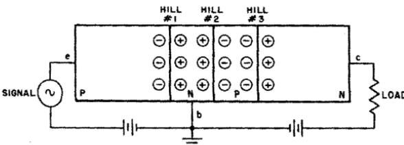
Fig. 2-10. Basic P-N-P-N transistor construction.
