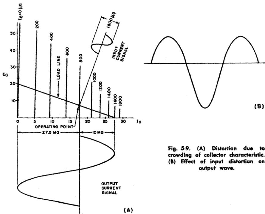
Fig. 5-9. (A) Distortion due to crowding of collector characteristic. (B) Effect of input distortion on output wave.
