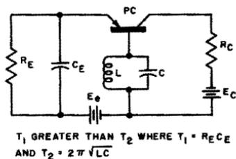
Fig. 6-19. Basic self-quenching oscillator.
