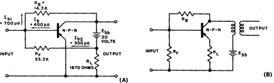
Fig. 5-6. (A) Stabilization of d-c operating point with one battery. (B) Typical power output stage.
