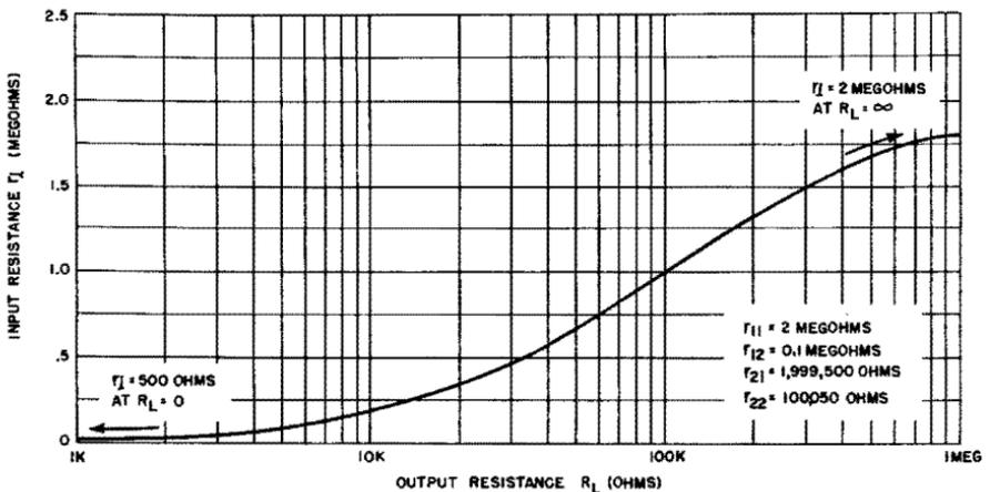
Fig. 4-11. Input resistance vs load resistance for typical junction transistor (grounded collector).
