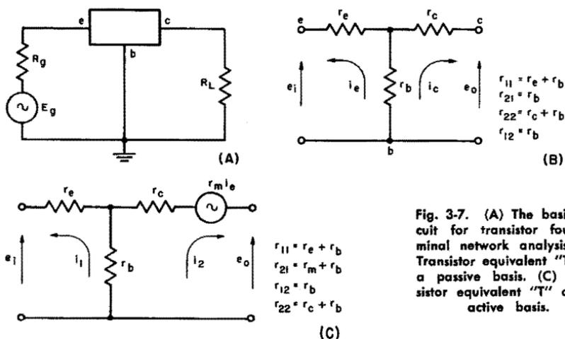
Fig. 3-7. (A) The basic circuit for transistor four-terminal network analysis. (B) Transistor equivalent "T" on a passive basis. (C) Transistor equivalent "T" on an active basis.
