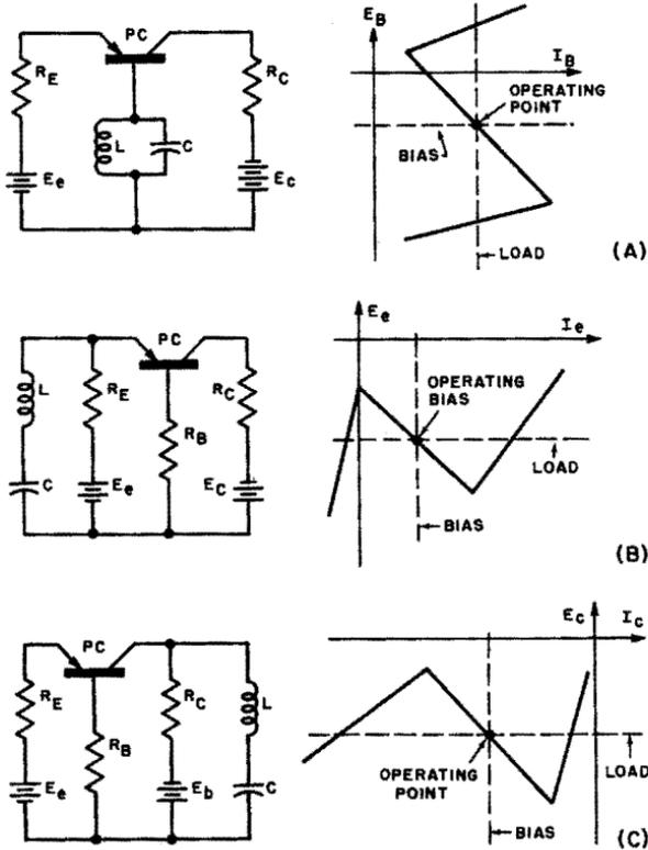
Fig. 6-9. (A) Base-controlled negative resistance oscillator and idealized characteristic. (B) Emitter-controlled negative resistance oscillator and idealized characteristic. (C) Collector-controlled negative resistance oscillator and idealized characteristic.
