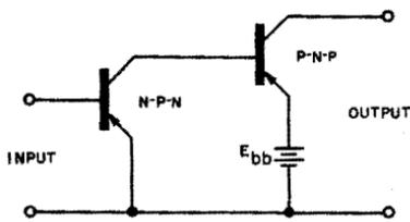
Fig. 5-23 (above). A direct-coupled symmetrical cascade.
