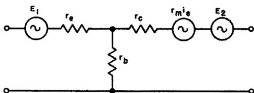
Fig. 4-17. Effect of noise on equivalent transistor circuit.
