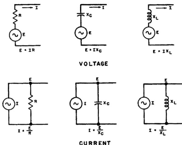
Fig. 5-7. Equivalent voltage-current sources.
