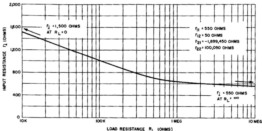
Fig. 4-4. Input resistance vs load resistance for typical junction transistor (grounded emitter).
