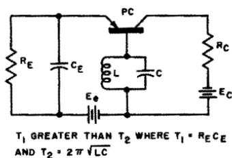
Fig. 6-19. Basic self-quenching oscillator.
