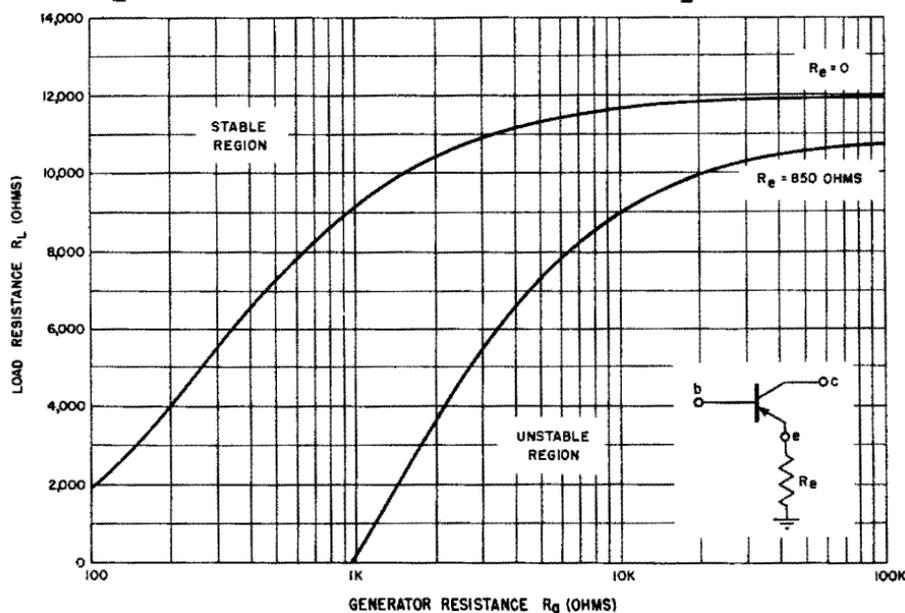
Fig. 4-7. Conditional stability characteristic (grounded emitter).
