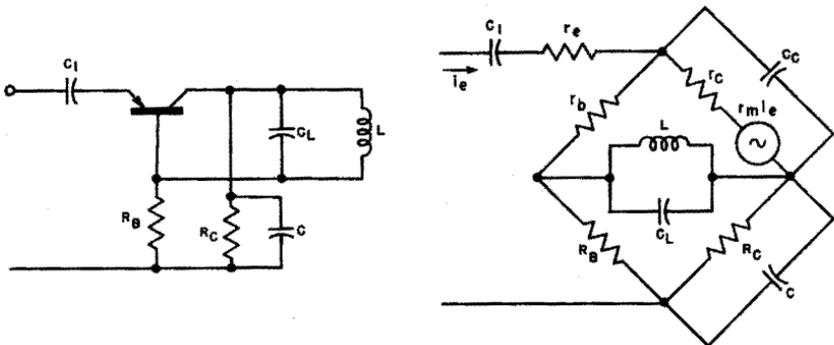
Fig. 7-6. (A) Neutralized i-f amplifier. (B) Equivalent circuit of neutralized i-f amplifier.
