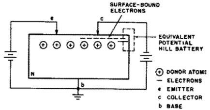
Fig. 2-1 (left). Construction of point-contact transistor. Courtesy CBS-Hytron.
