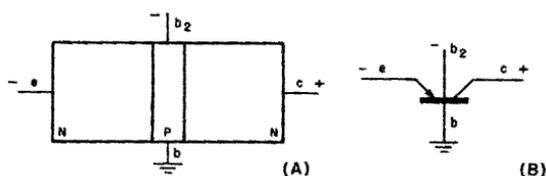
Fig. 2-11. Tetrode junction transistor: (A) structural representation, (B) symbolic representation.
