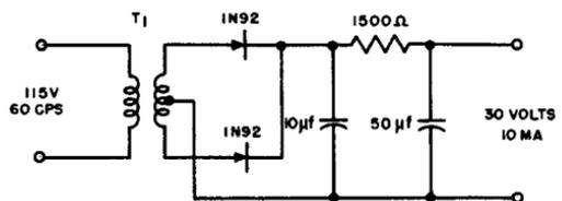
Fig. 7-9. Transistor power supply.
