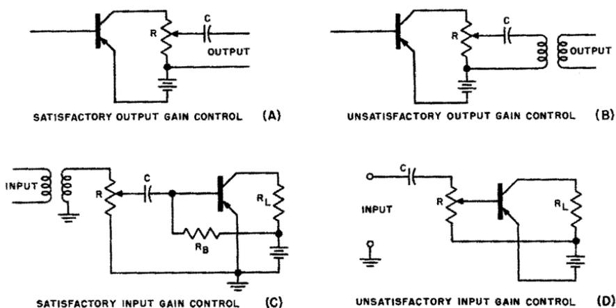
Fig. 5-15. Gain controls.
