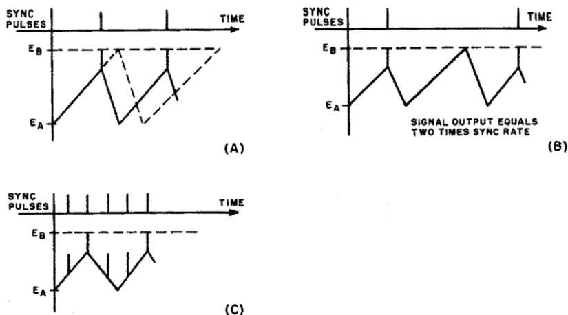
Fig. 6-20. Synchronized controlled (A) waveform, (B) frequency multiplication waveforms, (C) frequency divider waveforms.
