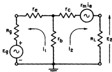
Fig. 3-9. Equivalent circuit for grounded base connection.
