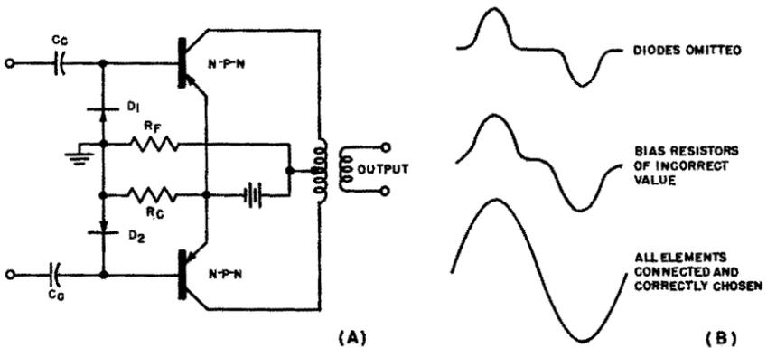
Fig. 5-13. (A) Class B push-pull operation without input transformer. (B) Output waveforms.
