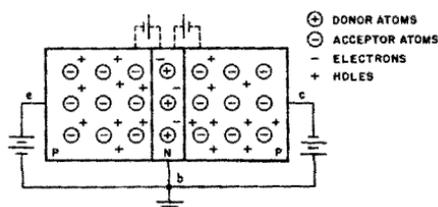
Fig. 2-7. Basic P-N-P transistor.
