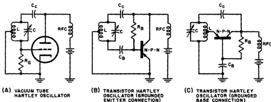
Fig. 6-1. Vacuum tube and transistor Hartley oscillator circuits.
