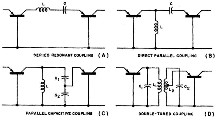
Fig. 7-5. Transistor i-f coupling networks.
