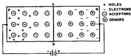
Fig. 1-5. P-N junction with reverse bias.
