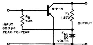
Fig. 5-1 (left). Selecting the d-c operating point.
