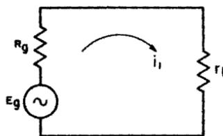
Fig. 3-10. Simplified transistor equivalent circuit for analysis of input resistance  $r_1$ .
