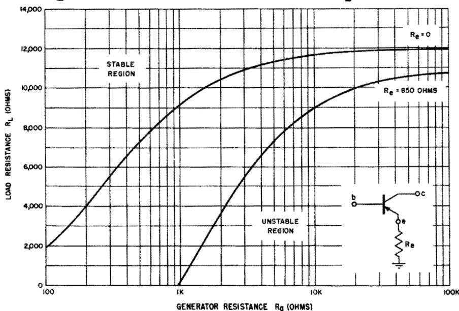
Fig. 4-7. Conditional stability characteristic (grounded emitter).
