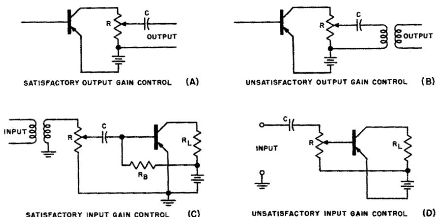
Fig. 5-15. Gain controls.
