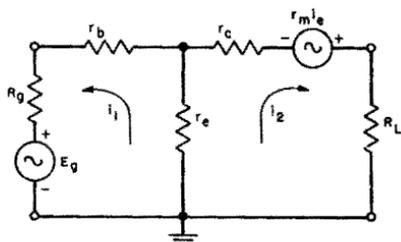
Fig. 4-2. Operating circuit, grounded emitter connection.
