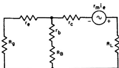
Fig. 6-5 (right). Basic resistance controlled negative resistance circuit.
