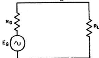
Fig. 3-16. Simplified transistor equivalent circuit for analysis of power gain.
