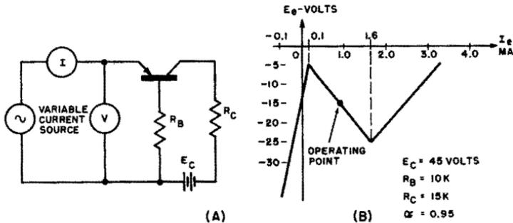
Fig. 6-10. (A) Basic measuring circuit for obtaining negative resistance characteristics. (B) Typical negative resistance characteristic.
