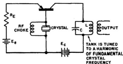
Fig. 6-16. Crystal-controlled frequency multiplier.
