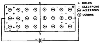
Fig. 1-5. P-N junction with reverse bias.
