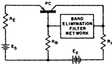
Fig. 6-14. Phase-shift oscillator.
