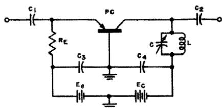
Fig. 7-7. Typical transistor r-f amplifier.
