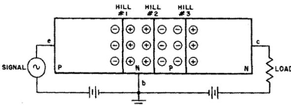
Fig. 2-10. Basic P-N-P-N transistor construction.
