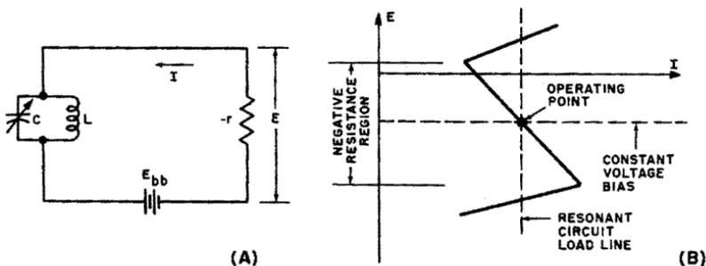
Fig. 6-7. (A) Voltage controlled negative resistance equivalent circuit. (B) Idealized current-voltage characteristic.
