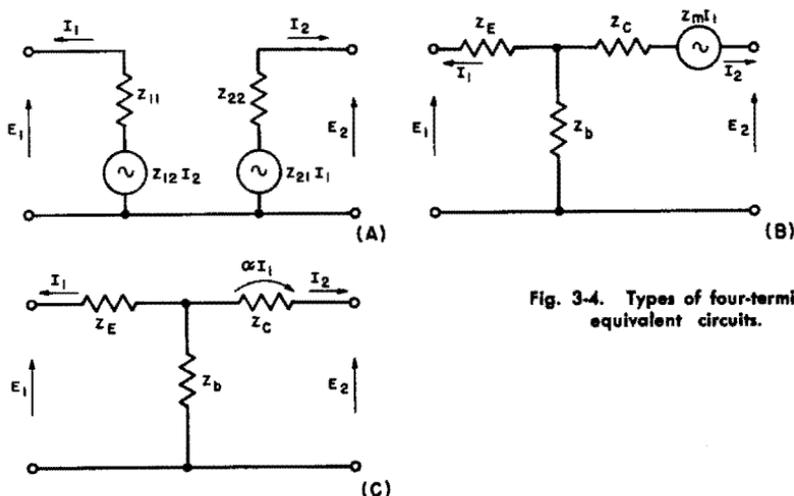
Fig. 3-4. Types of four-terminal equivalent circuits.
