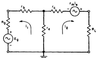
Fig. 4-2. Operating circuit, grounded emitter connection.
