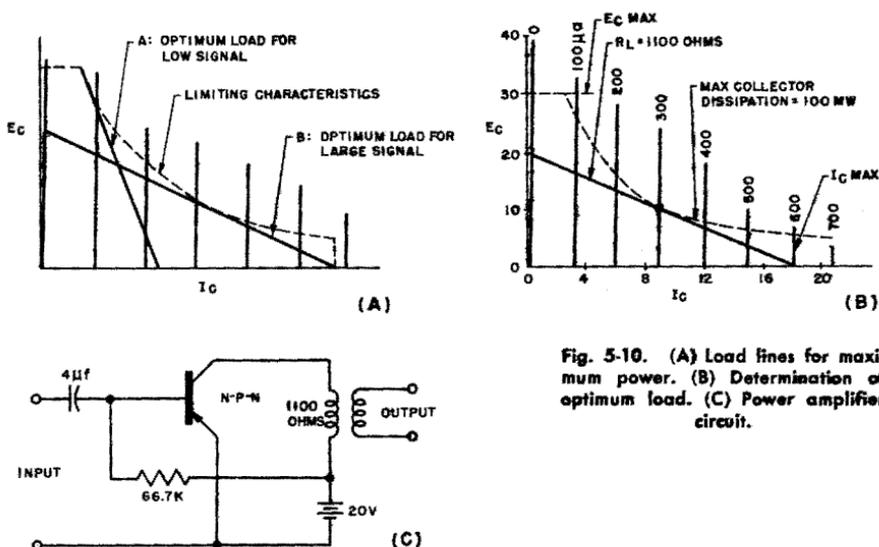
Fig. 5-10. (A) Load lines for maximum power. (B) Determination of optimum load. (C) Power amplifier circuit.
