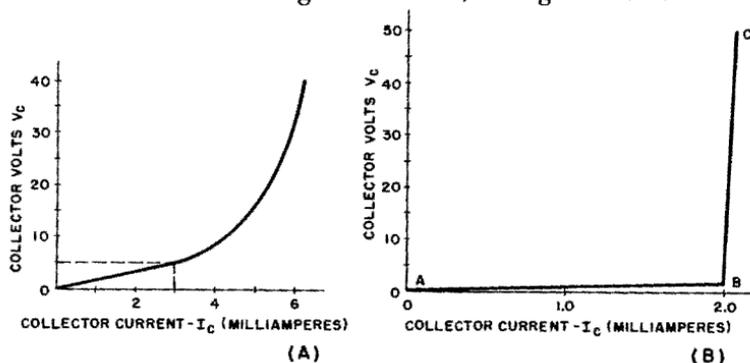
Fig. 2-8. (A) Typical point-contact  $V_c$ - $I_c$  characteristic. (B) Typical junction  $V_c$ - $I_c$  characteristic.
