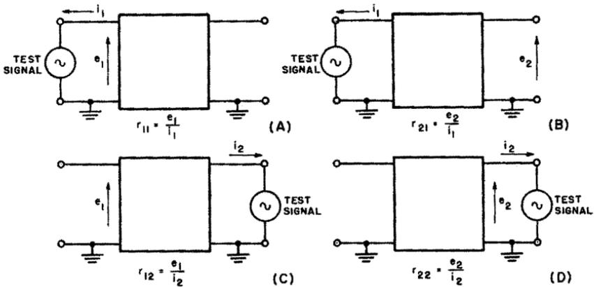
Fig. 3-8. Basic circuits for measuring four-terminal parameters.
