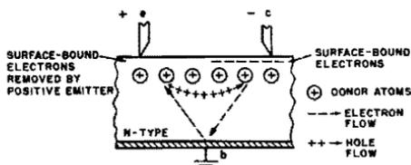
Fig. 2-4 (bottom). N-type and P-type point-contact transistor connections.
