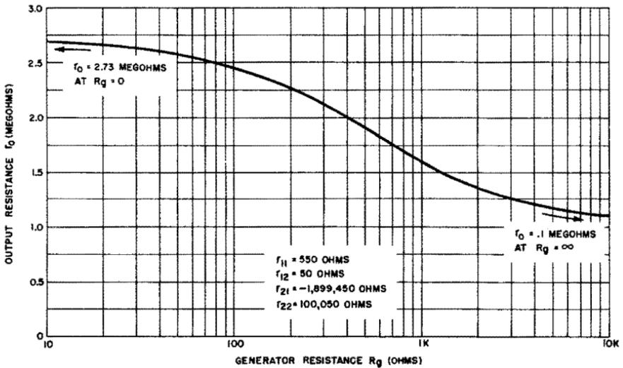
Fig. 4-6. Output resistance vs generator resistance for typical junction transistor (grounded emitter).
