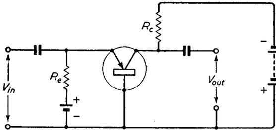
*Fig. 6.1. Simple uncompensated common-base amplifier which has good thermal stability*
