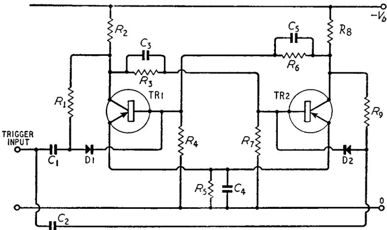
*Fig. 12.3. The circuit of Fig. 12.2 with diode triggering gate*
