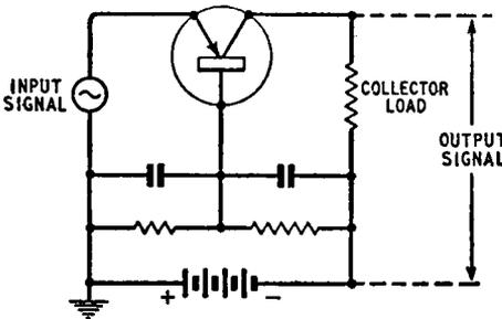
*Fig. 2.7. The circuit of Fig. 2.6 using a single battery and a potential divider providing base bias*
