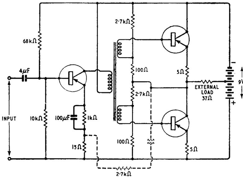
Fig. 10.7. Circuit for a driver and asymmetric class-B output stage. Dotted lines show how negative feedback can be applied when the driver stage has a voltage input
