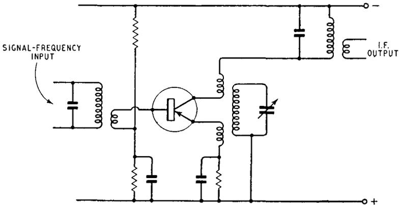
Fig. 11.11. One possible circuit for a self-oscillating mixer
