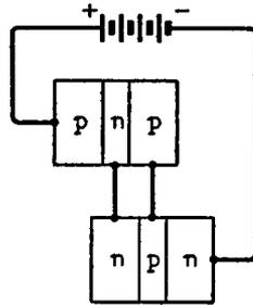
*Fig. 14.6. Forward-biased rectifier represented as two direct-coupled transistors*
