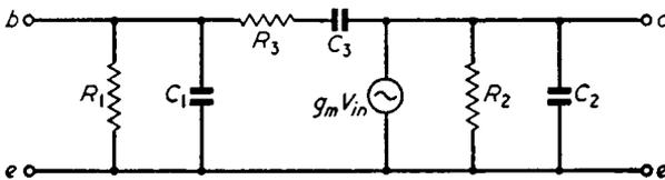
*Fig. 8.3. At a single frequency the  $\pi$ -section equivalent circuit of Fig. 8.2 can be reduced to this form*
