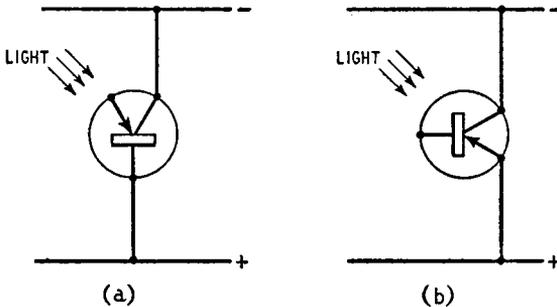
Fig. 13.11. Photo-sensitivity of a transistor arranged as at (b) is considerably greater than when arranged as at (a)
