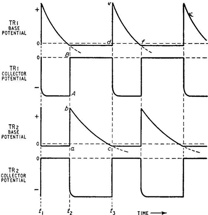
Fig. 12.8. Base and collector waveforms for the astable multivibrator of Fig. 12.7
