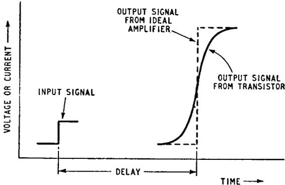
*Fig. 2.12. Form of distortion due to variation in current-carrier velocity in a junction transistor*
