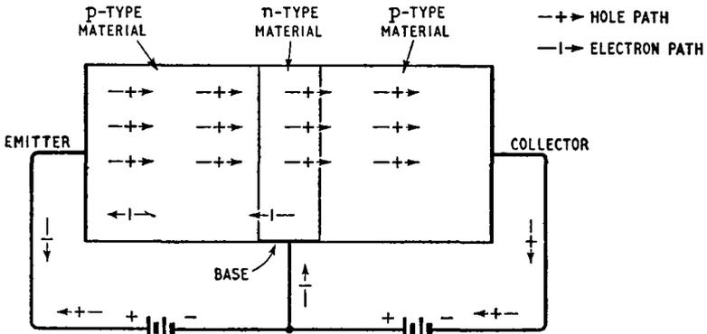
Fig. 2.5. Hole and electron paths in a pnp junction transistor connected for amplification
