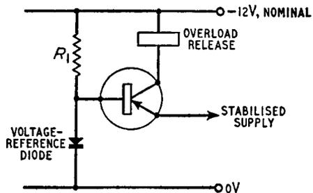
*Fig. 13.3. Voltage-stabilising circuit suitable for supplying large currents*
