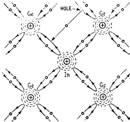
Fig. 1.7. Illustrating covalent bonds in the neighbourhood of an atom of a Group III element, introduced into a crystal of pure germanium. For simplicity, only electrons in the valence rings are shown
