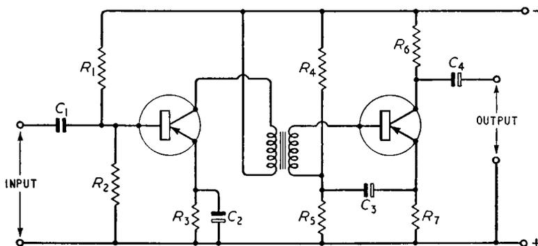
*Fig. 7.3. A small-signal a.f. amplifier consisting of two transformer-coupled common-emitter stages*
