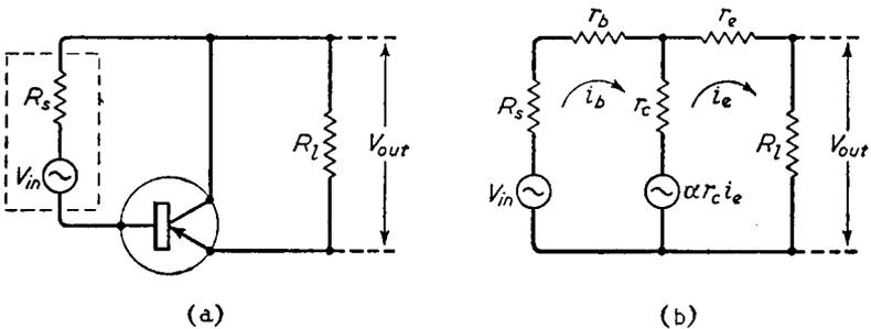
Fig. 5.1. The basic circuit for the common-collector transistor amplifier is given at (a), and the equivalent circuit at (b)
