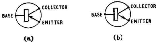
Fig. 2.3. Circuit diagram symbols for (a) a pnp and (b) an npn junction transistor
