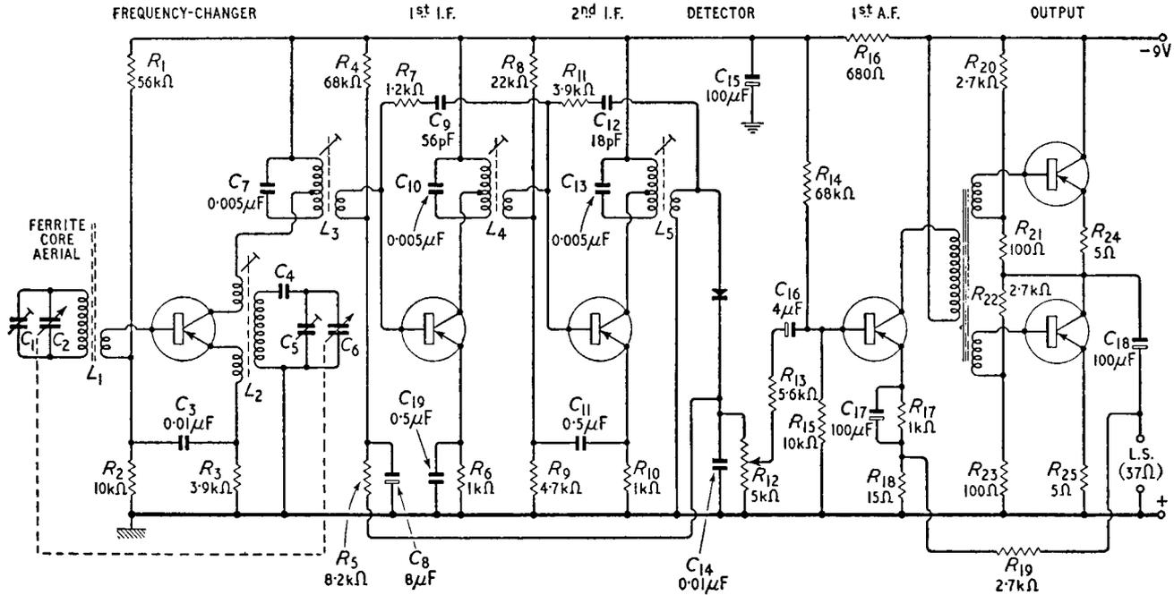
Fig. 11.13. Circuit diagram of complete single-waveband superheterodyne transistor receiver
