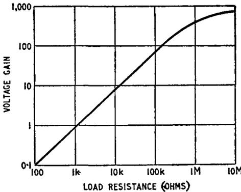
Fig. 3.9. Variation of voltage gain with load resistance for a common-base amplifier
