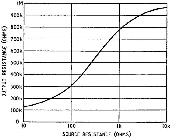
Fig. 3.8. Variation of output resistance with source resistance for a common-base amplifier
