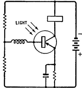
Fig. 13.14. Circuit using a photo-transistor with an interrupted light input
