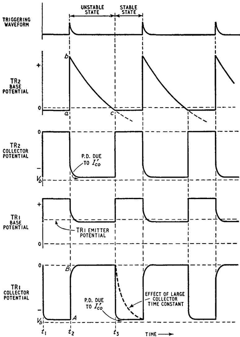
Fig. 12.6. Base and collector waveforms for the monostable multivibrator of Fig. 12.5
