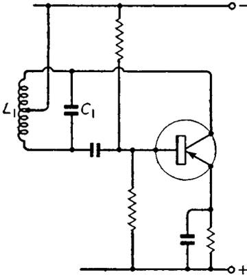
Fig. 11.1. One possible circuit for a transistor Hartley oscillator
