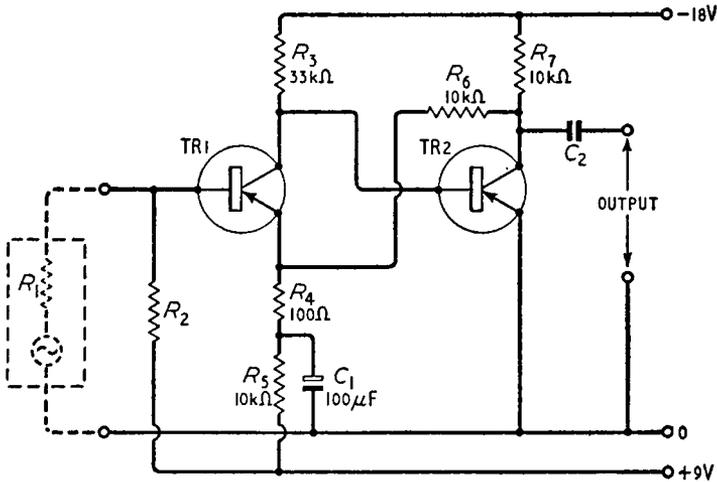
Fig. 9.3. A two-stage voltage amplifier with negative feedback
