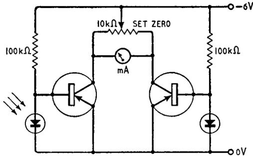
Fig. 13.10. Light-meter circuit employing two photo-diodes and two transistors
