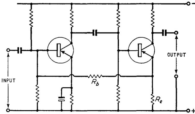
Fig. 7.5. A two-stage transistor current amplifier with low input resistance and high output resistance
