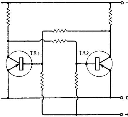
*Fig. 12.1. Basic circuit of bistable multivibrator using transistors*
