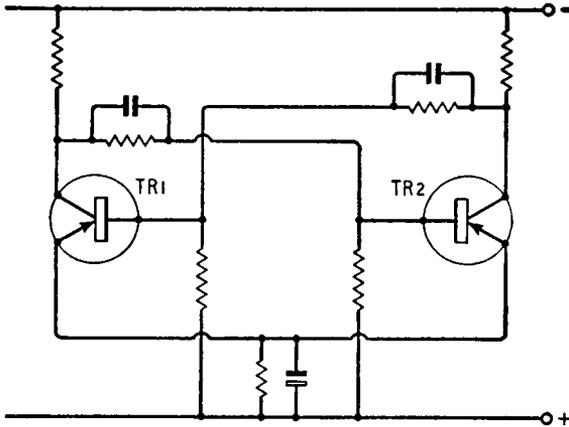
*Fig. 12.2. Transistor bi-stable multivibrator with speed-up capacitors*
