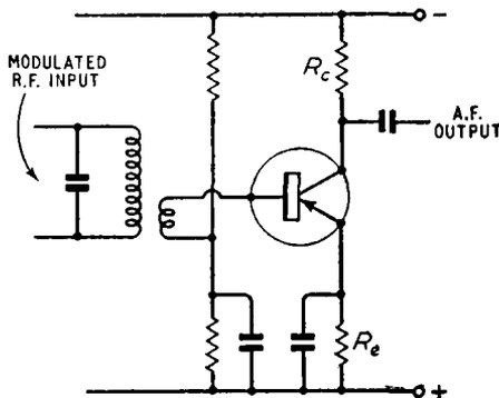
Fig. 11.4. One circuit for a common-emitter transistor a.m. detector
