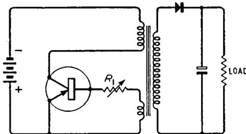
*Fig. 13.8. Complete circuit of transistor d.c. converter*
