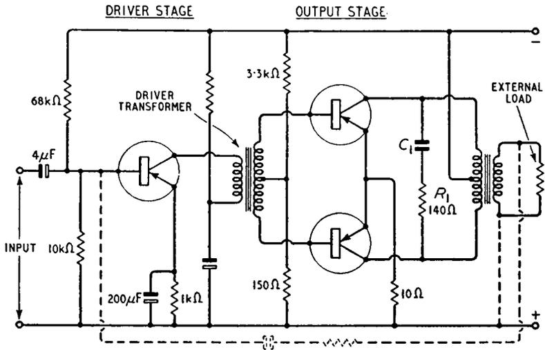
Fig. 10.6. Circuit for a driver and a symmetrical class-B output stage. Dotted lines show how negative feedback can be applied when the driver stage has a current input
