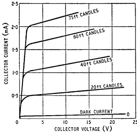
Fig. 13.12. Characteristics of a photo-transistor
