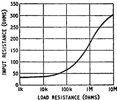
*Fig. 3.6. Variation of input resistance with load resistance for a common-base amplifier*
