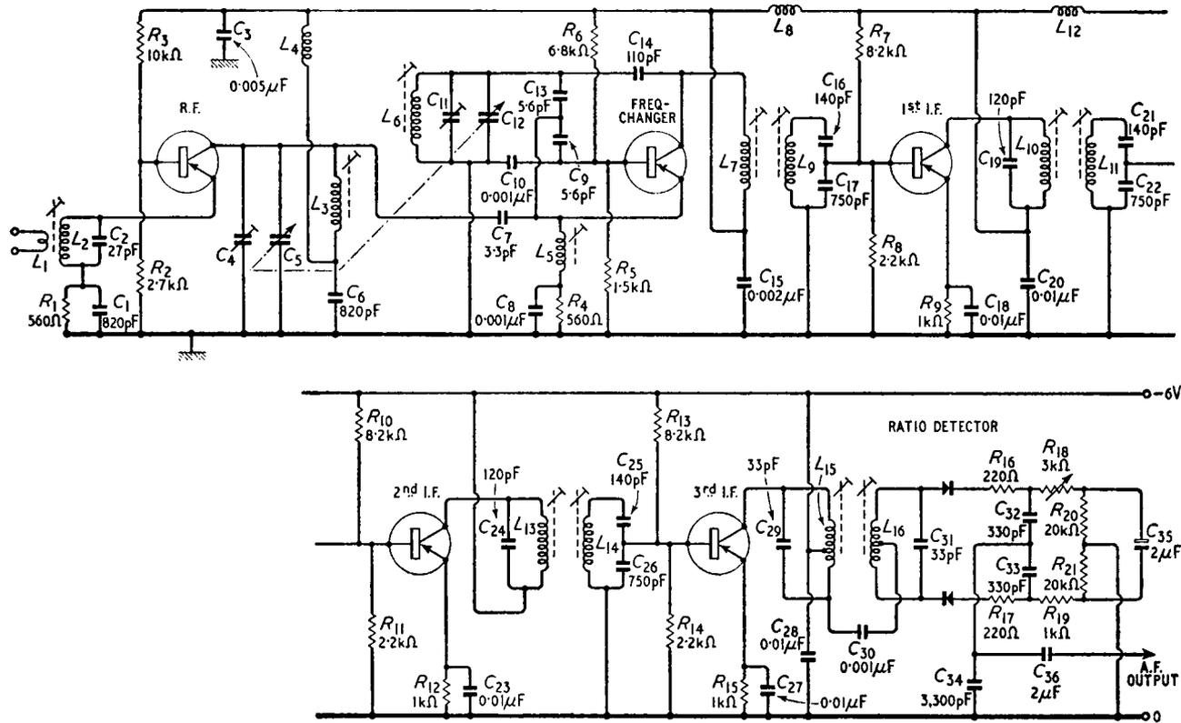
Fig. 11.14. Circuit diagram of a transistorised f.m. receiver up to the a.f. output from the detector
