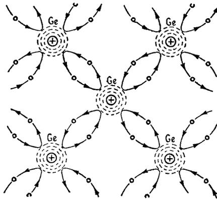
*Fig. 1.5. Illustrating covalent bonds in a crystal of pure germanium : for simplicity, only electrons in the valence rings are shown*
