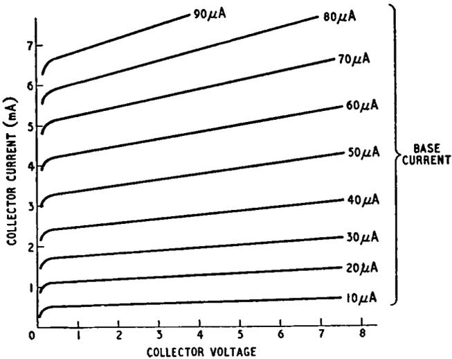
Fig. 4.6. Typical collector current-collector voltage characteristics for common-emitter connection
