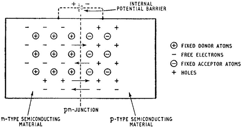
Fig. 1.8. Pattern of fixed and mobile charges in the region of a pn junction
