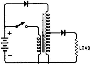
*Fig. 13.7. Basic converter circuit with provision for returning reverse secondary e.m.f. to the low-tension battery*
