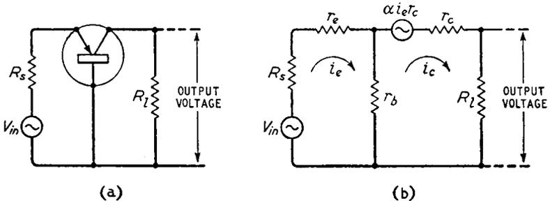
Fig. 3.4. Simplified circuit of a common-base amplifier (a), and its electrical equivalent (b)
