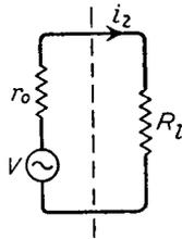
*Fig. 3.7. Circuit illustrating the meaning of output resistance*
