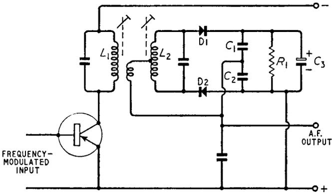
Fig. 11.8. One circuit for a ratio detector
