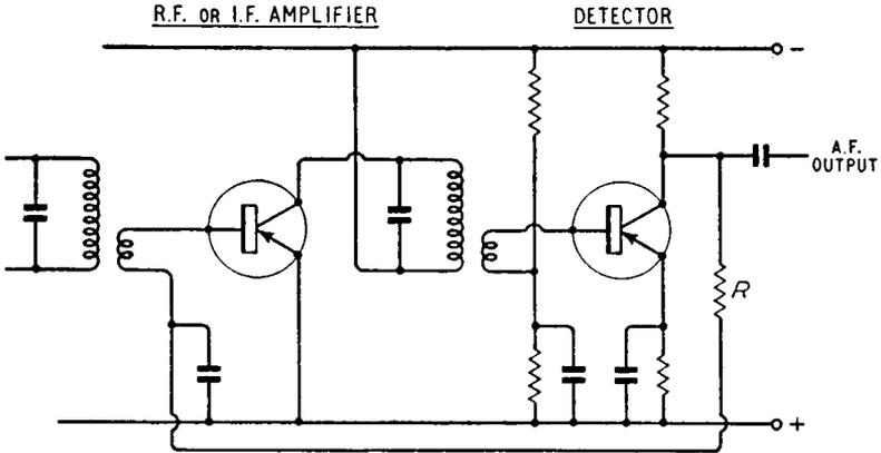
*Fig. 11.5. An a.g.c. circuit using emitter-current control*
