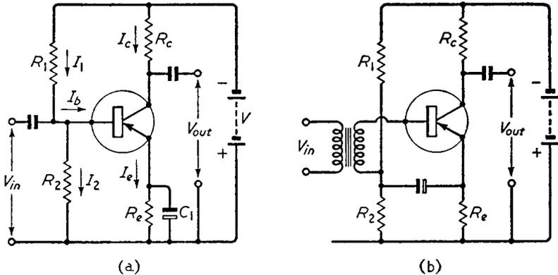
*Fig. 6.6. Potential divider method of stabilising the d.c. conditions in a common-emitter amplifier (a) in an RC-coupled amplifier and (b) in a transformer coupled amplifier. Arrows indicate electron flow*
