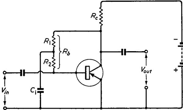
Fig. 6.4. To avoid negative feedback due to  $R_b$ , decoupling may be introduced as shown here
