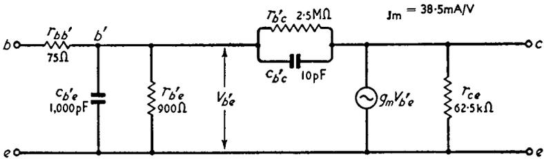
*Fig. 8.2. A  $\pi$ -section equivalent circuit of a uniform-base junction transistor*
