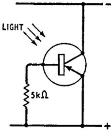
Fig. 13.13. A resistor connected between base and emitter of a photo-transistor can be used to improve the ratio of light current to dark current
