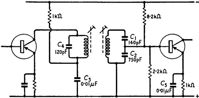
Fig. 8.10. A stage of a 10.7 Mc/s i.f. amplifier using drift transistors and double tuned transformers
