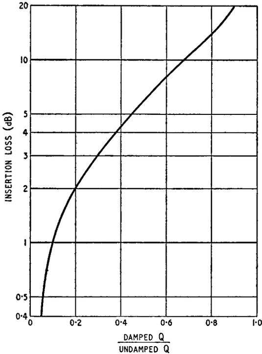
Fig. 8.7. Dependence of insertion loss on the ratio of damped to undamped  $Q$  values
