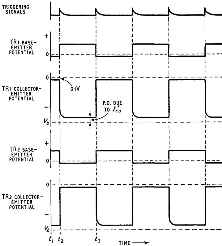
Fig. 12.4. Base and collector waveforms for the bi-stable multivibrator of Fig. 12.3
