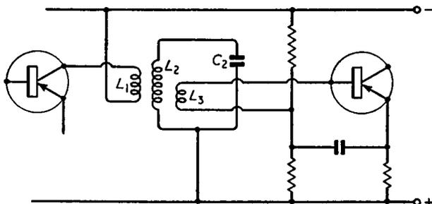
Fig. 8.6. Essential features of a transistor r.f. or i.f. amplifier: for simplicity neutralising components are omitted
