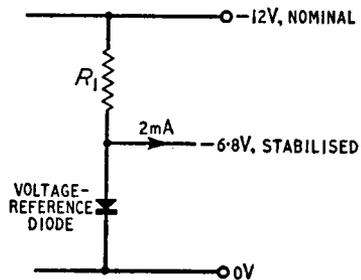
*Fig. 13.1. Simple junction-diode voltage stabilising circuit suitable for small currents*
