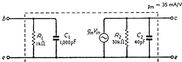
Fig. 8.5. For perfect unilateralisation the equivalent circuit for a uniform-base transistor reduces to this form
