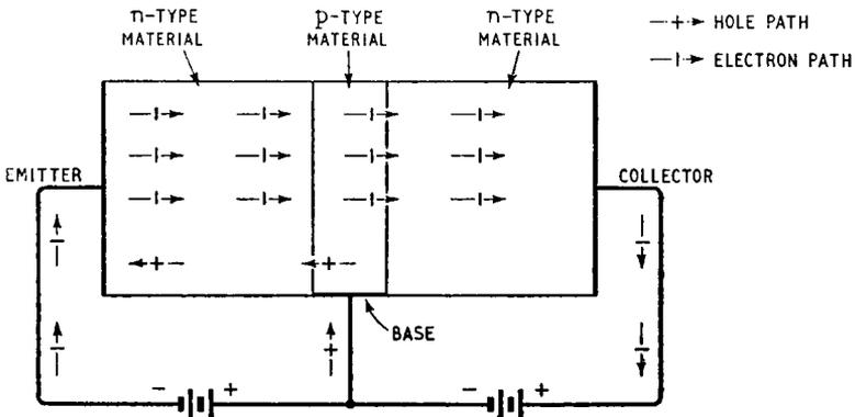
Fig. 2.8. Electron and hole paths in an npn junction transistor connected for amplification
