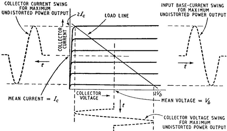
*Fig. 10.2. Conditions in a class-A transistor output stage*
