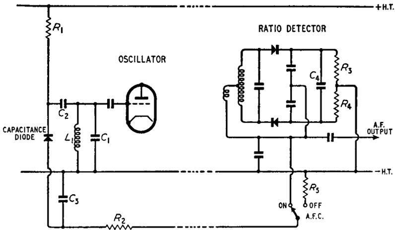
Fig. 13.4. Circuit illustrating the use of a junction diode to give a.f.c.
