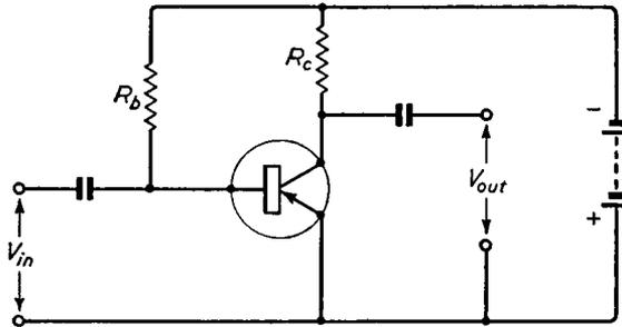
*Fig. 6.2. Simple uncompensated common-emitter amplifier which has poor thermal stability*
