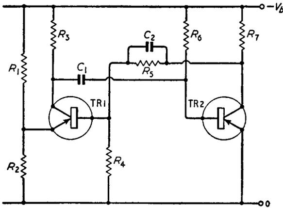
*Fig. 12.5. Transistor monostable multivibrator*
