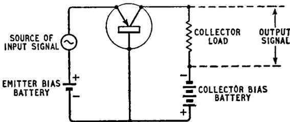
*Fig. 2.6. Basic circuit for using a pnp junction transistor as an amplifier*
