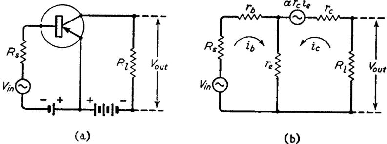
Fig. 4.1. Basic form of common-emitter amplifier (a), and its equivalent circuit (b)
