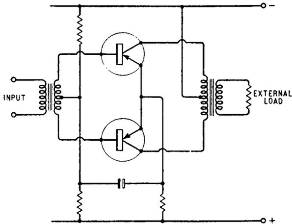
*Fig. 10.3. Circuit for a push-pull class-A transistor output stage*
