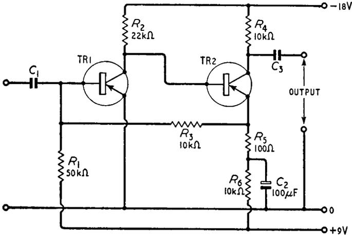
*Fig. 9.2. A two-stage current amplifier with negative feedback*
