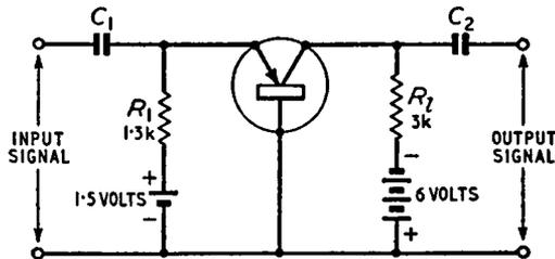
*Fig. 3.10. Circuit for small-signal common-base transistor amplifier*
