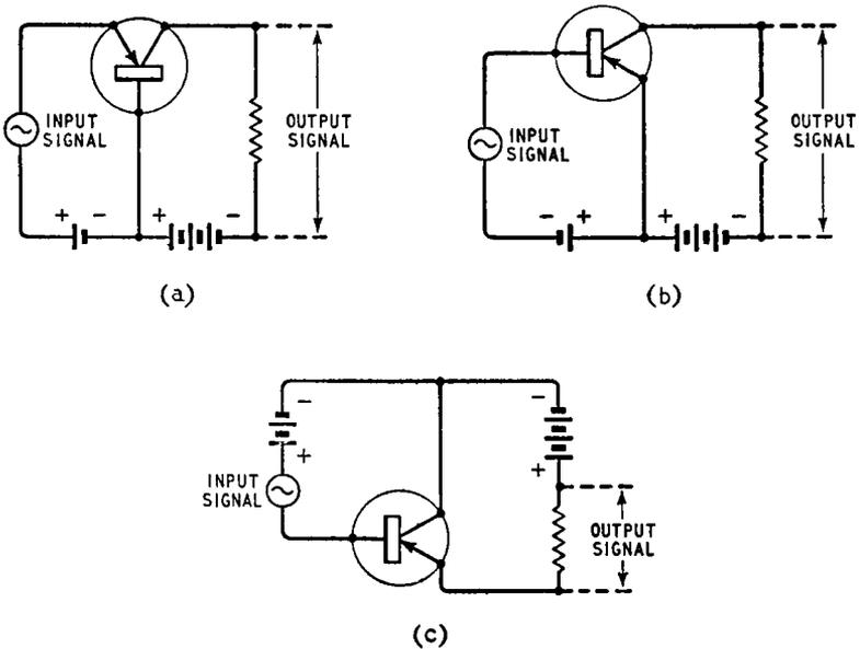
Fig. 3.1. The three basic forms of transistor amplifier: (a) common-base, (b) common-emitter, and (c) common-collector
