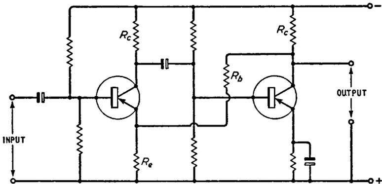
Fig. 7.6. A two-stage transistor voltage amplifier having high input resistance and low output resistance
