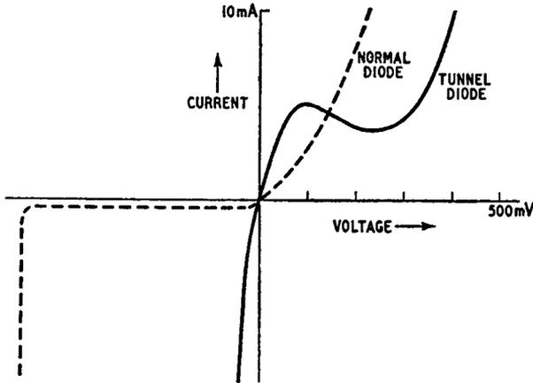
Fig. 14.3. Characteristic of a tunnel diode (solid) compared with that of a normal junction diode (dashed)
