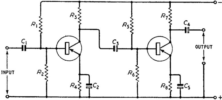
Fig. 7.2. A small-signal a.f. amplifier consisting of two RC-coupled common-emitter stages
