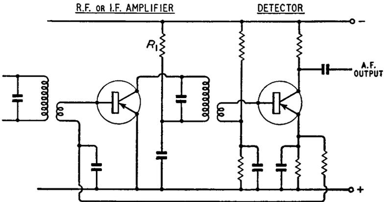
*Fig. 11.6. An a.g.c. circuit using collector-voltage control*
