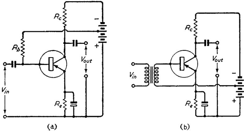
Fig. 6.7. Two-battery method of stabilising the d.c. conditions in a common-emitter amplifier (a) in an RC-coupled amplifier and (b) in a transformer-coupled amplifier
