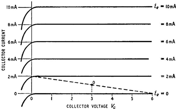
Fig. 3.11. Typical collector current–collector voltage characteristics for a junction transistor
