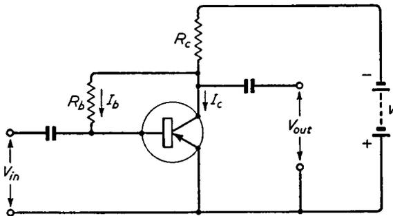
Fig. 6.3. A simple method of improving the thermal stability of a common-emitter amplifier
