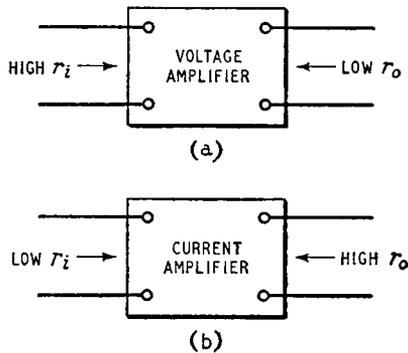
Fig. 7.1. Fundamental properties of (a) a voltage amplifier and (b) a current amplifier
