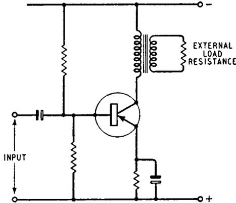
Fig. 10.1. Essential features of a single-ended class-A transistor output stage
