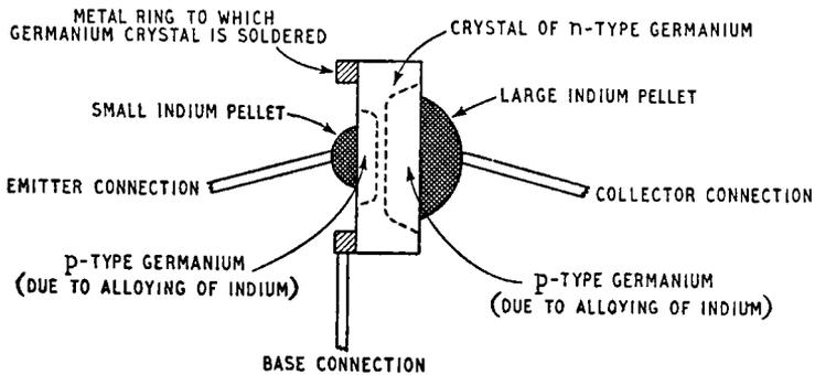
Fig. 2.4. Construction of alloy junction pnp germanium transistor
