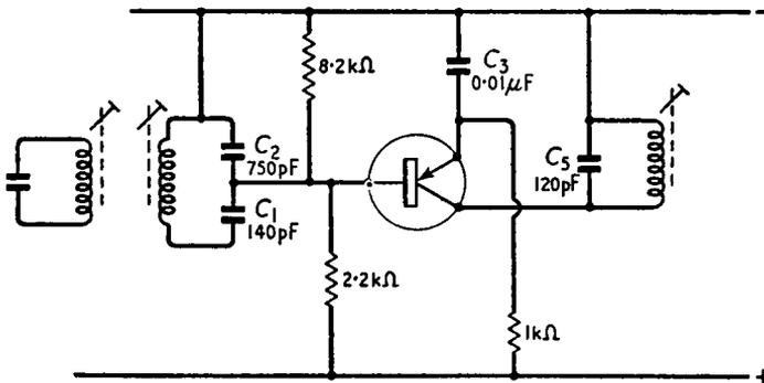
Fig. 8.11. A modified version of the wiring of Fig. 8.10 which eliminates the need for collector decoupling components
