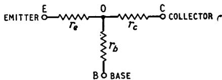
Fig. 3.2. A three-terminal passive network which can be used to build an equivalent circuit for a transistor
