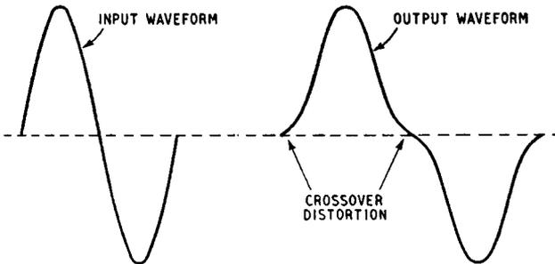
Fig. 10.5. Input and output waveforms for an amplifier giving cross-over distortion
