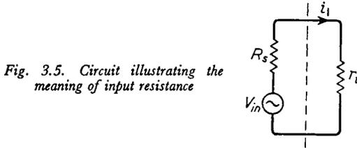
feedback of the transistor mentioned earlier. For a given transistor operating under constant d.c. conditions,  $r_b$ ,  $r_e$ ,  $r_c$  and  $\alpha$  are constant, and  $r_i$  therefore depends solely on  $R_l$ , increasing as  $R_l$  increases.
