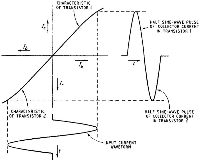
Fig. 10.4. Operation of a push-pull class-B transistor amplifier
