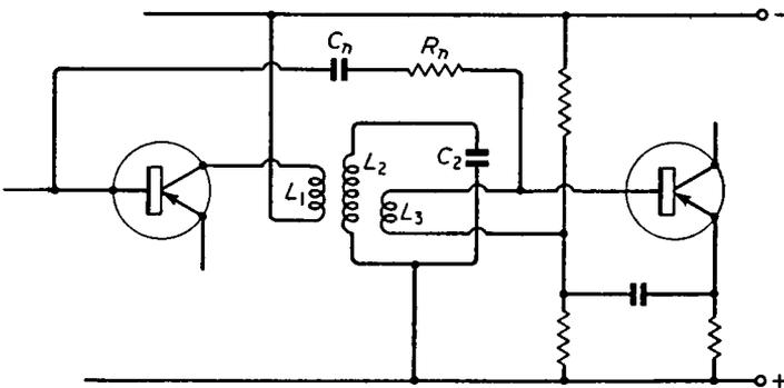
Fig. 8.9. Complete circuit of common-emitter transistor r.f. or i.f. amplifier including unilateralising components  $R_n$  and  $C_n$
