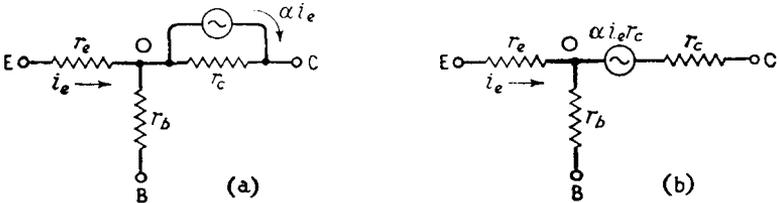
Fig. 3.3. A three-terminal active network which can be used as an equivalent circuit for a transistor (a) including a constant-current generator, and (b) a constant-voltage generator
