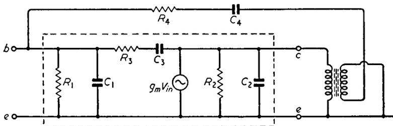
*Fig. 8.4. Method of unilateralising a junction transistor by means of a phase-inverting transformer and components  $R_4$  and  $C_4$*
