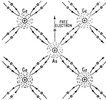
Fig. 1.6. Illustrating covalent bonds in the neighbourhood of an atom of a Group V element introduced into a crystal of pure germanium. For simplicity, only electrons in the valence rings are shown
