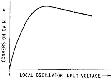
Fig. 11.10. Variation of conversion gain with local-oscillator input voltage
