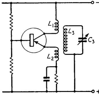
Fig. 11.3. One possible circuit for a transistor Reinartz oscillator
