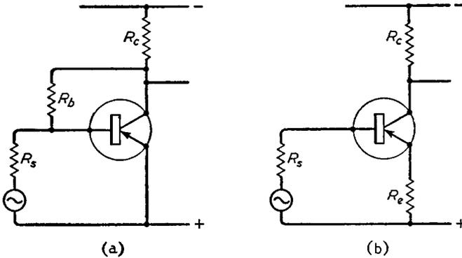
Fig. 7.4. Essential connections for two methods of applying negative feedback to common-emitter transistor amplifiers
