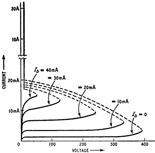
Fig. 14.7. Characteristics of a controlled rectifier
