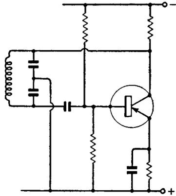
Fig. 11.2. One possible circuit for a transistor Colpitts oscillator
