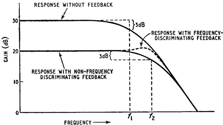
Fig. 9.1. Effect of negative feedback on the frequency response of an amplifier
