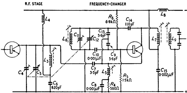
Fig. 11.12. A self-oscillating mixer of the Colpitts' type suitable for use in v.h.f. receivers
