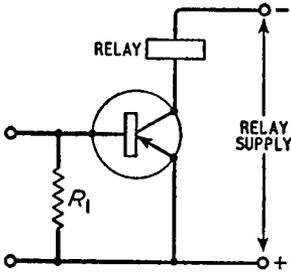
Fig. 13.5. Use of a transistor to increase relay sensitivity
