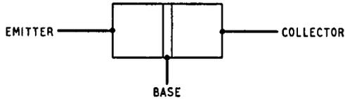
Fig. 2.2. Electrical connections to a junction transistor
