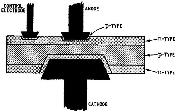
*Fig. 14.4. Construction of a controlled rectifier*
