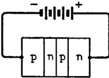
*Fig. 14.5. Reverse-biased controlled rectifier*
