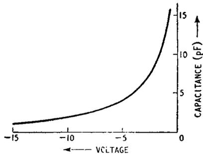
limits by alteration in the bias voltage. This is illustrated in the curve of Fig. 1.14: the capacitance varies with the voltage according to a law of the type
