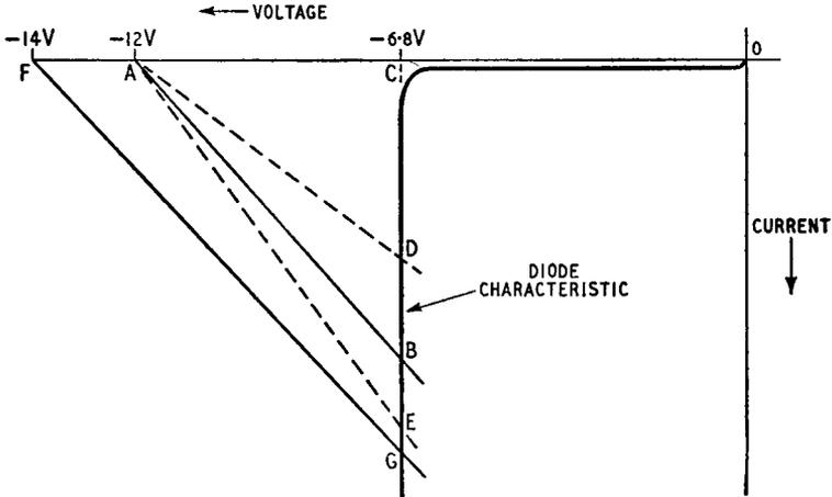
*Fig. 13.2. Illustrating the operation of a simple voltage-stabilising circuit*
