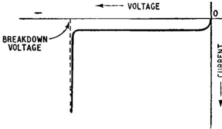
*Fig. 1.13. Breakdown in a reverse-biased pn junction*
