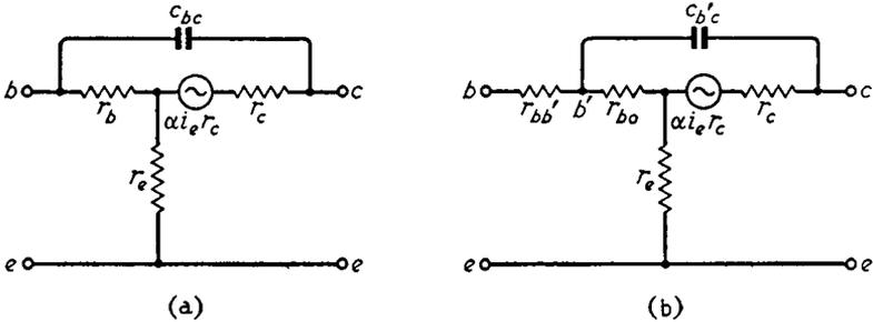
*Fig. 8.1. T-section equivalent circuit of a transistor showing collector capacitance, (a) returned to base input terminal and (b) returned to a tapping point on the base resistance*
