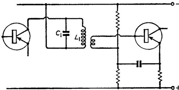
*Fig. 8.8. Simple form of transistor r.f. or i.f. amplifier: neutralising components are again omitted*
