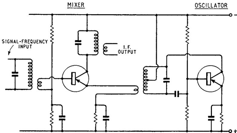
Fig. 11.9. One possible circuit for a two-transistor frequency changer
