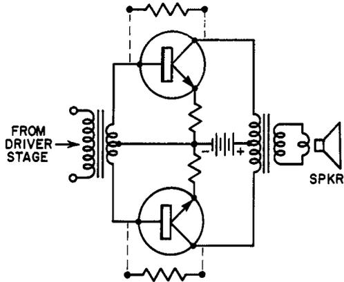
greater than  $I_{CQ}$ . The objective here is to keep operation within relatively linear regions of transistor characteristics, thereby minimizing distortion. The resistances form a voltage divider in conjunction with the resistance of the secondary of the driver transformer. The slight amount of feedback produced does not generally alter circuit performance; if anything, decreased distortion at the crossover points results.
