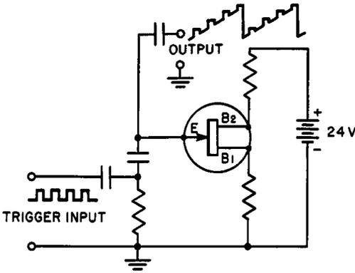
Fig. 7-9. Double-base diode connected as a synchronized frequency divider.
