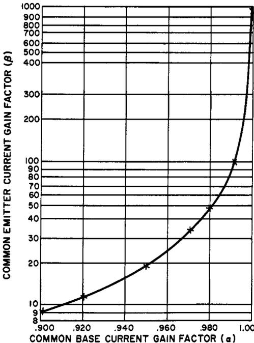
Fig. 6-6. Relationship between current gain factors  $\alpha$  and  $\beta$ .
