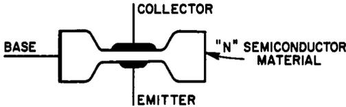
Fig. 4-8. The surface-barrier transistor.
