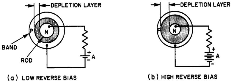
Fig. 7-6. Electronic control of effective cross-sectional area in rod of unipolar field transistor.
