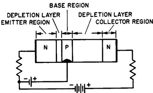
Fig. 3-6. An alternative method for biasing the transistor.
