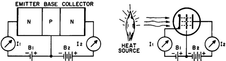
Fig. 3-12. A vacuum-tube analogy for  $\alpha$  in the transistor. Here we produce cathode emission with the aid of an external heat source. Space current is then governed by positive grid voltage supplied by battery  $B_1$ .
