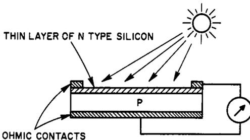
Fig. 7-28. The silicon solar generator.
