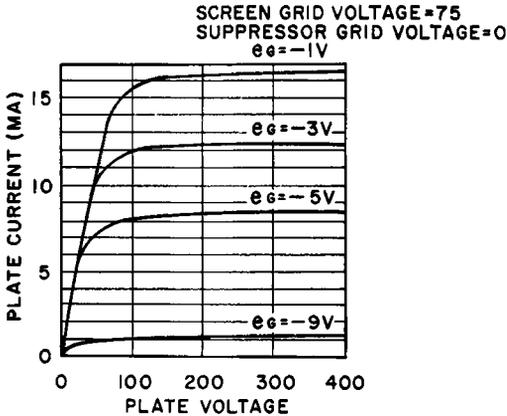
Fig. 3-9. Plate current vs. plate voltage for a typical small pentode tube. Note similarity with Fig. 3-8.
