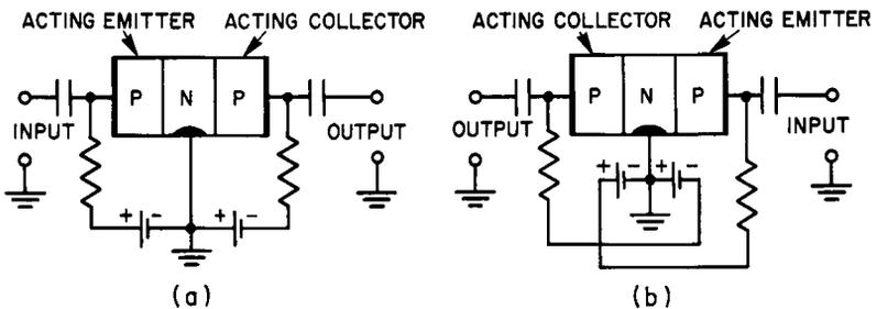
Fig. 7-20. Example of possible use of bilateral transistor in an intercommunications amplifier: (A) bias connected for "listen"; (B) bias connected for "talk."
