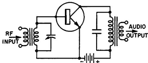
Fig. 5-12. Detector circuit.
