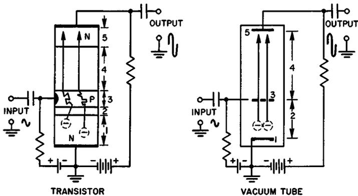
Fig. 3-7. Amplification in a transistor is in many ways analogous to amplification in a vacuum tube. Although generally not required and often undesirable, a small positive bias is shown applied to the grid of the vacuum tube in order to reinforce the analogy.
