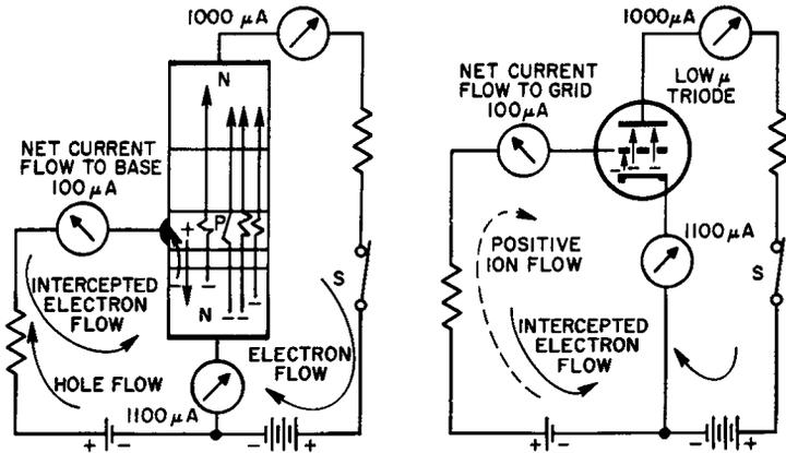
Fig. 3-10. Transistor amplifier and an analogous tube arrangement for demonstrating current in control circuit. In both circuits the current in the connection to the control element circulates in the input circuit and is lost to the collecting element. The situation for a p-n-p transistor would be the same as that shown for an n-p-n structure except for reversal of battery polarities and interchange in roles of electrons and holes.
