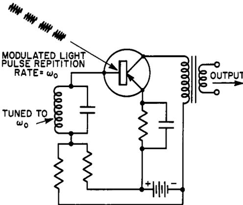
Fig. 7-30. Phototransistor circuit for high signal-to-noise ratio.
