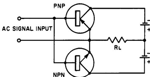
Fig. 6-12. Circuit illustrating basic principle of complementary symmetry in push-pull class-B amplifier.
