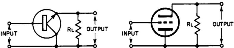
Fig. 6-2. Common collector and cathode follower circuits redrawn to facilitate comparison with other configurations.
