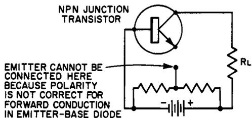
Fig. 5-7. Circuit showing that a divider network in conjunction with a single battery cannot provide both biases in d-c common-base circuit.
