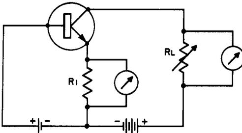
Fig. 5-5. Relative effects on d-c feedback stabilization produced by emitter and collector resistances.
