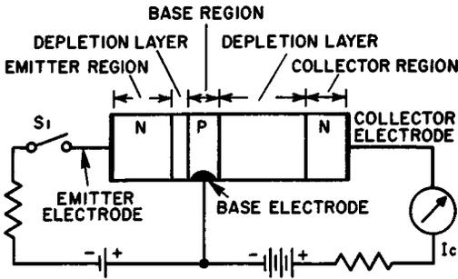
Fig. 3-5. Complete transistor structure with a possible biasing arrangement. Basic transistor action is demonstrated by this circuit. Collector current flows when switch  $S_1$  is closed, but falls to very low value when  $S_1$  is open.
