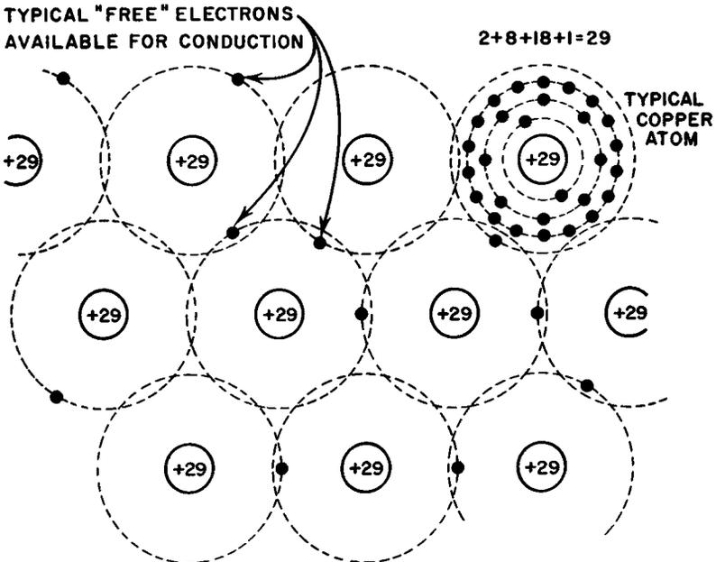
Fig. 2-1. Copper atoms are densely packed. The outer orbit electrons are free to move from atom to atom because these orbits overlap one another.
