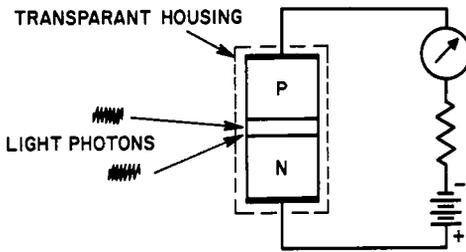
Fig. 7-27. The junction photodiode.
