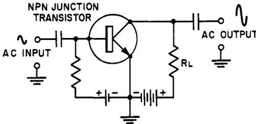
Fig. 5-2. Two-battery bias arrangement in d-c common-emitter circuit.
