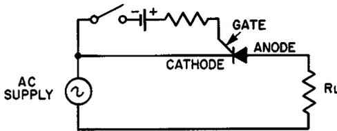
Fig. 7-11. Basic half-wave controlled silicon rectifier circuit.
