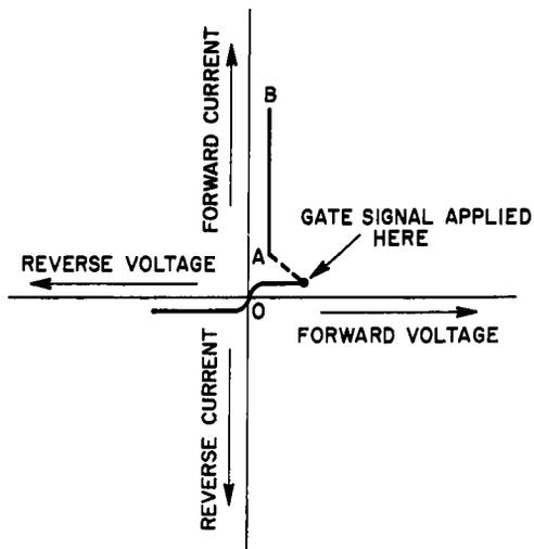
Fig. 7-15. Effect of gate signal on forward conduction of silicon controlled rectifier.
