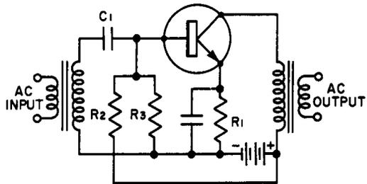
Fig. 6-9. One way of using transformer coupling.
