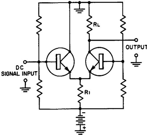
Fig. 5-15. The transistor differential amplifier.
