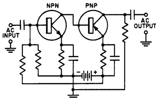
Fig. 6-11. Transistor amplifier employing principle of complementary symmetry.
