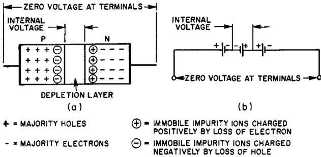
Fig. 2-11. (A) Static representation of charge condition within a p-n diode; (B) equivalent battery circuit showing why internal voltage does not appear across terminals.
