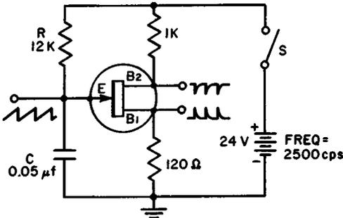
Fig. 7-8. Double-base sawtooth generator.
