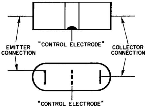
Fig. 1-2. Analogous electrode functions and operating principles prevail for transistors and vacuum tubes.
