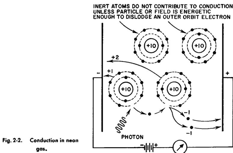
Fig. 2-2. Conduction in neon gas.
