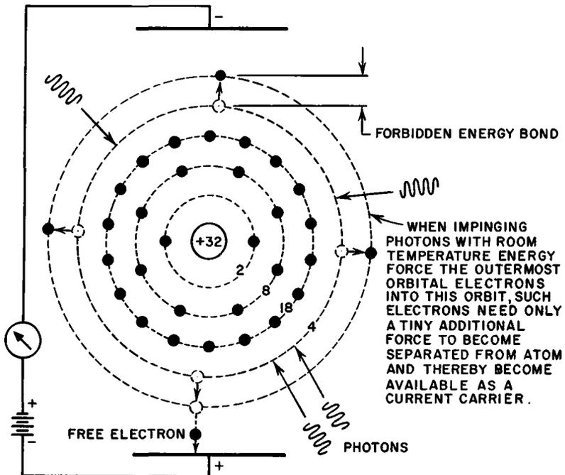
Fig. 2-5. At room temperature, a small force suffices to produce free electrons in germanium.
