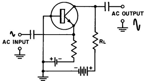
Fig. 5-1. Two-battery bias arrangement in d-c common-base circuit.
