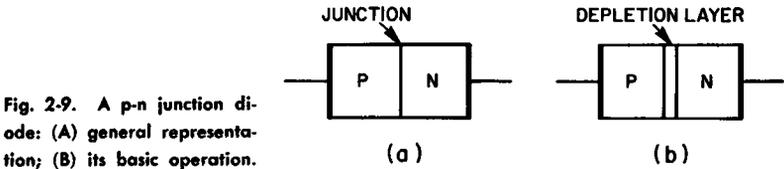
Fig. 2-9. A p-n junction diode: (A) general representation; (B) its basic operation.
