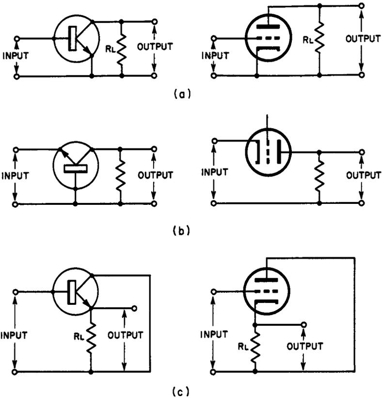
Fig. 6-1. The three transistor configurations and their vacuum-tube counterparts (a-c essentials only); (A) common emitter; (B) common base; (C) common collector.
