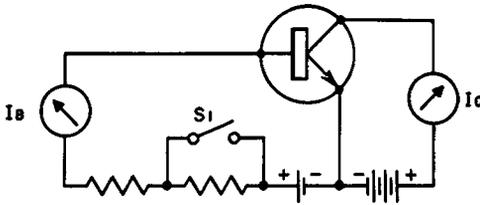
Fig. 6-5. Circuit for direct measurement of current-gain factor  $\beta$  in common-emitter amplifier.
