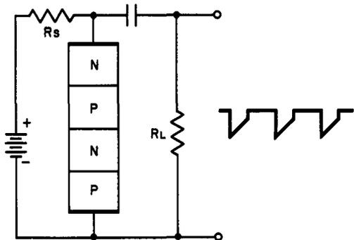
Fig. 7-17. The four-layer diode employed as a relaxation oscillator.
