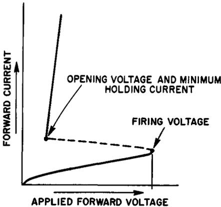
Fig. 7-16. Forward breakdown characteristic of the four-layer diode.
