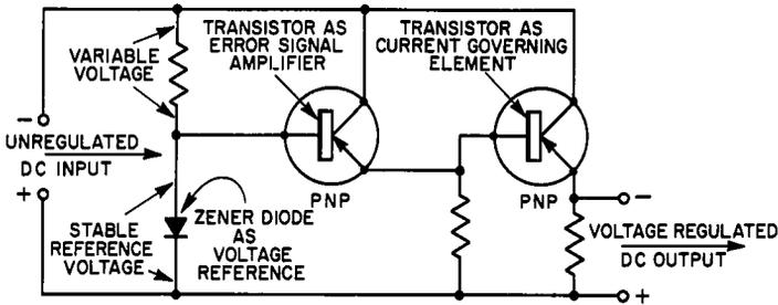
Fig. 7-24. The Zener diode as a voltage reference in a regulated d-c power supply.
