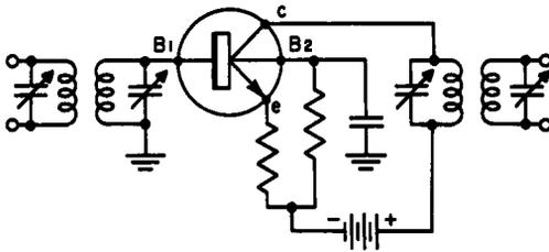
Fig. 7-3. Tetrode transistor i-f amplifier.
