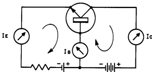
Fig. 6-7. Insight into common-emitter operation is provided by consideration of base current in the common-base amplifier.
