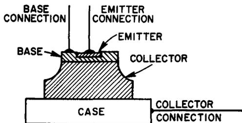
Fig. 4-5. Basic structure of diffused-base transistor.
