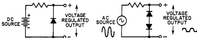
Fig. 7-22. D-c and a-c voltage-regulating circuits using Zener diodes.
