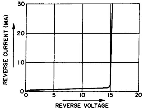
Fig. 2-14. Voltage breakdown characteristic in a p-n junction diode.
