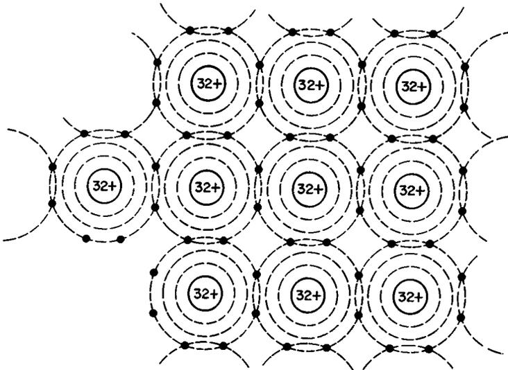
Fig. 2-3. Covalent sharing of electrons in germanium. Each atom satisfies its desire for eight outer-orbit electrons.
