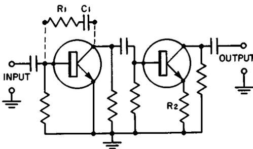
Fig. 6-14. A-c essentials of a two-stage amplifier which can be improved by load feedback.
