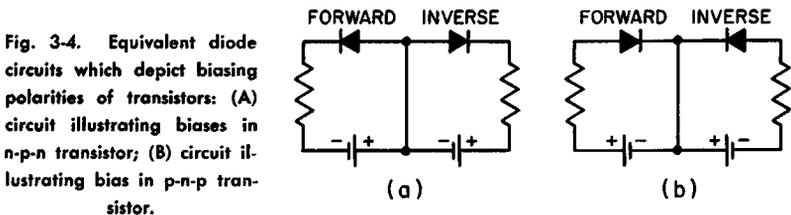
Fig. 3-4. Equivalent diode circuits which depict biasing polarities of transistors: (A) circuit illustrating biases in n-p-n transistor; (B) circuit illustrating bias in p-n-p transistor.
