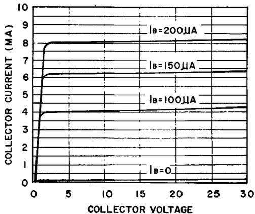
Fig. 3-8. Collector current vs. collector voltage for a typical n-p-n junction transistor (common emitter circuit). We are reminded of the pentode plate current vs. plate voltage relationship.
