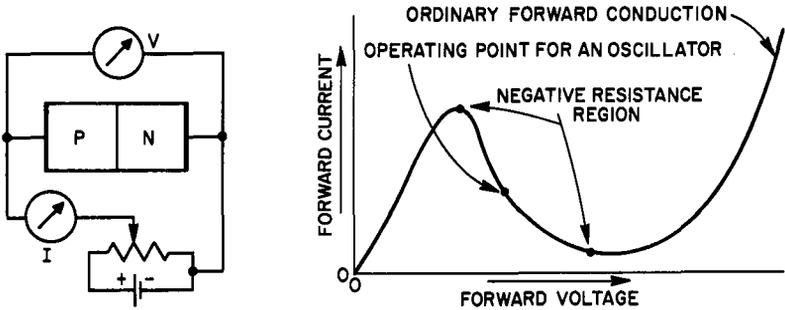
Fig. 7-31. Forward bias characteristics of the tunnel diode.
