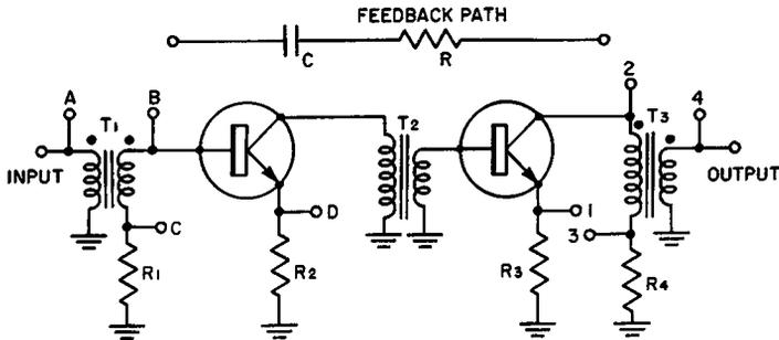
Fig. 6-13 A-c essentials of two-stage amplifier showing possible points for connection of feedback path. Refer to Table 6-3 for significance of various connections.
