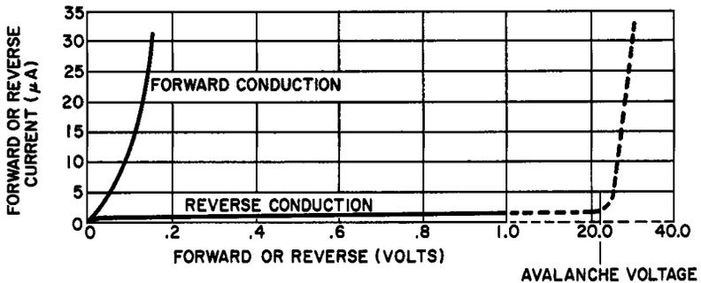
Fig. 4-10. Conduction in typical germanium junction diode.
