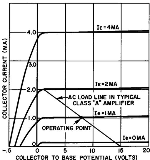
Fig. 6-4. Collector characteristics of typical small audio-type transistor in the common-base configuration.
