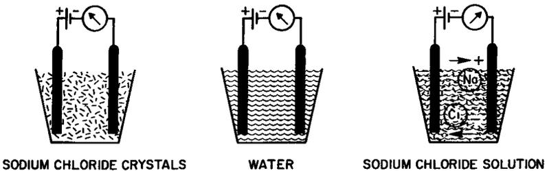
Fig. 1-10. Neither sodium chloride nor water provides charge carriers for the conduction of electricity. In the solution, however, disassociated sodium and chlorine ions move to the electrodes, thereby enabling the flow of the electric current.
