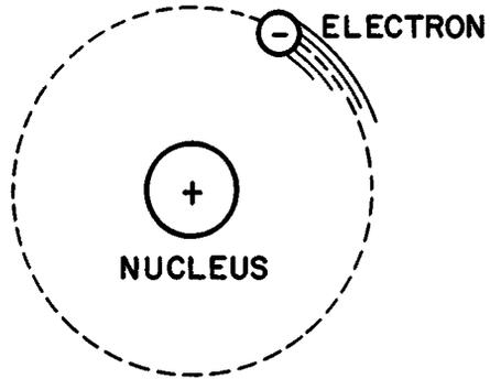
Fig. 1-5. The simple model of the hydrogen atom is depicted as a single electron in orbital motion about a nucleus, which bears a unit positive charge.
