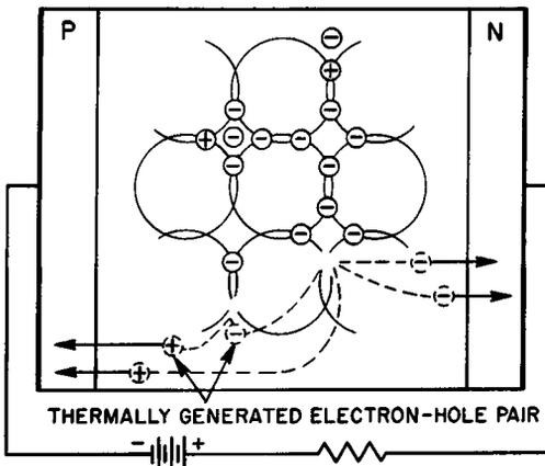
Fig. 2-15. Avalanche breakdown in p-n junction. Impact process is cumulative.
