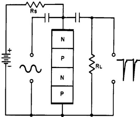
Fig. 7-18. The four-layer diode connected in a pulse generator circuit.
