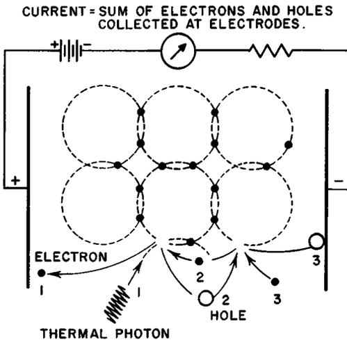
Fig. 2-4. Conduction in an intrinsic semiconductor such as pure germanium.
