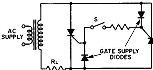
Fig. 7-12. Full-wave controlled rectifier circuit.
