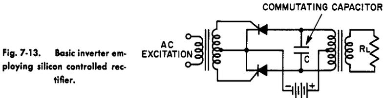
When the polarity of the current reverts to that necessary for conduction, the gate signal must be present to cause renewed firing. Instead of the switch, a control device such as a transistor may be used to satisfy a particular control requirement.
