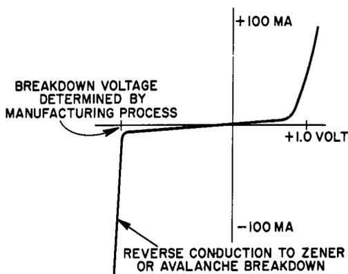
Fig. 7-21. Characteristic of the Zener diode. Reverse breakdown is caused by Zener phenomena when the breakdown voltage is less than about 5½ volts. For higher breakdown voltages, carrier avalanche is the predominant mechanics responsible for the abrupt increase in conduction.
