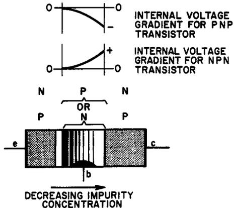
Fig. 4-7. The graded junction or "drift" transistor. Due to graded doping in base region, the base-collector "depletion layer" has no abrupt boundary in the base region.
