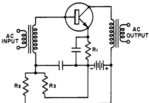
Fig. 6-10. Alternative transformer connections.
