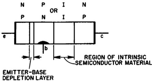
Fig. 4-6. The intrinsic-barrier transistor.
