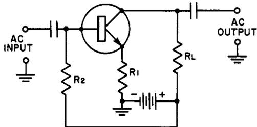
Fig. 5-8. Simplified single-battery stabilized bias circuit.
