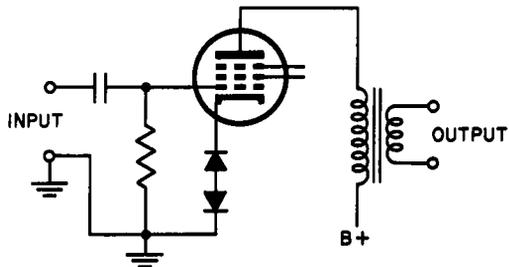
Fig. 7-23. Zener diode employed as source of cathode-grid bias in vacuum-tube amplifiers.
