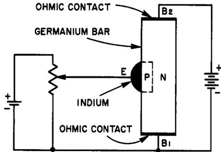
Fig. 7-7. The structure of the double-base diode and its biasing arrangement.
