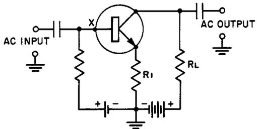
Fig. 5-4. Simple two-battery stabilized bias arrangement for d-c common-emitter circuit.
