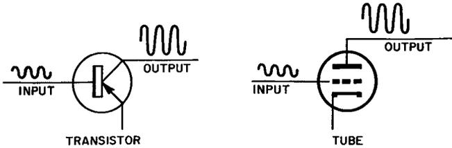
Fig. 1-1. The usefulness of both transistor and vacuum-tube stems from their ability to increase the power level of a weak signal applied to a control electrode.
