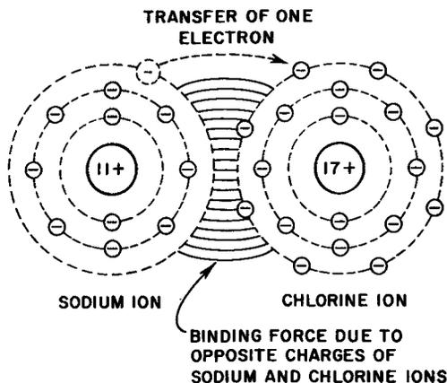
We see that the altered sodium atom now has a net positive charge of 1 unit, whereas the altered chlorine atom now has a net negative charge of 1 negative unit. These charge conditions constitute the force of chemical combination. As long as nothing is done to the resultant compound, sodium chloride, each atom satisfies its charge "hunger" on the other atom, thereby producing a condition of *charge stability*.
