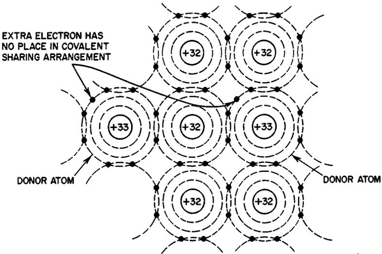
Fig. 2-6. Surplus electrons are contributed by a donor atom with five outer orbit electrons.
