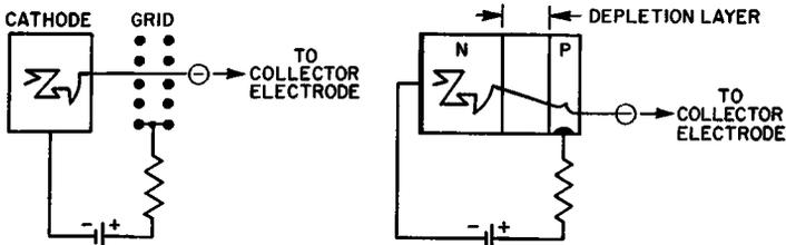
Fig. 3-3. Analogous mechanisms can be inferred from tube and semiconductor "electron gun."
