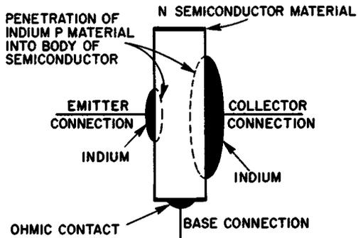
Fig. 4-4. Basic structure of p-n-p alloy junction transistor.
