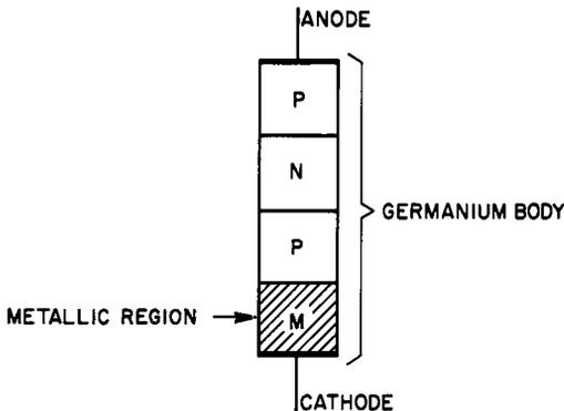
Fig. 7-19. Structure of the Westinghouse dynistor.
