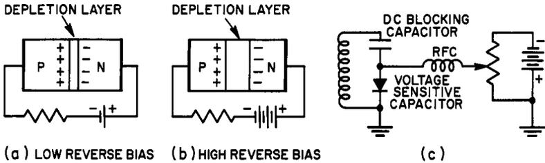
Fig. 7-26. The voltage-sensitive capacitor: (A) junction is narrow, producing a relatively high effective capacitance; (B) junction is wide, producing a relatively low effective capacitance; (C) turning a resonant circuit by means of a variable d-c voltage.
