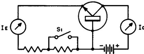
Fig. 6-3. Circuit for measuring  $\alpha$  in common-base configuration.
