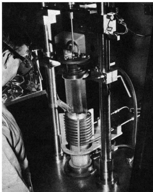
Fig. 4-1. Forming a silicon ingot. Ingot is slowly drawn upward from melt. Heat is supplied to melt from high-frequency induction generator via copper tubing coil.
