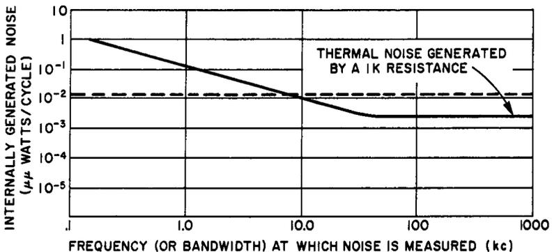
Fig. 6-18. Internally generated noise power as a function of frequency for typical small germanium junction transistor.
