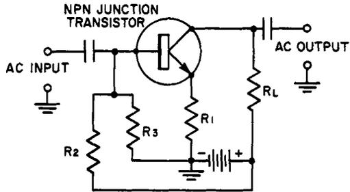
Fig. 5-6. Single-battery bias circuit.
