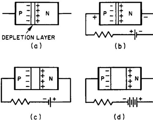
Fig. 2-12. Variation in width of depletion layer with applied voltage: (A) no voltage applied to diode; (B) forward conduction voltage; (C) low reverse voltage; (D) higher reverse voltage.
