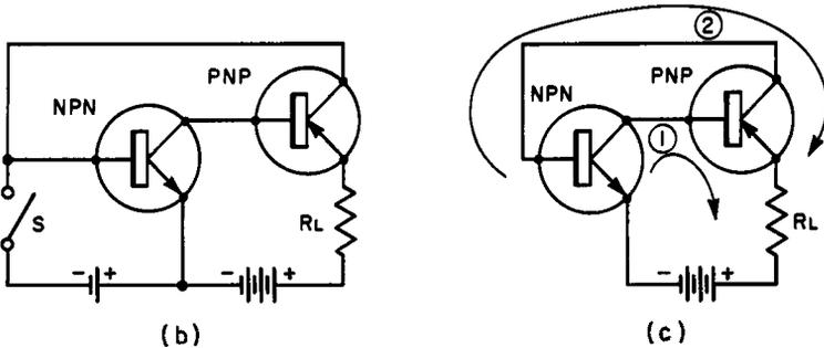
Fig. 7-10. The silicon controlled rectifier: (A) basic structure; (B) its approximately equivalent circuit; (C) flow of load current after conduction has been initiated by momentarily closing switch S.
