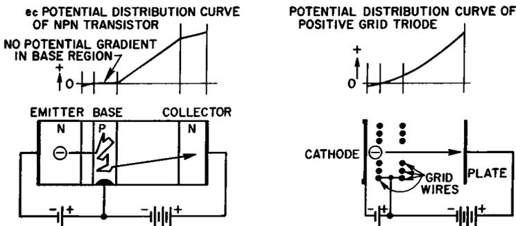
Fig. 3-13. A significant difference between transistor and tube action. The emitted charge carriers of the two devices encounter different field conditions in their respective control regions. In the transistor charge movement is by thermal diffusion. In the tube a potential gradient accelerates the charge through the grid region.
