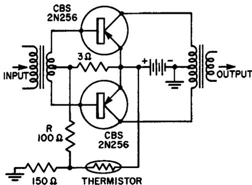
Fig. 5-13. Insertion of thermistor in power amplifier bias network to prevent degradation of performance and thermal runaway.
