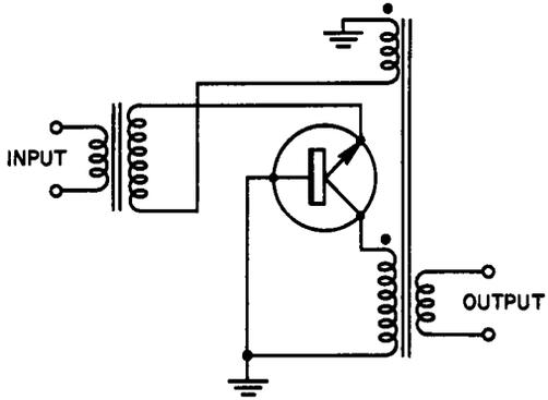
shunt-applied. Accordingly, both input and output impedance decrease with increasing feedback.
