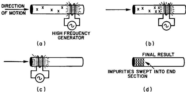
Fig. 4-2. Purification of semiconductor ingot by zone refining process.
