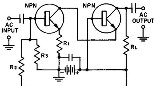
Fig. 5-10. Bias stabilization of transistor from constant-current source provided by previous stage.
