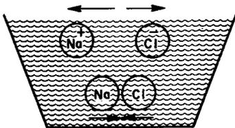
Fig. 1-11. Free ions continuously dissociate and reassociate.
