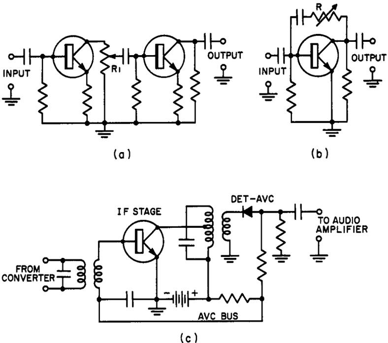
Fig. 6-17. Three gain-control methods: (A) Control of a-c input level to audio amplifier; (B) control of a-c gain by variable feedback in audio amplifier; (C) gain control by variation of base-emitter bias in i-f amplifier.
