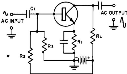
Fig. 6-8. A-c amplifier using capacitance coupling.
