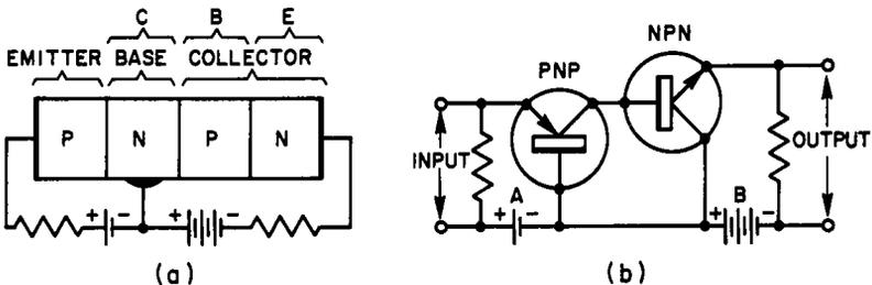
Fig. 7-4. The p-n-p-n hook transistor and an approximately equivalent circuit.
