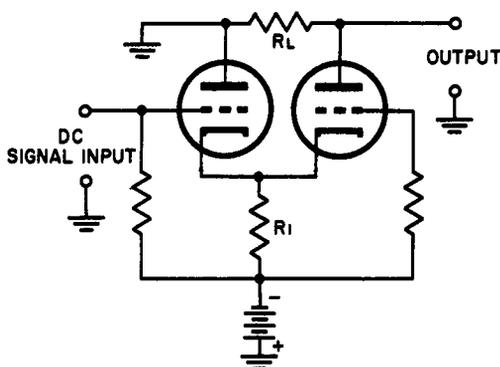
Fig. 5-14. The vacuum-tube differential amplifier.
