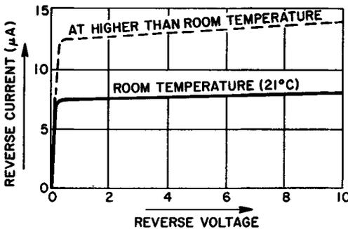
Fig. 2-13. The reverse current in a p-n junction diode is substantially constant over a wide range of applied voltage.
