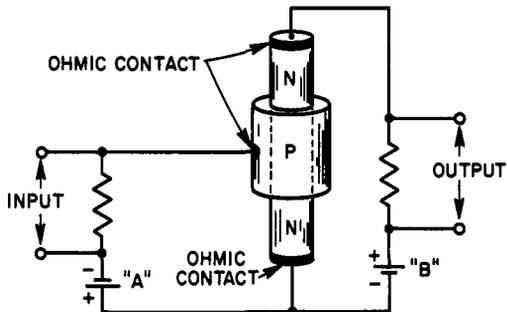
Fig. 7-5. Structure of the unipolar field controlled transistor.
