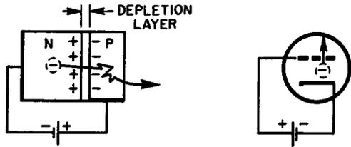
3-1 projects electrons into an n-p-n transistor, whereas the gun in Fig. 3-2 projects holes into a p-n-p transistor. The semiconductor guns differ from the p-n diode in two essential respects. First, one electrode contacts the *side* rather than the end of the structure; secondly, one doped region is very narrow. Let us consider the result of biasing the n-p gun in the forward direction.
