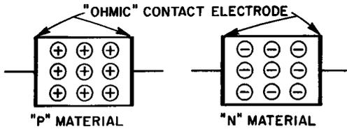
Fig. 2-7. Majority current carriers in "doped" semiconductor wafer. Conductivity in both devices is greatly enhanced over that of intrinsic conduction.
