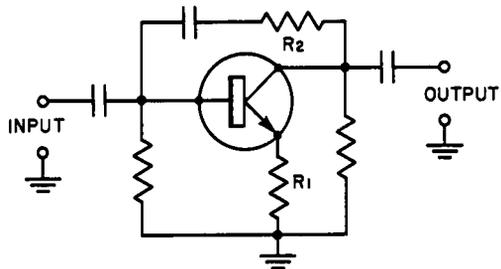
Fig. 6-15. Use of conjugate feedbacks to retain no-feedback impedances.
