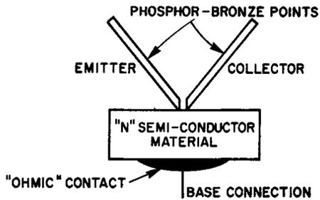
Fig. 4-9. Basic structure of the point-contact transistor.
