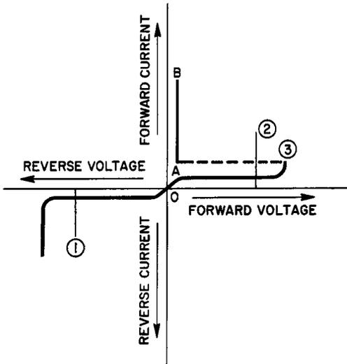
Fig. 7-14. Effect of a-c voltage impressed across silicon controlled rectifier with gate circuit open.
