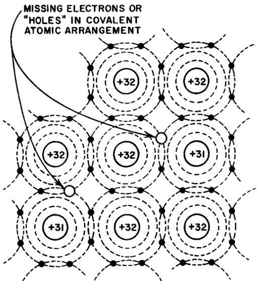
Fig. 2-8. "Holes" or loosely bound positive charges are contributed by acceptor atoms with three outer-orbit electrons.
