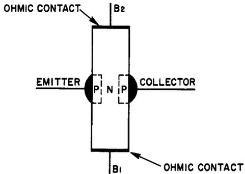
Fig. 7-1. The tetrode transistor.
