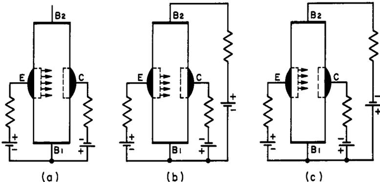
Fig. 7-2. Electronic control of effective emitting area in tetrode transistor: (A) no bias on  $B_2$ ; (B)  $B_2$  is negative with respect to  $B_1$ ; (C)  $B_2$  is negative with respect to  $B_1$ .
