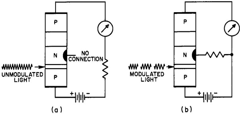
Fig. 7-29. The phototransistor: (A) connections with unmodulated light source; (B) connections with modulated light source.
