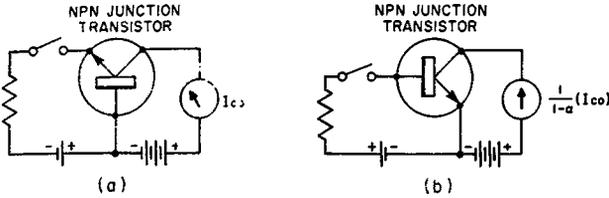
Fig. 5-3. The collector current with no forward bias applied to input diode: (A) collector battery is connected from collector to base, producing common-base circuit for dc; (B) collector battery is connected from collector to emitter, producing common-emitter circuit for dc.
