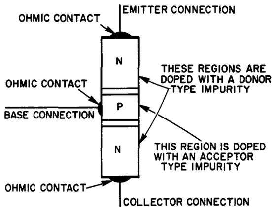
Fig. 4-3. Basic structure of grown junction and rate-grown junction transistors.
