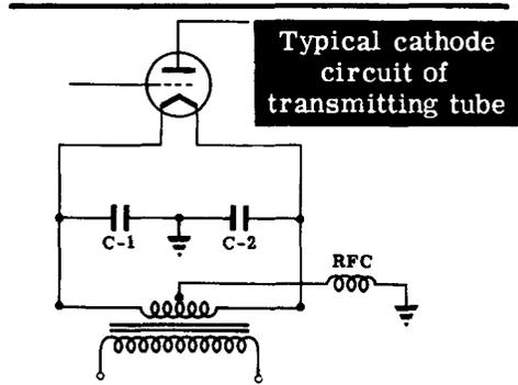
The filament is connected across a secondary winding of a filament transformer. This secondary winding is center-tapped to prevent the 60-cycle filament voltage from appearing in the plate signal of the tube.
