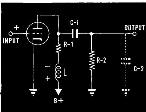
When the grid voltage swings negative, as at (b), the plate current decreases and the back emf across L is in the opposite direction. This then adds to the plate voltage—normally high anyway—causing another peak to appear at (b). Because of the effect of this inductance, it is always referred to as a "peaking coil."
