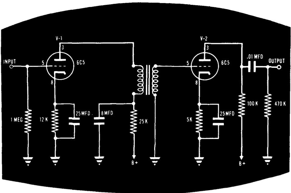
On the next sheet, a signal will be traced through the transformer-coupled amplifier and you will see how amplification occurs in this circuit.
