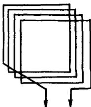
Another type of antenna used for portable and home receivers is the loop antenna. The loop consists of a coil of wire which is connected to the two ends of the primary of the antenna coil. Most home broadcast-band receivers contain a loop antenna within the cabinet.
