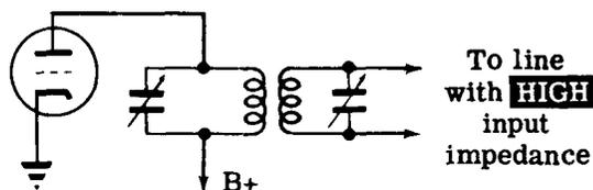
If the input impedance of the line is other than pure resistive, either of the above two tuned coupler circuits can be adjusted so that the reactance of the line is cancelled by the reactance of the tank circuit. This results in a pure resistive load, which is the requirement for maximum power transfer.
