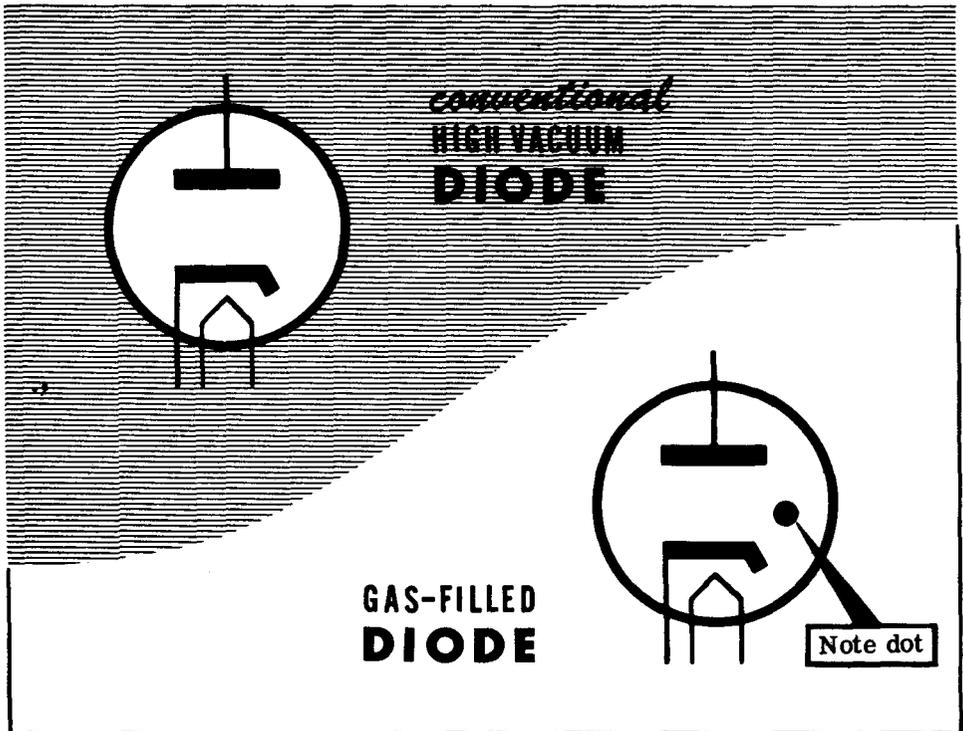
As you can see in the illustration, a gas tube has the same basic type of heater and cathode arrangement as the conventional diode. Many gas tubes have directly heated cathodes similar to the one in the type 80 high vacuum rectifier diode. Furthermore, the purpose of the cathode is the same in both types of tubes—to emit electrons.
