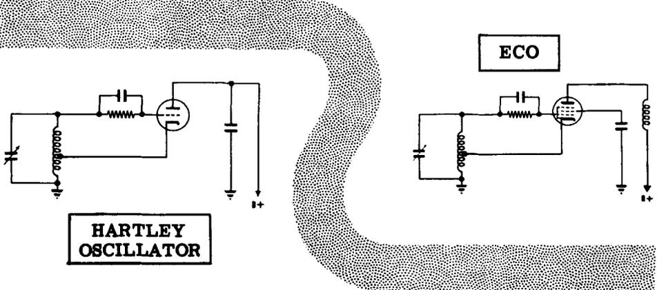
The oscillator section of the electron-coupled oscillator may be a Colpitts circuit instead of a Hartley circuit with equally satisfactory results. The "electron-coupling" effect refers to how energy is delivered from oscillator to plate circuit, not to how the oscillations are generated.
