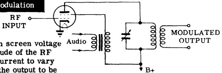
The variations in screen voltage cause the amplitude of the RF pulses of plate current to vary and this causes the output to be modulated by the audio signal.
