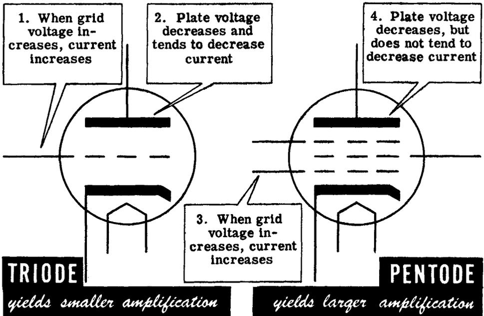
In the pentode the plate voltage can vary considerably with almost no effect on the current and, therefore, with no cancellation of the grid's control of the plate current. As a result, the amplification of a pentode is many times greater than that of a triode.
