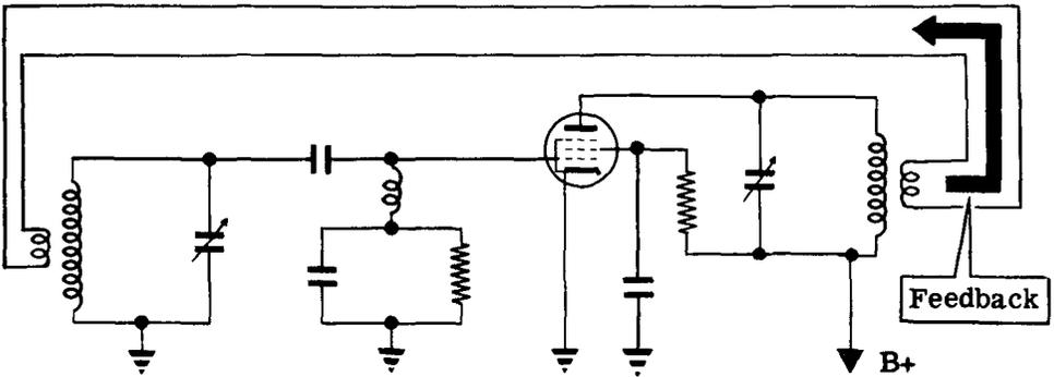
With sufficient coupling, feedback energy will compensate for resistance loss in the grid tank and oscillation will continue.
