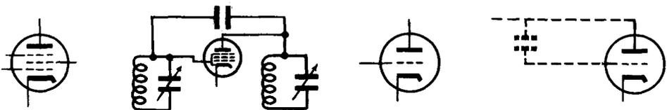
Thus you can see that feedback to sustain oscillation can be accomplished without the use of coil or capacitor. The internal capacitance of tube elements provides the feedback.
