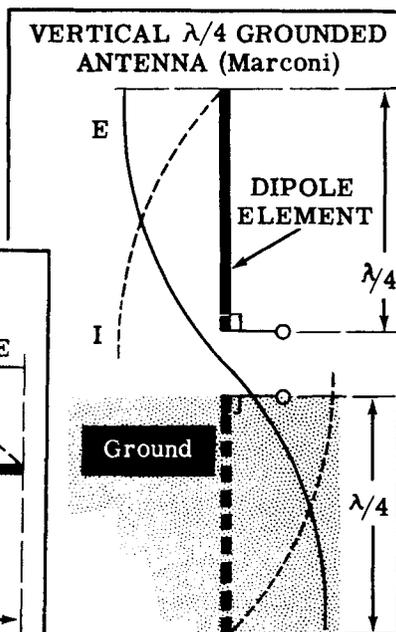
When a Marconi antenna is used, the earth directly beneath the antenna must be a good electrical conductor. Sometimes copper tubing is driven into the ground at the base of the antenna to improve the ground conductivity. On shipboard a vertical quarter-wave antenna may be some distance above the deck. A simulated ground is provided by using grounded metal rods at least a quarter wavelength long and placing them at the base of the antenna. This simulated ground is called a "counterpoise."
