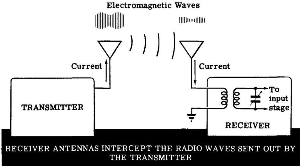
A receiving antenna should feed as much signal and as small an amount of undesired interference to the receiver as possible. It should be constructed so that the signal is not lost or dissipated before reaching the receiver. It should give maximum response for the frequency or band of frequencies to which the receiver is tuned. An antenna can also be directional, which means that it will give best response in the direction from which the operator wishes to receive.
