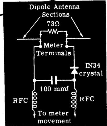
The instructor places the wavemeter far enough away from the transmitting antenna so that the meter needle does not deflect off scale. Then, the transmitter frequency is varied until the meter goes through a peak reading. At this point the transmitting antenna is exactly a half-wavelength long and is therefore radiating at maximum.
