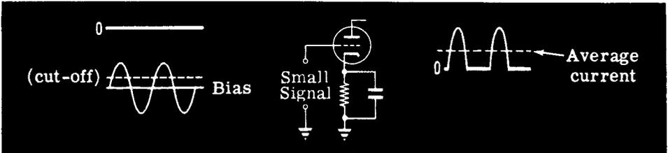
If a larger signal is applied to the grid, the current will be larger during the positive half-cycles of voltage but will remain zero during the negative halves. Thus, the average tube current increases as the grid signal becomes larger, resulting in increased bias for larger signals.
