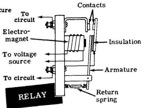
The relay consists of soft iron core, a coil and an armature which will be attracted to the core when the coil is energized, thereby closing the contacts. A spring opens the contacts when the coil is de-energized.
