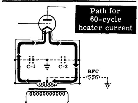
The center tap of the transformer is connected to ground through the RF choke to keep the RF current from flowing in the transformer winding. The RF current gets to the filament through C-1 and C-2.
