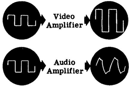
**LOW FREQUENCY RESPONSE** can be improved by increasing capacity of the coupling capacitor and by adding a low frequency compensating network.
