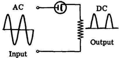
**TRANSFORMER TYPE HALF-WAVE RECTIFIER** — A circuit which uses a transformer to supply high-voltage AC to a vacuum tube rectifier, which then rectifies it to pulsating high-voltage DC.
