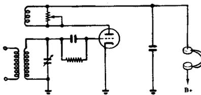
**PLATE DETECTOR**—This detector employs a triode or pentode, biased near cut-off. Rectification takes place in the plate circuit since the negative half of the modulated RF grid signal drives the tube into cut-off.
