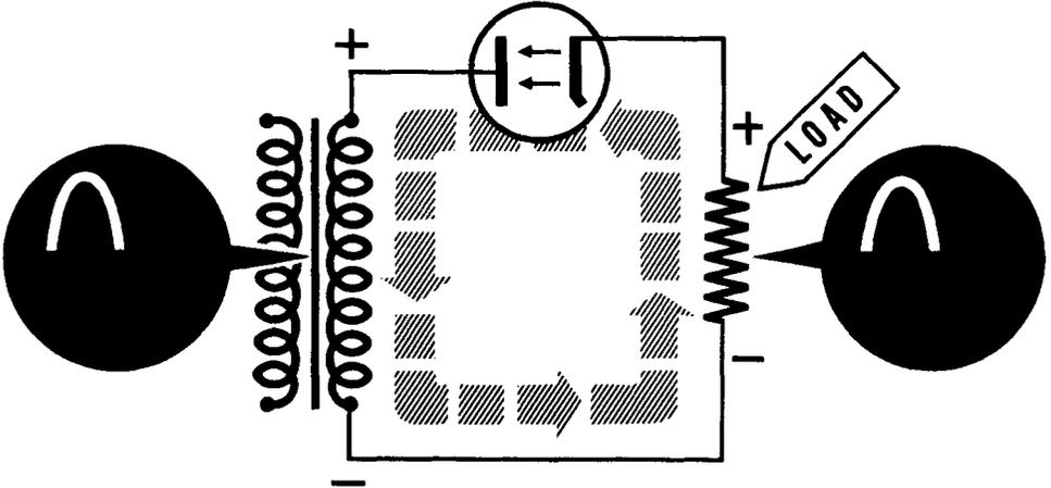
When the transformer voltage makes the rectifier tube plate negative, electrons cannot flow and, of course, no voltage can appear across the load.
