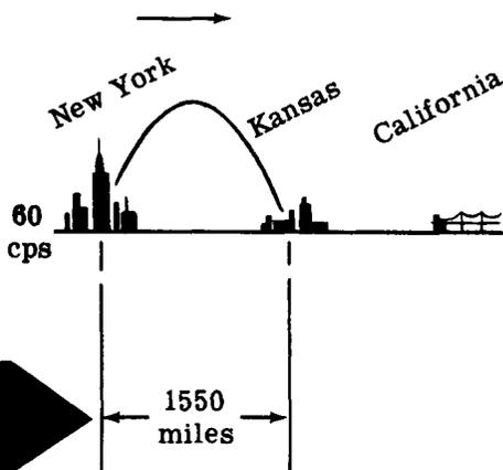
When another half cycle or a total of a full cycle has elapsed ( $\frac{1}{60}$  of a second), the zero voltage point will have traveled a distance of 3100 miles ( $186,000 \times \frac{1}{60}$ ) which is the approximate distance from New York to California. This distance of 3100 miles is the wavelength of the 60 cycle AC, which is the distance that the wave travels during the time interval for one cycle. The symbol for wavelength is the greek letter " $\lambda$ ".
