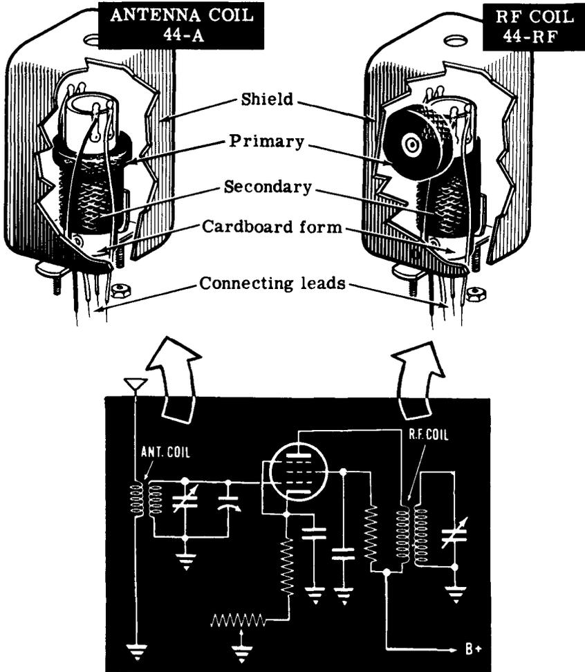
The coils are usually wound on a form made of cardboard or bakelite. They are generally of the air core type, although occasionally, when the frequency of operation is not too high, powdered iron cores may be employed.
