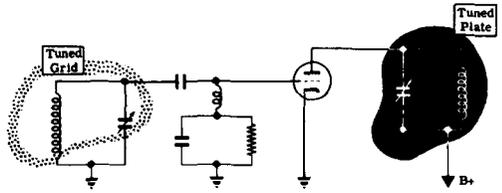
**FEEDBACK**—can be provided by means of link coupling or a capacitor when a pentode is used. The plate-to-grid capacitance provides feedback when a triode is used.
