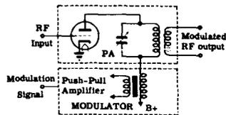
**GRID MODULATION**—The modulating signal is applied to the grid of the PA tube. Varying grid voltage in this manner controls PA tube plate current and hence modulates output voltage.
