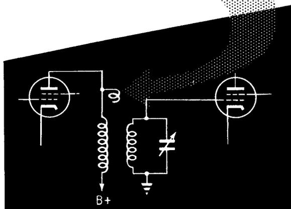
Perhaps you will recall some references, made in "RF Amplifiers," to the "Q" of a resonant circuit. This Q, which is equal numerically to the reactance of the coil divided by its resistance, determines both the selectivity and voltage gain that can be obtained from a resonant circuit. In order to keep the selectivity high, it is therefore necessary to use RF transformers whose resistance is fairly low.
