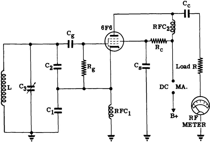
A pentode connected as a tetrode is used in place of the triode of the Colpitts oscillator. The cathode, control grid and screen, along with the tank circuit, act as a conventional Colpitts oscillator. The screen RF bypass capacitor,  $C_g$ , shields this triode from the plate and supplies feedback across  $C_1$ , the AC screen grid load.
