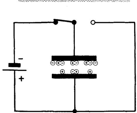
When a short circuit is put across the charged capacitor, the excess electrons are attracted through the shorting wire onto the positive plate. Each plate once more has an equal number of positive and negative charges and the capacitor is uncharged.
