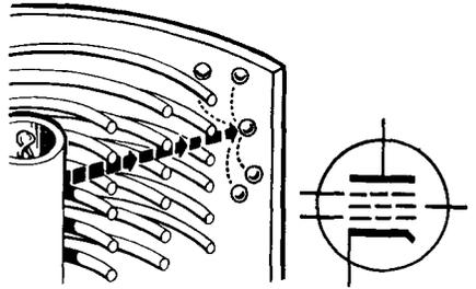
**THE BEAM POWER TUBE** — Tube using beam-forming plates instead of the suppressor to reduce the effects of secondary emission. Its power output is greater, for a given amount of cathode emission, than that of a pentode.
