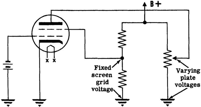
Notice that at high plate voltages above 300V, the plate current does not change when the plate voltage is increased. This is because the screen shields the plate from the space charge at the cathode which causes the screen to exert a greater control over plate current than the plate itself.
