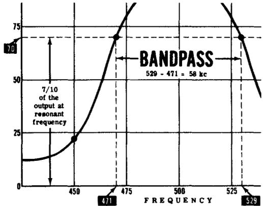
**ALIGNMENT** — The process of adjusting trimmers in a group of tuned amplifier stages so that all the stages tune to the same frequency. When a multiple-stage RF amplifier is correctly aligned, it will give more selectivity than a single-stage amplifier. When it is not correctly aligned, it may give far less selectivity or even tune to two frequencies at once.
