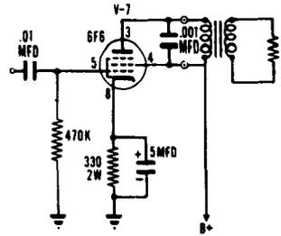
**PHASE INVERTER** — A circuit which uses one or two vacuum tubes to produce two signal voltages 180 degrees out of phase. It is also called a phase splitter and replaces the transformer in a push-pull circuit.
