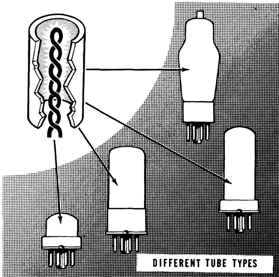
The differences between the diode and the other vacuum tubes lead to their different uses. The diode is used to change an AC voltage into a pulsating DC voltage; the other tubes are used to change a small AC voltage into a large AC voltage
