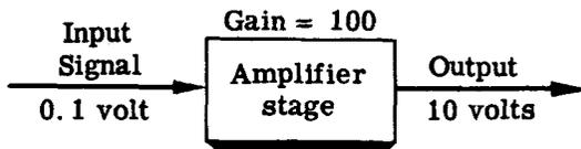
When an amplifier builds up the voltage 10 times, it has a voltage gain of 10. The voltage gain is the number of times a stage or group of stages amplifies the signal.
