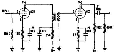
**VOLTAGE GAIN** — The total amplification of a two-stage (or multistage) amplifier is the product of the amplifications of each stage. The ratio of the output voltage of the final stage to the input voltage to the first stage is called the gain of the amplifier.
