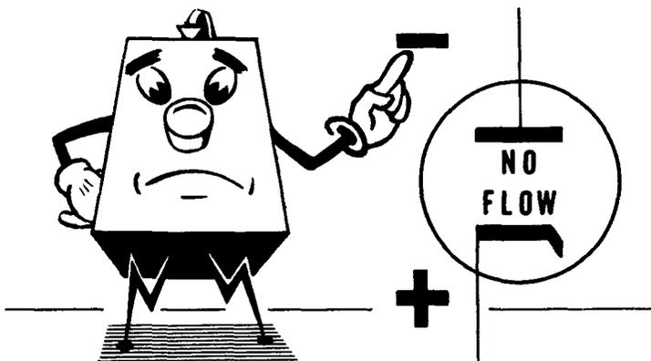
You know from your previous experiment with a diode that when the tube is connected across the 60 cycle power line the diode plate becomes positive 60 times per second and negative 60 times per second. Connecting the diode to the high voltage winding of a transformer keeps the situation exactly the same except that the voltage put on the plate is much higher, and the resulting pulsating DC is at a correspondingly higher voltage.
