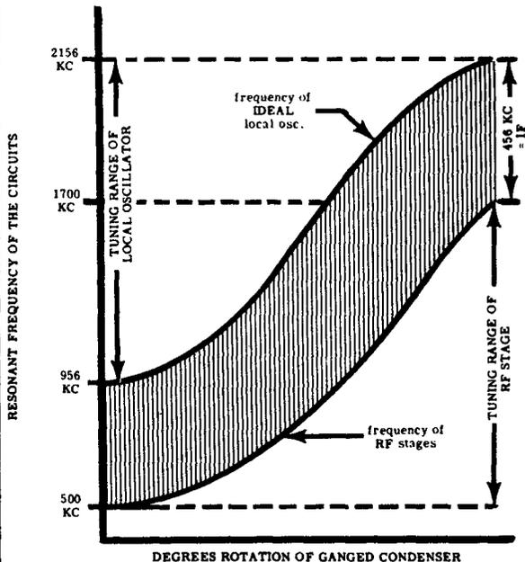
The first step is to adjust the trimmers on the two-ganged variable capacitor. Since these trimmers are in parallel with the tuning capacitors, they affect the total capacitance more at the high frequency end of the band (when the variable capacitor has minimum capacitance) than at the low frequency end. For this reason, the trimmers will be adjusted at 1500 kc, which is close to the high end of the broadcast band.
