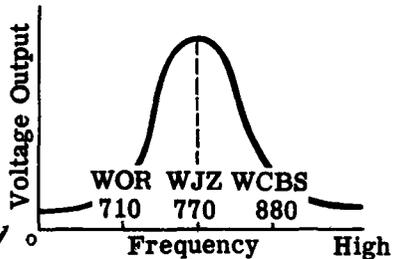
The selectivity of an RF amplifier is determined by its tuned circuits. The lower we can make a coil's resistance in proportion to its reactance, the more selective it will be. The measure of a coil's selectivity is "Q," which is equal to its reactance divided by its resistance. Since the resistance of a capacitor is lower than that of a coil, the coil is the weakest link in a tuned circuit. The Q of the tuned circuit is the Q of the coil.
