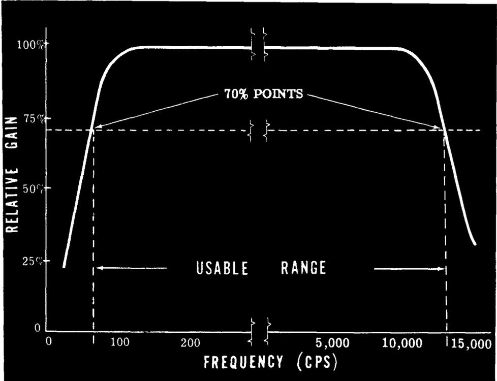
The general shape of the curve shows a flat region (plateau) between the ends of the curve. This means that the gain does not vary by very much as the frequency changes from the low end to the high end of this portion. This represents the usable frequency range of the amplifier.
