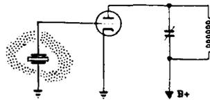
**CRYSTAL OSCILLATOR**—is very similar to the TPTG oscillator, but uses a crystal in place of the grid tank circuit. Power output is low, but frequency stability is excellent where only one frequency is required.
