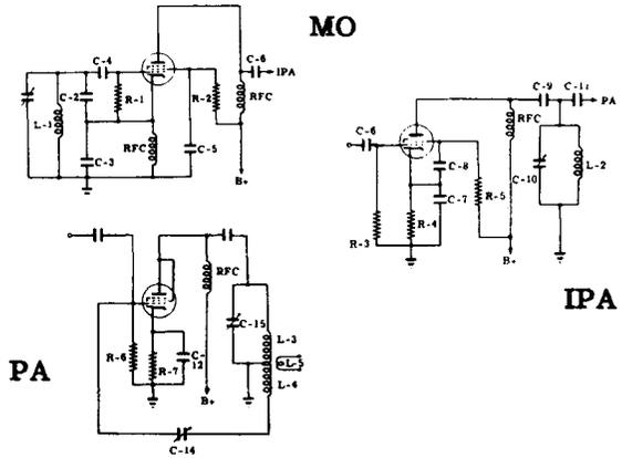
**TUNING**—For efficient operation, the plate tank circuit of the amplifier must resonate at oscillator frequency. Adjusting the variable capacitor to reach this condition is called "tuning."
