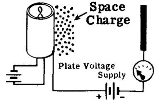
**RECTIFIER TUBE** — A vacuum tube made especially for use as a rectifier.
