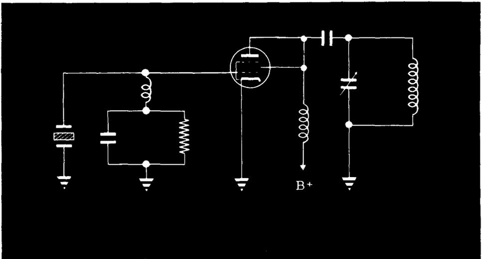
This circuit behaves like the TPTG oscillator in every respect. Feedback is obtained through the plate-grid capacity of the vacuum tube or by using a small feedback capacitor. This voltage feedback causes the crystal to vibrate mechanically at its natural frequency. When the crystal vibrates, an emf appears across the electrodes on the two faces of the crystal. This emf is applied to the grid. The changing emf on the grid controls the flow of plate current and hence the amount of feedback.
