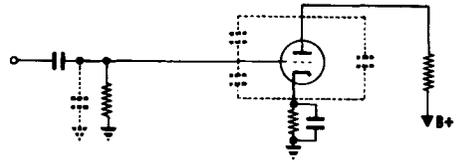
**FREQUENCY RESPONSE** — A measure of the ability of an amplifier to amplify AC signals of various frequencies by the same amount.
