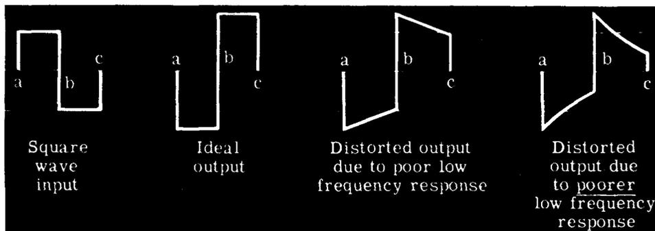
This is what happens in the amplifier. During the flat portion of the square wave between time (a) and time (b) the grid voltage, the plate current and the plate voltage remain constant. At time (b), the grid voltage drops suddenly to a new value and the plate voltage rises just as suddenly to its new value.
