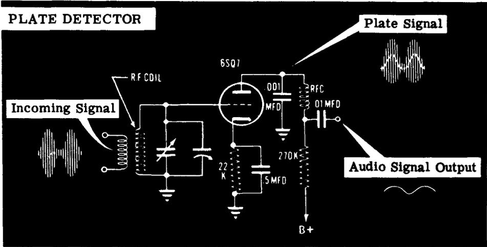
A brief analysis of the functions of the components used in the plate detector should help you to understand how this detector operates.
