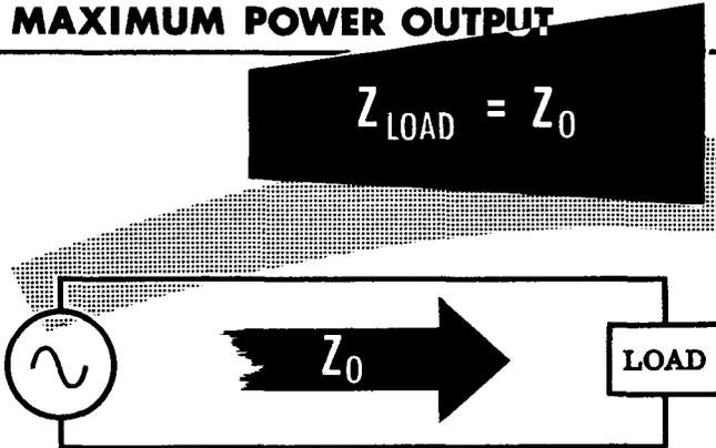
An example of getting maximum power transfer from a transmission line to a load is the case of a line feeding an antenna. If a certain type of antenna, called a "half-wave dipole," is used, the impedance at its center feed point is 73 ohms. Therefore in order to get maximum power transfer from the transmission line to the antenna, the characteristic impedance of the line should be 73 ohms or close to it. When this is the case, the line is said to be "matched" to the antenna.
