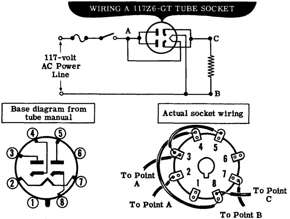
There is a wide variation in the method of representing a vacuum tube in a circuit diagram and tube pins as well as elements are sometimes indicated.
