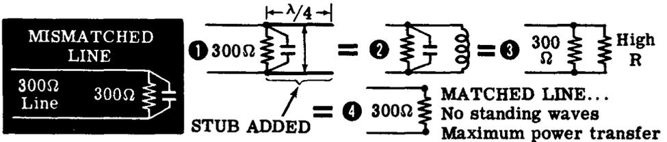
Quarter-wavelength sections are also used as transformers or matching devices to connect circuits of unequal impedances. If a low impedance input circuit is to be connected to a high impedance grid circuit, the input circuit may be tapped down on the coil of a tank circuit as shown. If a tuned line is used, the input circuit can similarly be tapped down on the tuned line. This is an example of a tuned line used as a step-up transformer.
