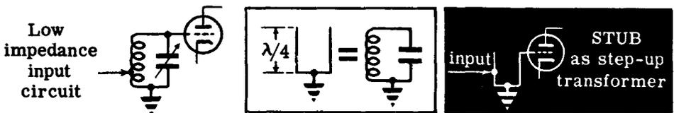
A quarter-wave stub can be used as a step-down transformer to match a high impedance line to a low impedance dipole antenna. The line is connected to the high impedance input of the stub and the antenna is connected near the low impedance shorted end of the stub.
