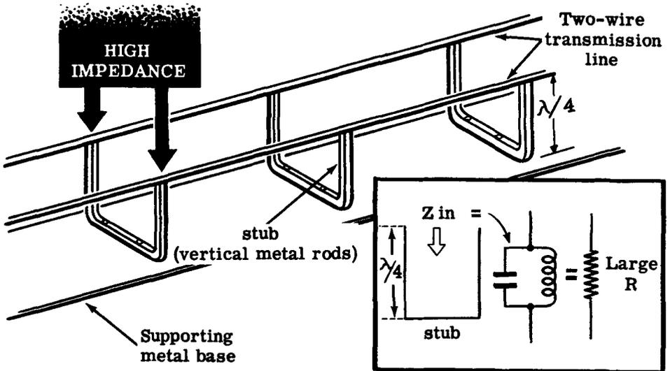
The shorted quarter-wave stub also makes a very effective filter for harmonic frequencies of the fundamental which one does not desire to transmit. For the fundamental frequency the stub is a high impedance as was shown above. For the second harmonic, the stub is now a half wavelength long and will act as a short circuit across the transmission line, shorting out the undesirable harmonic and preventing it from getting to the antenna.
