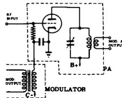
**TRAPEZOID FIGURE**—The oscilloscope pattern obtained by using the transmitter output voltage as 'scope's Y input, and the modulating signal as X input.
