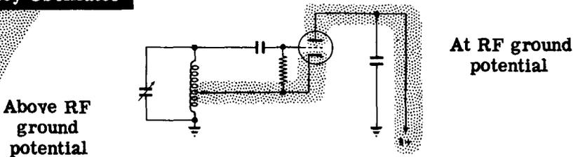
There is a capacitor between the plate of the Hartley oscillator and ground. This capacitor offers a very low impedance path for RF. Since it goes to ground, the plate is considered at RF ground potential, even though it is at a high DC potential.
