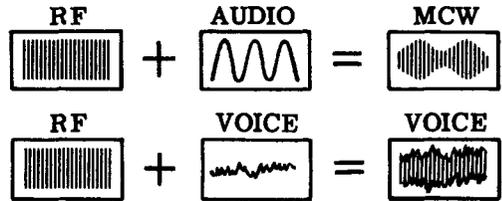
**SIDEBANDS**—Frequencies contained in the transmitted signal in addition to the RF carrier frequency. Sidebands are equal to the sum and difference of carrier and modulating signals. MCW has two sidebands; voice has many.
