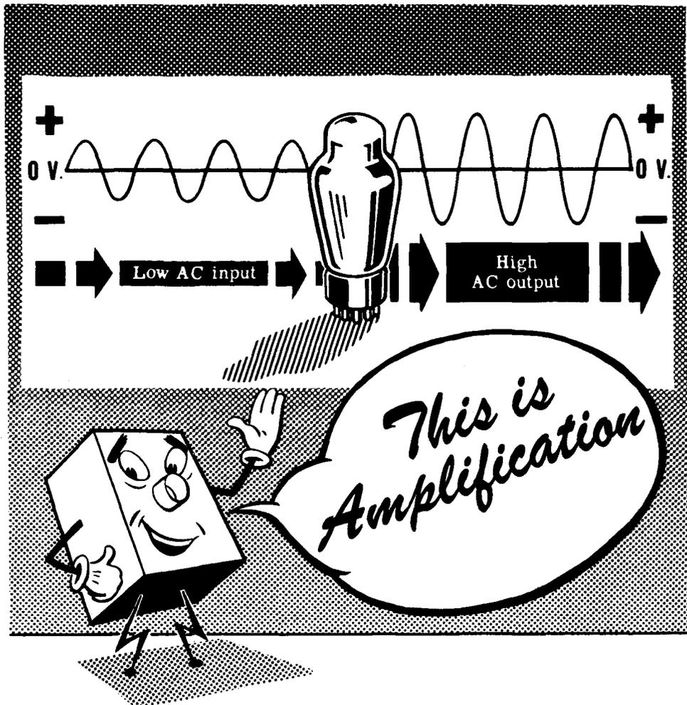
You will find that vacuum tubes are used to produce amplification in receivers, in transmitters, in sonar, in radar and in loran; and it is a foregone conclusion that when new types of electronic equipment come into use, some of the tubes there, too, will be used for amplification.
