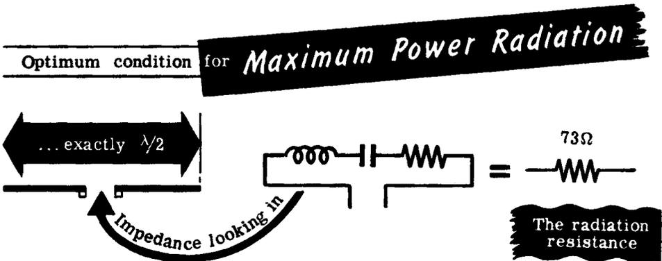
If the frequency of the transmitter goes up, the antenna will be longer than a half wavelength. The series circuit is then operating at a frequency which is above its resonant frequency. At this applied frequency, the inductive reactance is larger than the capacitive reactance and the antenna appears inductive to the transmitter.
