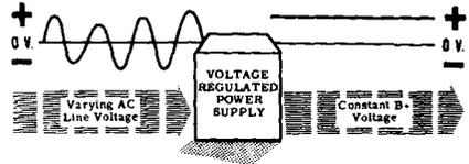
**VOLTAGE REGULATOR TUBE** — The voltage regulator (VR) tube contains a plate and a cathode with no filament—both enclosed in a glass envelope containing a gas at low pressure. When a large enough voltage is applied across the tube, a current is conducted through the tube. As long as the current flowing through the tube remains within the limits listed by the manufacturer, the voltage at the plate will remain essentially constant.
