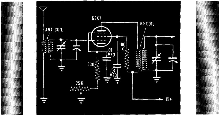
Since signals arriving from different transmitters will vary in intensity, it is necessary to provide a volume control so that the gain of the RF amplifier and the loudness of the signal can be varied. One of the most common methods of controlling the gain of a TRF is to change the bias voltage of the RF amplifier stage by placing a variable resistor in the cathode circuit.
