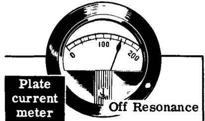
As the tuning control is rotated, no change in the milliammeter reading will be noticed until the tuned circuit frequency is near the oscillator frequency. When the current starts to "dip," the control should be rotated slowly.
