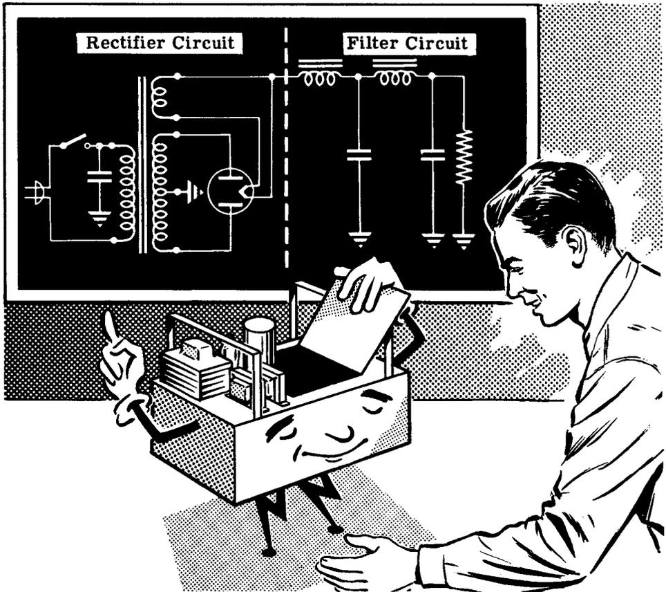
You already know that there are only two types of rectifier circuits in general use—the full-wave and the half-wave rectifiers—and they both perform the same job of changing AC into pulsating DC. There are only three types of filter circuits that are in general use. These filter circuits all have one thing in common—they remove the ripple from the pulsating DC output of the rectifier.
