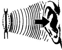
**MICROPHONES** change sound waves into electrical impulses. "Mikes" may be carbon, crystal, dynamic or ribbon type. The electrical impulses are fed into the grid of an amplifier either directly or through a step-up transformer.
