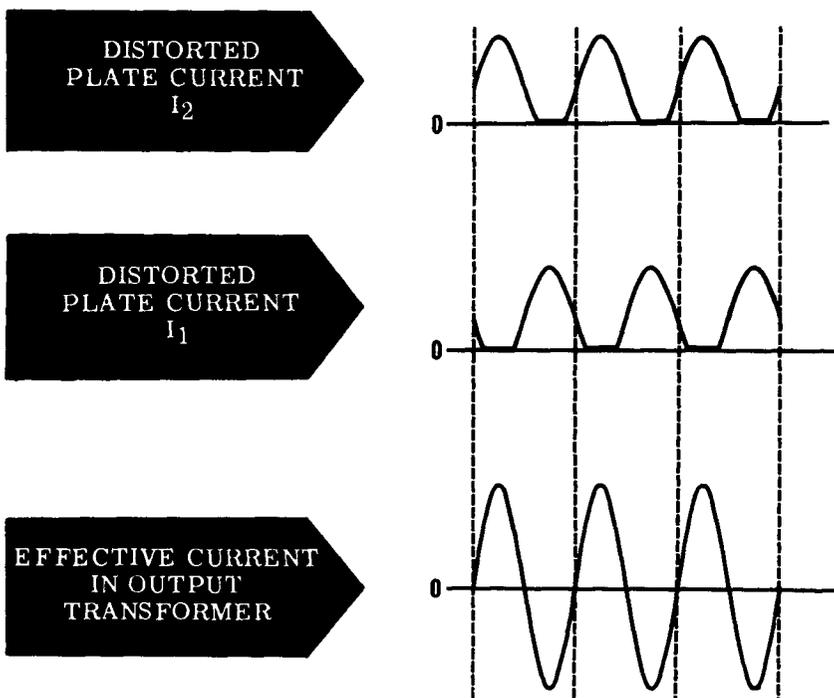
The reason that it is such a big advantage that the push-pull circuit reduces distortion is this—the tubes can be intentionally overdriven to produce a larger output and the output still will be practically undistorted.
