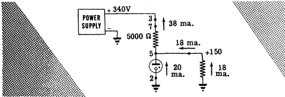
Under the operating conditions shown, 38 ma. flow through the dropping resistor, 20 ma. flow through the VR tube, and 18 ma. flow through the load. If the B+ voltage were to rise to +360 volts, the VR tube would have to adjust its internal resistance so that its plate voltage remained at 150 volts. Let's see if the VR tube is able to make this adjustment.
