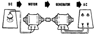
**DYNAMOTOR** — A rotating DC machine that operates from a low voltage DC source and puts out one or more high DC voltages. A dynamotor is basically a DC motor and a DC generator built onto one armature and having two or more commutators.
