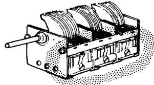
**RESONANT CIRCUIT**—A circuit in which a capacitor and a coil are connected in series or in parallel. Its function is to tune.
