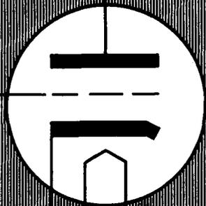
As in the diode, saturation in a triode occurs because there is a limit to the amount of current which the cathode can emit. In the triode, saturation (limiting current) can be reached at a lower value of plate voltage if a positive voltage is applied to the grid; in the diode, of course, it depends only on the plate voltage.
