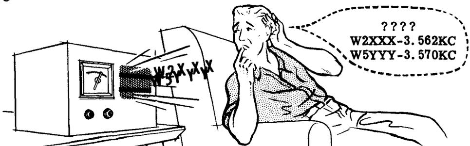
MORE RF STAGES ARE NEEDED WHERE SIGNAL FREQUENCIES ARE CLOSE TOGETHER
