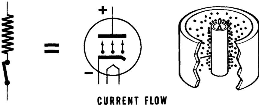
When the plate becomes the least bit negative with respect to the cathode, no electrons will flow from the cathode to the plate. The tube acts as if it were a resistor in series with a switch and the switch were opened up.
