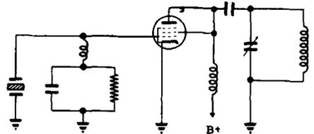
**POWER OUTPUT**—of the crystal oscillator is maximum when the plate tank is tuned to the natural mechanical frequency of vibration of the crystal. The oscillator is usually operated at less than maximum power output to achieve stability of operation.
