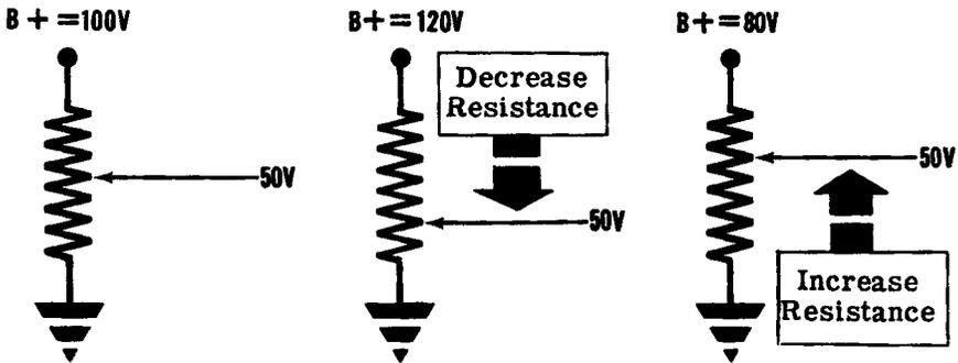
You can see that the hand-operated voltage regulator works very well. You increase or decrease the resistance between ground and the output voltage tap to increase or decrease the output voltage back to the desired value whenever the B+ supply voltage falls or rises for any reason.
