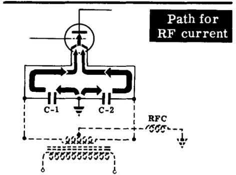
The DC tube current flows through the RF choke, divides in going through the filament transformer winding and arrives at the filament. Because the DC current divides, both ends of the filament are at the same DC potential. If one side were less positive than the other, more plate current would be drawn from that side. Since the two sides of the filament are at the same potential, equal currents are drawn from each, resulting in longer life for the tube.
