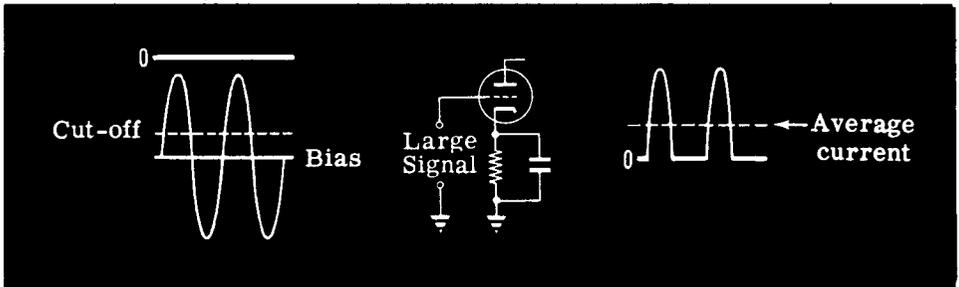
This effect of bias varying with signal strength tends to stabilize the amplitude of that portion of the grid signal above the cut-off level. As a result the amplitude of the current pulses in the plate will not vary as much as their corresponding grid signals vary. Because of the above mentioned effect, self-bias tends to produce amplitude stability of the plate signal and, therefore, is sometimes called "automatic bias." Cathode bias is not common in high-powered transmitter circuits.
