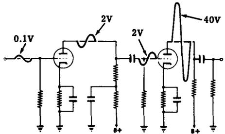
**AMPLIFICATION LOSSES** — At low frequencies the high reactance of the coupling capacitor reduces voltage gain; at high frequencies stray capacitance causes loss of voltage gain.
