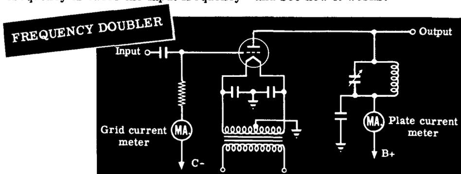
The circuit of a frequency doubler appears to be the same as that of an amplifier which operates at the input frequency. The only differences are that the plate circuit will be tuned to twice the input frequency and no neutralization is required since the input and output operate at different frequencies. This reduces the possibility of self-excited oscillations.
