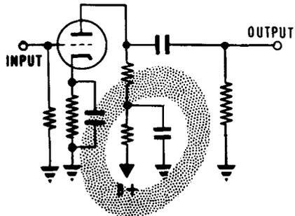
**HIGH FREQUENCY RESPONSE** can be improved by reducing the value of the plate load resistor and by adding a peaking coil in the plate lead.
