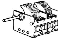
**TRIMMERS**—Are small capacitors placed in parallel with each unit of a ganged capacitor. Their function is to compensate for small differences in capacity between the units.
