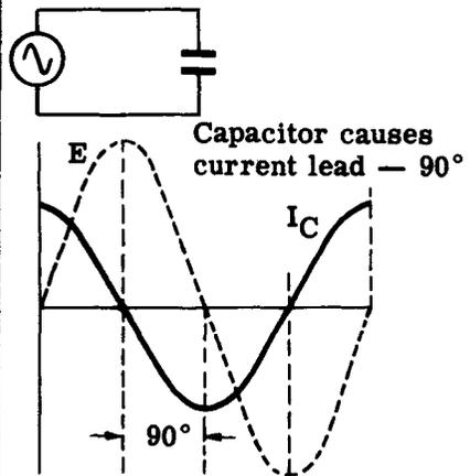
If you connect a coil in parallel with a capacitor, the current in the coil is 90 degrees behind the applied voltage plus 90 degrees behind the current in the capacitor, or, a total of 180 degrees out of phase with the capacitor current. You remember from Basic Electricity that currents which are 180 degrees out of phase cancel one another. If the capacitor alone draws 3 amps and the coil alone draws 2 amps, then the combination of the two will draw 3 - 2 or 1 amp.
