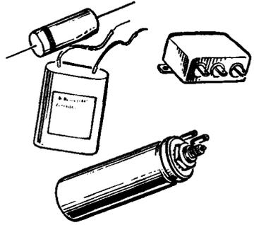
**PAPER FILTER CAPACITORS** — Paper filter condensers are bulky and their value is usually limited to less than 10 mfd. They are not polarized and can be made to withstand very high voltages. There is no appreciable leakage across a paper filter condenser. Oil-impregnated paper condensers are used in high voltage filter circuits.
