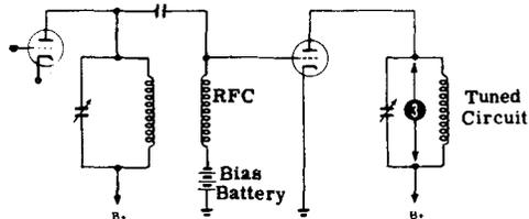
**GRID-LEAK BIAS**—Depends on grid current and varies as the strength of input signal changes.
