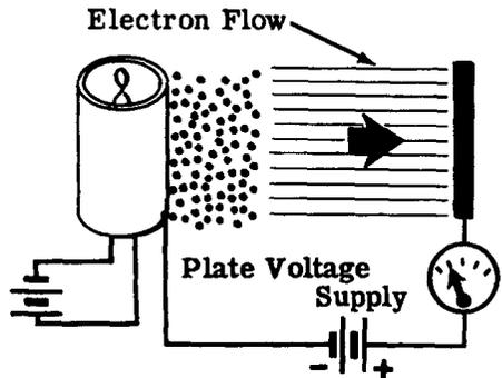
If this plate voltage is doubled, the current which flows is also doubled. This is the normal way for a diode to work: as long as the plate is positive with respect to the cathode, every change in plate voltage causes a corresponding change in plate current.
