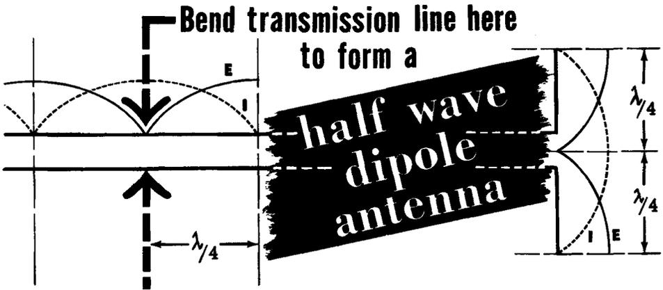
Although the voltages at any two points on the antenna wires (also on the transmission line), equidistant from the ends, are equal in amplitude, they are opposite in polarity just as the ends of a transformer winding are equal in amplitude but opposite in polarity. The same holds true for current. Therefore, to indicate polarity as well as amplitude on the wires that comprise the transmission line and antenna, the wave forms are redrawn as shown.
