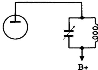
**SHUNT FEED**—A circuit arrangement in which the plate current of the tube flows through an RF choke and only RF voltage gets to the tank. This avoids the possibility of DC shock, but the RF choke cannot operate efficiently over a wide band of frequencies.
