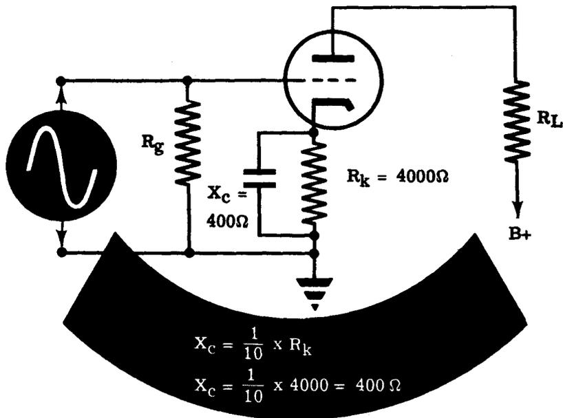
Since  $X_c = \frac{1}{2\pi fC}$ , the capacity of the bypass condenser can be found by using the formula  $C = \frac{1}{2\pi fX_c}$ , where  $f$  is the lowest frequency signal to be amplified. Suppose  $f$  is 60 cps and  $X_c$  is 400Ω as shown above, then  $C$
