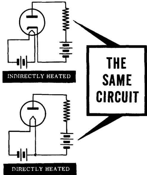
There are two different ways of using a rectifier tube which has two plates and one filament. If both plates are connected together, the tube is acting the same as one diode because, in effect, you have only increased the plate area.
