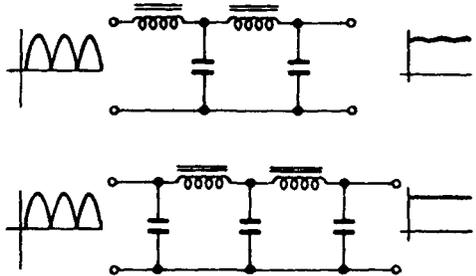
**COMPLETE POWER SUPPLY** — The complete circuit consisting of full-wave rectifier and filter circuits, used to supply high DC voltage to other circuits.
