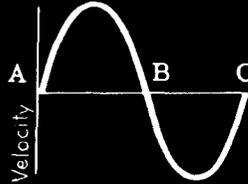
Did you ever notice that one complete trip on the swing takes the same time as any other trip? You can represent three cycles of the swing like this: the time from  $t_1$  to  $t_3$  is the same as that from  $t_3$  to  $t_5$  or that from  $t_5$  to  $t_7$ , as shown below. Also the time required for the various half cycles ( $t_1$  to  $t_2$ ,  $t_2$  to  $t_3$ , etc.) is always the same.
