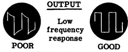
**LOW FREQUENCY COMPENSATING NETWORK** develops a varying voltage, which, when added to the square wave input voltage, counteracts the distortion of flat portion of square wave due to the coupling capacitor.
