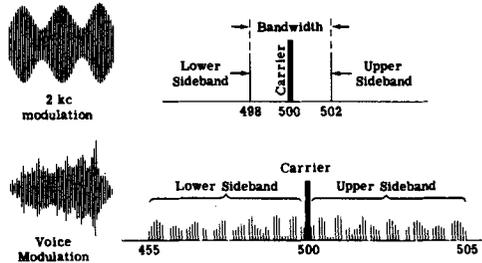
**PLATE MODULATION**—The method whereby the modulating signal varies the PA tube voltage, thus modulating its output in response to the audio signal.
