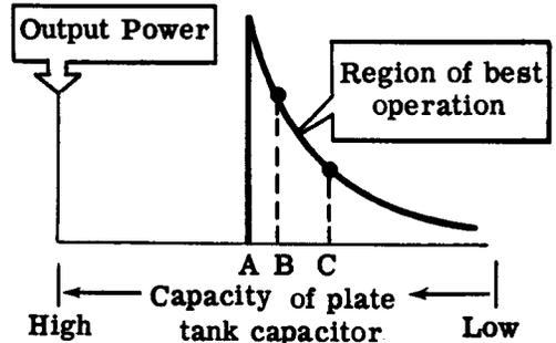
Since a crystal has low frictional losses, it doesn't require much feedback to sustain oscillations. Besides, a large amount of voltage across the crystal plates can make the crystal vibrate so hard as to overheat or shatter—much as a powerful explosion causes window panes to vibrate so strongly as to shatter. Overheating causes frequency drift. Thus, smaller feedback results in a greater safety factor and in less frequency drift.
