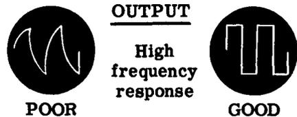
**PEAKING COIL** counteracts the effect of stray capacitance, which tends to round off the leading edge of the square wave.
