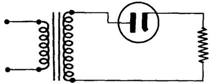
**FULL-WAVE RECTIFIER CIRCUIT** — A circuit which uses a transformer and a full-wave rectifier diode to produce full-wave rectified pulsating DC from an AC input.
