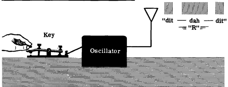
A signal of this type contains intelligence since a message can be obtained from it. The radio would produce a sound somewhat like "dit-dah-dit" which a radio operator understands as the letter "R."
