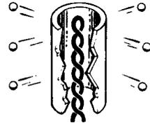
**SPACE CHARGE** — The negative charge in the area surrounding the cathode caused by the emission of electrons from the cathode.
