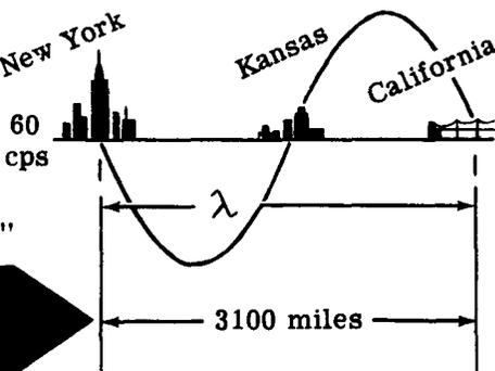
Similarly the wavelength of any frequency radiation can be determined by multiplying the constant velocity by the time for one cycle. Since the time for one cycle is equal to 1 divided by the frequency ( $\frac{1}{f}$ ), the wavelength equals constant velocity over frequency ( $\lambda = \frac{V}{f}$ ) or the velocity equals the frequency times the wavelength ( $V = f\lambda$ ). Since  $V$  is constant, the higher the frequency, the lower the wavelength and vice versa.
