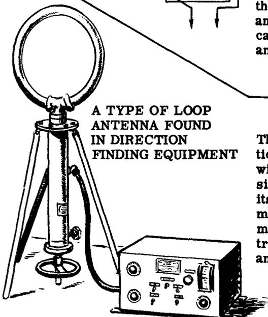
The loop antenna is highly directional. When it is pointed edge-wise toward a transmitter, the signal pickup is maximum; when its flat side is toward the transmitter, the signal pickup is minimum. This property makes it extremely useful for radio-beacon and direction-finding equipment.
