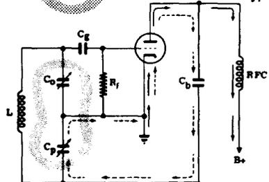
**TPTG OSCILLATOR**—uses the grid-plate capacitance of a triode to feed back pulses to a tuned circuit connected to the grid. It oscillates only when the two tuned circuits are set to or near the same frequency.
