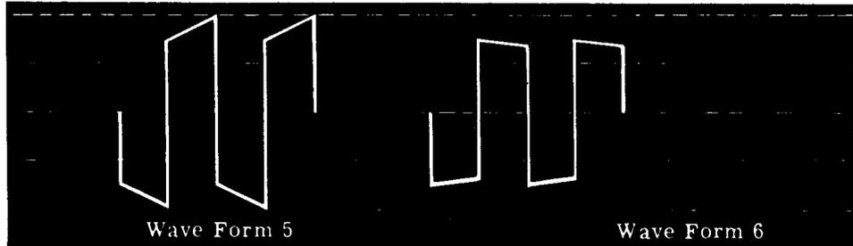
You will notice that the new input wave form (no. 4) is smaller than wave form 1, the old input. This is so because the voltage that was fed back is out of phase with, and so subtracts from, the original signal input. Thus the output is smaller than it would ordinarily be and the gain of the stage is apparently lessened. More important than the loss of gain is the decrease in the amount of distortion. This method of decreasing distortion is known as "degeneration" or as "negative feedback."
