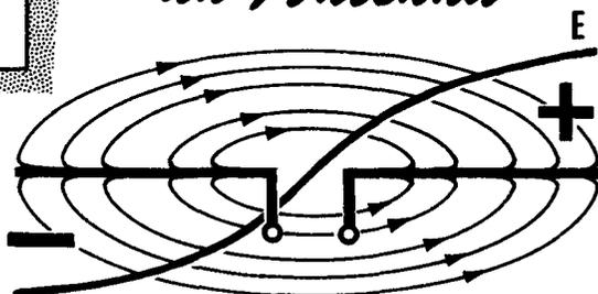
Besides this electric field, there is also a magnetic field which is generated by the antenna current. The plane of this magnetic field is at right angles to the direction of the current flow and therefore is at right angles to the antenna, as shown. The electric and magnetic fields must therefore be at right angles to each other.
