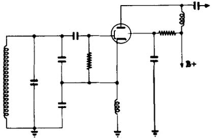
**SERIES FEED**—a circuit arrangement in which the plate current of the tube flows through the tank circuit. In cases where the plate of the tube goes directly to the tank, the entire B+ voltage is present at the tank. This presents the danger of shocks.
