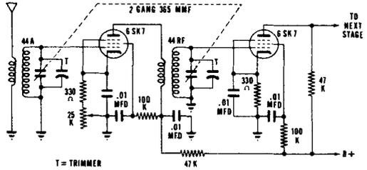
**BANDPASS** — The width of the band passed by an amplifier between the two points where the output is seven-tenths of the output at the resonant frequency. The greater the selectivity, the narrower the bandpass. The greater the bandpass, the poorer the selectivity.
