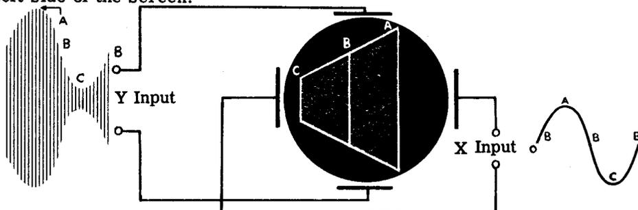
Because of the way in which trapezoid figures are obtained, they represent a graph of the output voltage as compared to the modulating voltage. If the output voltage is always proportional to the modulating voltage—as it will be when the modulation is linear—there will be a straight line along the top and on the bottom of the trapezoid.
