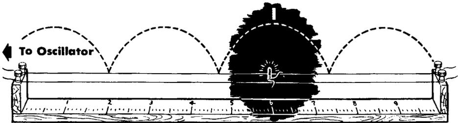
The voltage peaks can be found by using a neon bulb. The instructor holds the glass end of the bulb with his fingers and moves it along one wire, keeping a wire from the current bulb in contact with the line at all times. The bulb remains out at the current peaks previously noted, but lights up between the current peaks, reaching maximum brilliance equidistant between two current peaks. The point of maximum brilliance is a voltage peak.
