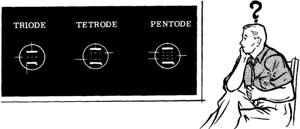
There are three types of tubes which might be used—the triode, the tetrode and the pentode. At first glance it might seem that the triode is the best tube to use since it is the simplest of the three. However, the triode has two great disadvantages when used as an RF amplifier—no triode has an amplification factor of over 100. Tetrodes and pentodes have much higher amplification factors and therefore are capable of amplifying many more times.
