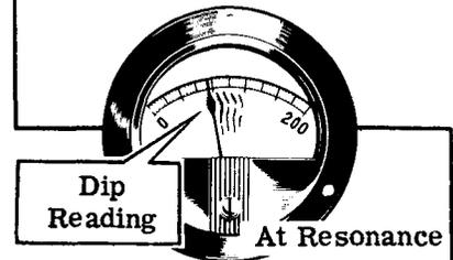
Continuing to rotate the control in the same direction will detune the circuit and the current will rise again.
