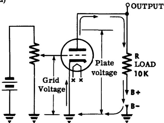
Now a slight change in grid voltage causes a large change in plate current and this causes a corresponding change in the voltage drop across the load resistor. If the voltage drop across the load resistor increases, the plate voltage will decrease by the same amount. This change in plate voltage is called the "output voltage." Because a change in grid voltage produces a much larger change in plate voltage, the triode amplifies.
