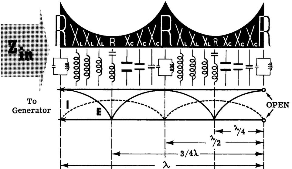
The following diagrams illustrate different lengths of open and shorted lines and the input impedance they present to a generator.
