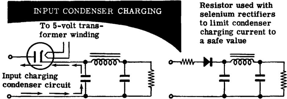
Because of the time lapse between pulses of direct current, the output of a half-wave rectifier requires more filtering than that of a full-wave rectifier and the filtered output voltage will be lower. Filter capacitors used in half-wave power supplies are usually from 2 to 4 times as large as those used in full-wave power supplies. Increasing the size of the filter capacitors provides additional filtering.
