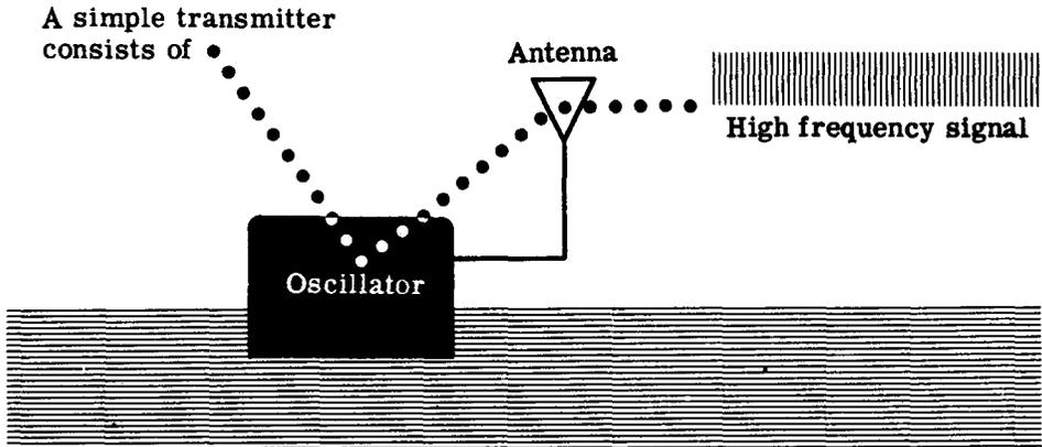
If your home radio set picked up the constant-amplitude signal from such a transmitter, you would hear nothing at all. If a special type of radio received this signal, a constant audio tone would be heard. In either of these cases, no message could be "read" from the incoming signal—such a signal is said to contain "no intelligence." To add intelligence to the signal, the oscillator would be turned on and off with a key to produce dots and dashes.
