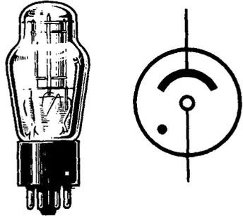
**VR TUBE CIRCUIT** -- The simplest (and very widely used) voltage regulator circuit consists of a voltage dropping resistor and a VR tube placed in series across the power supply output and ground. The regulated voltage is taken from the plate of the VR tube. The load current and the VR tube current both flow through the dropping resistor, and the VR tube current changes along with the load current so as to keep the dropping resistor current constant.
