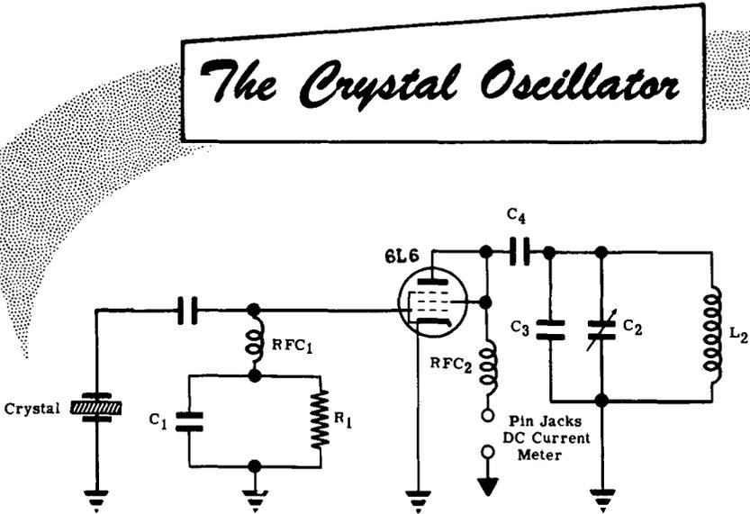
$C_3$  in parallel with  $C_2$  adds to its capacity and reduces the resonant frequency. This is required if the range of  $C_2L_2$  alone does not extend down to the crystal frequency.
