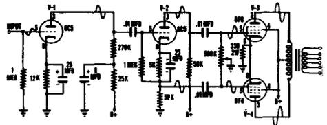
**THE OUTPUT TRANSFORMER** — A transformer used to couple the power amplifier output to the load. It matches the low load impedance to the high impedance required by the amplifier.
