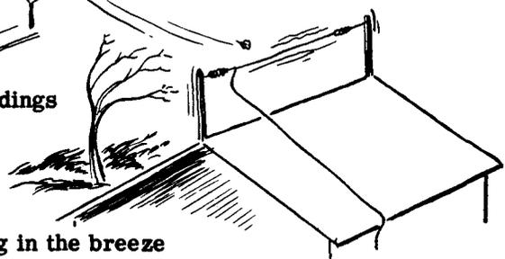
Signal losses will also be increased if a high resistance is present in the antenna circuit. To reduce resistance, all joints and connections should be carefully soldered and, wherever possible, the antenna and lead-in should consist of a single piece of wire with no joints.
