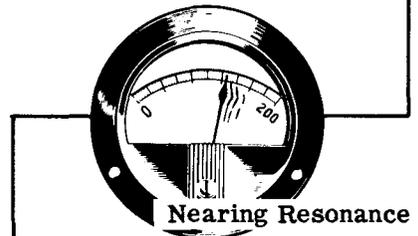
The current will continue to decrease as the tuning control is rotated until a minimum value occurs. This is the dip reading.
