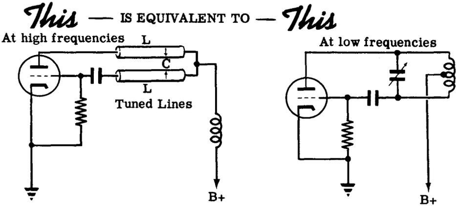
The characteristics of these tuned lines are calculated in the same way as characteristics of transmission lines, which you will find out about in "Transmitters." Inductance and capacitance of ordinary coils and capacitors is said to be "lumped." Inductance and capacitance of tuned lines is said to be "distributed." Here are some other high frequency oscillator circuits using distributed reactance (capacity and inductance).
