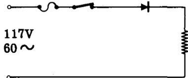
**RECTIFIER CIRCUIT WAVEFORMS** — If the applied voltage is an AC sine wave, the output waveform consists of half cycles of the applied AC voltage. This output waveform is a pulsating DC voltage.
