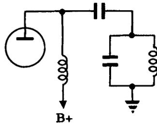
**GROUNDING POINTS**—Most oscillator circuits can be made to work with the plate, cathode or grid at RF ground potential.
