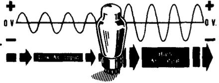
**THE TRIODE** — A vacuum tube similar to a diode but containing a grid which controls plate current between cathode and plate.
