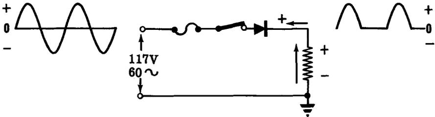
To reverse the polarity of the DC voltage obtained, the rectifier is reversed. This allows current to flow only on the opposite half cycles as compared to the previous circuit. This circuit is used to obtain a negative DC voltage with respect to ground. The grounded end of the load resistor is positive.
