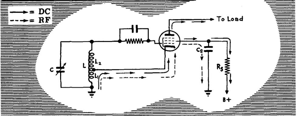
From the diagram it can be seen that both DC and RF paths are identical with DC and RF paths in the Hartley oscillator.
