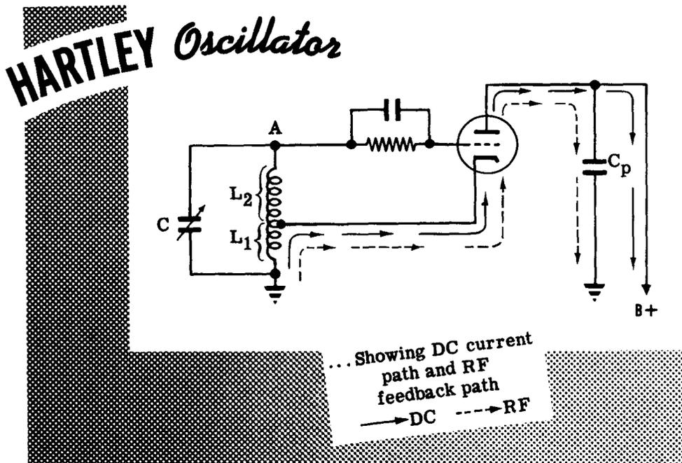
Once oscillation has begun, the cycle is very much the same as in the Armstrong oscillator. The tube is biased below cut-off from shortly after the top plate of the LC circuit, point A, has reached its peak positive value until shortly before it reaches its peak positive value again. During all this time the tube serves no purpose whatsoever, and the surge of electrons through the tank circuit goes on solely because of the flywheel effect of that LC circuit.
