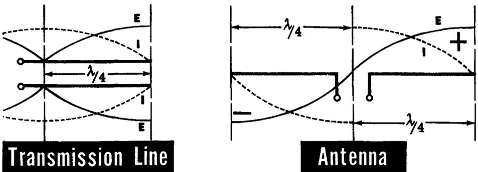
Observe that the standing waves of voltage and current indicate that the antenna ends are points of maximum voltage and minimum current, whereas the center of the antenna is a point of maximum current and minimum voltage.
