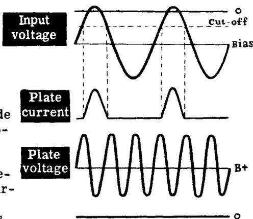
Pulses of current flow from cathode to plate—one pulse per cycle of applied signal. These pulses arrive at the tuned circuit during every third cycle of output voltage and deliver enough energy to the tuned circuit to sustain oscillations during those cycles when no current flows.
