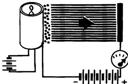
If we had reduced the filament voltage, the current would have decreased because the cathode could not emit as many electrons as before. In practice, the filament voltage is not varied. Changes in plate current are achieved by varying the plate voltage as already described. However, after a tube has been used for some time, the cathode's emission decreases and the result is the same as if the filament voltage were decreased.
