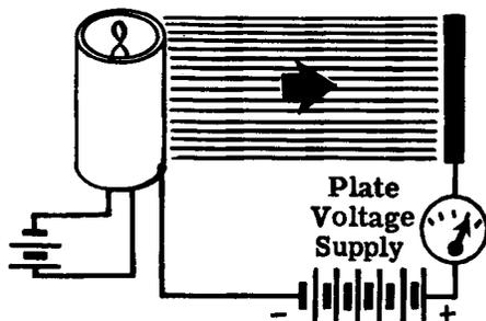
At this point, a further increase in plate voltage does not result in any additional current. The current does not increase because the cathode is emitting all the electrons it can. It is NOT normal to operate a diode at such a high plate voltage that changes in plate voltage do not produce changes in plate current.
