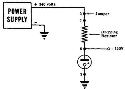
**VR TUBE JUMPER** — The purpose of the jumper in a VR tube is to prevent unregulated voltage from reaching a special electronic circuit if the VR tube is pulled out. Without the jumper, unregulated voltage would reach the circuit, causing improper operation and possible damage. Pulling out the VR tube removes the jumper and disconnects the voltage from the special circuit.
