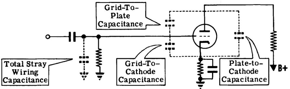
The effect of this total capacitance is to shunt the grid leak resistor. At low and medium frequencies the reactance of this small capacitance is high and therefore it does not disturb the operation of the circuit. At high frequencies, the reactance drops and effectively decreases the impedance between grid and ground. The signal appearing between grid and ground decreases as the impedance between grid and ground decreases.
