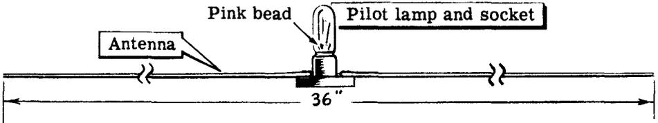
First, the transmitter is retuned until the bulb is brightest. Then, the intensity of the radiation around the antenna is demonstrated by moving the dipole, parallel to the antenna, from the center out to either end. Observe that the bulb is brightest when the center of the wavemeter dipole is lined up with the center of the antenna, and the bulb goes out when the center of the wavemeter dipole is in line with the end of the transmitting antenna.
