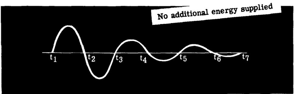
This is called a "damped" wave. It is like a sine wave, but with the height (amplitude) of successive cycles diminishing gradually. The time interval remains the same.
