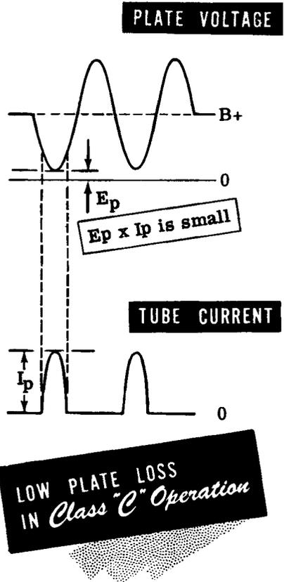
If the tuned circuit in the plate is not tuned to the frequency of the input signal, then the voltage across it will be lower—in proportion to how much it is mistuned. The further off it is tuned, the less power will appear across it and the more power will be dissipated by the tube itself. Then the efficiency of the amplifier is lower, the tube heats up more, and the power output is lower.
