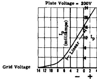
**GRID BIAS** — The amount of grid bias voltage determines the class of amplifier operation. In Class A the bias is less than cut off; in Class B bias is at or near cut-off; in Class C bias is much less than cut-off.
