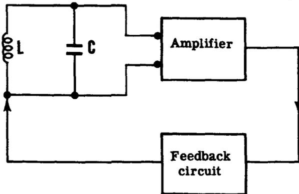
All the oscillators you will learn about in this section operate on the principle illustrated above. The major difference between various oscillators is the method in which a voltage is fed back to the LC circuit in proper phase. You will learn about six basic oscillators: the Armstrong, the Colpitts, the Hartley, the tuned-plate—tuned-grid, the crystal controlled and the electron-coupled oscillators. You will see how these oscillators work, and the advantages and disadvantages of each type.
