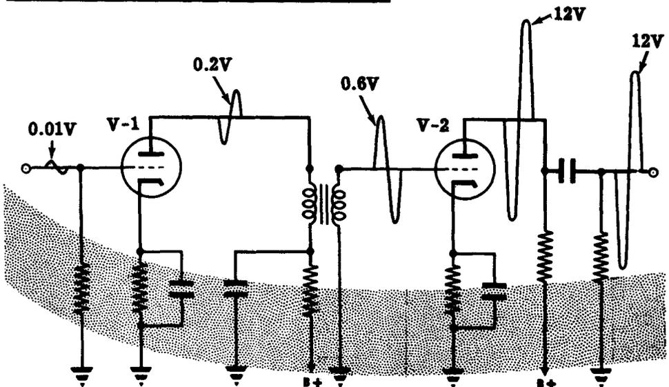
The voltage across the secondary of the transformer (0.6V) is now applied to the grid of V-2. If we assume that the gain of V-2 is equal to  $\mu$ , then V-2 will amplify this signal 20 times. Therefore, the output voltage at the plate of V-2 will be  $-20 \times 0.6 = 12V$ .
