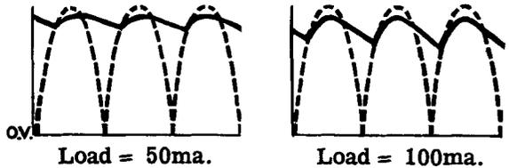
The smaller the capacity of the condenser the greater the ripple
