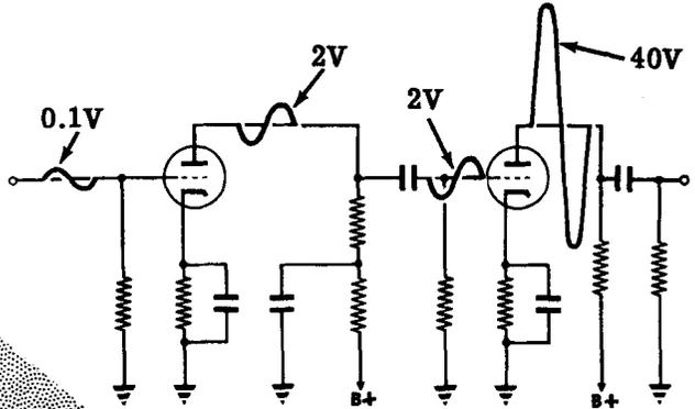
Suppose each amplifier stage can deliver an amplification of 20. If a 0.1 volt AC signal is applied to the grid of the first stage, the output of this stage will be  $20 \times 0.1 = 2\text{V}$ . Since the output of the first stage is connected to the input of the next stage there will be 2 volts AC on the grid of the second stage. The second stage amplifies the signal 20 times and produces an output voltage of  $20 \times 2 = 40\text{V}$ .
