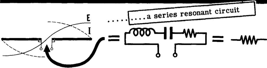
The radiation resistance is not an actual resistance. It is an equivalent resistance which, if connected in place of the antenna, would dissipate the same amount of power as the antenna radiates into space.
