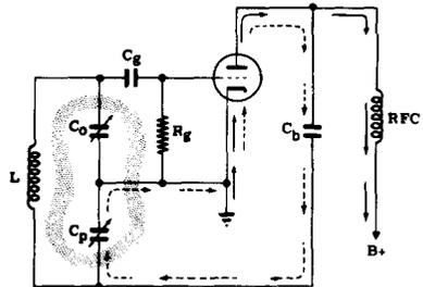
**GRID LEAK BIAS**—a method of bias in which excess electrons accumulate on the grid, producing a negative bias. They are allowed to leak off slowly through a large resistor which is placed in parallel with the grid capacitor or from grid to cathode. Making the resistor large enough produces more than cut-off bias and results in Class C operation.
