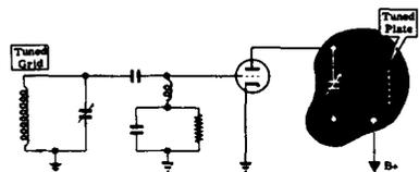
**CRYSTAL OSCILLATOR**—is like a TPTG oscillator, but a crystal is connected in place of the grid tank circuit. It can only oscillate at, or very close to, the frequency of the crystal. It has more frequency stability than any other oscillator.
