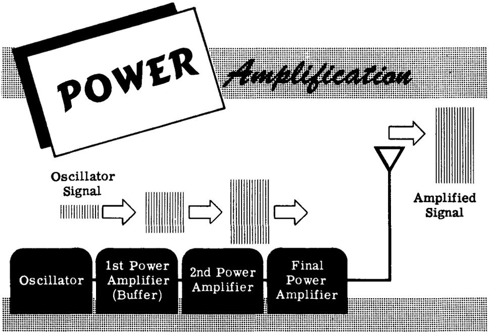
The RF signal is generated in the oscillator circuit and is amplified by the first and second power amplifiers which drive the final power amplifier. The powerful signal from the final power amplifier is fed to the antenna which radiates the signal into space.
