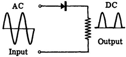
**RECTIFIER TUBE** — A vacuum tube diode consisting of plate and cathode which allow electron flow only from cathode to plate and thus acts as a rectifier.
