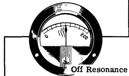
When the current is observed to be rising, the control should be turned in the opposite direction until it is set for minimum current. At this point, the tuned circuit is at the same frequency as the signal frequency and the output of the stage is maximum.
