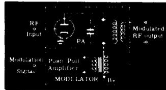
**GRID MODULATION**—The modulating signal is applied to the grid of the PA tube. Varying grid voltage in this manner controls PA tube plate current and hence modulates output voltage.
