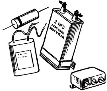
**ELECTROLYTIC FILTER CAPACITORS** — Electrolytics have a high value of capacitance as compared to a paper condenser of the same physical size. They are polarized and are normally constructed to operate at less than 600 volts. There is appreciable leakage across an electrolytic condenser but this effect is usually offset by their large values of capacitance. Electrolytics range in value from 1 to 1000 mfd.
