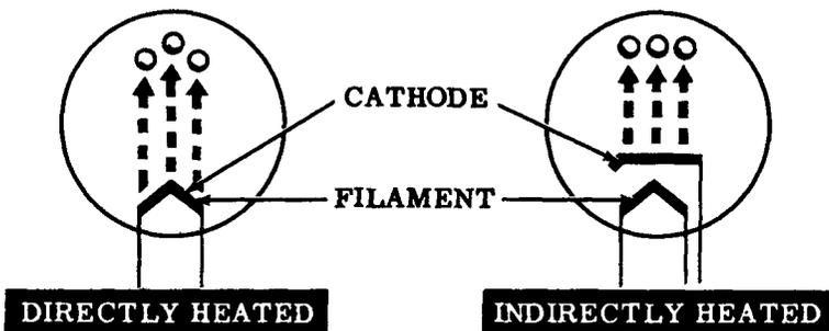
Because they can emit many more electrons than the indirectly heated type, directly heated cathodes are used in vacuum tubes designed for power supplies which supply high currents. Indirectly heated cathodes are more frequently used in low-current power supplies. Having the heater (filament) and the electron emitter (cathode) separate in an indirectly heated tube allows for the separation of the filament's and the cathode's electrical circuits.
