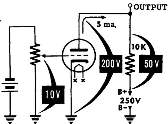
Here is an example of what happens in an actual tube: With the grid voltage = -10 volts, load resistor = 10K ohms, B+ = 250V, the plate current that flows is 5 ma. This current causes a voltage drop across the load of  $E = IR = .005 \times 10,000 = 50$  volts. Therefore, the plate voltage is 200 volts (250 - 50).
