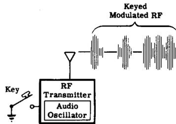
**VOICE TRANSMISSION**—In amplitude modulation a voice signal varies the amplitude of the RF carrier. Transmission is continuous, and is the type used for standard radio broadcasting.
