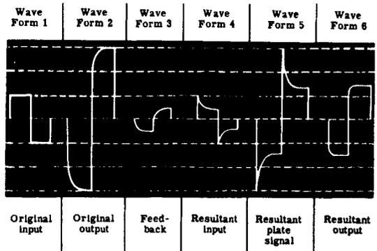
**UNBYPASSED CATHODE RESISTOR** provides degeneration by forcing the cathode voltage to vary as the current varies, introducing distortion opposite to, and thus reducing, that present.
