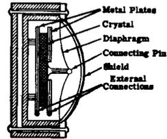
**EARPHONES** operate like microphones in reverse, and produce sound waves in response to electrical impulses. Both the crystal and magnetic earphones are widely used, the magnetic type being most common.
