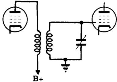
**GAIN**—The number of times a tube or RF coil amplifies a signal. The gain of an RF amplifier can be varied with a pot. placed between the cathode and ground (if a remote cut-off pentode is used).
