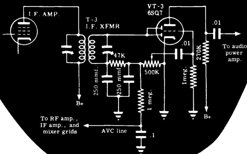
The two 250-mmf capacitors function as the detector filter capacitors. Their purpose is to bypass the IF component of the signal to ground around the 47K and 500K diode load resistors. The 47K resistor is part of the filter network, while the 500K potentiometer also acts as a bleeder resistor across the filter. It controls the amount of detector output delivered through the .01-mfd coupling capacitor to the grid of the first audio amplifier and thus serves as a volume control.
