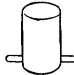
**KLYSTRON**—A vacuum tube designed to operate at frequencies above 1000 mc. It has several forms, all of which use a positive grid as an accelerator and other grids to bunch the electrons together in clusters.
