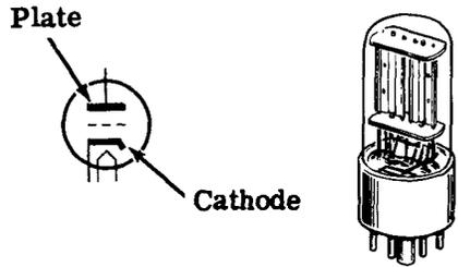
**VACUUM-TUBE RECTIFIER CIRCUIT** — A diode vacuum tube connected in series with an AC voltage source to change AC to DC.
