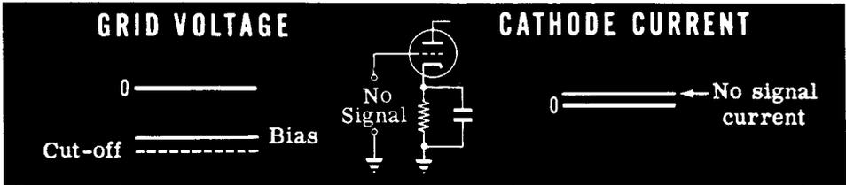
When there is a signal applied to the grid, the cathode current will increase on the positive half-cycles, and become zero (cut-off) on the negative half-cycles. The average current will be increased and the bias will increase.
