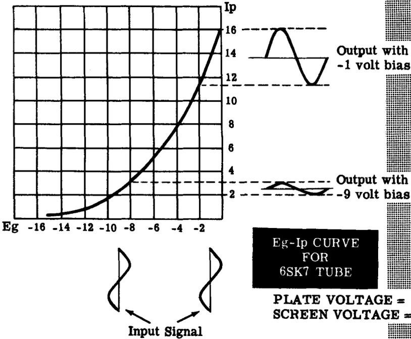
In a remote cut-off pentode the turns of the control grid are spaced closely at the edges and farther apart at the center. The electron flow through the edges of the grid is cut off by very little negative bias. However the electron flow through the center of the grid can only be cut off by a high negative bias. The grid of a sharp cut-off pentode is uniformly spaced. The entire plate current is cut off by one value of bias.
