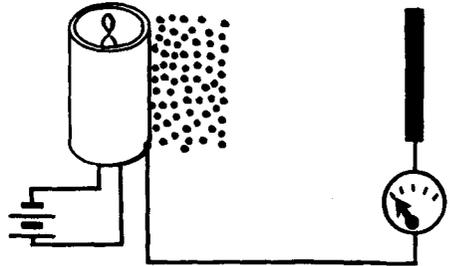
As soon as the plate becomes positive with respect to the cathode, current will flow from the space charge.
