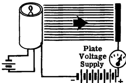
If we now increase the filament voltage above its normal value, we enable the cathode to emit more electrons and, with the same plate voltage as before, we observe that a larger plate current is flowing.
