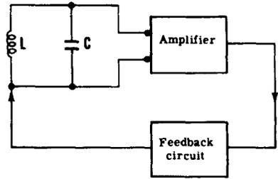
**ARMSTRONG OSCILLATOR**—uses a tickler coil to feed back pulses from the plate circuit to the tank circuit.
