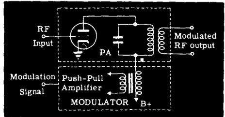
While the applied plate voltage is varying, a constant amplitude of RF is being fed to the grid of the tube from the output of the previous stage, the IPA.
