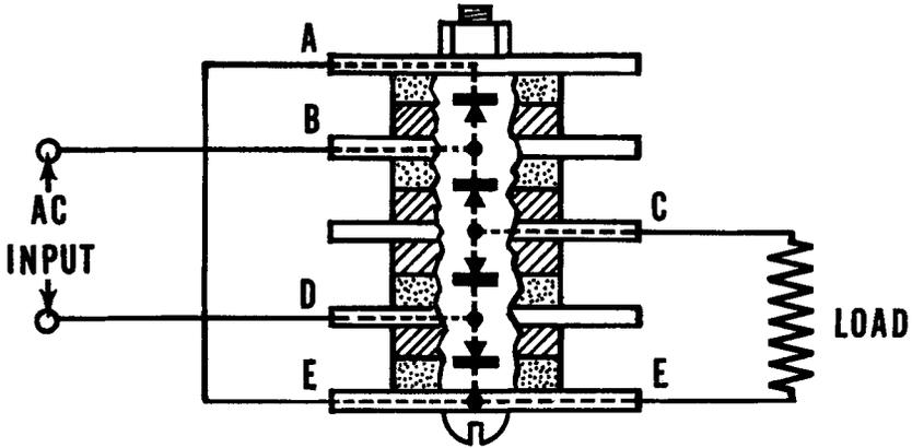
To get from the pictorial to the schematic diagram, just imagine the two end units being rotated around as shown below. Before you continue, make sure you understand the relationship between the physical unit and the schematic.
