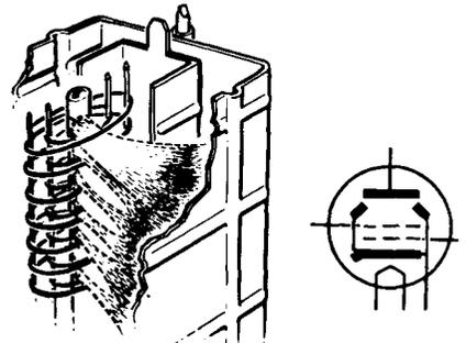
**PENTODE CIRCUIT** — A circuit providing proper operating voltages for control grid, screen grid and suppressor grid.
