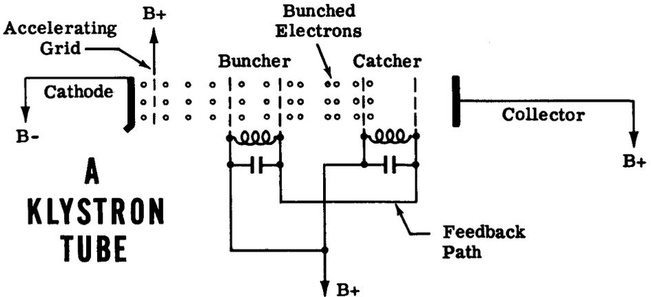
Then these bunched electrons reach the catcher grids and start the second tuned circuit oscillating. Since they keep arriving in bunches, they keep the second tuned circuit oscillating. The oscillations in the first tuned circuit will stop unless voltage is fed back from the catcher grids to keep it going. Of course the tuned circuits in the klystron are not coils and capacitors. They are cavity resonators.
