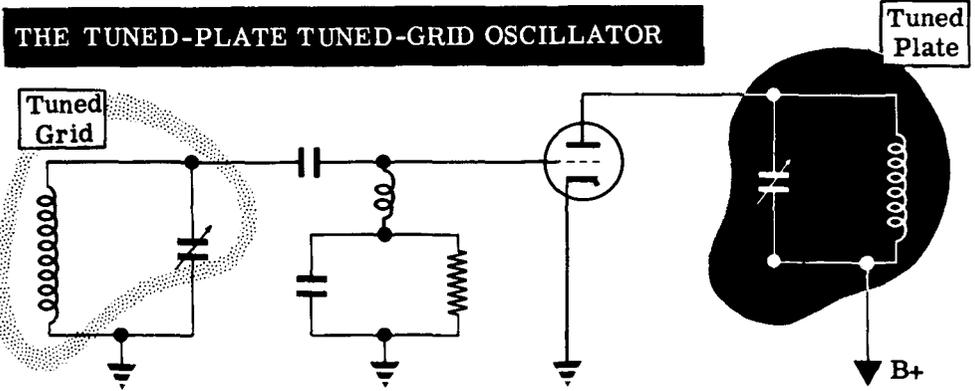
Feedback is accomplished without using either capacitor or coil to couple the energy back. To prove this, suppose you start with the above circuit, but with a pentode tube in place of a triode and use link coupling to feed back energy from plate to grid tuned circuit.
