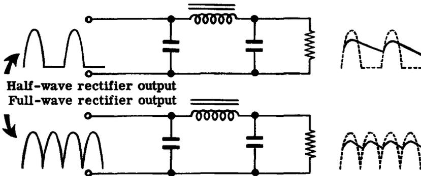
The higher the frequency of the AC input voltage to a power supply the lower the value of the filter capacitors required. The time between pulses is shorter at higher frequencies and the inductive action of the choke is greater at higher frequencies.
