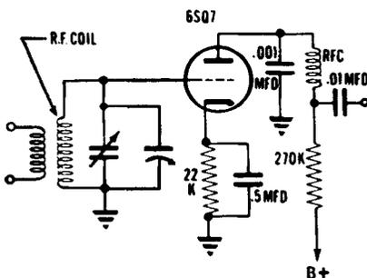
**TRF RECEIVER**—This receiver employs RF amplifiers, a detector and AF amplifiers. The tuned circuits are ganged-capacitor tuned. A shortcoming of the TRF is that since the tuned circuits are not fixed-tuned, constant sensitivity and selectivity cannot be realized over a tunable band.
