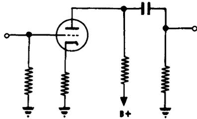
**VOLTAGE DIVIDER FEED-BACK** introduces part of the output voltage across the grid but 180 degrees out of phase, so that distortion is introduced in reverse and thus reduced.
