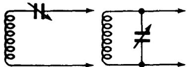
**PARALLEL RESONANT CIRCUIT**—The tuning capacitor is connected in parallel with the coil. It has high impedance at the resonant frequency and low impedance at all other frequencies. It builds up a high voltage at the resonant frequency and a low voltage at all other frequencies. This type of circuit is used most often to tune radio receivers.
