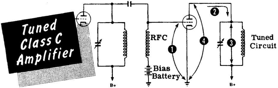
The operation of a Class C amplifier will become clear when you analyze what happens in a tuned amplifier such as the one shown in the schematic diagram. An AC signal is developed across the tuned circuit in the plate of the previous stage. This voltage also appears across the RF choke (RFC) in the grid circuit of the tuned Class C amplifier stage. The DC bias provided by the bias battery causes the tube to operate Class C.
