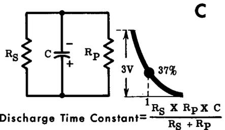
Discharge Time Constant =  $\frac{R_s \times R_p \times C}{R_s + R_p}$
