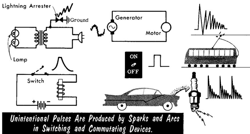
*Unintentional Pulses Are Produced by Sparks and Arcs in Switching and Commutating Devices.*
