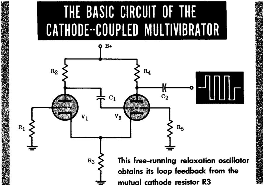
They all produce an overly excited oscillator in which the amplitude of grid signals greatly exceeds the limits required to confine the operation of the tubes to their linear regions. Both the Eccles-Jordan multivibrator and the cathode-coupled multivibrator may be biased to provide single-shot action in which pulses are generated only under provocation of an input trigger pulse supplied from an external source.
