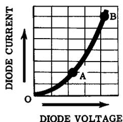
Forward-Conduction Characteristic of a Nonlinear Diode
