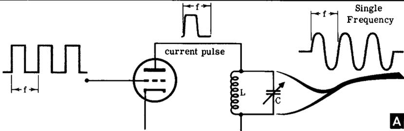
A Frequency Multiplier is Obtained by Resonating the L-C Circuit at the Frequency of One of the Harmonics of the Pulsetrain Applied to the Tube
