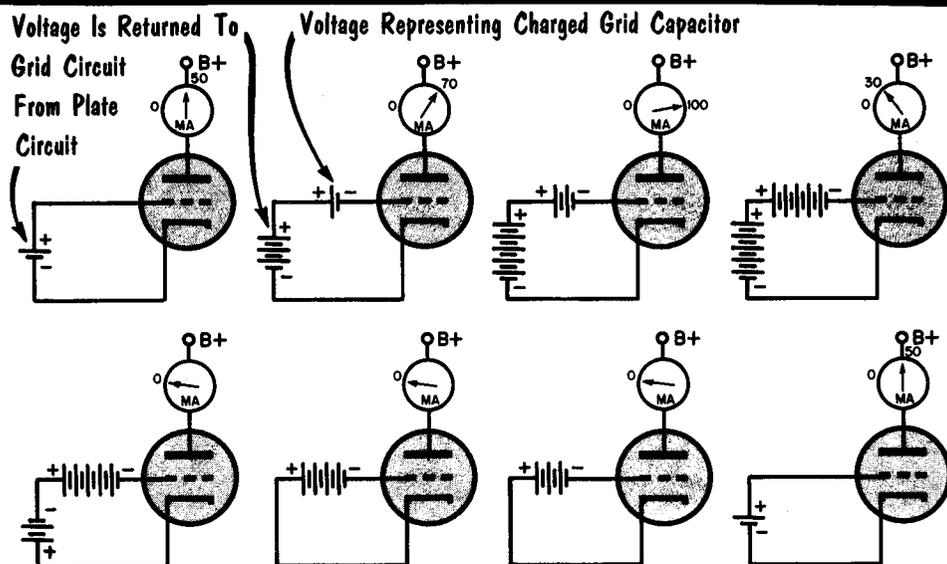
The operation of the blocking oscillator may be better visualized by contemplating the equivalent circuits shown. In these circuits, the grid capacitor is represented by a battery which during plate-current buildup opposes current flow. This flow is produced by another battery symbolizing the feedback voltage delivered to the grid circuit by the transformer secondary. The key to blocking-oscillator action is to be found in the relative polarities and amplitudes of the two batteries.
