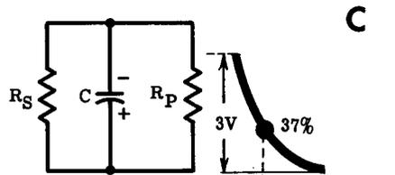
Discharge Time Constant =  $\frac{R_s \times R_p \times C}{R_s + R_p}$
