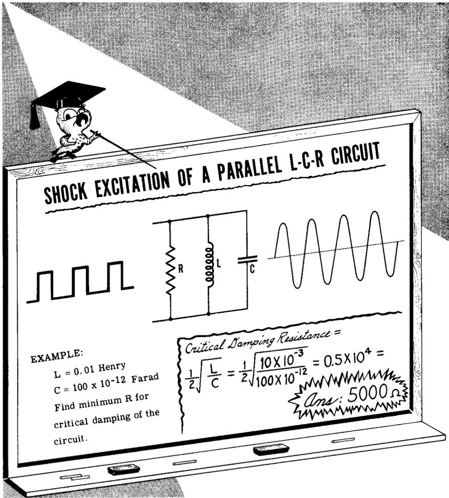
**Question:** A parallel L-C-R circuit is subjected to steep pulses. How can we know whether or not oscillations will be shock excited.
