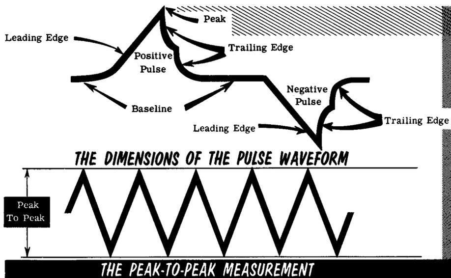
Usually, peak amplitude is measured with respect to the baseline. In some wavetrains, such as the one shown above, it may not be easy to locate the baseline with acceptable accuracy. Here, instead of dealing with the peak amplitude measured from the baseline, we measure from negative peak to positive peak and designate the value thereby obtained as the peak-to-peak amplitude of the waveform.
