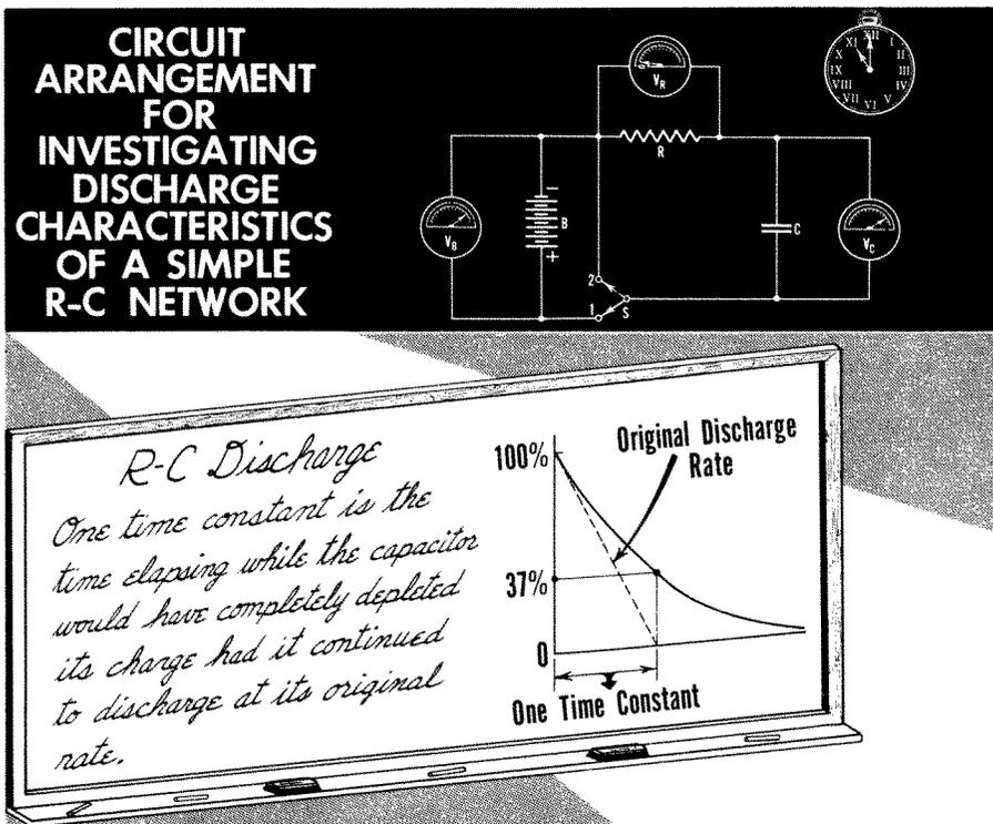
The switch is positioned at its number 1 setting for a length of time corresponding to at least 5 time constants. This assures attainment of virtually full charge of the capacitor. Consequently, at the end of this time  $V_C$  is equal to the charging source voltage  $V_B$ . Next, the switch is positioned at its number 2 setting. Immediately after this, voltmeter readings are recorded at a number of convenient time intervals until  $V_R$  and the  $V_C$  have ceased changing.
