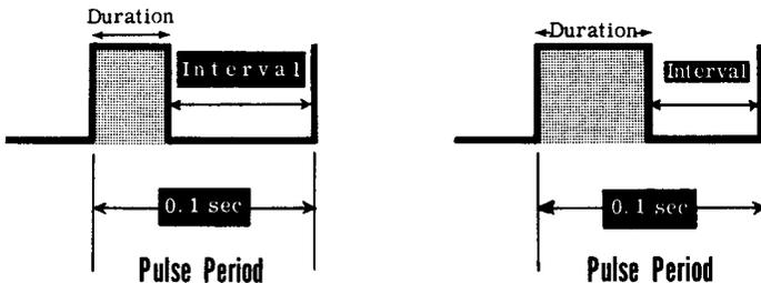
**The Pulse Interval, but NOT the Period, is Affected by Varying Pulse Duration.**
