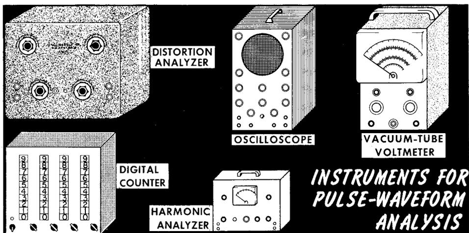
A *distortion analyzer* is essentially a tunable narrow-band rejection filter in conjunction with a vtvm. The level of the composite wave form is measured, then a measurement is made with the tunable filter adjusted to reject the fundamental frequency. From the ratio of the two measurements, the distortion percentage is obtained.
