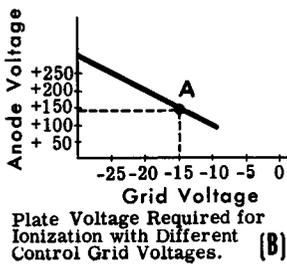
Plate Voltage Required for Ionization with Different Control Grid Voltages. (B)
