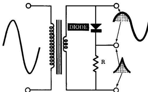
Circuit for Producing Modified Waveshapes
