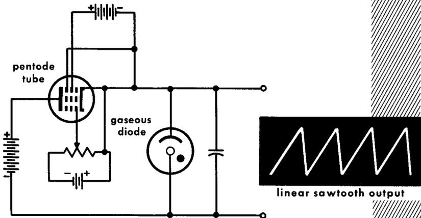
***SUBSTITUTING a PENTODE for a CHARGING RESISTOR IMPROVES the WAVESHAPe of a GASEOUS-DIODE RELAXATION OSCILLATOR***
