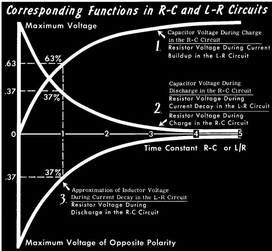
Page 92 shows that three basic curves represent in theory, or approximate in practice, all voltage functions in circuits containing a resistance in series with an energy-storage element, that is, a capacitor or an inductor.
