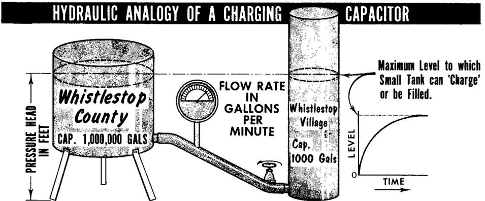
The term capacitance is very descriptive, applied to a capacitor. It is the measure of the number of positive and negative charges required to bring the capacitor to a given voltage level. In an analogous situation, we would say that the capacity of a water tank is the measure of the number of gallons of water required to bring the stored water to a given tank level.
