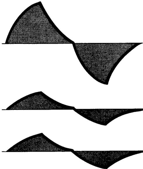
However, a good approximation to the mathematical exponential wave would not be greatly changed by “good” integrating or differentiating networks—R-C or L-R combinations with relatively low resistance. A peculiar property of the exponential wave is that its phase is not shifted by integration or differentiation. Its amplitude is, however, greatly attenuated, as is any other waveshape subjected to integration or differentiation.
