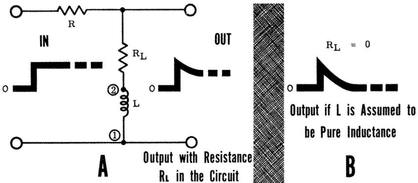
**DEGRADATION OF EXPONENTIAL VOLTAGE CHANGE ACROSS INDUCTOR TERMINALS BECAUSE OF THE RESISTANCE CONTAINED IN THE INDUCTOR**
