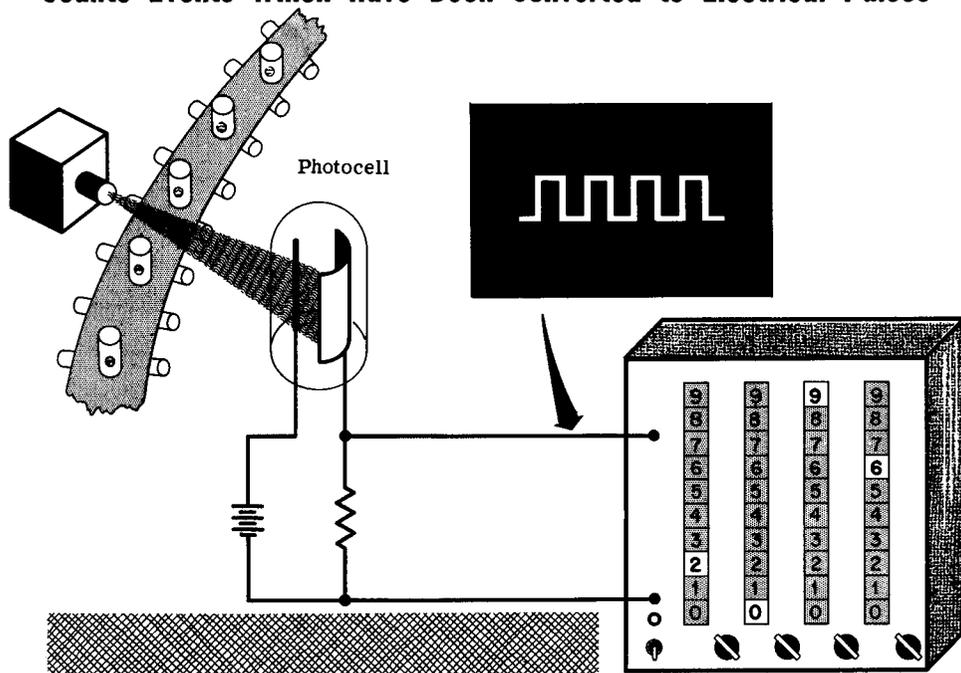
In the illustration, cans moving along a conveyor belt interrupt a beam of light. The interruptions are converted to electrical pulses by the photoelectric cell. Each successive pulse is registered on the indicator panel of the digital counter.
