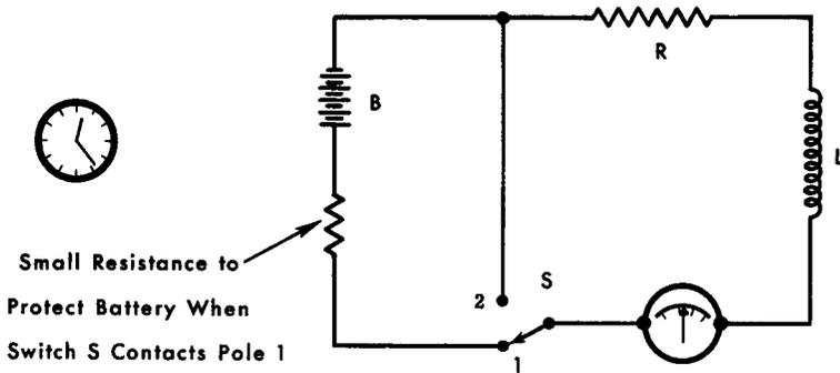
*Behavior of Current in an L-R Circuit Reveals Energy Storage Phenomena Similar to that of Voltage in the R-C Circuit.*
