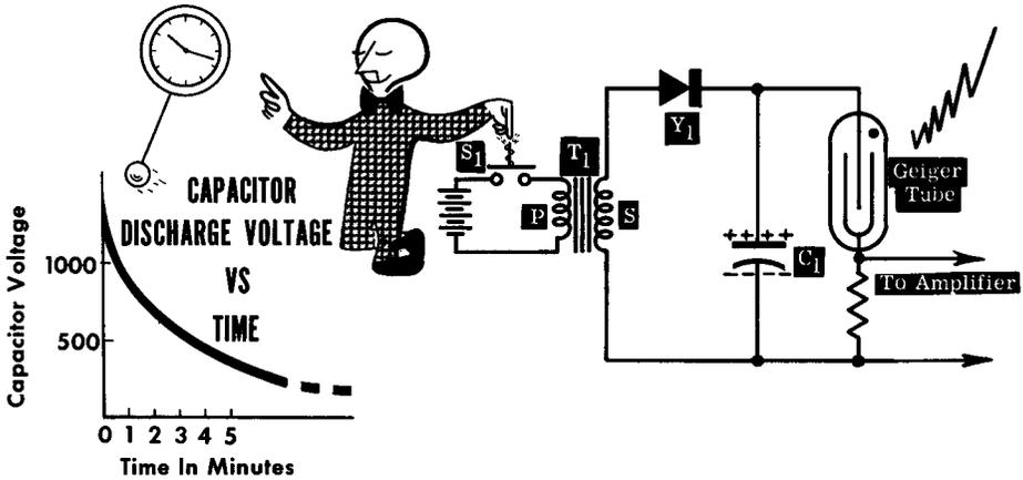
*A Geiger Tube Energized from an Occasionally Charged Capacitor*
