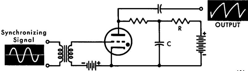
Thyatron Sawtooth Generator Circuit with Provision for Synchronizing Signal. (A)
