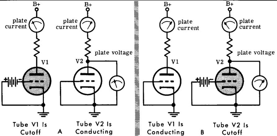
The waveform diagrams of the Eccles-Jordan multivibrator corresponding to the described sequence of events are shown, as are the two conductive states of the circuit. In these circuits, the charged coupling capacitor which holds one of the tubes at cutoff is represented by a battery. Tube V2 in the circuit diagram is assumed to be the output tube; that is, the output waveform is derived from the plate of this tube.
