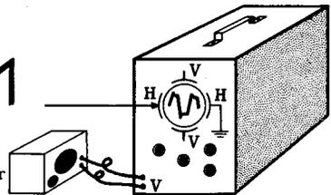
*The Sawtooth Waveform Provides a Linear Time Base for Oscilloscopes*
