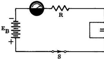
$E_C$  is zero and the capacitor resembles a short circuit
