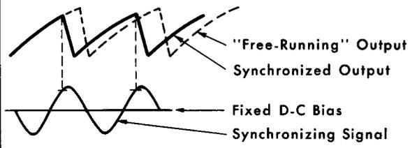
Synchronization of Sawtooth Frequency by Injected Sine-Wave Synchronization Signal. (C)
