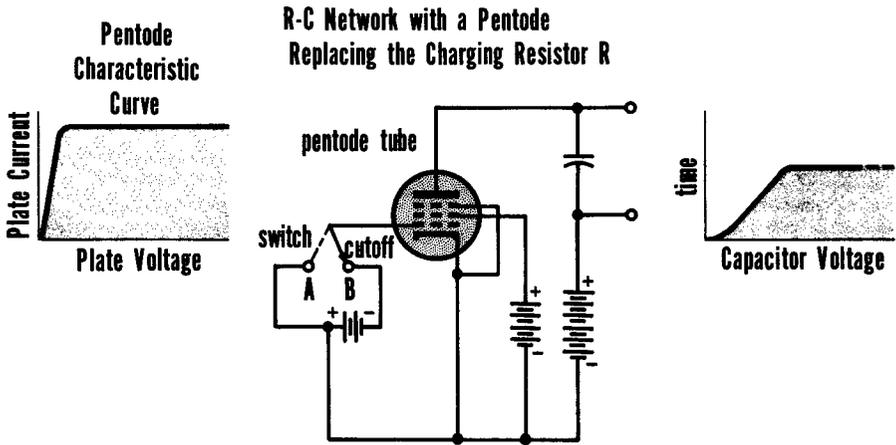
An important kind of nonlinearity is provided over a substantial portion of the plate-voltage plate-current operating characteristic of a pentode tube.
