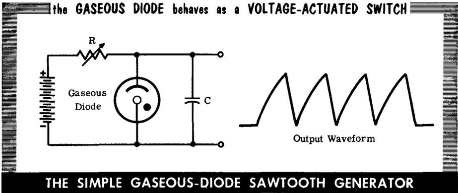
the PEAK-TO-PEAK AMPLITUDE of the GENERATED SAWTOOTH is determined by the DIFFERENCE between the IONIZATION and DE-IONIZATION VOLTAGE LEVELS
