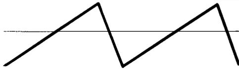
Obvious Distortion of the Output Wave Because of a Small Time Constant
