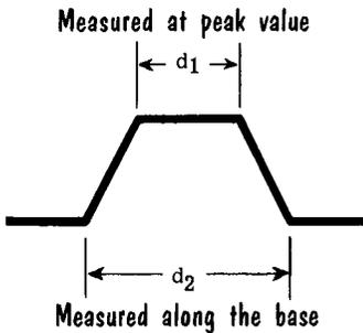
Either the top or the base measurement conveys useful information about pulse duration
