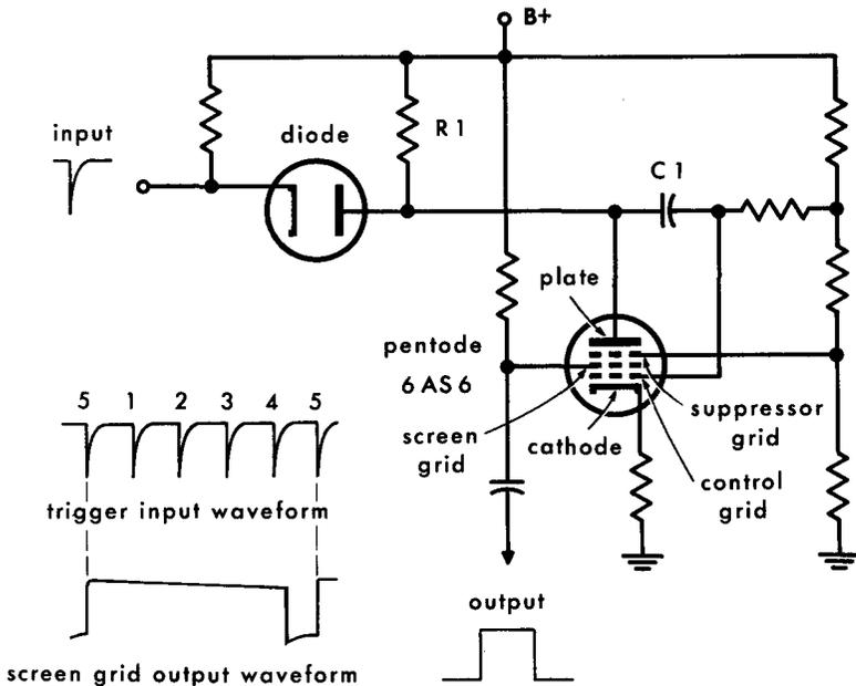
What we have described constitutes division by *five*; if we were to produce simple synchronization (division by one) the *second* pulse would be used to re-trigger the phantastron; if we wished to produce division by two, it follows that the phantastron cycle would have to be adjusted to permit re-triggering by the *third* pulse, and so on for other dividing factors.
