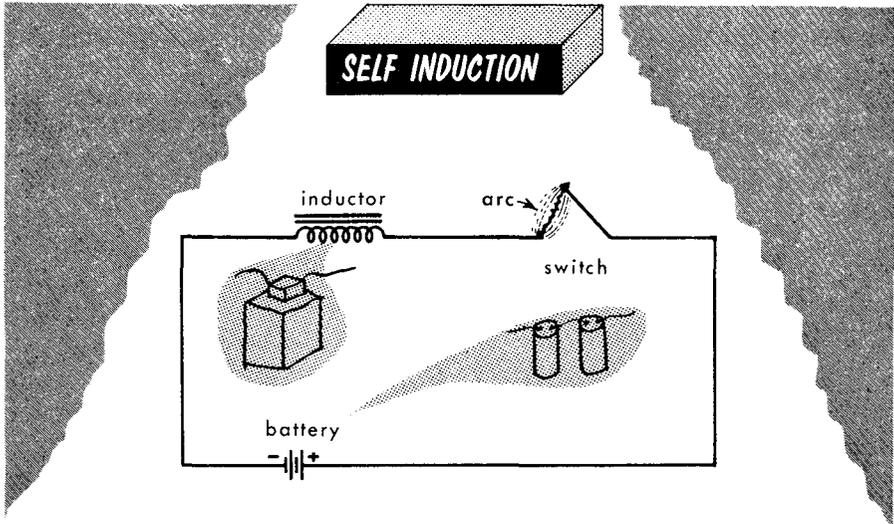
When the switch is opened, the self-induced voltage of the inductor is considerably greater than is the battery voltage
