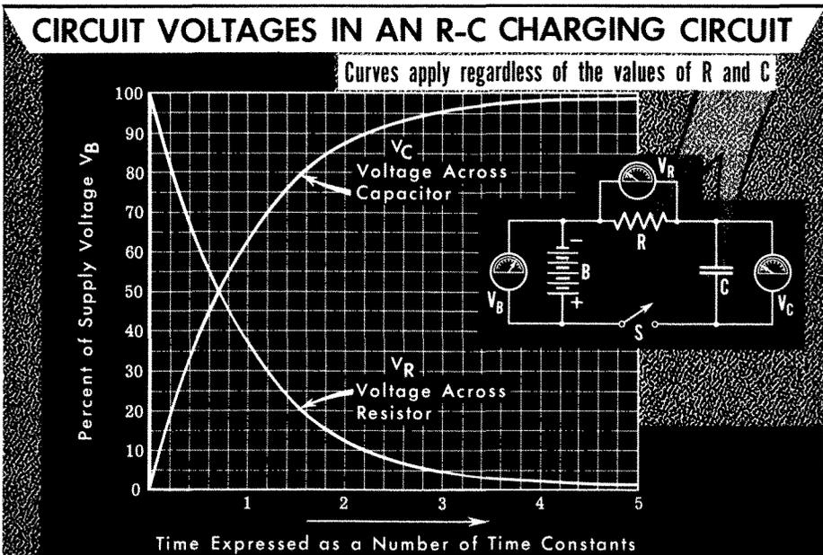
Thinking in terms of time constant is of great value in visualizing circuitry response to pulses. This will be particularly evident when we investigate the emergent waveshapes from low- and high-pass filters when the time constant is changed.
