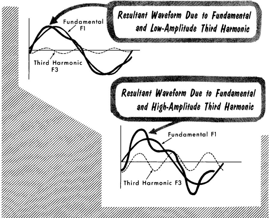
The amplitude of the fundamental frequency in both waveshapes is the same, as is the phasing of the third harmonic. The only difference in the constituent sine waves is the amplitude of the third harmonic. Where the amplitude of the third harmonic is low, there is relatively little distortion of the fundamental sine wave. A high-amplitude third harmonic produces a peaked waveform.
