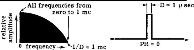
**(C)** When PRR is zero, (when a single pulse is generated) the Harmonic Frequency Spectrum is Continuous.
