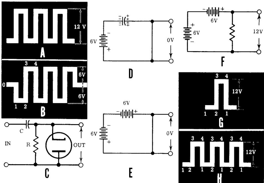
**EQUIVALENT CIRCUITS SHOWING HOW A DIODE RESTORES THE D-C COMPONENT WHICH HAS BEEN REMOVED FROM A PULSE TRAIN BY A CAPACITOR**
