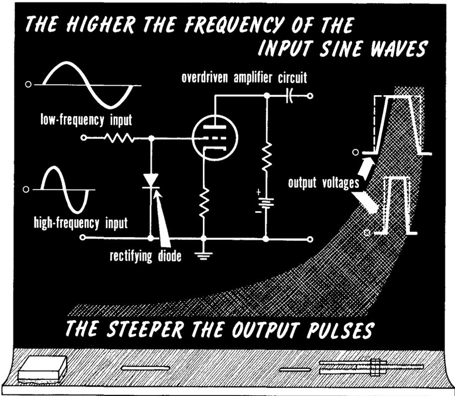
**Question:** What is the pulse-repetition rate of the resultant pulses produced by the amplifier shown.
