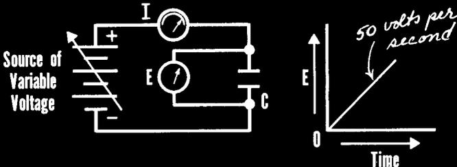
**EXAMPLE:** What current flows in a  $100 \mu\text{f}$  capacitor when the applied voltage across it varies at the rate of 50 volts per second?
