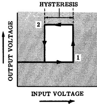
The Relationship between the Input Triggering Wave and the Conduction State of Output Tube V2
