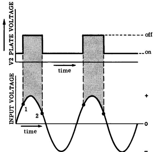
A very rapid switching action ensues, ending with tube V1 in its *off* state and tube V2 in its *on* state. The Schmitt Trigger has been restored to its originally assumed conductive state. The negative excursion of the input sine wave does not effect the conductive state of the Schmitt Trigger; no further switching transition is triggered until the sine wave undergoes its next positive excursion and attains a suitably high positive voltage. When this occurs, the action is repeated.
