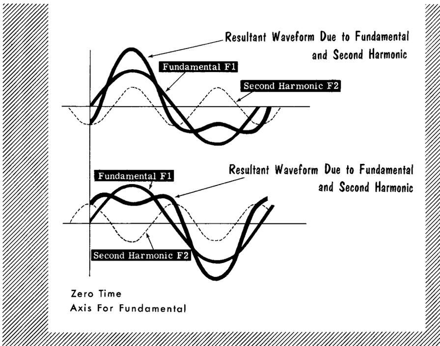
We show the constituents of a simple nonsinusoid made up of a fundamental and a second harmonic. The resultant waveshapes owe their differences to the different phase conditions.
