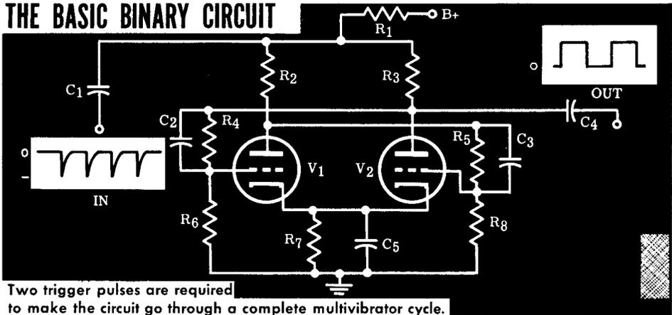
Two trigger pulses are required to make the circuit go through a complete multivibrator cycle.
