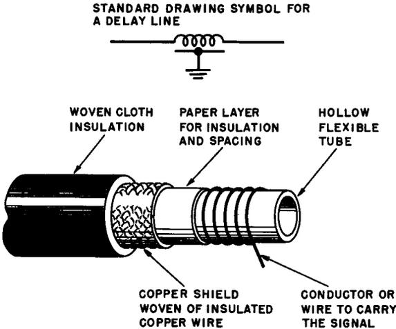
Fig. 38 Delay line construction.
