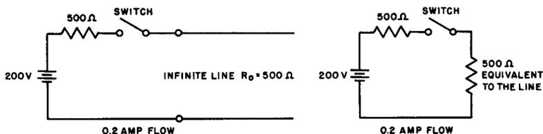
Fig. 30 Charging an infinite line.
