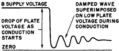
Fig. 17 Damped wave on conduction pulse
