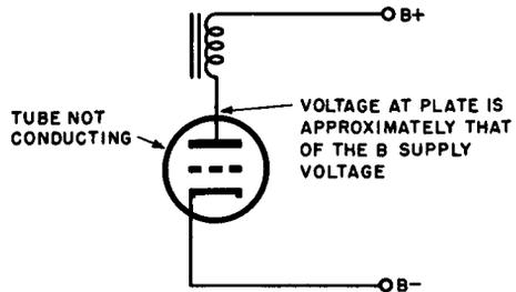
former couples the grid current change to the plate, causing it to appear as a varying potential. This coupled voltage adds to that of the supply. The voltage is, of course quite tiny, both because of the low frequency (gradual change) involved and the small current flow. In many cases it may be neglected.
