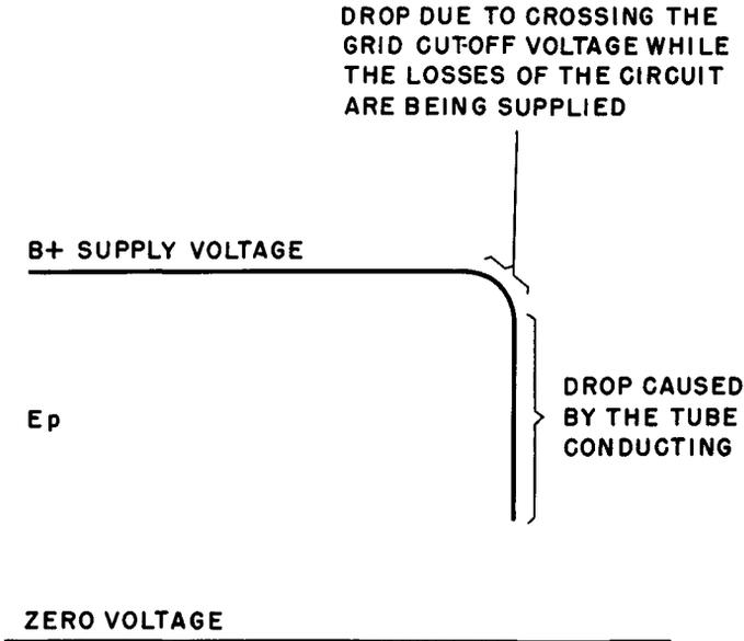
Fig. 12 Plate voltage variation during, and just following, plate cutoff period.
