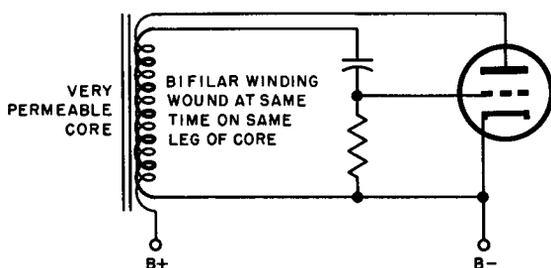
Fig. 8 Bifilar winding.
