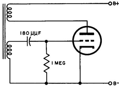
The resistance of the grid resistor is many times greater than the resistance of the grid winding of the transformer. Thus most of the capacitor voltage appears across it.
