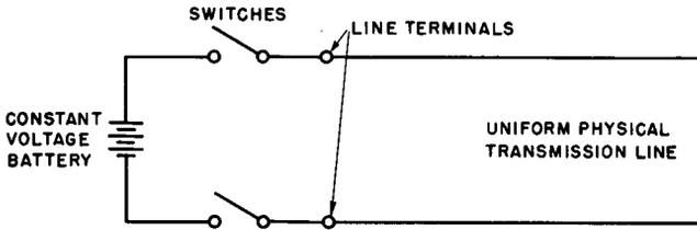
Fig. 29 Battery supply connected to a line.
