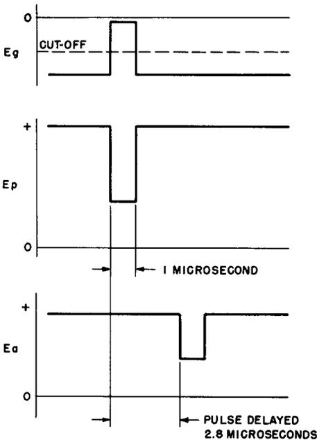
Fig. 34 Pulse delay.
