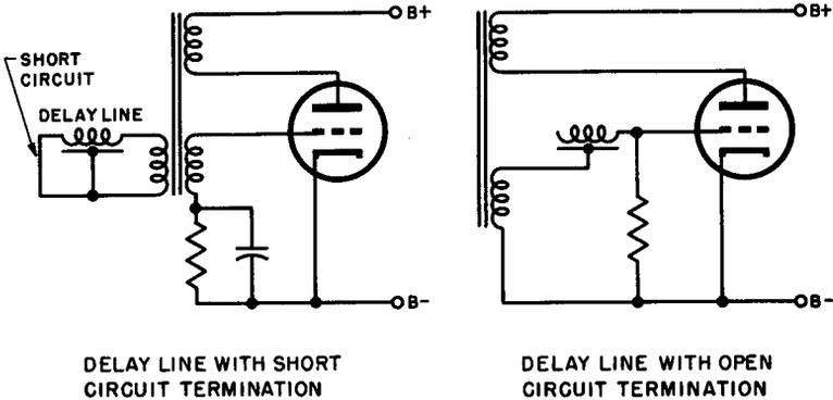
Fig. 39 Methods for terminating the conduction period.
