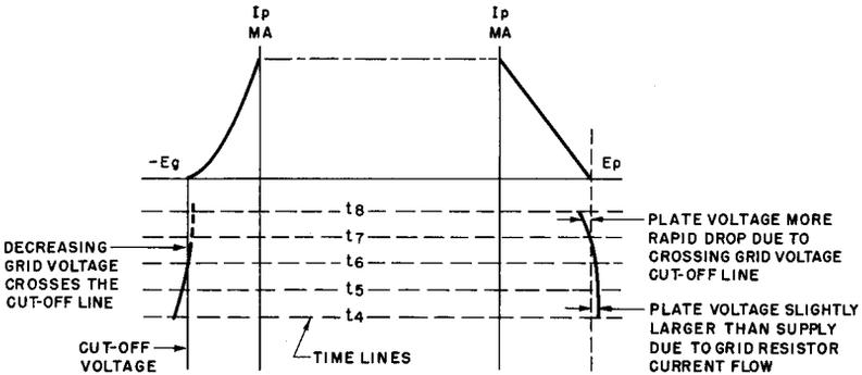
Fig. 7 Conduction due to grid bias.
