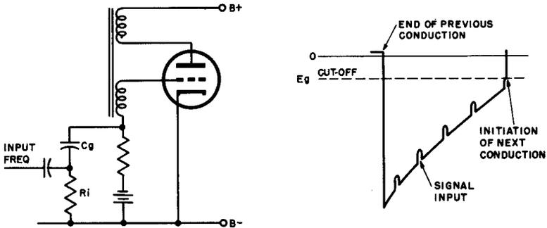
Fig. 43 Blocking oscillator divider.
