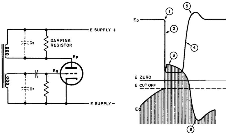
Fig. 18 Plate and grid voltages plotted together.
