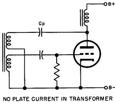
In parallel synchronization, the synchronizing pulse is applied through the amplifying tube to produce a current flow through the plate winding of the blocking oscillator transformer. In the series method, a voltage pulse is applied to the grid circuit of the blocking oscillator. In either case, the oscillator is made to recycle.
