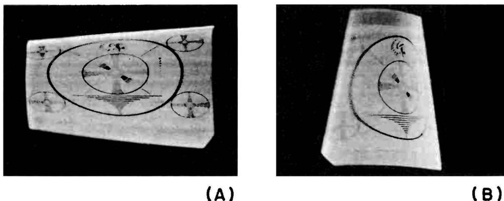
Fig. 9-14. Examples of keystoneing (wedge-shaped raster).
