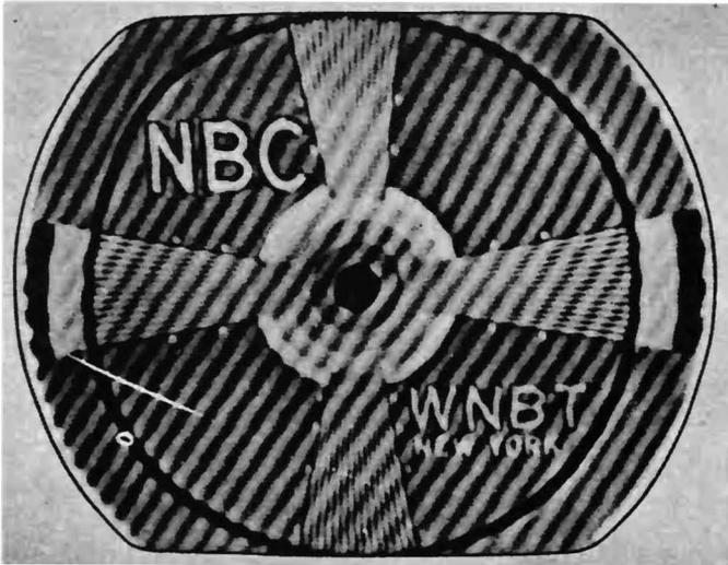
Fig. 9-16. Typical r-f interference pattern.
