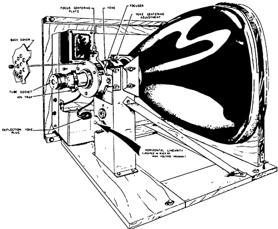
Fig. 6-5. Typical focus adjustment assembly on neck of picture tube.
