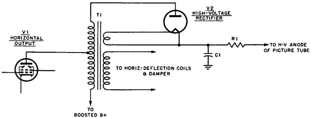
Fig. 2-9. Typical high-voltage power supply circuit.
