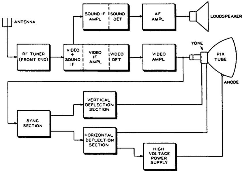
Fig. 2-1. Block diagram of split-sound TV receiver, showing division into sections appropriate for troubleshooting indications.
