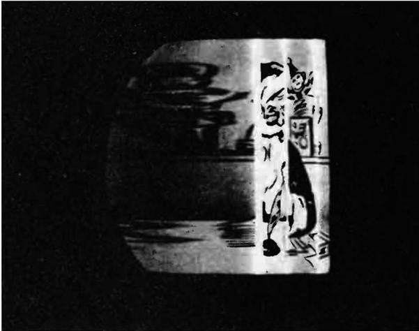
Fig. 9-13. Typical case of picture fold-over resulting from transients in the horizontal sweep section.
