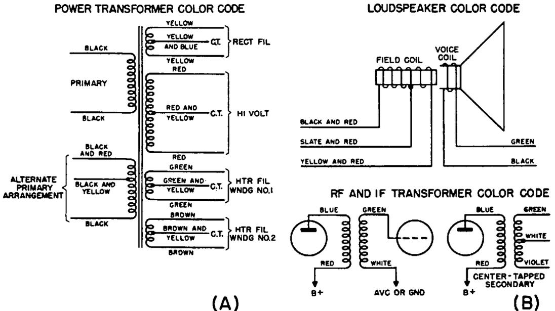
Fig. 1-12. RTMA color codes for wiring of power transformers, i-f transformers, and loudspeakers.
