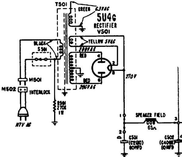
Fig. 1-11. Use of RTMA color code as indicated by the labels showing the colors of the wires coming from the power transformer.
