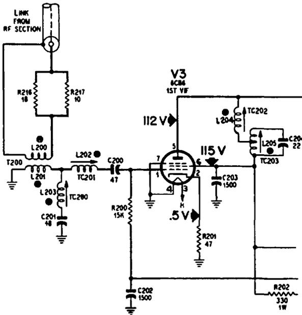
Fig. 1-1. Section of a typical service-type schematic diagram showing particularly how capacitance and resistance values are indicated, and how labels indicate the voltages at strategic points.
