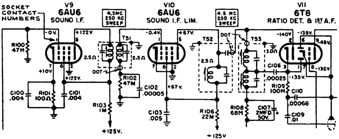
Fig. 1-7. Portion of a TV schematic, showing how the pin numbers of the tubes are indicated on the symbols of the tubes.
