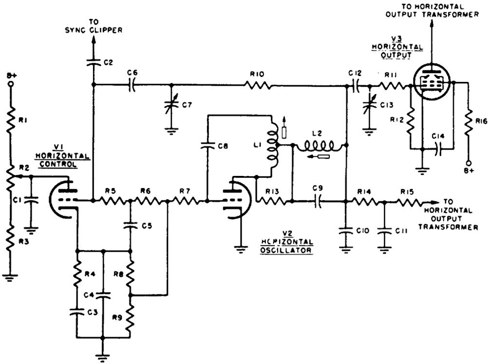
Fig. 2-8. Typical pulse-width horizontal AFC circuit.
