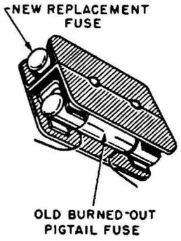
Fig. 3-3. Illustration of use of a fuse clip suitable for replacing pigtail fuses without soldering. One side of the clip slips on the old fuse, still mounted in position, while the other side holds the replacement.
