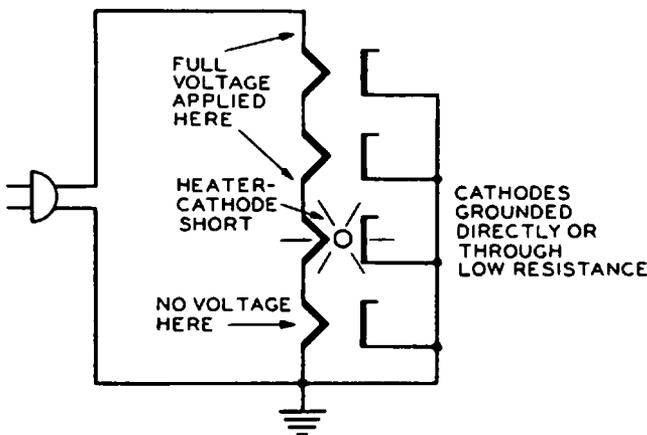
Fig. 8-3. How a heater-cathode short circuit can cause some heaters to glow overbrightly and others to be dead.
