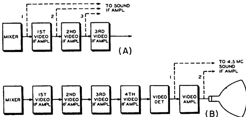
Fig. 2-5. Points at which the sound i-f signal is tapped off in the two main types of receivers: (A) split-sound, and (B) intercarrier. In a given receiver, the tap-off point may be any one of those shown in dotted lines. Where this juncture is found in a serviced receiver is important in determining the source of trouble.
