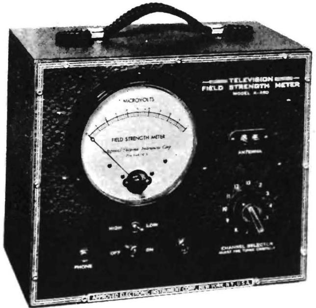
antenna terminals of the receiver is sufficient to provide proper reception. It has been found that a really surprising number of cases of weak reception are caused by deterioration of the antenna due to effects of the weather, gases, dust, etc. These can be spotted immediately with a field strength meter<sup>1</sup> before more laborious and time-consuming receiver tests are undertaken. A typical field strength meter suitable for this work is illustrated in Fig. 3-4.
