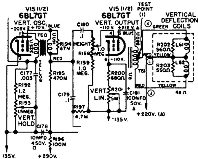
Fig. 6-11. One circuit arrangement for controlling height of the picture.
