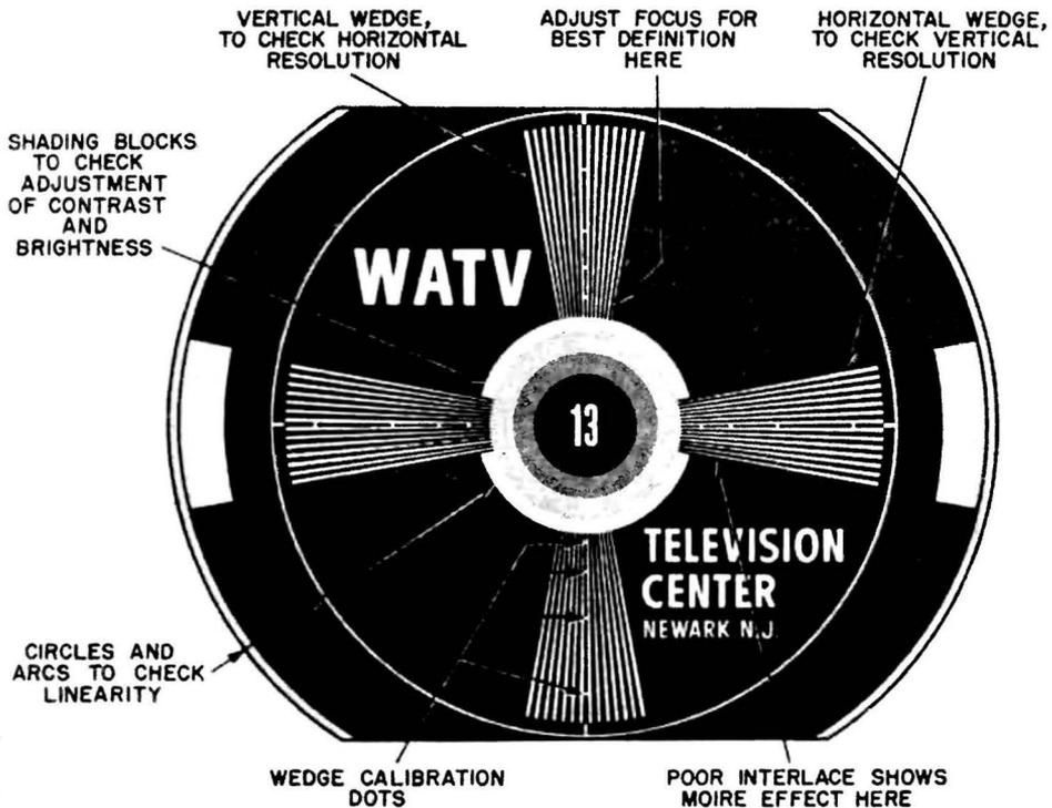
Fig. 5-1. Typical test pattern and the information which it presents.
