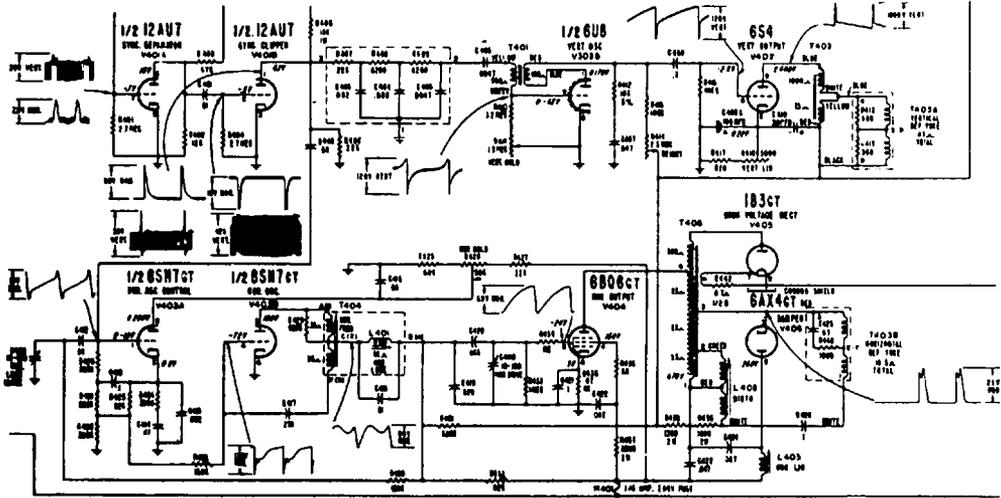
Fig. 1-13. How the waveforms of the voltages at various test points in a receiver circuit are sometimes placed right on a schematic diagram for convenience in oscilloscope testing.
