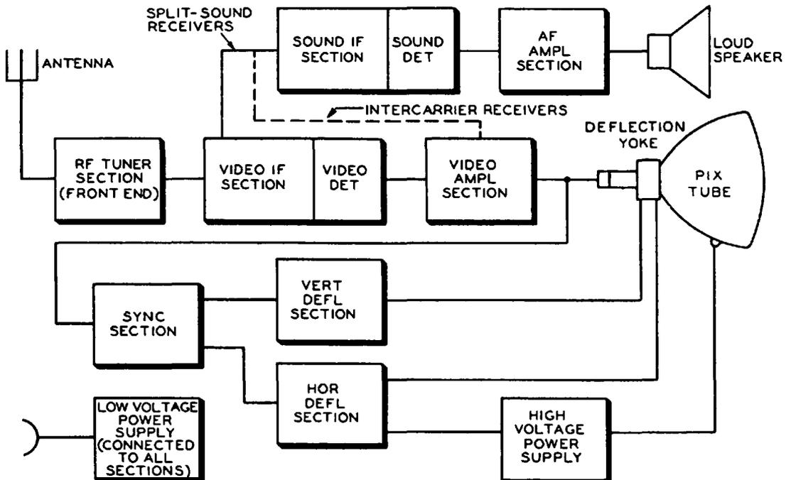
Fig. 2-10. The difference between the division points between the sound and video i-f signals for split-sound and intercarrier type receivers.
