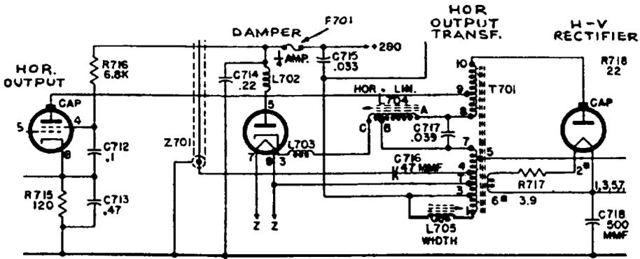
Fig. 6-10. Typical width control circuit.
