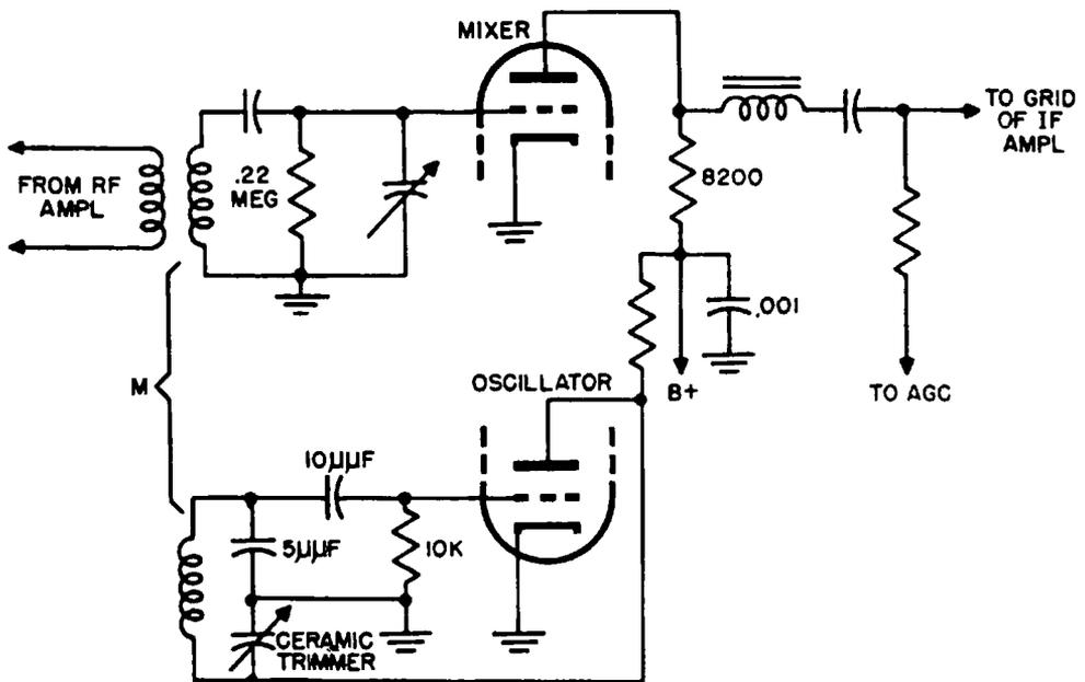
Fig. 2-3. Typical dual-triode mixer-oscillator circuit.
