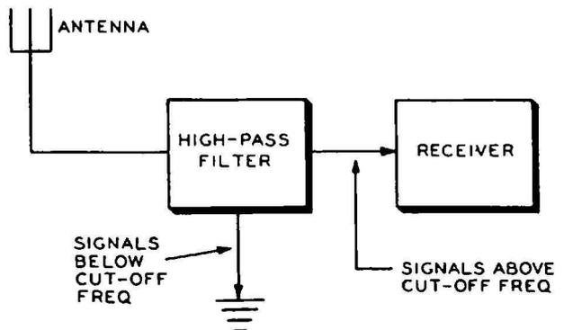
but passes normally all signals having frequencies higher than 45 mc. Thus our interfering signal at 31 mc is filtered out and the desired TV station signal at 60 to 66 mc passes normally into the receiver. Since the strong 31-mc signal is thus kept out of the front end, the latter is not overloaded, and the second harmonic is not generated.
