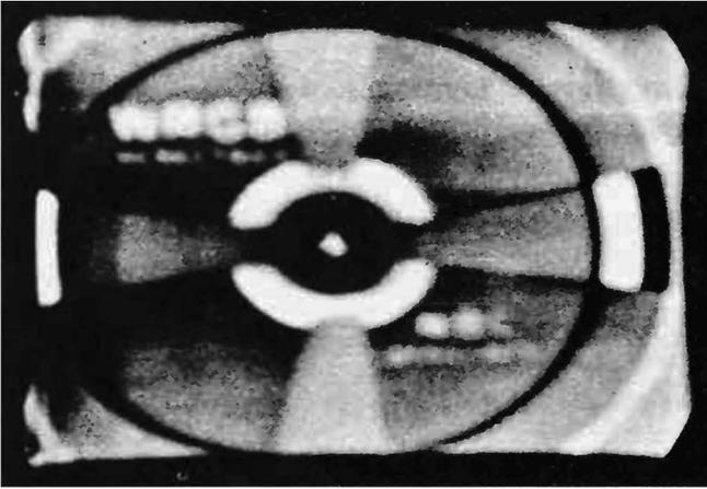
Fig. 6-6. Example of a picture which is not properly focused.
