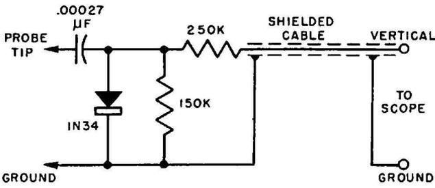
Fig. 9-7. Typical crystal probe circuit suitable for use with an oscilloscope to trace video signals in the i-f section.
