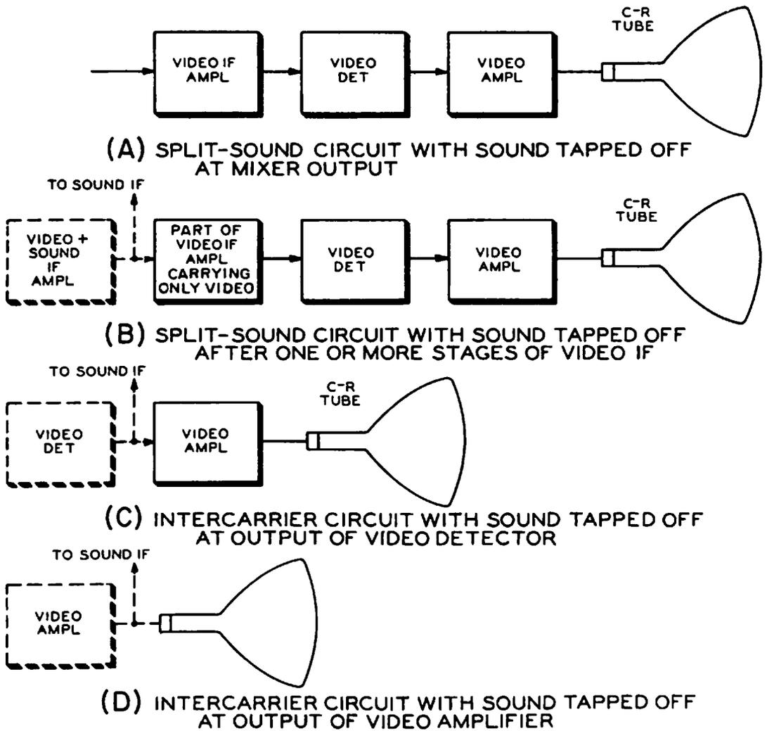
Fig. 9-6. Possible trouble areas for different circuit arrangements when the symptom is raster and sound but no picture.
