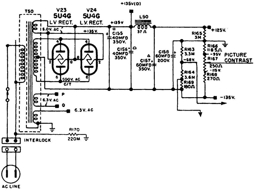
Fig. 2-11. Typical low-voltage power supply.
