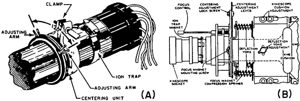
Fig. 6-13. Yoke and other adjustments on the neck of the picture tube.
