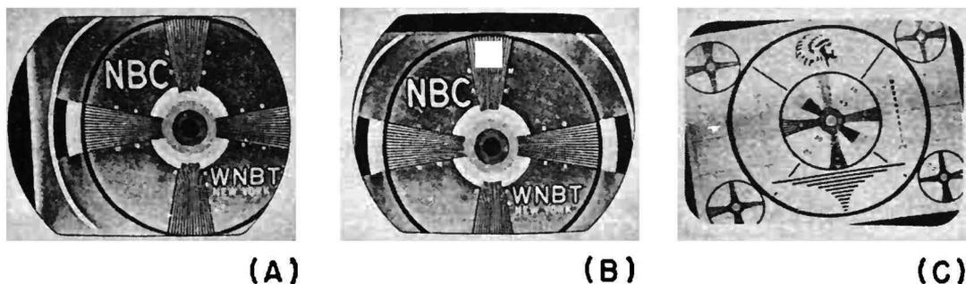
Fig. 6-12. (A) Improper centering, picture to right. (B) Improper centering, picture low.
