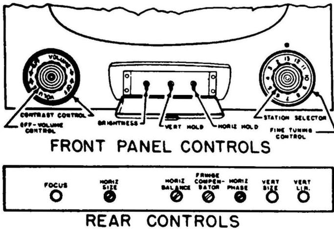
Fig. 1-8. Typical control location diagram.
