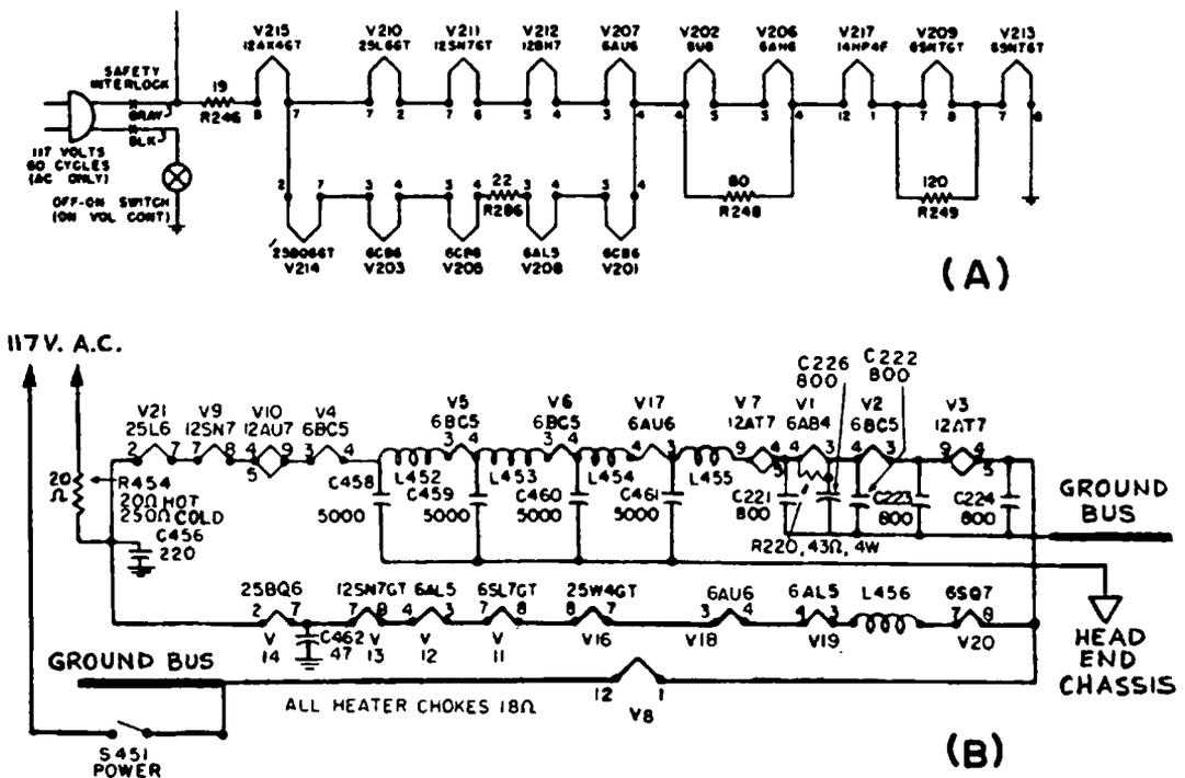
Fig. 8-1. Examples of series-heater circuits used in transformerless TV receivers.
