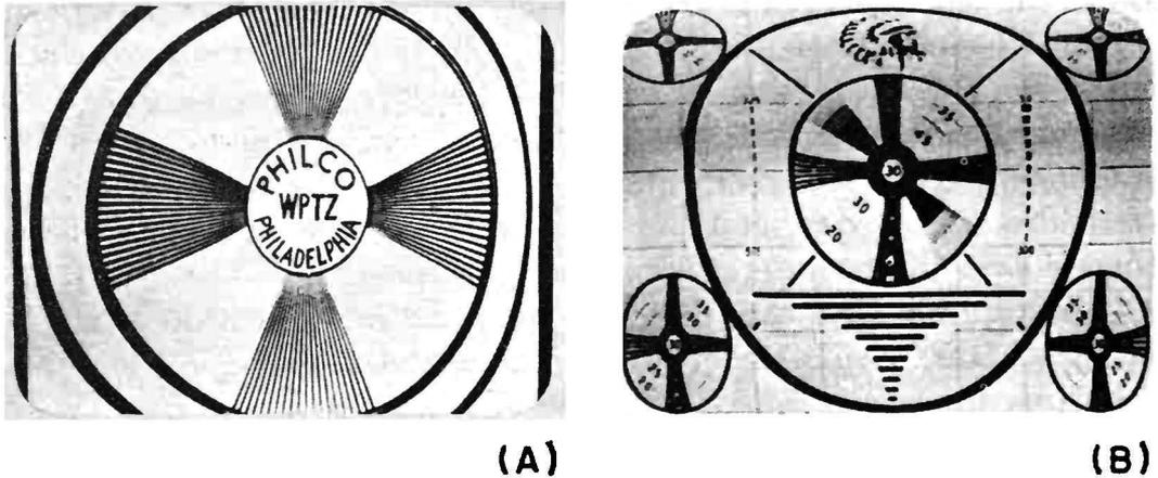
Fig. 6-7. (A) Horizontal nonlinearity. (B) Vertical nonlinearity.
