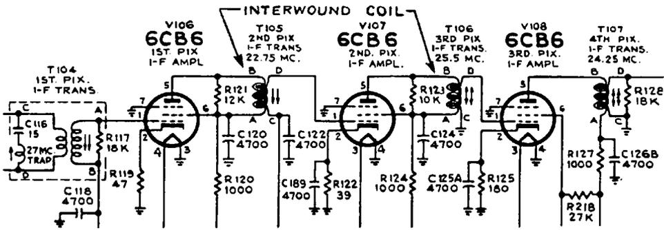
Fig. 1-3. How interwound, or bifilar, windings of a transformer are indicated on a schematic diagram.
