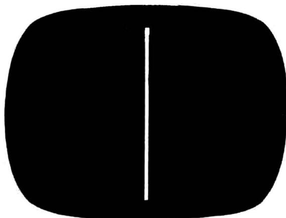
Fig. 9-4. Pattern when there is no horizontal sweep but with high voltage still present.
