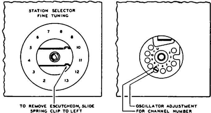
If there is sufficient range to the oscillator trimmer, there may be two points at which reception of sound is possible. However, only one will give proper picture reception, so the picture must also be noted while the adjustments are being made.
