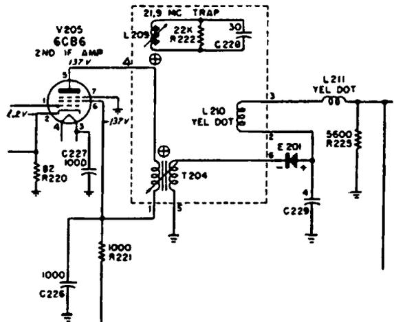
Sometimes i-f transformers are designed so that the primary and secondary windings are *interwound*, that is, the turns of the secondary winding are wound between alternate turns of the primary winding in order to obtain maximum coupling. Figure 1-3 shows how this is indicated on a typical i-f amplifier diagram. Such windings are also called *bifilar*.
