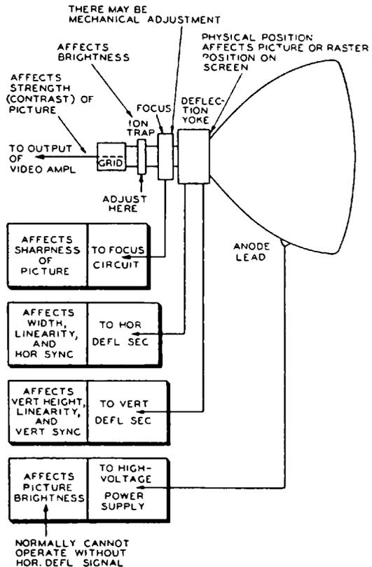
Fig. 2-6. Block diagram showing the source of each indication on the picture-tube screen.
