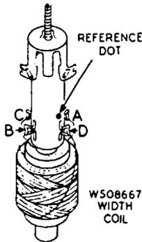
Fig. 1-4. Drawing used to indicate the physical locations of the connection points on a component. Such drawings are frequently placed alongside the appropriate symbol on the schematic diagram.
