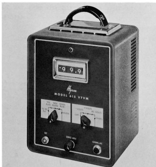
Fig. 14-9. Digital VTVM. Hycon model 615
