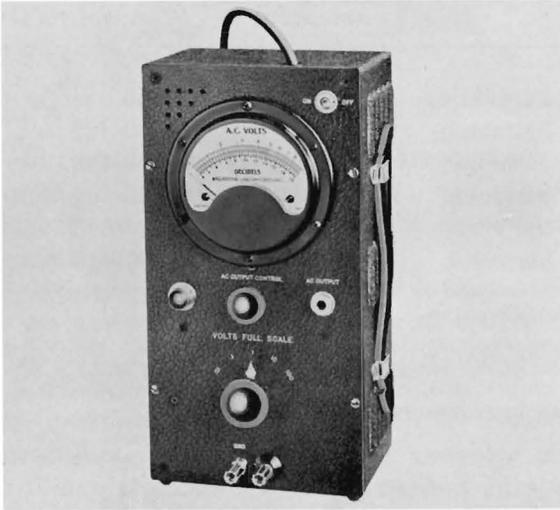
Fig. 14-3. Logarithmic-type meter. Ballantine a-c VTVM model 300
