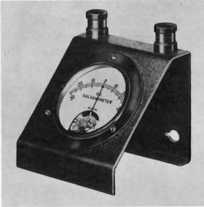
Fig. 1-5. A Weston center zero galvanometer.
