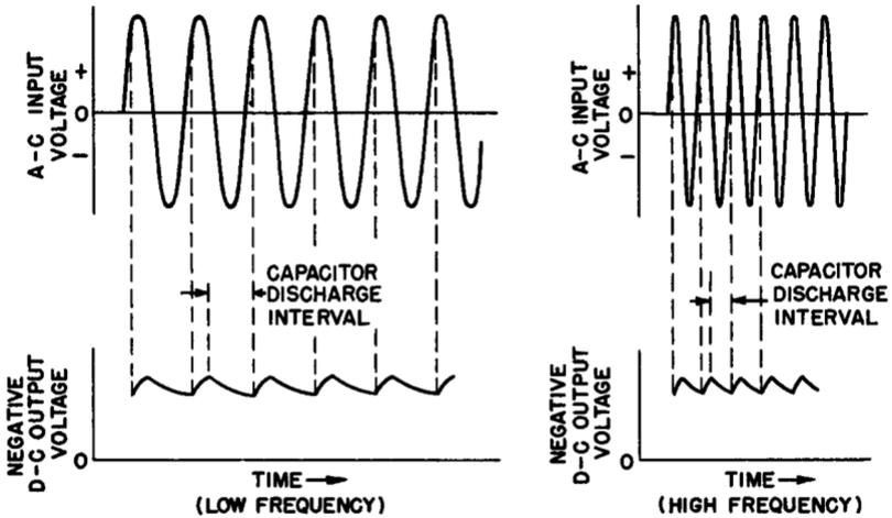
Fig. 6-6. Effect of the frequency of the voltage under measurement on the time constant requirements of the rectifier circuit of a vtvm. A longer time constant is required when a low-frequency voltage is to be measured, since the time duration of the interval during which the R-C circuit capacitor is required to discharge during each cycle is longer, the lower the frequency.
