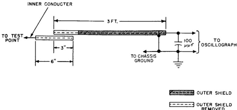
Fig. 2-3. Simple shop-constructed capacitance-divider type high-voltage probe made of coaxial cable. The voltage stepdown ratio is approximately 100-to-1. Courtesy: DuMont Service News
