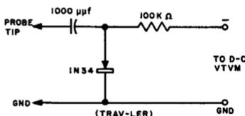
HIGH IMPEDANCE, HIGH SENSITIVITY, PEAK-INDICATING TYPE. SHUNT RECTIFIER. INTENDED FOR HIGH-FREQUENCY APPLICATIONS.
