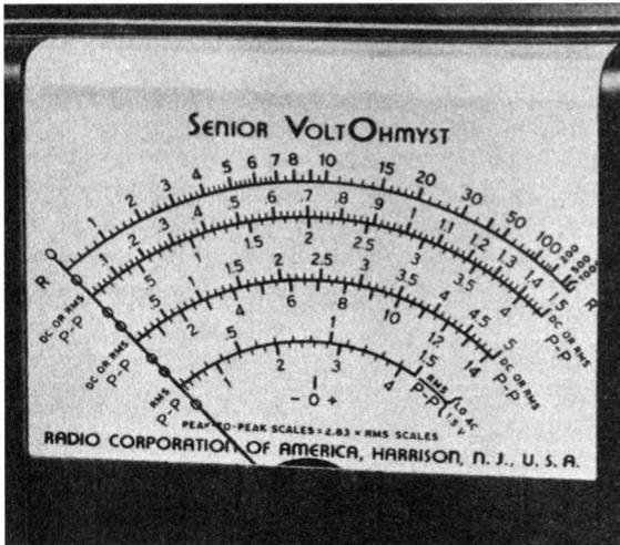
Fig. 6-8. Convenient direct-reading d-c, rms (sine-wave), and peak-to-peak (sine or complex wave) voltage scales available in a typical service-type peak-to-peak vtvm. Courtesy: RCA
