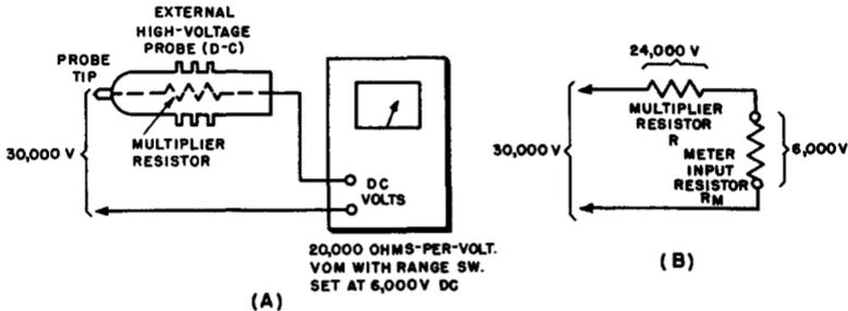
Fig. 1-2. (A) Connection of multiplier resistor in series with vom input circuit. (B) Voltage distribution in the series probe-plus-meter circuit, for the particular conditions specified in the text problem.
