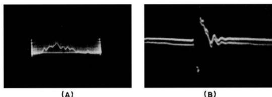
Fig. 7-26. An attempt to obtain signal pickup for a demodulator probe by means of a floating tube shield may be disappointing unless the horizontal- and vertical-sweep circuits of the tv receiver are first disabled. (A) Interference from stray field of horizontal sweep circuit. (B) Interference from stray field of vertical sweep circuit.
