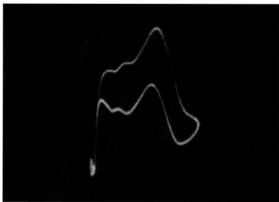
Fig. 7-38. Distorted video response trace obtained when a simple series-type demodulator probe is used to demodulate the output sweep signal from a video amplifier in which strong hum voltage is present. The hum distortion is seen to be severe, and the time constant of the probe is excessively long for the rate of change of the modulation envelope.
