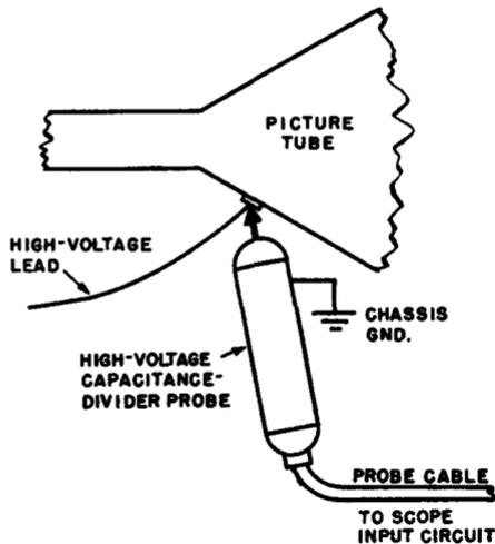
Fig. 2-6. High-voltage ripple and 60-cycle regulation buzz can be displayed on the scope screen with the use of a capacitance-divider type high-voltage probe applied to the crt second-anode terminal. (See also Fig. 2-7 and Fig. 2-9.)
