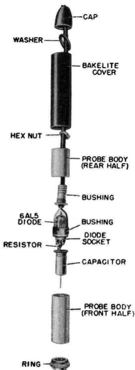
Fig. 6-4. Disassembled twin-diode tube-type peak-indicating rectifier arranged in probe form, for measurements for audio frequencies up to about 250 mc. The second diode section is used to balance out the contact potential of the first one. *Courtesy: RCA*
