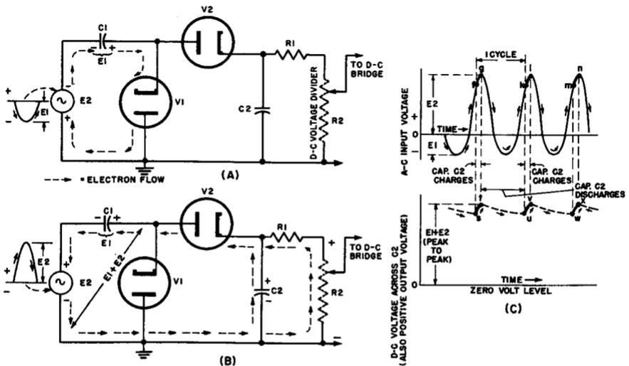
Fig. 6-7. (A), (B) Basic circuit arrangement and action of a cascade-type tube diode half-wave voltage-doubler rectifier circuit during successive negative and positive half-cycles of the a-c input voltage. (C) Graphs of the a-c voltage input, and the d-c voltage output, showing the inherent peak-to-peak response of this type of rectifier for any waveform.
