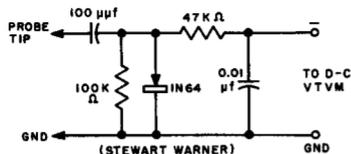
RELATIVELY HIGH IMPEDANCE, MEDIUM-HIGH SENSITIVITY. PEAK-INDICATING TYPE. SHUNT RECTIFIER. INTENDED FOR HIGH-FREQUENCY APPLICATIONS.
