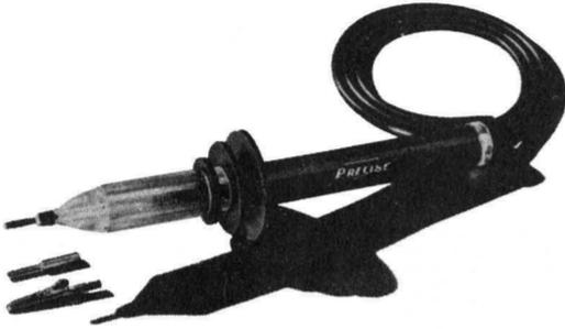
Fig. 1-5. External appearance of a high-voltage d-c probe for use with a vom or a vtm, provided with an interchangeable conventional tip for probing, and an alligator clip for permanent connection to the circuit. The multiplier resistor cartridge is held between a double-spring suspension system inside of the clear plastic portion at the left. This probe is rated at 30,000 volts maximum. *Courtesy: Precise Development Corp.*
