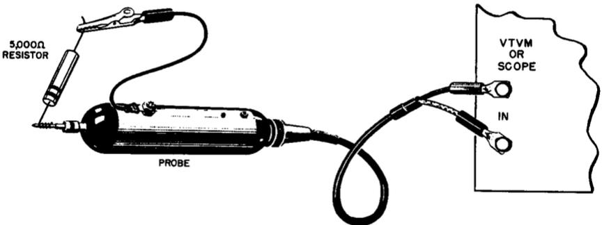
Fig. 7-20. Method of testing a probe to determine if its shielding is adequate to prevent spurious-voltage induction into its components or wiring by the extraneous fields around a tv chassis. Use the very smallest amount of exposed resistor leads in this arrangement.
