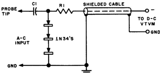
Fig. 6-17. High-impedance peak-indicating crystal probe which employs a number of crystal diode rectifiers in series.
