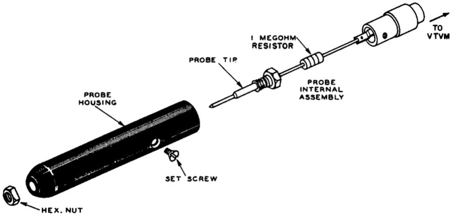
Fig. 4-1. Exploded view of typical vtvm d-c probe containing a 1-megohm series-connected isolating resistor. The particular probe illustrated here is designed to be slipped on to a standard direct-probe and cable whenever d-c voltages are to be measured. *Courtesy: RCA*
