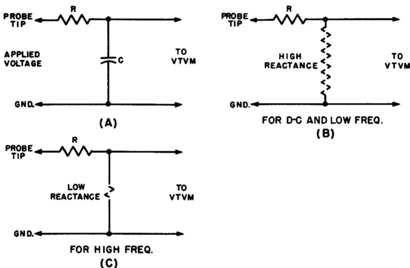
Fig. 4-3. Resistive-isolation probe circuit action which illustrates why the high frequencies are discriminated against when an attempt is made to employ a resistive isolation probe to minimize the loading effect of the cable capacitance upon the circuit under test during high-frequency a-c voltage measurements made with a vtvm.
