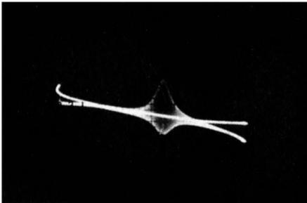
Fig. 5-20. Abnormal displays are sometimes obtained on the scope screen when a low-capacitance probe is being used. For example, because the shielded input cable to the scope becomes resonant at certain high frequencies causing resonant rises of voltage at these frequencies with consequent rectification occurring in the scope input stage, the unexpected pattern shown here may appear on the screen when the high-frequency output from a sweep generator is applied to a low-capacitance probe.
