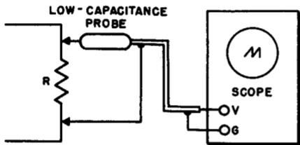
Fig. 5-21. A low-capacitance probe and scope may be used to display the waveform of the current in a circuit by connecting a small resistance in series with the circuit and applying the probe across the resistance.
