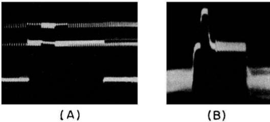
Fig. 7-34. (A) Display of demodulated composite video i-f signal obtained when scope is connected via a low-capacitance probe at the output of the video detector in a tv receiver. (B) Stripped appearance of the display of the demodulated composite video r-f signal obtained when the scope is connected via a demodulator probe at one of the video i-f amplifier stages. There is a definite reason for the difference in the appearance of the two displays (see text).
