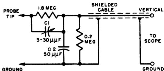
Once the probe has been adjusted for proper operation with a certain scope and cable, it should be used only with that instrument and cable; it must be readjusted if used with any other instrument and cable. In fact, when used with some scopes, it may be necessary to readjust the probe if the scope Gain selector setting is changed from that employed when the original adjustment of the probe was made. This is discussed in detail in Sec. 5-3.
