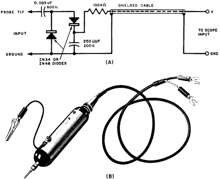
Fig. 7-18. (A) Voltage-doubler type of demodulator probe for obtaining increased output and greater deflection on the scope than is provided by conventional type of demodulator probes. (B) A typical commercial probe of this type. This probe is provided with its own shielded cable for connection to the scope input terminals. (B) Courtesy: Scala Radio Co.
