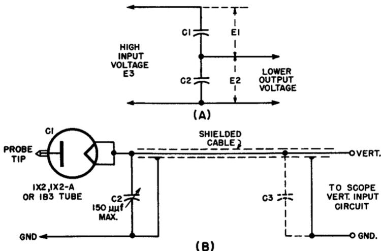
Fig. 2-2. (A) Basic circuit arrangement of a capacitive-type voltage divider. (B) A practical capacitance-divider type high-voltage probe for attenuating high test voltages to the lower values that lie within the safe input voltage rating of the scope. Trimmer capacitor C2 is adjusted to provide the correct desired voltage-stepdown ratio when the probe and its cable are connected to the input circuit of a given scope.
