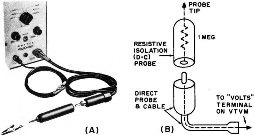
Fig. 4-5. (A) Separable-probe arrangement used for vtm resistive isolation (d-c) probe. Provides d-c and a-c voltage test facilities with one test cable. (B) Circuit arrangement of separable probe and test cable. (A) Courtesy: RCA
