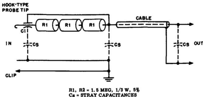
Fig. 5-13. Construction details of the special 40-to-1 low-capacitance probe shown at the lower left of Fig. 5-11. Courtesy: Linear Equipment Laboratories, Inc.
