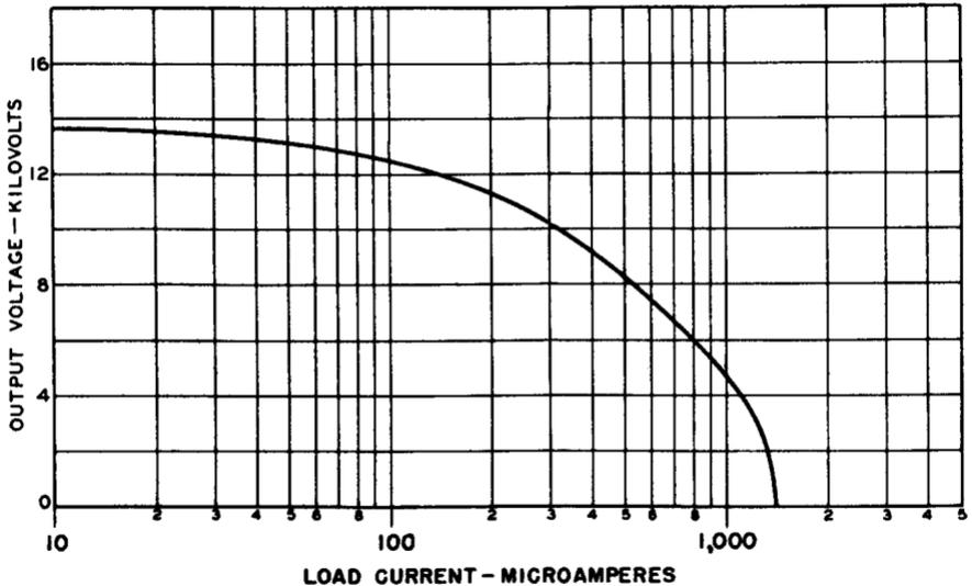
Fig. 1-3. Measured steady-load voltage regulation characteristic of high-voltage supply for the 16AP4 picture tube. Courtesy: RCA
