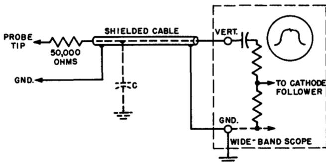
Fig. 4-8. Use of an isolating resistor with scope to produce sharp markers in visual alignment work.
