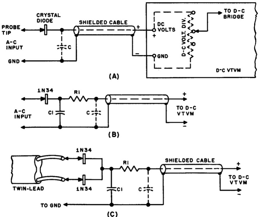
Fig. 6-14. Three versions of the series type crystal-diode peak-indicating rectifying circuit arranged in a probe for use with a vtvm. The double-ended circuit in (C) is useful for checking voltage in a 2-wire transmission line.
