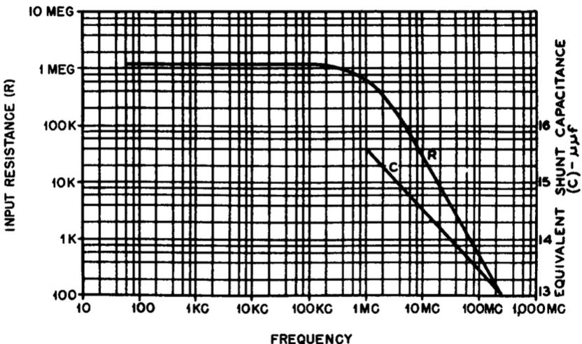
Fig. 6-22. Variation of the effective input resistance and capacitance, with frequency, for a peak-to-peak rectifying probe employing a 6AL5 twin-diode rectifier. Courtesy: RCA
