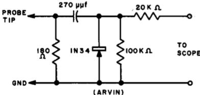
LOW IMPEDANCE; RELATIVELY LOW SENSITIVITY. SHUNT RECTIFIER. SCOPE CABLE ISOLATED.
