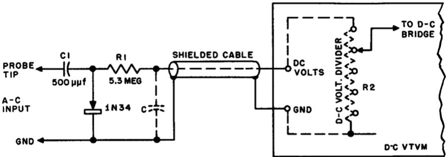
Fig. 6-15. Shunt-type crystal-diode peak-indicating rectifying circuit widely used in probe form for measuring sine-wave radio-frequency voltages with a d-c vtvm. Rectifying circuits of this type, constructed in probe form, can usually be used up to 100 to 250 mc with an accuracy of  $\pm 10\%$ . Observe the simplicity of this arrangement—no heater-supply wiring, or contact-potential bucking-voltage circuit is required as it is when a tube type diode rectifier is employed.
