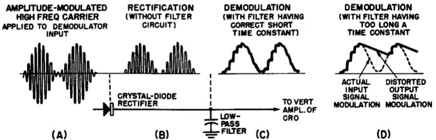
Fig. 7-2. Principle of operation of the diode demodulator, and effect of the time constant of the filter circuit on the waveform of its output voltage.
