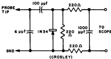
LOW IMPEDANCE; RELATIVELY LOW SENSITIVITY. SHUNT RECTIFIER. SCOPE CABLE PARTIALLY ISOLATED.
