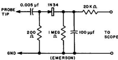
LOW IMPEDANCE; RELATIVELY LOW SENSITIVITY. SERIES RECTIFIER. SCOPE CABLE ISOLATED.
