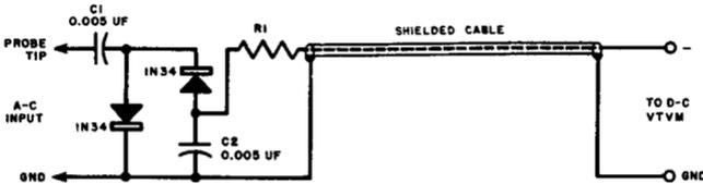
Fig. 6-18. A basic peak-to-peak indicating probe employing two crystal diodes in a voltage-doubler rectifying circuit. This arrangement is very useful in tv troubleshooting to measure the peak-to-peak voltage values of complex waveforms in order to compare them with the specified values.
