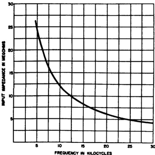
Fig. 2-4. The input impedance of a typical capacitance-divider type high-voltage probe decreases as the frequency increases.
