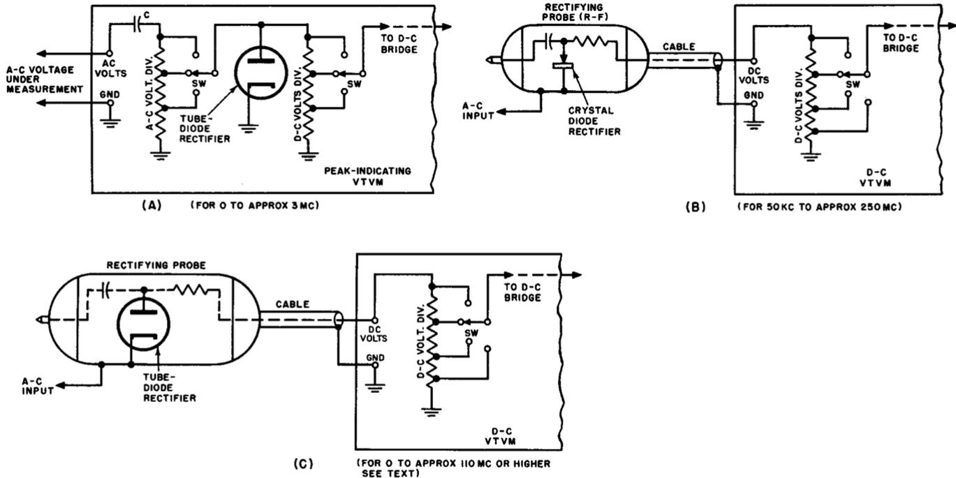
Fig. 6-2. Typical rectifier arrangements employed with peak-indicating type vtvm's. (A) Built-in tube-diode rectifier used for low and medium-frequency a-c voltage measurements. (B) Crystal diode rectifier, arranged in the form of an accessory exterior probe, used for high-frequency a-c voltage measurements to approximately 250 mc. (C) Alternate type of probe rectifier that employs a diode tube.
