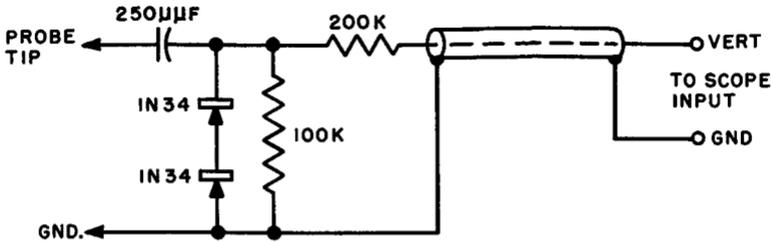
Fig. 7-15. By employing two crystal diodes in series, the voltage-handling capability of the demodulator probe is doubled.
