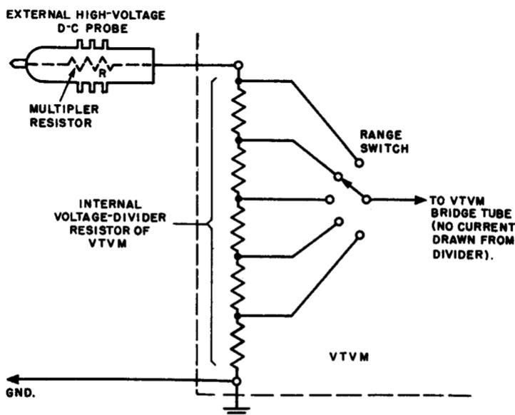
Fig. 1-4. The measuring tube of a vtvm draws no current, and hence the meter in the vtvm really indicates the voltage drop at any selected point along the internal voltage-divider resistor, instead of measuring the current through the instrument, as does a vom. For convenience, the value of the external multiplier resistor in the the resistive high-voltage probe can be selected to multiply each of the vtvm voltage ranges by a convenient decimal factor, such as 100.
