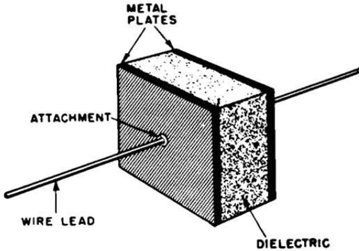
Fig. 3-2. Basic capacitor construction.
