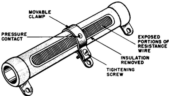
Fig. 1-2. Adjustable resistor.
