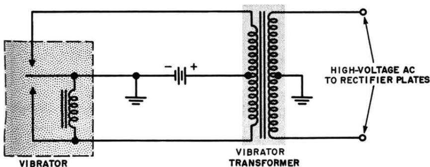
Fig. 6-9. Vibrator transformer hook-up.
