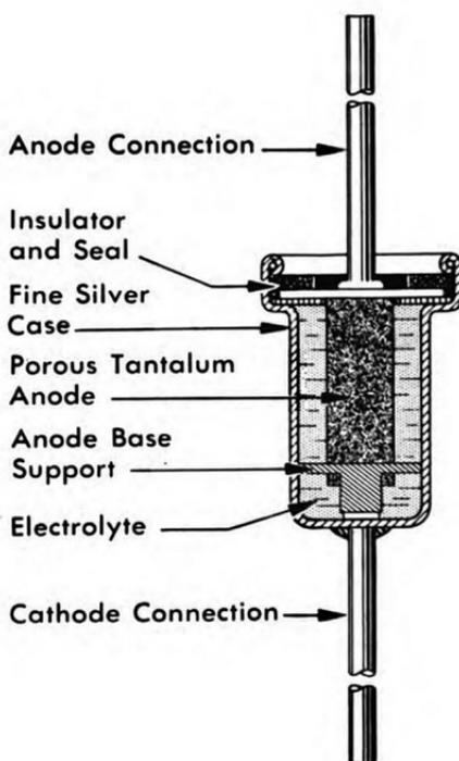
Fig. 4-5. Construction of tantalum electrolytic capacitor. Courtesy Fansteel Metallurgical Corp.
