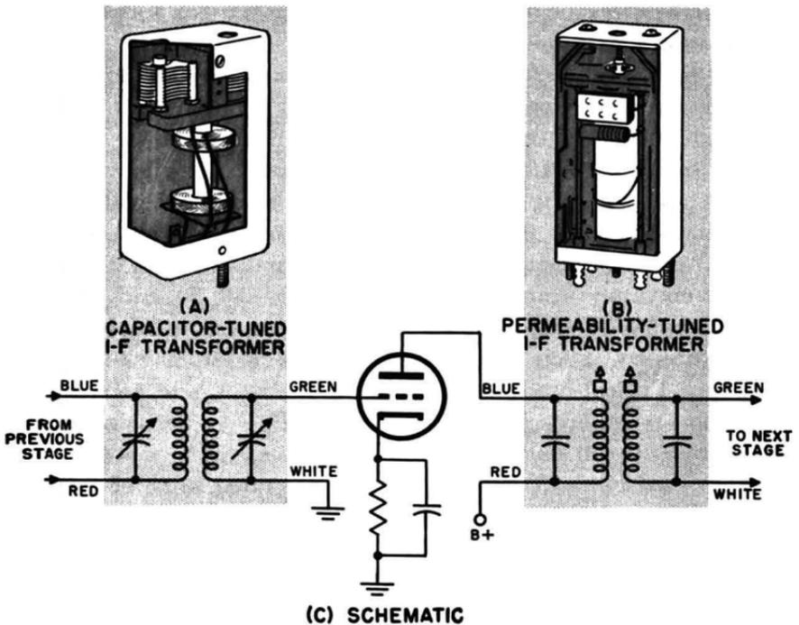
Fig. 6-12. I-f transformers. (A) Capacitor tuned. (B) Permeability tuned. (C) Basic circuits.
