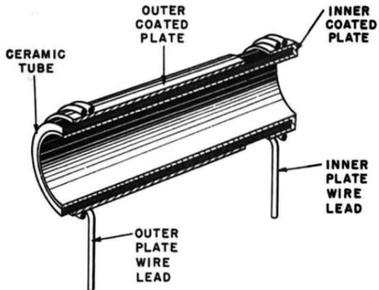
Fig. 4-7. Tubular ceramic capacitor, simplified construction diagram.
