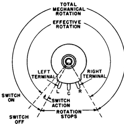
Fig. 2-5. Variable resistor terminology.
