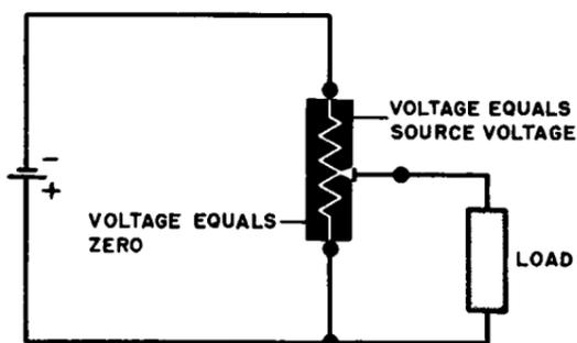
Fig. 2-11. Potentiometer connection.
