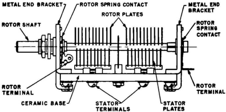
Fig. 4-9. Variable capacitor construction. Courtesy Hammarlund Mfg. Co., Inc.
