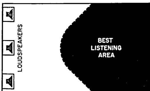
Fig. 29. Best position for loudspeakers with three-channel stereophonic is along one of the shorter walls of a listening room.
