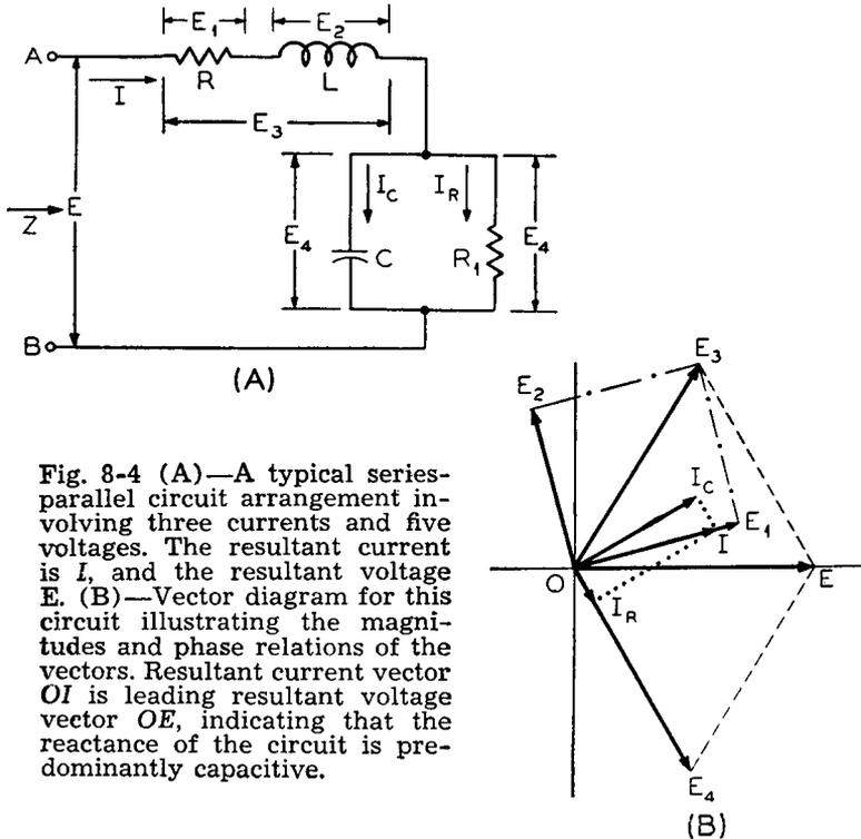
Fig. 8-4 (A)—A typical series-parallel circuit arrangement involving three currents and five voltages. The resultant current is  $I$ , and the resultant voltage  $E$ . (B)—Vector diagram for this circuit illustrating the magnitudes and phase relations of the vectors. Resultant current vector  $OI$  is leading resultant voltage vector  $OE$ , indicating that the reactance of the circuit is predominantly capacitive.
