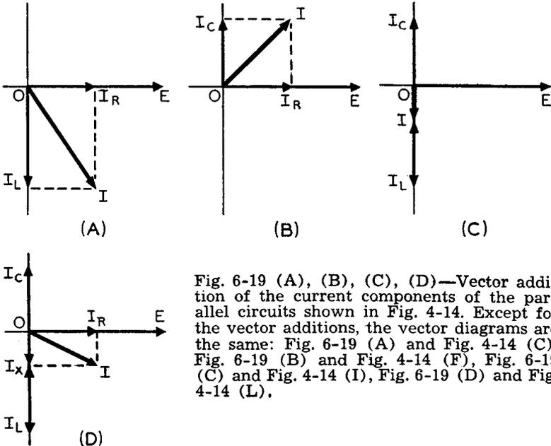
Fig. 6-19 (A), (B), (C), (D)—Vector addition of the current components of the parallel circuits shown in Fig. 4-14. Except for the vector additions, the vector diagrams are the same: Fig. 6-19 (A) and Fig. 4-14 (C), Fig. 6-19 (B) and Fig. 4-14 (F), Fig. 6-19 (C) and Fig. 4-14 (I), Fig. 6-19 (D) and Fig. 4-14 (L).
