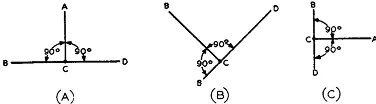
Fig. 1-5 (A), (B), (C)—Three examples of perpendicular lines. When two lines meet and form right angles, they are said to be perpendicular to each other.
