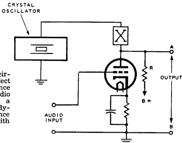
Fig. 8-17—A p-m circuit in which the effect of a variable resistance is made by an audio input signal and a triode tube. The dynamic plate resistance of the tube varies with audio input.
