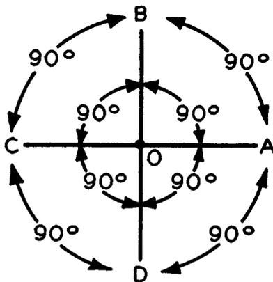
Fig. 1-4—Two diameters  $AC$  and  $BD$  perpendicular to each other divide a circle into quarters, each of which embraces  $90^\circ$  degrees.
