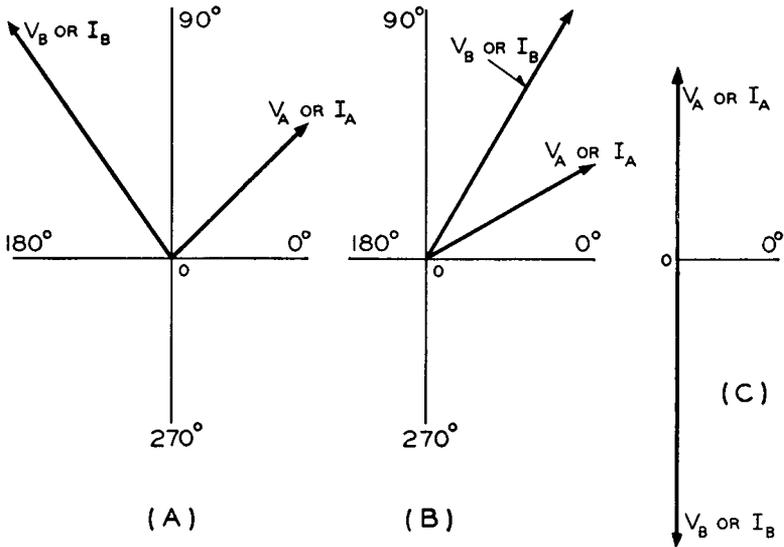
Fig. 4-5—Examples of two voltage vectors on a single set of axes. In (A), (B), and (C) the vectors can represent voltage or current. In all parts vector  $OV_B$  (or  $OI_B$ ) is greater in magnitude and leads vector  $OV_A$  (or  $OI_A$ ). Though the four coordinate lines are not shown in (C), the relative phase of each vector and the phase difference between them are readily apparent.
