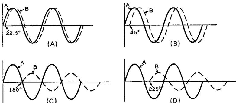
Fig. 4-2—Sine waves of the same amplitude are illustrated in (A) and (B). (A) indicates a phase difference of  $22.5^\circ$  and (B) indicates a phase difference of  $45^\circ$ . In each case A is leading B, or B is lagging A. In (C) and (D) wave A is still leading wave B, even though the amplitude of wave A is twice that of wave B. The phase difference of  $180^\circ$  in (C) and  $225^\circ$  in (D) remain constant throughout.
