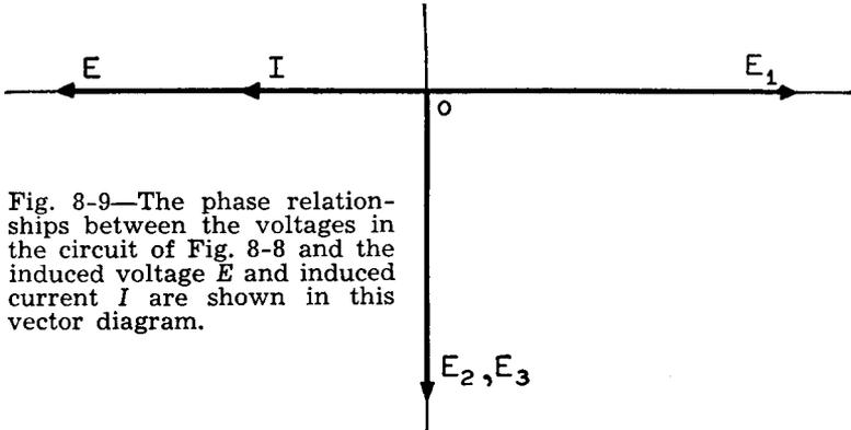
Fig. 8-9—The phase relationships between the voltages in the circuit of Fig. 8-8 and the induced voltage  $E$  and induced current  $I$  are shown in this vector diagram.
