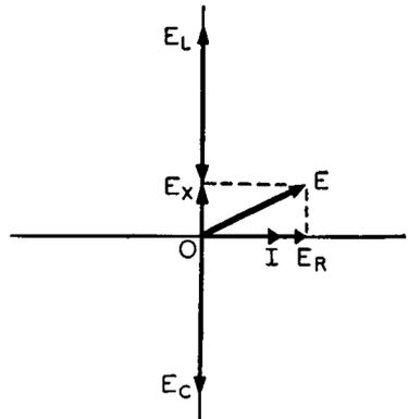
the capacitive reactance let us refer to the vector diagram of Fig. 6-18. This vector diagram is exactly the same as that one of Fig. 4-13. The process of vector addition of the three individual voltages is quite simple. Since three voltages are present, two separate vector additions have to be made. We can start with any two voltage vectors we desire,
