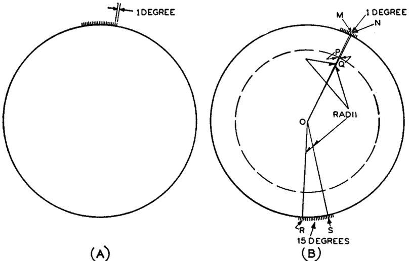
Fig. 1-2—(A) A circle is usually divided into 360 divisions of 1 degree each. (B) Any line from the center to the circumference of the circle is called a radius. The angle embraced by radii  $OP$  and  $OQ$  is the same as that embraced by radii  $OM$  and  $ON$ .
