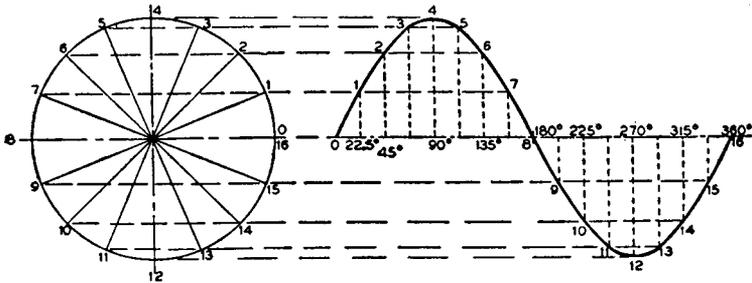
Fig. 3-2—Illustration of how the rotating armature of the two-pole a-c generator of Fig. 3-1 develops a sine wave output during one revolution of the armature.
