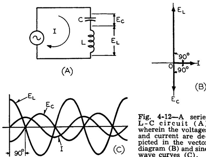
Fig. 4-12—A series L-C circuit (A) wherein the voltages and current are depicted in the vector diagram (B) and sine wave curves (C).
