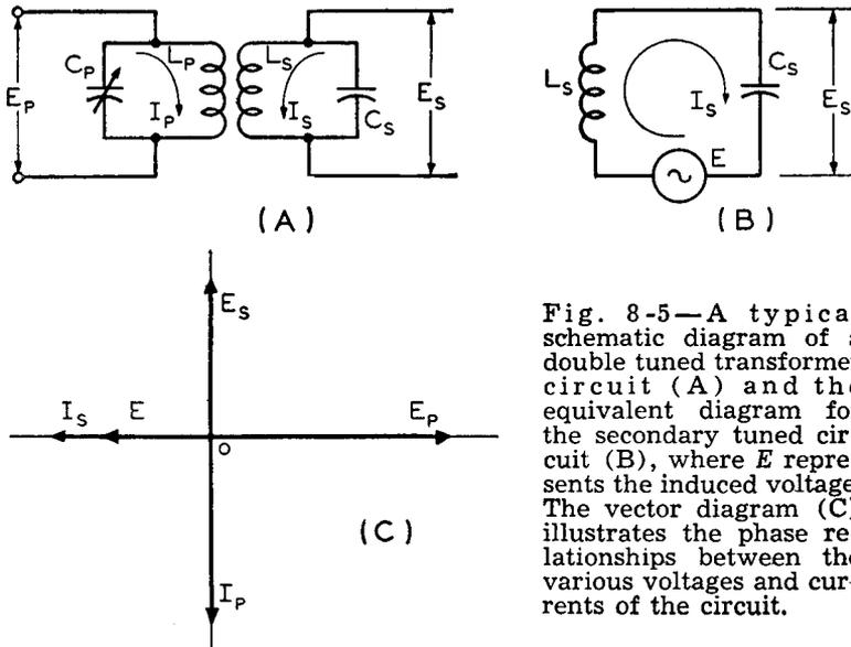
Fig. 8-5—A typical schematic diagram of a double tuned transformer circuit (A) and the equivalent diagram for the secondary tuned circuit (B), where  $E$  represents the induced voltage. The vector diagram (C) illustrates the phase relationships between the various voltages and currents of the circuit.
