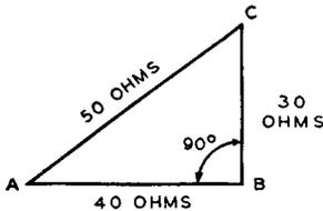
Fig. 6-15—Computations to determine the magnitude of the impedance or components of a series circuit are based on this triangle: given any two sides, the third one can be simply computed.
