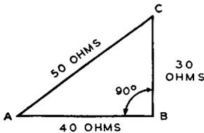
Fig. 6-15—Computations to determine the magnitude of the impedance or components of a series circuit are based on this triangle: given any two sides, the third one can be simply computed.
