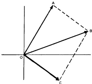
Fig. 7-1—A parallelogram is constructed to subtract one vector from another, but the minuend, in this case  $OB$ , is used as a diagonal and not as a side of the parallelogram, as both quantities are in addition. Vector  $OC$  is the resultant of this subtraction.
