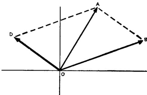
line of equal length *from* the initial point of the vector, then this new line will represent the resultant vector of the two vectors  $OA$  and  $OB$  when the subtraction is reversed; that is when vector  $OB$  is subtracted from vector  $OA$ . In other words this extended vector will be the same as the resultant vector  $OD$  in Fig. 7-2.
