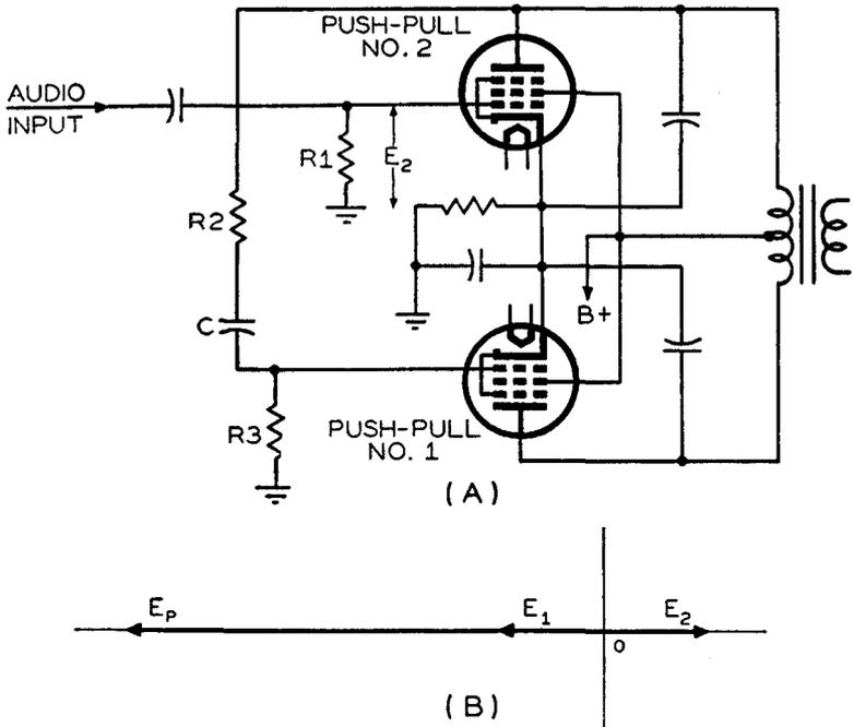
Fig. 8-7—The push-pull circuit (A) uses push-pull tube No. 2 as the phase inverter. Here the audio is impressed directly across the grid of tube No. 2 (B) illustrates the equal but 180° out-of-phase voltages  $E_1$  and  $E_2$  which are applied to tubes No. 1 and No. 2, respectively.
