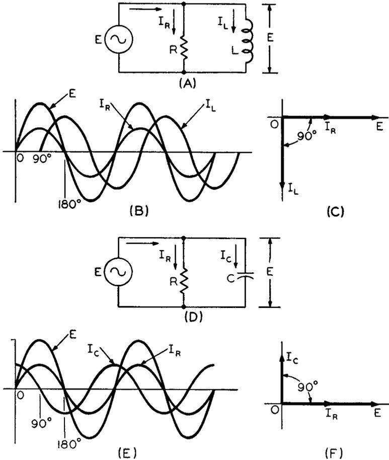
Fig. 4-14 (A) to (L)—The vector diagrams and accompanying sine waves of the different parallel circuits are included to show the magnitude and phase relations of their voltages and currents. A quick comparison of
