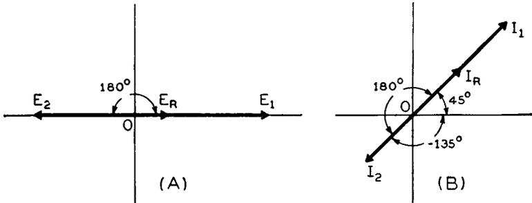
Fig. 6-2 (A), (B)—When vectors opposite in phase are added, the resultant vector is smaller in magnitude than either vector being added and has the phase angle of the larger of the two.
