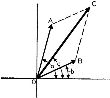
Fig. 6-5—The addition of two vectors  $OA$  and  $OB$  by the parallelogram method. These two vectors are chosen as adjacent sides of a parallelogram and  $OACB$  is drawn. The diagonal from the origin  $O$  of the coordinate system to the opposite angle of the parallelogram ( $C$ ) is the resultant vector  $OC$  of the addition.
