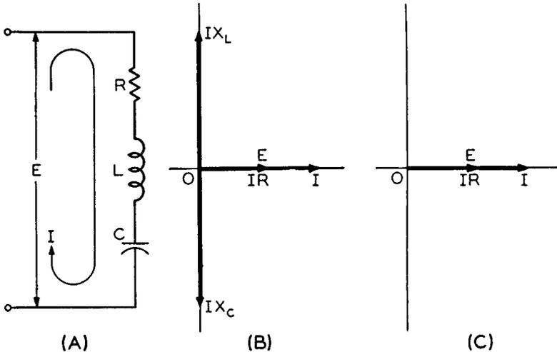
Fig. 8-1—The three voltages and the current of the series resonant circuit in (A) are laid out in vector form (B) to correspond to the circuit conditions, and by vector addition of the voltages the resultant voltage vector  $OE$ , which equals the voltage drop across the resistance, is obtained (C).
