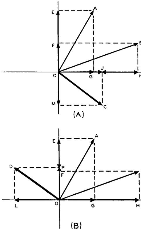
Fig. 7-3—In (A) we have subtraction by the resolution method of the vectors of Fig. 7-1. The resultant vector is  $OC$  which checks with vector  $OC$  in Fig. 7-1. In (B) subtraction by the resolution method of the vectors of Fig. 7-2 yields resultant vector  $OD$  which checks with vector  $OD$  of Fig. 7-2.
