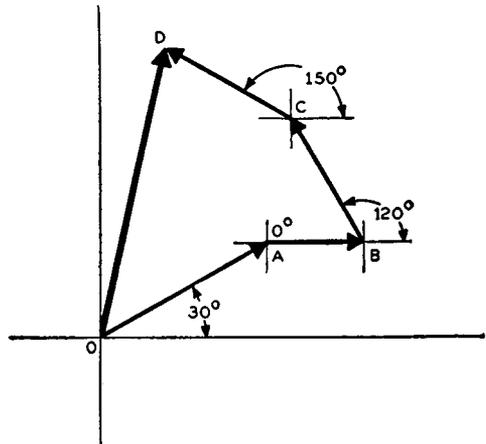
vector diagram for their addition is illustrated in Fig. 6-8, where the vectors are all drawn to a scale of 1 inch equal to 10 volts. Vector OA is first drawn at a phase angle of 30 degrees with its initial point starting at the origin of the main coordinate system. Then the tail of vector AB is drawn from the head of vector OA at an angle of zero degrees from point A. Then from the head of vector AB the tail of
