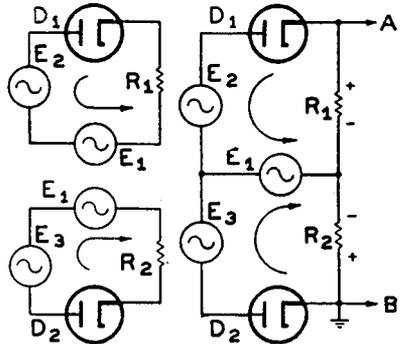
in one case one of the voltages is leading the current and in the other case the voltage is lagging the current by  $90^\circ$ . This also means that one half of the secondary voltage drop is leading voltage  $E_1$  by  $90^\circ$  and the other half lagging voltage  $E_1$  by  $90^\circ$ . All of which is simply indicated in the revised vector diagram of Fig. 8-9 as appearing in Fig. 8-10, in which vector  $OE_3$  of the previous vector diagram has been shifted  $180^\circ$ .
