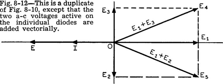
and  $E_1$  across diode  $D_2$  and vector  $OE_5$  represents the resultant vector of the vector addition of  $E_2$  and  $E_1$ . Since side  $E_1$  is common to both rectangles formed by the vector additions and since  $E_3$  and  $E_2$  are equal in magnitude and  $E_3$  is  $90^\circ$  leading and  $E_2$   $90^\circ$  lagging  $E_1$ , from resultant vectors  $OE_4$  and  $OE_5$  are equal in magnitude, causing the same current to flow in each diode circuit.
