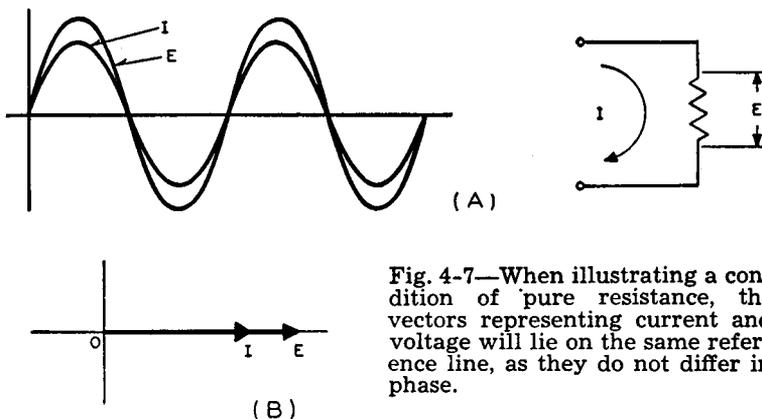
Fig. 4-7—When illustrating a condition of pure resistance, the vectors representing current and voltage will lie on the same reference line, as they do not differ in phase.
