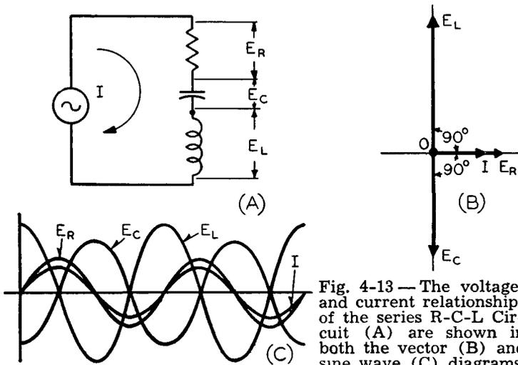
Fig. 4-13 — The voltages and current relationships of the series R-C-L Circuit (A) are shown in both the vector (B) and sine wave (C) diagrams.
