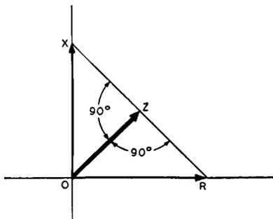
Fig. 5-4—Component parts of parallel impedance vector  $OZ$  can be found by drawing a straight line from the vertical to the horizontal axis that is perpendicular to vector  $OZ$  at  $Z$ . Line  $OR$  is the resistive component, and  $OX$  the reactive component.
