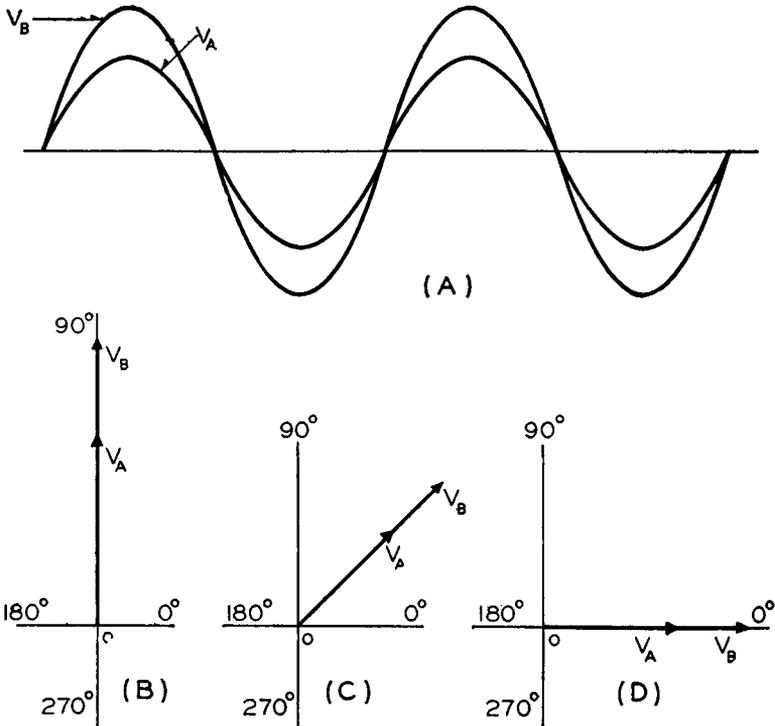
Fig. 4-6— $V_B$  and  $V_A$  (A) represent two waves which are of different amplitude but of the same phase. In vector representations (B) and (C) of this relationship, one vector must be superimposed on the other, and because of their different magnitudes, one is longer. Each vector diagram represents a different instant of time. (D) shows the common method of expressing the practical values of curves A and B vectorially.
