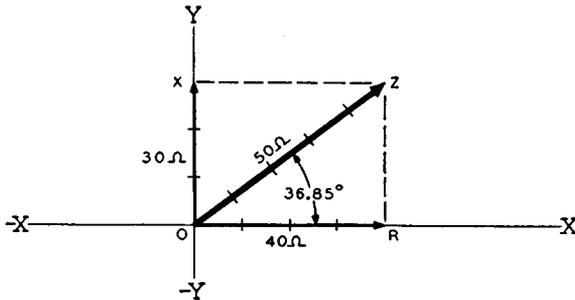
Fig. 5-2—A typical impedance vector of a series circuit shown being resolved into its resistive and reactive components, the reactive component being predominantly inductive.
