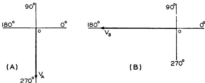
Fig. 4-3—The scale for both voltage vectors is 10 volts to the inch. Voltage  $V_A$  being 10 volts is a vector one inch long as indicated in (A). Voltage  $V_B$  being 15 volts is a vector  $1\frac{1}{2}$  inches long as indicated in (B). Both vectors are drawn with respect to their relative phase.
