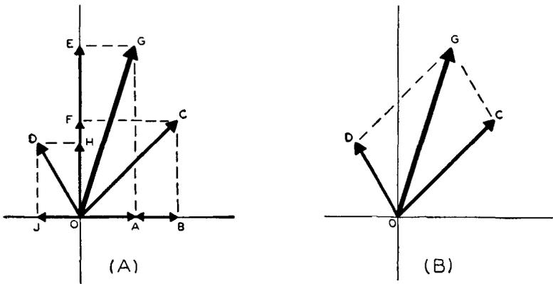
Fig. 6-10—Addition of two vectors by the resolution method (A) showing that the horizontal resultant component  $OA$  can be smaller than the largest single component  $OB$  making up the resultant. In (B) the vectors are added by the parallelogram method, and the same resultant vector is obtained.
