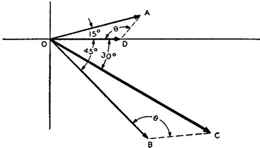
Fig. 7-5—Vector multiplication involving current vector  $OA$  with a positive phase angle and impedance vector  $OB$  with a negative phase angle. The resultant voltage vector is seen to have a negative phase angle.
