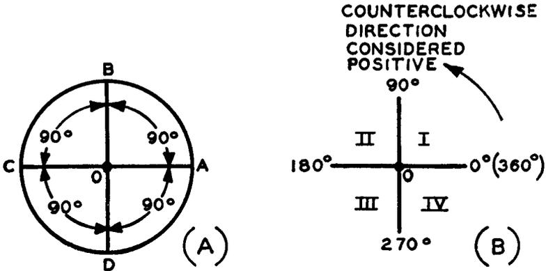
Fig. 2-2 (A)—Coordinate lines within a circle divide it into four segments of 90 degrees each. (B)—In the coordinate system the direction of rotation and the quadrant designations have been standardized, so that counterclockwise rotation is considered positive.
