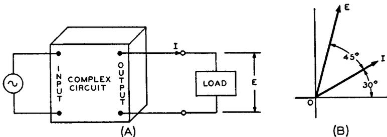
Fig. 4-15—The current  $I$  flowing out of the complex network (A) is a combination of the individual currents within the network. The impedance load has an effective reactance that is predominantly inductive and equals the resistive component of the load. Therefore the voltage  $E$  across the load leads the current  $I$  flowing through it by  $45^\circ$ , as seen in the vector diagram (B).
