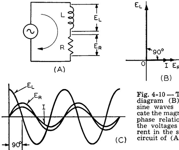
Fig. 4-10 — The vector diagram (B) and the sine waves (C) indicate the magnitude and phase relationships of the voltages and current in the series R-L circuit of (A).
