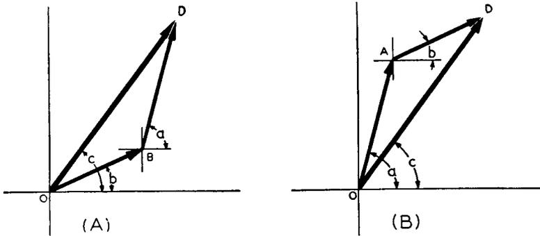
Fig. 6-7—The head-to-tail method of vector addition may be started with either of the two vectors to be added. In (A) the supplementary set of coordinates is drawn at the terminal point of vector  $OB$  and in (B) at the terminal point of  $OA$ . The resultant vector in either case is  $OD$ .
