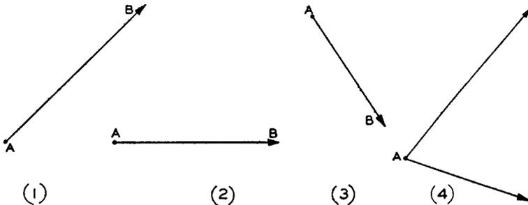
Fig. 1-1—Typical vectors illustrating different magnitudes and directions.
