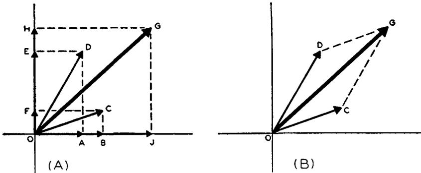
Fig. 6-9—Two vectors  $OC$  and  $OD$  are added by the resolution method in (A). Horizontal component  $OJ$  and vertical component  $OH$  combine to give resultant vector  $OG$ . As a check, the vectors are added by the parallelogram method (B) with the same result.
