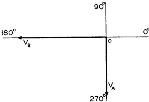
Fig. 4-4—To facilitate the comparison of magnitude and phase, vectors  $OV_A$  and  $OV_B$  of the two separate coordinate systems of Fig. 4-3 are shown on a single coordinate system.
