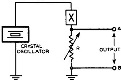
Fig. 8-15—A simple phase modulator circuit in which the reactance  $X$  and the resistance  $R$  represent a time delay network that imparts a phase change to the crystal oscillator frequency. The variable resistance  $R$  can alter the phase of the crystal frequency.
