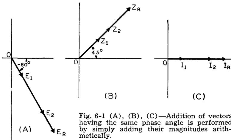
Fig. 6-1 (A), (B), (C)—Addition of vectors having the same phase angle is performed by simply adding their magnitudes arithmetically.
