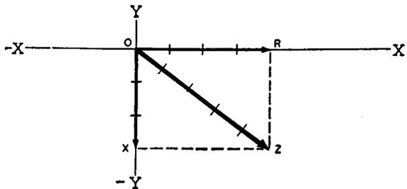
found to be equal to 1 inch. This means that the magnitude of resistance is equal to 40 ohms since the original scale was set for 1 inch to equal 40 ohms. Similarly the length of  $OX$  is found to be equal to  $\frac{3}{4}$  inch, which means that the magnitude of the reactive component under the same scale, is equal to 30 ohms.
