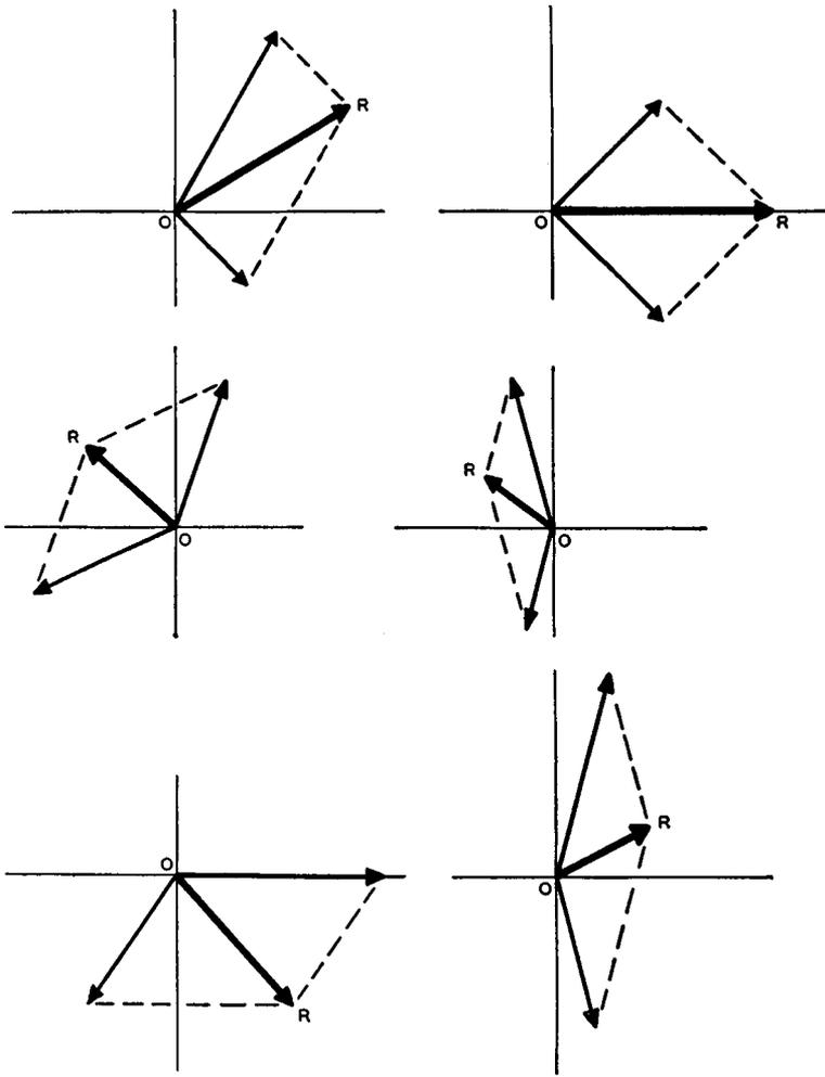
Fig. 6-6—A number of examples of the addition of two vectors by the parallelogram method. The magnitude of the resultant vector relative to that of its components will vary, depending upon the phase angle of the component vectors.
