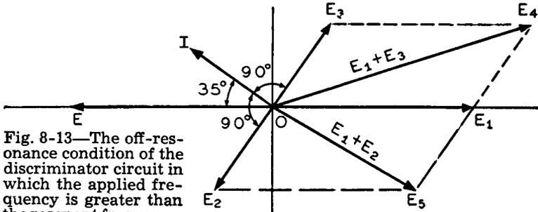
Fig. 8-13—The off-resonance condition of the discriminator circuit in which the applied frequency is greater than the resonant frequency.
