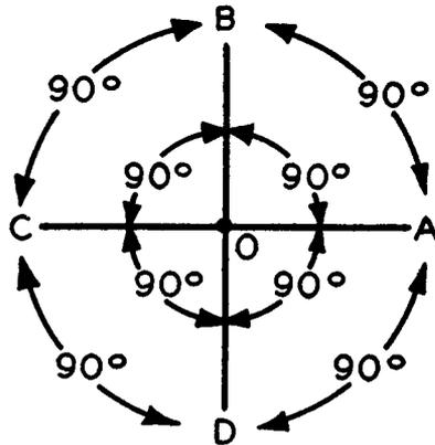
Fig. 1-4—Two diameters  $AC$  and  $BD$  perpendicular to each other divide a circle into quarters, each of which embraces  $90^\circ$  degrees.
