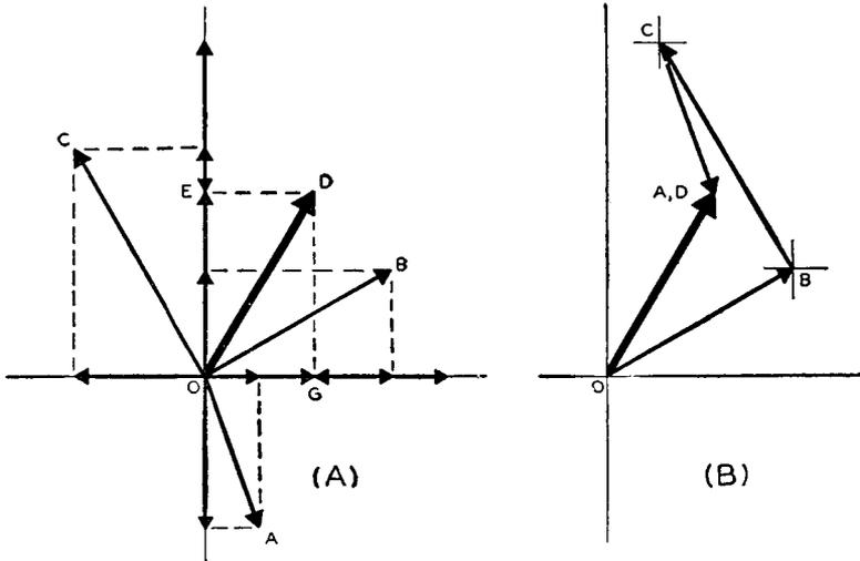
Fig. 6-11—Three vectors  $OA$ ,  $OB$ , and  $OC$  are added by the resolution method in (A) to form resultant vector  $OD$ . This resultant vector checks with the results of the head-to-tail method in (B).
