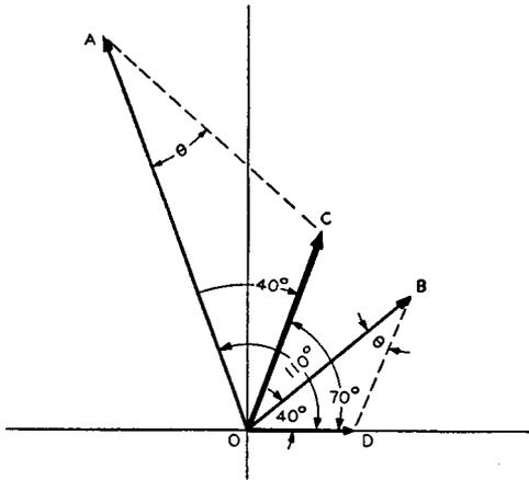
Fig. 7-6—Vector division of voltage vector  $OA$  by current vector  $OB$  results in impedance vector  $OC$ . The scale used is one inch to two units. The geometric method employed is discussed in the text.
