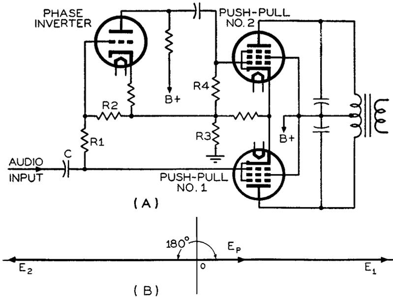
Fig. 8-6—(A) is a typical push-pull circuit using a separate tube as a phase inverter. The vector diagram (B) illustrates that voltage vector  $OE_1$  of push-pull tube No. 1 is equal in magnitude but  $180^\circ$  out of phase with voltage vector  $OE_2$ .
