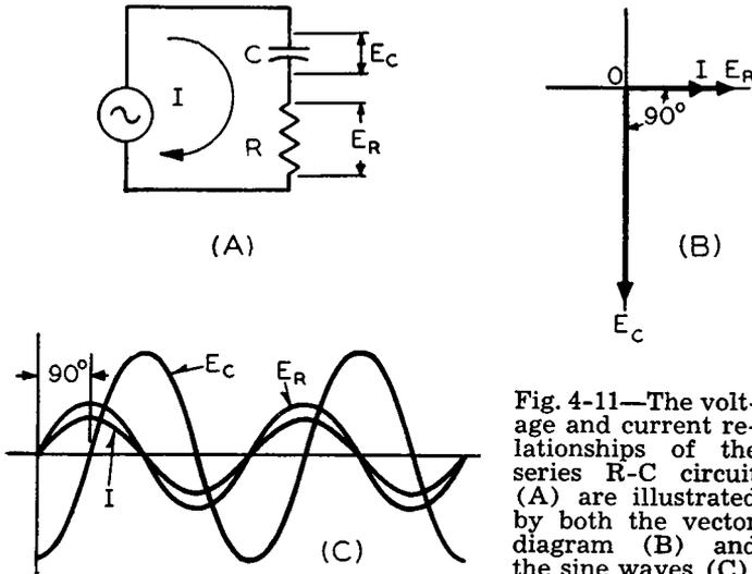
Fig. 4-11—The voltage and current relationships of the series R-C circuit (A) are illustrated by both the vector diagram (B) and the sine waves (C).
