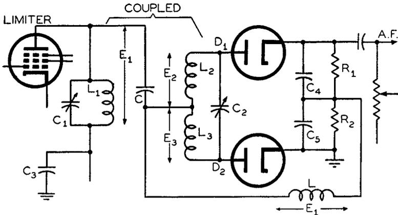
Fig. 8-8—A typical discriminator circuit as used in f-m receivers where the two diodes can be separate tubes or a duo-diode tube.
