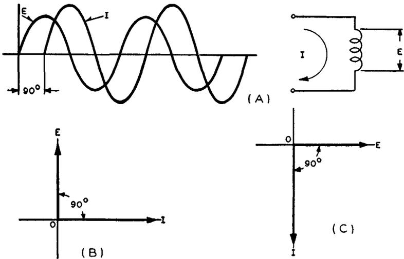
Fig. 4-8—The voltage and current curves for a pure inductance (A) can be shown vectorially in two ways, (B) and (C). In the former, the current  $I$  is considered the reference quantity and in the latter the voltage  $E$  is located on the reference line. In both diagrams the voltage is leading the current by 90 degrees.
