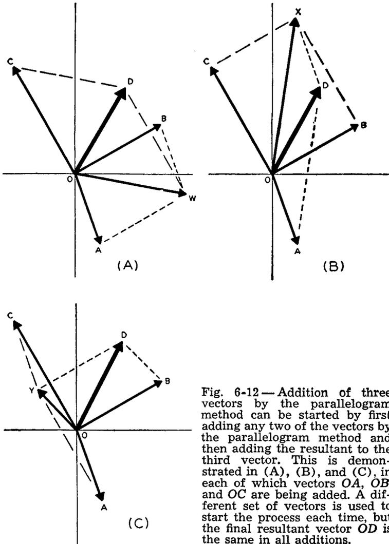
Fig. 6-12—Addition of three vectors by the parallelogram method can be started by first adding any two of the vectors by the parallelogram method and then adding the resultant to the third vector. This is demonstrated in (A), (B), and (C), in each of which vectors  $OA$ ,  $OB$ , and  $OC$  are being added. A different set of vectors is used to start the process each time, but the final resultant vector  $OD$  is the same in all additions.
