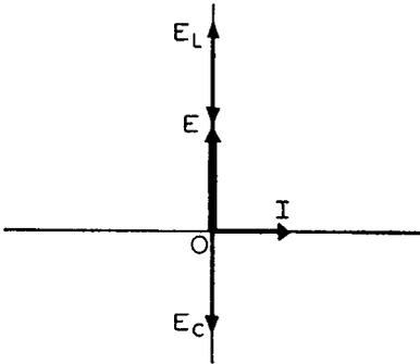
Fig. 6-17—Vector addition of the voltage components across a series L-C circuit of Fig. 4-12 yields a resultant voltage vector  $OE$  which is predominantly inductive since the inductive reactance is larger than the capacitive. Consequently, the resultant voltage leads the current through the circuit by  $90^\circ$ .
