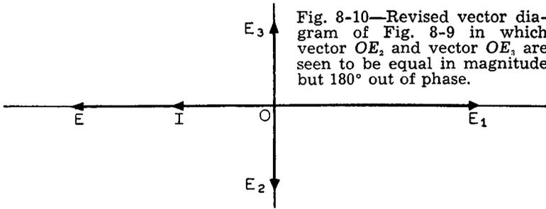
Fig. 8-10—Revised vector diagram of Fig. 8-9 in which vector  $OE_2$  and vector  $OE_3$  are seen to be equal in magnitude but  $180^\circ$  out of phase.
