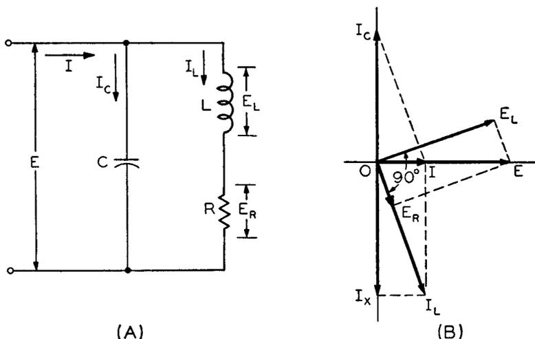
Fig. 8-3 (A)—A true parallel L-C circuit has inherent resistance in the inductance. (B) The vector addition of the different voltages and currents, where vector  $OE$  is the resultant voltage vector and vector  $OI$  the resultant current vector.
