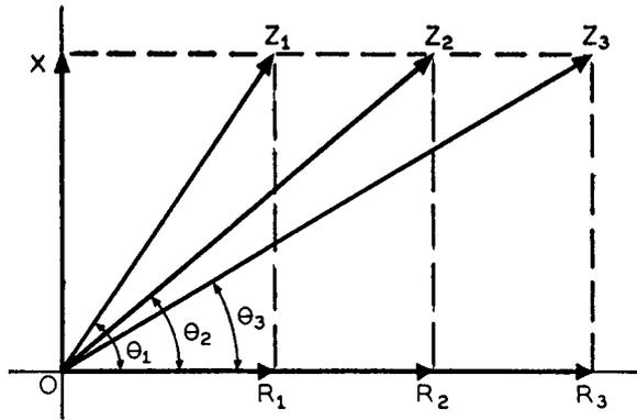
Fig. 8-16—From this vector diagram it is readily seen that by varying values of resistance ( $R_1$ ,  $R_2$ , and  $R_3$ ) the phase angle of the system changes ( $\theta_1$ ,  $\theta_2$ ,  $\theta_3$ ).
