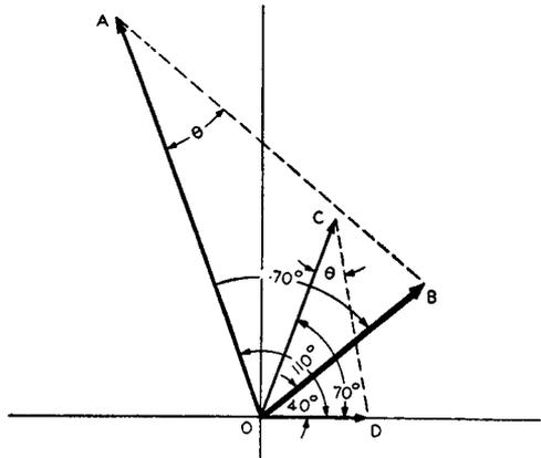
Fig. 7-7—To check the accuracy of the diagram of Fig. 7-6, it is assumed that the impedance vector  $OC$  and voltage vector  $OA$  are known, and the current vector  $OB$  is found by vector division.
