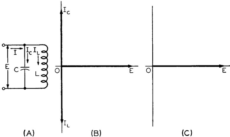
Fig. 8-2—(A) The ideal parallel L-C resonant circuit has the two branch currents  $I_C$  and  $I_L$  equal. They are shown by equal but  $180^\circ$  out-of-phase current vectors  $OI_C$  and  $OI_L$  in (B) with respect to the voltage  $E$  across the circuit. Addition of these two currents (C) ideally results in zero current.
