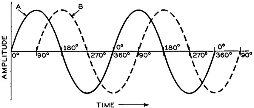
Fig. 4-1—Sine waves A and B maintain a constant phase difference of 90 degrees set when voltage source B started functioning one-quarter cycle later than voltage source A. Here A is said to be leading B or, conversely, B is lagging A.
