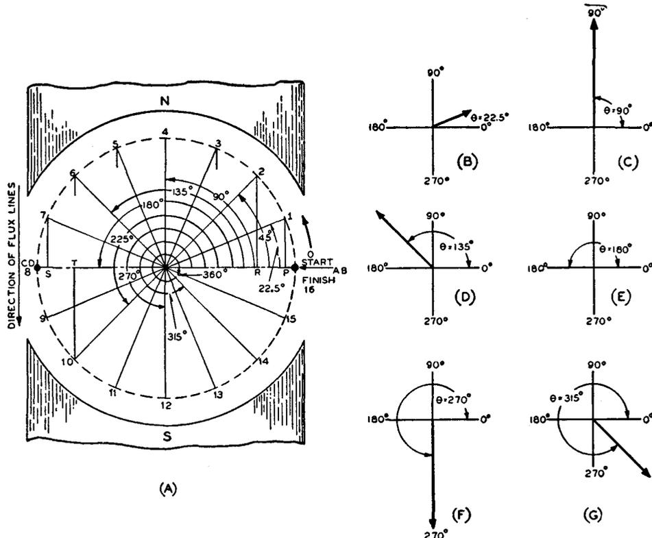
Fig. 3-3—In (A) is the graphical representation of the coil side movement in the generator of Fig. 3-1 (B). Vectorial representations of the instantaneous voltage developed by an a-c generator at six different angular positions of the armature between 22.5 degrees and 315 degrees are shown in Figs. 3-3 (B) to (G) inclusive.
