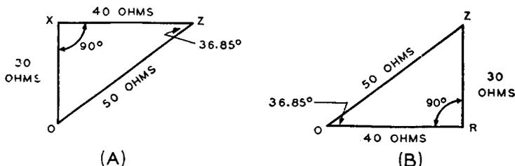
Fig. 6-14—The rectangle of Fig. 6-13 can be split into two right triangles, each of which has  $OZ$  equal to an impedance of 50 ohms at a phase angle of  $36.85$  degrees and the 30- and 40-ohm sides equal to the reactive and resistive components, respectively.
