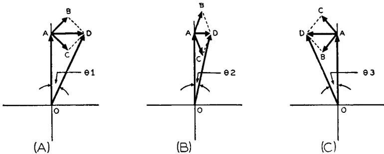
Fig. 8-19—The double sideband vectors  $AD$  of the a-m signals of Fig. 8-18 have been shifted in phase by  $90^\circ$ . The final resultant vectors,  $OD$  in this case, are seen to be varying in phase with respect to vector  $OA$ .
