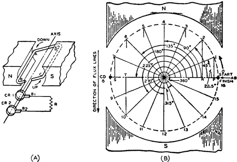
Fig. 3-1 (A)—A basic a-c generator in which the coils rotate past the pole pieces in a counterclockwise direction with an alternately positive and negative polarity. (B)—A head-on view of the generator reveals how the coil sides in conjunction with the parallel lines of flux provide a zero-voltage reference line. During the armature rotation a varying vertical displacement also occurs. The center of the circle is point  $O$ .
