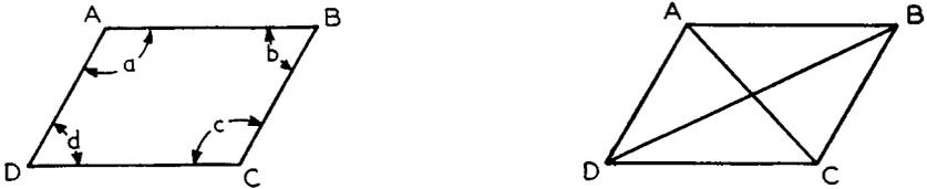
Fig. 6-3 (left)—A four-sided figure that has its opposite sides equal and parallel to each other and its opposite angles equal is called a parallelogram. Fig. 6-4 (right)—In a parallelogram the diagonal joining the smaller angles,  $B$  and  $D$ , is longer than the diagonal joining the larger angles,  $A$  and  $C$ .
