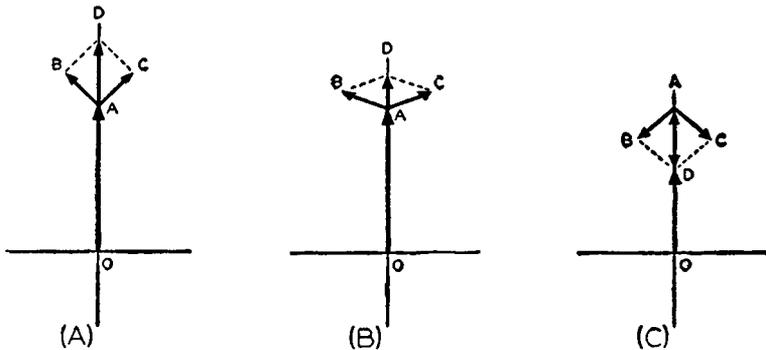
Fig. 8-18—Vector diagrams of an a-m signal. In (A) and (B) the double sideband component vector  $AD$  is in phase with the center frequency component vector  $OA$ , making the resultant vector  $OD$  greater than  $OA$ . In (C) vector  $AD$  is  $180^\circ$  out of phase with vector  $OA$ , making the resultant vector  $OD$  smaller than  $OA$ .
