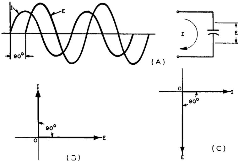
Fig. 4-9—Voltage and current sine waves for a pure capacitance (A). For vector representation two diagrams can be drawn, as in (B) and (C). In (B) the voltage  $E$  is the reference quantity, and in (C) current  $I$  is the reference quantity. In each case the current is leading the voltage by 90 degrees.
