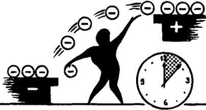
**POWER FORMULA** — Electric power used in a resistance equals the voltage across the resistance terminals times the current flow through the resistance. It is also equal to the current squared times the resistance or, the voltage squared divided by the resistance.
