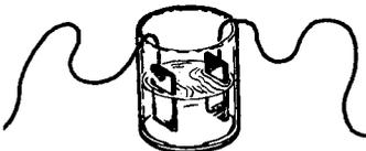
**CHEMICAL ACTION** — Electricity produced by chemical reaction in an electric cell.
