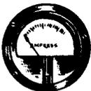
6. AMMETER — Meter used to measure amperes.
