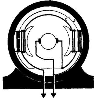
**MOTOR REVERSAL** — The direction of rotation of a DC motor can be reversed by reversing the field connections or by reversing the armature connections.
