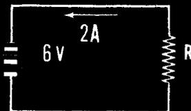
A third use for Ohm's law is to find the voltage when the current and resistance are known. To find the voltage across a resistance, the current is multiplied by the resistance.
