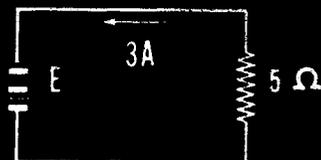
In using Ohm's law, the quantities must always be expressed in the basic units of current, voltage and resistance. If a quantity is given in larger or smaller units, it must first be changed so that it is expressed in amperes, volts or ohms.
