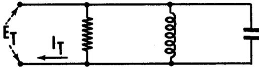
**AC PARALLEL CIRCUIT IMPEDANCE AND POWER FACTOR** — The impedance of an AC parallel circuit is equal to the circuit voltage divided by the total circuit current. The power factor equals the resistive current divided by the total circuit current.
