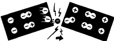
10. ARC DISCHARGE — Electrons crossing over from a negative charge to positive through an arc.
