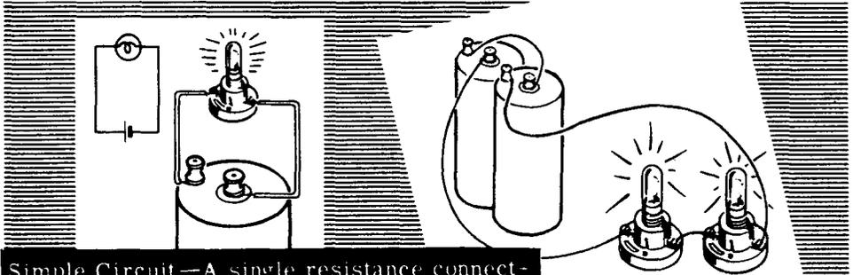
**Simple Circuit**—A single resistance connected across a voltage source.
