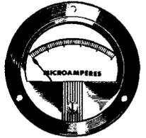
7. **PARALLAX** — Meter reading error due to taking a reading from an angle.
