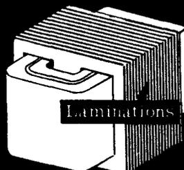
Hysteresis loss depends on the core material used. Each time the AC current reverses in the primary winding, the field in the core reverses its magnetic polarity. This field reversal requires a certain amount of power, resulting in a loss called "hysteresis loss." Some materials, such as silicon steel, change polarity easily, and when these materials are used as the core material, hysteresis loss is reduced to a minimum.
