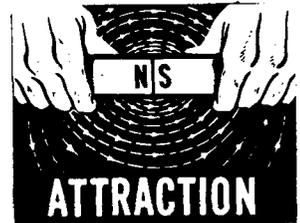
The action of the magnetic poles in attracting and repelling each other is due to the magnetic field around the magnet. As has already been explained, the invisible magnetic field is represented by lines of force which leave a magnet at the north pole and enter it at the south pole. Inside the magnet the lines travel from the south pole to the north pole so that a line of force is continuous and unbroken.
