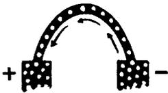
3. CURRENT FLOW — Movement of "free" electrons in the same direction in a material.
