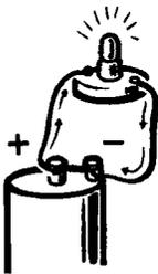
5. CONVENTIONAL CURRENT — Current flow from a positive charge to a negative charge.
