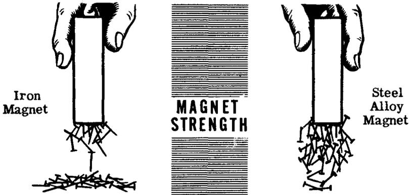
Iron becomes magnetized more easily than other materials but it also loses its magnetism easily so that magnets of soft iron are called temporary magnets. Magnets made of steel alloys hold their magnetism for a long period of time and are called permanent magnets.
