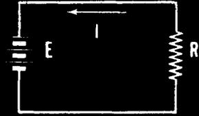
As you know, the current in a circuit increases if the voltage increases and the resistance remains the same. By giving values to  $E$  and  $R$ , you can see how this works. Suppose that  $R$  is 10 ohms and  $E$  is 20 volts. Since the current equals 20 divided by 10, the current is 2 amperes as shown:
