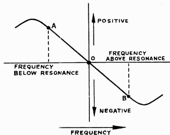
Fig. 5-15.—The S curve represents the typical output characteristic of the discriminator circuit with the output a-f voltage plotted against the instantaneous values of input frequency.
