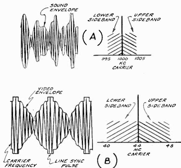
Fig. 1-22.—The sidebands in an a-m sound signal occupy a bandwidth of only about 10 kc, whereas the sidebands in a television signal require a bandwidth of about 8 mc.
