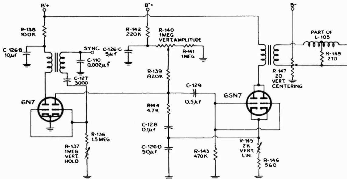
FIG. 9-9.—The vertical deflection circuit of the Stromberg-Carlson model TV10P, Series 10 and 11.
