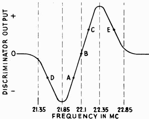
Fig. 4-12.—The discriminator characteristic of the Westinghouse model H-181.
