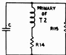
FIG. 6-8.—In this simple network representing the primary of *T2*, *C* is the over-all capacitance in the circuit; *R115* is the grid-leak resistor and together with *R14* the load resistor, reduces the *Q* and makes the response less sharp than it otherwise would be.
