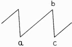
FIG. 11-9.—The current in the sweep coils must have a saw-tooth form, *a-b* being the trace period and *b-c* the retrace.
