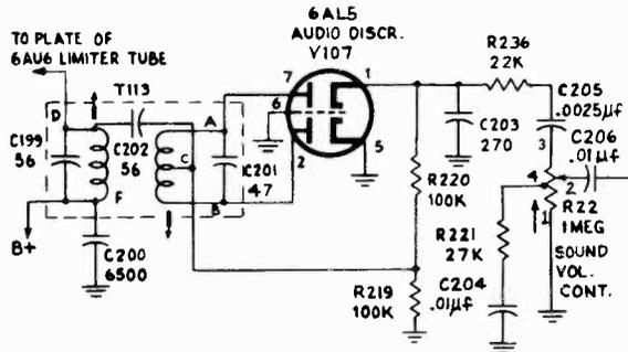
Fig. 5-18.—Discriminator detector used in the Crosley models 307TA, 307TA-50.
