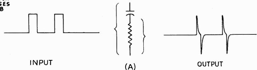
FIG. 8-3, right.—Effect of series resistance-capacitance circuit on input pulses, showing (A) the signal observed when like narrow pulses are applied and (B) when the input consists of two different kinds of pulses.
