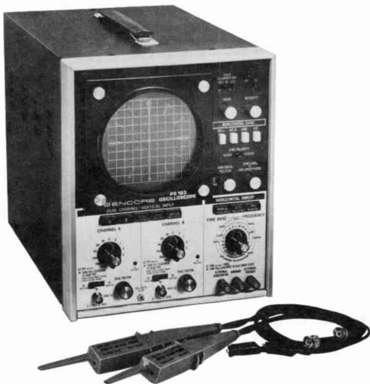
Fig. 1-2. A widely used type of dual-trace oscilloscope.
