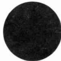
(C) Pattern with STABILITY control set to extreme left-hand end of its range.
