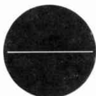
(A) Pattern with STABILITY control set to extreme right-hand end of its range.
