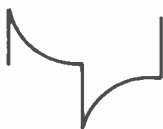
(I) Combination of extensive low-frequency attenuation and leading low-frequency phase shift (differentiation).
