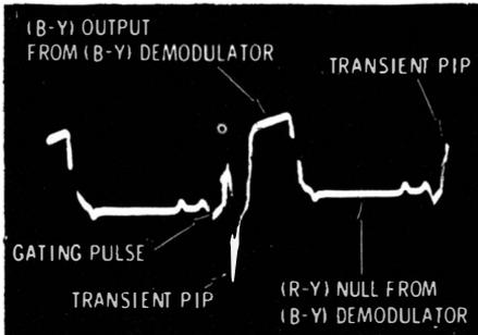
**B—Y demodulator output signal waveform.**
