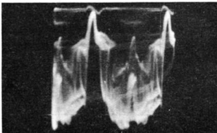
**Appearance of normal signal from pattern generator at detector output.**
