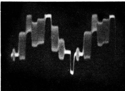
**Color-bar waveform processed through a linear IF amplifier strip.**
