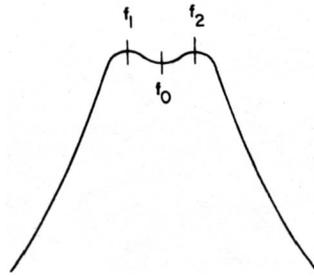
The two resonant frequencies are  $f_1$  and  $f_2$ , and the ringing frequency is  $f_0$ .
