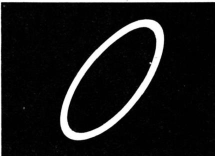
**Typical phase shift and loss of gain.**
