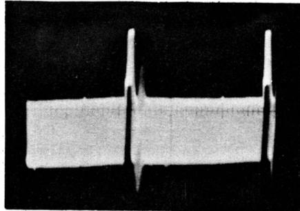
**Waveform distorted by 60-cycle hum voltage.**
