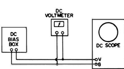
**Test setup for DC response.**
