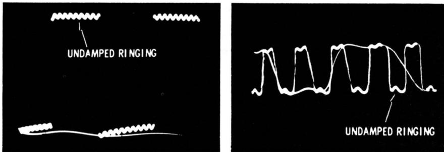
Square waveforms displaying essentially undamped ringing.
