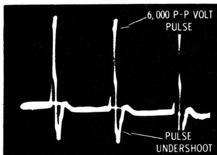
**Waveform at plate of horizontal-output tube.**
