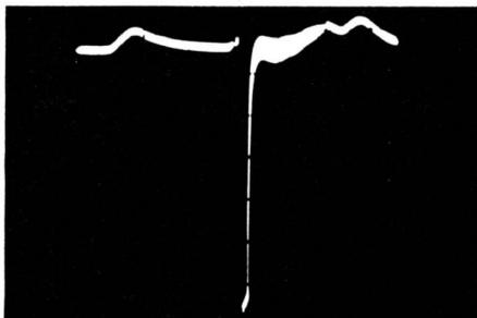
A pulse waveform displayed using conventional sawtooth sweep.
