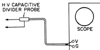
**Connection of a high-voltage, capacitor-divider probe.**
