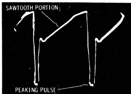
**Waveform at grid of horizontal-output tube.**
