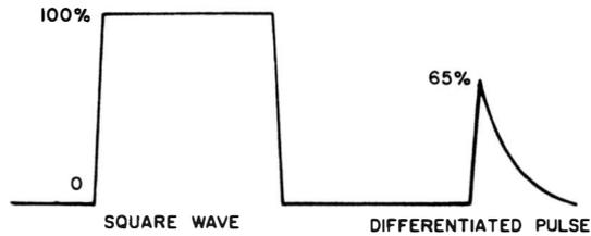
**Input and output of test circuit.**
