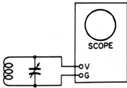
Coil connected across scope vertical input.
