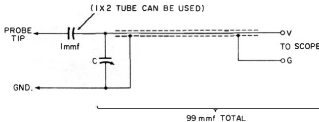
**Configuration of a typical high-voltage, capacitor-divider probe.**
