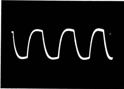
High-frequency attenuation and phase shift.
