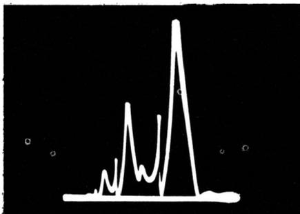
If the receiver has a response curve like this, the pattern will jump up and down rapidly when the pattern generator is tuned across the pass-band of the receiver.
