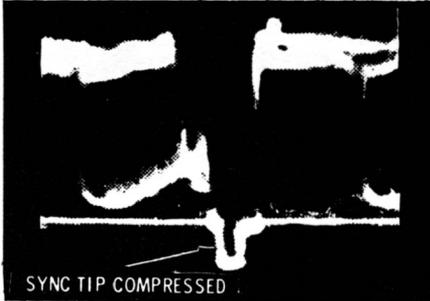
**Horizontal sync pulse with amplitude limiting present.**
