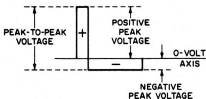
Fig. 2. A pulse waveform.
