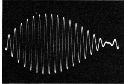
To the technician "in the know" this pattern provides complete information concerning the transformer; even the number of cycles in each ringing group is significant. A group display can be expanded when a triggered sweep is used as shown in Fig. 11. Amplifiers often ring when tested with a square-wave signal (Fig.
