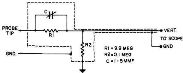
**Configuration for a 100-to-1 high-impedance compensated probe. (Adjust C for 100-to-1 attenuation at 60 cycles and 100 kc.)**
