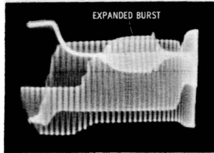
oscillator out of cutoff. Then the beam is deflected across the face of the scope once by a single sawtooth cycle. The beam rests after the one sweep until the sync signal rises once again to the triggering level.
