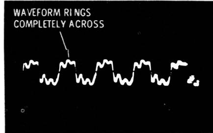
500,000-cycle square wave. Pattern shows ringing completely across the top and bottom.
