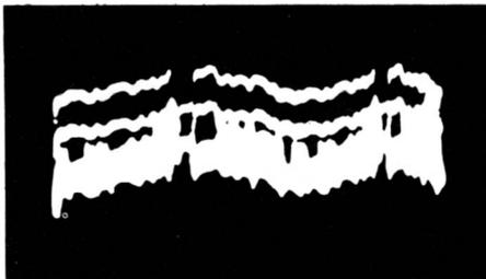
**Effect of poor low-frequency response and 60-cycle hum in video amplifier on composite video signal.**
