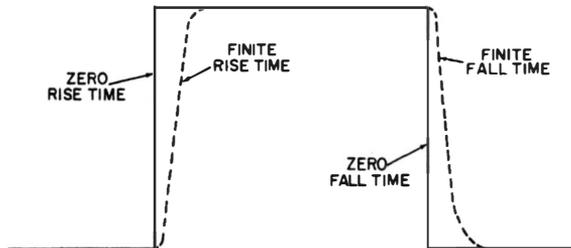
**Comparison of zero rise and fall times to finite rise and fall times.**
