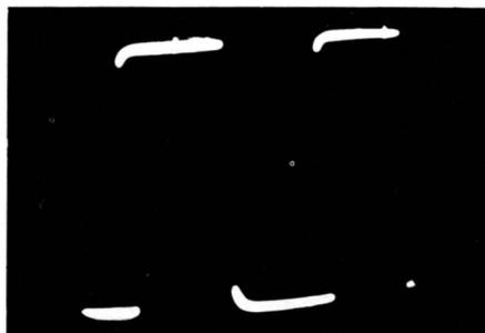
Corner rounding occurs when control is set to low level.
