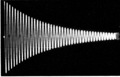
Fig. 9. Ringing test of a single coil.
