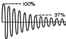
**Bandwidth of a coil-capacitor combination.**
