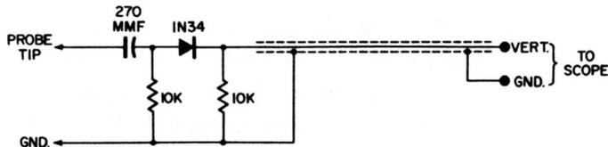
Medium-impedance demodulator probe circuit.
