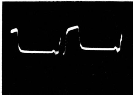
Tilt in chroma demodulator waveform, caused by phase shift resulting from inaccurate alignment of signal circuits.
