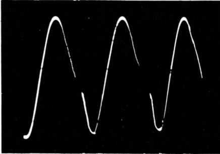
60-cycle hum modulation seen in display of 60-cycle sine wave.
