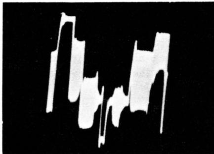
**Color-bar waveform showing amplitude distortion in the IF amplifier.**
