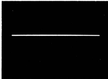
**Horizontal gain advanced; vertical gain zero.**
