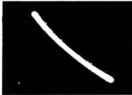
**No phase shift, but amplitude non-linearity shows as a curvature of the diagonal line.**
