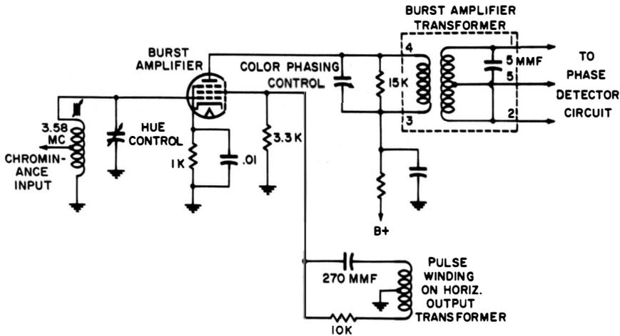
**A burst-amplifier circuit.**
