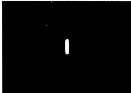
**Cross talk between the sawtooth oscillator and the vertical amplifier.**
