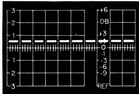
Triggered-sweep scope has its graticule stepped off in centimeter intervals.
