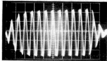
triggered-sweep scope provides the expanded display seen in Fig. 7. Why is there no overlap in the pattern of Fig. 7? It is because the beam deflects only once for each horizontal sync pulse, regardless of sweep speed. Since the sweep speed can be set at any value, we choose a speed that fills the screen horizontally with only the burst display. Unlike a conventional scope, sync lock is unaffected by changing the horizontal sweep speed.
