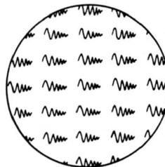
**Display at 15,750-cycle horizontal sweep in scope.**
