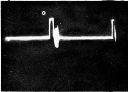
**Undistorted sync and burst waveform.**
