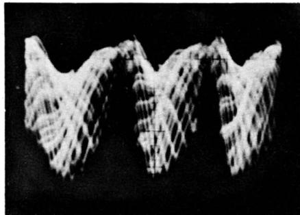
**Change in ripple waveform on B+ lead to chroma section when receiver is out of color sync.**
