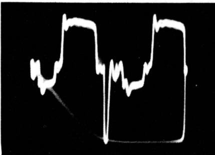
Overshoot and ringing, caused by sharply peaked signal circuits.
