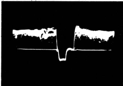
Poor horizontal sync separation.
