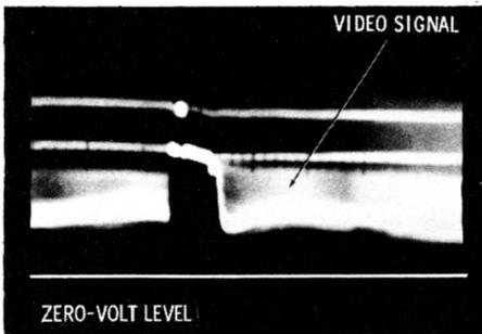
**Waveform obtained when checking the percentage modulation of a video signal.**
