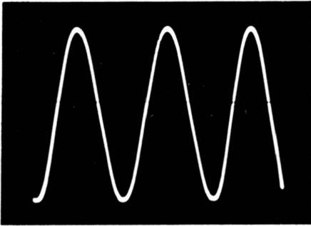
**Waveform when a 60-cycle sine wave is viewed at a horizontal sweep rate of 20 cps. Three cycles are displayed. NOTE: A portion of one cycle is lost on retrace.**
