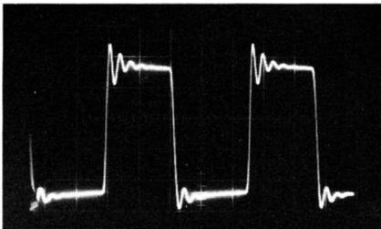
(A) 2-kc square-wave response with resistive load on the amplifier.
