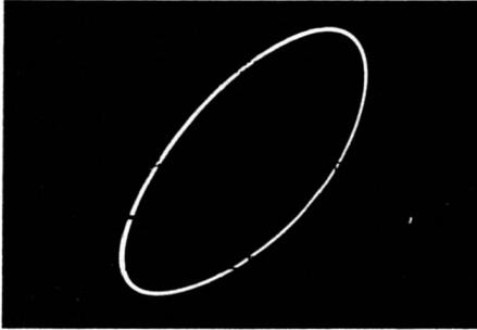
An ellipse, as shown above, is displayed unless R and C have suitable values. A circle is obtained only when R and C are of suitable values and the scope gain controls are suitably adjusted.
