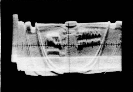
(A) Test setup. NOTE: Proximity of hand injects 60-cycle hum into exposed vertical-input terminals.
