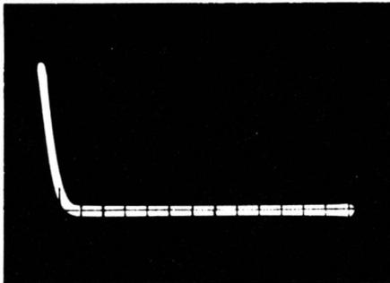
**Severe amplitude distortion.**
