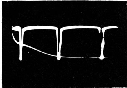
**To Check the Action of a Horizontal Dynamic Convergence Phasing Control**
