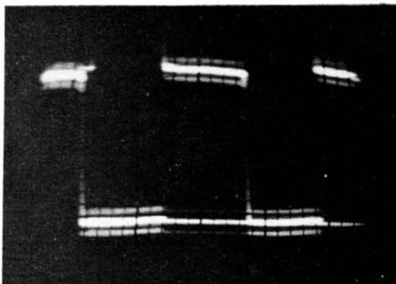
**Leading edge is invisible at brightness level where trailing edge is visible. Rise time is faster than the fall time in this waveform.**
