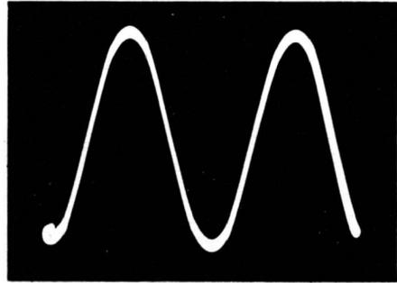
Both vertical and horizontal gain controls advanced.
