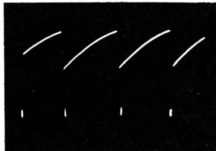
**Waveform at grid of typical vertical-oscillator tube.**
