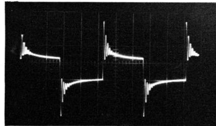
(B) 2-kc square-wave response with voice-coil load on the amplifier.
