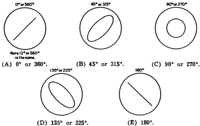
**Waveforms obtained with different degrees of phase shift.**
