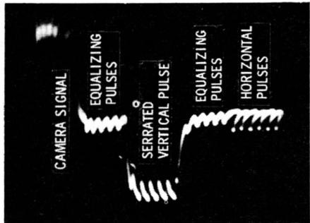
Waveform obtained with resistive probe.
