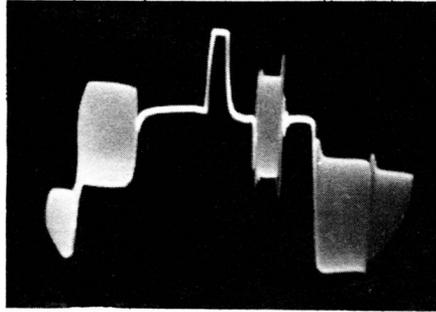
**Burst waveform observed when color-bar generator is connected directly to scope.**
