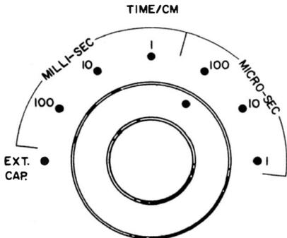
Typical sweep-speed control on triggered-sweep scope.
