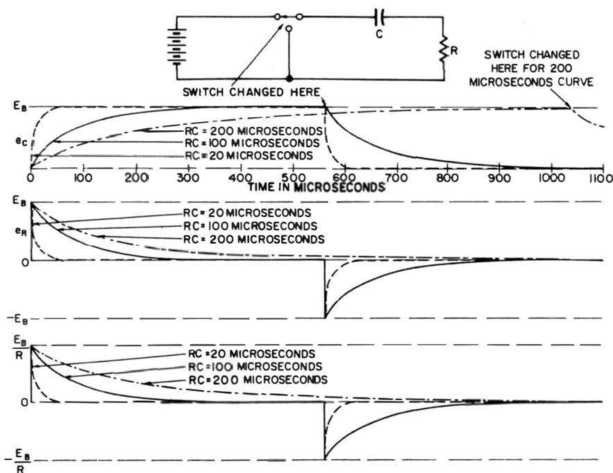
**Fig. 15. Effect of varying R and C in an RC circuit.**
