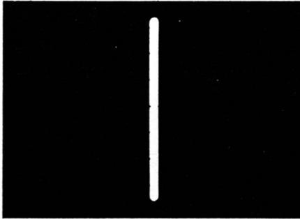
Vertical gain advanced; horizontal gain zero.
