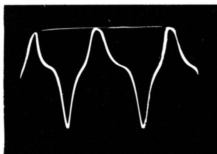
Typical waveform at grid of horizontal-discharge tube.
