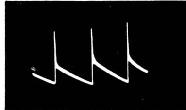
**Fig. 3. Typical waveforms found in a TV receiver. (Courtesy Motorola, Inc.)**
