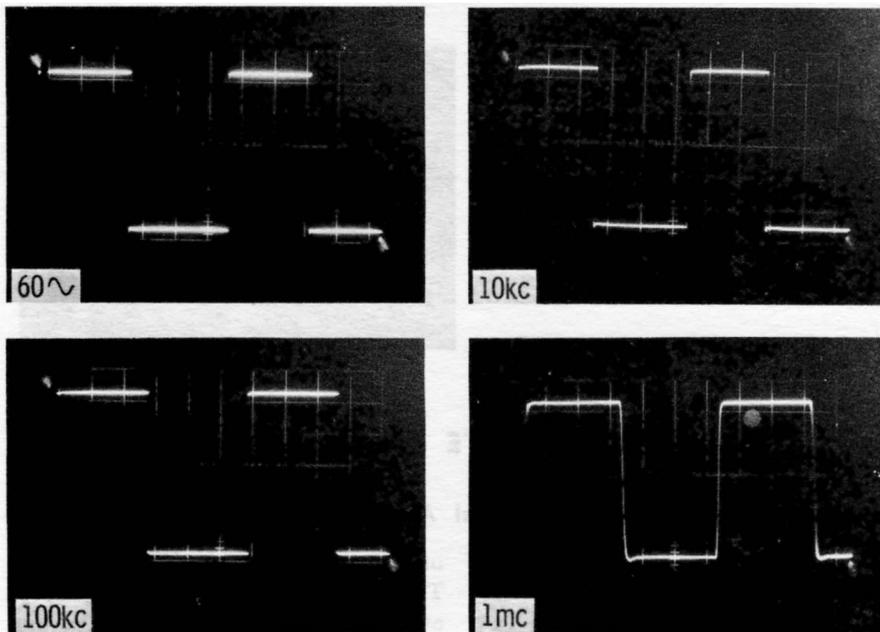
(C) Response of a lab-type 15-mc scope.
