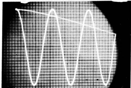
**Fig. 5. Appearance of a graticule, used to measure peak-to-peak voltages.**
