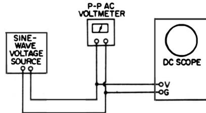
**Test setup for AC response.**
