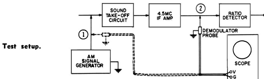
**Output signal from AM signal generator.**
