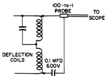
**Method of connecting scope ground lead to the return lead of the deflection coils.**
