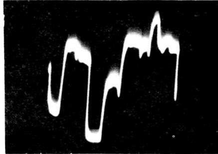
**Interference from vertical sweep circuit.**
