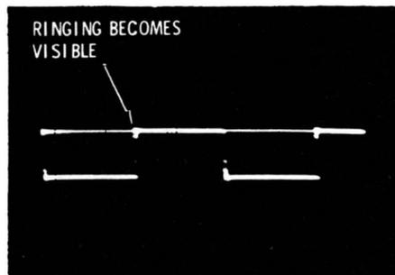
**10,000-cycle square wave. High-frequency ringing can be seen on leading and trailing edges.**
