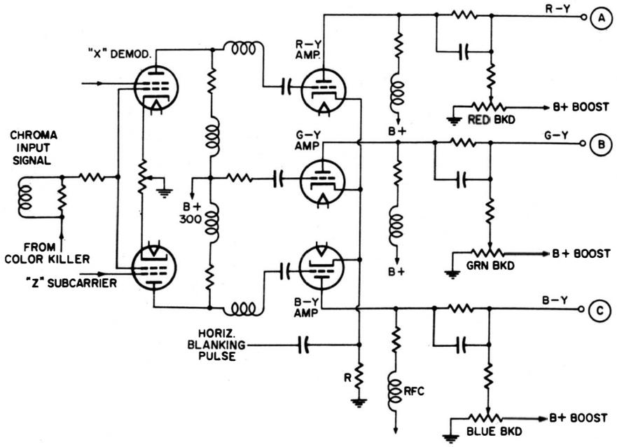
X and Z demodulator circuit.
