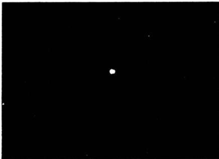
**Both horizontal and vertical gain controls set to zero.**
