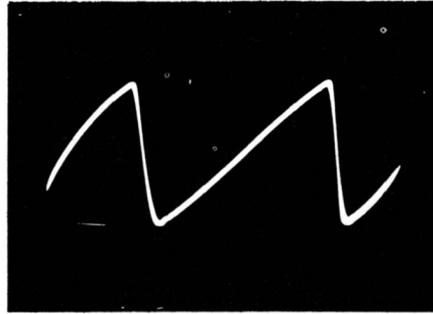
**Current waveform of a typical vertical-deflection voltage.**
