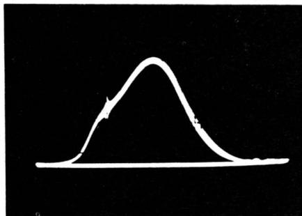
Pattern has half-height on scope screen when generator RF frequency is tuned to half-voltage point on curve; pattern has full height when RF frequency is tuned to top of curve.
