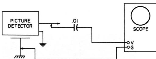
**Scope connected to floating mounting bracket.**
