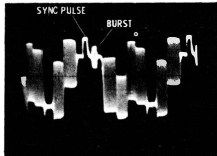
Waveform obtained from color-bar generator.
