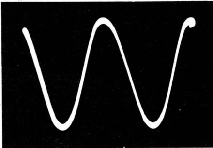
**Waveform observed across the horizontal phasing control.**
