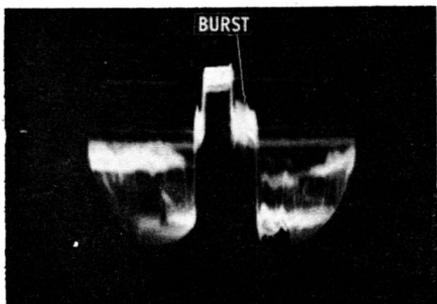
**Burst position in a typical color TV broadcast.**
