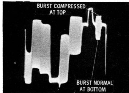
**To Check the Output from a Keyed Rainbow Color-Bar Generator**
