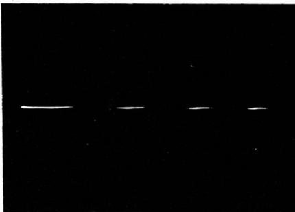
Hum modulation of beam at normal brightness setting.
