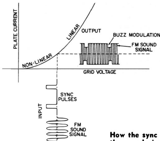
**How the sync voltage becomes modulated into the sound signal.**
