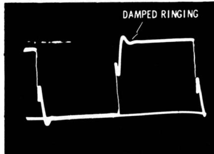
**Square waveforms displaying damped ringing.**
