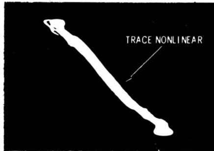
**Moderate amplitude distortion (audio oscillator frequency varied).**
