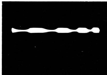
Hum modulation of beam at high brightness setting.
