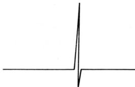
**Normal appearance of a pulse voltage on base line.**
