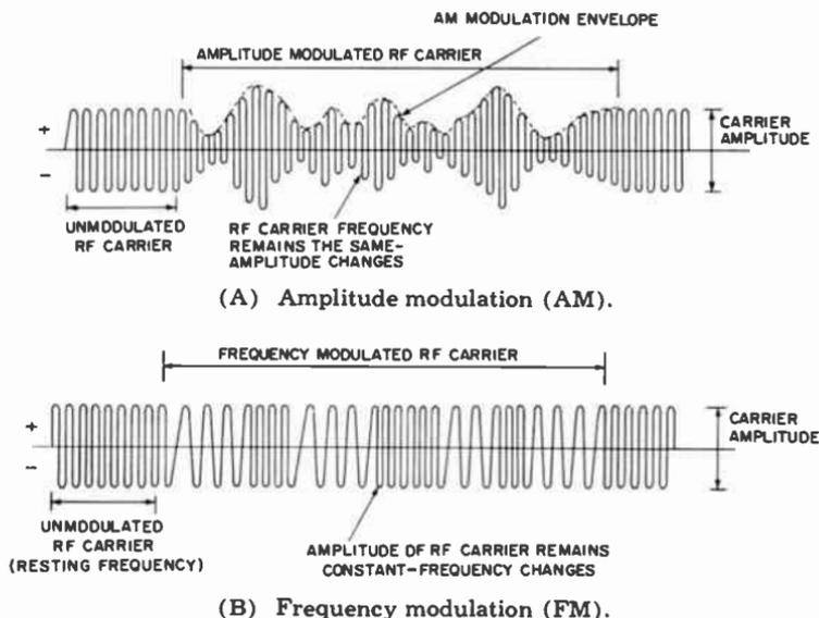
Fig. 1-4. Two types of modulation used in CB radiotelephone communications.
