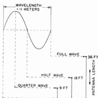
Fig. 4-2. Wavelength versus antenna length.
