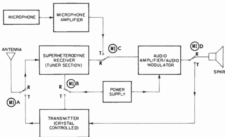
Fig. 3-2. Block diagram of a Class-D transceiver employing a superhet receiver.
