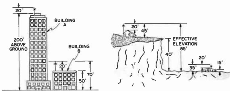
(A) Elevation provided by man-made structure.
