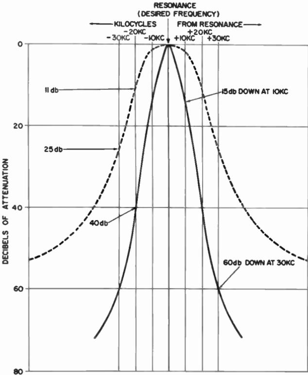
Fig. 2-1. A typical CB receiver selectivity curve.
