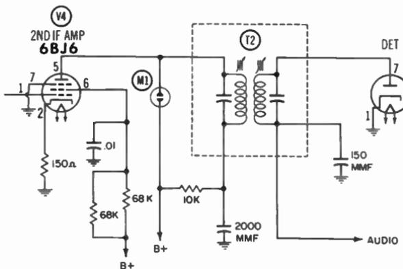
Fig. 3-19. A simple noise-clipping circuit using a neon bulb.
