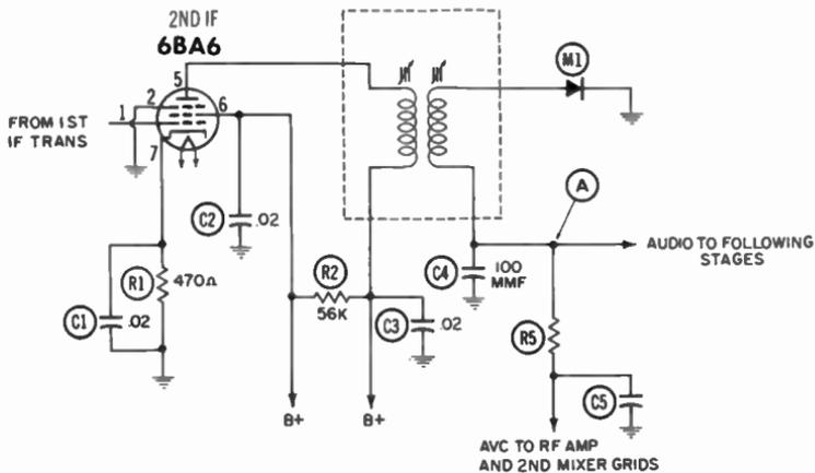
Fig. 3-15. An AVC system using the second detector as the rectifier.
