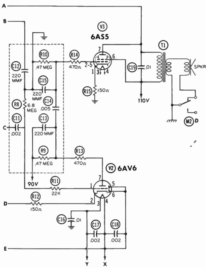
using a superregenerative receiver circuit.
