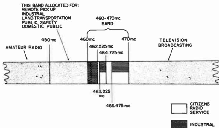
Fig. 1-1. Position of Class-A and -B channels in the frequency spectrum.
