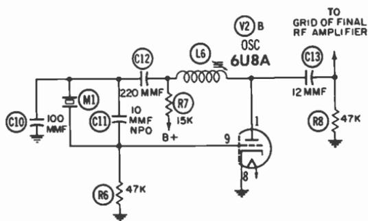
Fig. 3-22. A crystal-controlled transmitter oscillator circuit.
