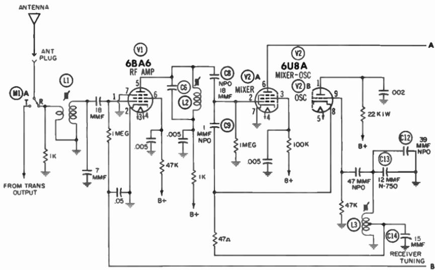
Fig. 3-3. Schematic of the
