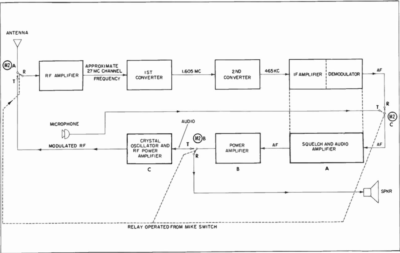
Fig. 3-4. Block diagram of a transceiver employing a dual-conversion super-het circuit.
