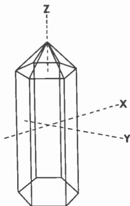
Fig. 3-10. The quartz crystal in its natural state.
