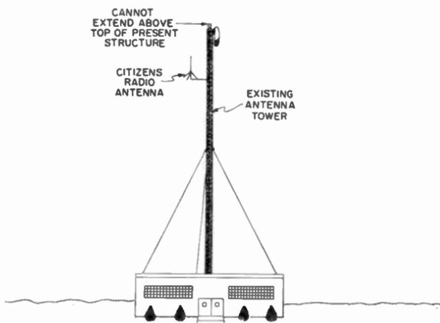
Fig. 4-7. The CB antenna mounted on the existing structure of another station.
