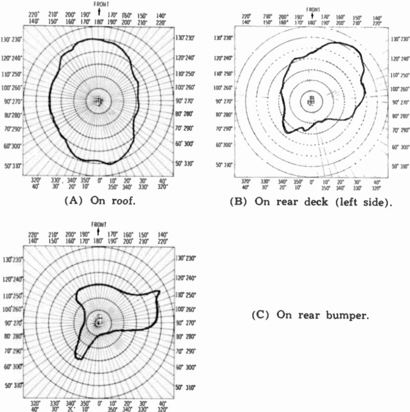
Fig. 4-19. Horizontal radiation patterns when whip antenna is mounted at various places on a car.
