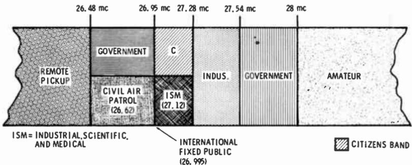
Fig. 1-7. Position of Class-D channels in the frequency spectrum.
