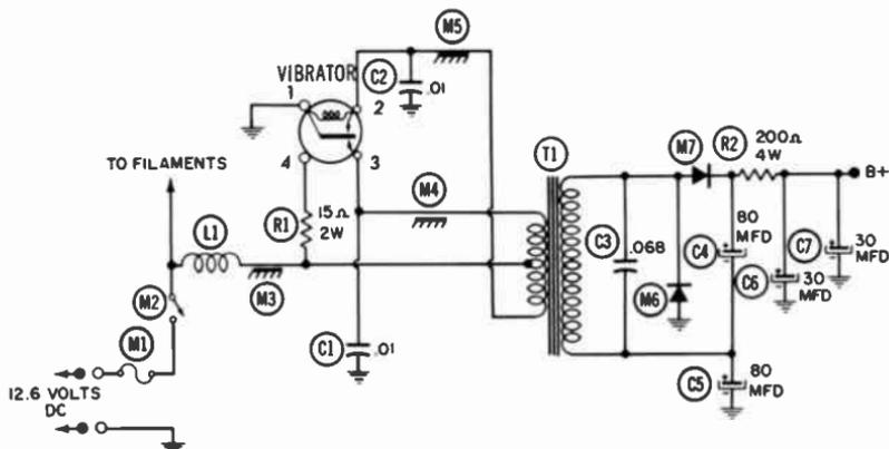
Fig. 3-26. Vibrator power supply employed for DC operation.
