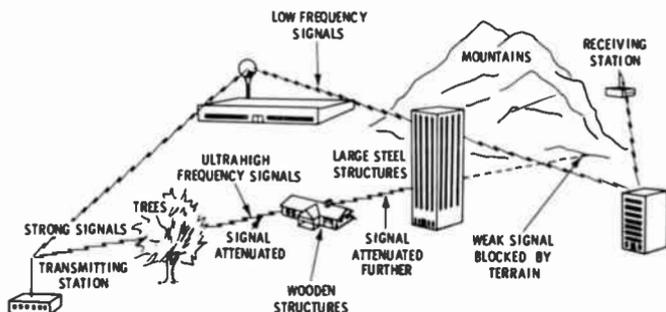
Fig. 1-2. An example of the UHF signal's line-of-sight characteristics.
