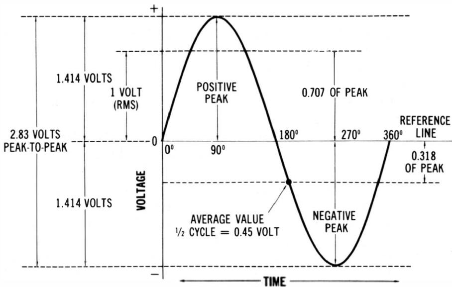
**Fig. I-4. A sine wave with important values.**
