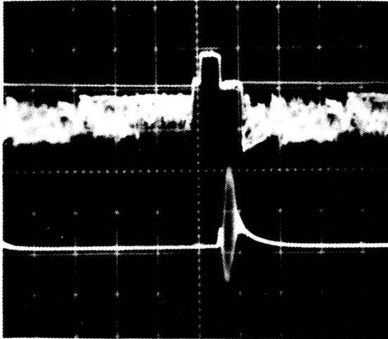
**Fig. 3-28. Display of the color burst from the complete color signal.**
