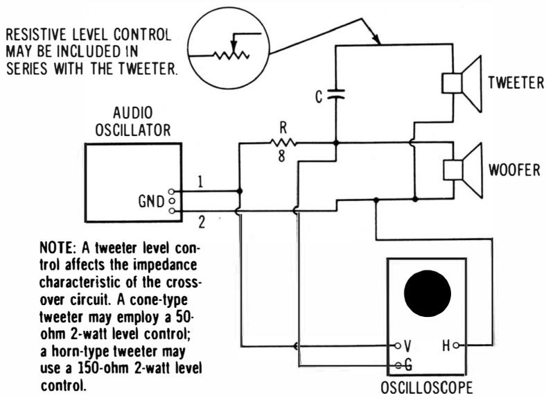
**Fig. 2-4. Measurement of input impedance of a crossover network.**
