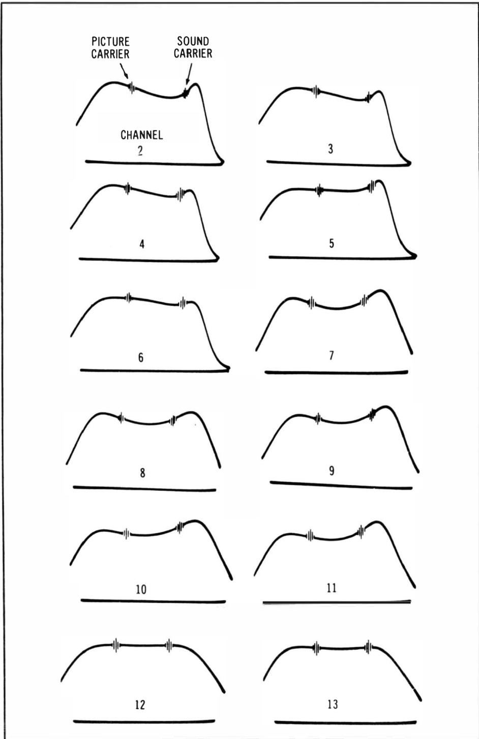
**Fig. 3-15. The rf response curves showing normal tolerances on the 12 vhf channels for a good-quality receiver.**
