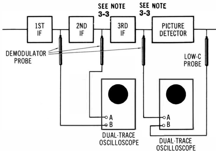
(B) Two dual-trace scopes monitoring four signal points in the if section.
