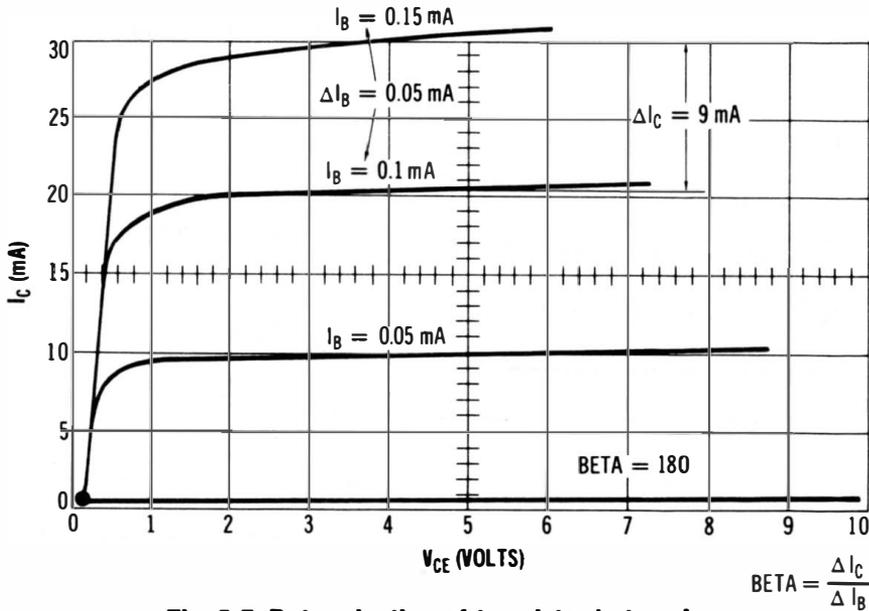
Fig. 5-7. Determination of transistor beta value.
