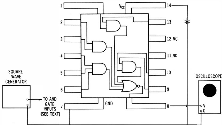
(A) Typical package pin-out and test setup.
