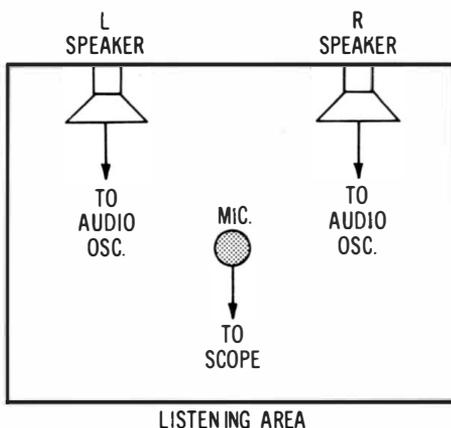
**Fig. 1-18. Check of ringing frequencies (acoustic standing waves) in a listening area.**
