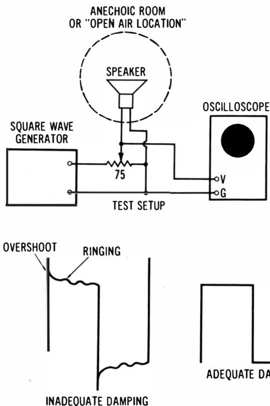
**Fig. 1-17. Checking the optimum value of speaker damping resistance.**
