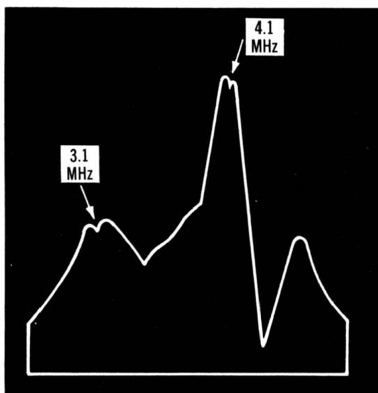
**Fig. 3-35. Typical bandpass-amplifier response curve, with absorption markers at 3.1 and 4.1 MHz.**
