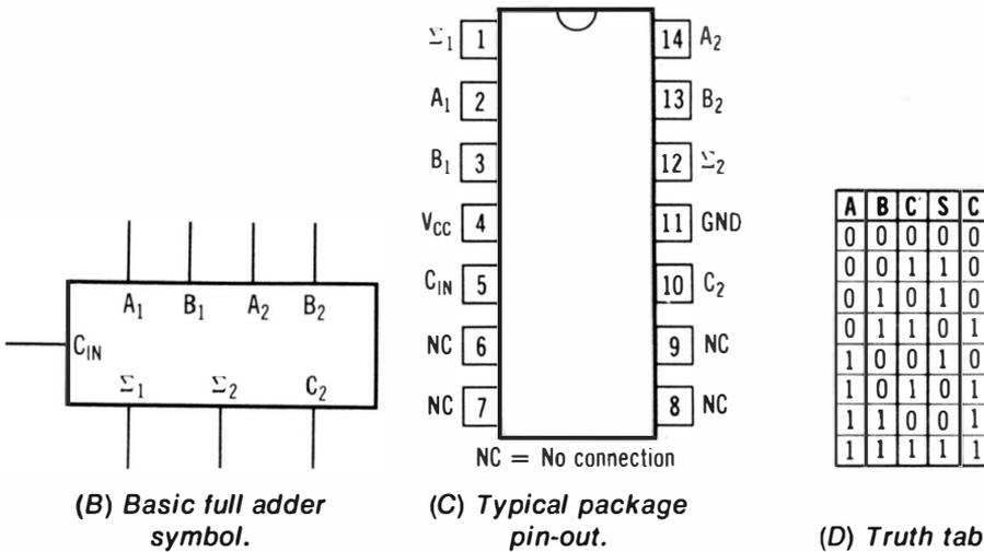
**Fig. 4-9. Check of full adder operation.**
