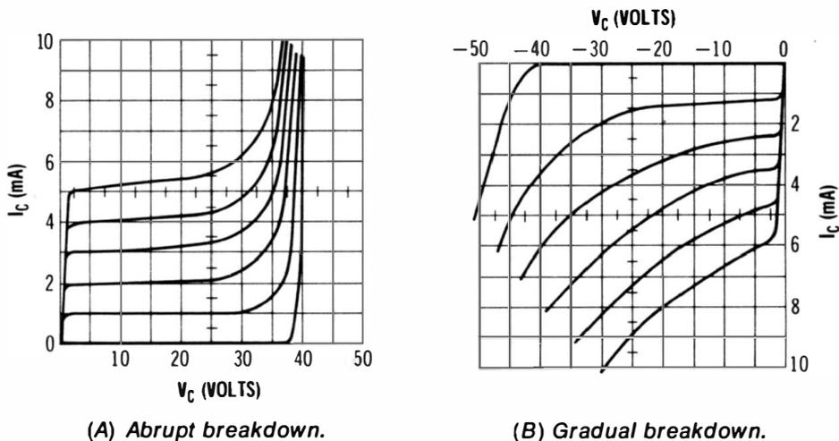
**Fig. 5-15. Patterns observed during breakdown voltage measurements.**
