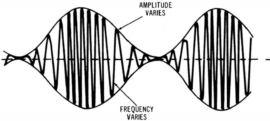
**Fig. 3-22. A 100-percent amplitude-modulated output signal from an am generator, with incidental frequency modulation.**
