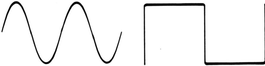
**Fig. 1-6. Sine wave and square wave with the same peak-to-peak voltage.**
