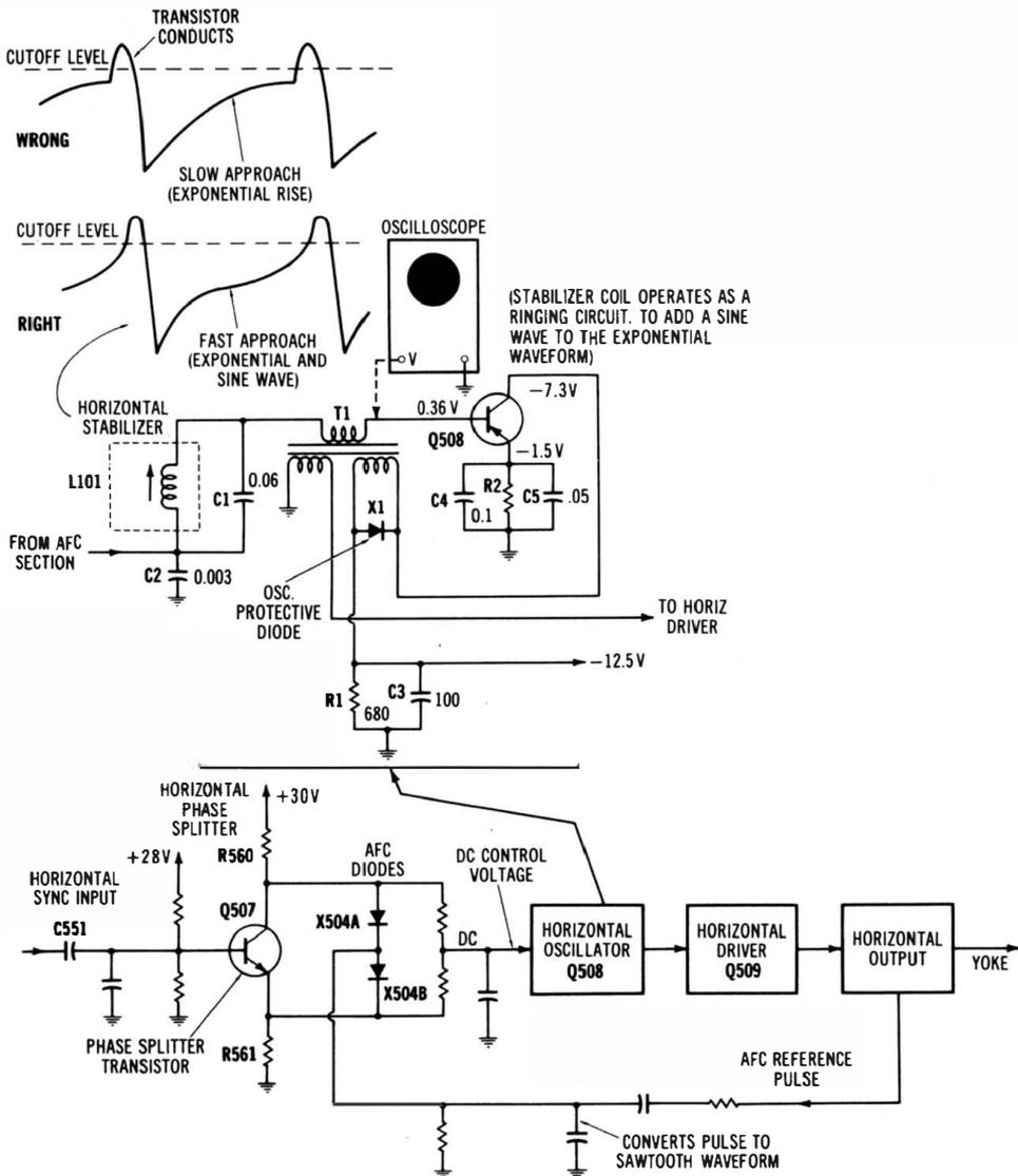
**Fig. 3-25. The afc section is a portion of the servo (feedback control system).**
