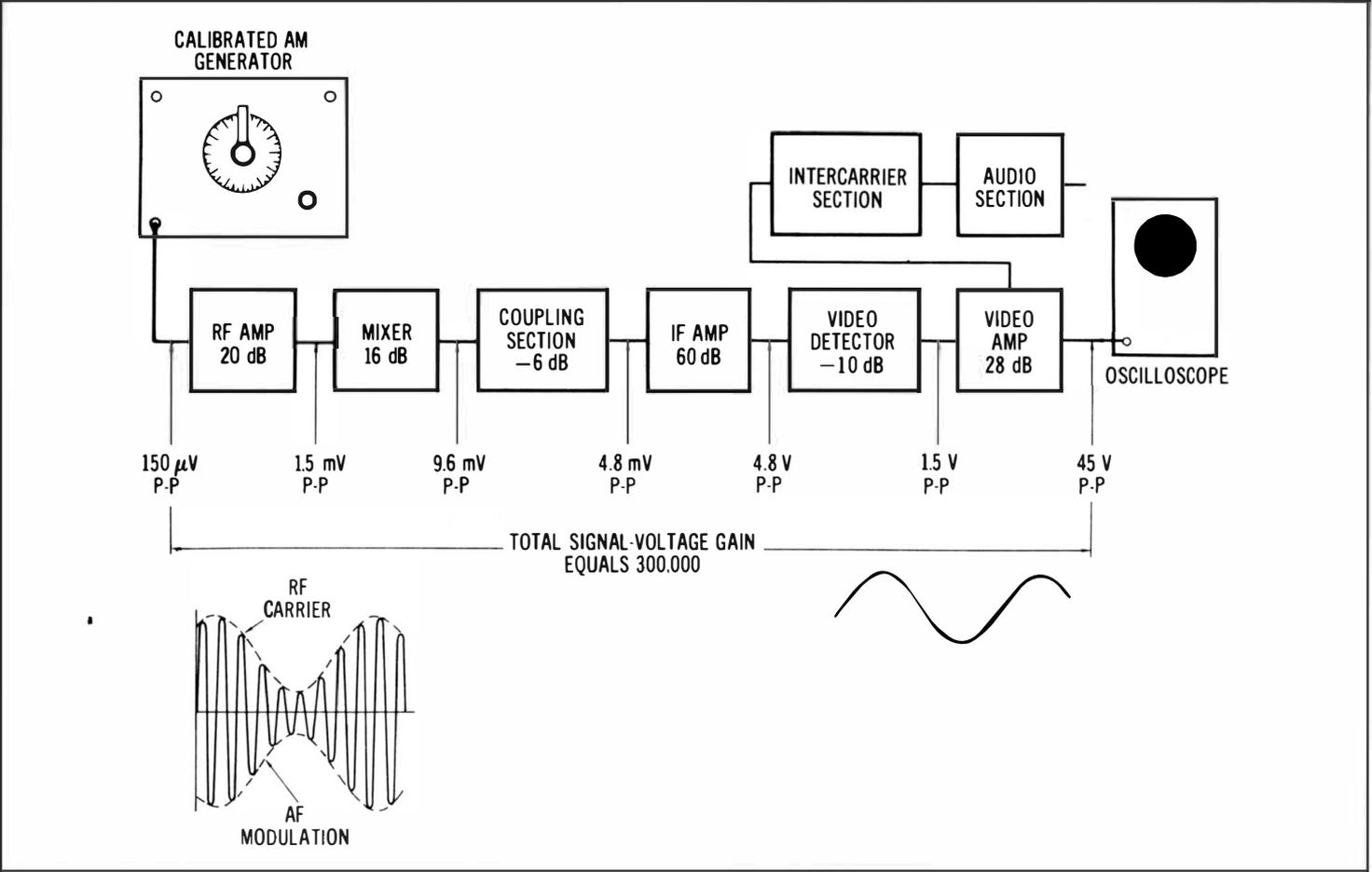
Fig. 3-4. Block diagram of typical black-and-white tv receiver operating at maximum available gain.
