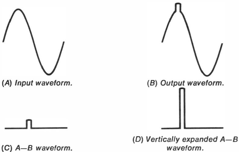
**Fig. 1-3. Difference waveform consists of distortion products.**
