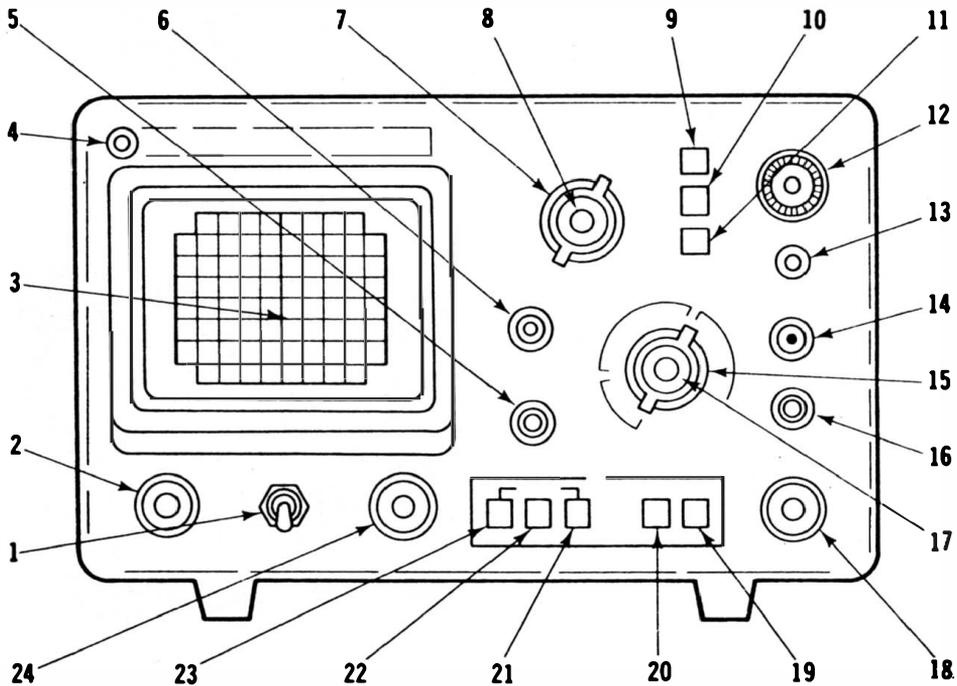
1. POWER ON-OFF toggle switch. Applies power to oscilloscope.
