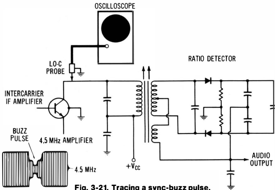
**Fig. 3-21. Tracing a sync-buzz pulse.**
