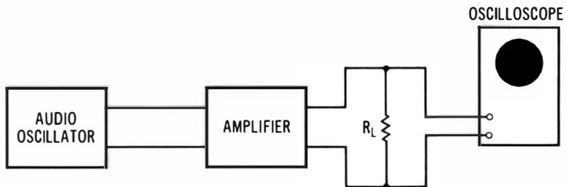
(A) Output voltage is measured at 1 kHz.
