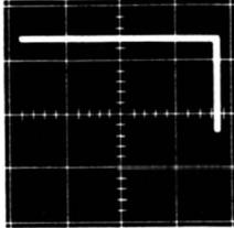
(C) Ppn collector-base waveform with red lead connected to collector.
