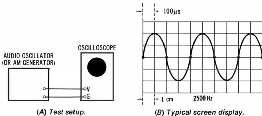
**Fig. 7-1. Checking the accuracy of a calibrated time base.**
