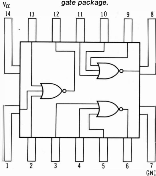
(E) Typical triple 3-input NOR gate package.
