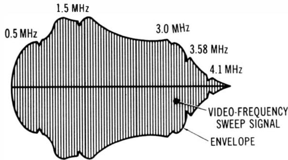
(B) Representative scope pattern at picture detector output.
