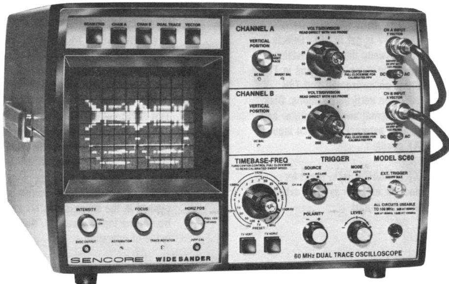
**Fig. 1-4. A modern oscilloscope that provides dual-channel displays and a choice of A-B or A+B patterns.**
