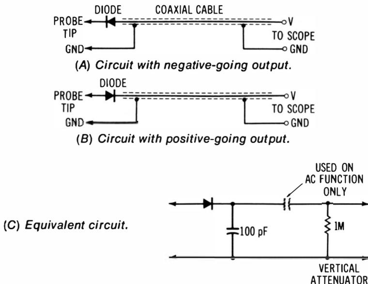
**Fig. 3-8. Simplest demodulator probe design (series detection).**
