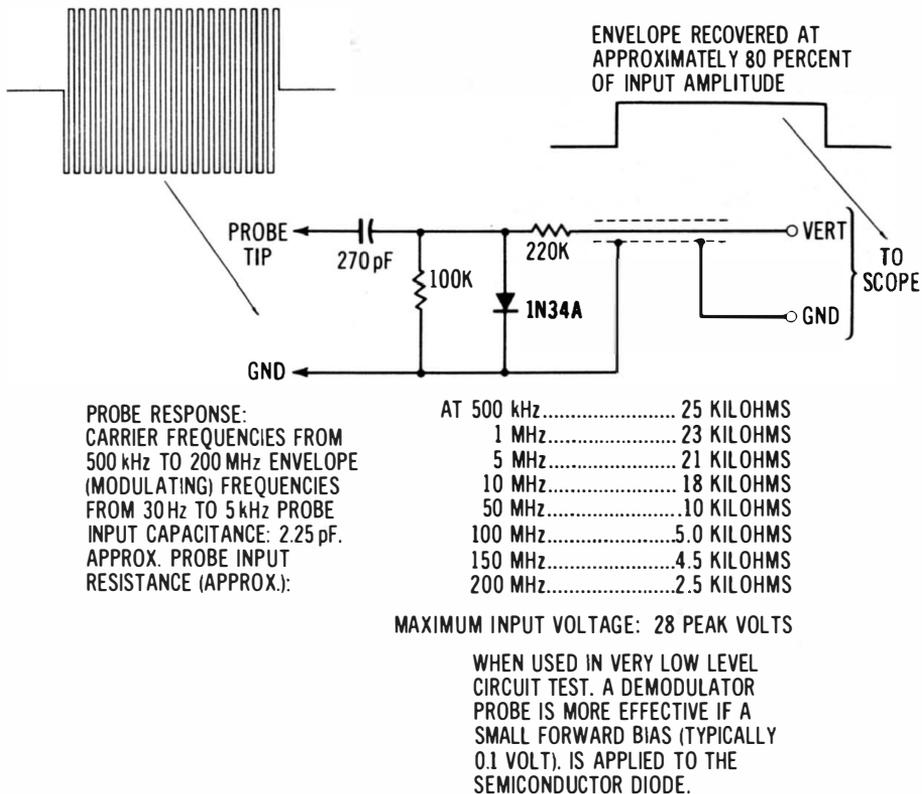
**Fig. 3-6. Standard demodulator probe configuration and characteristics.**
