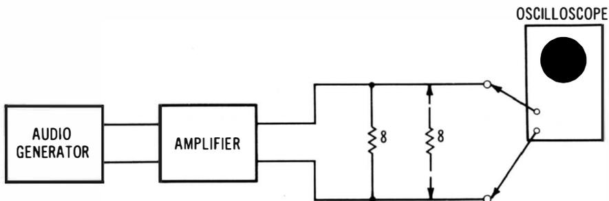
Fig. 1-13. Measurement of amplifier output resistance.
