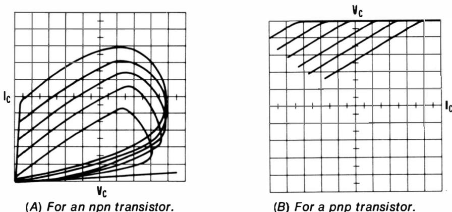
**Fig. 5-10. Typical in-circuit curve-tracer patterns.**
