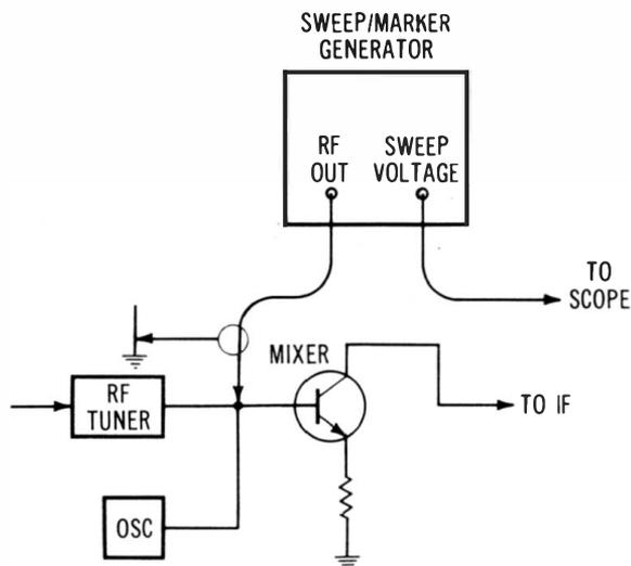
**Fig. 3-14. Standard signal-injection point for checking the if frequency response.**
