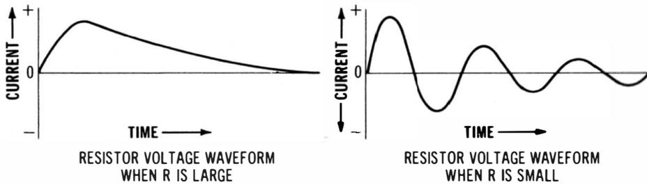
**REDUCTION IN RINGING FREQUENCY CAUSED BY CIRCUIT RESISTANCE**
