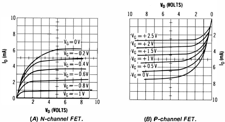
**Fig. 5-17. Typical FET drain family characteristics.**
