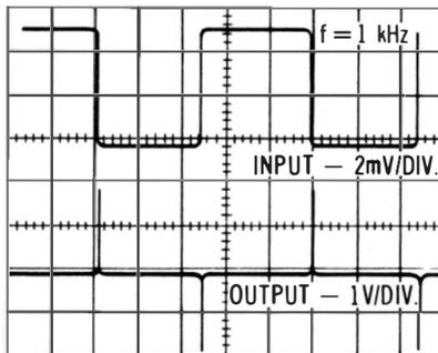
(B) Normal input/output waveforms.
