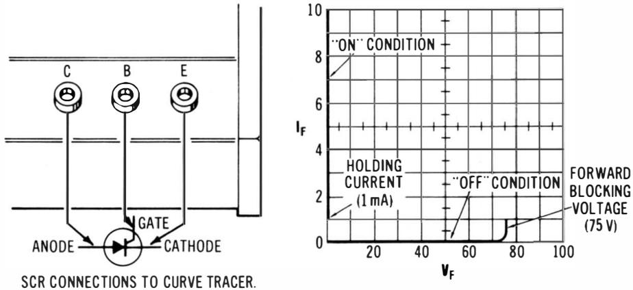
**Fig. 5-21. Measurement of forward blocking voltage for an SCR; holding current is also displayed.**
