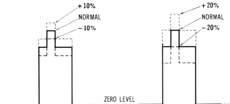
**Fig. 3-24. Sync pulse amplitude tolerances.**
