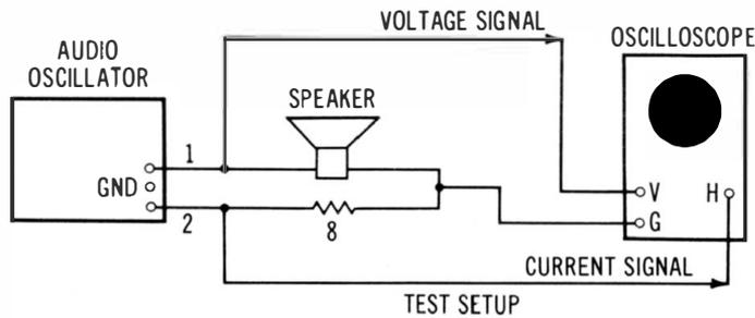
NOTE: Terminals (1) and (2) of the audio oscillator "float" with respect to ground. In other words, the Gnd terminal is not returned to any point of the (1)-(2) circuit in this type of instrument. The Gnd terminal is merely connected to the metal case of the audio oscillator.
