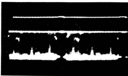
SYNC NORMAL; VERTICAL-SYNC INTERVAL IS LEVEL WITH THE HORIZONTAL SYNC INTERVAL
