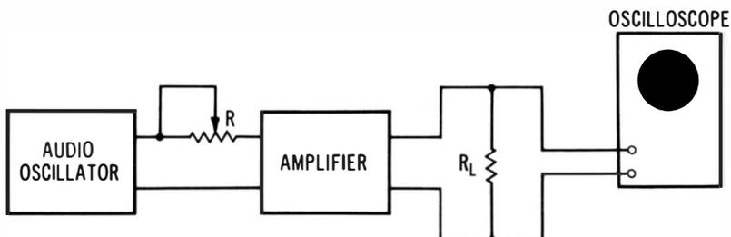
(B) Potentiometer resistance inserted to reduce output voltage to one-half.
