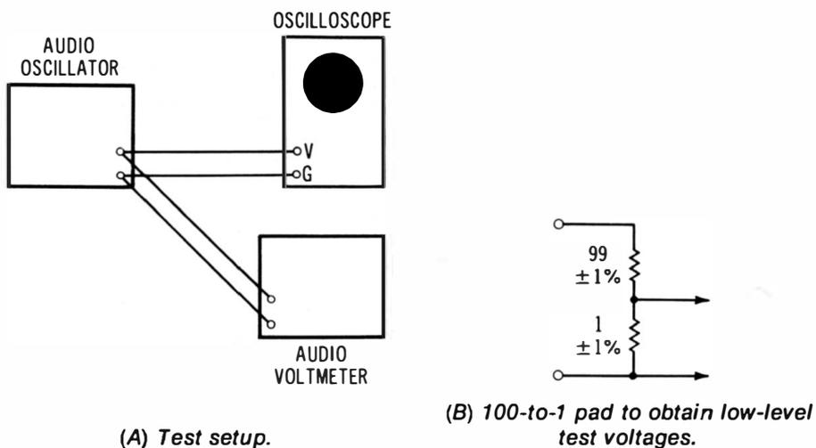
**Fig. 7-2. Checking the accuracy of a calibrated vertical attenuator.**
