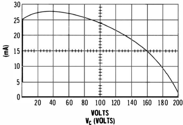
**Fig. 5-22. Example of forward conduction at 200 volts, followed by holding-current indication of 5 mA.**
