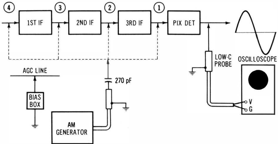
**Fig. 3-11.** Gain of third if stage is measured by transferring signal-injection point from (1) to (2).
