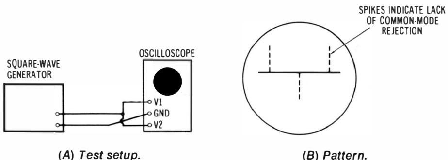
**Fig. 7-6. Checking a differential-input scope for common-mode rejection.**
