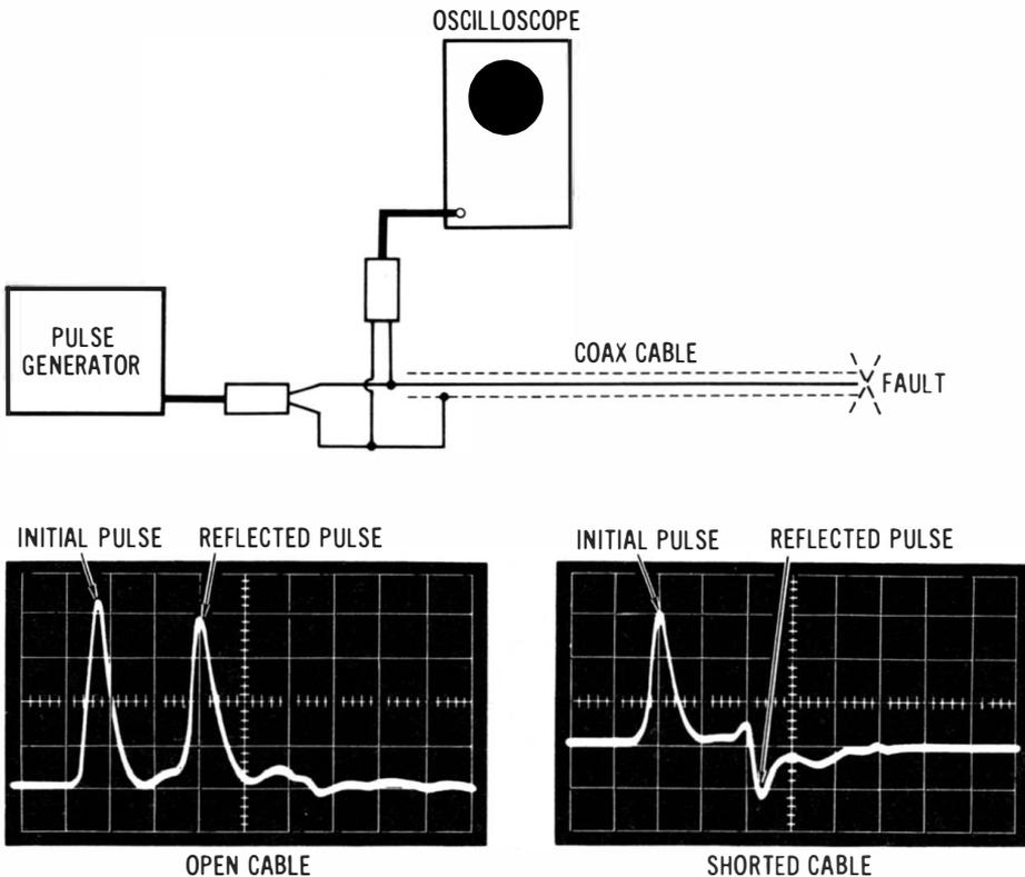
**Fig. 3-43. Measurement of distance to a cable fault.**
