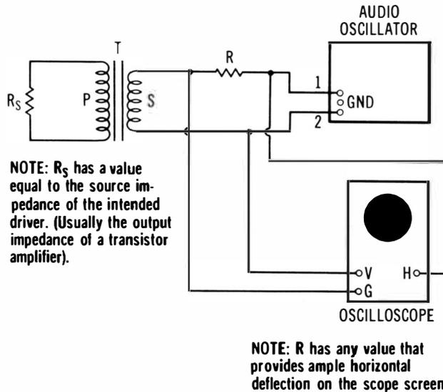
**Fig. 2-3. Measurement of output impedance of a transformer.**
