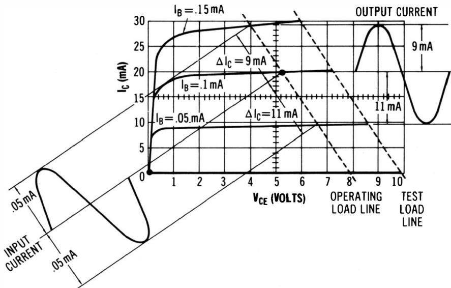
**Fig. 5-13. Measurement of nonlinearity in transistor characteristics.**
