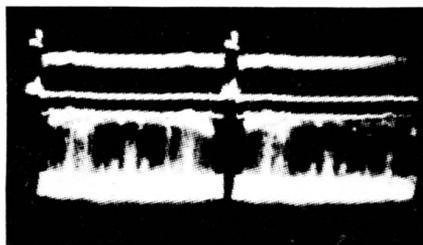
OPPOSITE DISTORTION FROM SYNC PUNCHING; VERTICAL-SYNC INTERVAL IS ABOVE HORIZONTAL-SYNC LEVEL
