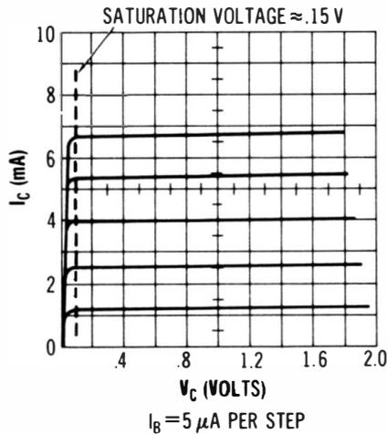
gion up to and including the knee of each curve. Thus, the display can be expanded, using a low-voltage horizontal calibration value, such as 0.2 volt per division. This facilitates accurate measurement of low collector voltage values. Data sheets usually specify saturation-resistance values as maximum acceptable limits.
