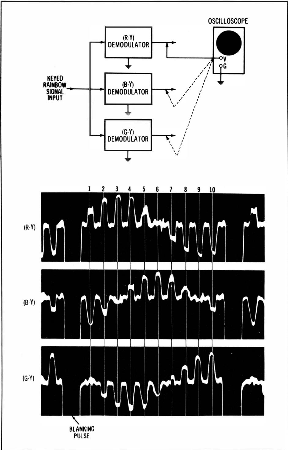
**Fig. 3-32. Phase checks of R-Y, B-Y, and G-Y waveforms.**
