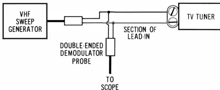
**Fig. 3-40. Check of tv tuner input impedance.**
