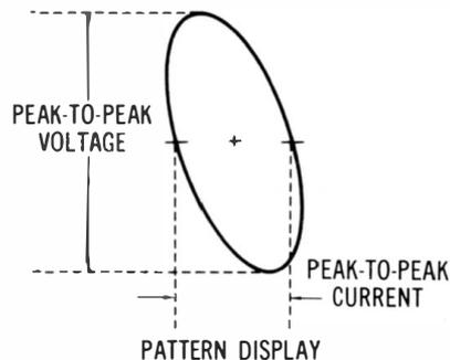
**Fig. 2-1. Measurement of speaker impedance.**
