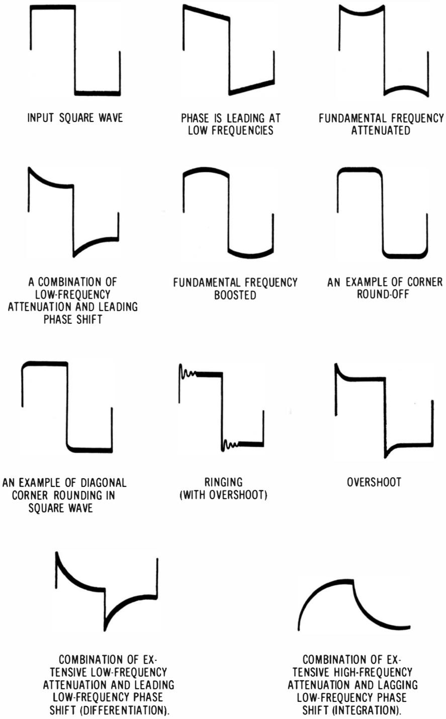
**Fig. 1-10. Basic types of square-wave distortion.**
