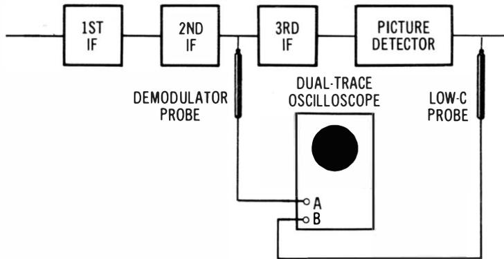
(A) A dual-trace scope monitoring the output of the second if stage and output of picture detector.
