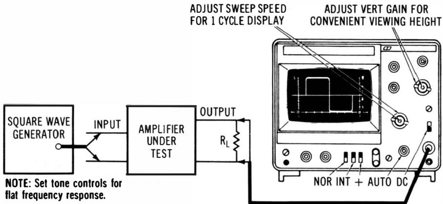
**Fig. 1-9. Test setup for square-wave response.**
