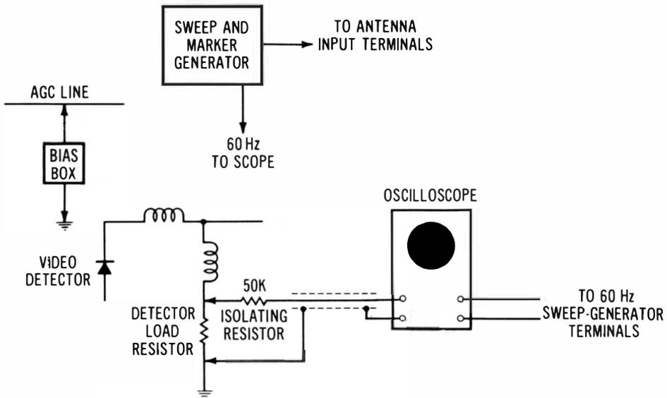
(A) Test connections for check of overall rflif response curve.
