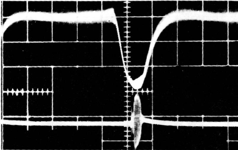
**Fig. 3-30. Display of the burst keying pulse with the color burst, and of the separated burst.**
