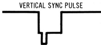
WAVEFORM REPRODUCED BY CONVENTIONAL DEMODULATOR PROBE
