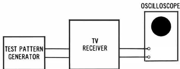
**Fig. 3-1. Test setup for basic video signal distortion check.**
