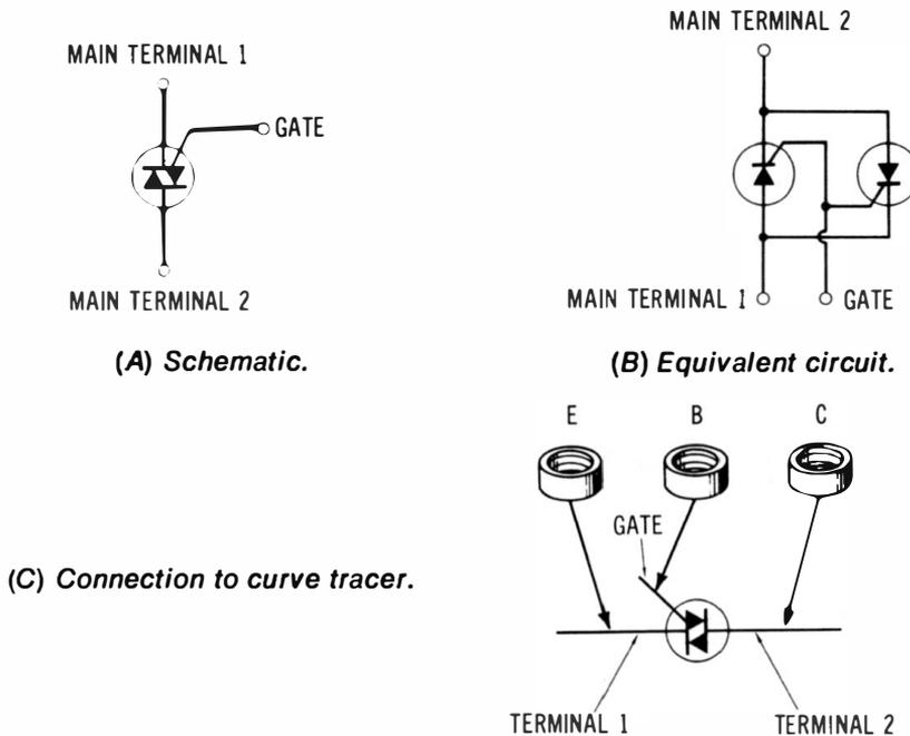
**Fig. 5-25. A triac consists of two paralleled and oppositely polarized SCRs.**
