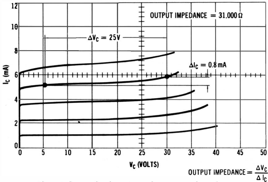
**Fig. 5-9. Determination of transistor output impedance.**
