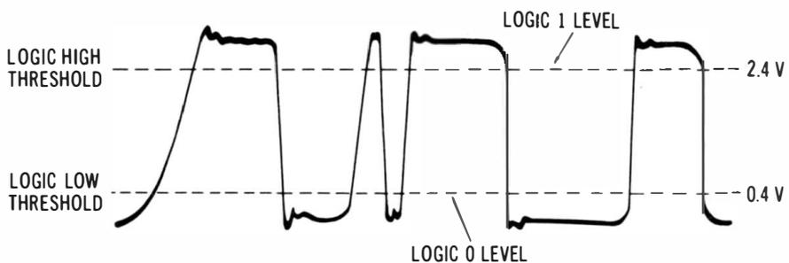
**Fig. 4-2. Typical digital waveform in TTL circuitry, showing High (1) and Low (2) thresholds. (CMOS circuitry employs supply voltages in the range from 3 to 18 volts; check manufacturer's data sheet).**
