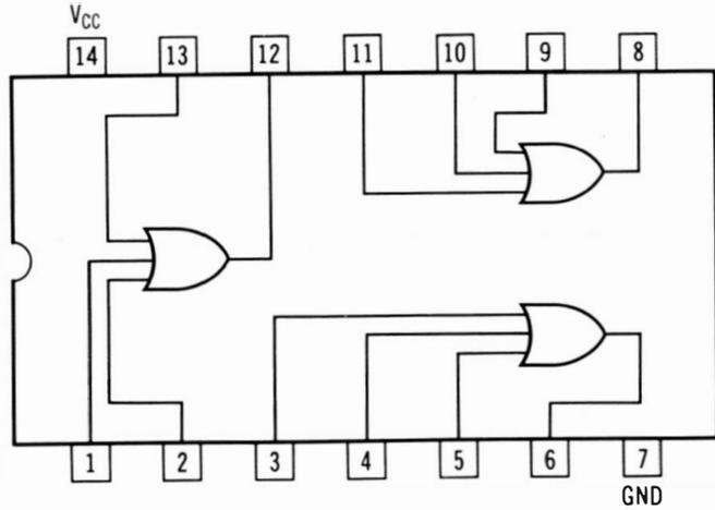
(C) Typical triple 3-input OR gate package.
