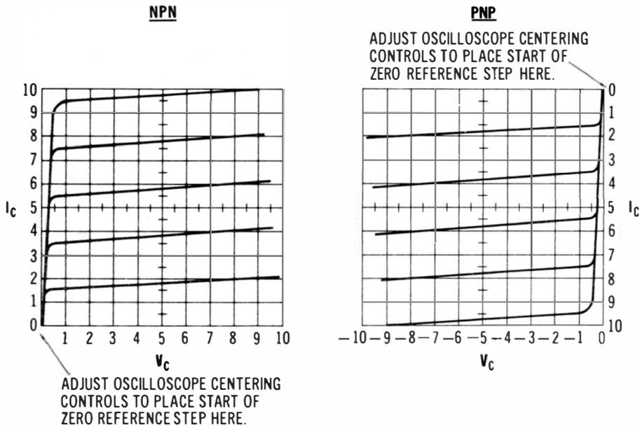
Fig. 5-8. Pnp display is "upside down" with respect to npn display.
