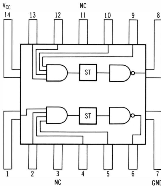
(B) Typical dual Schmitt trigger package pin-out.
