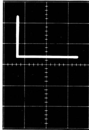
(B) Black test lead connected to diode anode.
