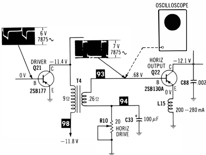
**Fig. 3-26. Drive waveform must have normal amplitude and fast rise.**
