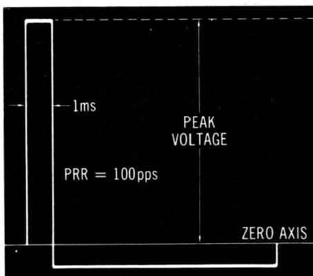
(B) Undistorted output pulse.
