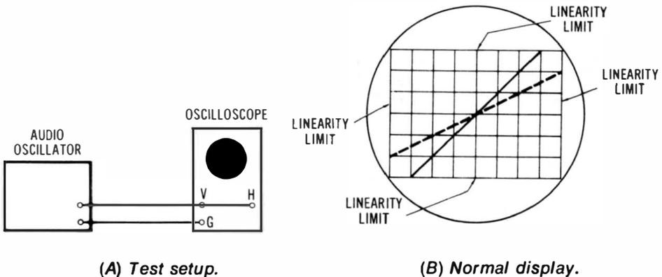
**Fig. 7-3. Checking the vertical and horizontal amplifiers for linearity.**
