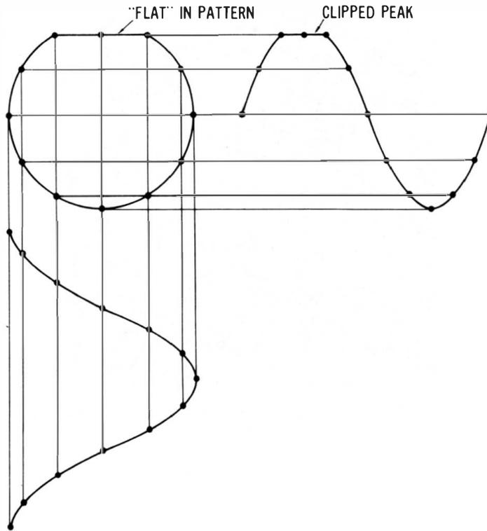
**Fig. 3-34. Pattern becomes flattened when one of the input waveforms is clipped.**
