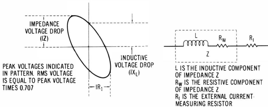
**Fig. 2-6. Voltage indications in a Lissajous figure for a coil.**
