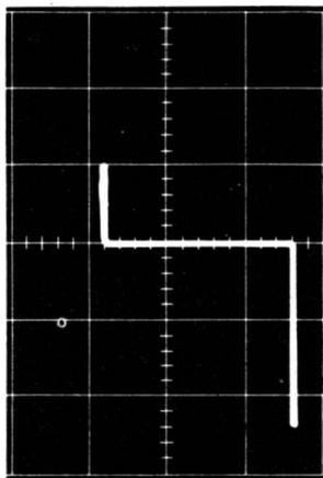
(C) Waveform of a 30-volt zener diode.
