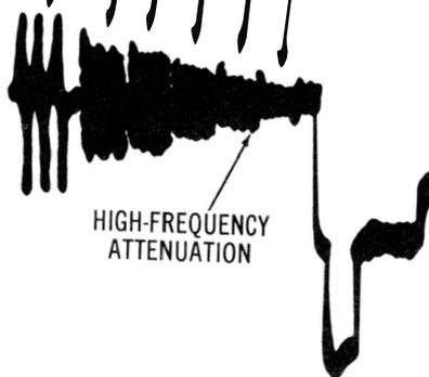
NOTE: These waveforms are transmitted by color-TV stations on two lines of the vertical-retrace interval.
