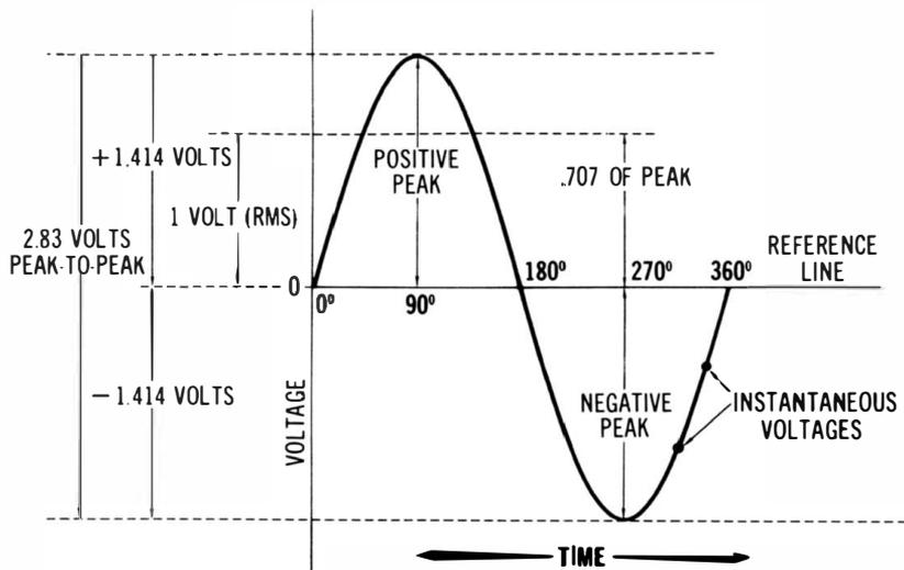
**Fig. 1-14. Voltage values in a sine wave.**
