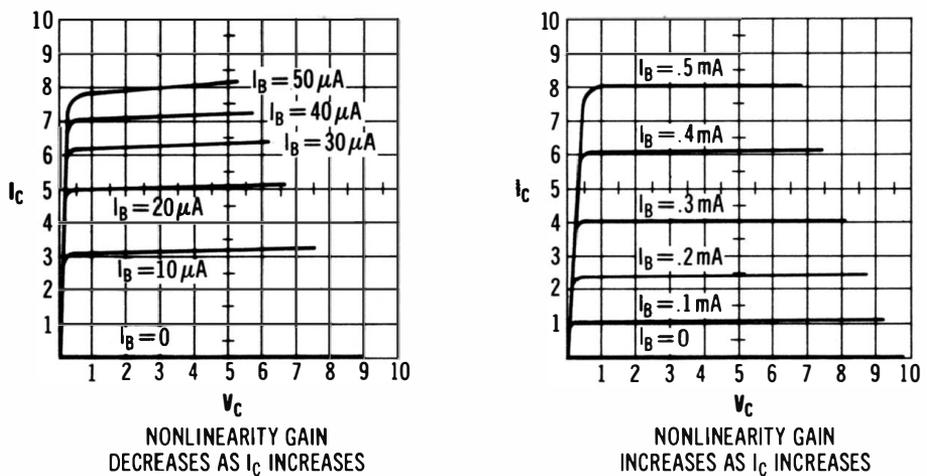
**Fig. 5-14. Two types of nonlinear collector family characteristics.**
