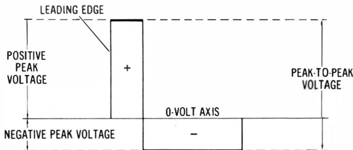
**Fig. I-5. Basic pulse waveform.**
