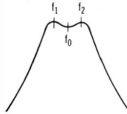
(B) The two resonant frequencies are  $f_1$  and  $f_2$ , and the ringing frequency is  $f_0$ .
