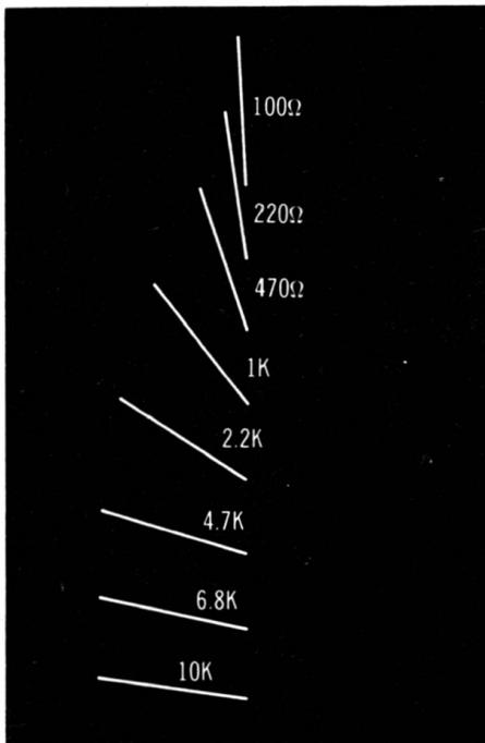
**Fig. 5-3. Slopes of screen traces for corresponding values of resistances.**
