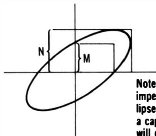
Note that if an inductive impedance causes the ellipse to lean to the left, a capacitive impedance will cause the ellipse to lean to the right.
