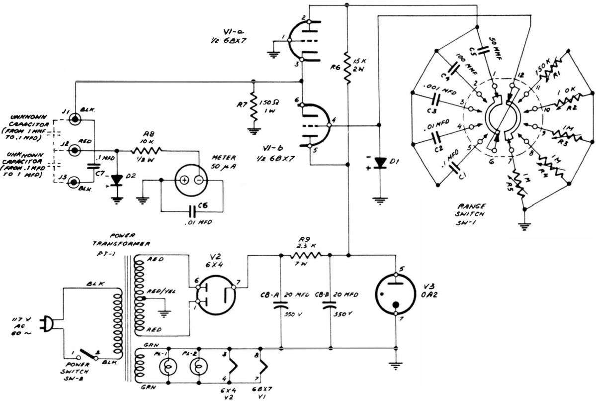
Fig. 2-12. Schematic of a simple capacitance meter.
