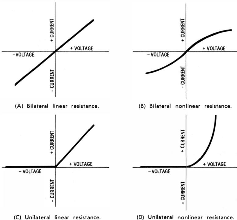
Fig. 1-14. Characteristic curves of bilateral and unilateral resistances.
