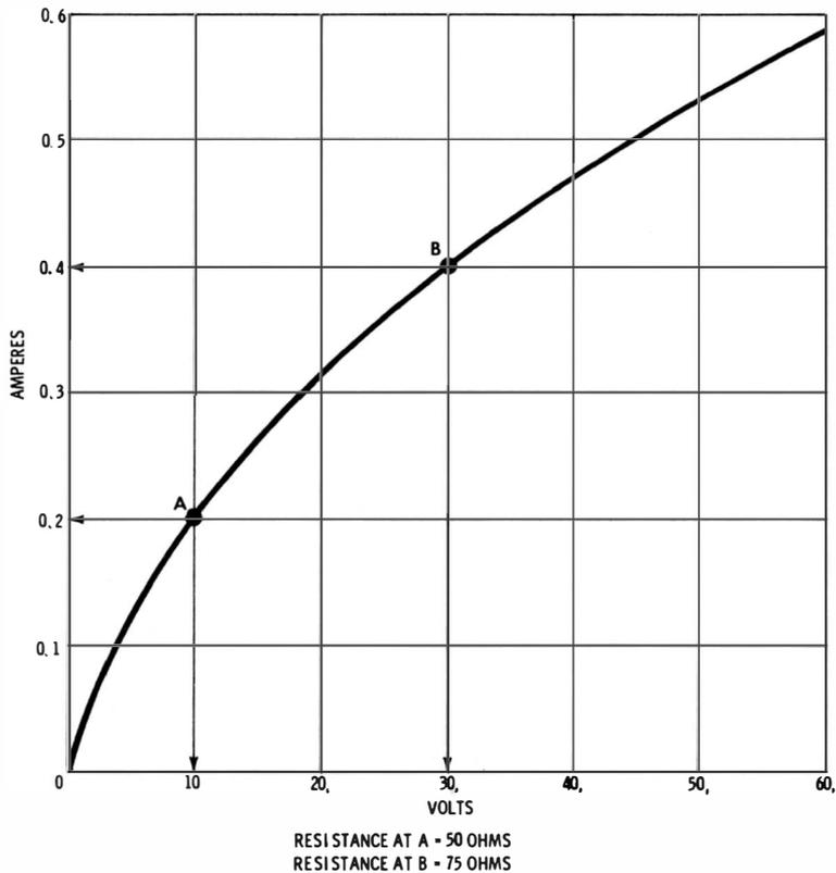
Fig. 1-7. Curve for positive temperature coefficient of resistance.
