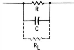
Fig. 2-22. The value of  $R_L$  when C is shunted by R is a difficult test.
