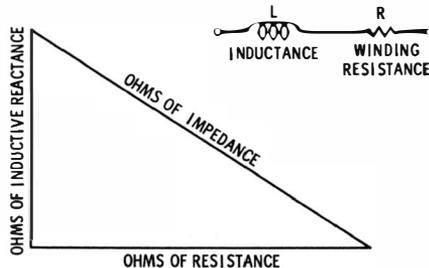
Fig. 3-18. Inductance and resistance form impedance.
