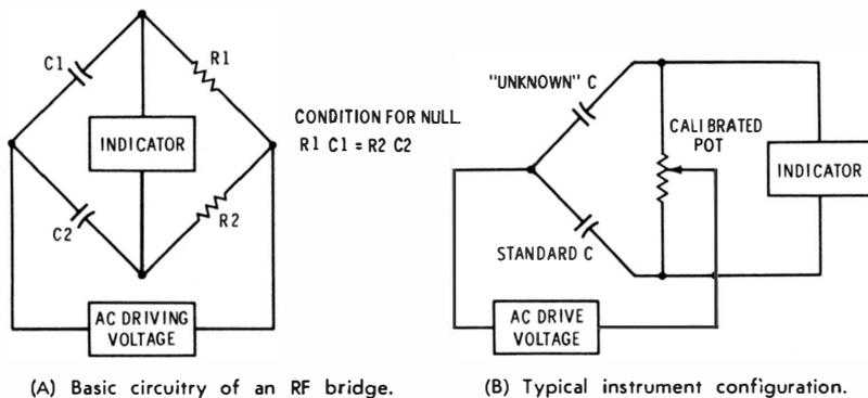
Fig. 2-2. RC bridge used to measure capacitor values.
