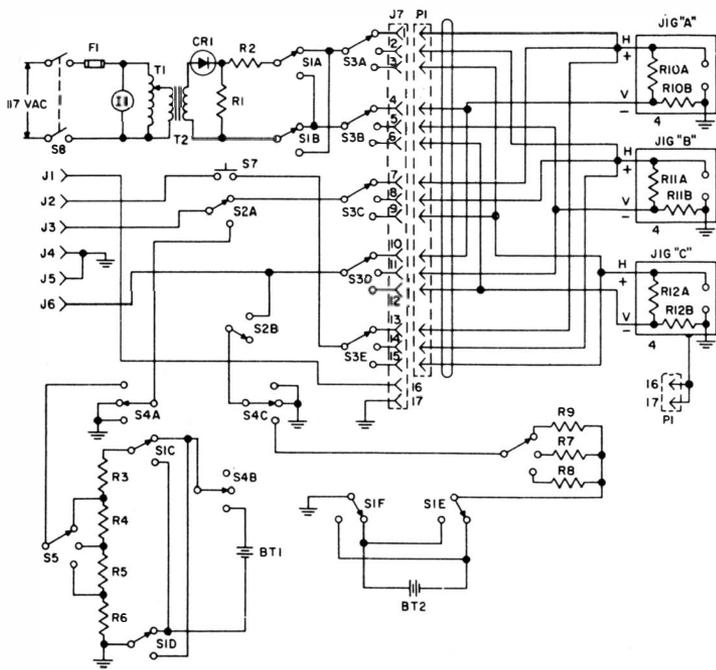
Fig. 1-24. A laboratory-type tunnel-diode tester.
