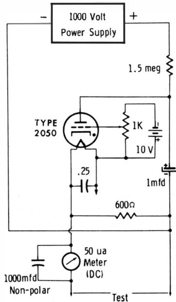
Fig. 2-25. Working-voltage pulse-test circuit.
