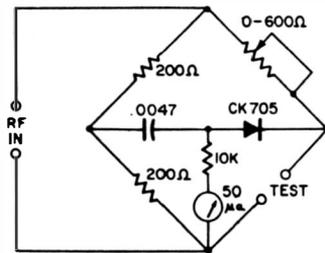
Fig. 4-2. Antenna-impedance meter circuit.
