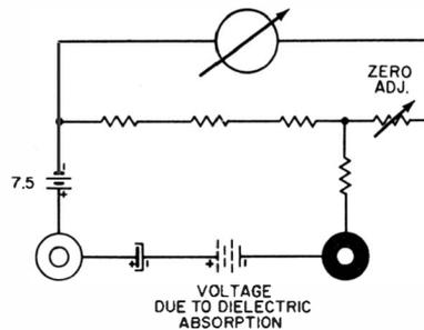
Dielectric absorption imposes another difficulty. Fig. 2-8 illustrates the nature of dielectric absorption. If an electrolytic capacitor is charged, and its terminals are then short-circuited, it might be supposed that all the charge is drained out of the capacitor. On the contrary, if the capacitor is allowed to stand open-circuited for a short time after the short-circuit is re-
