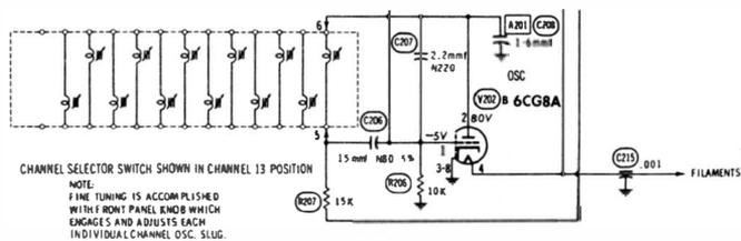
Fig. 4-11. C207 has negative temperature coefficient.
