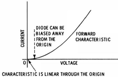
Fig. 4-20. Characteristic of a diode at low signal level.
