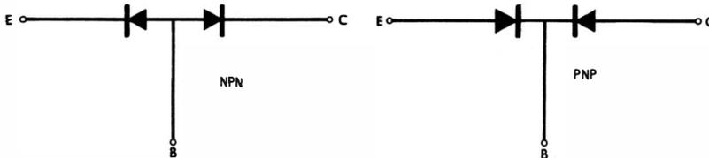
Fig. 1-25. Equivalent circuits for transistors.
