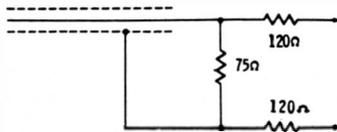
Fig. 5-18. Simple resistive balun.
