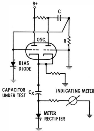
Fig. 2-13. Basic capacitance-meter circuit.
