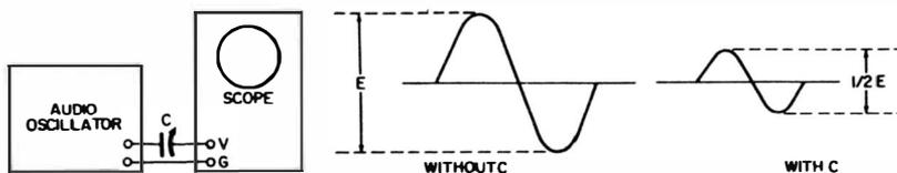
Fig. 2-26. Measuring input capacitance of an oscilloscope.
