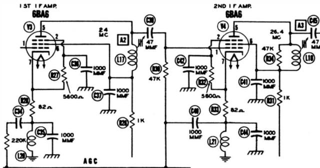
Fig. 4-12. L17 is reference in measurement of stray capacitance.
