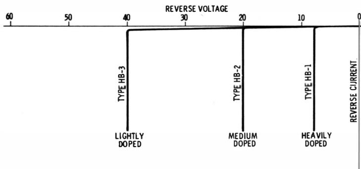
Fig. 1-15. The zener voltage point depends on the doping concentration used in the semiconductor materials.
