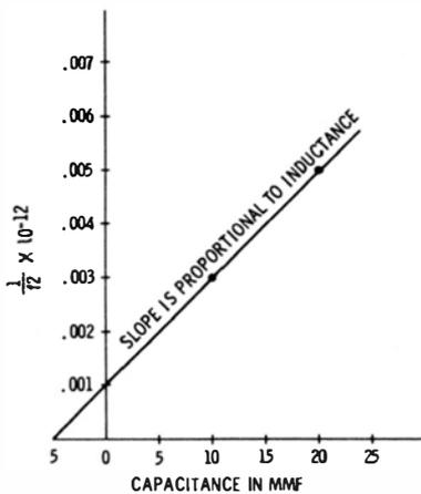
Fig. 4-15. Distributed capacitance is 5 mmf.
