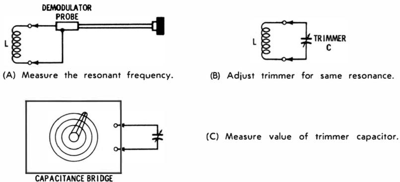
Fig. 4-14. Measurement of HF-probe input capacitance.
