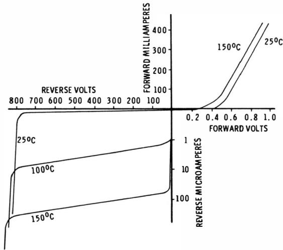
(A) Temperature effects on a typical silicon diode.
