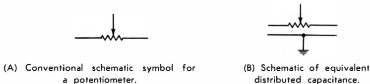
Fig. 5-22. Distributed capacitance in a potentiometer.
