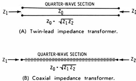
Fig. 5-16. Impedance matching with resonant stubs.
