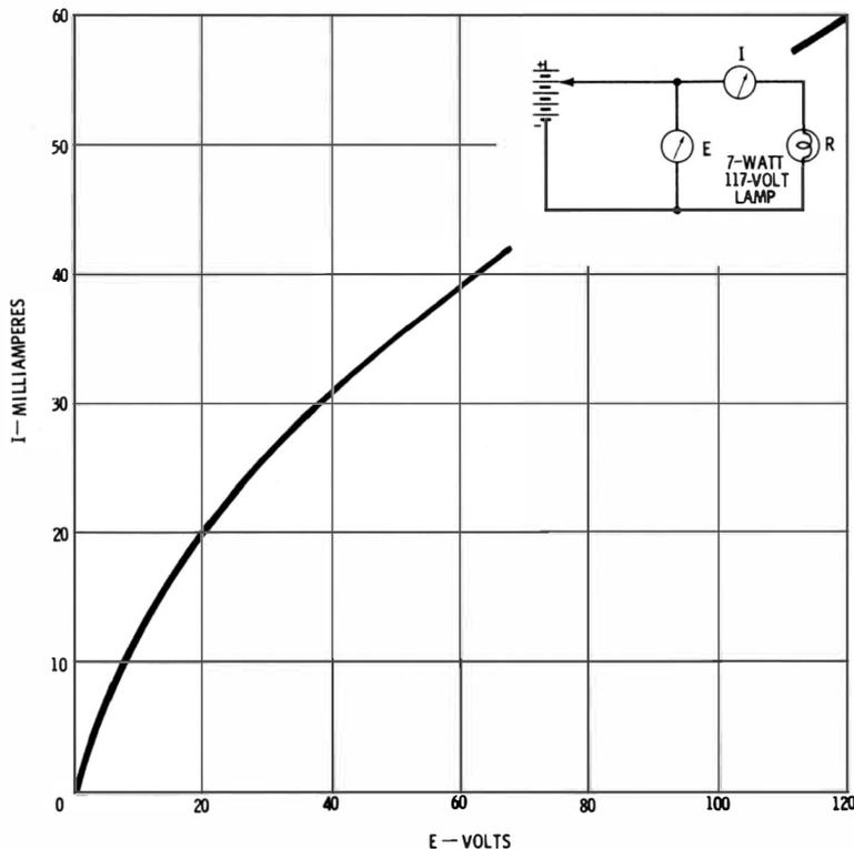
Fig. 1-2. An "electrical picture" of filament resistance.
