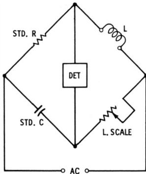
Fig. 3-13. Simplified schematic of inductance bridge.
