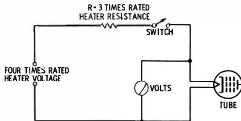
$$R = \frac{3E}{I} \text{ WHERE } E \text{ AND } I \text{ ARE THE RATED HEATER VOLTAGE AND CURRENT}$$
