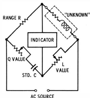
Fig. 3-14. Complete bridge for measuring L and Q.
