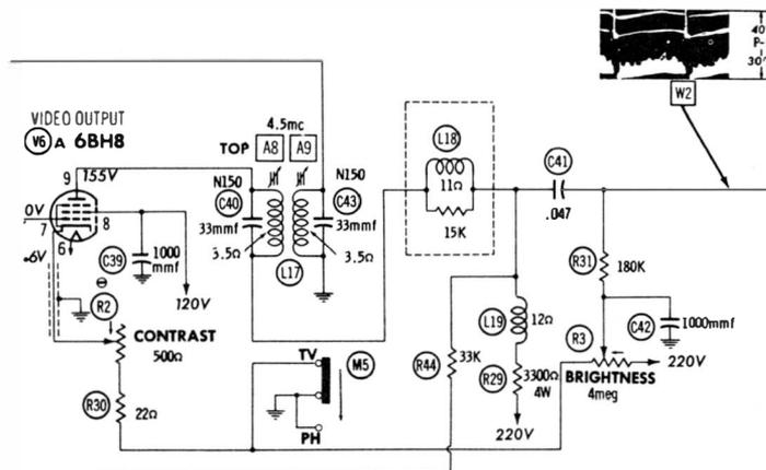
Fig. 2-28. Waveform W2 normally found on both sides of C41.
