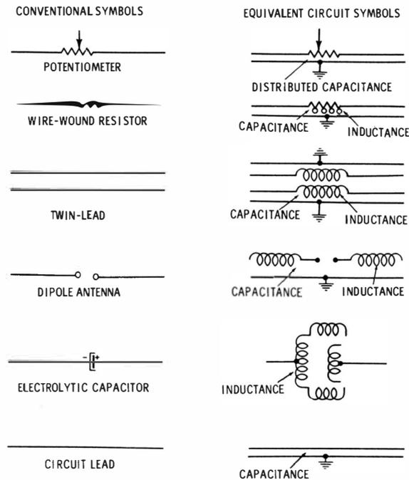
Fig. 5-3. Distributed parameters of components.
