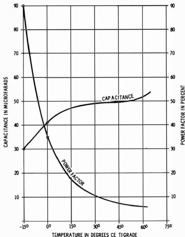
Fig. 2-9. Temperature coefficient of an electrolytic capacitor.
