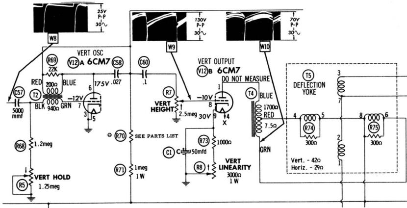
Fig. 1-11. Thermistor R70 stabilizes height and linearity.
