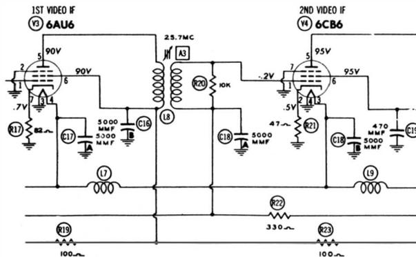
Fig. 3-5. Leakage in L8 upsets AGC action.
