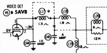
Fig. 3-1. Typical winding-resistance specifications.
