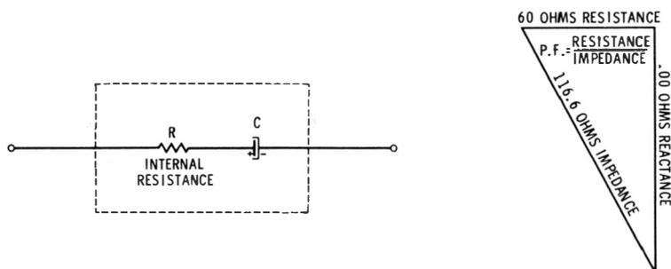
Fig. 2-6. Power factor defined as resistance divided by impedance.
