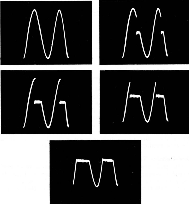
Fig. 6-21. Voltage waveforms from anode to cathode of a thyatron, showing the conduction time for various phase relationships between grid and plate voltage.
