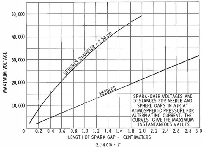
Fig. 6-1. Voltage-to-space relationship for spark gaps.
