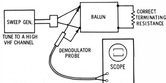
Fig. 5-15. Efficient balun shows flat trace.
