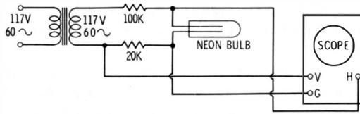
Fig. 6-8. Scope test of a neon bulb.
