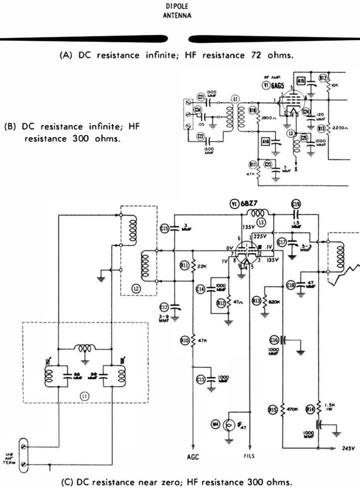
**Fig. 4-1. High-frequency resistance measurements.**
