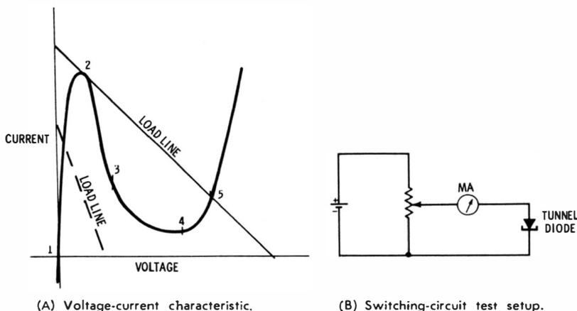
Fig. 1-23. Switching test for a tunnel diode.
