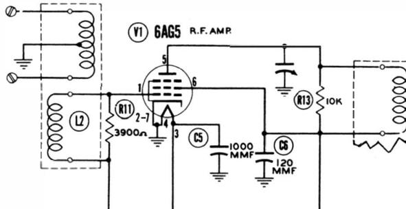
Fig. 4-8. Coupling controls input impedance.
