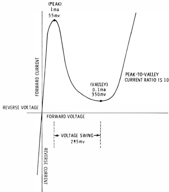
Fig. 1-21. Typical tunnel-diode voltage-current characteristic.
