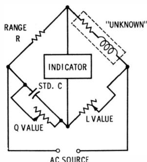
Fig. 3-15. Bridge for measuring low Q.
