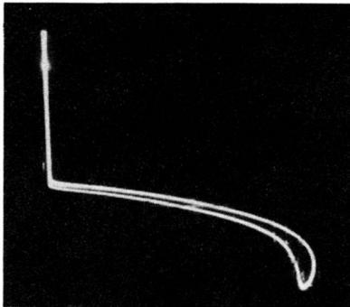
Fig. 1-19. Diode driven into negative-resistance region.
