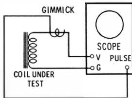
Fig. 3-8. Setup for ringing test.
