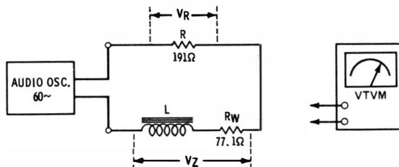
Fig. 3-22. Separation of inductance and winding resistance.
