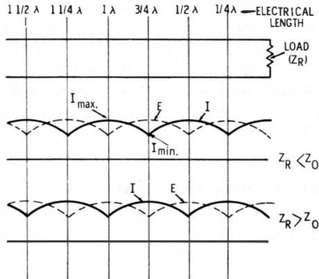
Fig. 5-9. Standing waves on a resistively terminated load.
