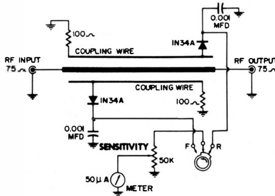
Fig. 5-13. Circuit of typical SWR/reflected-power meter.
