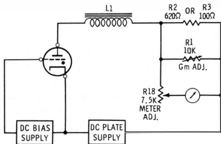
Fig. 6-17. Test circuit for a thyratron tube.
