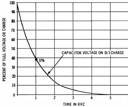
Fig. 2-15. Exponential curve of a capacitor discharging.
