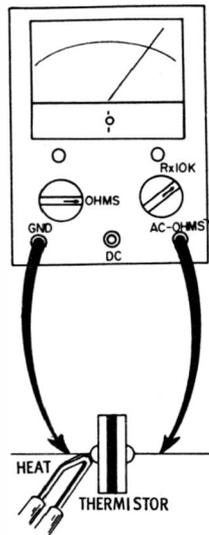
Fig. 1-10. Resistance decreases as the thermistor is heated.
