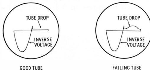
Fig. 6-19. Scope patterns obtained in thyatron test.
