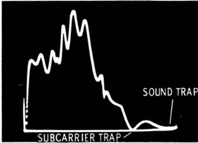
Fig. 5-20. Typical response curve of delay-line test.
