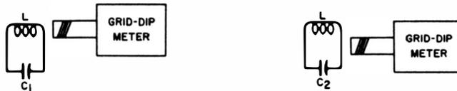
(A) First test where  $C_1$  equals 47 mmf. (B) Second test where  $C_2$  equals 100 mmf.
