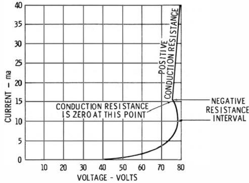
Fig. 6-3. VR tube often has a negative-resistance interval.
