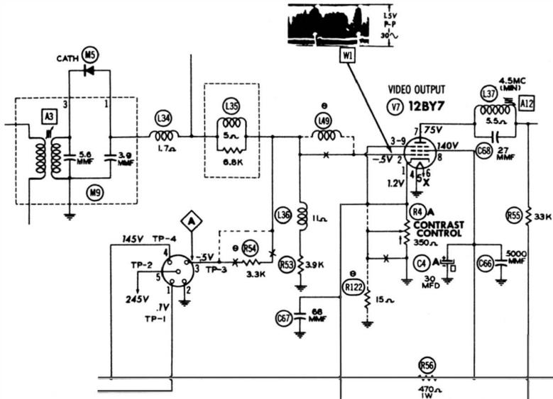
Fig. 4-18. Typical video-detector circuitry.
