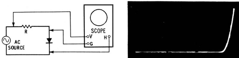
(A) Oscilloscope test setup for diodes.
