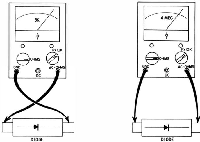
Fig. 1-12. Checking a semiconductor diode.
