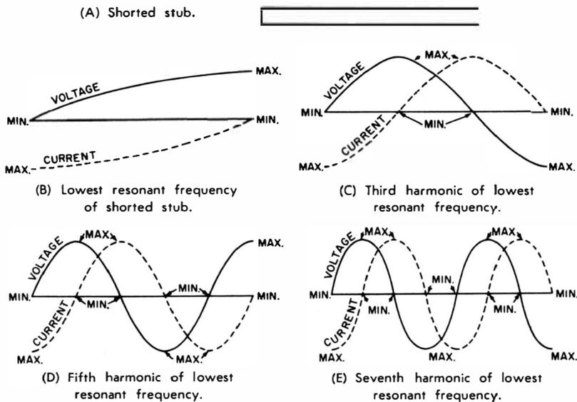
Fig. 5-4. Voltage and current distribution along a shorted stub.
