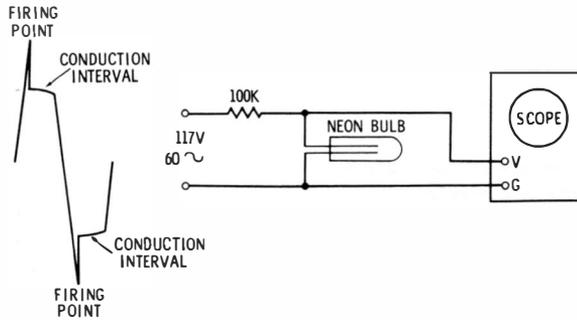
Fig. 6-12. Voltage drop displayed on a linear time base.
