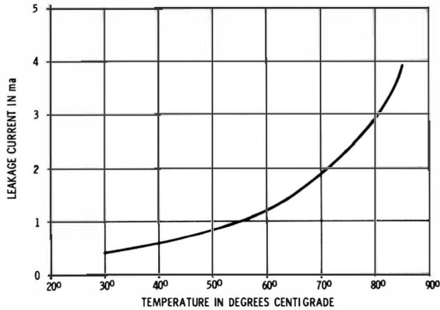
Fig. 2-10. Leakage current at rated working voltage for a typical electrolytic capacitor.
