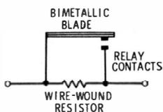
Fig. 1-6. Relay-type surge resistor.
