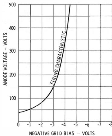
Fig. 6-6. Relation of grid bias and anode voltages to firing.
