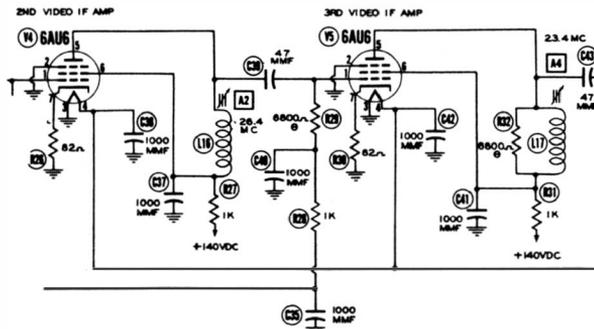
Fig. 2-31. C39 and C43 are checked for an open condition with a demodulator probe and scope.
