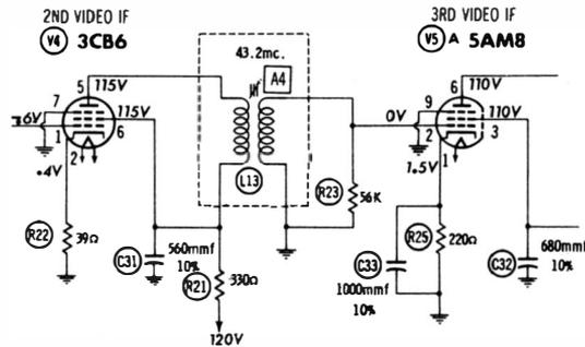
Fig. 3-2. Signal-circuit coil tested with demodulator probe.
