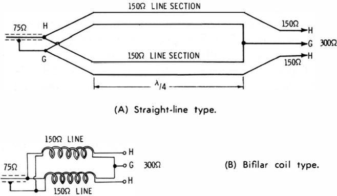
Fig. 5-14. Typical balun matching couplers.
