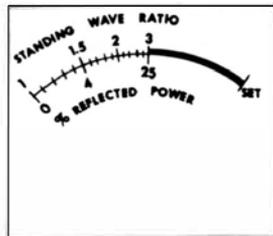
Fig. 5-12. Dial scale of SWR/reflected power meter.
