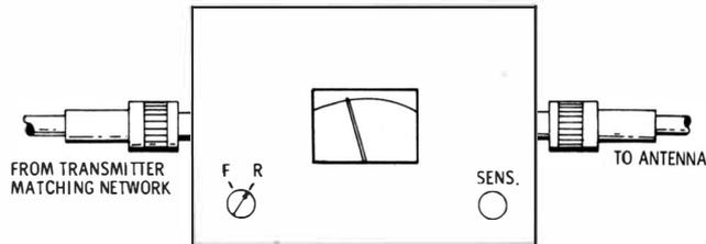
Fig. 5-11. SWR meter connected in a transmission line.
