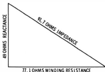
Fig. 3-23. The impedance triangle.
