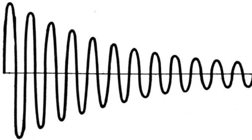
Fig. 3-9. Exponentially damped sine wave.
