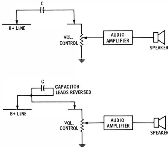
Fig. 2-16. If C is open, there is no click from the speaker in either the first or the second test.
