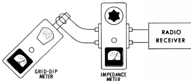
Fig. 4-6. Checking input impedance of a radio receiver.
