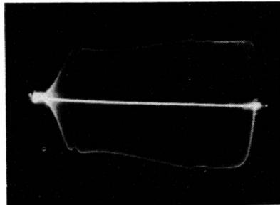
Fig. 3-12. Frequency response of scope vertical amplifier.
