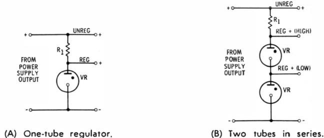
Fig. 6-4. Basic configuration for VR tubes.
