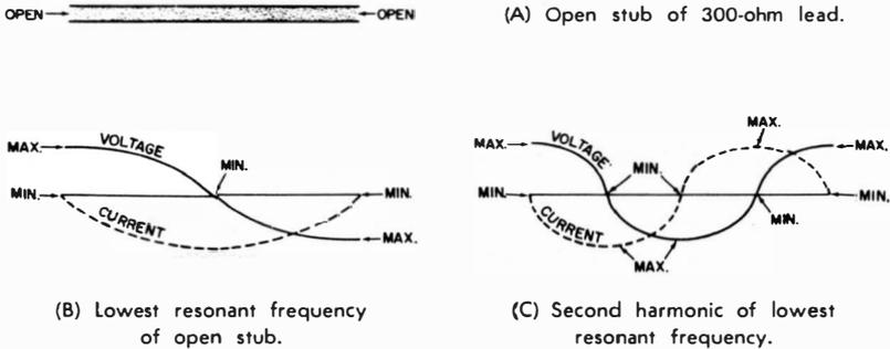
**Fig. 5-7. Voltage and current distribution on an open stub.**
