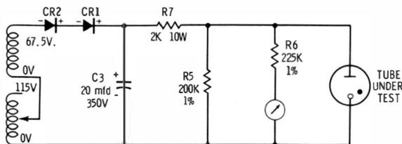
Fig. 6-14. A test circuit for VR tubes.
