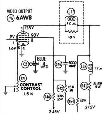
Fig. 4-9. C46 bypasses inductive reactance.
