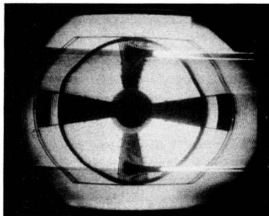
Fig. 3-3. Pattern showing regenerative IF amplifier.
