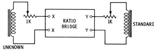
Fig. 3-19. Potentiometers used to equalize Q values.
