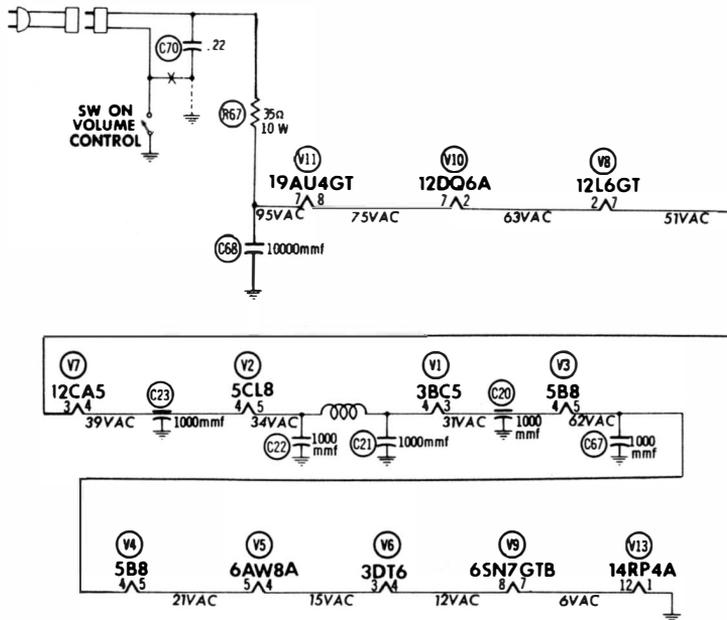
Fig. 1-4. A typical series heater string.
