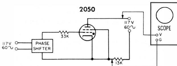
Fig. 6-20. A conduction-angle scope test.
