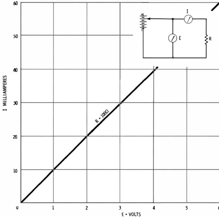
Fig. 1-1. An "electrical picture" of resistance.
