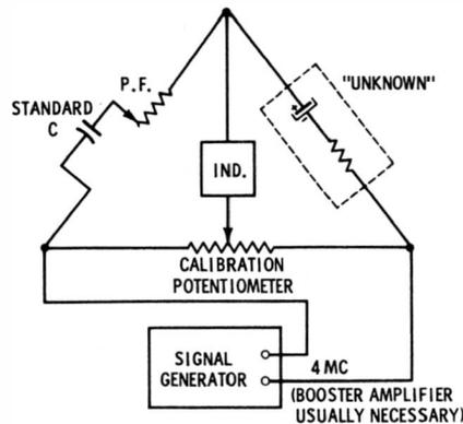
Fig. 4-10. Test for HF characteristic of electrolytic capacitor.
