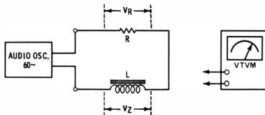
Fig. 3-21. Inductance test circuit.
