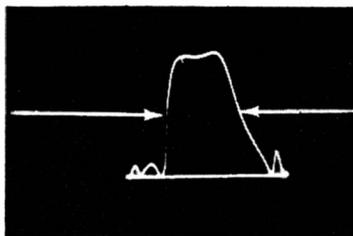
Fig. 4-17. Bandwidth is measured at half-voltage points.
