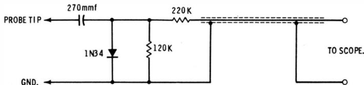
Fig. 4-19. Schematic of a demodulator probe.
