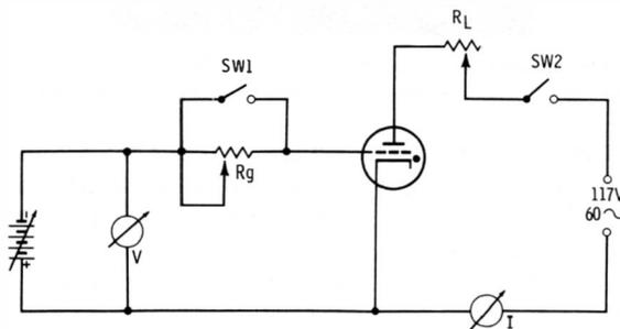
Fig. 6-23. Grid-emission test of a thyatron.
