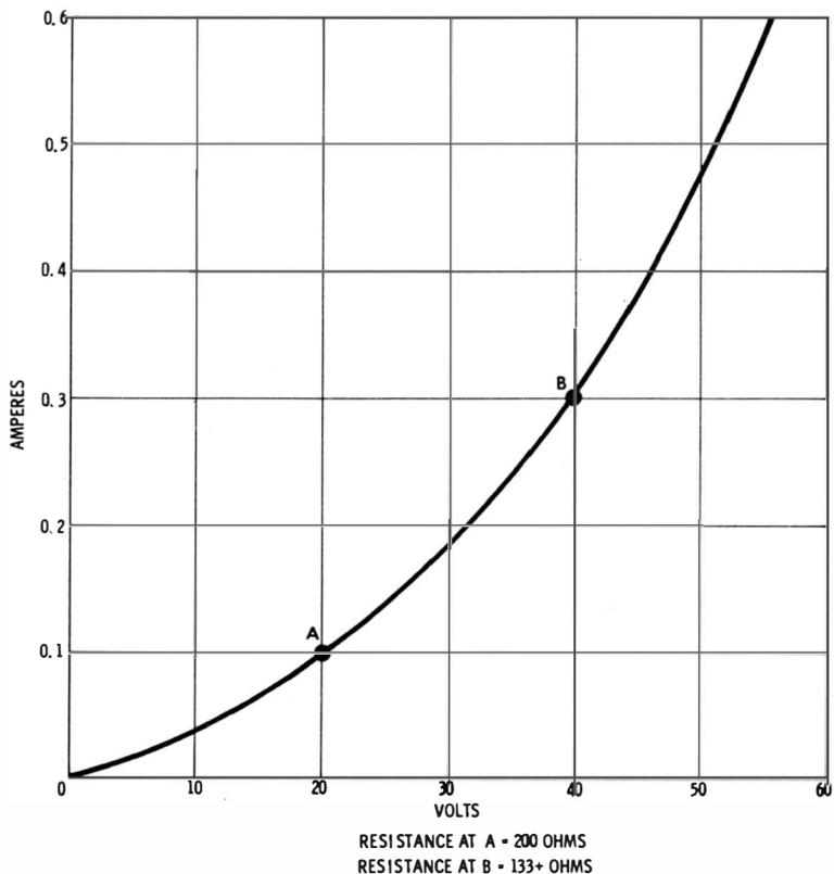
Fig. 1-8. Curve for negative temperature coefficient of resistance.
