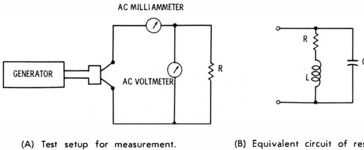
Fig. 5-21. Measuring reactance of a wirewound resistor.
