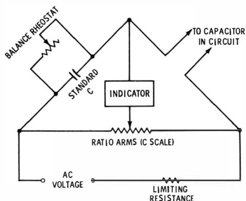
Fig. 2-17. Bridge for measuring capacitance shunted by resistance.
