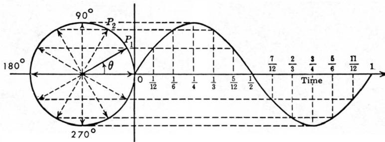
Fig. 6-22. Construction of sine wave based on angles of a circle.
