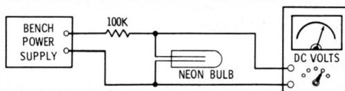
Fig. 6-7. Neon bulb firing-voltage test.
