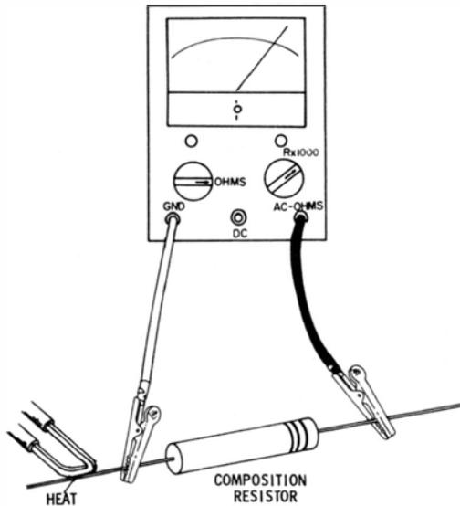
Fig. 1-3. Resistance increases with increase in temperature.
