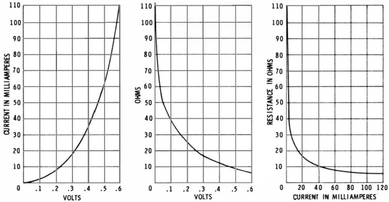
Fig. 1-9. Three methods of presenting negative temperature coefficient.
