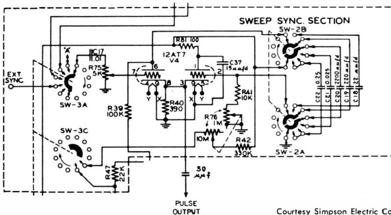
Fig. 3-7. Typical pulse take-off circuit.
