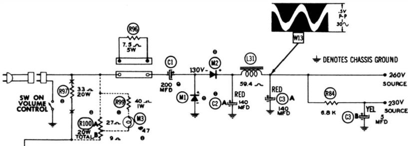
Fig. 2-30. Waveforms indicate condition of filters.
