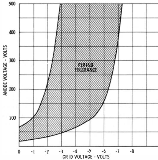
Fig. 6-18. Firing tolerance for a typical thyatron.
