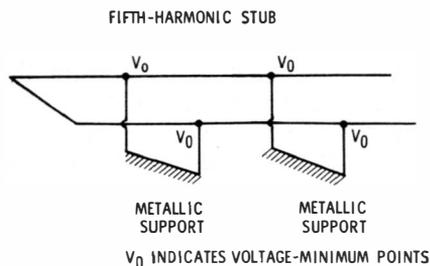
Fig. 5-5. Metallic insulators at minimum voltage points.
