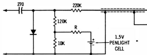
Fig. 4-21. Biased-diode demodulator probe.
