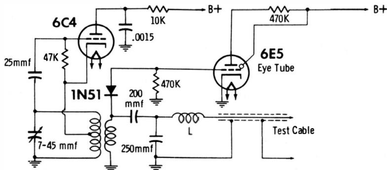
Fig. 2-23. Basic circuit for the "opens" test in the RF-type checker.
