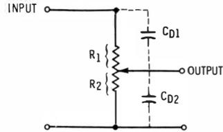
**Fig. 5-24. Output is undistorted when  $R_1 C_{D1} = R_2 C_{D2}$ .**
