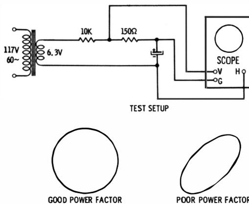
Fig. 2-32. Oscilloscope test of the power factor of an electrolytic.
