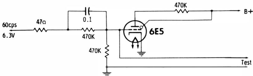
Fig. 2-24. A shorted capacitor kills the bias on the 6E5 and opens the eye.
