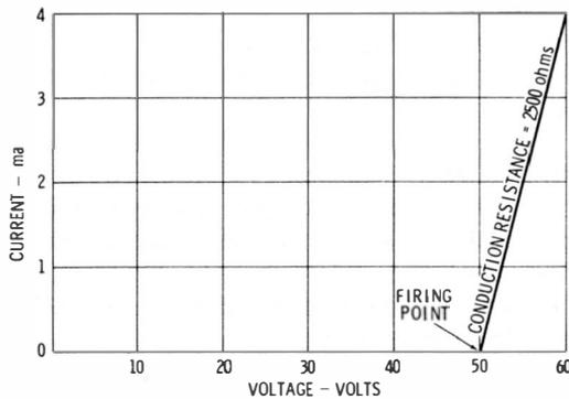
Fig. 6-2. Neon-bulb characteristic.
