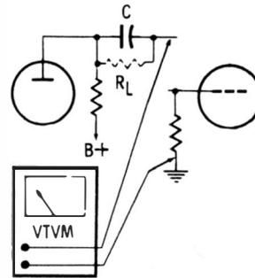
Fig. 2-19. Sensitive leakage test.
