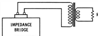
Fig. 3-25. Test of reflected resistance.
