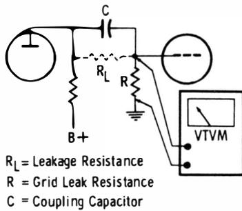
Fig. 2-18. Test for leakage current.
