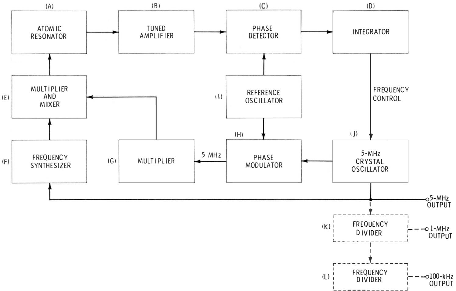
The output of the resonator is amplified (Stage B) and, through phase detector C and integrator D corrects the frequency of the crystal oscillator. This oscillator thus may be described as an atomic-resonator-controlled oscillator operated in a phase-locked system.
