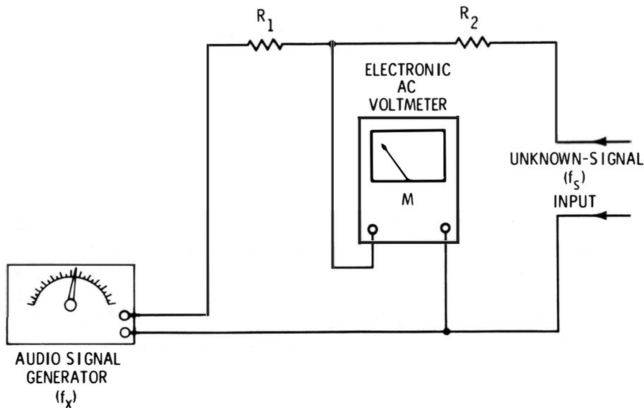
Fig. 2-2. Voltmeter method of measuring audio frequency.
