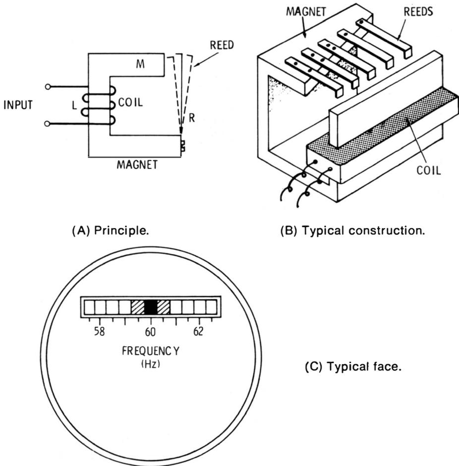
**Fig. 2-4. Reed-type frequency meter.**
