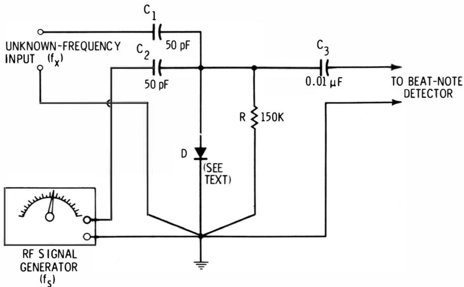
**Fig. 3-5. Signal-generator method of rf measurement.**
