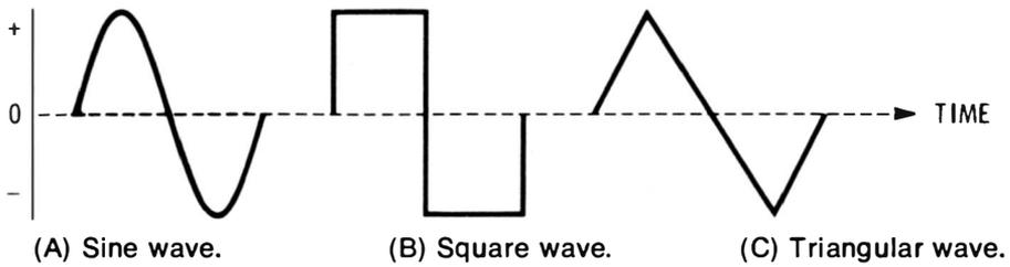
**Fig. 1-1. Typical single ac cycles.**
