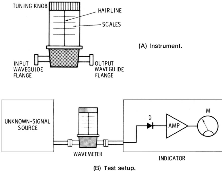
**Fig. 3-2. Microwave wavemeter.**
