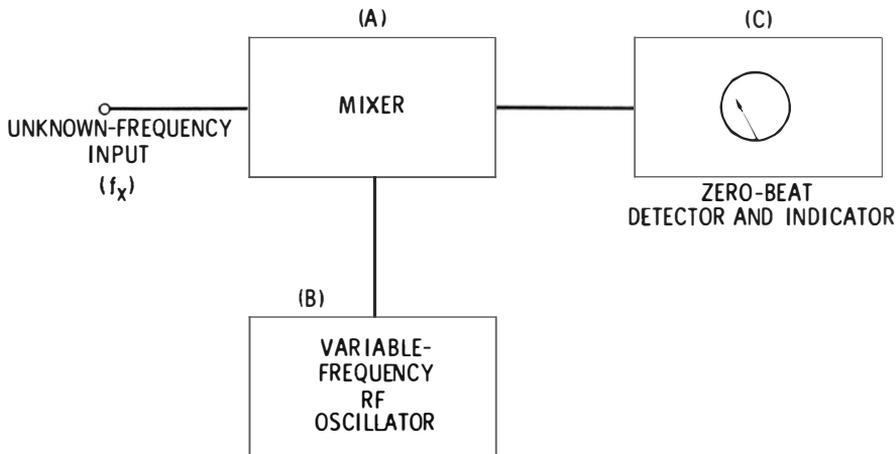
**Fig. 3-6. Heterodyne frequency meter.**
