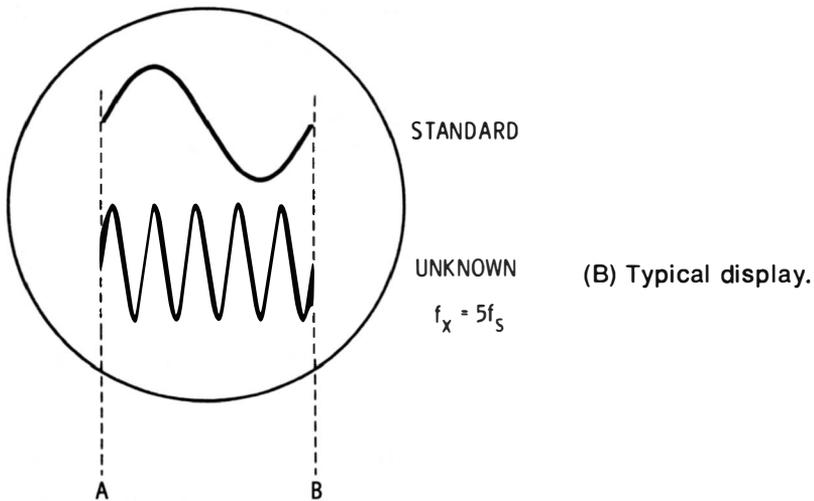
Fig. 2-13. Arrangement for dual-trace oscilloscope.
