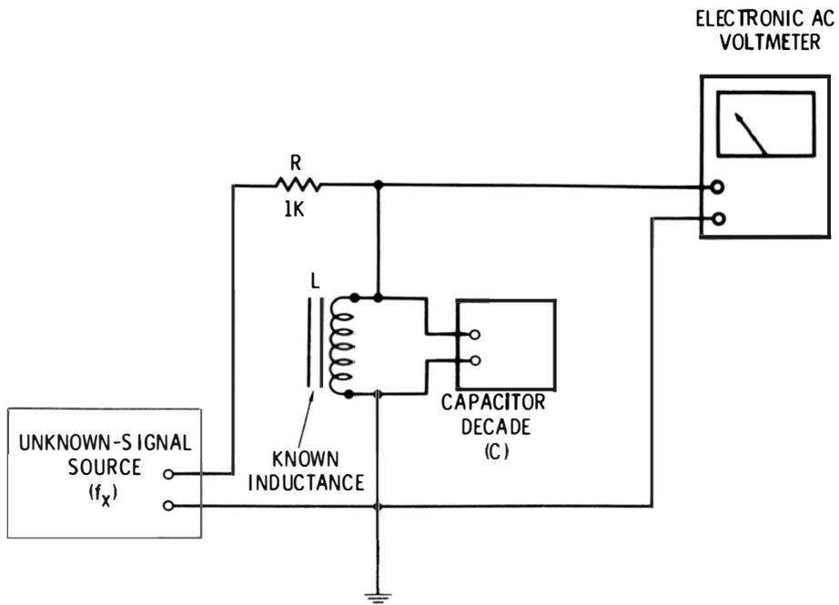
**Fig. 2-17. Resonant circuit.**
