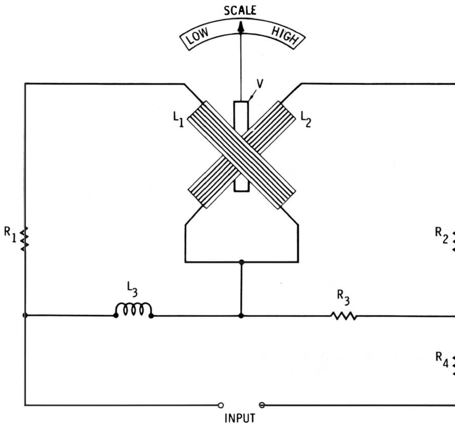
Fig. 2-3. Induction-type frequency meter.
