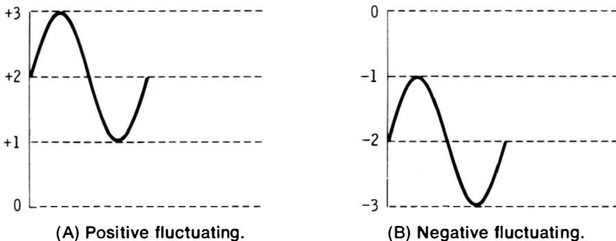
**Fig. 1-2. Typical single fluctuating cycles.**
