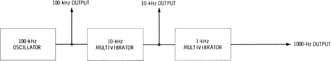
**Fig. 4-4. Secondary-standard layouts.**
