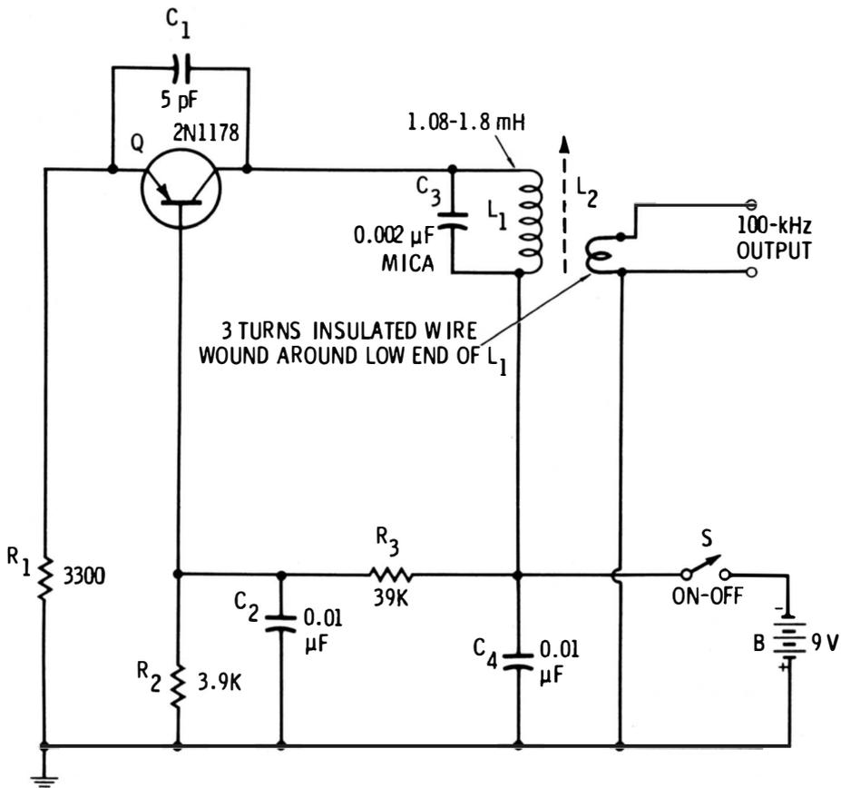
Fig. 4-5. Self-excited secondary standard.
