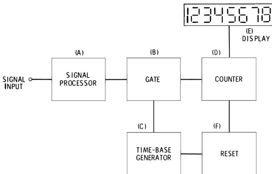
**Fig. 2-6. Digital-type electronic frequency meter.**
