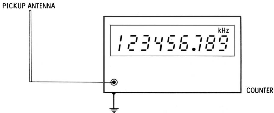
Fig. 3-7. Digital-type electronic frequency meter.
