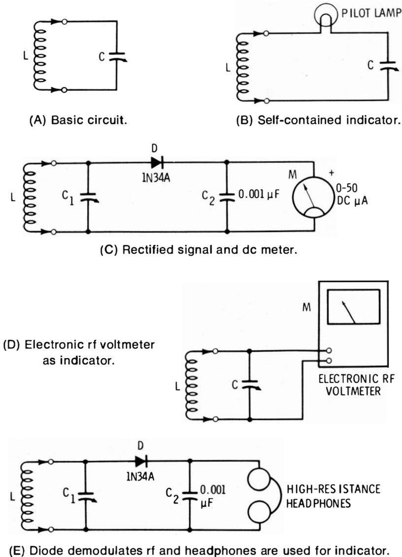
**Fig. 3-1. Absorption wavemeters.**
