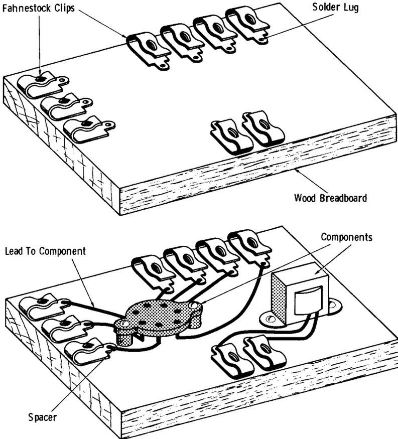
Fig. 4-3. Wooden breadboards.
