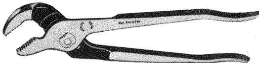
**Fig. 2-4 Tongue and groove pliers.**
