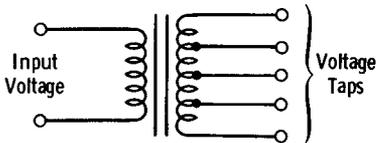
Fig. 3-18. Voltage-adjusting transformer.
