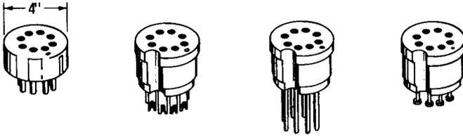
**Fig. 6-15. Sockets for integrated circuits.**
