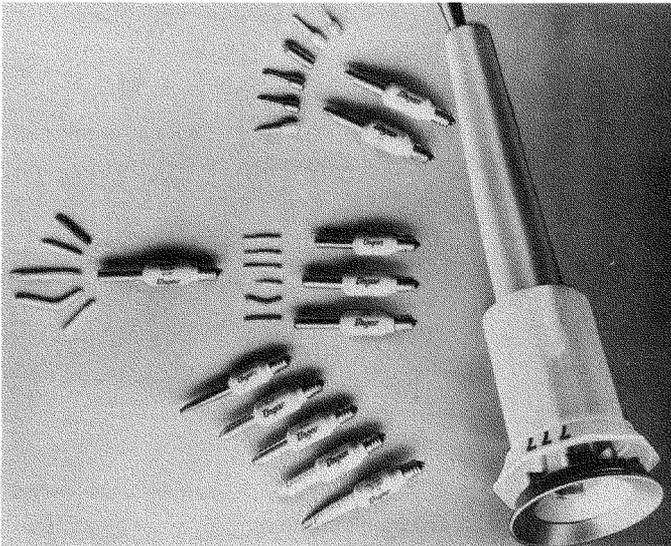
**Fig. 2-7. Soldering iron and replacement tips.**
