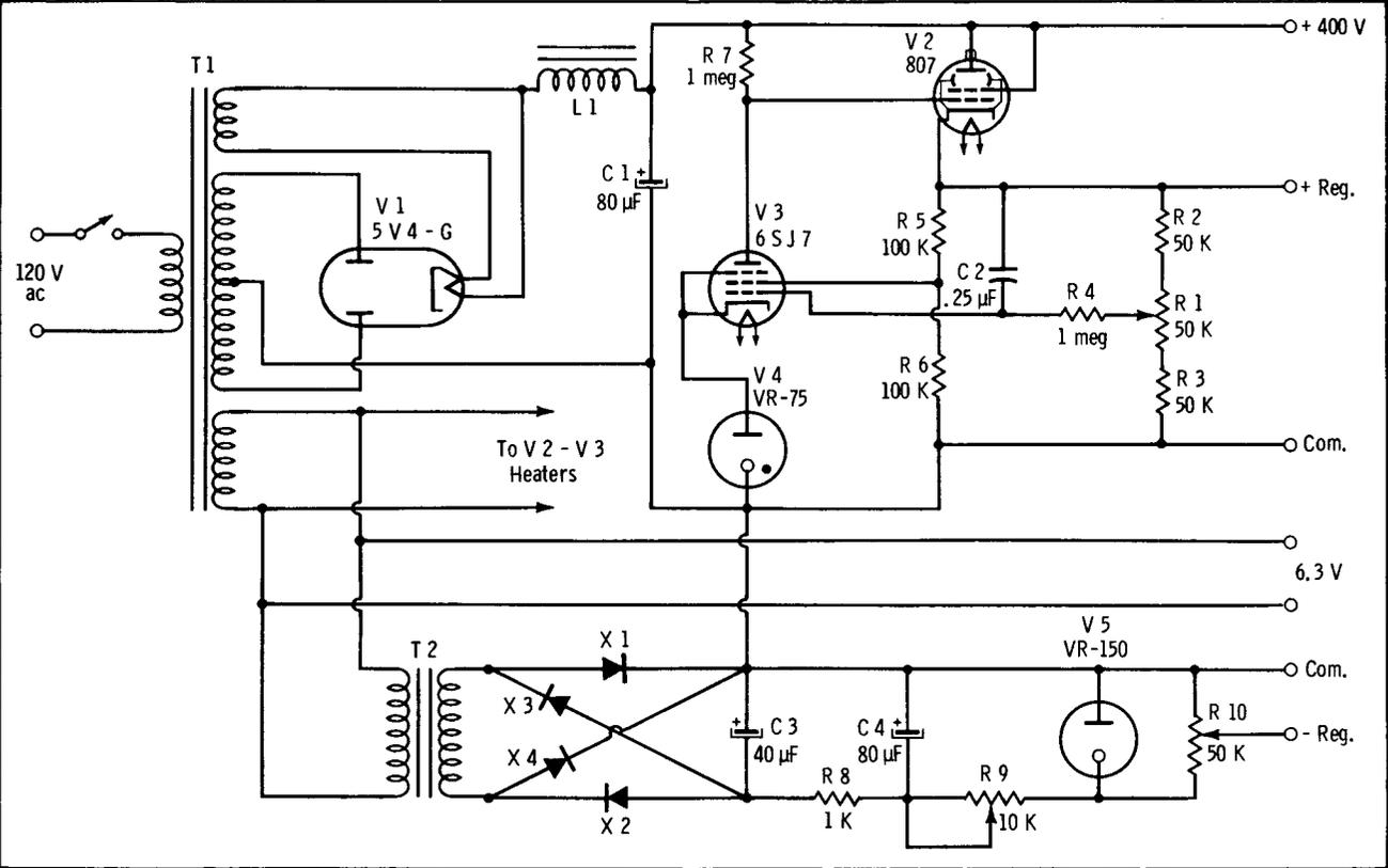
Fig. 4-7. Schematic of regulated power supply.
