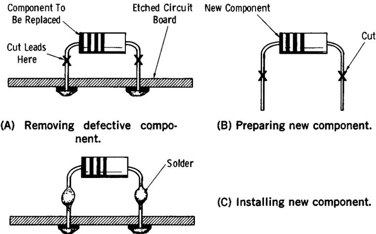
**Fig. 2-14. Method of replacing defective component.**
