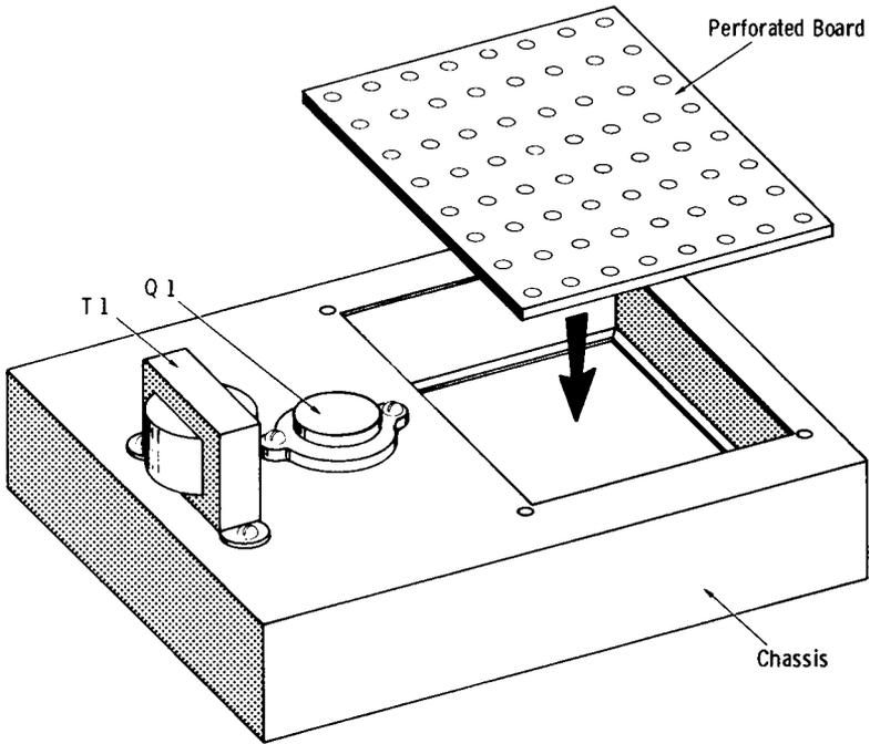
**Fig. 4-12. Integral power-supply breadboard.**
