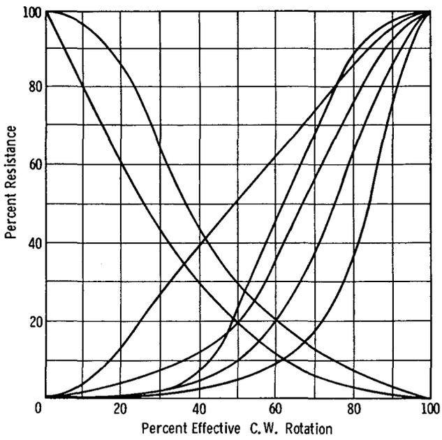
**Fig. 3-5. Potentiometer resistance tapers.**
