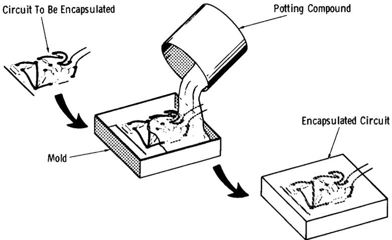
**Fig. 1-20. Encapsulated circuit.**
