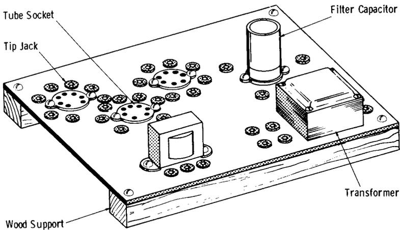
**Fig. 4-1. Simple breadboard chassis.**
