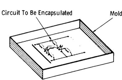
(A) Placing circuit in mold.
