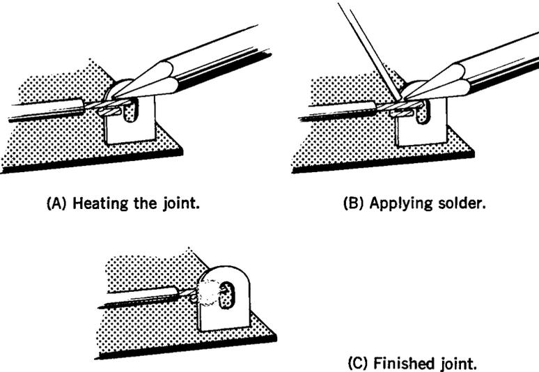
Fig. 2-11. Proper soldering techniques.
