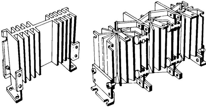
**Fig. 5-5. Transistor heat sinks.**
