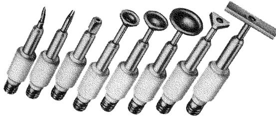
**Fig. 2-15. Desoldering tips.**
