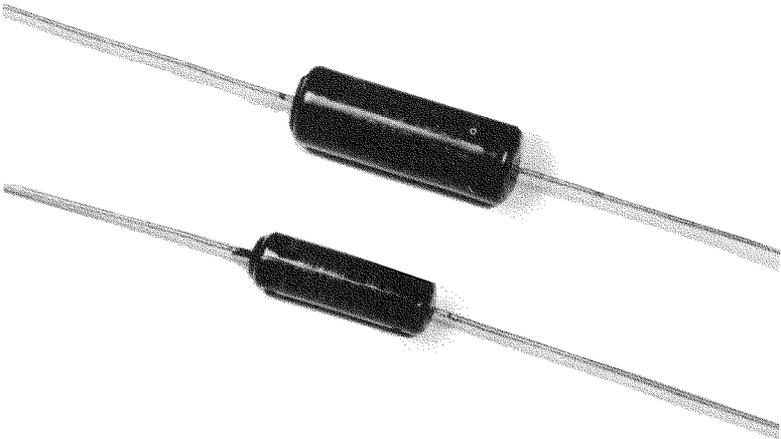
(B) Deposited-film resistor.
