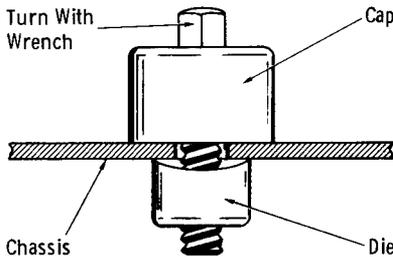
Fig. 1-3. Operation of a chassis punch.
