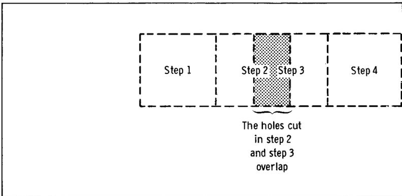
Fig. 1-4. Successive holes with square chassis punch.
