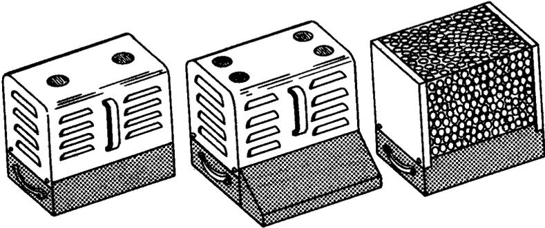
**Fig. 1-16. Amplifier foundations.**
