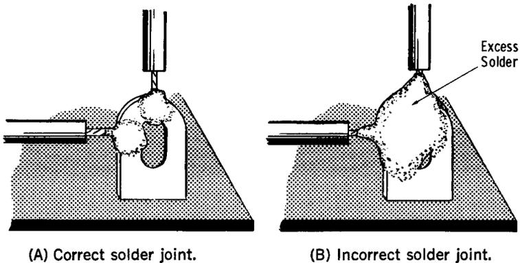
**Fig. 2-12. Correct and incorrect soldering techniques.**
