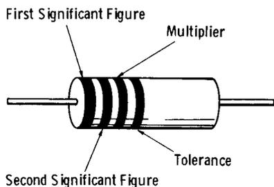
**Fig. 3-1. Arrangement of color coding bands.**
