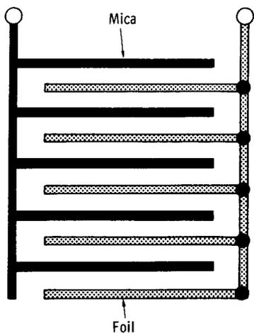
(A) Construction of a typical mica capacitor.
