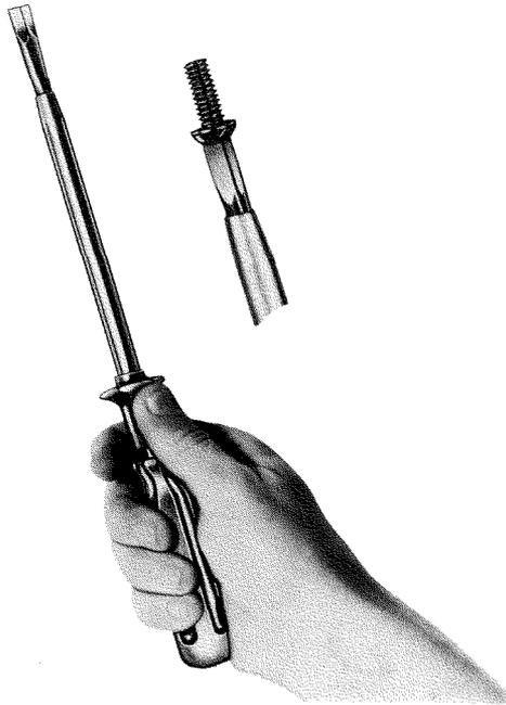
**Fig. 1-8. Screw holding screwdriver.**
