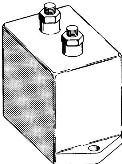
(C) High-capacitance mica capacitor.
