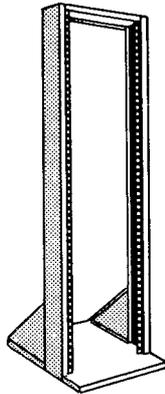
Rack panels are available in either steel or aluminum. Panel thickness may be either  $\frac{1}{8}$  inch or  $\frac{3}{16}$  inch.
