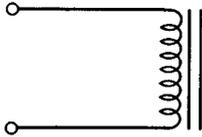
Fig. 3-22. Filter choke.
