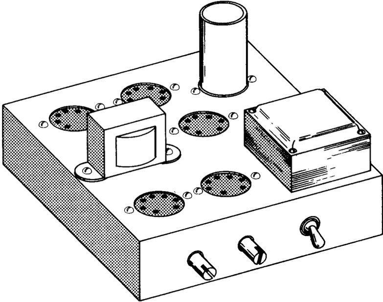
**Fig. 4-4. Permanent breadboards.**
