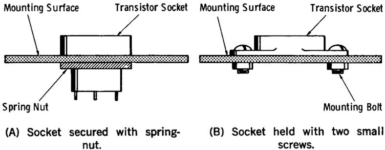
Fig. 5-3. Methods of mounting small transistor socket.
