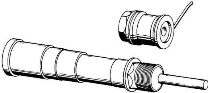
**Fig. 3-13. Piston capacitors.**
