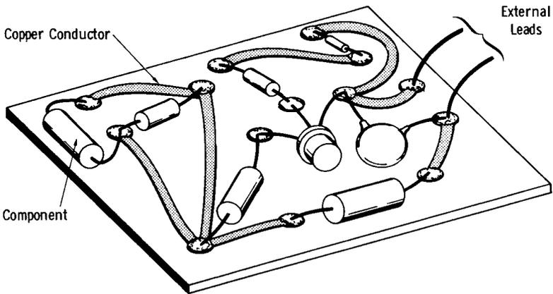
**Fig. 1-19. Etched circuit board.**
