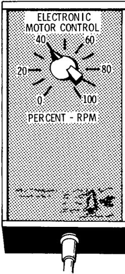
**Fig. 2-16. Variable speed control.**
