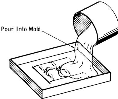
(C) Pouring potting compound in mold.
