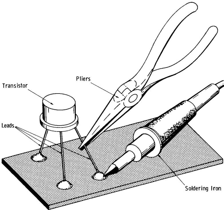
**Fig. 5-1. Using pliers as a heat sink.**
