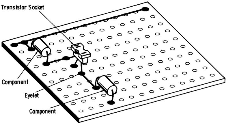
Fig. 4-8. Perforated-board breadboard.
