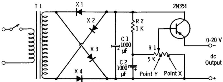
X 1, X 2, X 3, X 4, = 1 A, 100 Piv. Silicon Diodes
