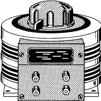
Fig. 3-17. Variable-voltage transformer.
