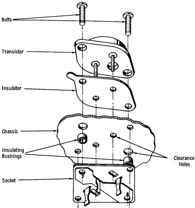
**Fig. 5-4. Method of power transistor mounting.**
