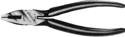
**Fig. 2-1. Electrician's side-cutting pliers.**
