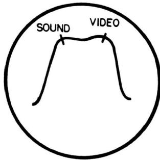
**Fig. 11-12. Idealized tuner response curve.**
