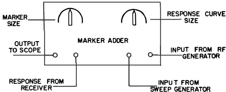
**Fig. 11-10A. Block diagram showing connections when using marker adder unit.**
