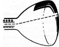
toward the positive plate and repelled from the negative plate (Fig. 1-6) because unlike electron charges attract and like charges repel each other. The electron beam is always negative and, therefore, is always attracted to the positive plate.
