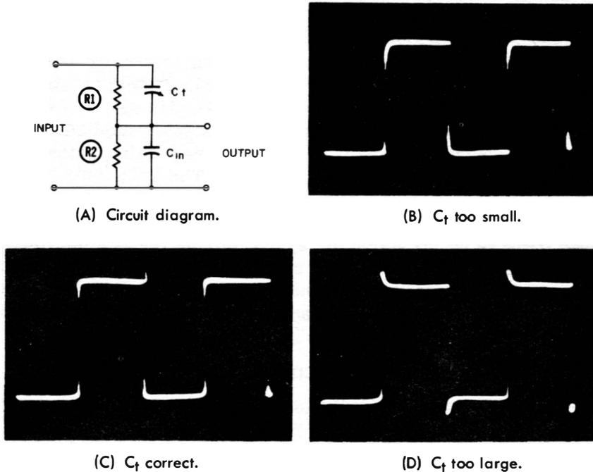
**Fig. 8-3. A frequency compensated attenuator and the effect of various degrees of adjustment on a square wave signal.**
