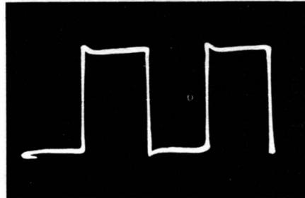
**Fig. 10-2. Preamplifier Response to the 1 kc square wave. Tone controls were adjusted for flat response.**
