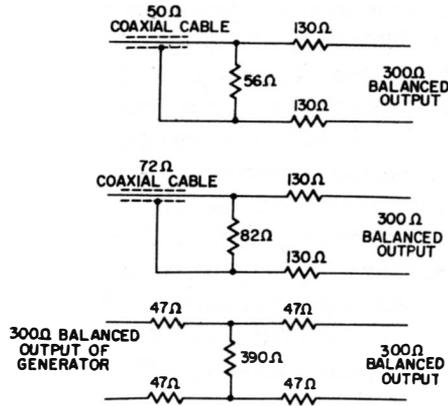
**Fig. 11-5. Sweep generator attenuator pads.**
