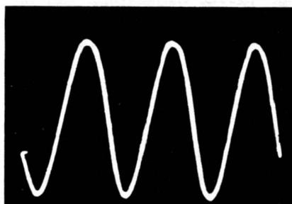
**Fig. 12-12B.** Sine-wave output of triode.
