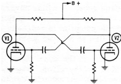
Fig. 3-7. Basic multivibrator circuit.
