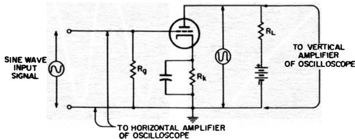
**Fig. 12-11. Method of connecting oscilloscope to an amplifier stage to view the operating characteristic curve.**
