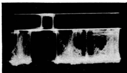
**Fig. 8-6. Oscilloscope response using amplifier of 4-megacycle bandwidth.**
