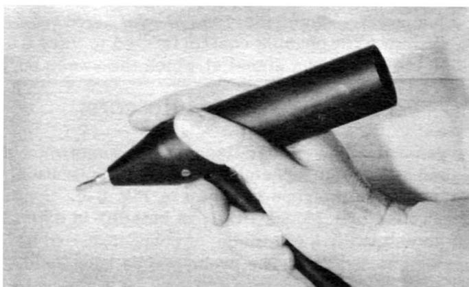
**Fig. 6-7. Probe assembly of the Probescope Model PO-1.**
