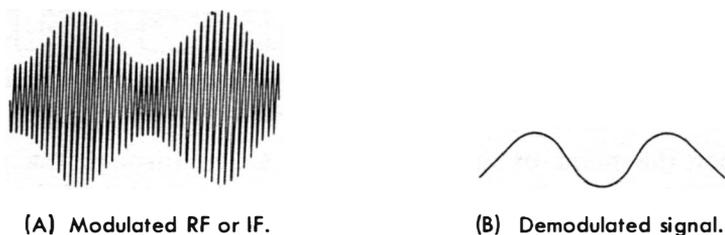
**Fig. 12-2. Response patterns obtained in signal tracing an AM radio receiver.**
