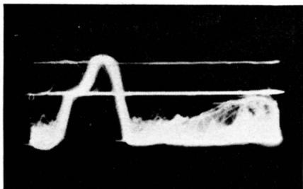
**Fig. 8-8. Response showing effect of added input capacitance.**
