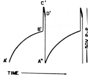
**Fig. 3-16. Waveform at pin 7 (second grid) of multivibrator of Fig. 3-12.**
