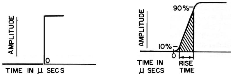
**Fig. 5-6. Diagram illustrating rise time.**
