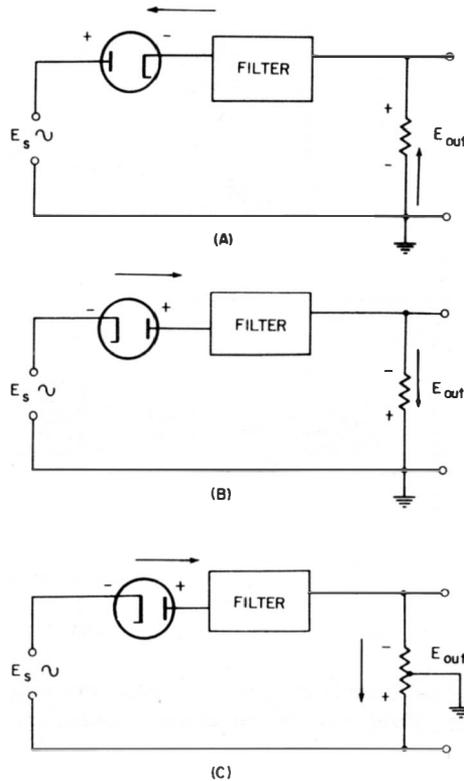
**Fig. 2-4. Several variations of half-wave rectifier circuits.**
