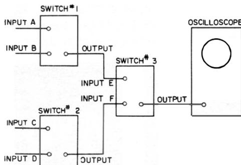
**Fig. 7-19. Electronic switch arrangement for viewing 4 signals simultaneously on an oscilloscope.**
