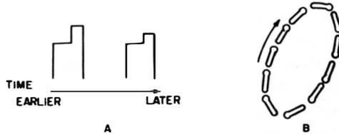
**Fig. 9-13. Intensity marker signal at A produces markers as at B. Beam rotation is as indicated by arrow.**
