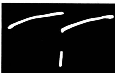
**Fig. 12-7. Vertical deflection waveform from vertical output stage.**
