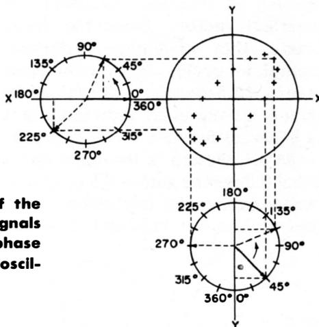
**Fig. 9-10. Graphical illustration of the manner in which two sine-wave signals of identical frequency but different phase develop a phase indication on an oscilloscope.**
