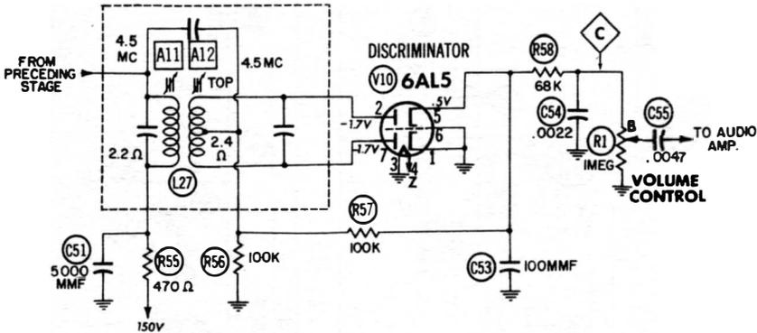
Fig. 11-7. Typical FM discriminator circuit.
