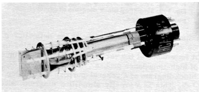
**Fig. 1-4. Electron gun of cathode-ray tube.**
