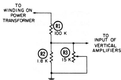
In this example, R3, the 15K-ohm control, is adjusted to provide .1-volt peak-to-peak for calibration of the vertical amplifier. In another example, the network was connected to one of the low voltage rectifier plate windings of the power transformer and adjusted to give a basic calibration voltage system, using a regulator tube to stabilize the calibration voltage.
