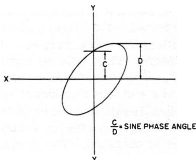
manner: Find the value of the sine by the preceding method. Locate this value and corresponding angle in the sine table. An angle between 0 and 90 degrees will be given, which should then be subtracted from 180 degrees for the final correct value.
