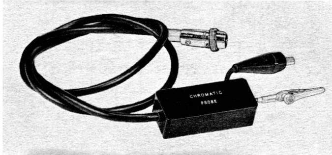
**Fig. 7-7. The Simpson chromatic probe.**
