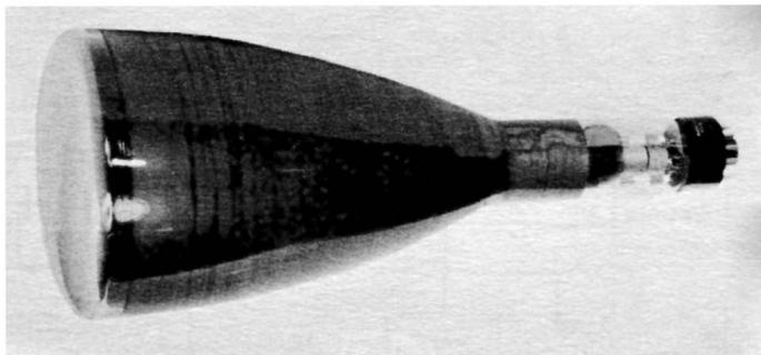
**Fig. 1-3. Modern 5-inch cathode-ray tube.**
