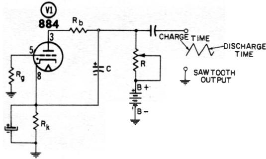
**Fig. 3-4. Basic Thyratron sawtooth oscillator.**
