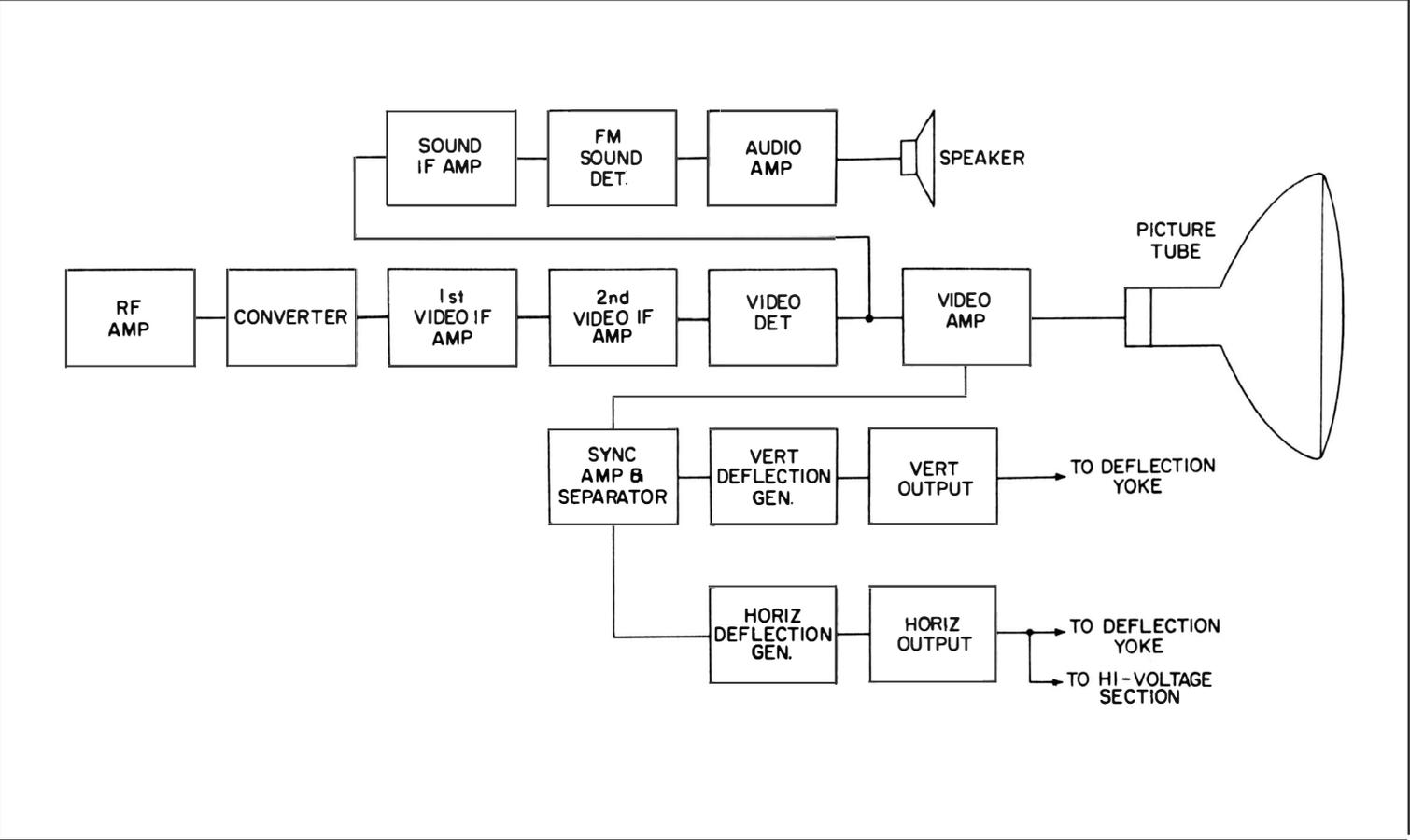
Fig. 12-3. Block diagram of typical TV receiver.
