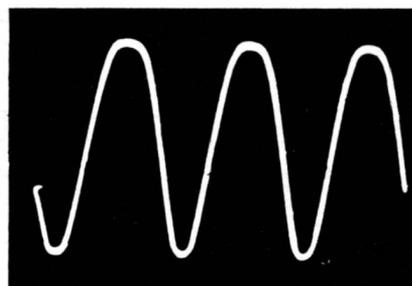
**Fig. 12-13B. Sine-wave output showing slight amount of distortion.**
