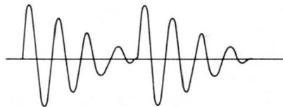
higher value of signal voltage is required for this method as compared with the method of Fig. 3-10. A square-wave signal displayed in this manner results in a "cog wheel" pattern rather than the pattern of Fig. 3-10.
