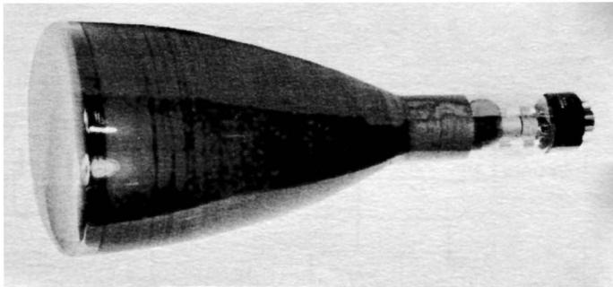
**Fig. 1-3. Modern 5-inch cathode-ray tube.**
