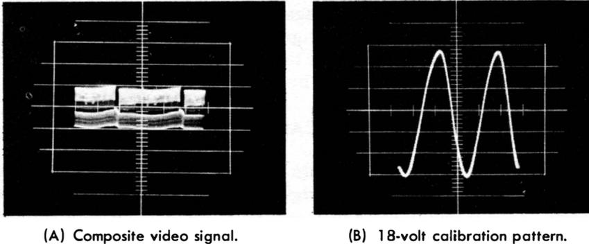
**Fig. 6-2. Photographs taken directly from the screen of a typical service scope.**
