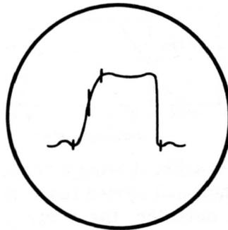
Since the sweep signals for the receiver response curve and marker adder are both taken from the same sweep generator, the marker will appear at its proper location when combined with the response curve. The marker signal does not pass through the receiver circuits and, therefore, is not attenuated by the trap circuits or amplified at peak response frequencies. The marker remains at the same amplitude on the oscilloscope screen as it is tuned across the entire response curve.
