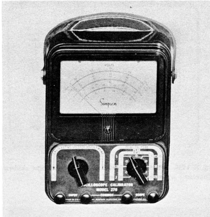
**Fig. 7-12A. Simpson Model 276 Oscilloscope Calibrator.**
