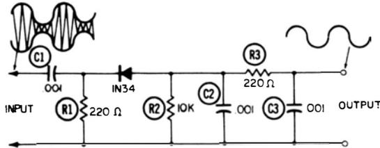
**Fig. 7-5. A crystal diode probe for demodulating RF signals.**
