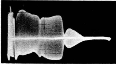
**Fig. 10-12. Normal response of video amplifier.**
