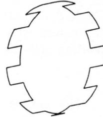
If a square-wave signal is applied to the horizontal input of the oscilloscope shown in Fig. 3-9, the resulting waveform appears as in Fig. 3-10. In this example the frequency of the square wave is eight times that of the signal used to develop the elliptical sweep.
