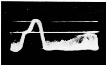
**Fig. 8-8. Response showing effect of added input capacitance.**
