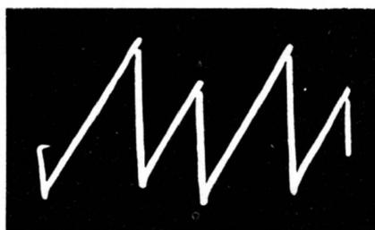
(B) Sawtooth signal developed at second section.
