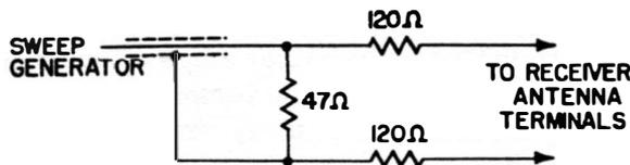
(C) Schematic diagram of terminating network.
