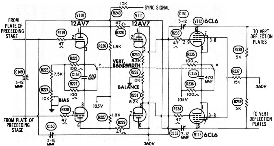
Fig. 5-2. Partial schematic diagram of the vertical amplifier of the Hickok Model 770 oscilloscope.
