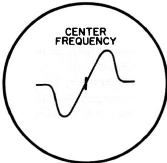
**Fig. 11-14. FM discriminator or ratio detector response curve.**
