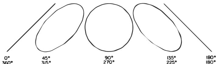
**Fig. 9-11. Phase indications from 0° to 360° at intervals of 45°.**
