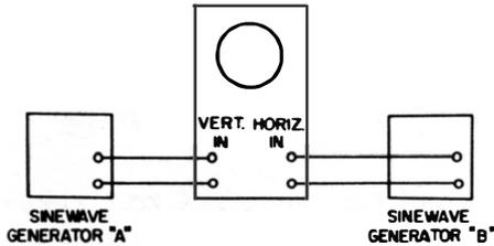
**Fig. 9-1. Method for generating Lissajous figures.**
