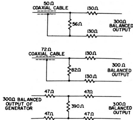
**Fig. 11-5. Sweep generator attenuator pads.**
