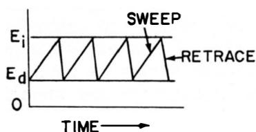
**Fig. 4-1. Free-running operation of a thyatron sweep oscillator.**
