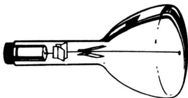
**Fig. 1-5. Path of electron beam through deflection-plate assembly.**
