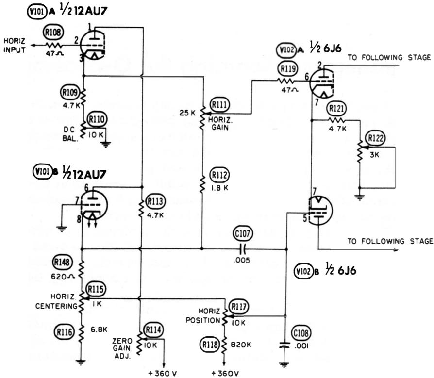
**Fig. 8-1. Input stage of an oscilloscope having DC balance adjustment.**
