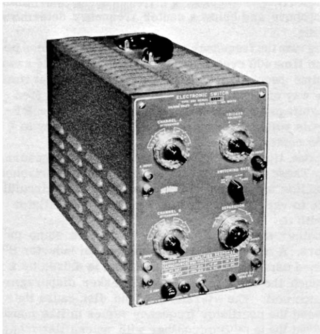
**Fig. 7-20. The DuMont Model 330 electronic switch.
