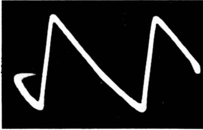
(A) Input signal to phase detector.
