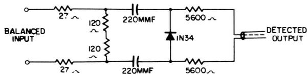
**Fig. 7-6. A balanced input demodulator.**
