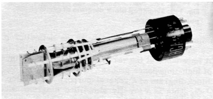
**Fig. 1-4. Electron gun of cathode-ray tube.**
