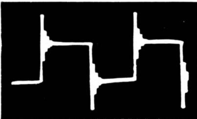
Fig. 10-7. Moderate ringing induced by application of square waves.
