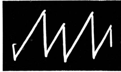
(B) Sawtooth signal developed at second section.
