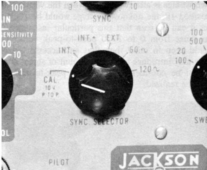
**Fig. 6-3. Sync selector includes CAL position for internal calibrating voltage.**
