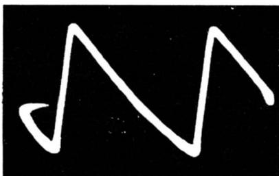
(A) Input signal to phase detector.
