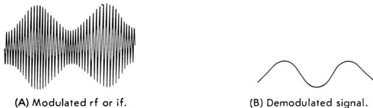
**Fig. 12-2. Response patterns obtained in signal tracing an a-m radio receiver.**
