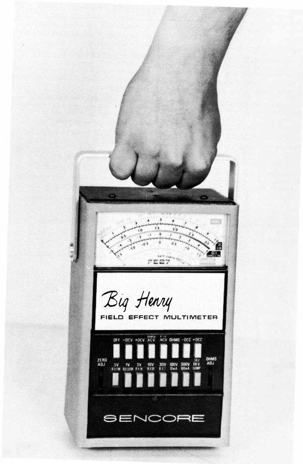
Fig. 8-12. Sencore Model FE27 field-effect multimeter.
