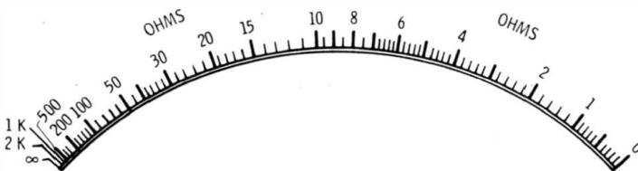
**Fig. 4-2. Resistance scale of vom showing crowded high-resistance end of scale.**
