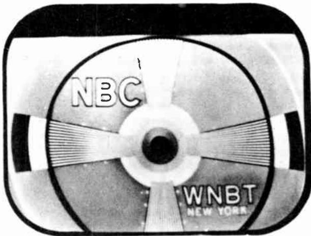
Fig. 129. Vertical Centering Control Misadjusted
