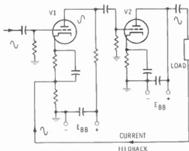
Fig. 10-5. Two-stage amplifier with current feedback.
