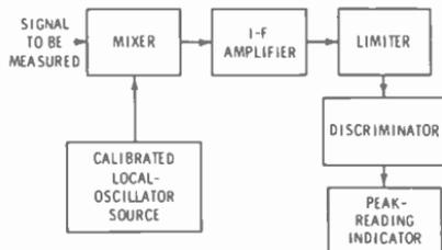
Fig. 14-11. Functional plan of an fm deviation meter.
