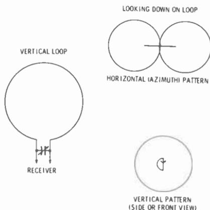
Fig 13-11 The loop antenna.
