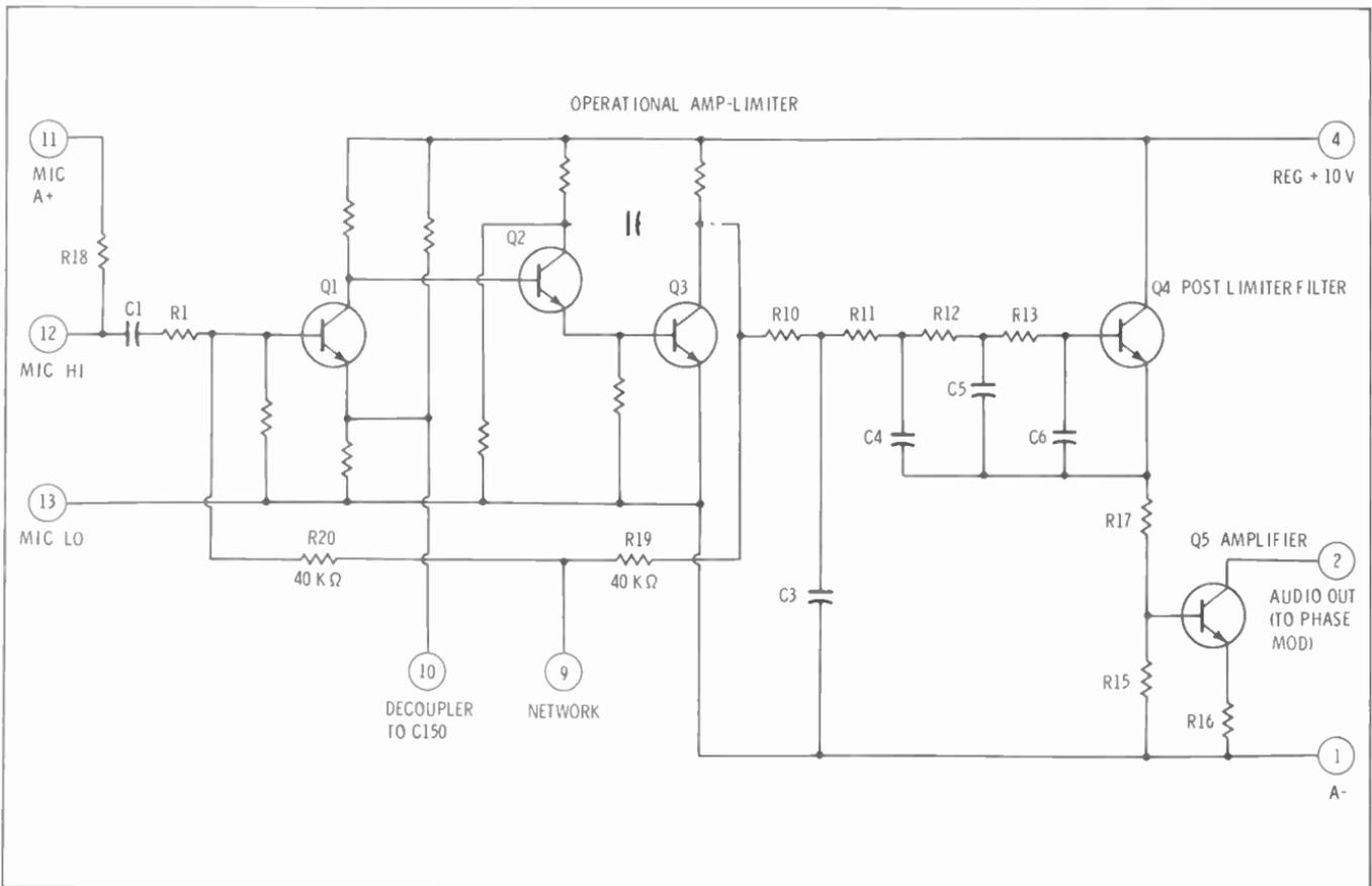
Fig. 4-10. Audio integrated circuit.
