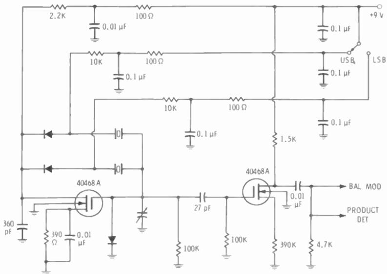
Fig. 4-17. Sideband carrier oscillator with usb-lsb diode switching.
