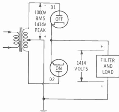
Fig. 9-7. Peak-inverse voltage across nonconducting tube of a full-wave rectifier.
