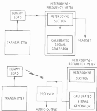
Fig. 12-7. Basic heterodyne-meter test arrangements.
