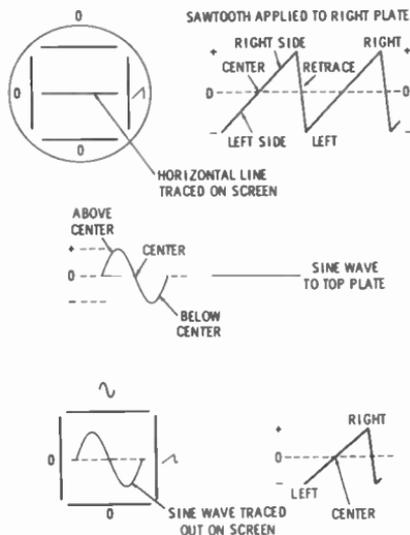
Fig. 14-6. Oscilloscope deflection waveforms and patterns.
