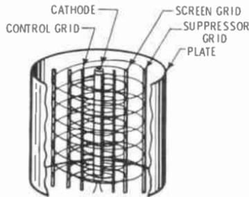
Fig. 8-4. Basic construction of a pentode power tube.
