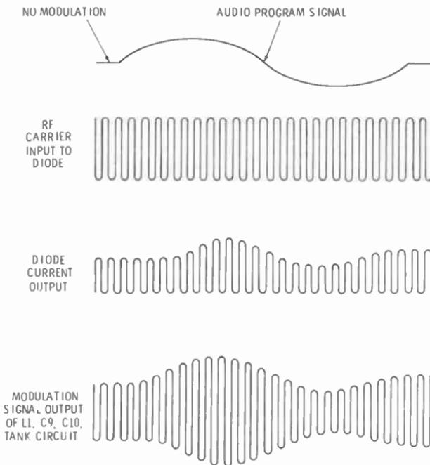
Fig. 5-15. Diode and diode-output tank-circuit waveform.
