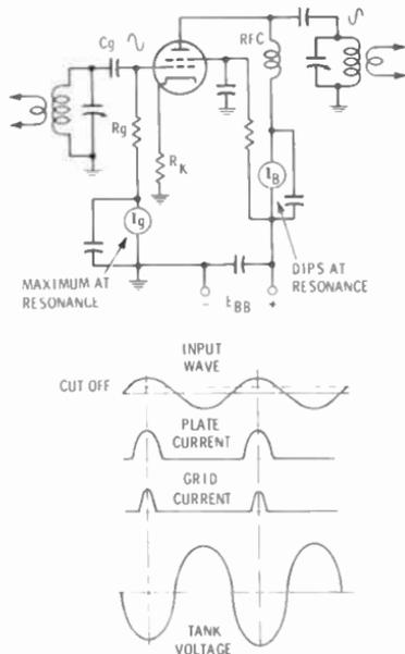
Fig. 10-12. Basic class-C amplifier.
