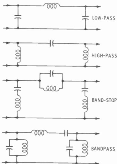
Fig. 7-2. Basic filter types.
