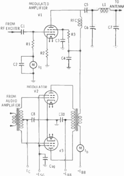
Fig. 11-5. High-level modulator.
