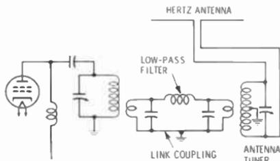
**Fig. 10-18.** Link-coupling arrangement to an antenna system.
