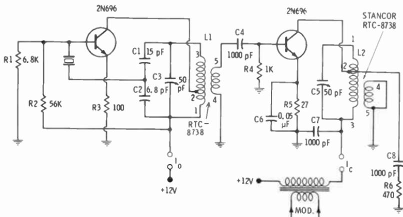
Fig. 14-23. Transistor crystal oscillator and class-C amplifier.
