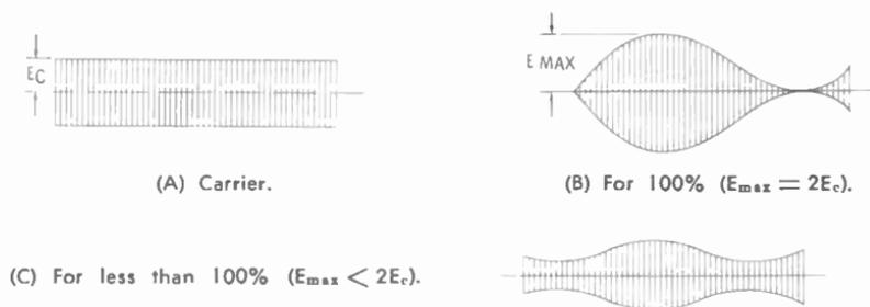
Fig. 4-23. Envelope check of modulation.
