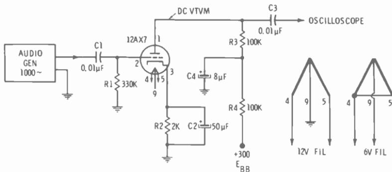
Fig. 14-14. Grounded-cathode amplifier.
