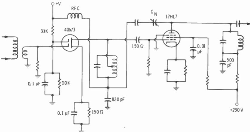
Fig. 4-21. MOSFET drive of vacuum-tube amplifier.
