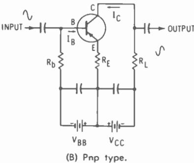
Fig. 8-21. Properly biased common-emitter stage.
