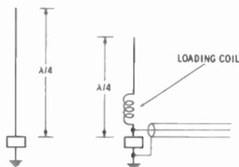
**Fig. 13-9.** Use of a loading coil to increase the electrical length of a short antenna.
