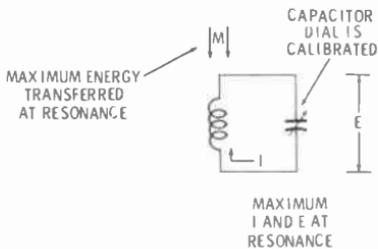
Fig. 3-1. Principle of the absorption wavemeter.
