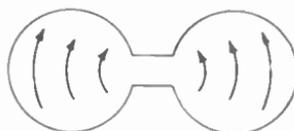
Fig. 13-5. Resonant cavity.
