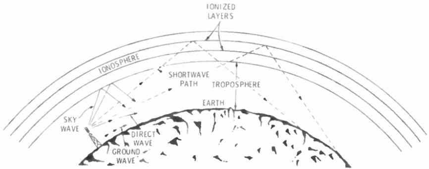
Fig. 2-1. Propagation of radio waves.
