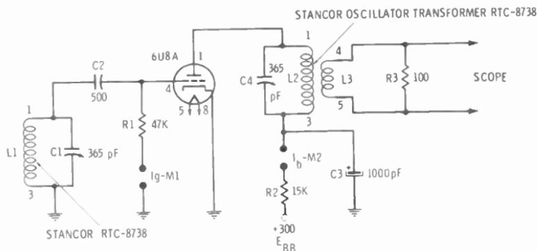
Fig. 14-17. Tuned-plate tuned-grid oscillator.
