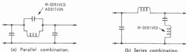
Fig. 7-1. Constant-K low-pass filter with M-derived section.
