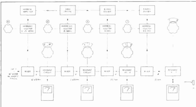
Fig. 3-15. Functional diagram of a divider-type frequency meter.
