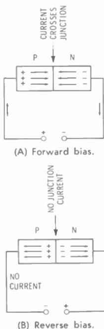
Fig. 8-19. The pn junction and its rectifier characteristics.
