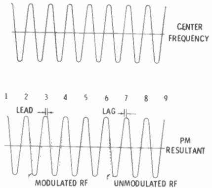
Fig. 12-3. The phase-modulated wave.
