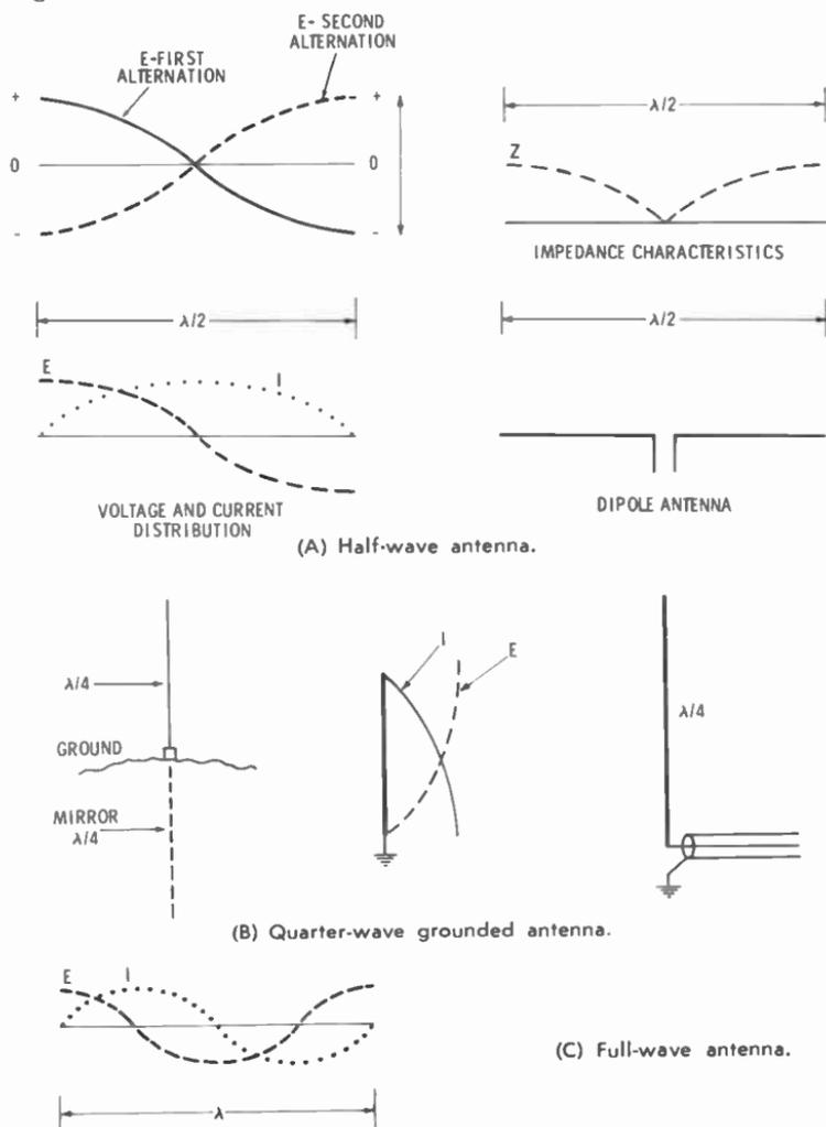
Fig. 13-6. Basic antennas, and voltage-current distribution.
