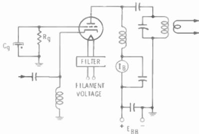
Fig. 10-13. Grounded-grid amplifier.
