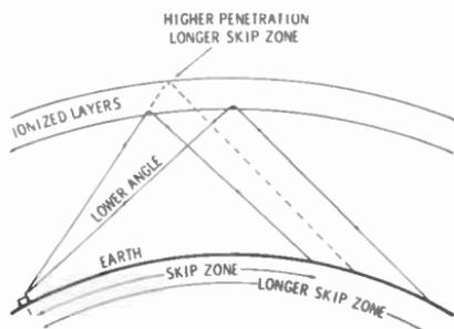
Fig. 13-14. Skip zone and radiation angle.
