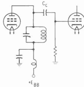
**Fig. 10-19.** Interstage capacitive coupling.
