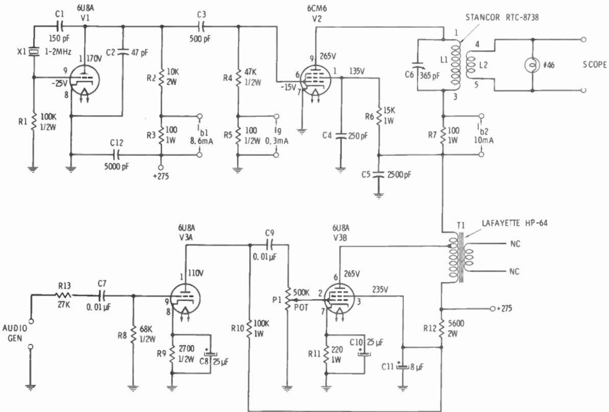
Fig. 14-19. An a-m transmitter.
