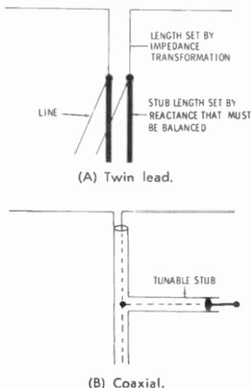
**Fig. 13-2.** Stub-tuning arrangements.
