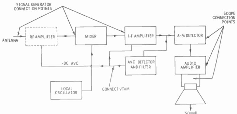
Fig. 11-10. Block diagram of an a-m receiver, showing test points.
