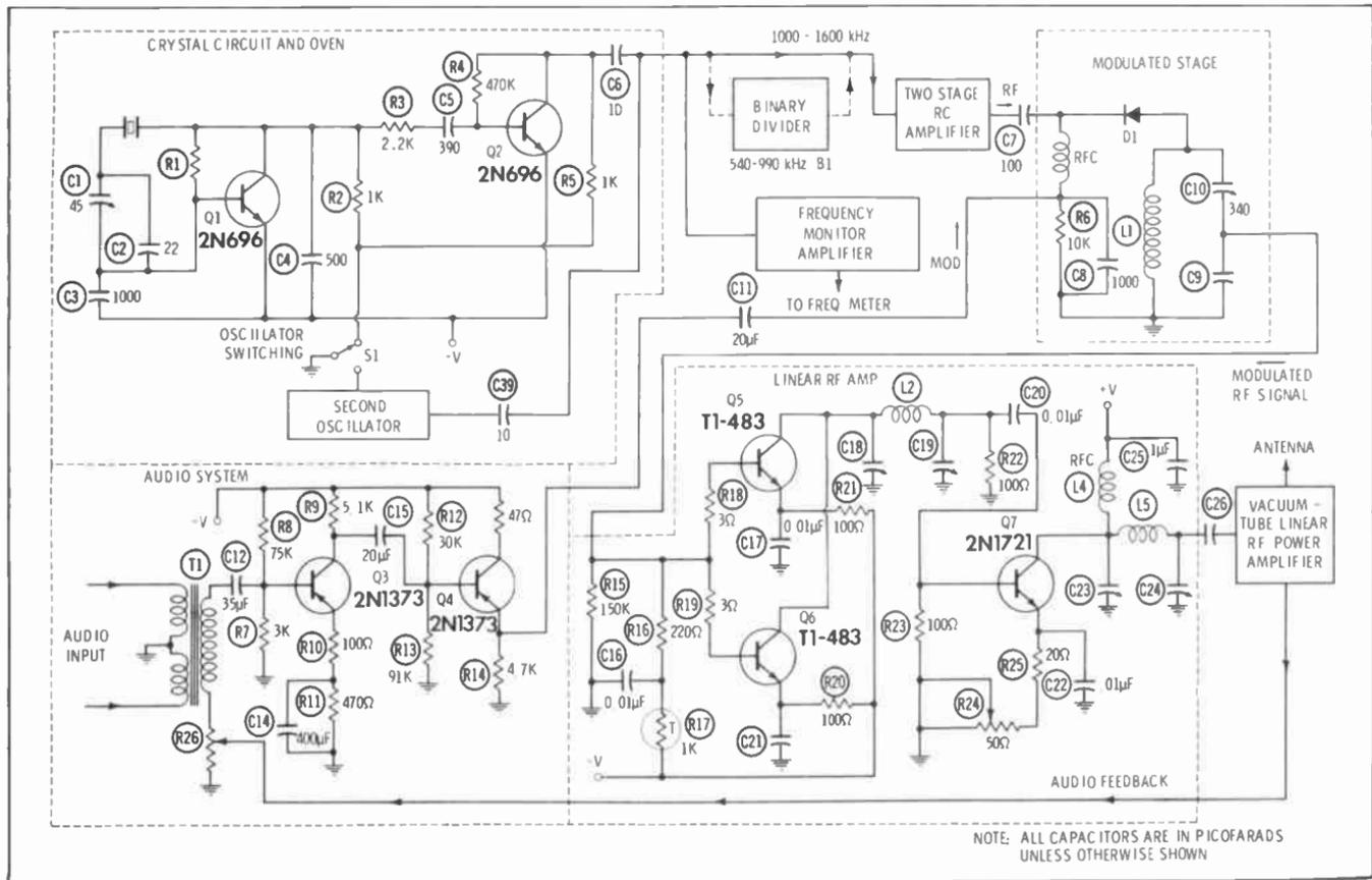
Fig. 5-13. Partial schematic of a solid-state transmitter.
