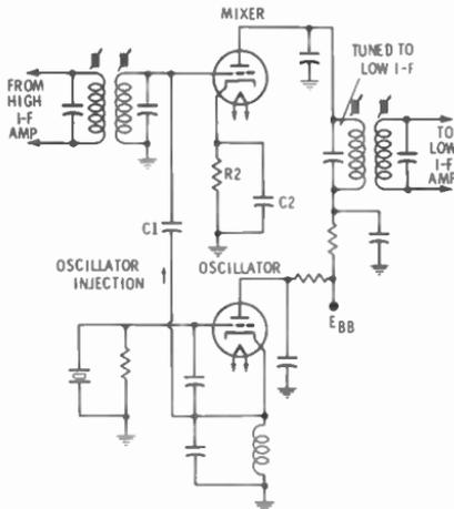
Fig. 12-8. A receiver second mixer/oscillator combination.
