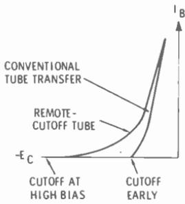
Fig. 8-7. Remote-cutoff operation.
