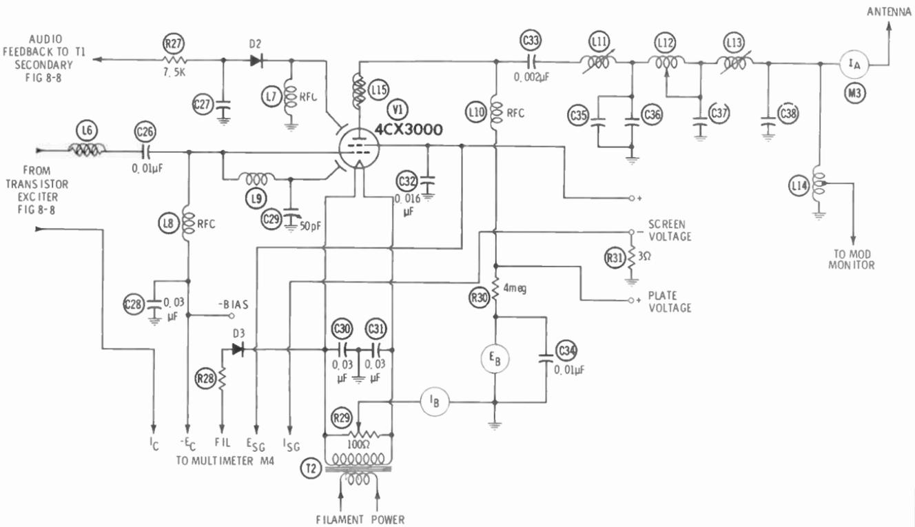
Fig. 5-16. A vacuum-tube power amplifier for a solid-state transmitter.
