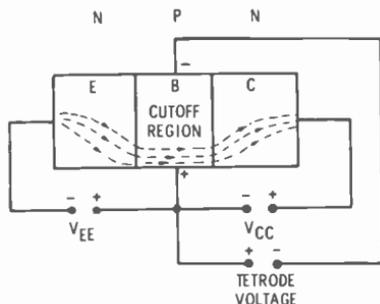
Fig. 8-29. Biasing and motion of carriers for a tetrode transistor.
