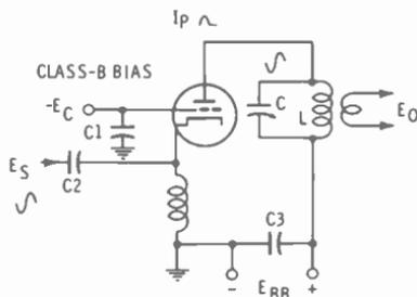
Fig. 8-12. Grounded-grid amplifier.
