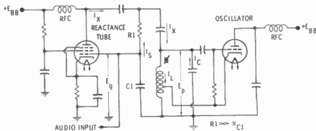
Fig. 12-1. Reactance-tube modulator.
