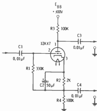
Fig. 14-16. Single-tube phase splitter.
