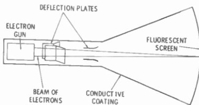
Fig. 14-4. Basic oscilloscope tube.
