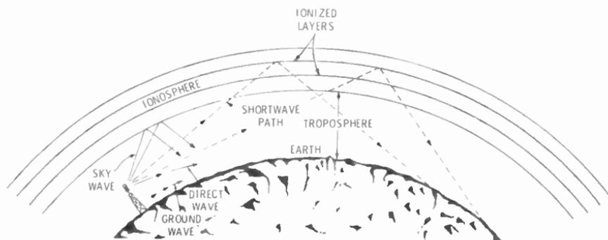
Fig. 2-1. Propagation of radio waves.
