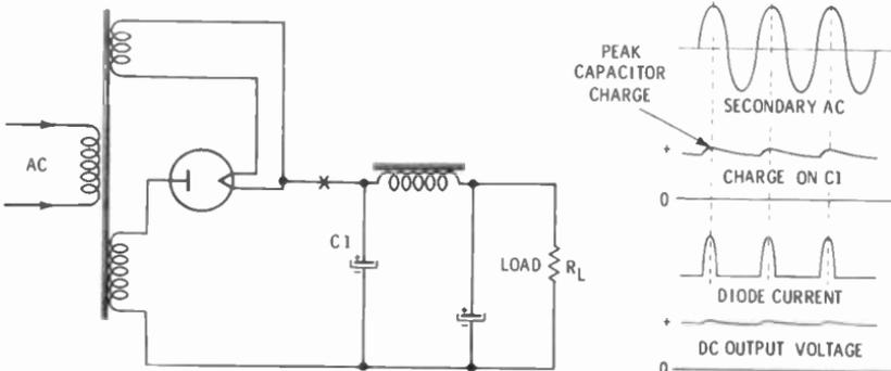
Fig. 9-2. Half-wave rectifier with capacitive-input filter.
