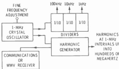
Fig. 14-9. Secondary-frequency standard.
