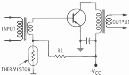
**Fig. 8-24.** Thermistor-stabilized bias system.
