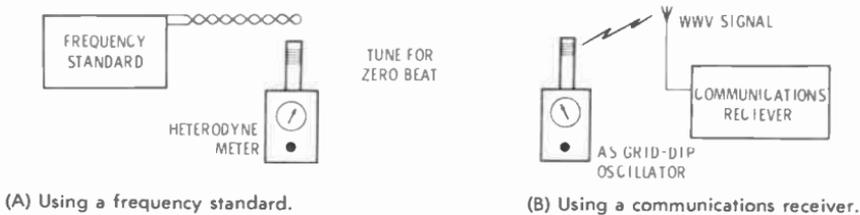
Fig. 3-8. Calibrating a grid-dip meter.
