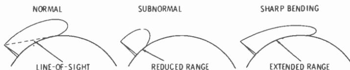
Fig. 2-2. Vhf propagation and tropospheric bending.
