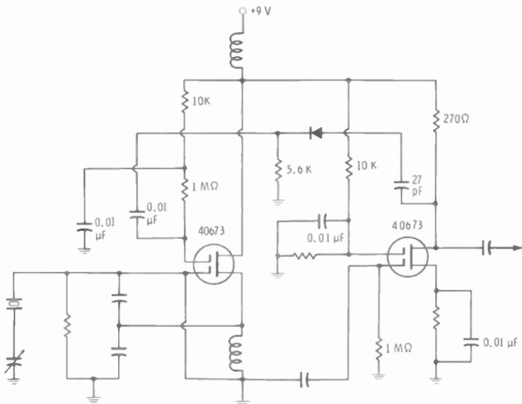
Fig. 4-18. Untuned wide-range hf oscillator.
