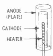
Fig. 8-1. Diode-tube construction.
