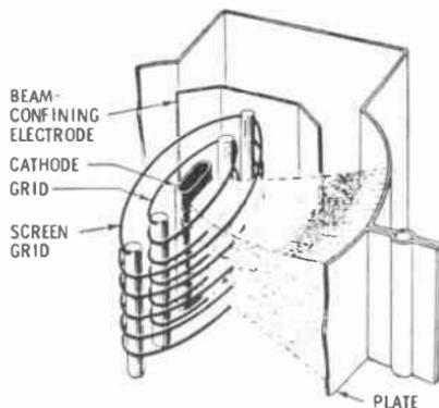
Fig. 8-6. Basic construction of a beam-power tube.
