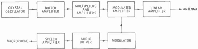
Fig. 11-3. Block diagram of an a-m transmitter.
