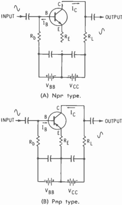
Fig. 8-21. Properly biased common-emitter stage.
