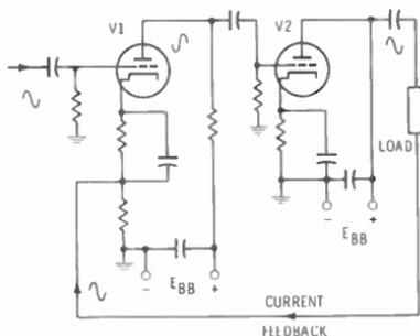
Fig. 10-5. Two-stage amplifier with current feedback.
