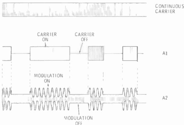
Fig. 2-7. A1 and A2 code transmission—Morse code letter L as an example.
