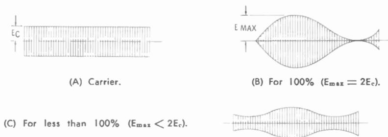
Fig. 4-23. Envelope check of modulation.
