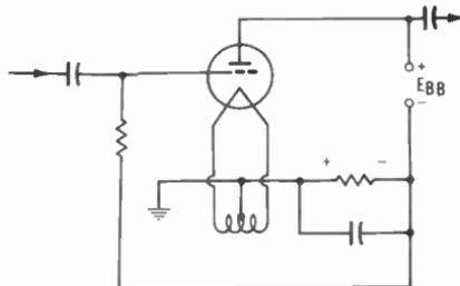
Fig. 10-2. Biasing a tube from the plate circuit resistor.
