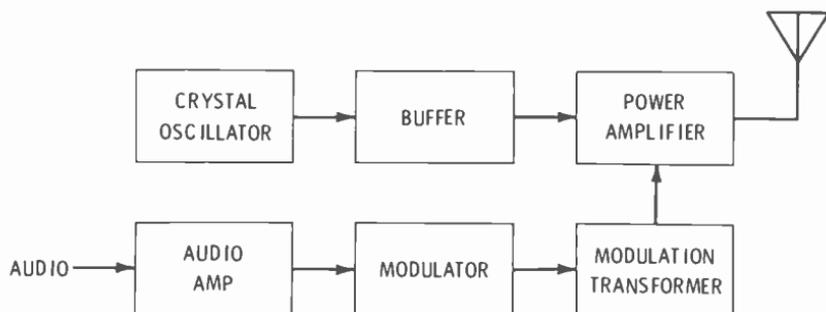
Fig. 5-6. Functional plan of an a-m broadcast transmitter.
