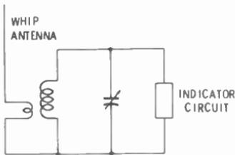
Fig. 3-4. Use of the wavemeter principle in an rf indicator.
