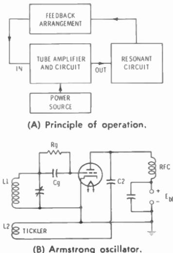
Fig. 10-22. Oscillator principle and circuit.
