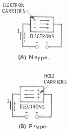
Fig. 8-18. P- and n-type semiconductors.
