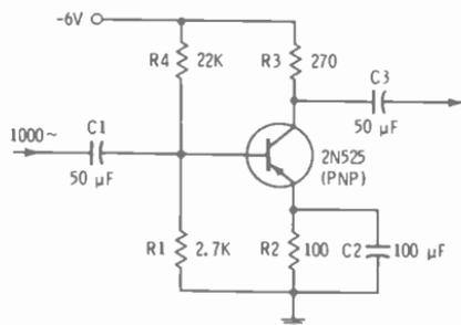
Fig. 14-20. Common-emitter stage.
