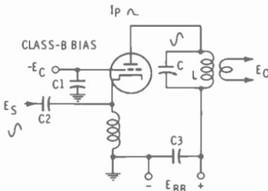
Fig. 8-12. Grounded-grid amplifier.
