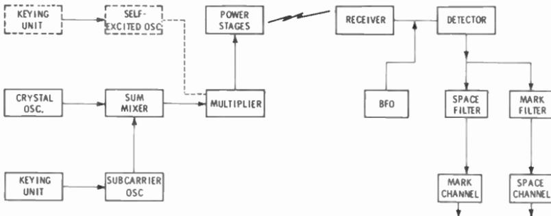
Fig. 12-15. FSK transmission system.
