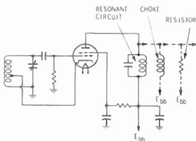
Fig. 10-27. Electron-coupled oscillator.
