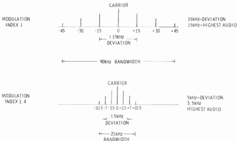
Fig. 2-6. Fm sideband and distribution as influenced by the modulation index.
