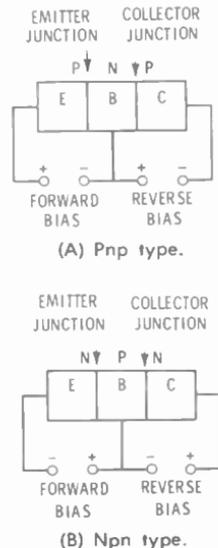
Fig. 8-20. Normal biasing of transistors.
