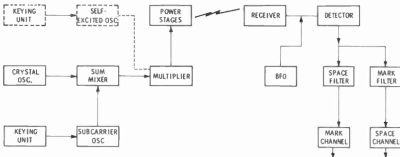
Fig. 12-15. FSK transmission system.
