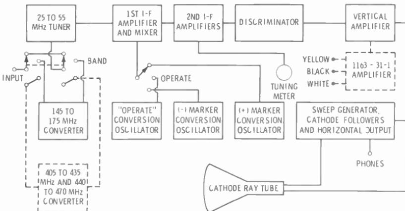
**Fig. 3-22. Functional block plan of the deviation meter in Fig. 3-21.**
