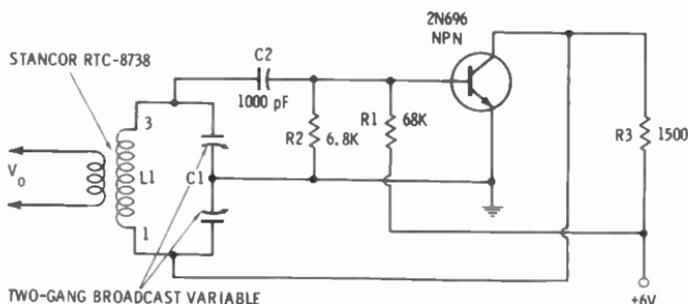
Fig. 14-22. Colpitts transistor oscillator.
