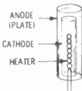
Fig. 8-1. Diode-tube construction.
