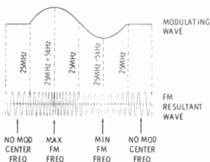
Fig. 2-5. Basic fm wave with a 25-MHz carrier.
