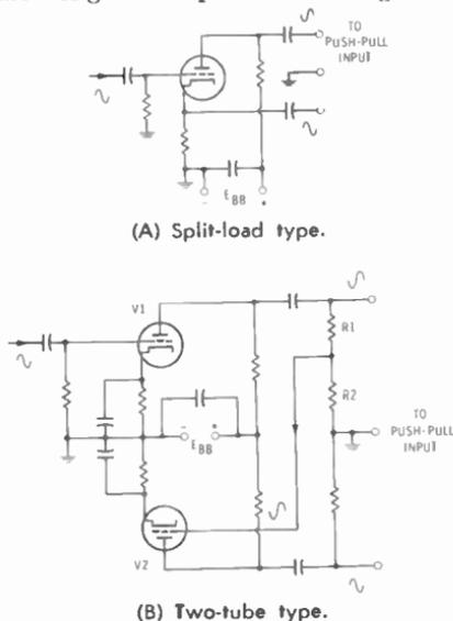
Fig. 10-4. Phase inverters.
