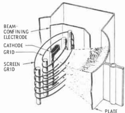
Fig. 8-6. Basic construction of a beam-power tube.
