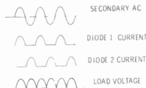
Fig. 9-3. Full-wave rectifier with a choke-input filter.
