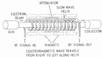
**Fig. 10-32. Traveling wave tube.**
