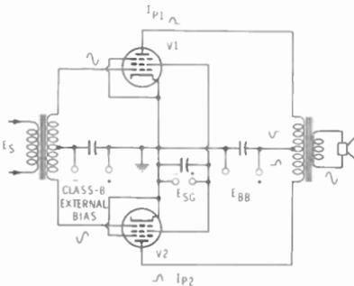
Fig. 8-14. Pentode push-pull class-B amplifier stage.
