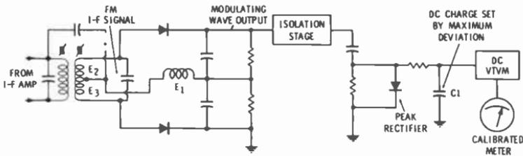
Fig. 14-12. An fm discriminator and peak voltmeter.
