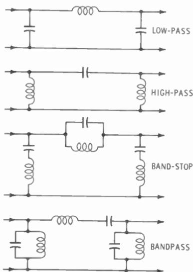
Fig. 7-2. Basic filter types.
