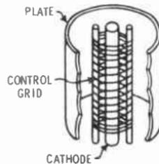
Fig. 8-2. Basic construction of a triode tube.
