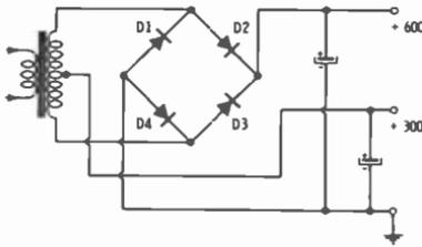
Fig. 9-8. Obtaining two differing voltages from a single supply.
