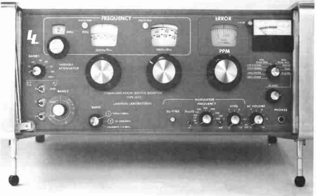
Fig. 3-16. Frequency- and fm deviation monitor.
