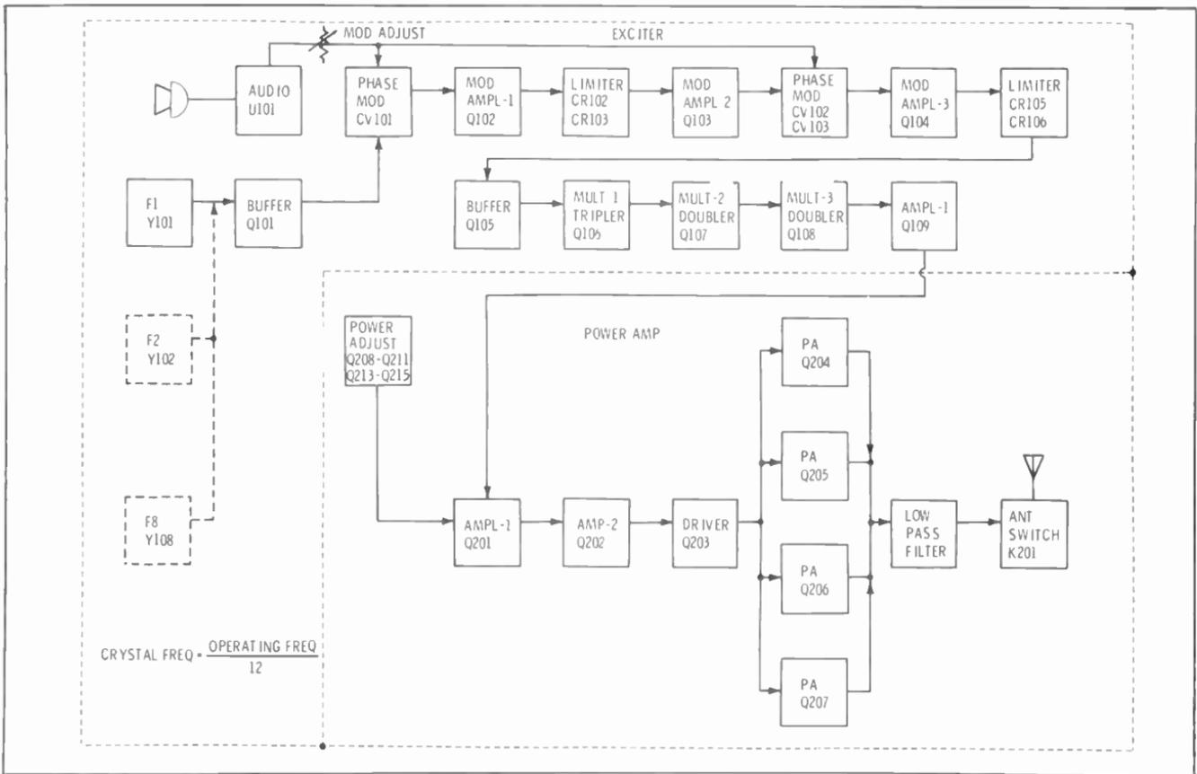
Fig. 4-8. Functional block diagram of the transmitter of Fig. 4-7.
