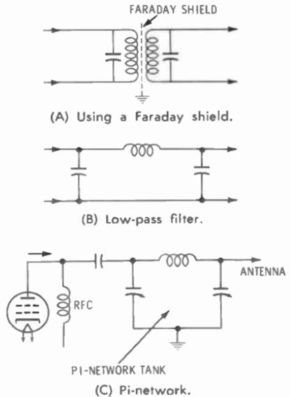
Fig. 11-2. Coupling systems that are used to reduce harmonics.
