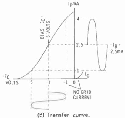
Fig. 8-10. Typical grounded-cathode stage.
