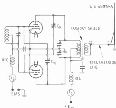
Fig. 10-14. Push-pull amplifier with plate cross-neutralization and grounded quarter-wave antenna
