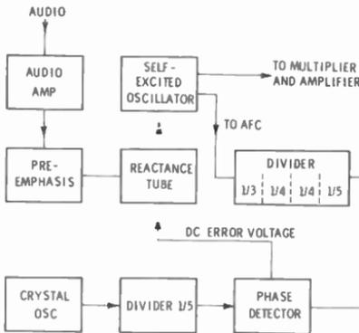
Fig. 12-2. AFC system used to stabilize the reactance-tube modulator.
