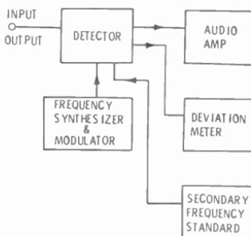
Fig. 3-17. Block plan for frequency and deviation meter.
