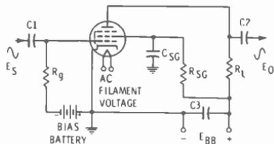
Fig. 8-11. Pentode grounded-cathode amplifier stage.
