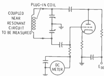
Fig. 14-8. Grid-dip meter.
