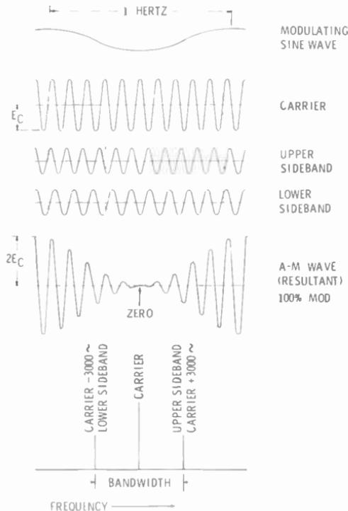
Fig. 2-3. The formation of an a-m wave.
