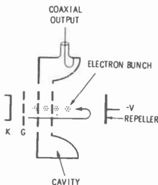
Fig. 10-30. Klystron oscillator.
