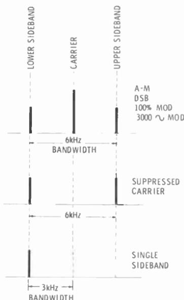
Fig. 2-4. Suppressed-carrier and single-sideband transmission.
