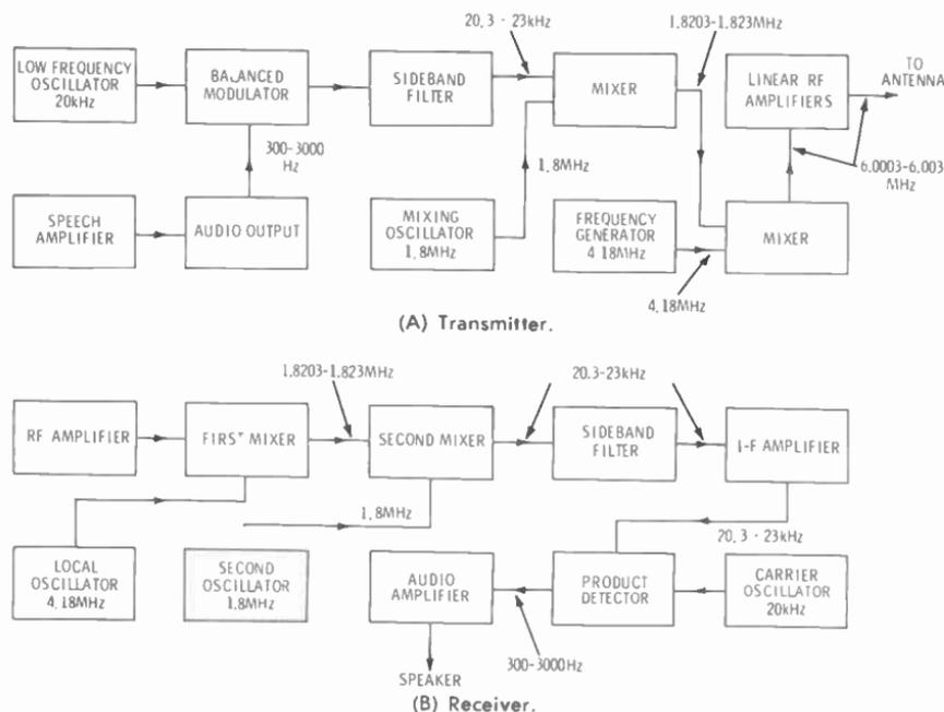
Fig. 11-9. The functional plan of an sssc system.
