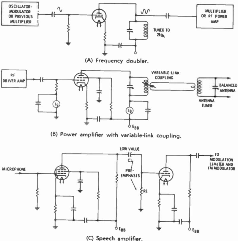
Fig. 12-5. Stages of a phase-modulated fm transmitter.
