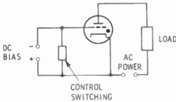
Fig. 8-9. Thyatron control circuit.
