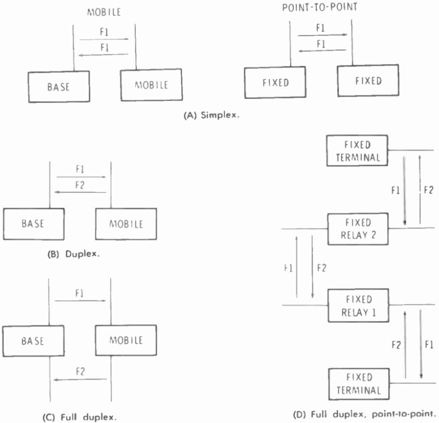
Fig. 1-1. Two-way radio systems.
