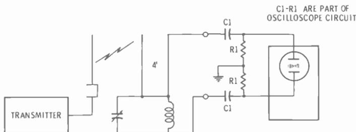
Fig. 4-22. Simple modulation-envelope check method.
