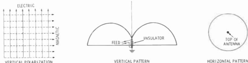
**Fig. 13-7.** Fields and patterns of a quarter-wave vertical antenna.
