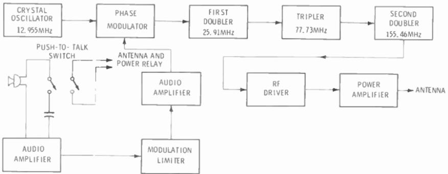
Fig. 12-6. Phase-modulated fm transmitter.
