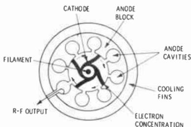
Fig. 10-31. Magnetron oscillator.
