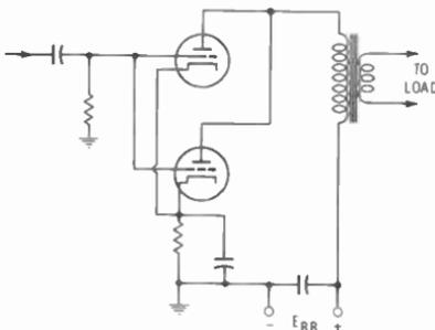
Fig. 10-6. Two triode tubes connected in a parallel arrangement.
