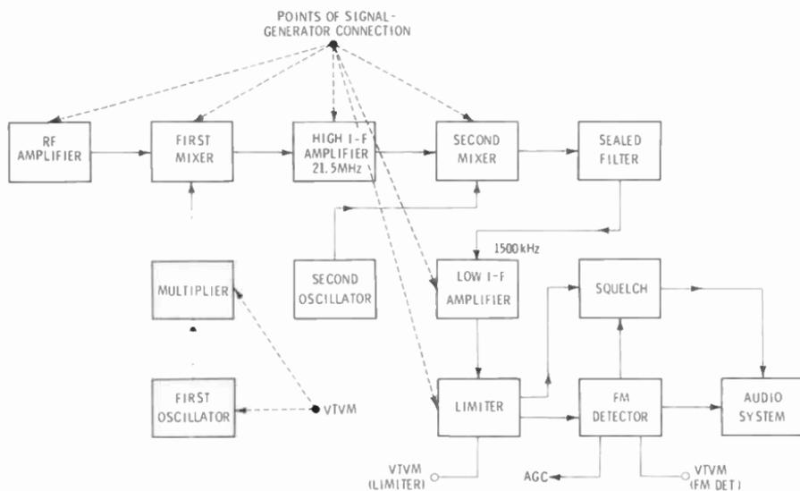
Fig. 12-13. Block diagram of a double-conversion receiver, with alignment points.
