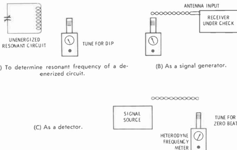
Fig. 3-7. Using the grid-dip meter.
