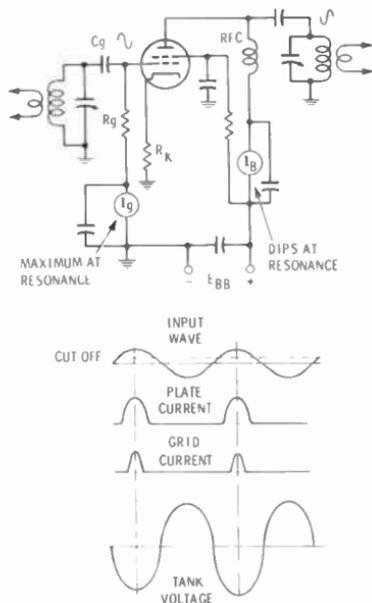
Fig. 10-12. Basic class-C amplifier.
