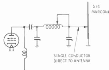
**Fig. 10-20.** Single-line direct coupling to a Marconi antenna.
