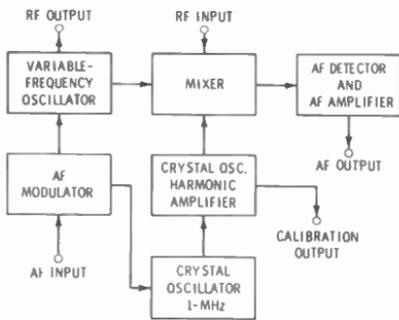
Fig. 14-10. Functional plan of a heterodyne-frequency meter.
