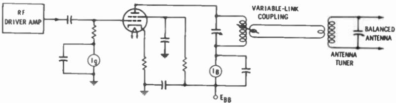
(B) Power amplifier with variable-link coupling.
