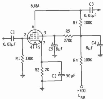
Fig. 14-15. Pentode grounded-cathode amplifier circuit.
