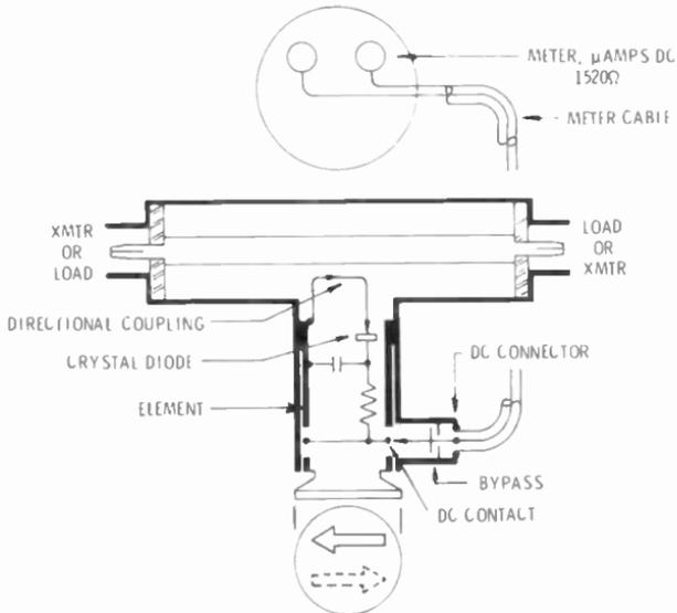
Fig. 3-12. Circuit of an rf wattmeter.
