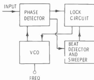
Fig. 3-19. Phase-locked loop plan.
