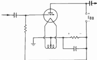
Fig. 10-2. Biasing a tube from the plate circuit resistor.
