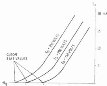
Fig. 8-16.  $I_p - E_g$  characteristics of a triode.
