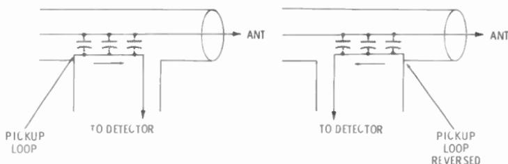
Fig. 3-13. Principle of a reflectometer.
