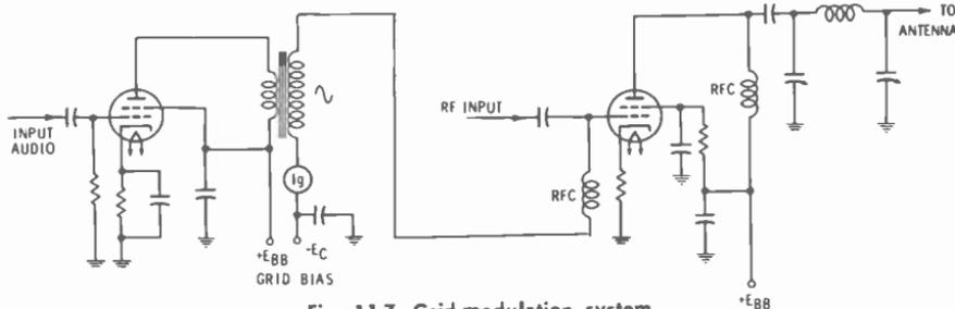
Fig. 11-7. Grid-modulation system.
