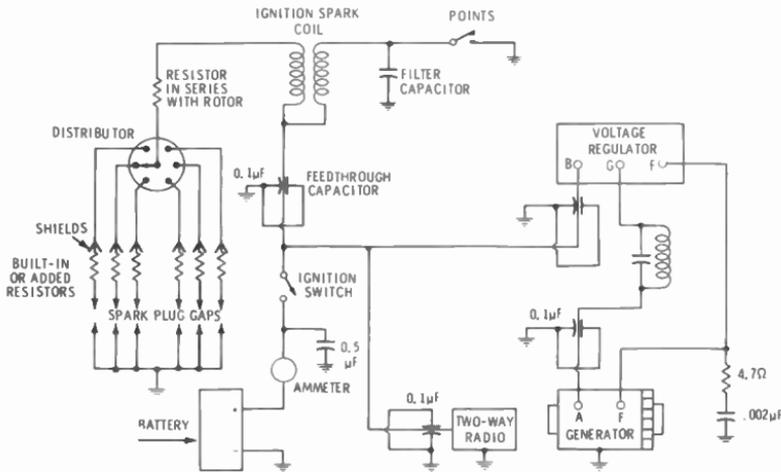
Fig. 12-14. Noise-reduction methods.
