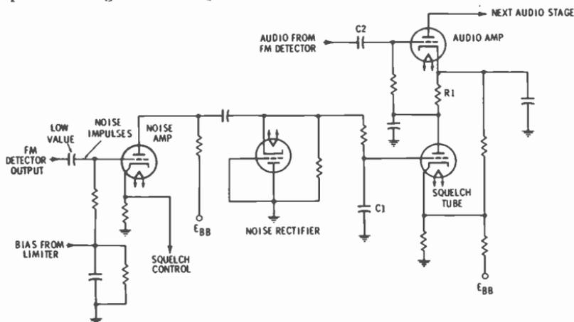
Fig. 12-11. Differential-squelch circuit.
