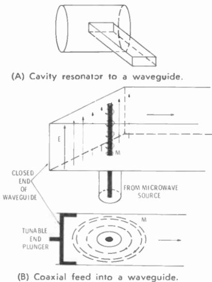
Fig. 13-4. Coupling microwave energy to a waveguide.
