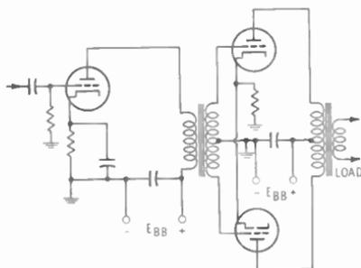
Fig. 10-8. Single-ended drive of a push-pull amplifier using an input transformer.
