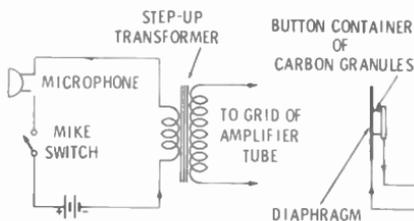
Fig. 10-10. Carbon-microphone circuit.
