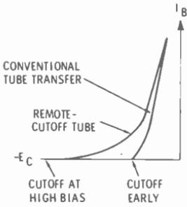
Fig. 8-7. Remote-cutoff operation.
