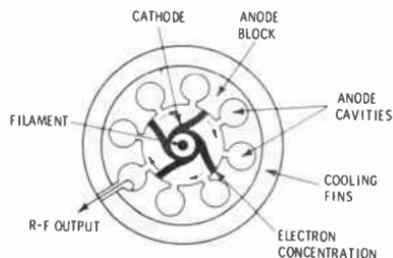
Fig. 10-31. Magnetron oscillator.
