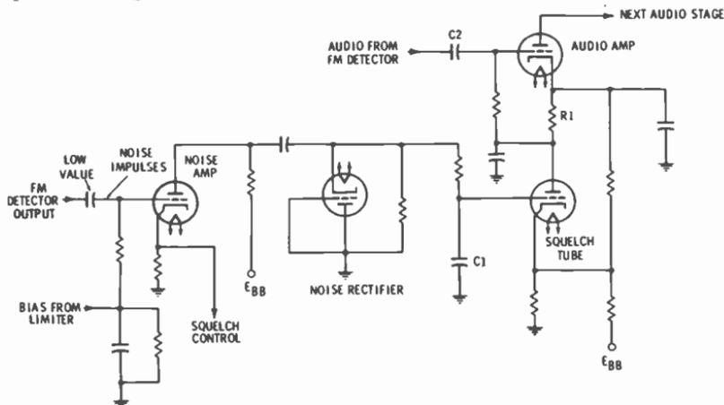
Fig. 12-11. Differential-squelch circuit.
