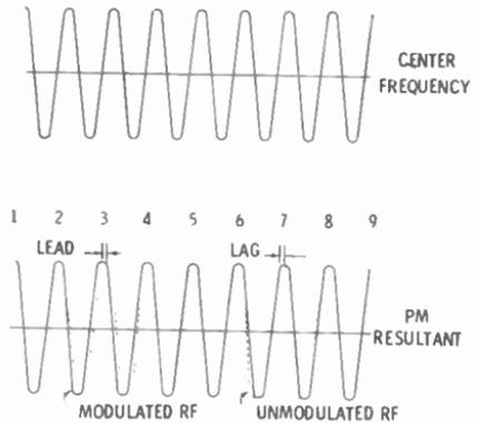
Fig. 12-3. The phase-modulated wave.
