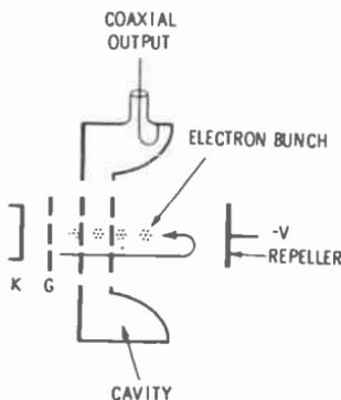
Fig. 10-30. Klystron oscillator.
