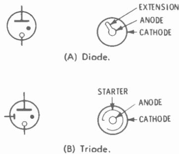
Fig. 8-8. Cold-cathode tubes.
