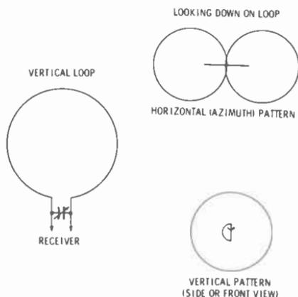
Fig 13-11 The loop antenna.
