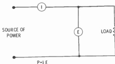
Fig. 14-3. Using an ammeter and voltmeter for power measurement.
