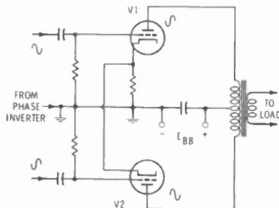
Fig. 10-7. Push-pull class-A amplifier.
