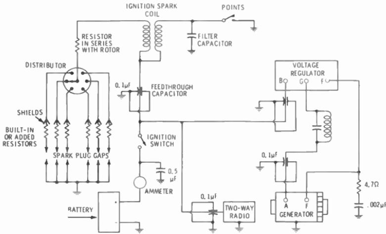
Fig. 12-14. Noise-reduction methods.
