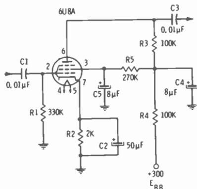
Fig. 14-15. Pentode grounded-cathode amplifier circuit.
