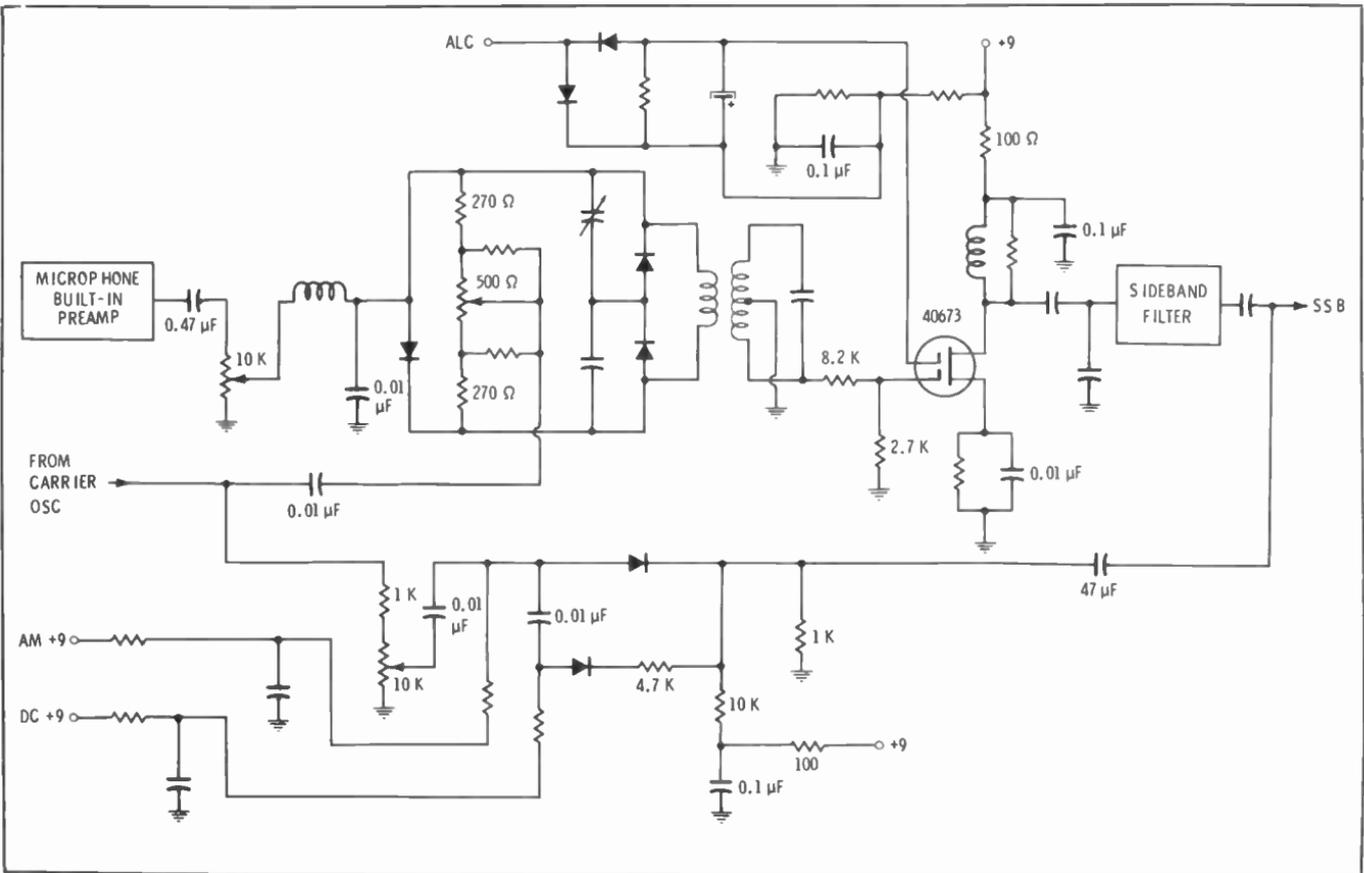
Fig. 4-19. Balanced modulator and sideband filter.
