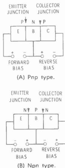
Fig. 8-20. Normal biasing of transistors.
