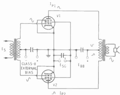
Fig. 8-14. Pentode push-pull class-B amplifier stage.
