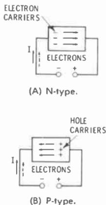
Fig. 8-18. P- and n-type semiconductors.
