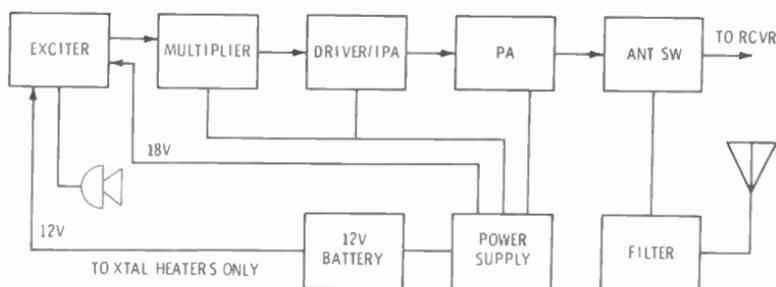
Fig. 4-4. Block diagram of transmitter, power supply, and exciter.
