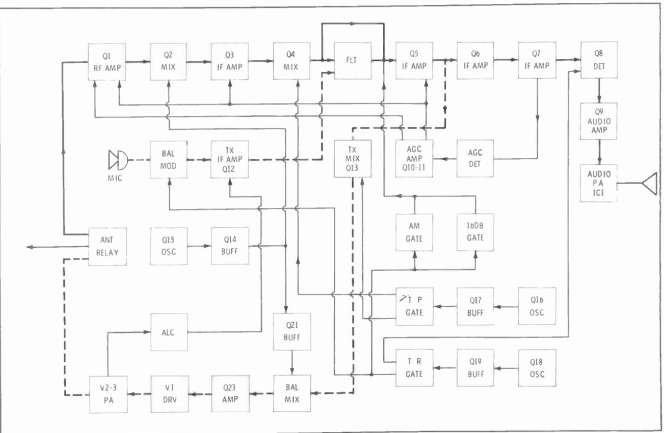
Fig. 4-16. Sideband transceiver block diagram.
