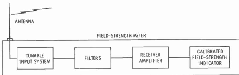
Fig. 14-13. Field-strength meter arrangement for measuring harmonics.
