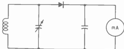
Fig. 14-7. Absorption wavemeter.
