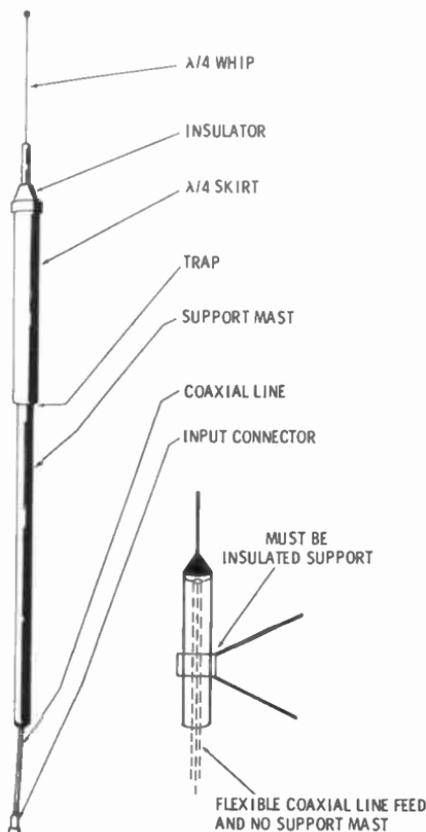
**Fig. 13-10.** Coaxial antenna.
