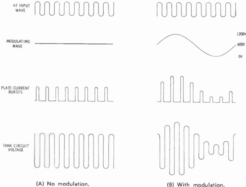
Fig. 11-6. The a-m modulation process in waveforms.
