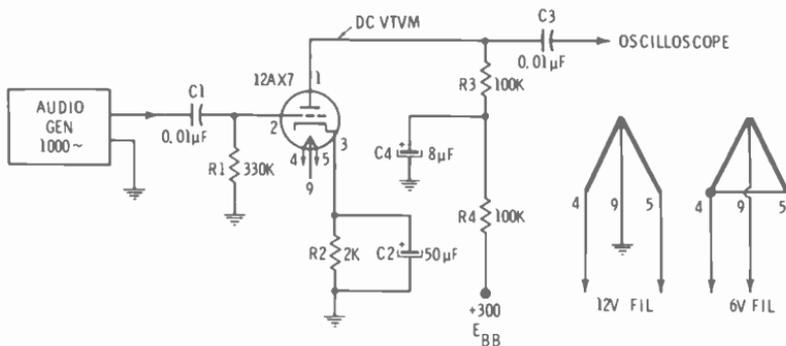
Fig. 14-14. Grounded-cathode amplifier.
