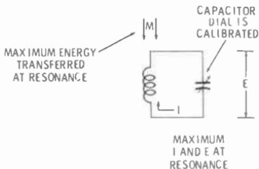
Fig. 3-1. Principle of the absorption wavemeter.
