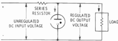
Fig. 9-1. Voltage-regulator circuit.
