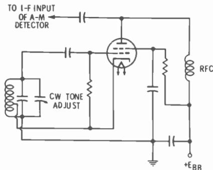
Fig. 11-12. Bfo circuit.
