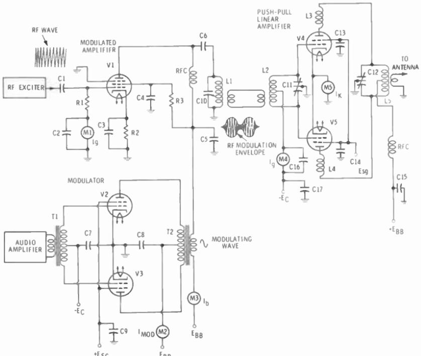
Fig. 11-4. Low-level plate-modulated amplifier and linear-output amplifier.
