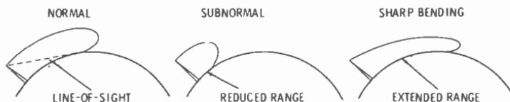
Fig. 2-2. Vhf propagation and tropospheric bending.
