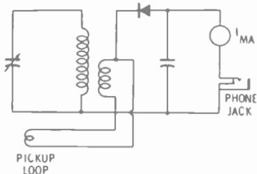
Fig. 3-3. Absorption wavemeter with pickup loop and phone jack.
