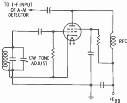
Fig. 11-12. Bfo circuit.
