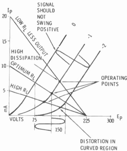
Fig. 8-15. Load lines on triode characteristics curve.
