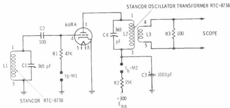
Fig. 14-17. Tuned-plate tuned-grid oscillator.
