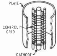
Fig. 8-2. Basic construction of a triode tube.
