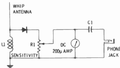
Fig. 3-5. A typical rf field indicator.
