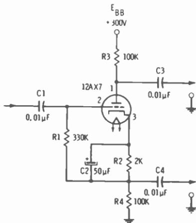
Fig. 14-16. Single-tube phase splitter.
