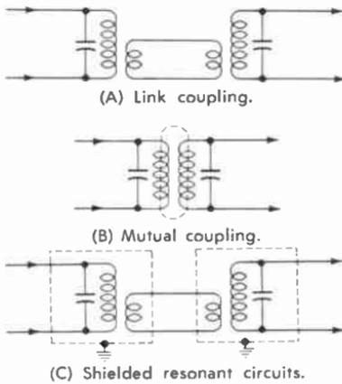
Fig. 11-1. Coupling arrangements.
