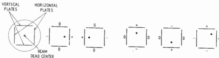
Fig. 14-5. Position of beam impact on fluorescent screen as a function of plate polarities.
