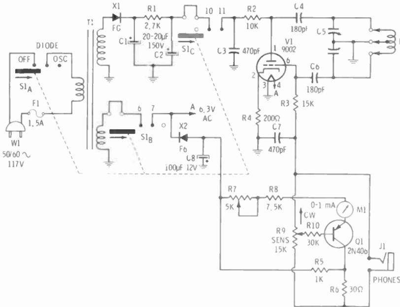
Fig. 3-6. Millen grid-dip oscillator.
