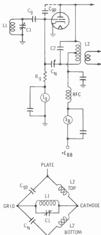
Fig. 10-15. Plate-neutralization system.
