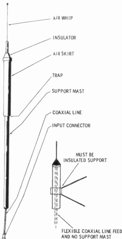
**Fig. 13-10.** Coaxial antenna.
