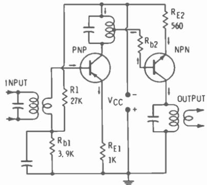
Fig. 8-28. Direct-coupled amplifier.
