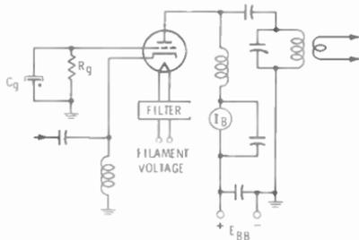
Fig. 10-13. Grounded-grid amplifier.
