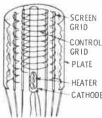
Fig. 8-3. Basic construction of a tetrode tube.
