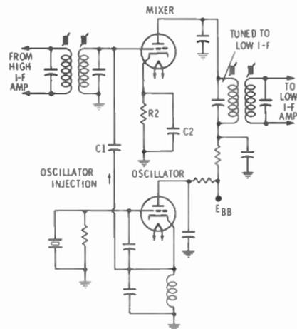
Fig. 12-8. A receiver second mixer/oscillator combination.
