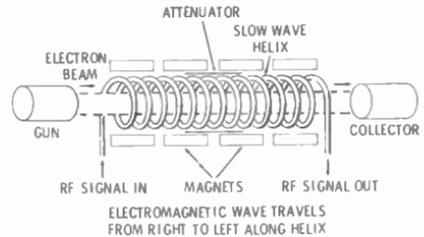
**Fig. 10-32. Traveling wave tube.**
