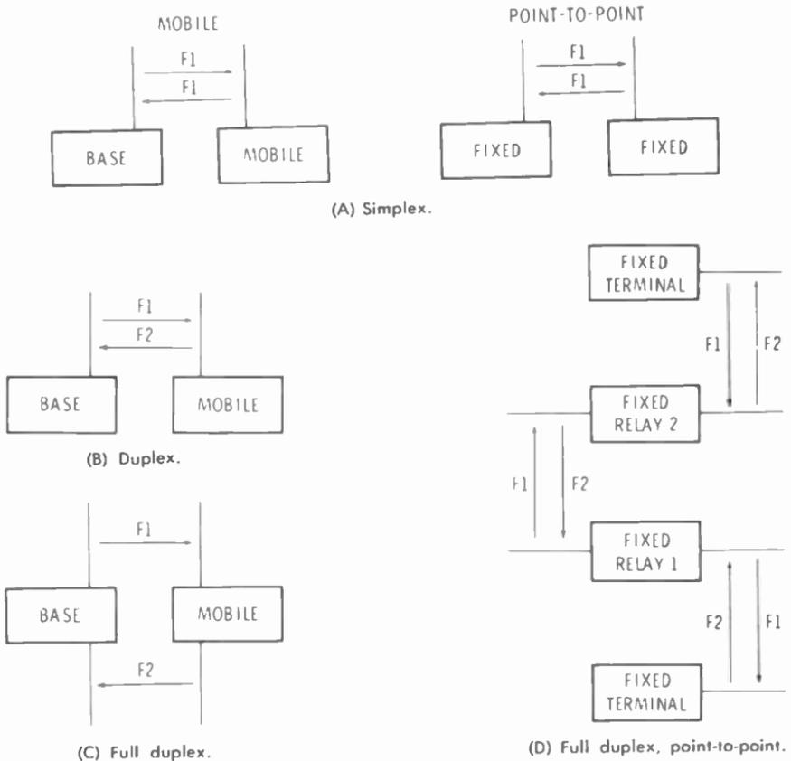
Fig. 1-1. Two-way radio systems.
