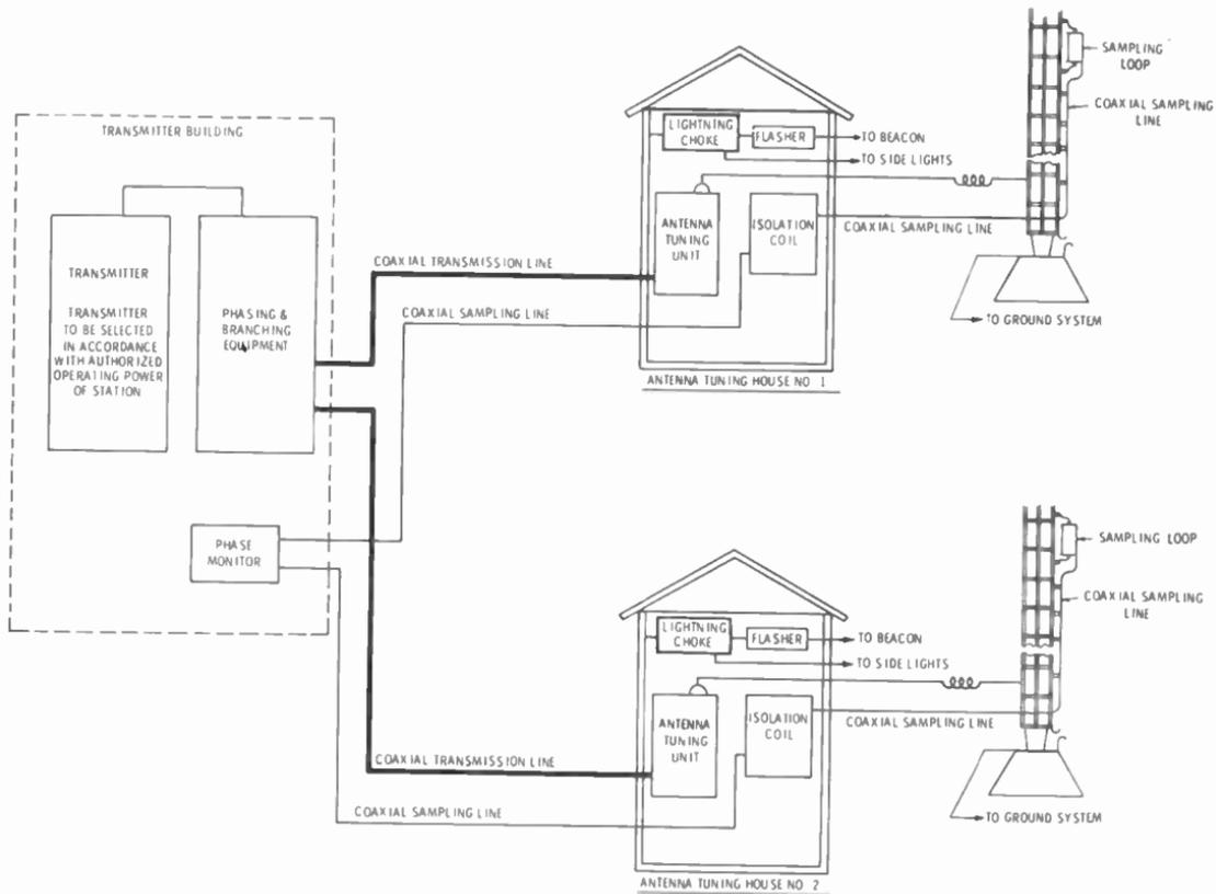
Fig. 5-18. The major units of a directional antenna system.
