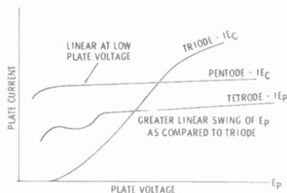
Fig. 8-5. Characteristics of triode, tetrode, and pentode tubes.
