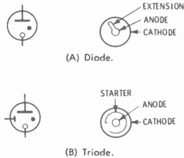
Fig. 8-8. Cold-cathode tubes.
