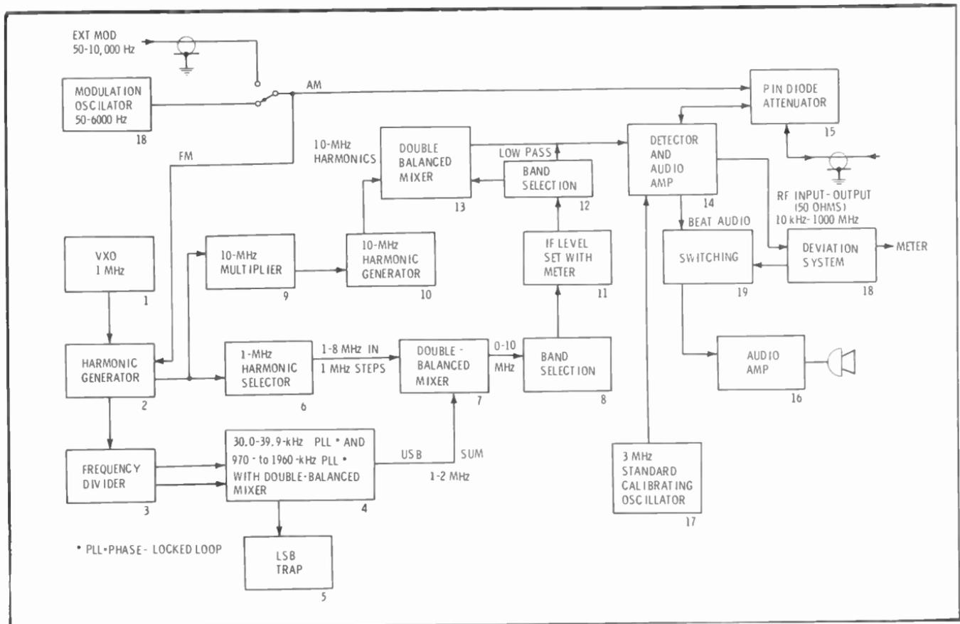
Fig. 3-18. Simplified functional block diagram of a frequency synthesizer.
