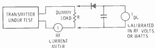
Fig. 3-9. Rf power measurement.
